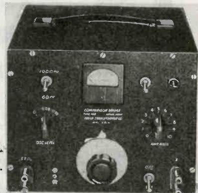
calibrated dial indicates the percentage difference between the unknown and the standard. The comparison bridge is supplied with three frequencies of 60, 1,000 and 10,000 cycles. Components being compared to a similar standard range are: capacitors 25  $\mu\text{f}$  to 20  $\mu\text{f}$ ; inductors 5 microhenries to 500 henries, resistors from 10 ohms to 5 megohms. The instrument measures  $10 \times 7\frac{1}{2} \times 8\frac{1}{2}$  in.
