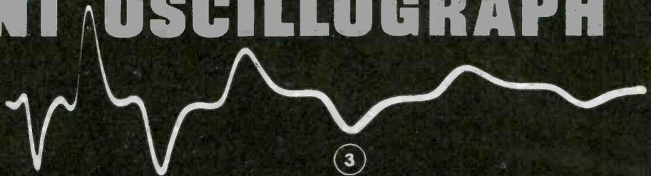
◆ The quickest method for determining co-ax line characteristics is that of applying a pulse to one end and observing reflections that follow. Type 248 Oscillograph, providing high-speed driven sweep and self-contained pulse generator, has proved invaluable for such work in our own laboratories and at the DuMont New York Television Station WABD.
