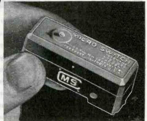
The basic Micro Switch is a thumb-size, feather-light, plastic enclosed, precision, snap-acting switch. Underwriters' listed and rated at 1200 V.A. at 125 to 460 volts a-c. Capacity on d-c depends on load characteristics. Accurate reproducibility of performance is maintained over millions of operations. Basic switches of different characteristics are combined with various actuators and metal housings to meet a wide range of requirements.
