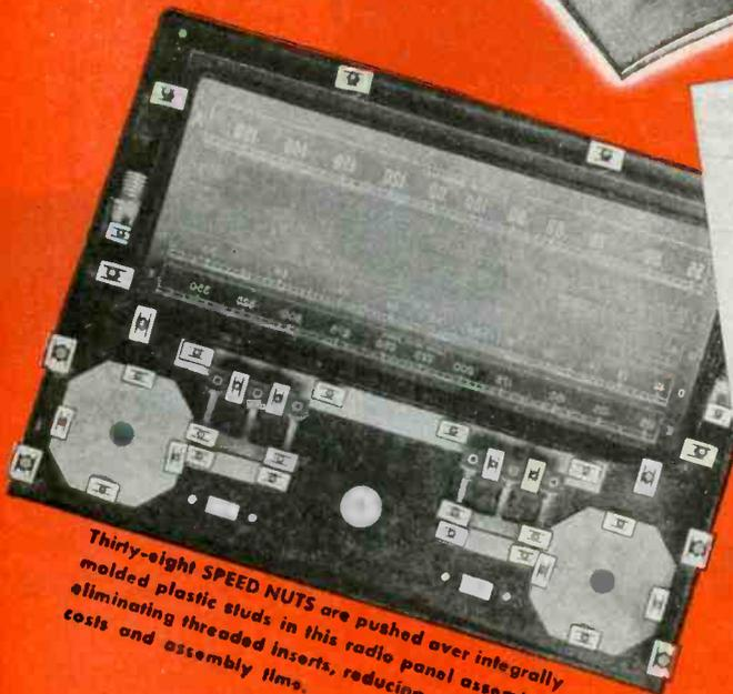
Thirty-eight SPEED NUTS are pushed over integrally molded plastic studs in this radio panel assembly, eliminating threaded inserts, reducing mold costs and assembly time.
