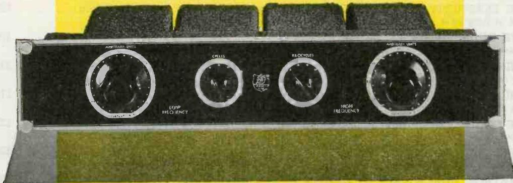
**3AX** . . . THE UNIVERSAL EQUALIZER FOR BROADCAST AND RECORDING SERVICE. PROVIDES ADJUSTABLE EQUALIZATION AT 25, 50, OR 100 CYCLES FOR LOW END, AND AT 4000, 6000, 8000, OR 10,000 CYCLES AT HIGH END. CALIBRATED CONTROLS READ DIRECTLY IN DB EQUALIZATION AND FREQUENCY SETTING. THE INSERTION LOSS EFFECTED BY THE EQUALIZER IS COMPENSATED THROUGH SPECIAL COMPENSATING PADS, SO THAT IT IS CONSTANT REGARDLESS OF SETTING. RAPID CHANGE IN TONE COLOR CAN BE OBTAINED WITH NEGLIGIBLE CHANGE IN VOLUME.
