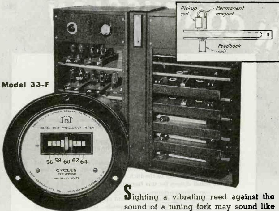
**S**ighting a vibrating reed against the sound of a tuning fork may sound like double talk . . . but that is essentially the principle in the exacting process of J-B-T Frequency Meter calibration.
