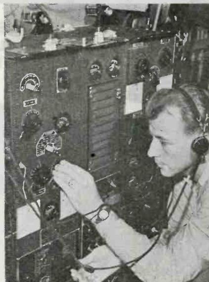
An intermediate-frequency transmitter is tuned by the radioman in the training mock-up of the forward section of a PBM-3 Mariner. All equipment operates normally, as does intercom system
