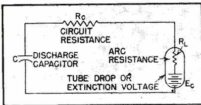
FIG. 9—Equivalent circuit of a gaseous discharge tube
