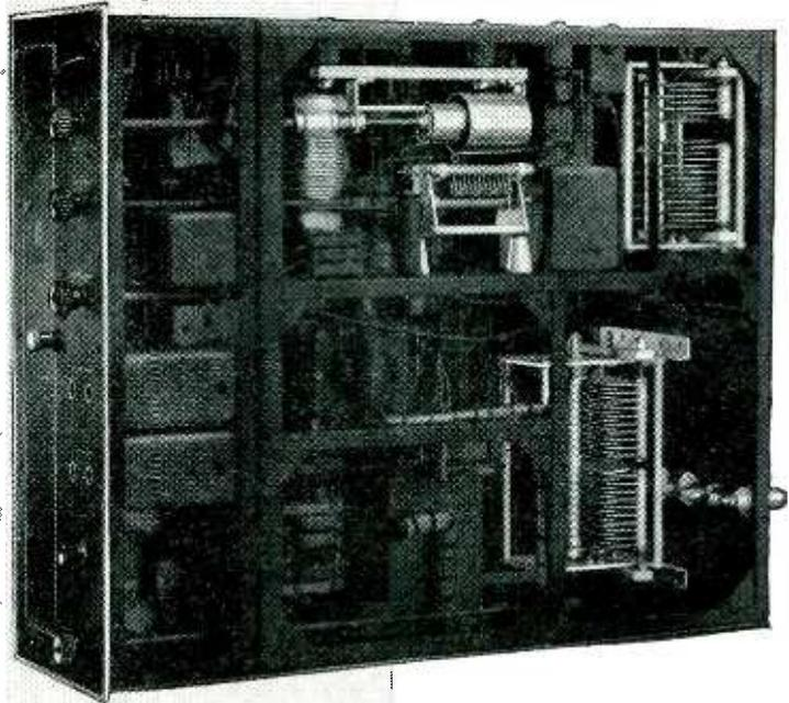
The new Wilcox 99A, medium power, transmitter designed primarily for airline fixed communication service, is provided with features including four removable radio frequency channels in the low, high and very high frequency ranges.
