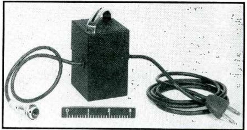
Miniature battery charger for the sensory aid unit. This is operated from ordinary 115 v a-c mains
