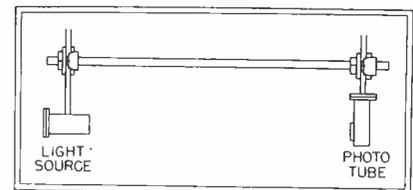
Fig. 1—The distance between the light source and the phototube was made as large as conveniently possible for use from a small boat
