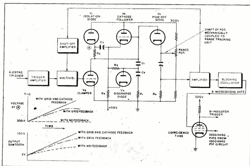
FIG. 7—Block diagram and simplified schematic of range delay circuit
