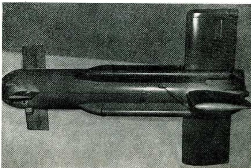
Radio controlled, rocket powered bomb being developed at the close of the war was to be launched from shipboard. It would race straight upward for 10,000 ft at 400 mph. A proximity fuse would detonate the 100-lb. general purpose charge if the bomb approached its target
