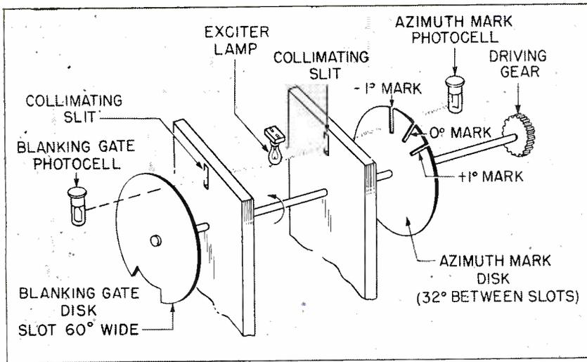
FIG. 11—Photo-mechanical system for producing azimuth marks and blanking pulses as antenna rotates
