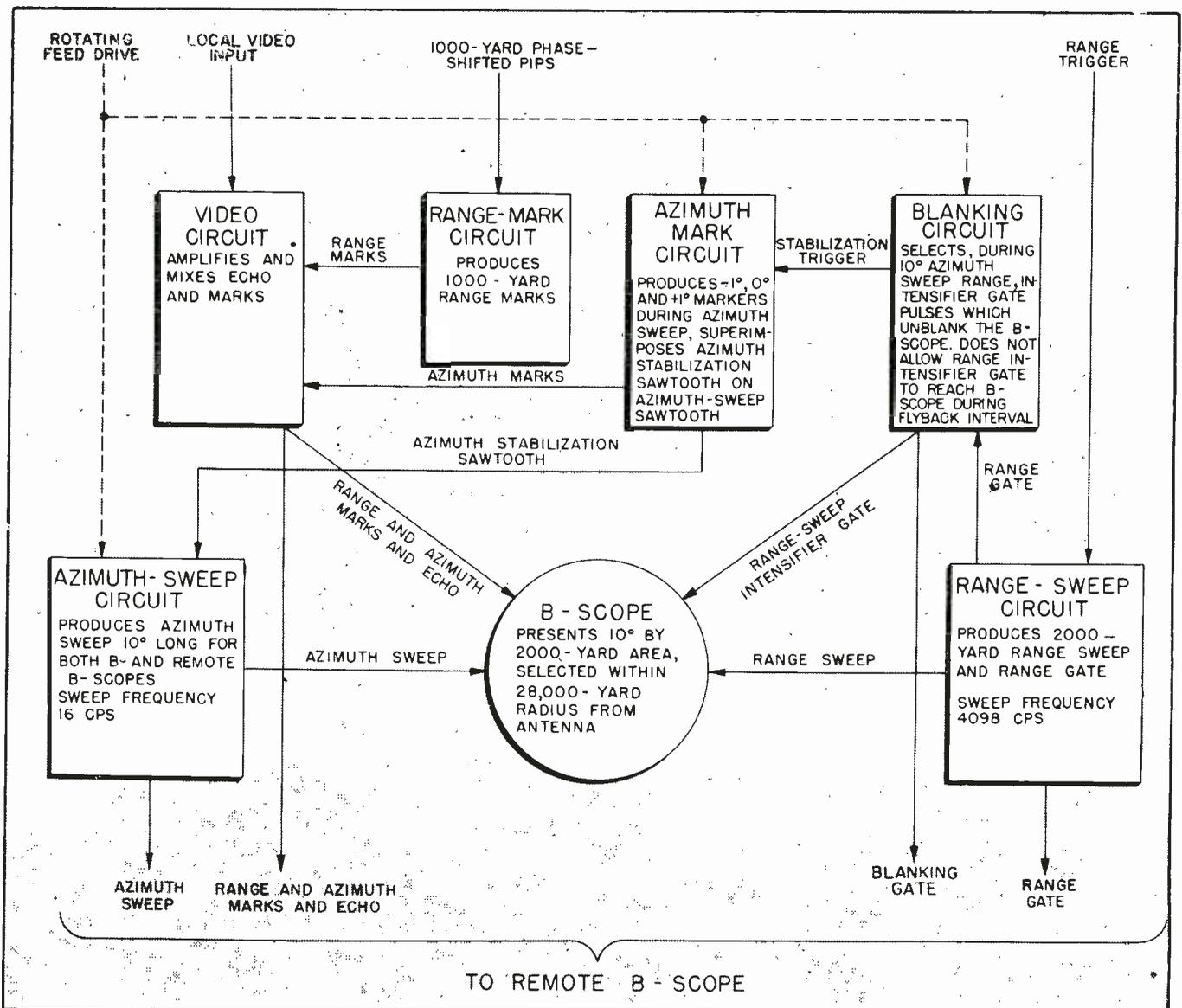
FIG. 10—Block diagram of elements of the B-scope system
