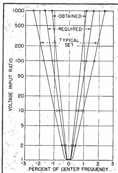
FIG. 2—Measured selectivities of superregenerative receiver
