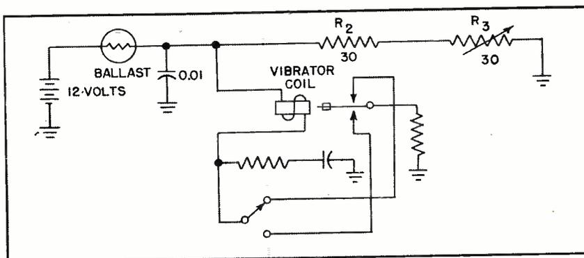
FIG. 4—Use of a special ballast permits regulation of the vibrator frequency
