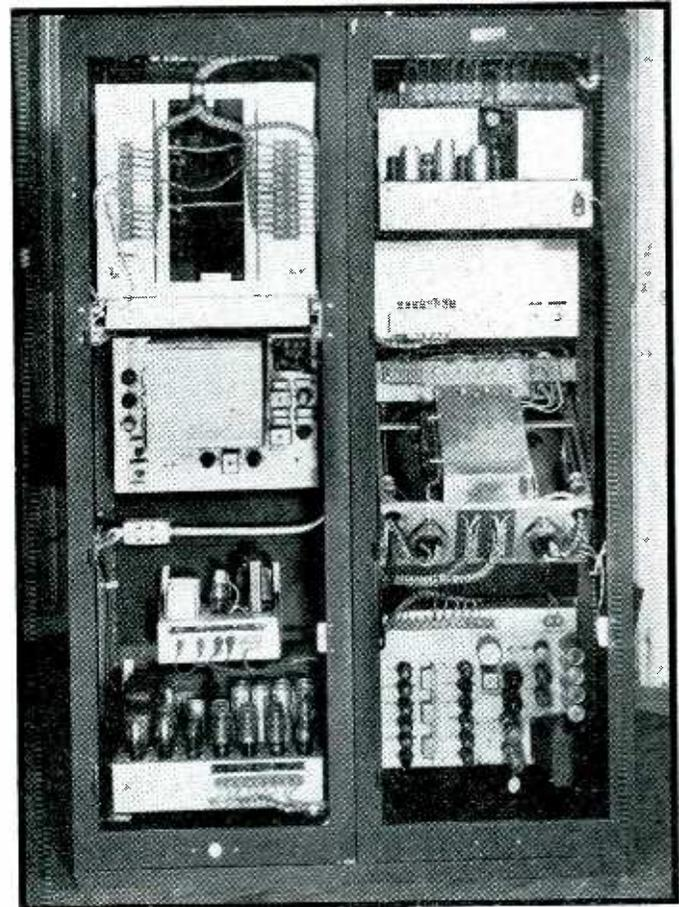
FIG. 7—Rear view of timer. Balsa-wood box at center of unit at left houses 50-kc quartz bar which maintains frequency constant
