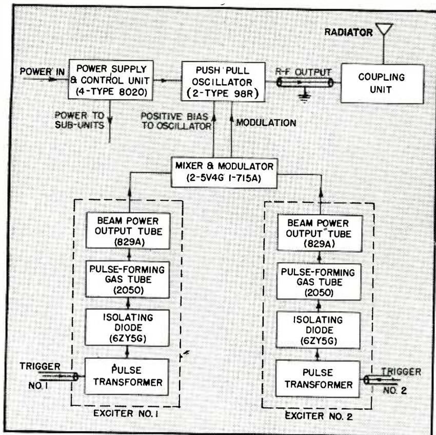
FIG. 1—Block diagram of the Loran transmitter. The modulator can be driven by two sets of pulses simultaneously, thus permitting synchronization with two adjacent stations
