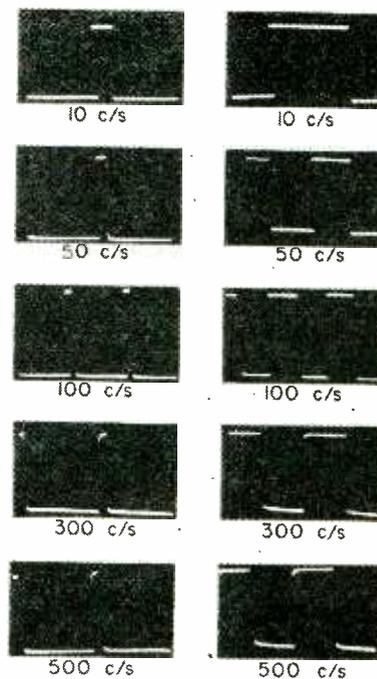
Fig. 2—Oscillograms of pulses, in the left-hand column, of one-tenth cycle duration, and, in the right-hand column, of one-half cycle duration for different frequencies
