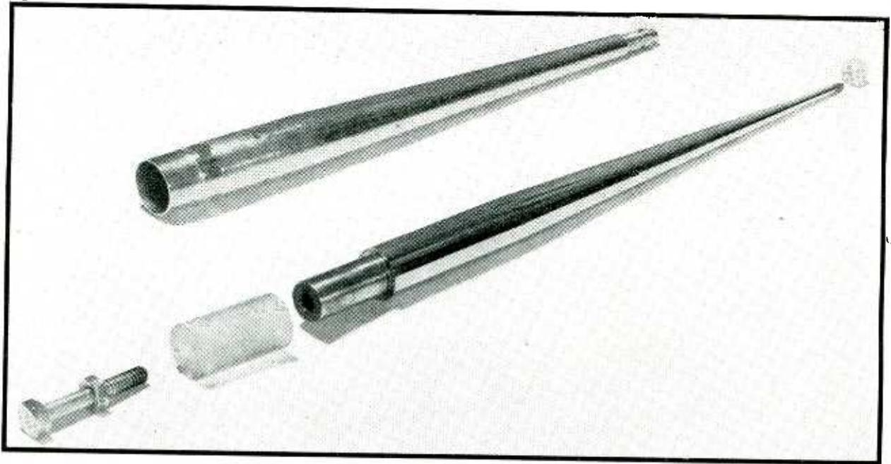
Separating-medium mandrel made of cold drawn steel, stress-relieved before machining, and finish ground to close tolerances to produce round tubing with a tapered section in the middle, the straight portions being parallel to within a fraction of a thousandth of an inch. End caps, supporting bolt and finished tubing also shown
