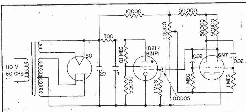
FIG. 6—Stroboscope circuit employing type 1D21/631P1 strobotron
