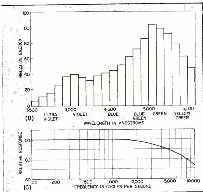
FIG. 3—Performance curves of new modulator glow lamp, showing (A) the average light response, (B) typical wavelength spectrum, and (C) average frequency response
