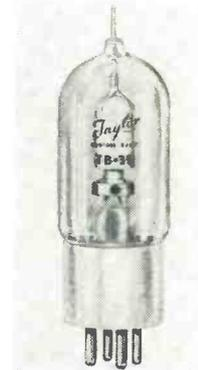
375; d-c plate current, 110 ma; d-c grid current, 15 ma; d-c screen current, 22 ma; plate dissipation, 35 w; peak r-f grid input volts, 350; driving power, 4.5 w; plate power output (to 250 mc), 130 w.
