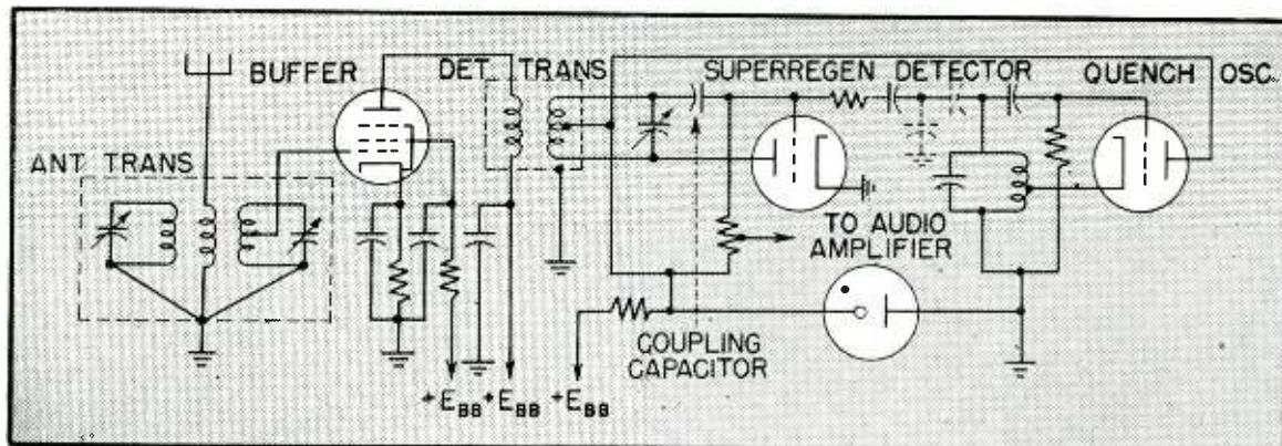
FIG. 1—Circuit of superregenerative receiver upon which tests were made. Dotted capacitors were added later to decrease bandwidth by reducing quench amplitude to the detector tube
