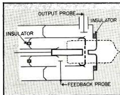
2C37 disc seal triode in a typical quarter-wave concentric line oscillator circuit
