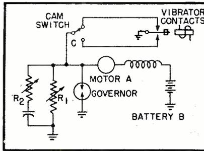
FIG. 3—(Right) In this circuit, a balance is sought between the action of the motor-driven cam switch and that of the vibrator
