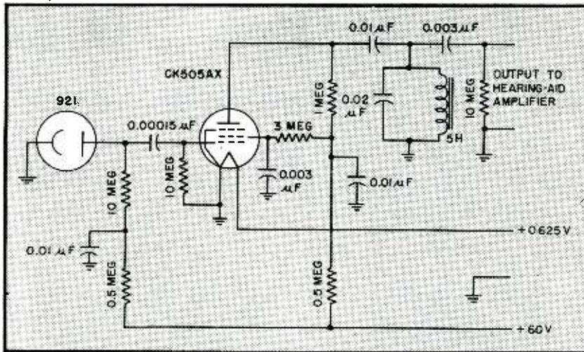
FIG. 3—Schematic wiring diagram of the phototube stage and the first stage of the amplifier. The output is fed into a slightly modified, conventional hearing-aid unit
