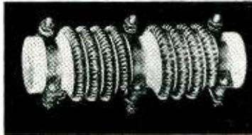
resistance element is helical wound upon a piece of solid steatite and clamped securely at both ends and in the middle. The element can be replaced without removing the assembly.
