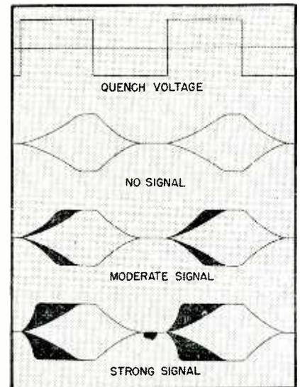
FIG. 8—Strength of the signal determines the rate at which detector oscillations grow
