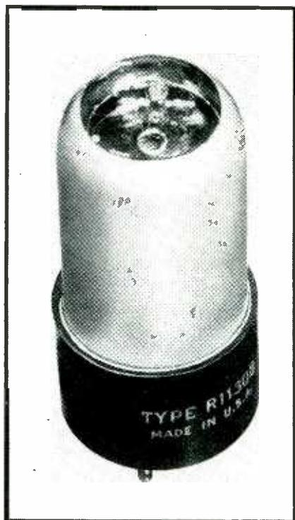
FIG. 1—New modulator glow lamp for facsimile equipment
