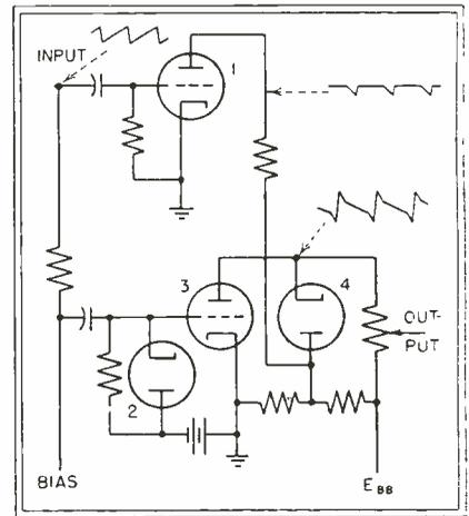
Fig. 1—Two different amplifications are obtained by electronically switching a shunt across the output load
