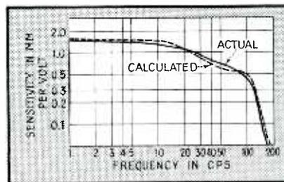
FIG. 5—Comparison of calculated and actual frequency response of the doubly resonant system
