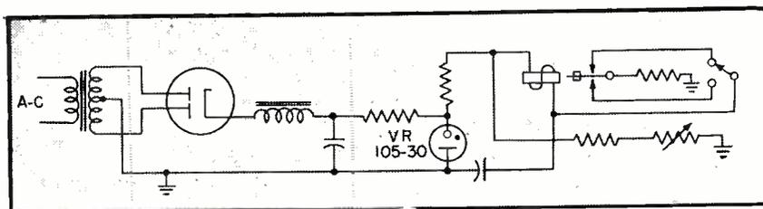
FIG. 5—Current through the vibrator is controlled by the voltage-regulator tube
