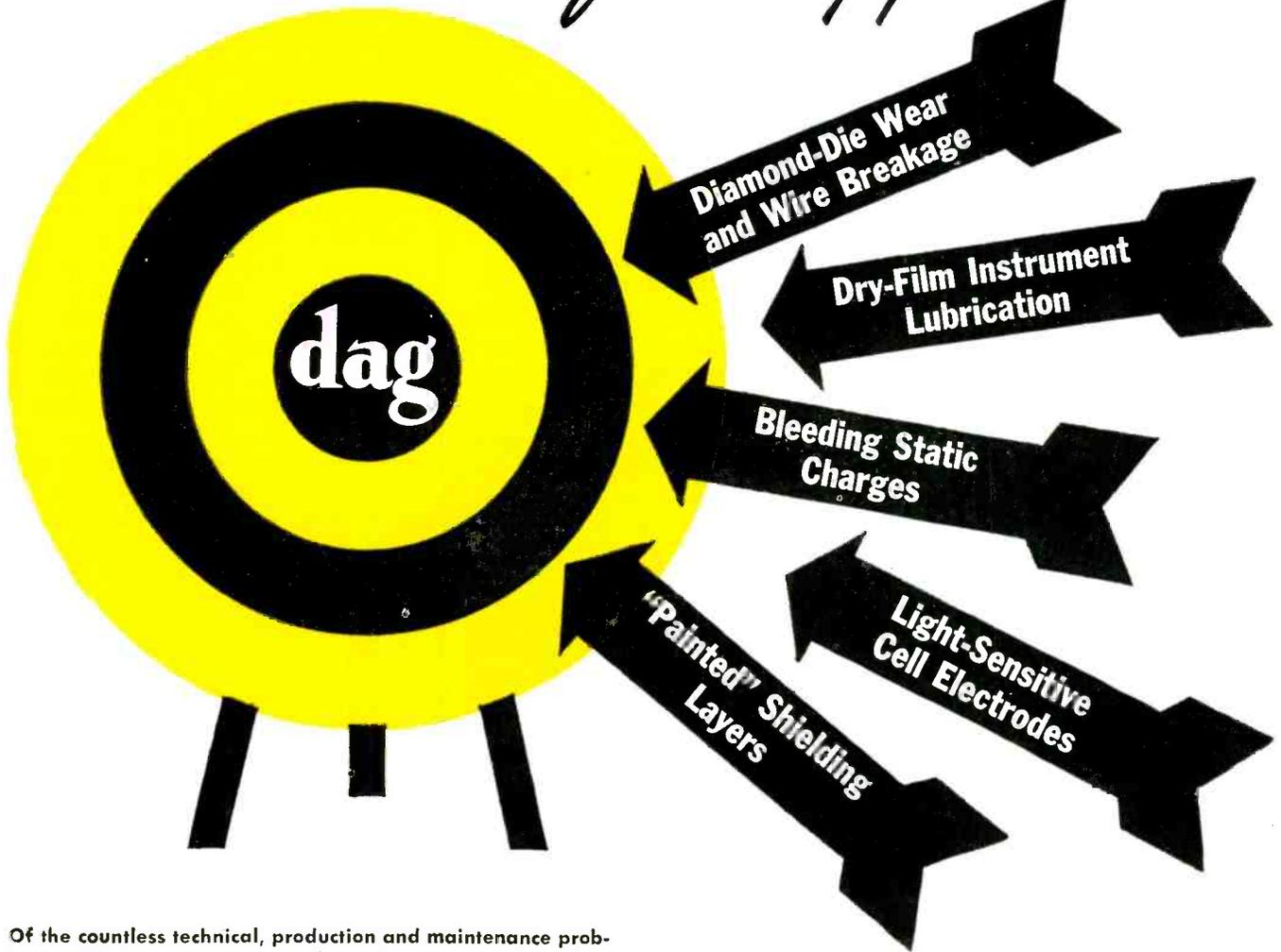
Of the countless technical, production and maintenance problems which beset the electronic industries, these are but a few of many *with the same solution*—"dag" colloidal graphite. The reason lies in the unique combination of properties of the material.
