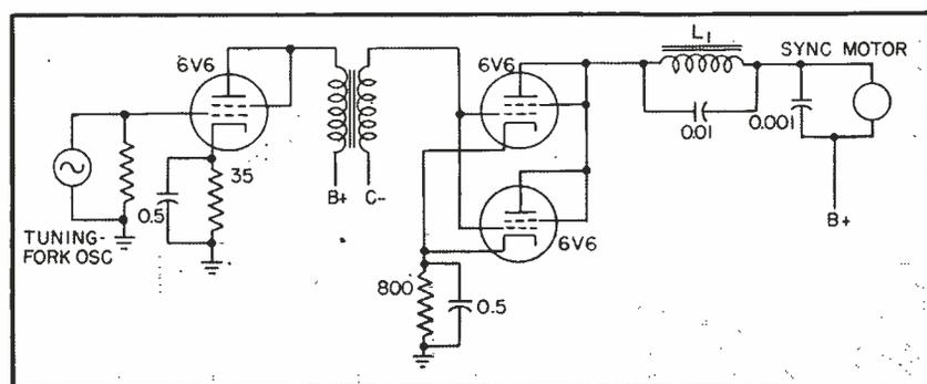
FIG. 1—Tuning-fork oscillator and class C amplifier supply high voltage to a synchronous motor. An additional motor brings the synchronous motor up to speed
