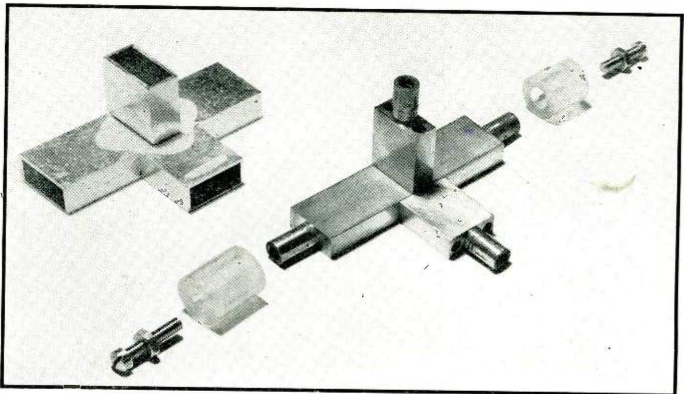
Waveguide tee section and the multiple mandrel used in its fabrication
