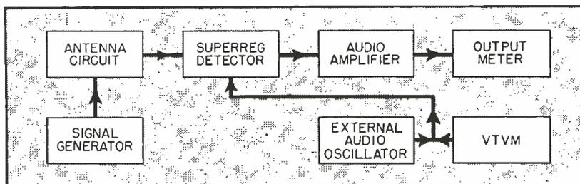
FIG. 4—Basic laboratory circuit used to study the effects on superregenerative detector of quench frequency and amplitude, and signal strength
