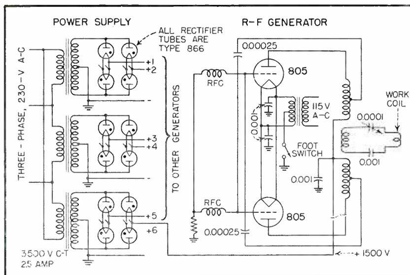
Circuit of remotely located 1500-volt d-c power supply and one of the r-f generators used at bench locations. No filtering is required in the power pack, which has six independent output lines. Generators having small loads may be paralleled on one line, so that the power pack can handle ten or more units simultaneously under some operating conditions. Automatic timers prevent closing of power pack plate circuits until the rectifier filaments are heated
