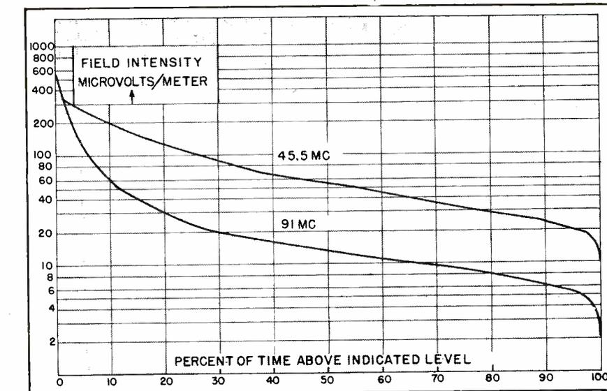
Field intensities of two f-m transmitters recorded at Deerfield, Illinois. The average 45.5-mc signal is well above the predicted value, while the 91-mc signal is below it most of the time
