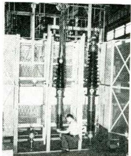
Capacitor bushings are completely assembled and placed in individual cells on a treating rack for dielectric heating. The workman is connecting an oil pressure line before placing the bushing on a small pedestal
