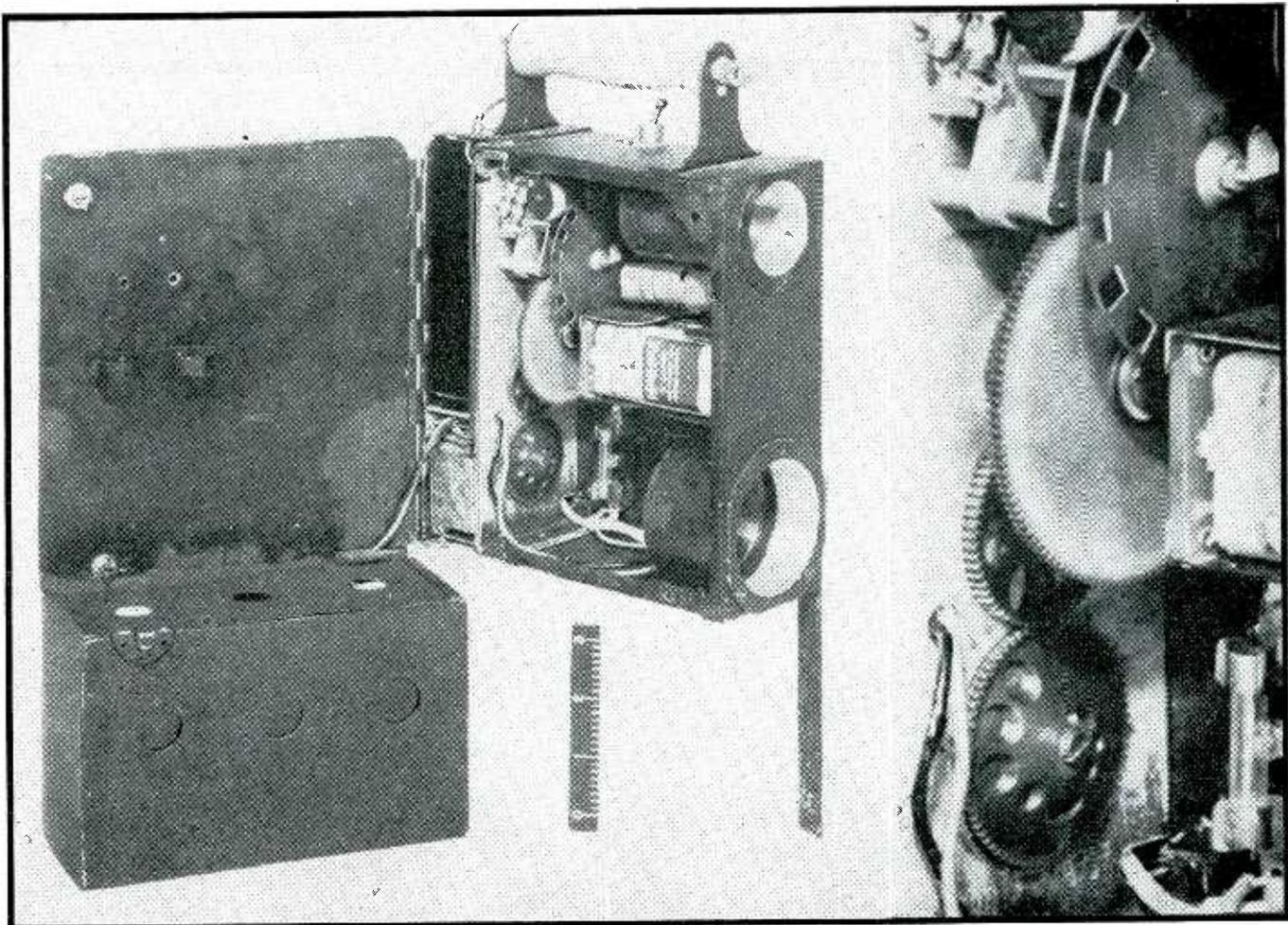
Interior view of the sensory aid. The battery which runs the driving motor is contained in the compartment at the lower left. The enlarged detail to the right shows the gear train driving the coding cone (lowest toothed wheel) and the 500-cps chopper modulator (at top with square apertures)
