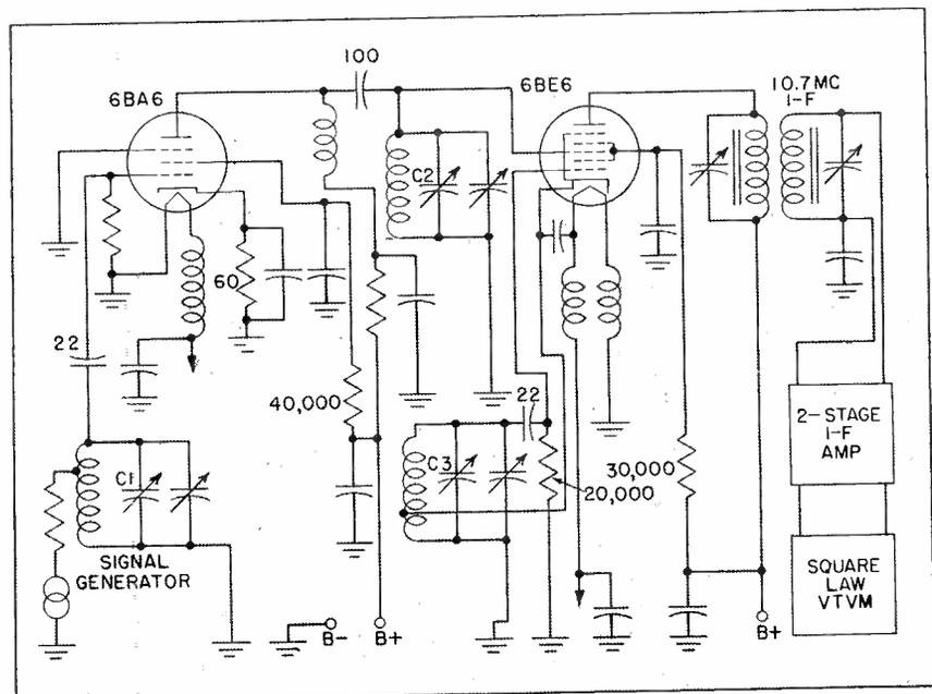
Typical self-excited converter and r-f amplifier circuits for the 6BE6 and 6BA6 tubes developed for the new f-m band
