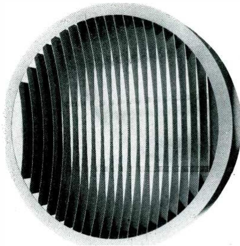
A plano-concave antenna having an aperture of 14 wavelengths
