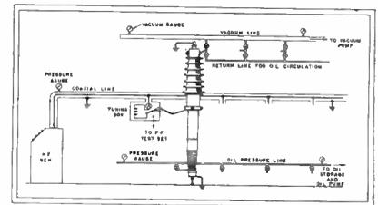
Fig. 1—Schematic diagram of the main elements used in processing capacitor bushings. Moisture driven from the bushing by dielectric heating is carried away through the vacuum line
