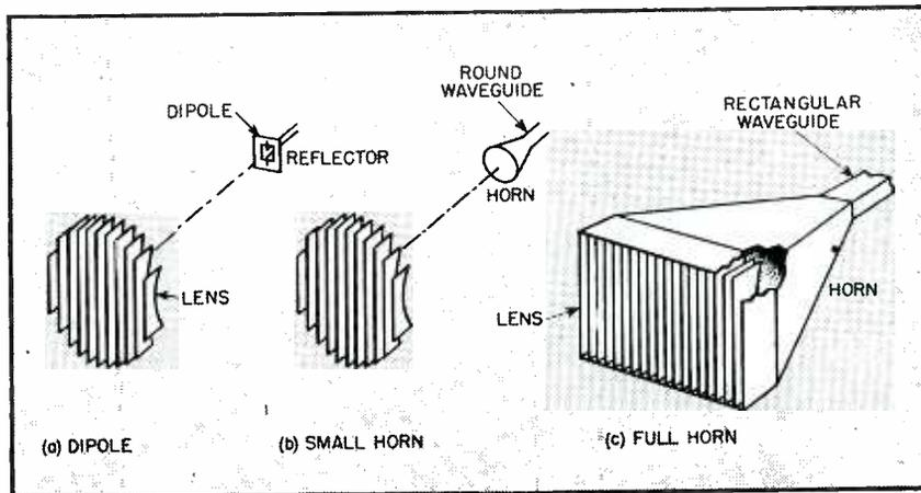
Three methods of energizing a metal lens antenna
