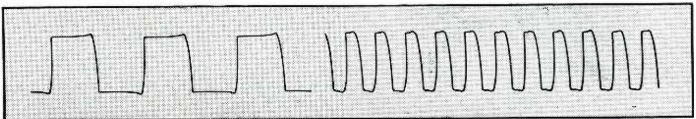
FIG. 7—Actual-size reproductions of tracings made with the new pen for 5 and 15 cps square-wave input voltages and a paper speed of 10 cm per sec
