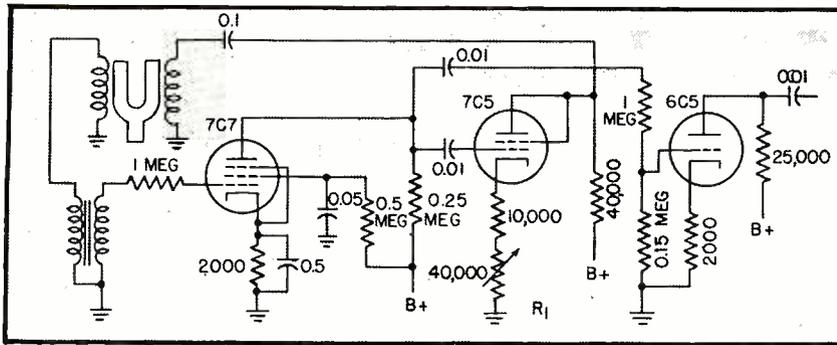
FIG. 2—(Above) Circuit of a tuning-fork oscillator using a multivibrator
