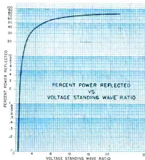
The curve shows the manner in which the reflected power increases with an increase in the voltage standing wave ratio. The curve is calculated from the following equation:
