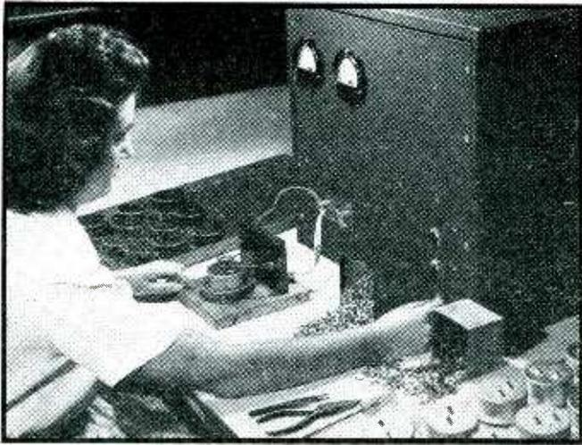
R-f soldering of feed-through insulators to back of meter case
