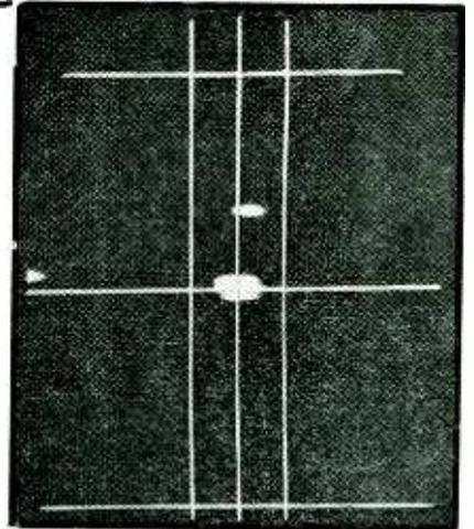
Type-B indicator presentation of shell splashes and marine target, taken on the MPG-1 by the Coast Artillery Board. The target (a corner reflector on a float) appears just above the intersection of the centerlines. A 155-mm shell has landed just short of the target (immediately below) while another shell splash can be seen above and 0.3 degrees to the right. The echo at the left is a tug towing the target. The range coordinate is 2000 yards from bottom to top of picture
