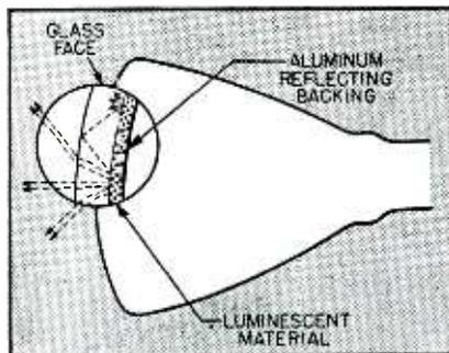
**New Kinescope with reflecting metallic film showing gain due to improved distribution of light**
