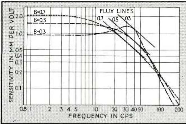
FIG. 3—Calculated response of the singly resonant system for constant mechanical impedance and varying flux density
