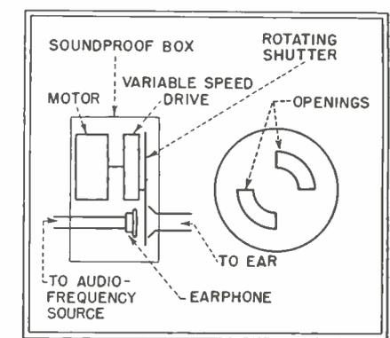
Fig. 1—Experimental equipment for measuring persistence of aural image
