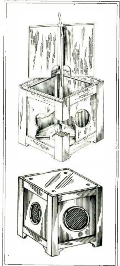
Fig. 1—The resonator cabinet is massively constructed of uniformly grained wood and houses five loudspeakers
