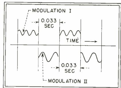
Fig. 2—Transmission of two signals by infrasonic switching. These signals can either be traveling in opposite directions as in two way communication or can be two simultaneous signals transmitted over a single electrical channel
