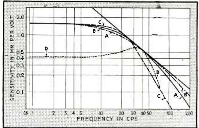
FIG. 4—Effect of varying mechanical impedances on sensitivity for a constant flux density of 0.6 weber
