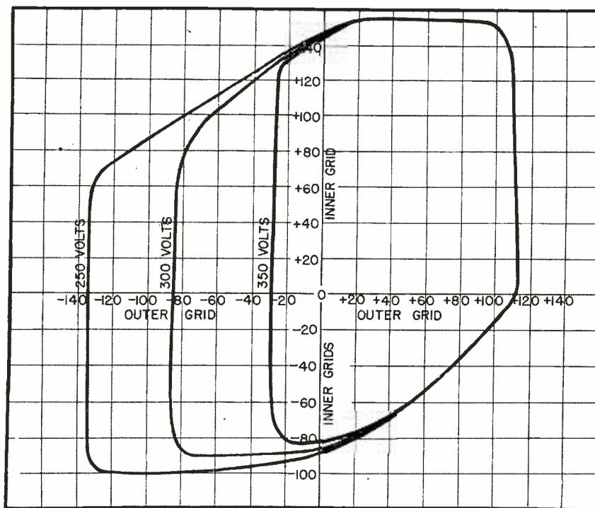
FIG. 7—Control characteristics of 1D21/631P1 strobotron
