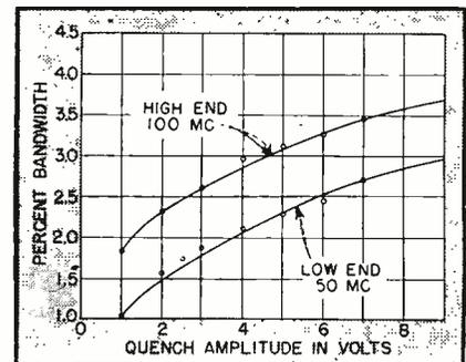
FIG. 6—Bandwidth is affected by quench amplitude
