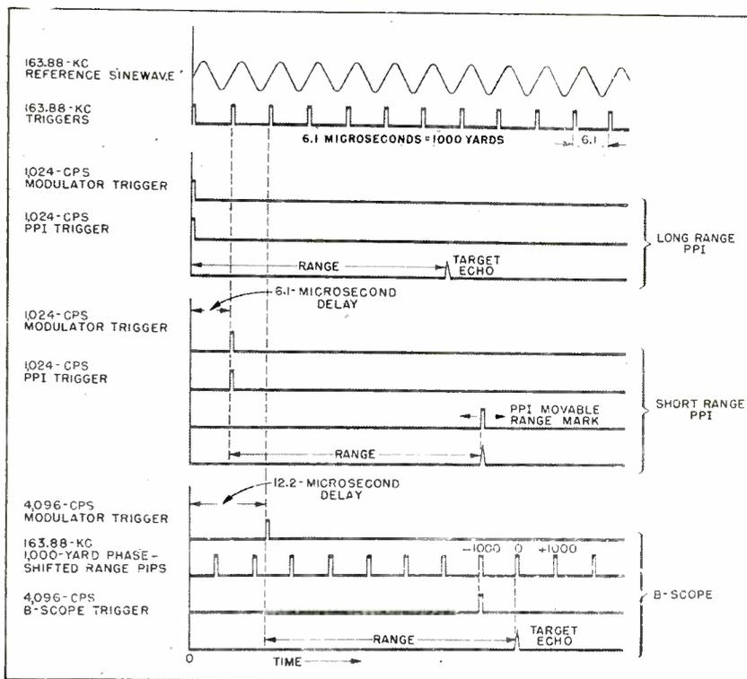
FIG. 1—Time coordination between sinewave reference voltage and various triggers which initiate modulator, B-scope and ppi
