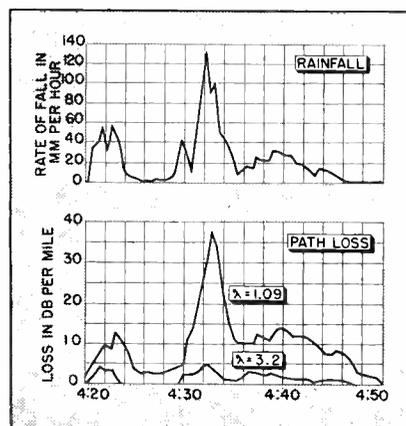
Transmission loss and rate of rain fall measured during a rainy day show relation of moisture content of air and microwave attenuation
