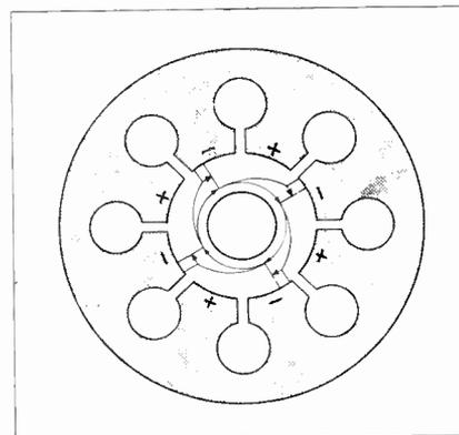
Revolving electron cloud delivers energy to radio field to sustain magnetron oscillation
