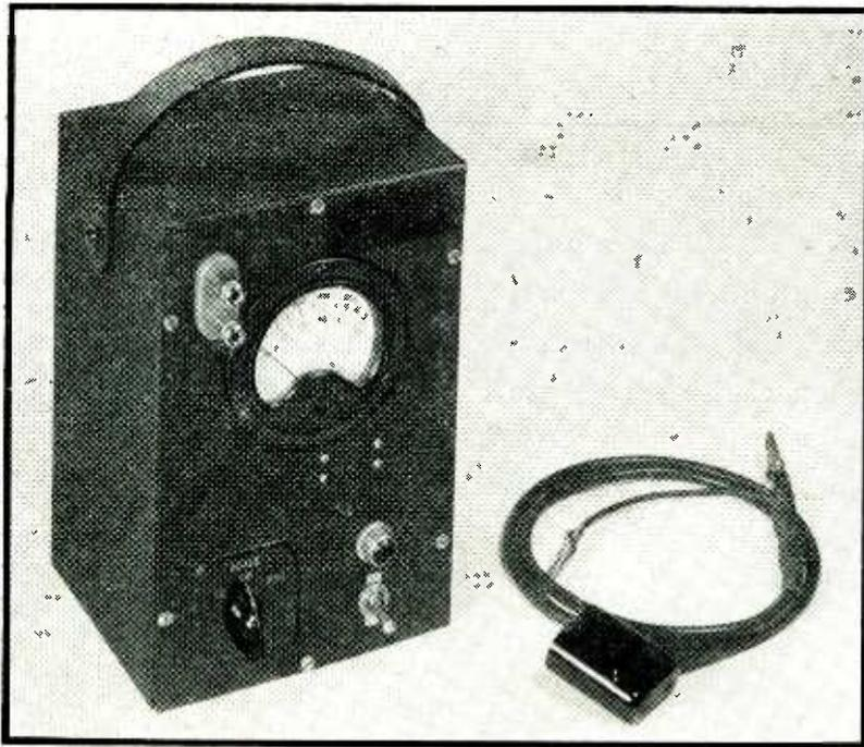
FIG. 4—The voltage range switch is the only control in the final instrument
