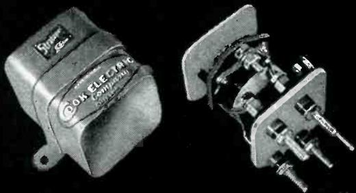
Contacter ready for Stratopaxing before covering. Wrap around mounting bracket, blister on cover for adequate terminal clearance, and binding post terminals meet specifications for unit.
