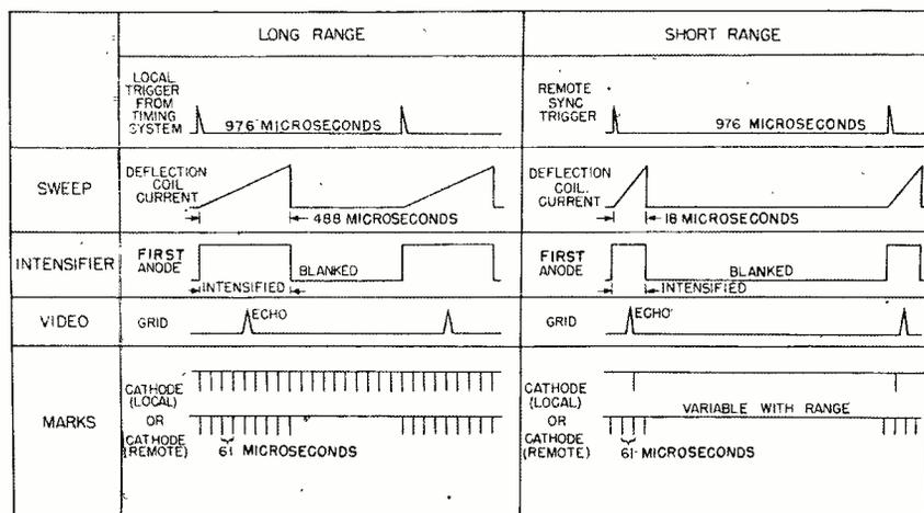
FIG. 9—Waveforms applied to the various electrodes of the ppi tube, for short-range and long-range indication
