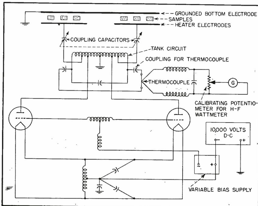
FIG. 3—Schematic diagram of the r-f heating unit showing oscillator, electrode arrangement, method of coupling the load to the tank coil and the thermal arrangement for measuring load power. The galvanometer is the central instrument shown in Fig. 2 and is calibrated to read watts directly
