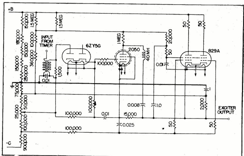
FIG. 2—Schematic diagram of the exciter unit, which produces 40-microsecond pulses to drive the modulator. The type 829A tube is connected as a "bootstrap" cathode-coupled stage which does not reverse polarity
