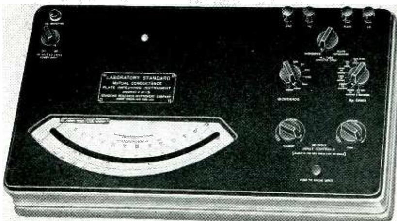
$R_p$  values from 250 to 2 megohms. Overall accuracy is 0.2 percent when used with accurately measured and regulated power supplies, competing successfully with other less facile methods.
