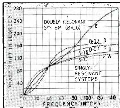
FIG. 6—Variation of phase shift with frequency for singly and doubly resonant systems
