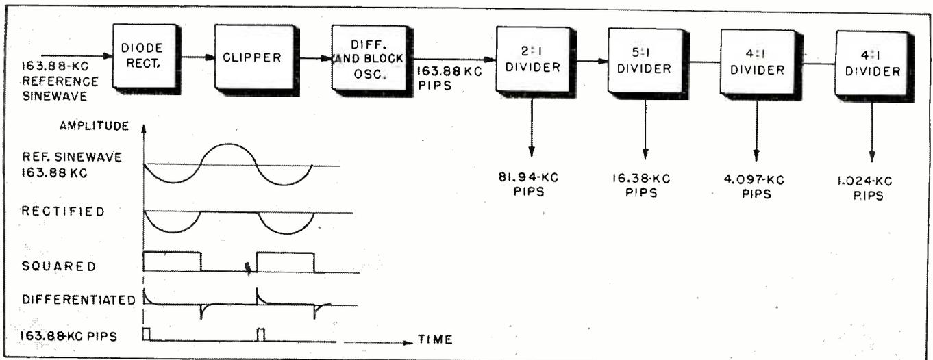
FIG. 3—Block diagram of frequency-dividing chain which reduces 163.88-kc reference voltage to pulse and indicator timing pulses
