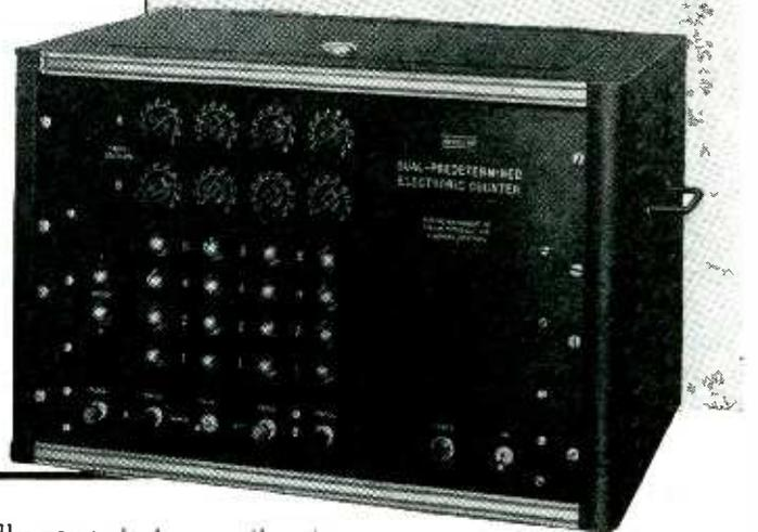
For processes requiring a rapidly repeated operation to occur after a predetermined number of counts!
