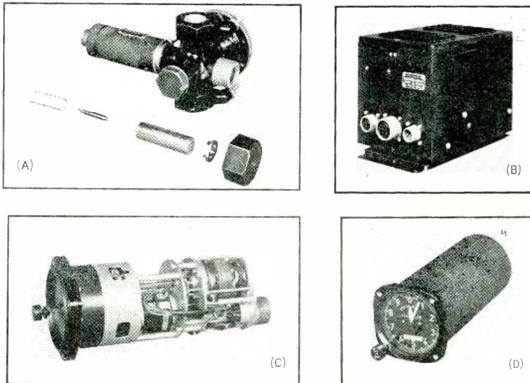
FIG. 1—Parts comprising the fuel-flow indicator and integrator. (A) The mechanical flow-valve with position transmitter at left. (B) Shock-mounted chassis containing vacuum tubes and other electronic components. (C) Interior of indicator-integrator instrument, showing one of the small motors and the precision potentiometer. (D) Aircraft-type indicator shows fuel flow up to 2,000 pounds per hour in easily read increments of ten pounds. Total consumed is displayed on the inset counter mechanism
