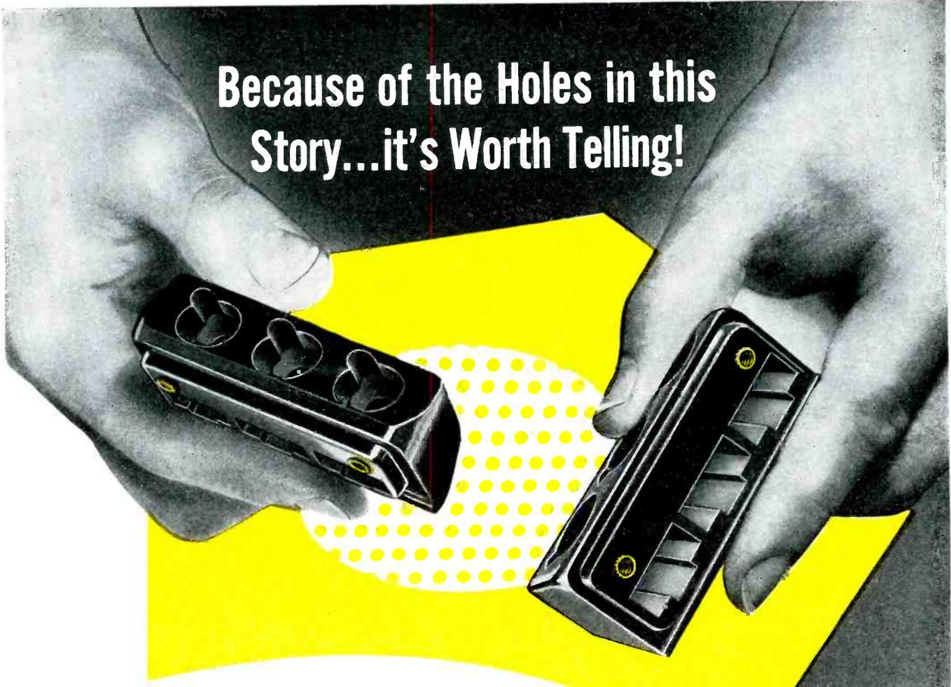
This is a Terminal Block. The two views of it reveal an alignment of three round, keyed holes molded into one side — and an opposing series of three rectangular, keyed holes molded into the adjacent face. Deep within the piece, these holes meet and form right-angle passages.
