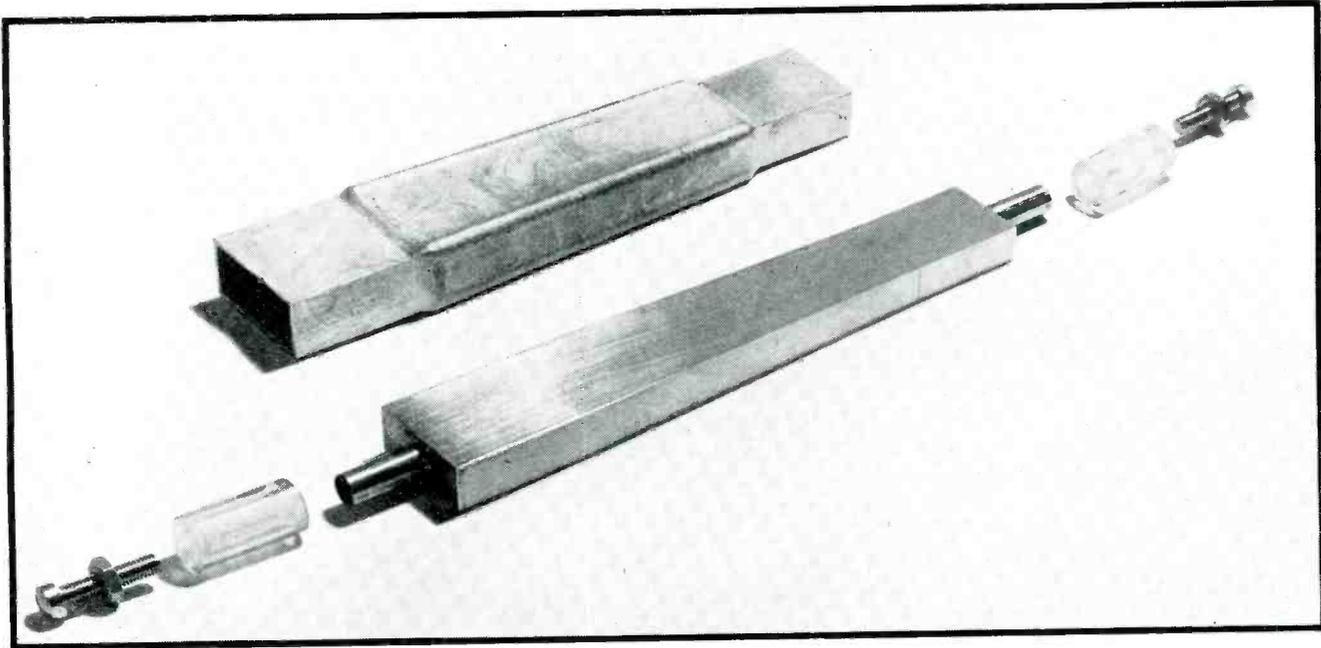
Tapered rectangular waveguide section and its mandrel, an example of the precision tubing made possible by electroforming methods
