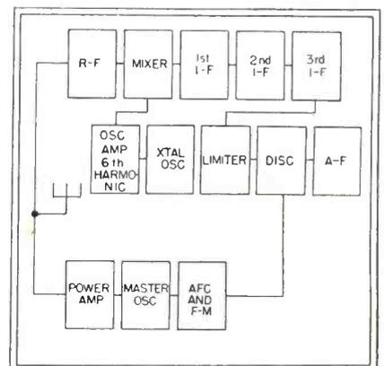
Stages of the new f-m handie-talkie. An amplifier is necessary to obtain sufficient power at the sixth harmonic of the receiver oscillator
