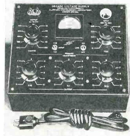
The secondary is tapped to provide the desired output voltages. A Weston meter, model 476, is placed in the secondary circuit and is calibrated with a single red line to indicate proper primary voltage adjustment. When the primary is adjusted to 100 volts the instrument may also be used as a variable-ratio transformer provided input voltages do not exceed calibration settings. One-thousand-to-one, to one-to-one values, in steps of 1/1,000 are furnished in ranges up to 10,000 cps.
