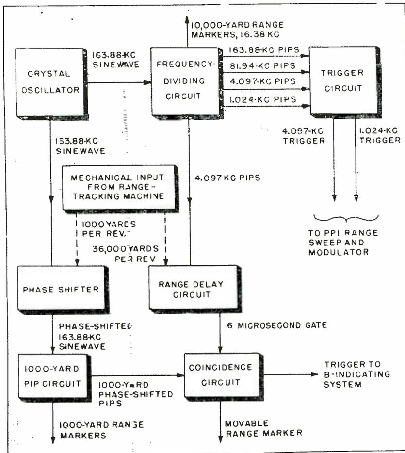
ical linkage of a potentiometer to the range tracking unit, is a coarse measure of range. The coincidence tube can conduct only one phase-shifted pip while the 6-microsecond gate is on, because the interval between pips is at least 6 microseconds. The pips formed from the phase-shifted sine-wave are a fine measure of target range.
