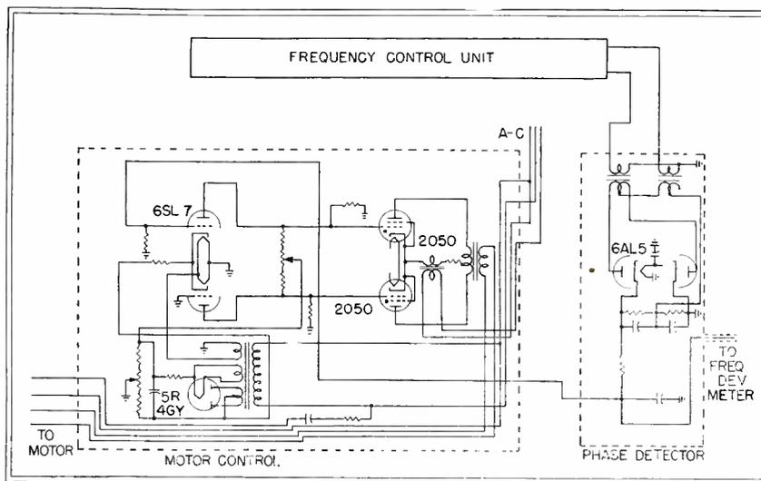
Fig. 1—Circuit arrangement for motor-driven correction of the center frequency of the primary oscillator
