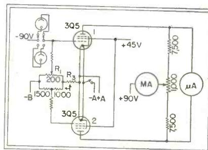
**Fig. 2—Circuit of the photoelectric fish detector**
