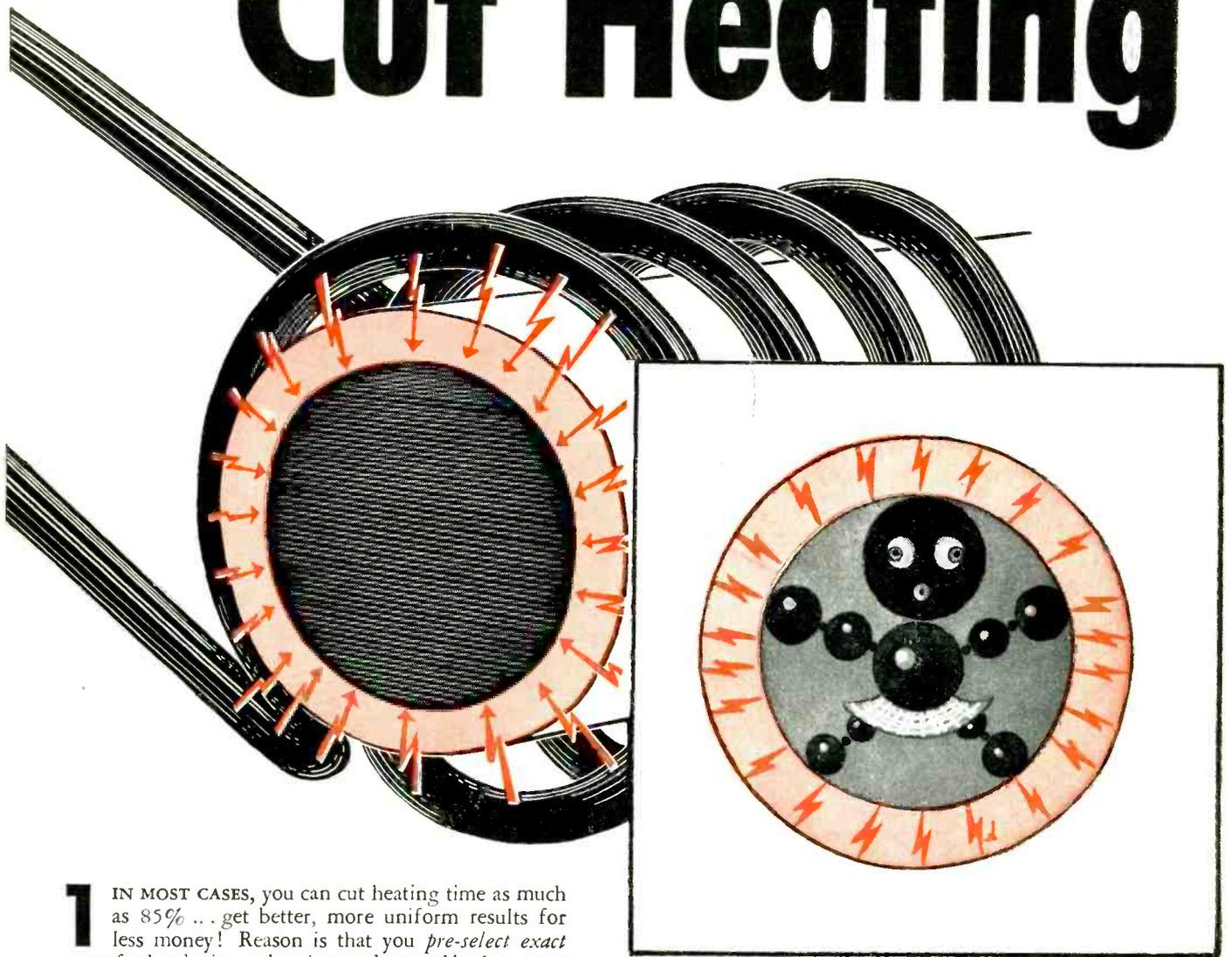
**1** IN MOST CASES, you can cut heating time as much as 85% . . . get better, more uniform results for less money! Reason is that you *pre-select exact areas* for hardening or brazing, and control both *amount* and *penetration* of heat! This new production tool is completely automatic . . . requires no experienced help. Just place part in work coil and press button. That's all! High frequency power passing through work coil induces a current in part being processed.
