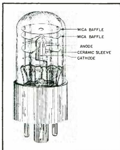
FIG. 2—Construction of modulator glow lamp. Crater forms inside hollow cathode
