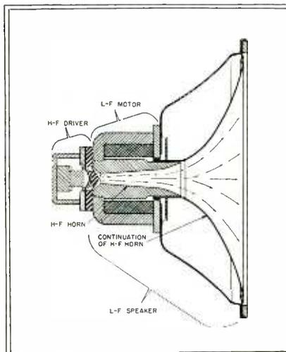
core of the l-f unit, the carefully shaped diaphragm of the l-f unit forming a continuation of the h-f horn. The l-f diaphragm is driven by a conventional voice coil assembly.
