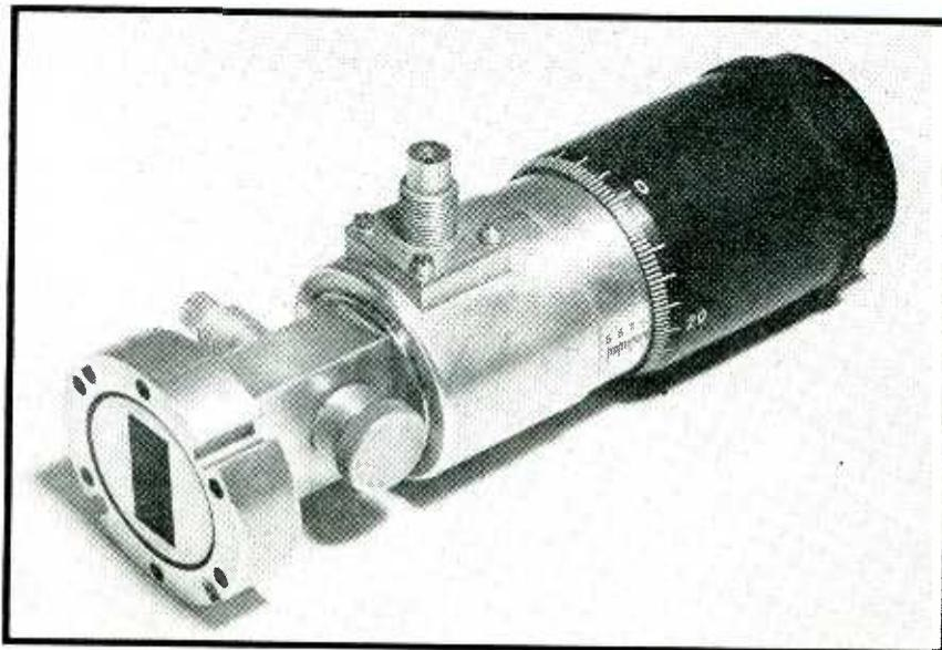
Wavemeter using waveguide feed in which the precision resonator is electroformed
