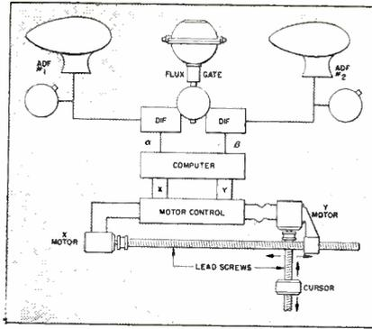
Pictorial block diagram of two loops, flux gate compass and integrating mechanism which drives a cursor to project a light spot upward through a map
