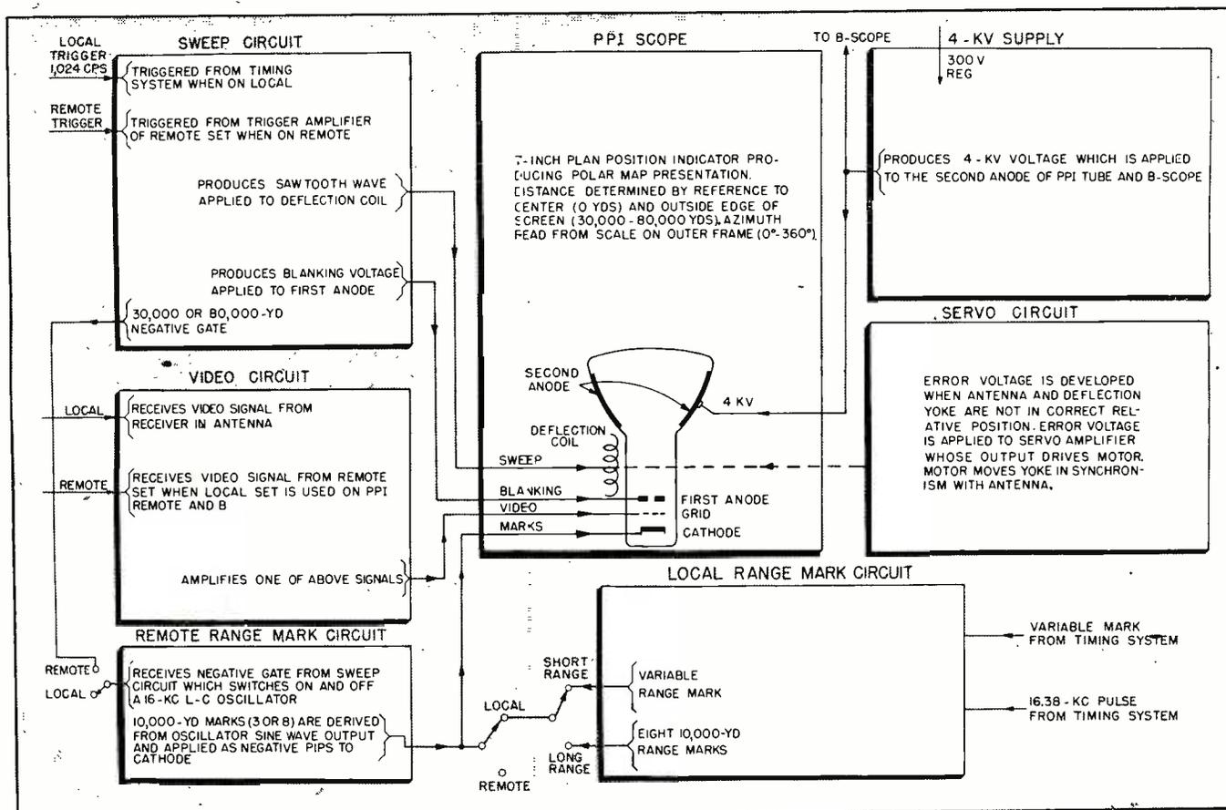
FIG. 8—Block diagram of ppi system. The deflection yoke is rotated mechanically about the neck of the cathode-ray tube, while intensity modulation imposes echo signals and range markers
