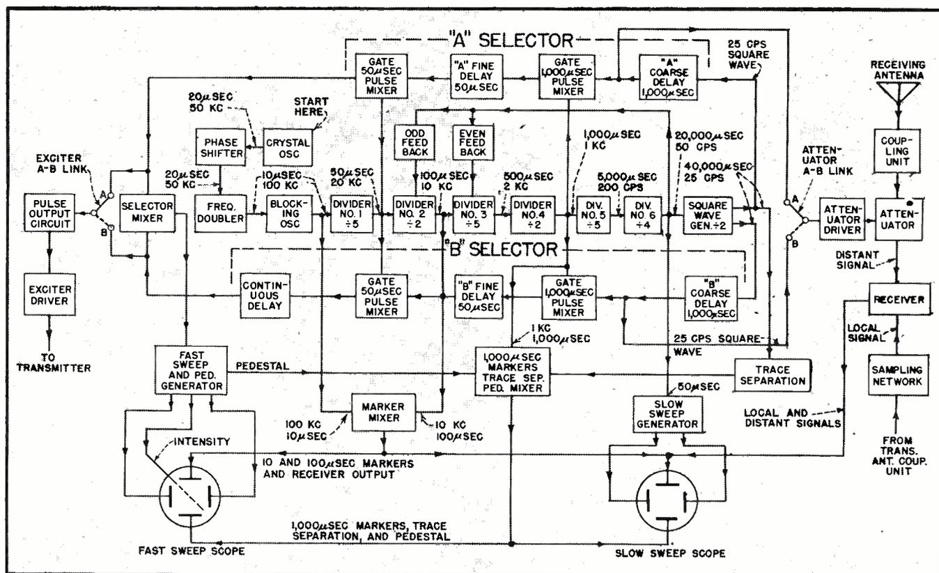
FIG. 8—Block diagram of timing unit. This equipment performs functions similar to the Loran receiver indicator but with greater precision and stability. Two indicators show slow and fast sweeps simultaneously
