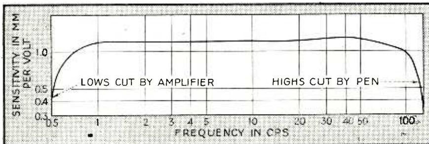
FIG. 1—Frequency response of high-speed direct-inking pen and amplifier
