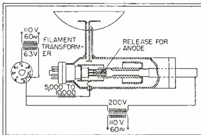
Two power transformers and a suitable dipole antenna with reflector must be connected to the oscillator as shown here. A detector consisting of a crystal detector and a microammeter or a-f amplifier can be used
