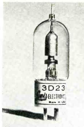
w plate dissipation) making the tube suitable as a power amplifier, oscillator or amplifier-doubler.
