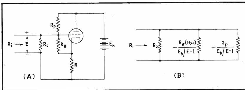
FIG. 2—(A) Circuit for calculation of the input resistance of the d-c voltmeter. (B) Equivalent input circuit composed of two negative resistances and one positive resistance
