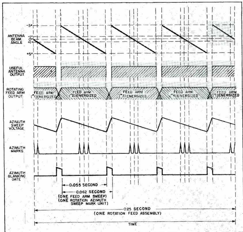
FIG. 12—Timing coordination between antenna rotation and azimuth-marking and blanking waveforms
