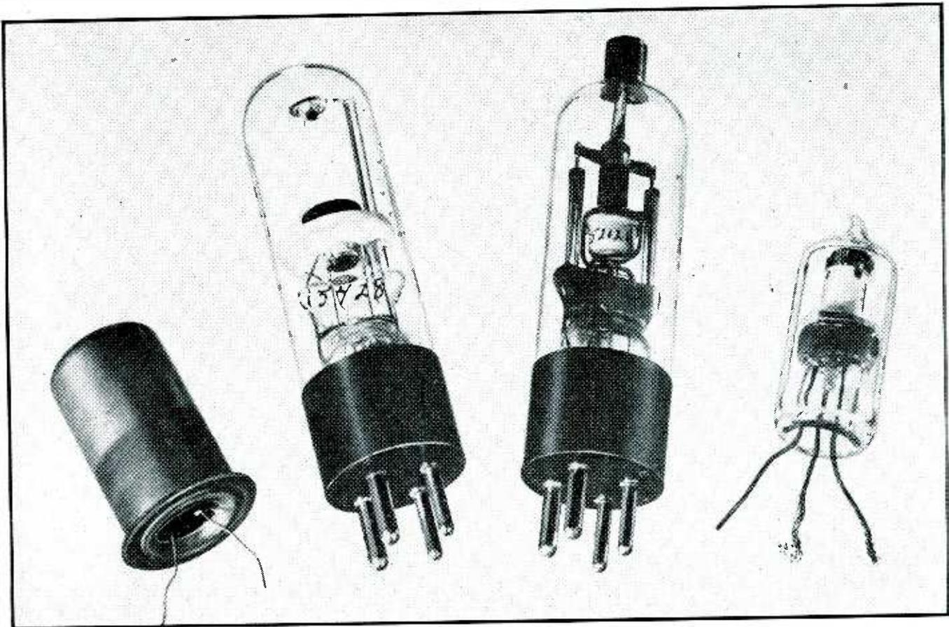
Special types of gaseous discharge tubes, used in various applications for generating short-duration pulses having extremely high peak current
