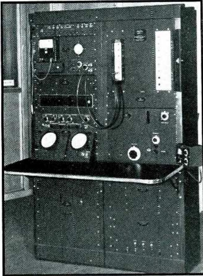
FIG. 6—Model C-1 Loran timer, which synchronizes the signals with the adjacent station
