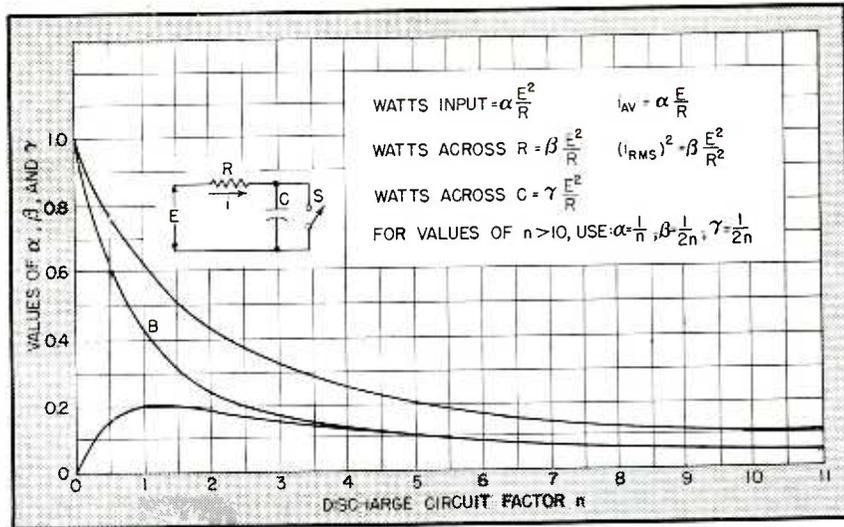
FIG. 10—Chart for determining power ratings of charging circuit components used in connection with a gaseous discharge tube
