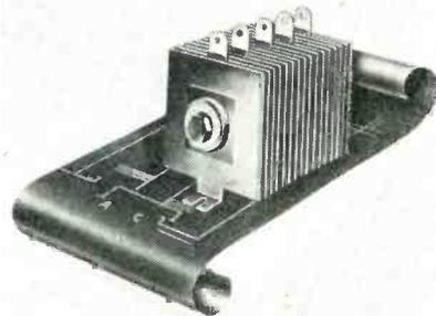
automotive batteries. Two rectifiers operated from separate transformer secondaries may be operated in parallel for 100 amp.
