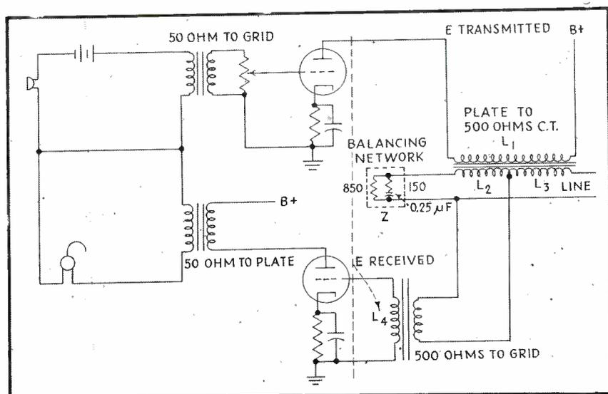
FIG. 1—Complete terminal equipment showing the handset and amplifiers, bridge circuit for reducing side tone, and detail of a typical balancing network. A conventional power supply is used
