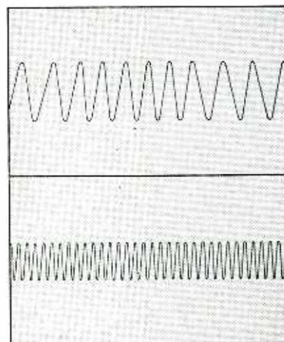
Magnified portion of a micro-oscilloscope trace showing (top) a 10-cm wave and (bottom) a 3-cm wave. Twelve such traces can be recorded on a plate 1½ x 15/8 in.
