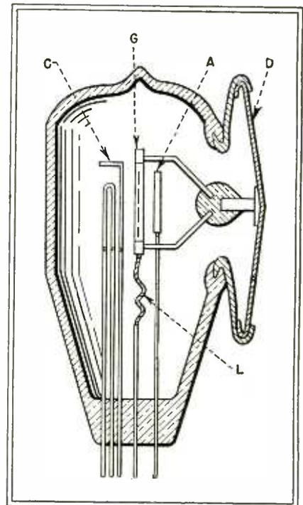
Fig. 1—Pressure-sensitive electron tube designed for use in pressure and motion measurements
