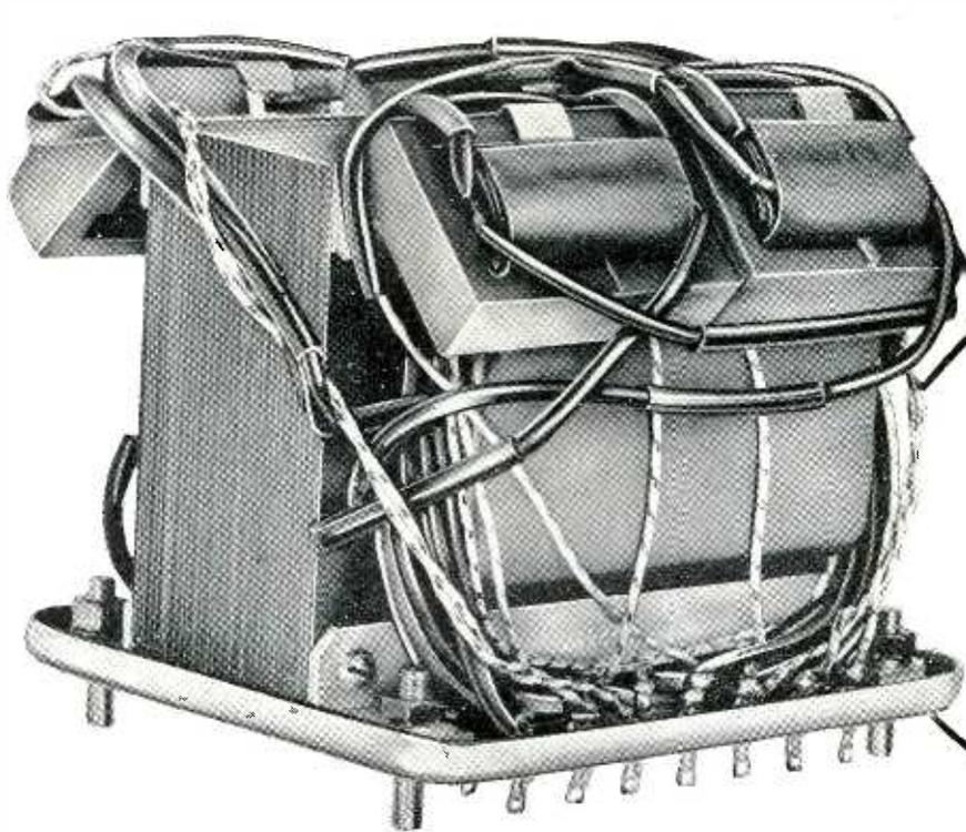
*New York Transformer Company's Type 11071 is a self-regulating power supply transformer. This interior view shows leads protected by NATVAR No. 400 high-heat-resistant extruded vinyl tubing before hermetic sealing in potting compound at elevated temperature.*
