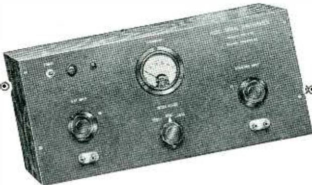
This instrument is essentially a dual input, sensitive vacuum tube voltmeter. In production and laboratory test procedures, typical applications are: synchronizing audio oscillators with radio WWV, calibrating modulation frequencies of transmitters, adjusting filter networks and tuned circuits—or any application where a beat must be observed down to a few cycles per second.
