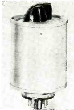
open-frame or plug-in metal enclosures; the adjustable unit in dust cover enclosure only. Timing range is from 1-12 pps; voltage, to 32 v d-c or to 125 v a-c, 60 cps. Contacts are spst normally open or closed, dpst normally open or closed and dpdt. Contacts carry 10 amp (non-inductive, at sea level).
