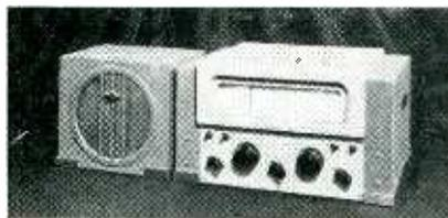
d-c, employs 10 tubes and has 4 watts audio output. An input of 5 microvolts gives 50 milliwatts output. Bandwidth is 4.5 kc at 6 db down with about 70 db at 10 kc off resonance. It is equipped with avc. The receiver is  $9\frac{1}{8} \times 17\frac{3}{8} \times 12\frac{3}{8}$  in. and weighs 8 lb. The matching speaker is  $8\frac{3}{8} \times 10\frac{1}{8} \times 7\frac{1}{2}$  in. and weighs 8 lb.
