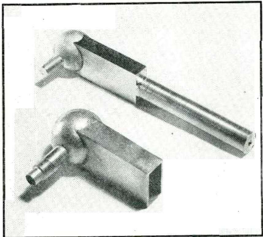
Dissolvable metal mandrel and experimental waveguide starting section using a special antenna housing, a typical use of the techniques for experimental models
