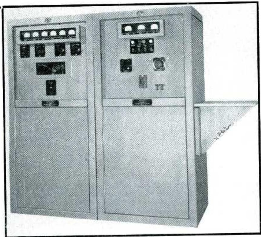
Front view of the transmitter, consisting of r-f unit and modulator; exciter, control circuits and power supply (right)
