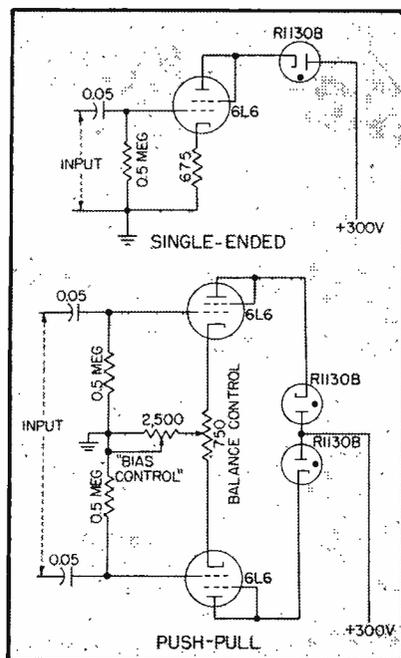
FIG. 4—Typical output circuits for driving the new type R1130B modulator glow lamps
