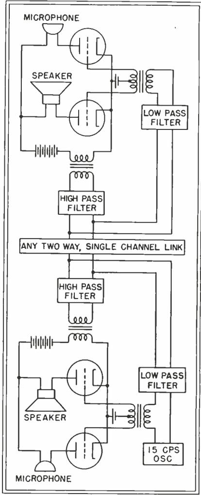
Fig. 3—Simple circuit illustrates the way in which simultaneous, two-way communication can be carried on over a single-channel link such as a two-wire line or a two-way radio
