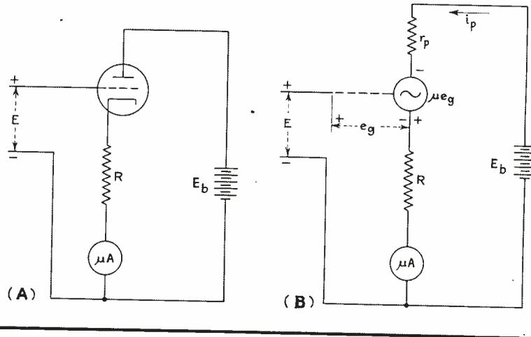
FIG. 1—(A) Basic circuit diagram of the d-c voltmeter. (B) Basic equivalent circuit arranged for analysis
