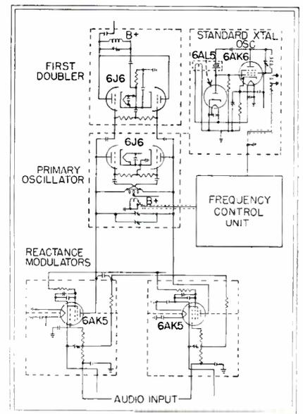
Fig. 2—Essential portions of the exciter unit of the Temco model 250 BCF f-m transmitter
