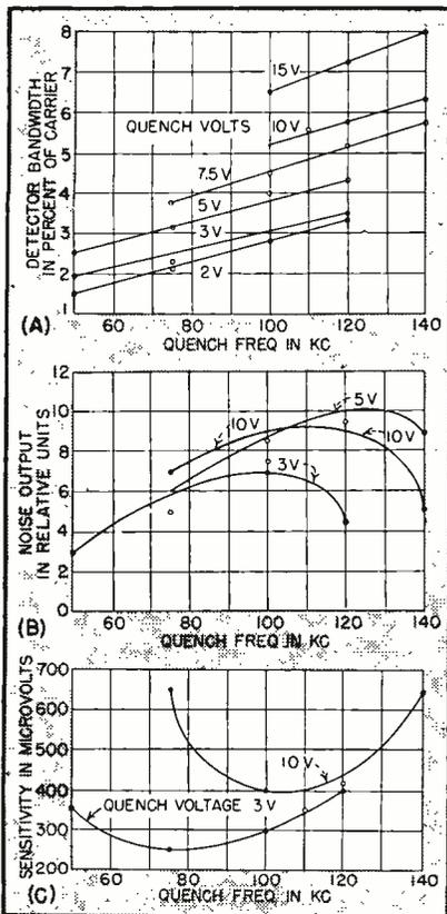
FIG. 5—Quench frequency affects detector bandwidth (A), detector noise output (B), and detector sensitivity (C)
