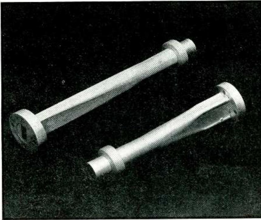
Round-to-rectangular waveguide sections made on expendable mandrels
