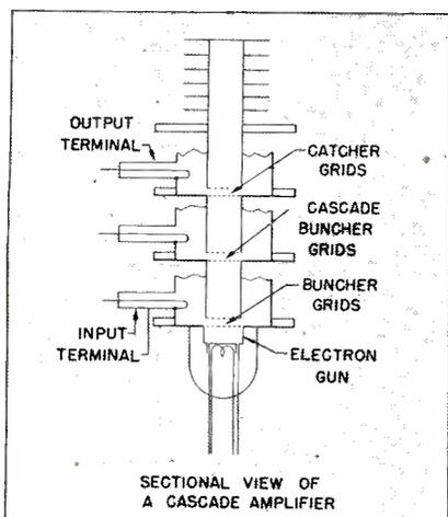
Three resonator Klystron provides greater power output from the beam modulation than two resonator or reflex types, for same input power
