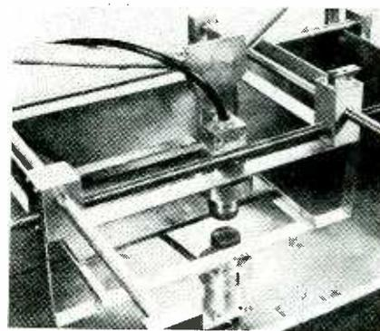
Continuous strip materials pass through a liquid-filled tank in which the piezoelectric transducers are mounted to face both sides of the strip
