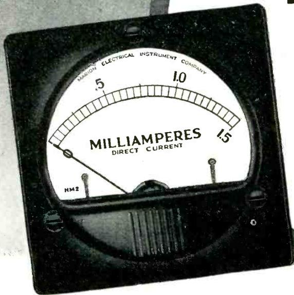
...they're **dustproof and moisture-proof** — foreign matter which oxidizes pivots and attacks bearings and thus shortens the life of an instrument cannot enter.
