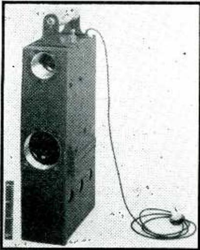
Sensory aid developed by Signal Corps Engineering Laboratories. The air-conduction headphone is shown at the right. The complete unit weighs about nine pounds
