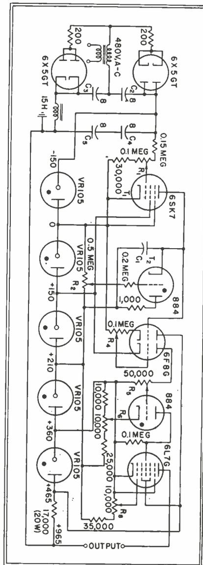
Fig. 1—A 65,000 ohm resistor in series with the thyratron grid lead from  $R_6$  is not shown
