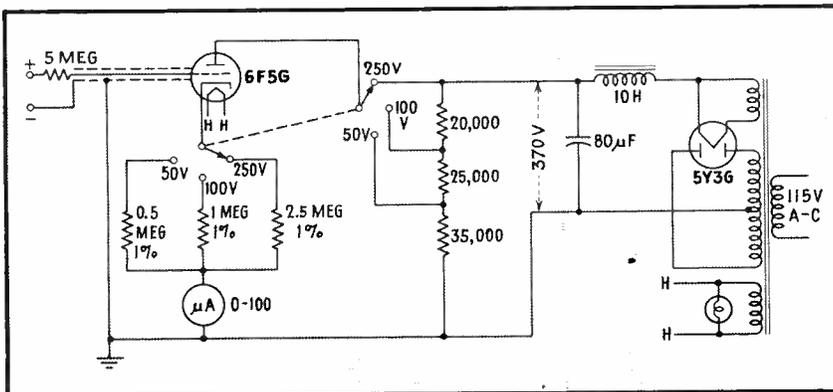
FIG. 3—Complete circuit of the high input resistance d-c voltmeter
