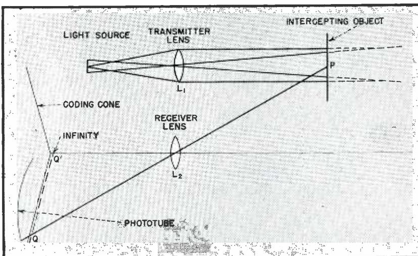
FIG. 1—Schematic diagram illustrating triangulation ranging principle. As the distance to the intercepting object becomes great, the reflected beam passes nearly straight through the axis of the receiver lens. A series of holes in the coding cone allows interpretation of the angle of intercepted light on the photocell
