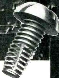
The P-K Type "F" Self-tapping Screw is used for a multitude of fastenings . . . for wire coats, insulation, switch covers, name and calibration plates, and even functions as terminals in these I. T. E. switchboards and circuit breakers. It cuts a clean, snug fitting thread as it is driven, and makes secure fastenings in such materials as the slate, epoxy asbestos, and bakelite used in these switchboards.
