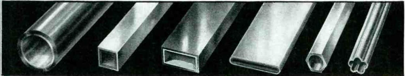
**TUBING:** Because our tubing is actually deep-drawn sheet, its quality is easily controlled. Dimensional limits lie between approximately .015" O.D. to 2" O.D. with wall thickness as small as .005". Very close tolerances can be maintained both on wall thickness and diameters. Laminated tubing is now used in the electrical industry, for electronic applications, high frequency radio parts, delicate instrument
