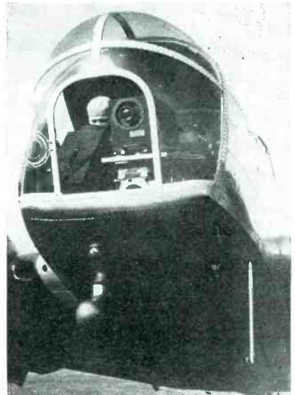
Camera unit of RCA's Bloc airborne television system, mounted in nose of plane for first public demonstration of this military television application. Many thousands of these units were built by RCA Victor for the armed forces, including special adaptations for pilotless bombers, gliders, rocket projectiles, aerial bombs, and explosive-crammed crash boats
