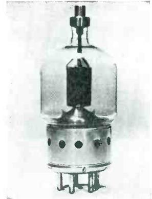
used as a 1,000-watt input final amplifier driven by a single 6L6 crystal oscillator. Low interelectrode capacitances make this tube useful at high frequencies. The grid-to-plate capacitance is  $0.19 \mu\mu\text{f}$ ; grid-to-filament  $9.04 \mu\mu\text{f}$ ; plate-to-filament  $4.16 \mu\mu\text{f}$ . Overall length of the tube is approximately  $6\frac{1}{2}$  inches, diameter,  $2\frac{3}{4}$  inches.
