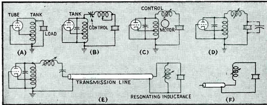
FIG. 1—Basic generator and coupling circuits employed in high-frequency heating
