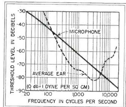
FIG. 3—Comparison of operating thresholds of microphone and of average ear
