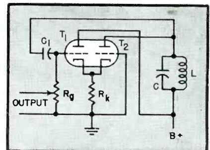
FIG. 3—Capacitor  $C_1$  provides feedback to the grid of  $T_1$  and also blocks the plate voltage
