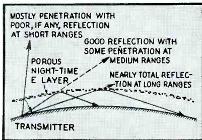
FIG. 9—The porous character of the night-time *E* layer is illustrated by the reflection at long ranges, the penetration at short distances
