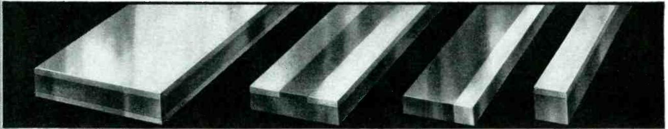
**SHEET:** Sheet is manufactured in any combination of metals and in any quality or ratio, single or double plate or striped. A recently developed specialty is edgelay. Laminated sheet can be produced as thin as .003 of an inch; in widths from 1/8 inch wide to 6 inches wide, and within tolerances of .0001" to .0002" depending on the material.
