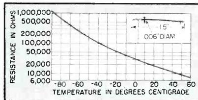
FIG. 3—Effect of temperature on ohmic value of temperature-responsive ceramic resistor used in radiosonde, and closeup view of unit
