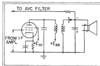
FIG. 1—Metallic-oxide rectifier simplifies audio output circuit
