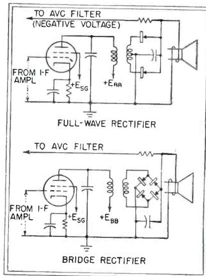
FIG. 2—Best results are obtained with a full-wave rectifier
