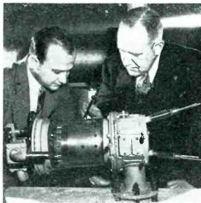
This resonatron, developed by the Westinghouse Research Laboratories and made in their Sharon, Pa. plant, is being modified for television and communications applications. Weighing 500 lb, it served during the European campaign to jam German night-fighter radar sets by generating a powerful barrage of static in a continuous wave that blanketed large areas
