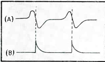
FIG. 1—(A) Pulses produced when a magnetized projectile passes through the two coils of a chronograph and (B) the same two pulses modified by wave-shaping networks
