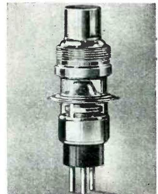
milliamperes, cavity voltage 325 volts and heater voltage 6.3 volts. Heater current is 1.1 amperes. The type SD-835F klystron has an overall length of 3 inches; bulb diameter 0.75 inches; and diameter of grid disc 1.125 inches.
