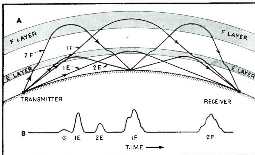
FIG. 10—Multiple-path transmissions occur in many combinations, only a few of which are shown. Their appearance on the loran indicator scope is suggested at B. Only the ground wave, G, and the 1-hop *E* will have any semblance of stability over a period of time
