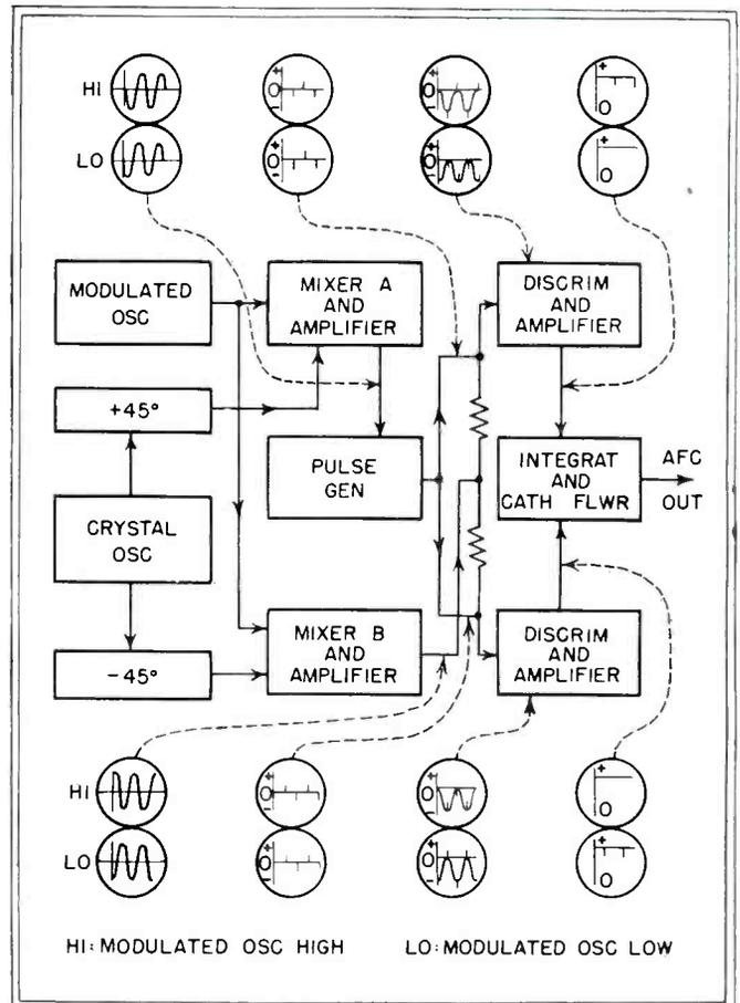
FIG. 2—Pulse counter stabilizes f.m. oscillator
