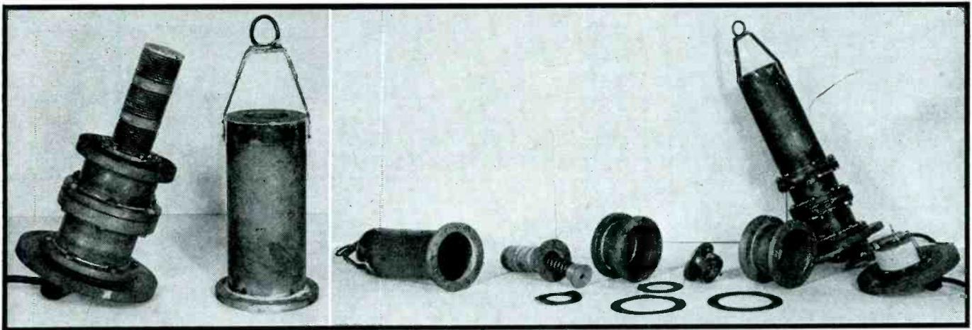
FIG. 3—Moving-coil type wave-pressure measuring unit developed by Woods Hole Oceanographic Institution, shown (left) with the cover removed, and disassembled, with the moving coil and magnet at the lower right
