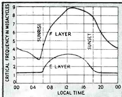
FIG. 6—Critical frequencies for the *E* and *F* layers at various times of the day. These plots are particularly important in showing that ionization in the *E* layer is not entirely dependent upon solar radiation
