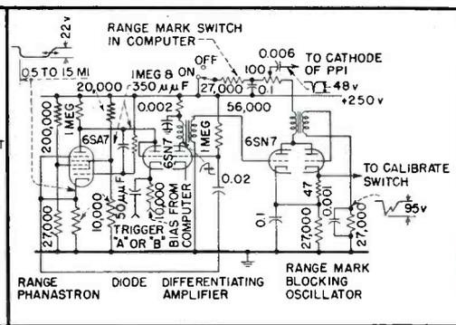
FIG. 5—Range phanastron circuit and succeeding stages in APS-15 system
