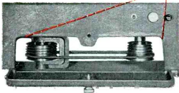
The belt on step pulleys slips instantly to any position to set cutting pitch at 96-104-112-120-128 or 136 lines per inch. Other pitches available on special order.
