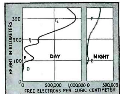
FIG. 2—Night and day distribution of free electrons showing disappearance of the D layer and combination of the F<sub>1</sub> and F<sub>2</sub> layers at night
