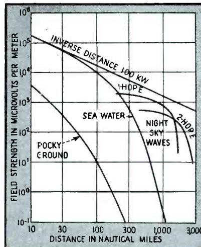
FIG. 4—Field strength as a function of distance from a 100-kw transmitter, over sea water and rocky ground. The 1-hop *E* sky waves can not be safely used beyond 1,400 miles because their strength falls rapidly below those of the 2-hop *E*
