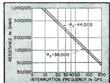
lator to the 72-mc oscillator results in a transmitted carrier having a pulsed or keyed characteristic, the frequency of which is determined by the resistance of the meteorological elements or reference resistors.
