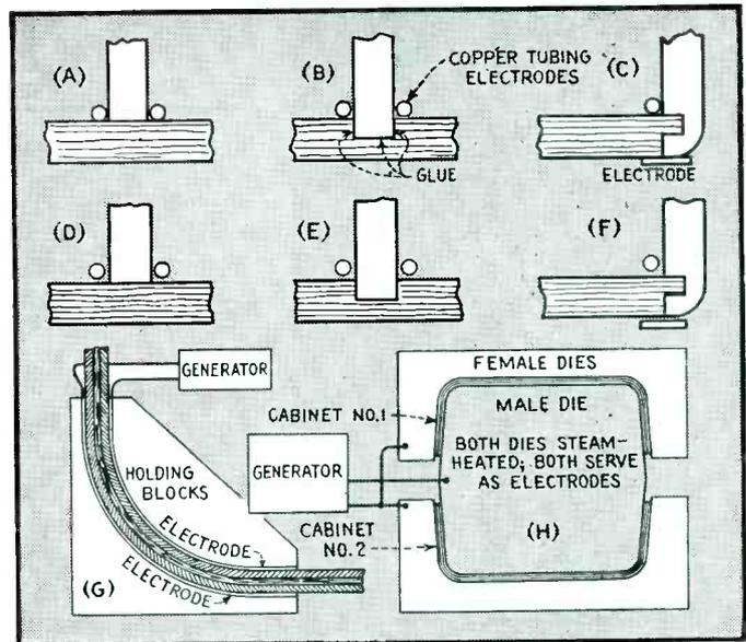
FIG. 6—Electrode arrangements for setting glue in joints
