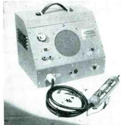
and variable gain control; used with the amplifier from which it obtains power it gives visual or audible signals at various points in the receiver circuit when the input to the receiver is energized by a signal generator.
