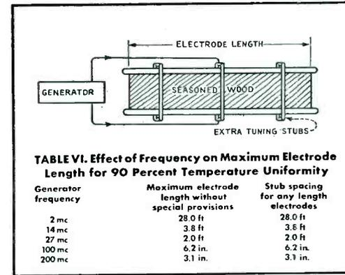
is considerably faster than conventional slotting and bending, and requires no block to be glued and clamped overnight. Several 15-kilowatt generators are now being used to set laminated chair and table frames in this manner, in about one minute.
