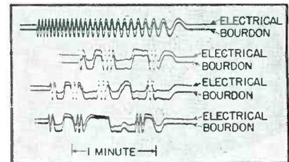
FIG. 5—Sample records of laboratory-generated waves, illustrating the ability of the electrical unit shown in Fig. 3 to reproduce complicated waveforms accurately by comparison with records obtained with a Bourdon gage and optical recording system
