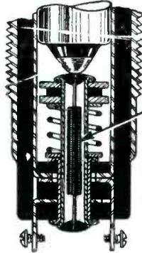
BUILT-IN RESISTOR HOUSED IN SPRING CONTACT EYELET
