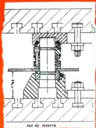
Sectional drawing illustrating simplicity of assembly of punch and die unit parts.
