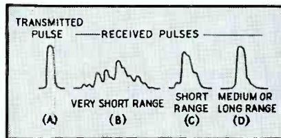
FIG. 11—Within 100 miles of a transmitter the pulses reflected from the *E* layer are complex and useless for accurate timing techniques. At 300-400 miles, the pulses have achieved sufficient stability
