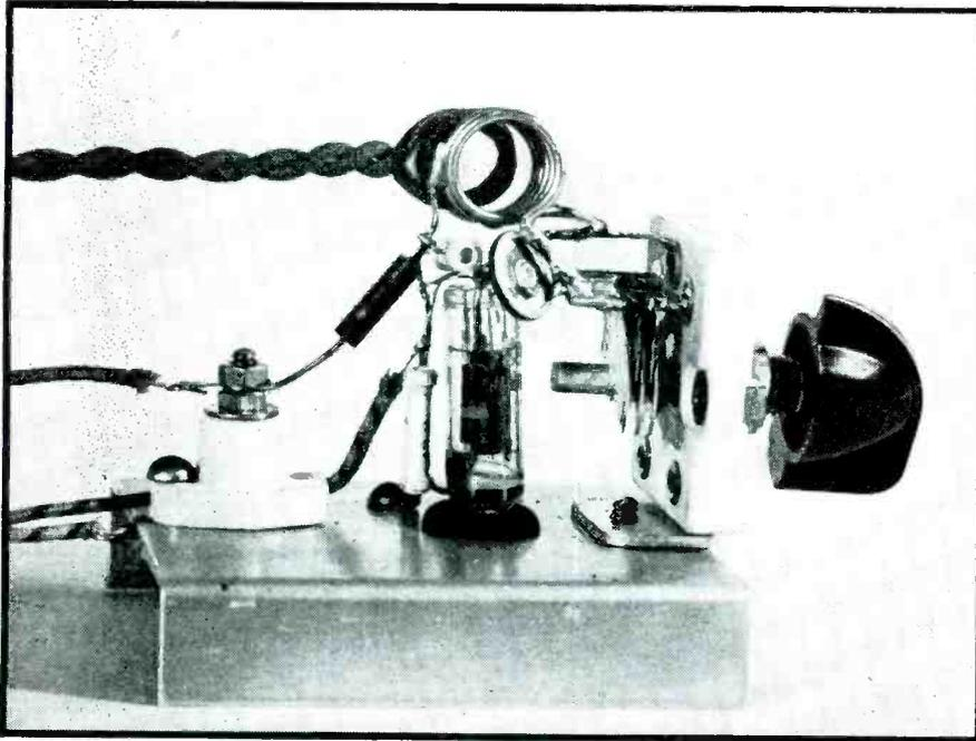
Full-size picture of the circuit diagrammed in Fig. 4 shows use of rubber grommet for shock mounting and compactness of circuit
