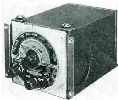
PAR-70A requires 2.5 amperes at 12 volts. The -70B type equipment requires 1.25 amperes at 24 volts. Overall size is 4½ x 5½ x 7 inches. The weight is 5 pounds, including a vibrator power supply. The loop antenna is 11 inches high, 9 inches in diameter and weighs 1.4 pounds including azimuth indicator and 6-foot transmission line.
