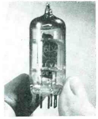
milliamperes; heating time, 30 seconds. The maximum voltage between elements is 450 volts. The maximum peak anode current is 100 milliamperes, maximum heater-to-cathode voltage ranges between +25 volts and -100 volts.
