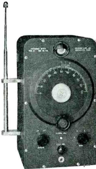
or f-m transmitters to an accuracy of 0.0025 percent. A telescoping antenna is employed to pick up radiated energy from the transmitter being checked. The unit measures 13 3/8 x 7 3/8 x 6 1/2 inches and weighs 15 pounds.
