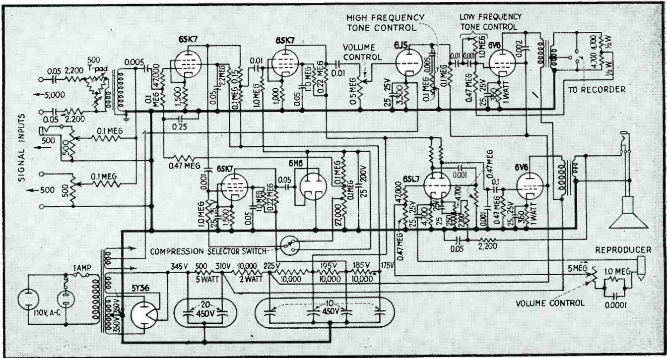
FIG. 3—Recording and reproducing amplifier circuit. Automatic volume compression, and high and low frequency compensation improve intelligibility of low velocity recordings
