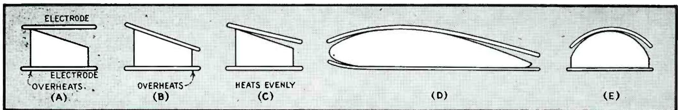
FIG. 3—Electrode contours for securing uniform heating of nonuniform thicknesses
