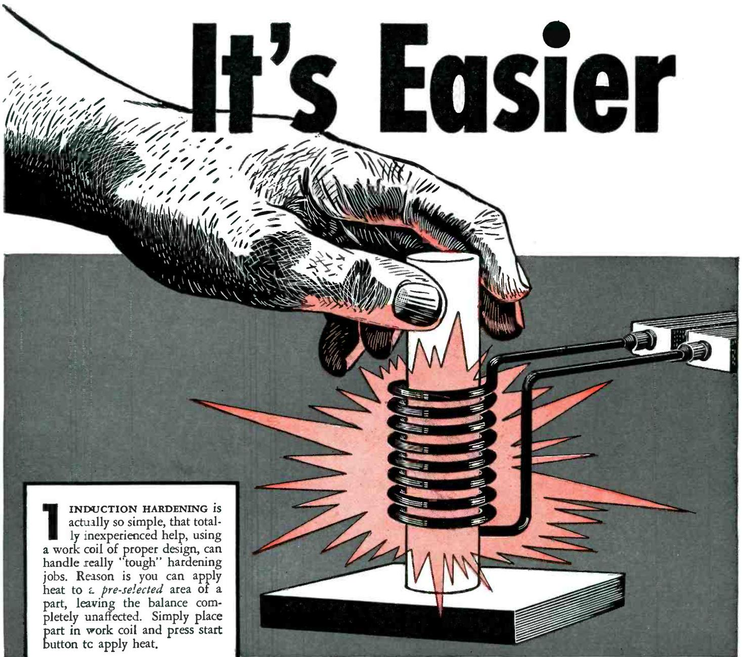
**1** INDUCTION HARDENING is actually so simple, that totally inexperienced help, using a work coil of proper design, can handle really "tough" hardening jobs. Reason is you can apply heat to a *pre-selected* area of a part, leaving the balance completely unaffected. Simply place part in work coil and press start button to apply heat.
