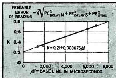
FIG. 14—The increasing value of the correlation factor, *K*, indicates that as the separation of transmitters increases, variations in delay tend to cancel less. This also shows that over great distances the ionosphere does not move uniformly
