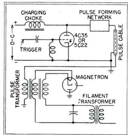
Circuit using a hydrogen thyratron in a line modulator arrangement for pulsing a magnetron
