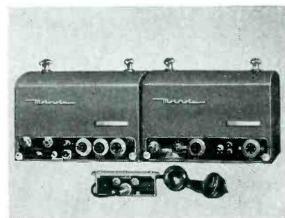
width of 60 kc at 6 db down, received signals in a field test with a 25 to 30 db signal-to-noise ratio. Mobile transmitters are similar to the fixed station but operate from a 6-volt vibrator power supply.
