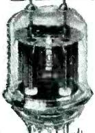
829-B push-pull R-F beam power amplifiers. Exceptionally efficient, with full input at frequencies up to 200 Mc. Max. ratings are: 750 plate volts, 40 watts plate dissipation. While they last...
