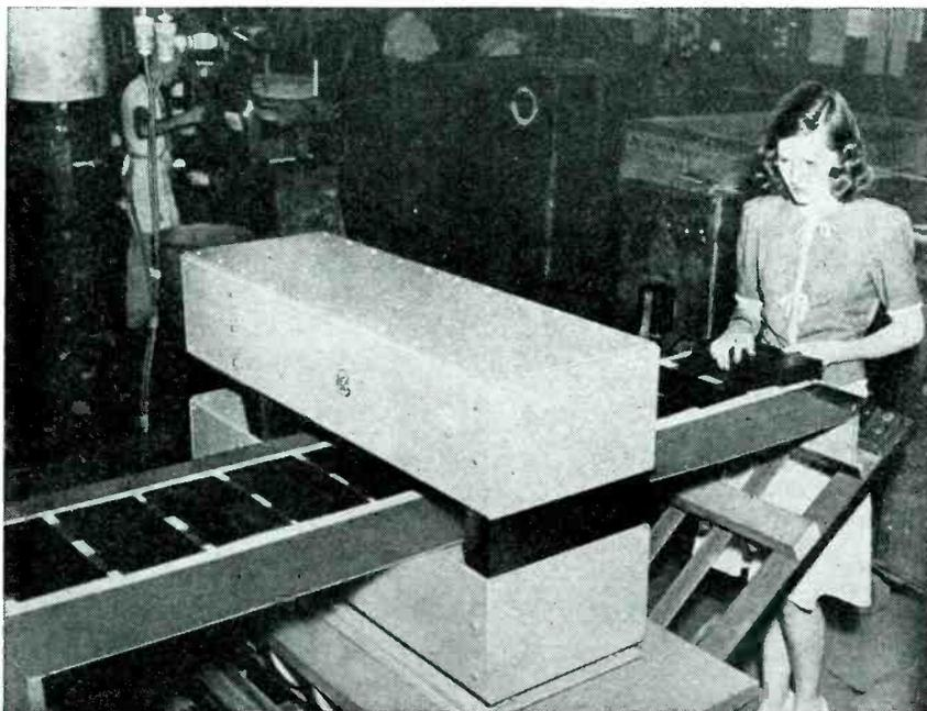
Plastic blanks are inspected for metal particles to prevent damage to dies used in pressing or molding. The blanks on the conveyor belt pass through an aperture where coils are embedded in surrounding panels
