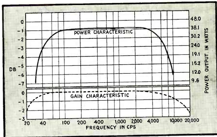
FIG. 4—Maximum undistorted power obtainable for a particular amplifier falls rapidly at low frequencies
