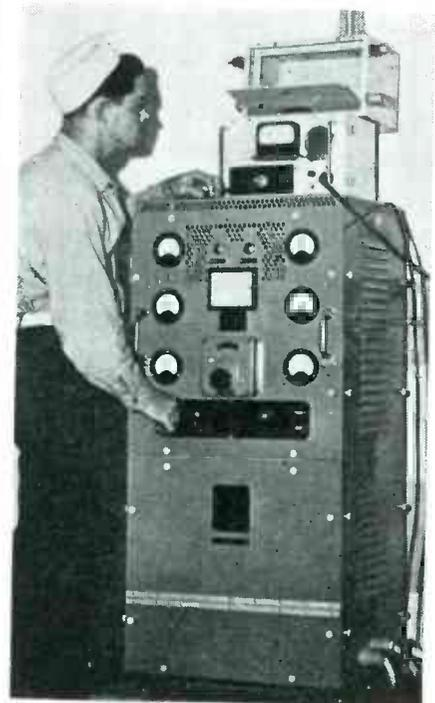
Driver unit of modern echo ranging sonar, being checked with portable test monitor. This unit energizes the magnetostriction transducer that sends the sound signal into the water
