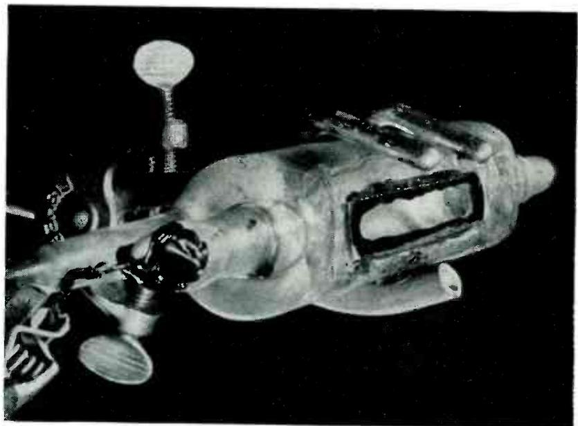
FIG. 2—Experimental detector tube containing a quartz radiation window in front of the cathode opening
