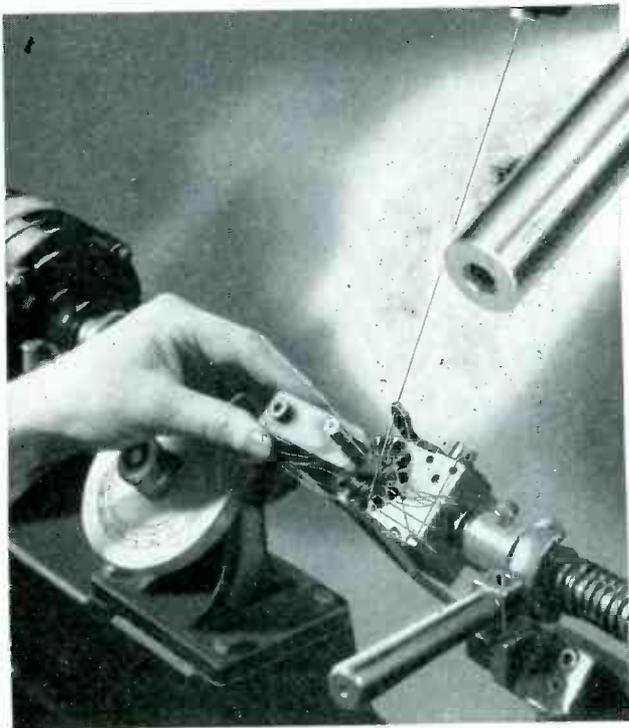
**H**IGH speed machine-winding of electric motor armatures necessarily exposes magnet wire to some rugged treatment. Insulating film must be *tough*, yet *pliable*. Copper must have the proper degree of anneal to "stay put" and insure uniformly filled slots and compact end-loops.
