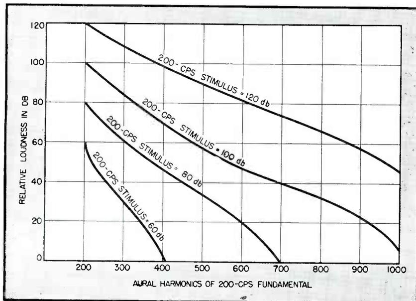
FIG. 3—Relative loudness of harmonics generated by the human ear when a stimulant 200-cps tone is applied at various intensity levels. The 2nd harmonic becomes important as the stimulus tone approaches 80 db, the third harmonic for 90 db, etc.
