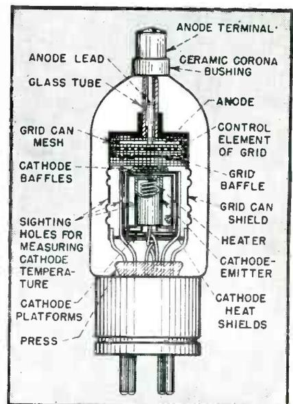
FIG. 3—Construction of type 4C35 hydrogen thyatron
