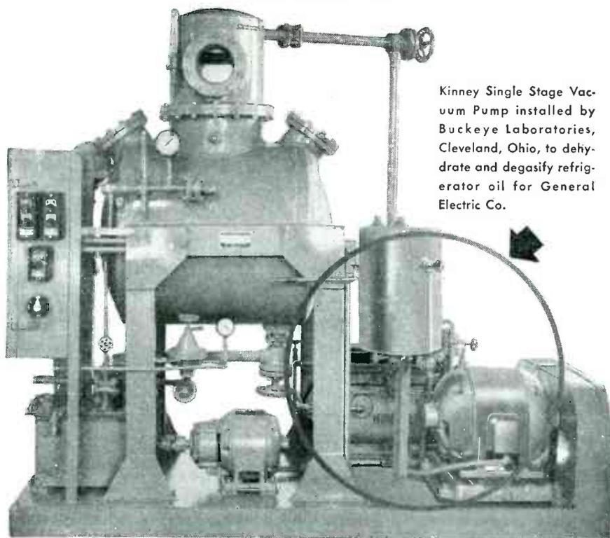
Kinney Single Stage Vacuum Pump installed by Buckeye Laboratories, Cleveland, Ohio, to dehydrate and degasify refrigerator oil for General Electric Co.
