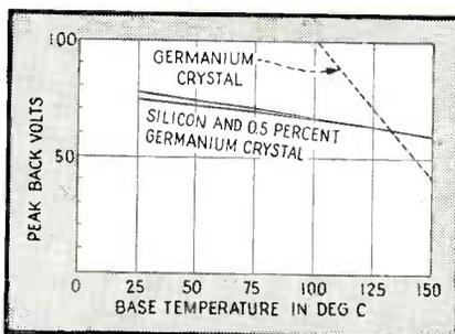
Fig. 7—A comparison of peak back voltage as a function of base temperature for two crystals of different composition
