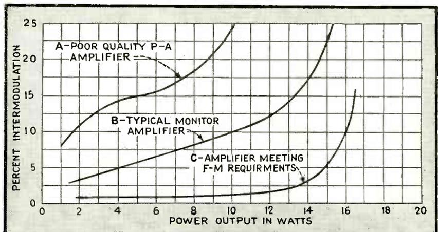
FIG. 3—Intermodulation tests indicate the increasing nonlinearity of amplifiers as they are called upon to handle larger signals
