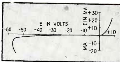
Fig. 6—The typical d-c characteristic curve of a high-back-voltage silicon crystal
