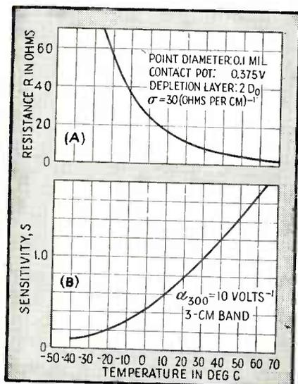
Fig. 5—Variation of resistance (A) and sensitivity (B) of a representative crystal with temperature
