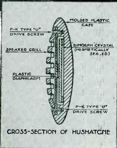
Recognizing the obvious cost advantages of P-K Type "U" Drive Screws over inserts or tapping for machine screws, The Brush Development Co. engineers came up with an idea for simultaneous driving that multiplied time saving. It also met tricky requirements for uniform holding pressure to insure a lasting, liquid-proof seal that would permit sterilization. They report "no failures due to leakage or loose screws".
