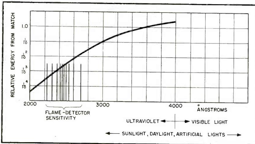
FIG. 1—Spectral distribution of sunlight, daylight, artificial light sources, energy radiated from a match, and sensitive region of flame detector
