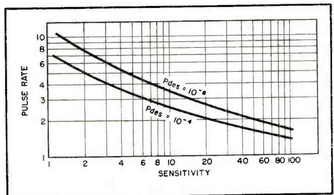
FIG. 6—Relationship of background pulse rate of detector and optimum sensitivity
