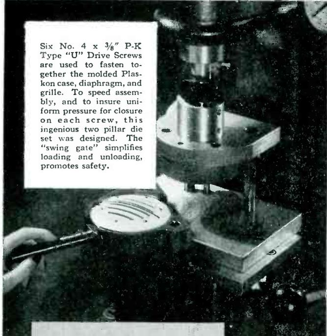
As the die closes, a pilot pin in the top shoe brings the matrix in location for accurate register of driving punches. Each of the punches is preloaded to over 580 lbs. pressure, requiring a total load of about 1 3/4 tons. Driving pressure is uniform on each screw, avoiding residual strains, but assuring a watertight closure.
