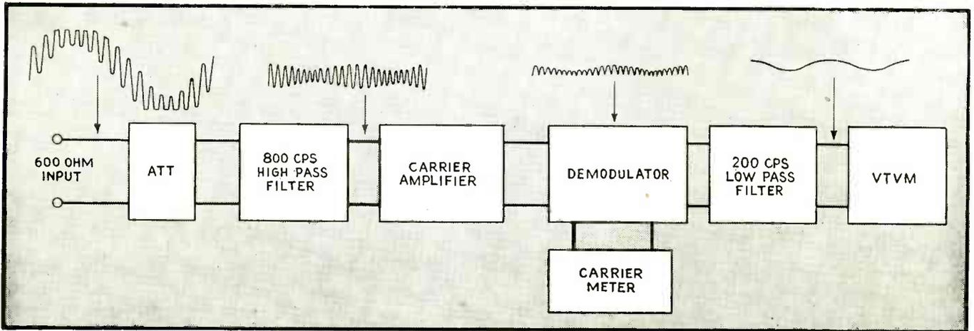
FIG. 2—Intermodulation analyzer detects high frequency modulation developed by nonlinearity of amplifier under test. (Word just received from author explains that 1,000 cps in test oscillator has been replaced by 2,000 cps so that analyzer accepts more sidebands—bandwidth is now 500 instead of 200 cps—eliminating tendencies for cancellation of sidebands of 100 cps.)
