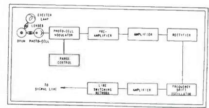
Block diagram of facsimile transmitter when using frequency-shift modulation. Similar stages are used for amplitude modulation but a re-keyer circuit is substituted for the frequency-shift oscillator.
