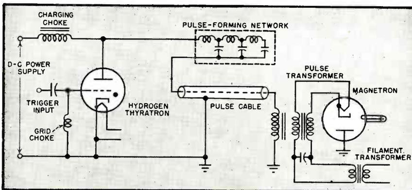
**FIG. 4—Practical line modulator circuit employing a hydrogen thyatron to drive a magnetron oscillator**
