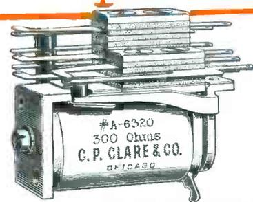
**Type "K" d.c. Relay.** This relay is outstanding for its speed of operation as well as for extremely small size (1½" x 1¼" x 13/16"). Operating voltage is up to 115 volts d.c.
