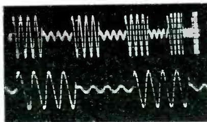
FIG. 7—Both beams are deflected by the same signal here, but one sweep is compressed by attenuating the sweep voltage
