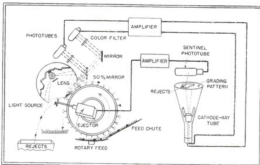
Essential elements of the electronic bean sorting system. A partial mask provides a grading pattern on the screen of the c-r tube
