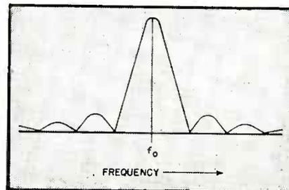
FIG. 11—Radio-frequency output spectrum of an oscillator pulsed by a rectangular pulse, as computed by Fourier analysis. At 10,000 mc the spread of the central lobe is of the order of a few megacycles
