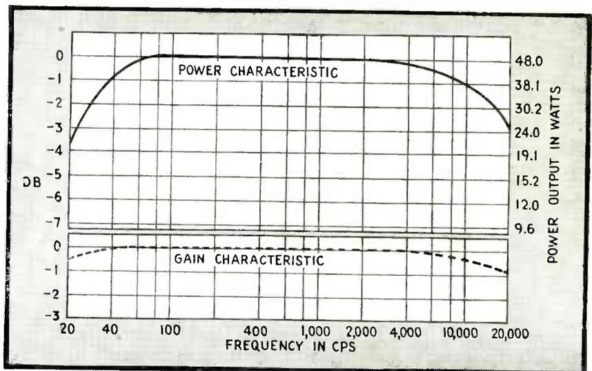
FIG. 6—Although not rated for as high power as the amplifier of Fig. 4 and 5, this amplifier has better high and low frequency response
