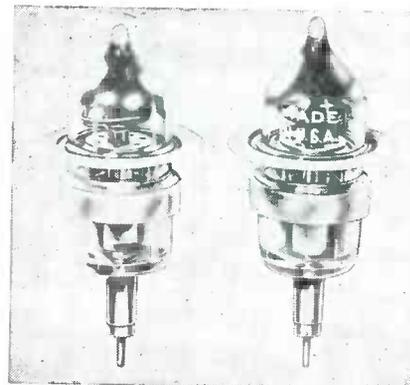
industrial electronic control, inspection and sorting applications. The new tubes feature streamlined cathode assembly, planar grids, minimum interelectrode capacitance, minimum transit-time effect and low power-input requirements. The type 2C36, shown at left, and type 2C37, shown at right, measure only 2 1/2 inches overall.
