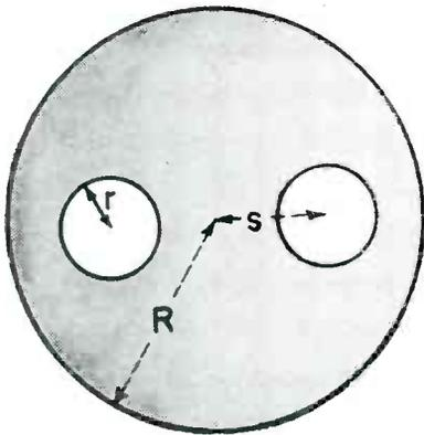
Comparison of three equations for  $Z_0$  of a balanced two-wire transmission line with a cylindrical shield, and expressions for the errors in the equations
