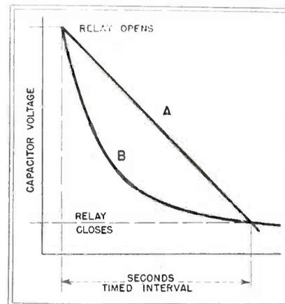
Fig. 2—Time-discharge relation showing the advantage of the linear discharge A over the logarithmic discharge B of a conventional R-C circuit
