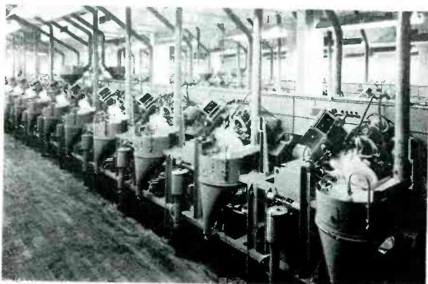
Billions of beans pass through this plant of the Michigan Bean Company where RCA phototubes and cathode-ray tubes control a sorting mechanism that separates good little beans from bad ones. Mirrors and lenses are used with the phototubes to judge the color range of each individual bean
