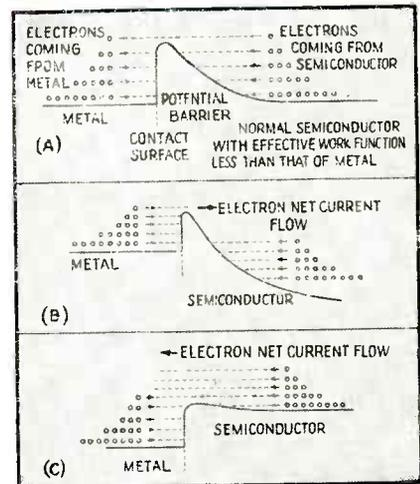
Fig. 2—Schematic diagram showing contact between metal and germanium semiconductor. In A, no voltage is applied, and hence the two electron flows are just equal. At B, the semiconductor has been made positive, lowering its electronic potential and decreasing electron current from the semiconductor, so that a slight net current flows. The semiconductor has been made negative at C, raising its electronic potential and increasing current from the semiconductor
