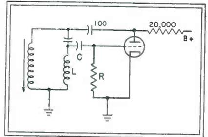
Fig. 2—This simplified circuit provides less hum sensitivity than that shown in Fig. 1
