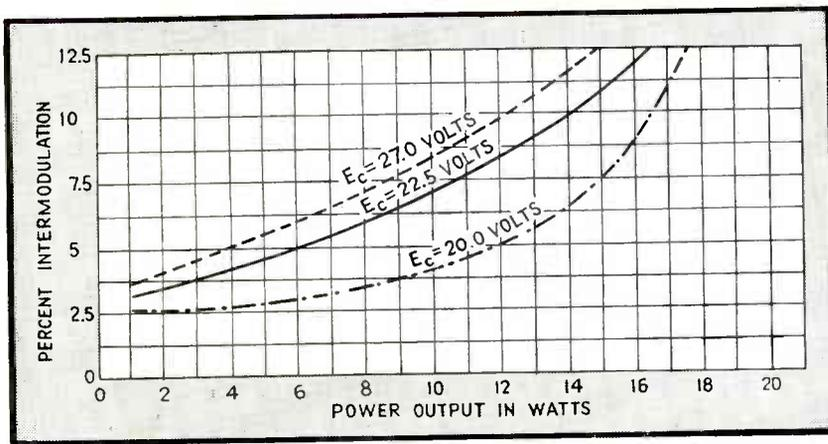
FIG. 8—Effect of cathode bias on linear operation of output tubes is shown by intermodulation tests
