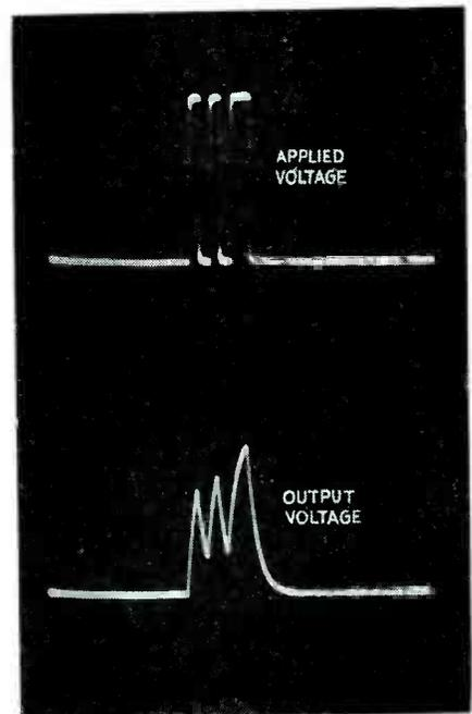
FIG. 5—Reproductions of patterns seen on c-r tube screen when using the system to determine the transient response of an RC network to an applied voltage consisting of three rectangular pulses
