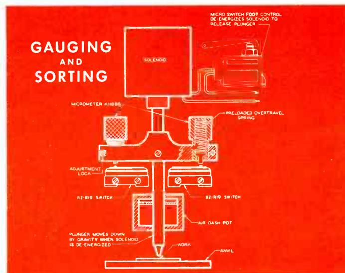
This is an example of how two of these new switches and one die cast enclosed type switch, in combination with a solenoid and micrometer knob, are used by one manufacturer in the gaging and sorting of mica. Micro Switch products, plus the extreme care used by the manufacturer in building the other parts, resulted in a reliable time and money saving tool.
