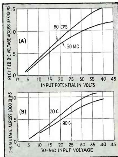
Fig. 9—Rectified d-c from a high-back-voltage silicon crystal as a function of input voltage as affected by frequency (A) and temperature (B)
