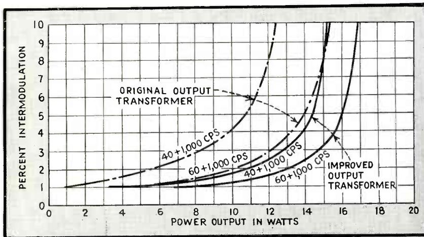
FIG. 9—Intermodulation testing shows the importance of the output transformer at low frequencies
