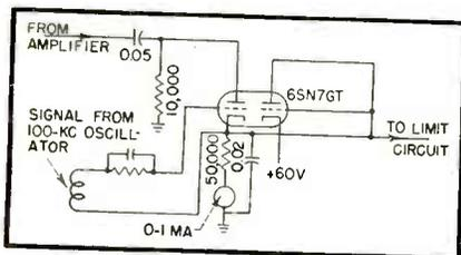
FIG. 2—The rectifier and meter protection circuit is arranged to simplify the mechanical problems in the gage head. It also avoids ambiguity in the readings by feeding a phasing signal from the 100-kc oscillator onto the grid of the rectifier tube
