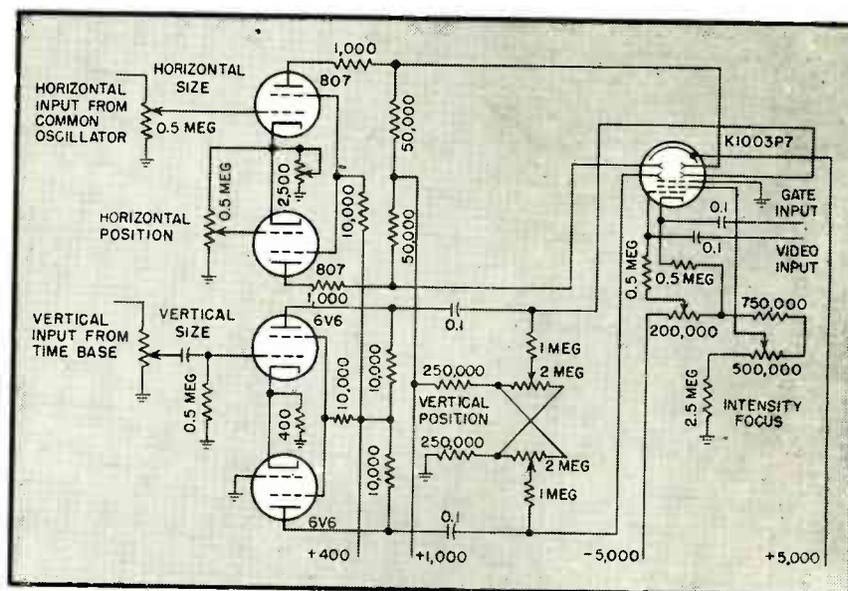
FIG. 6—Simplified schematic diagram showing the signal inputs to the plates of the cathode-ray tube indicator used to display the ionosphere characteristic information
