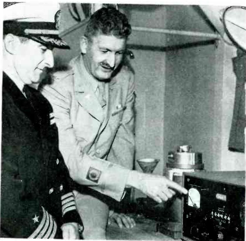
Radioactivity of seawater caused by atomic bomb test at Bikini will be measured by this electronic equipment. Geiger counter output is amplified and used to operate an indicating meter. Col. S. Warren, Radiological Safety Advisor to Joint Task Force One, shows Capt. A. C. Thorington what the indications will mean in terms of personnel safety
