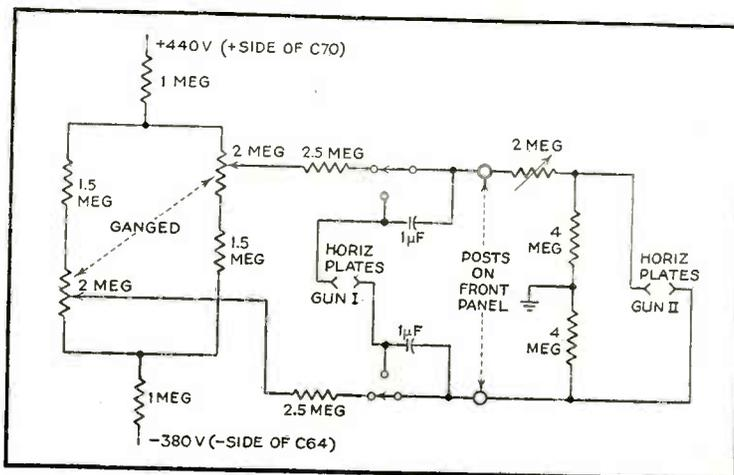
FIG. 5—Components added to type 247 oscilloscope for horizontal switching and for positioning of extra electron beam independently of normal beam
