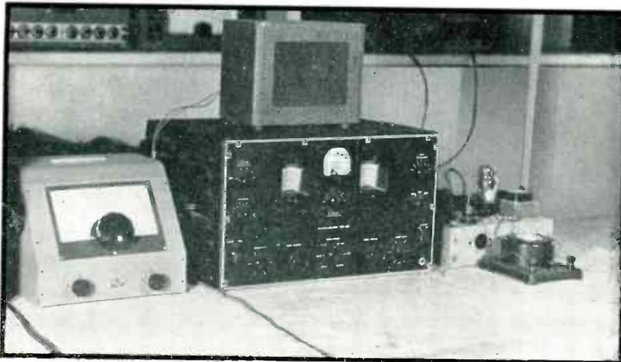
Left to right, the controlled multivibrator unit, receiver for reception of WWV, and a d-c amplifier and counter for determining the beat frequency. The large dial on the multivibrator is the fine frequency adjustment, the other two knobs control the input and output signals
