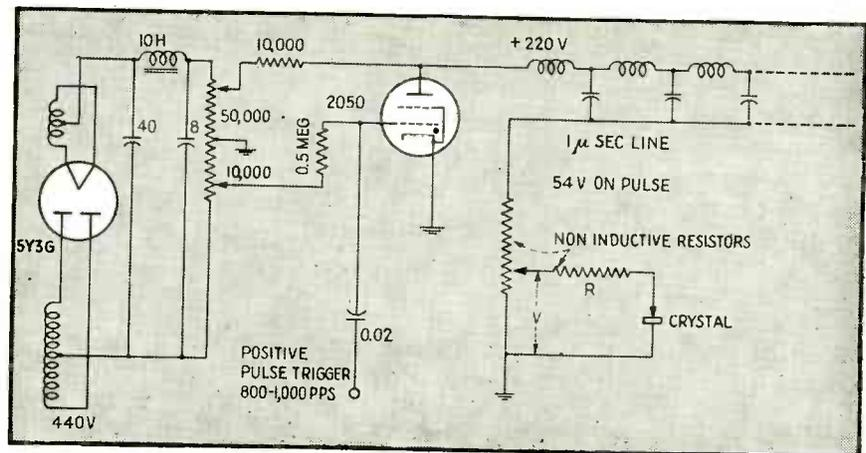
Fig. 12—The d-c pulser circuit used in the burnout tester
