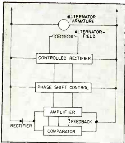
FIG. 1—Block diagram showing the operating principle of the single-phase device
