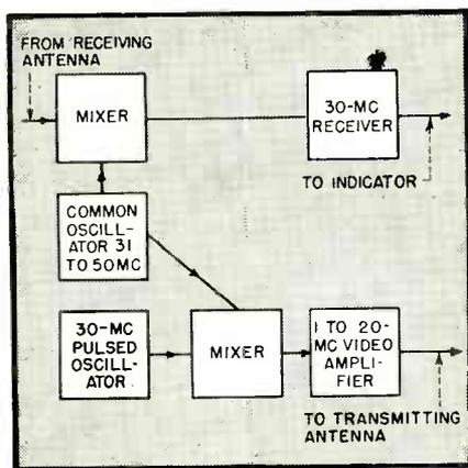
FIG. 1—Block diagram of the ionosphere sounding equipment, showing the common oscillator
