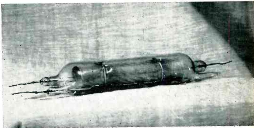
FIG. 3—Final design of fire-detector tube that is sensitive in all directions. The special glass envelope provides about 80 percent transmission at a wavelength of 2600 Angstroms
