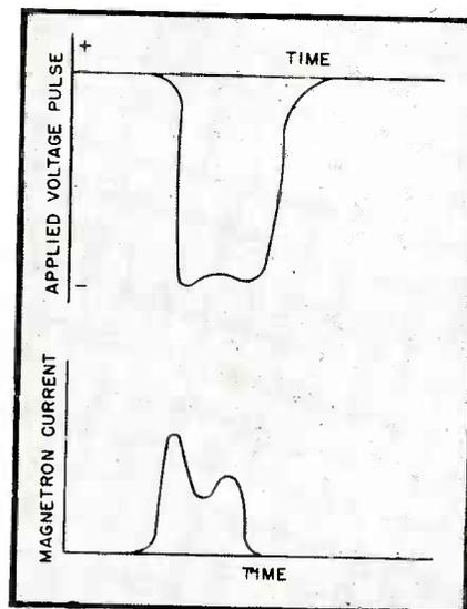
FIG. 12—Effect of a poor voltage pulse on magnetron current pulse shape, showing how a slight irregularity in the bottom of a voltage pulse is magnified in the current pulse
