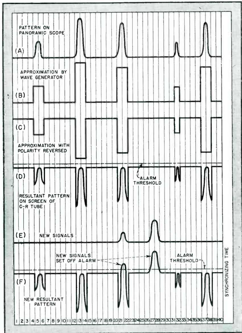
FIG. 2—Step-by-step illustration of how a panoramic receiver pattern is cancelled by the 40-control wave generator. Note that a new signal triggers the alarm even though it is directly on the frequency of a cancelled signal
