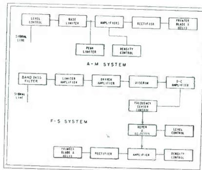
Essential stages of Press Wireless facsimile recording equipment for both amplitude modulation and the frequency-shift method
