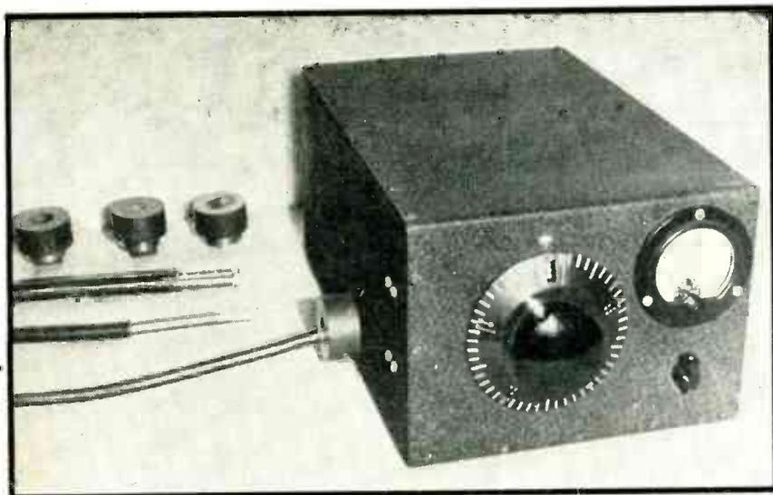
An odd quarter, electrical wavelength of line is inserted in the instrument. The single dial simultaneously tunes both oscillator and indicator. When the meter indicates resonance by maximum reading, the frequency indicated on the dial is proportional to velocity of propagation
