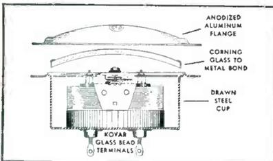
Exploded view of Marion instrument, showing how it is sealed like a vacuum tube with Corning metallized window, soldered into place.
