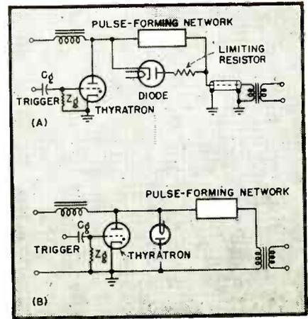
**FIG. 7—Two circuits for protecting a line modulator against magnetron sparking**
