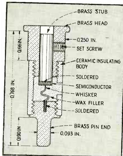
Fig. 1—Cross-section of a typical crystal rectifier. The dimensions are approximate
