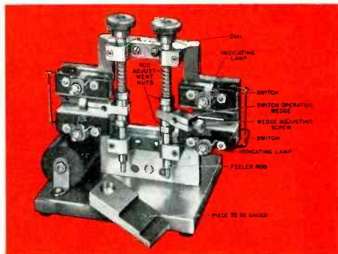
While you can employ this switch in building your own gages, we wish to point out that accurate gaging will be attained only as the other parts of the gage embody the same precision as the switch itself. The above illustration shows how four of these new switches are used in a specially built gage used by Micro Switch to insure close tolerances in the manufacture of this new switch, as well as other Micro Switch products.
