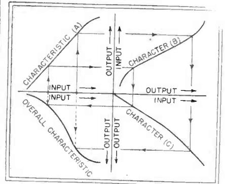
A graphical method is used to find overall characteristic of channel when transfer characteristic of each element is known, or to determine required characteristic of an equalizer to produce desired overall characteristic. For example, if the microphone has characteristic A, the film gamma a character B, and the reproducing system a character C, then the overall channel characteristic of a film recording system is as shown
