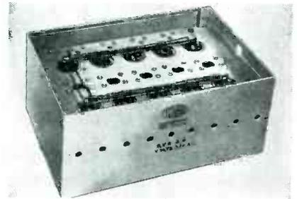
connected for either single-phase or three-phase operation. The capacitor sections, which are impregnated with mineral oil and hermetically sealed in oil-filled metal cases, show little drift through wide ranges of temperature, and are said to be capable of continuous operation at temperatures ranging as high as 75 C. Overall dimensions of the unit are 9 3/4 x 6 1/4 x 14 inches.
