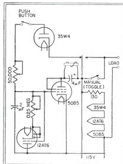
Fig. 1—Time intervals from 1/2 second to 30 seconds are provided by this electronic relay circuit
