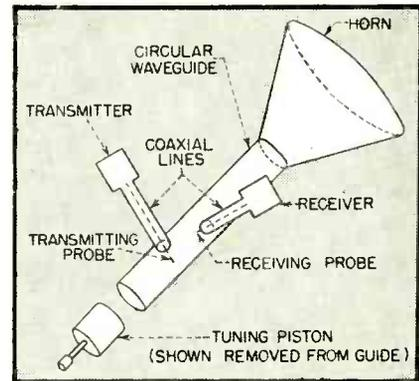
FIG. 1—Placing transmitting and receiving probes at right angles in a circular waveguide, as shown here, permits simultaneous transmission and reception
