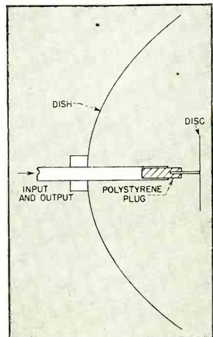
FIG. 2—Use of adjustable plug to control crystal current
