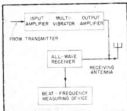
FIG. 1—Functional block diagram of the monitoring system
