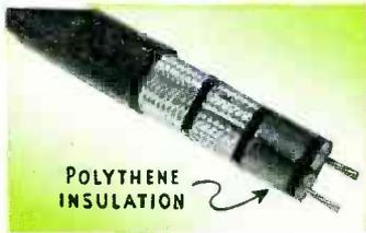
**CUT-BACK SECTION** of a modern twin coaxial cable for use in direction-finding equipment at ultra-high frequencies (400 to 10,000 megacycles). JAN-C-17 designation RG-23/U; made by Anaconda Wire & Cable Co. The insulation, about 140-150 mils thick, is Du Pont polythene.
