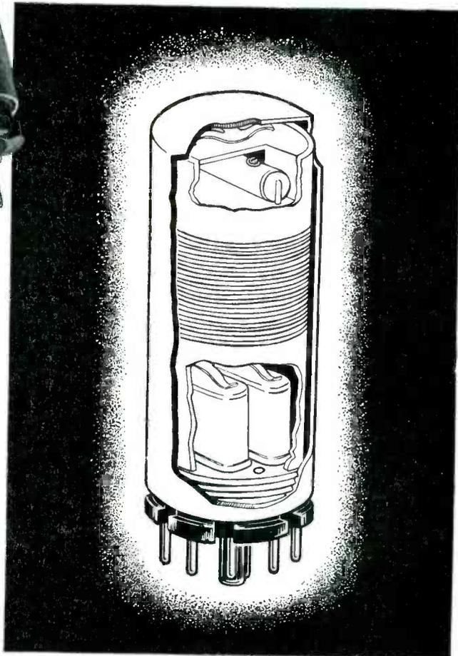
*4 m.c. to 8 m.c. crystals can be placed in these holders.*
