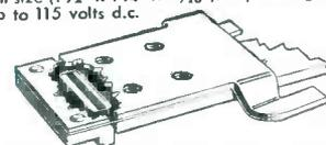
**Special Type "K" Hinge.** Uniform armature movement is assured by a hinge of "fatigueless" beryllium copper, heat treated and designed to provide a wide margin of safety.
