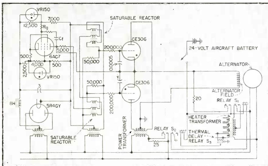
FIG. 3—Circuit of the single-phase, variable-frequency unit
