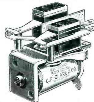
**With Mycalex Insulators.** Type "K" Relays are available with spring insulators of 1/8" Mycalex for high frequency circuits. Each relay is given a 1000 volt a.c. insulation breakdown test.
