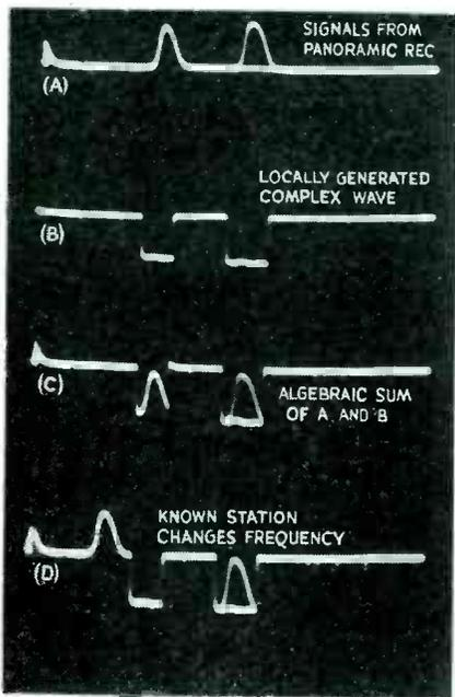
FIG. 3—Reproduction of patterns on screen of c-r tube, illustrating how a shift in the frequency of a signal is readily recognized
