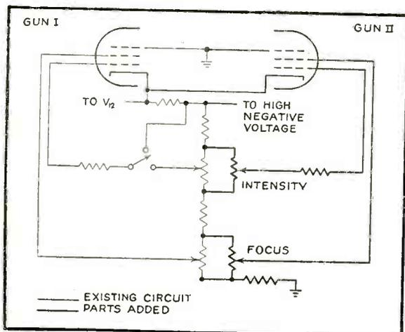
FIG. 4—Heavy lines show components added to DuMont type 247 oscilloscope for contact of extra gun
