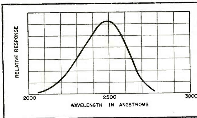
FIG. 4—Spectral sensitivity of copper-cathode detector
