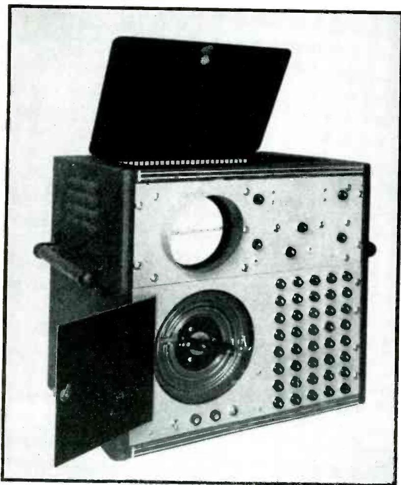
Final model of the wave generator, alarm system, and scope built as a single unit, ready for connecting to the output of any panoramic receiver. By adjusting the 40 control knobs while watching the resultant pattern on the cathode-ray tube screen, the output of the complex wave generator can be shaped to cancel exactly any pattern appearing on the screen
