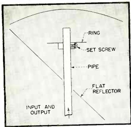
FIG. 3—Control of crystal current with sliding ring on circular waveguide
