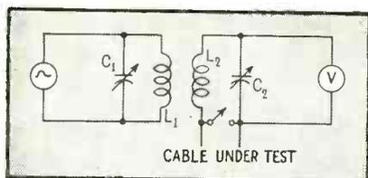
FIG. 1—Frequency is adjusted until cable under test presents a short circuit to the instrument
