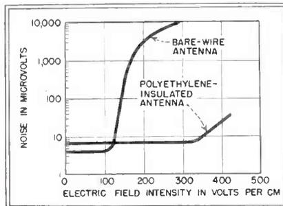
Effect of antenna insulation on radio noise due to precipitation static
