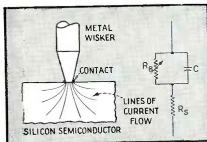
Fig. 10—Lumped parameter circuit to approximate crystal contact.  $R_B$  and  $C$  are resistance and capacitance of the contact and  $R_S$  is the spreading resistance in the semiconductor caused by small area of contact
