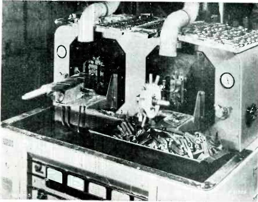
At left is a magnetic chuck block holding a large drill for induction brazing of tungsten carbide tip. The tips on small tools are held in place by the adhesion of the brazing material. At right, a rotary fixture holds seven tools ready for brazing
