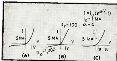
Fig. 4—The experimentally observed current-voltage curve at A agrees reasonably well with the curve deduced from front and back resistance constant at B and that from diode theory at C
