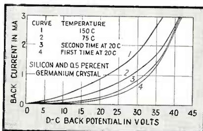
Fig. 8—D-c back voltage characteristic curves at different temperatures for the silicon crystal shown in Fig. 7
