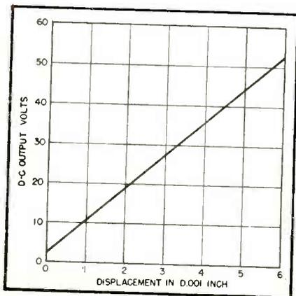
FIG. 3—The output voltage from the rectifier to the indicating meter is a linear function of the gage spindle displacement, but the curve does not pass through the origin
