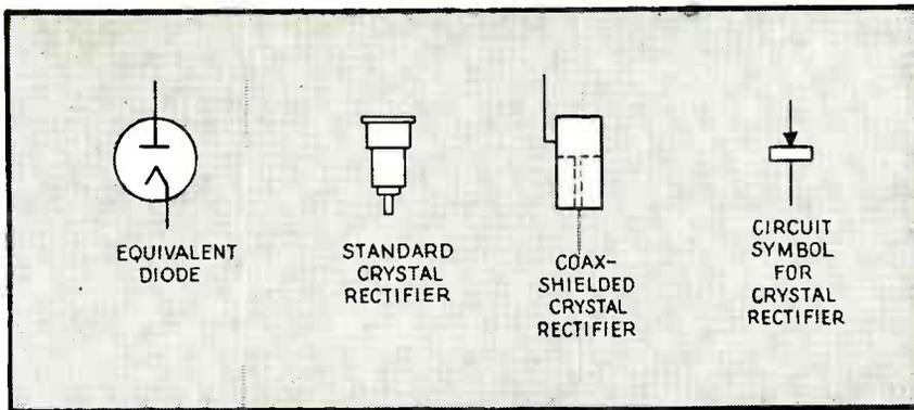
Symbols for diode and crystal rectifiers and the physical appearance of corresponding crystal units. The greatest current will flow when the top connection is positive
