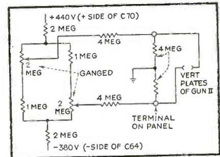
FIG. 8—Components added to type 247 oscilloscope for vertical positioning of the extra beam. The source for vertical deflection must tolerate a d-c voltage and must not be too low in resistance
