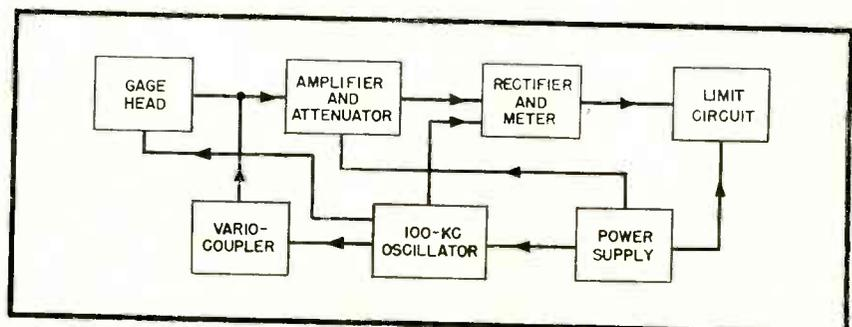
FIG. 1—Block diagram of the principal circuit elements used in the comparator gage. The variocoupler is used to set the indicating meter to zero center. The limit circuit flashes colored lights to show whether the work being gaged is under or over size, while the meter shows exactly how much
