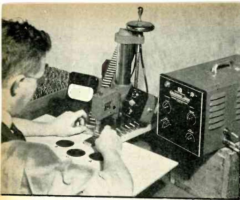
Complete electronic comparator gage in use for the production gaging of roller bearings. The principal circuits used to convert spindle displacement to meter reading and lamp indication are contained in the box at the right
