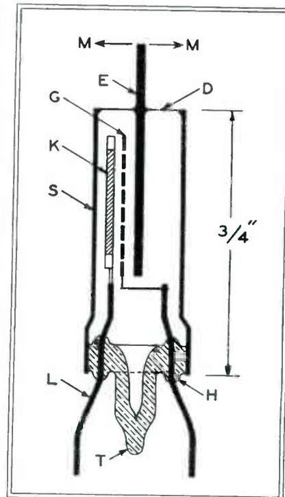
Construction of the new Vibrotron tube. Motion of the movable anode E in direction M-M is transferred through the thin metal diaphragm D to produce a proportional change in electron flow of the triode formed by K, G, and E. The envelope S is metal and leads such as L are brought out through a vacuum-tight glass header H with exhaust tip T
