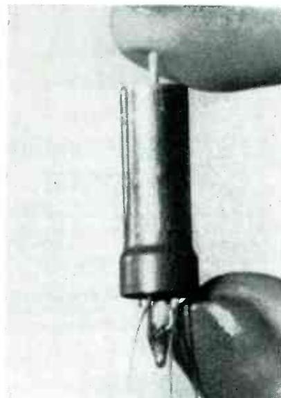
Close-up of the Vibrotron tube for converting mechanical motion to a variable electron flow. The movable anode appears at the top
