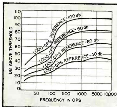
FIG. 2—Curves showing how response of human ear varies with intensity of sound. Each curve is for a definite loudness sensation to the ear, and shows the actual intensity in db above threshold required to produce that loudness sensation at various frequencies. The curves were obtained in each case by starting with a desired loudness sensation (40, 60, 80, and 100 db) at 1000 cps, hence in each case sensation and intensity are the same at this reference frequency
