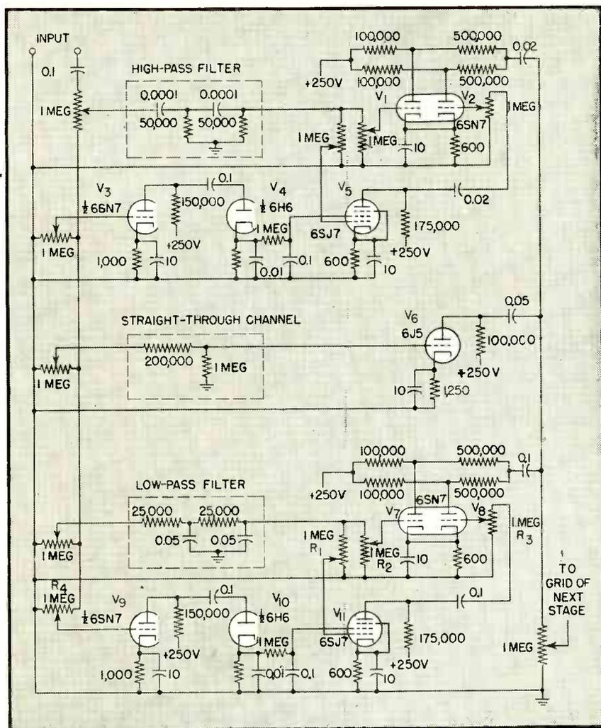
FIG. 1—Inverse volume-expansion circuit for automatic tone control compensates for changes in the response of the human ear at different intensity levels
