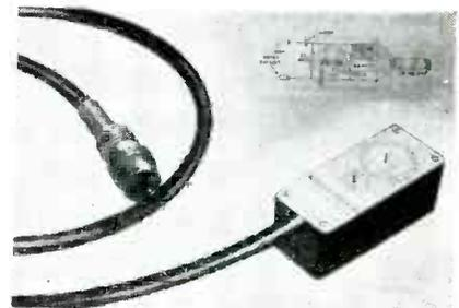
quency probe. Most existing probes have an input capacitance of 5 micro-microfarads or more. The effect of loading and detuning of very high frequency circuits is therefore greatly reduced in the new probe which has an input capacitance of
