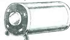
**Small Type "K" Coil.** Type "K" coils may be single or double wound. Screw holding coil in heelpiece is equipped with split-type lock washer. Coils may be supplied impregnated.
