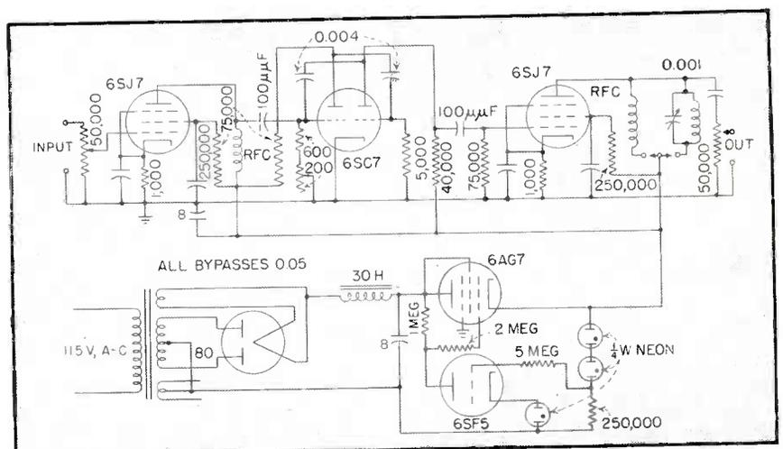
FIG. 2—Complete circuit of the multivibrator unit
