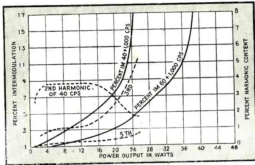
FIG. 5—Intermodulation and harmonic distortion of the amplifier whose characteristics are given in Fig. 4
