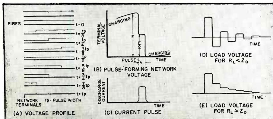
FIG. 5—Voltage and current waveforms in a line modulator circuit
