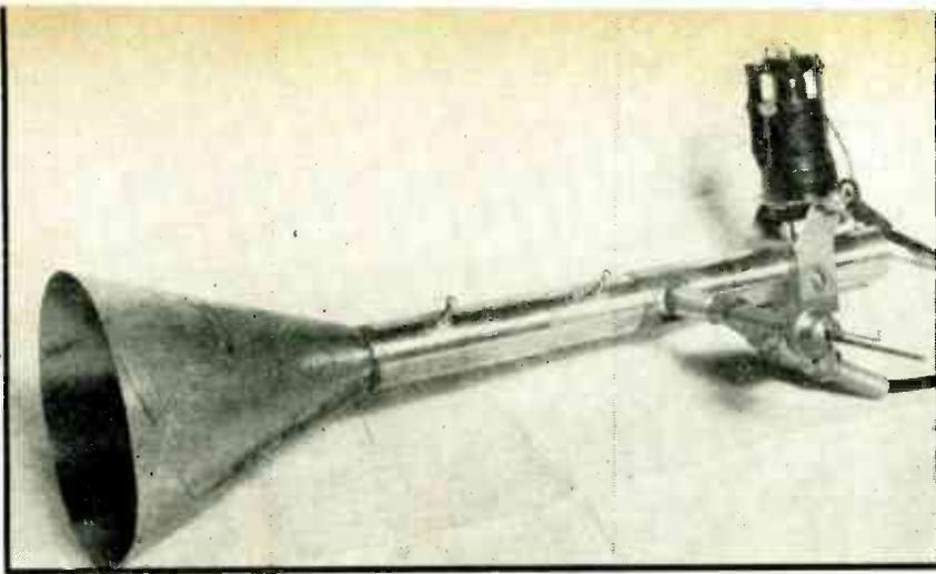
A 3-cm wave system as in Fig. 1, plus tuning screws and telescoping (line stretcher) section to produce rotary polarization and provide control of crystal current
