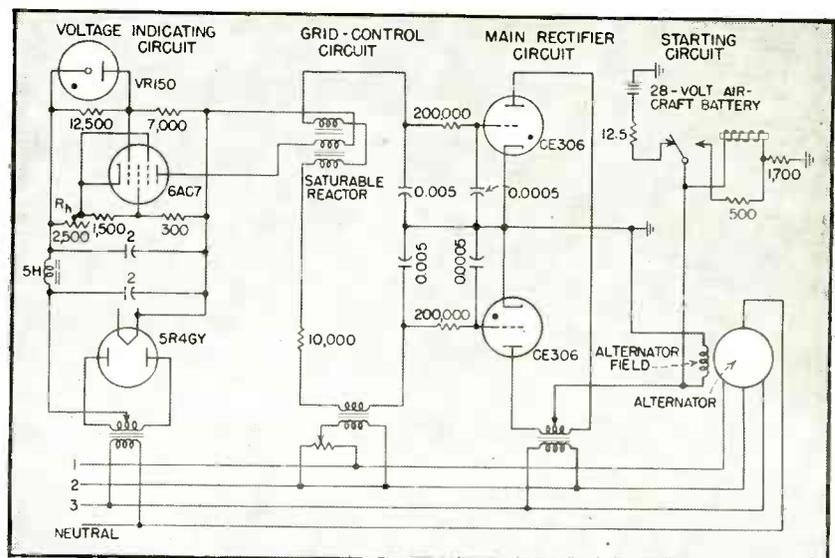
FIG. 2—Schematic of the three-phase, constant-frequency system
