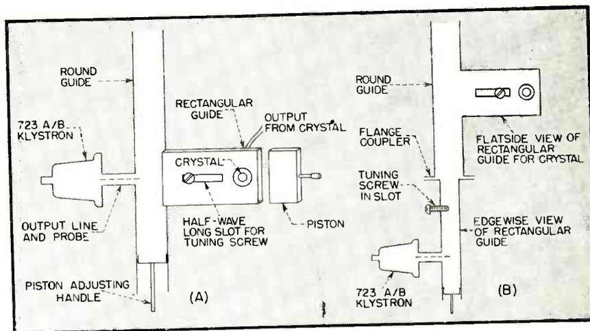
FIG. 4—Use of rectangular guide instead of probe to take off power for crystal detector (A) and to couple a klystron to the round guide (B)
