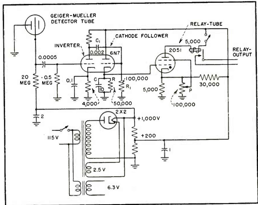
FIG. 5—Fire-detecting trigger circuit which fires thyatron when received impulses due to far ultraviolet radiation cause potential across capacitor C to rise above a predetermined value
