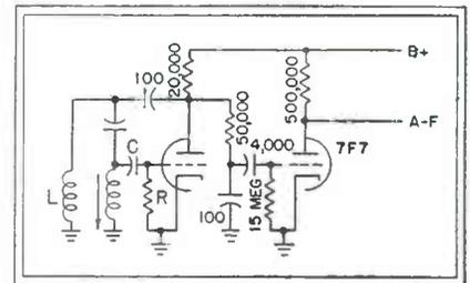
Fig. 1—Circuit arrangement of the modulated-oscillator pickup
