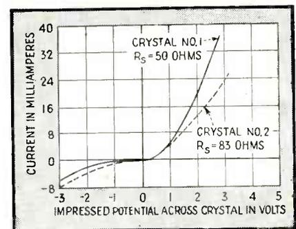
Fig. 3—Current-voltage curves for two different crystals
