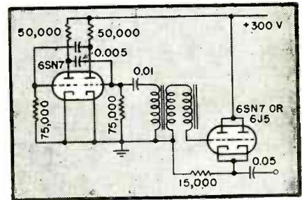
**FIG. 9—Compact trigger generator circuit recommended for use with 4C35 and 5C22 hydrogen thyatrons**
