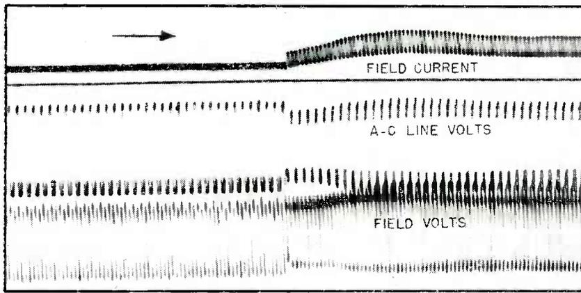
FIG. 4—Oscillogram showing the performance of the variable-frequency exciter-regulator upon application of a sudden 68-ampere, 0.8 power-factor load at 510 cycles
