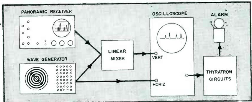
FIG. 1—Block diagram of system. When properly adjusted, arrival of a new signal at the panoramic receiver makes the alarm bell ring
