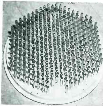
Diaphragm of sonar transducer, showing nickel magnetostriction tubes. Energizing coils are wound around the individual tubes
