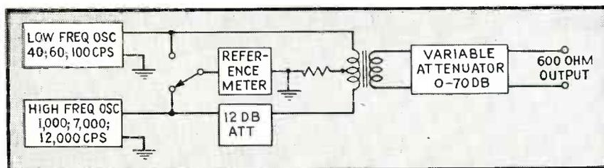
FIG. 1—Signal generator for intermodulation testing consists of two independent oscillators and a linear circuit for mixing their outputs
