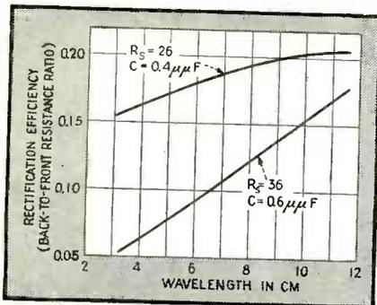
Fig. 11—Rectification efficiency (back-to-front resistance ratio) of two different crystals as a function of wavelength. The lower curve shows the effect of larger contact capacitance
