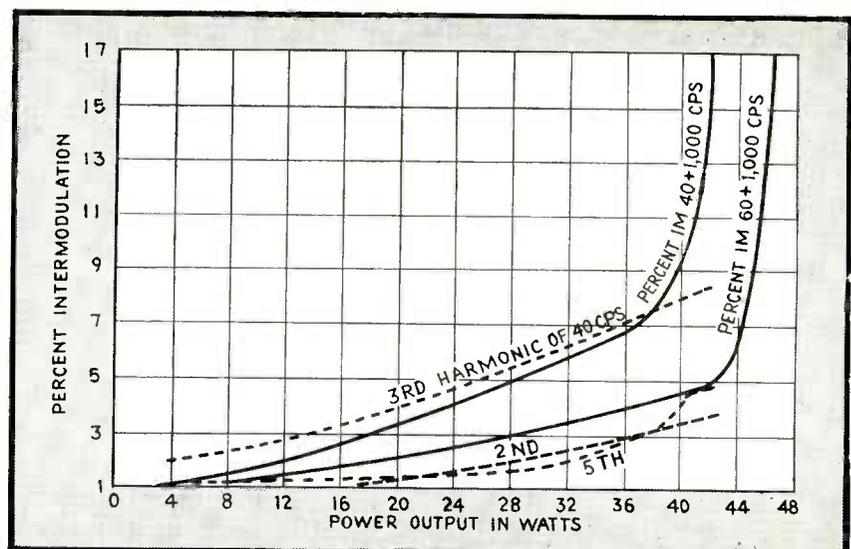
FIG. 7—Intermodulation distortion of the amplifier whose characteristics are shown in Fig. 6 remains low up to its rated output power
