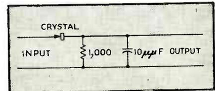
Fig. 13—Circuit used for measuring second detector characteristics
