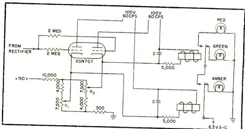
FIG. 4—The desired limits to the deviation from a standard are quickly adjusted by setting the positions of potentiometers  $R_1$  and  $R_2$ . This is a simple operation which can be rechecked at any time, correlating a meter reading with the flashing of the appropriate limit lamp
