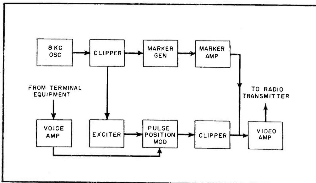
FIG. 3—Block diagram indicates sequence in which one channel of the voice signal position-modulates the pulses for transmission
