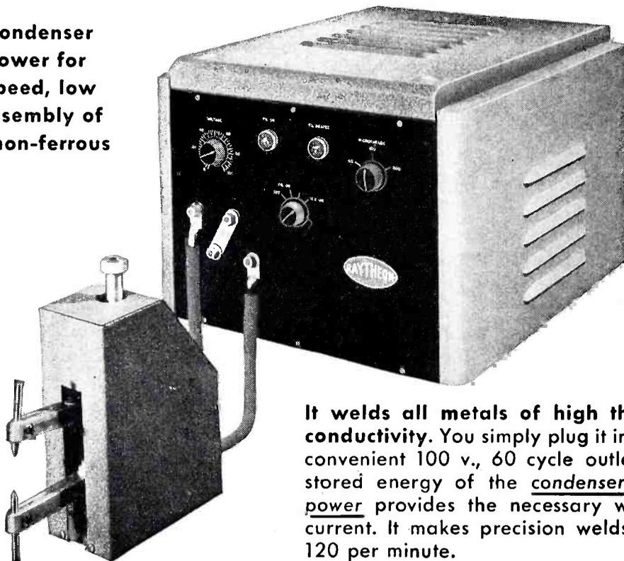
It welds all metals of high thermal conductivity. You simply plug it into any convenient 100 v., 60 cycle outlet. The stored energy of the condenser weldpower provides the necessary welding current. It makes precision welds up to 120 per minute.
