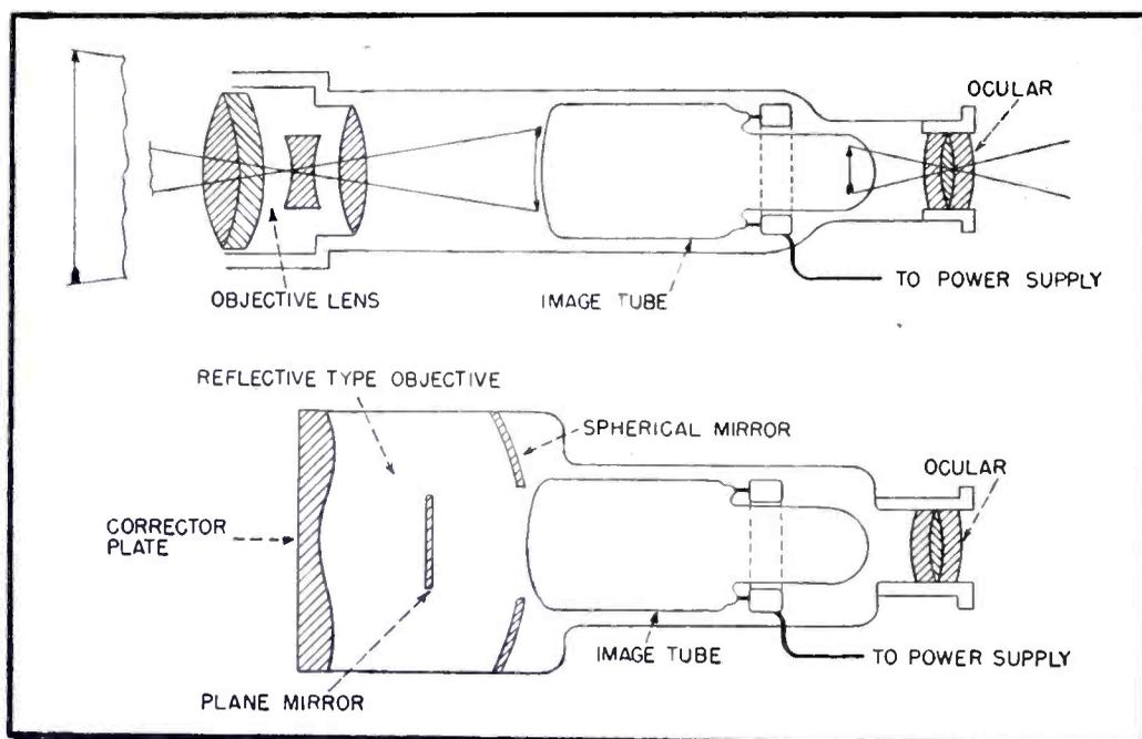
FIG. 1—Schematic diagrams of two infrared telescopes using the 1P25 tube. The refractive system at top is useful for short range; the reflective type is more suitable for long range
