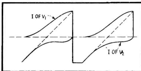
FIG. 5—The combination of the current through the damping tube and the output tube form a linear total current (dashed line)
