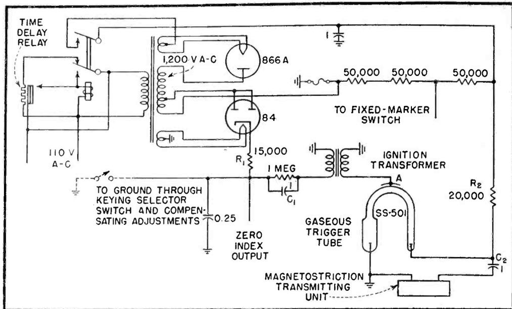
FIG. 3—Circuit diagram of driver unit, showing use of two diode rectifiers to charge capacitors  $C_1$  and  $C_2$ . Discharge of  $C_1$  by keying contacts ionizes trigger tube, allowing  $C_2$  to discharge through magnetostriction unit and shock-excite it into vibration at its mechanical resonant frequency of 21.5 kc to produce the desired supersonic signal
