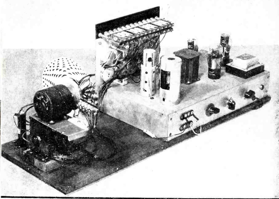
Rear view showing tone wheel and its driving motor, with the ten tiny projection lamps mounted on the bracket just behind the tone wheel
