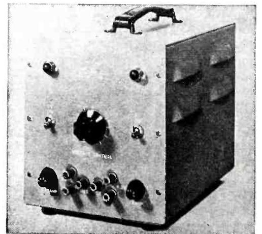
use. Output is continuously variable from 180 to 360 volts, and will remain constant to within 1 percent for loads from 0 to 75 milliamperes, and for line-voltage variations of plus or minus 10 percent. Either the positive or negative out-
