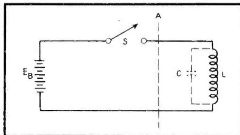
FIG. 2—Basic circuit of a reactive saw-tooth current oscillator
