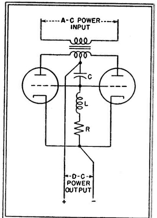
Fig. 1—Electronic control of the rectifiers provides some filtering
