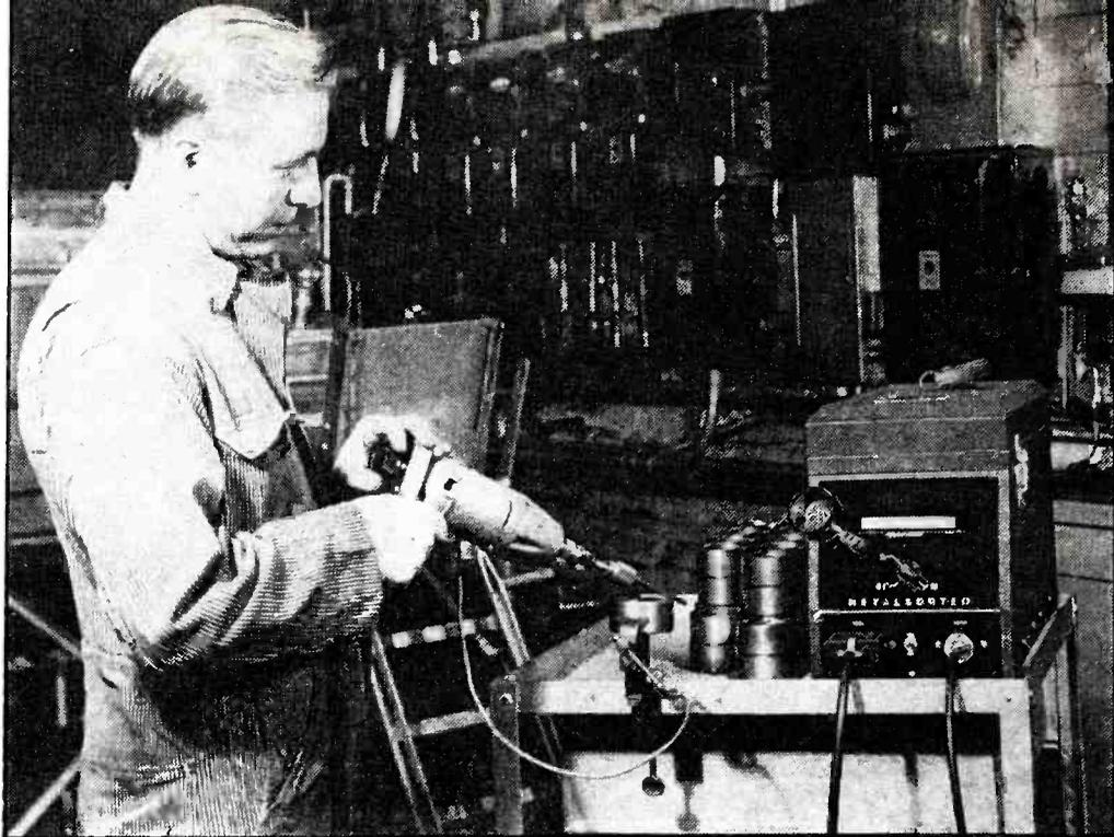
Checking machined alloy products to make sure all have same composition. Operator is adjusting knob on reciprocating tool to balance out stray voltages before making test
