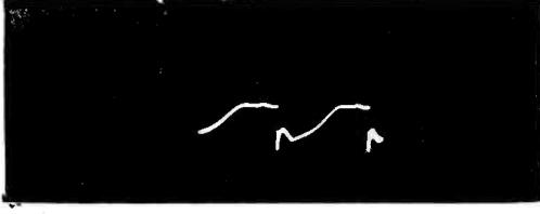
FIG. 10—Cathode current of oscillator tube
