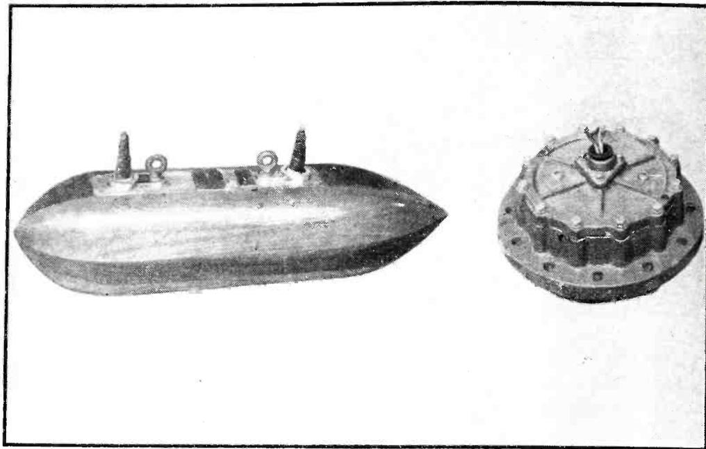
Streamlined outboard "fish" used to support portable magnetostriction units for hydrographic survey work, and one of the magnetostriction units
