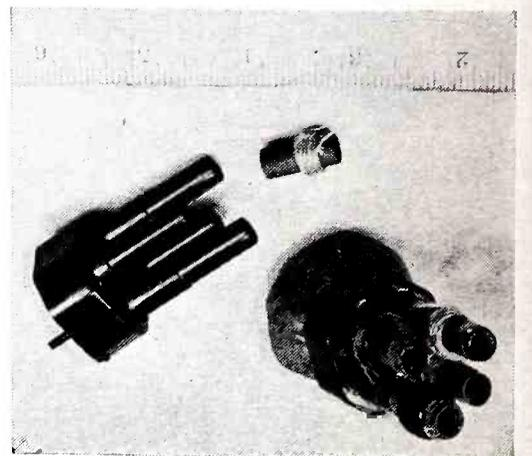
Fig. 3—The i-f coils are slipped over the posts on the molded piece at right to form the complete assembly at left
