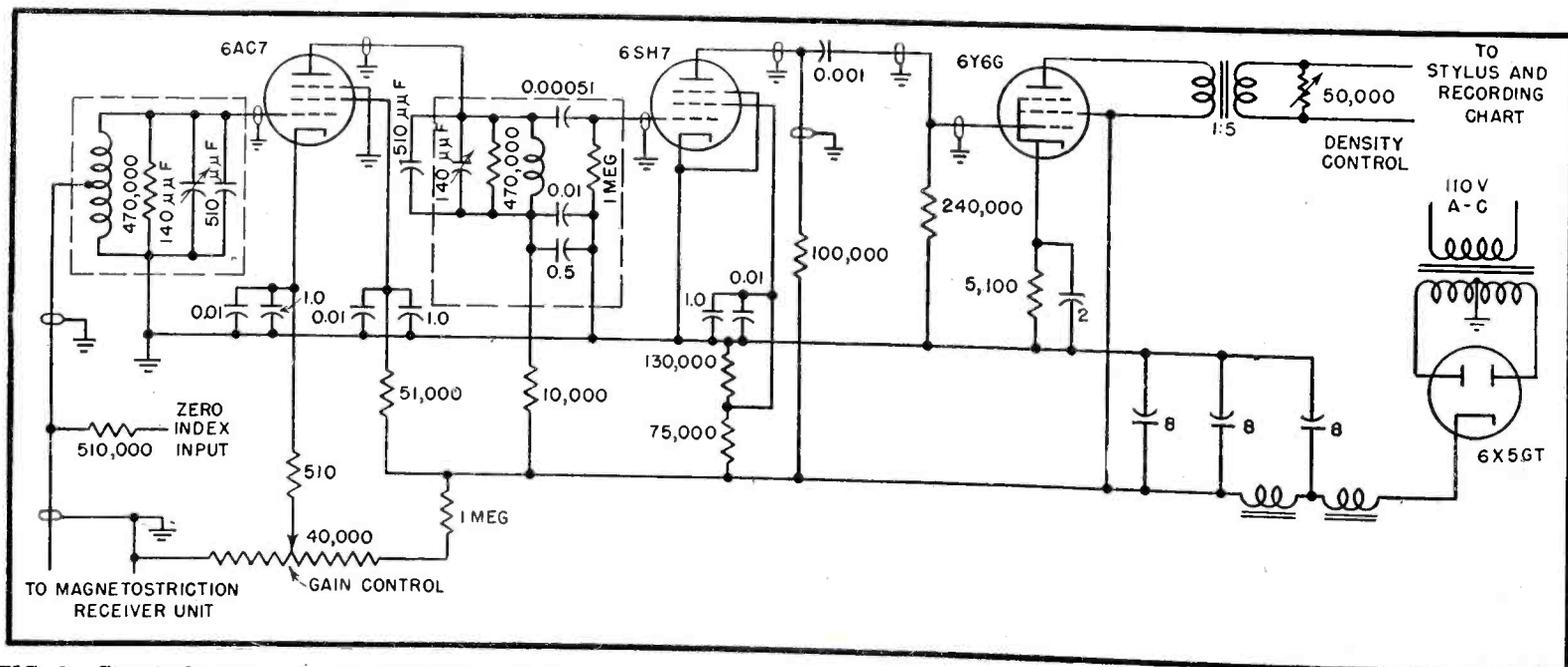
FIG. 2—Circuit diagram of echo amplifier, which is connected between the magnetostriction receiver unit and the recorder, and delivers output pulses strong enough to burn the desired marks on the recording paper
