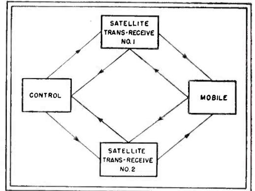
Fig. 1—Multicarrier diversity transmission system provides wide coverage at uniform signal strength
