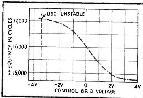
FIG. 6—Saw-tooth frequency and grid voltage for one value of screen voltage
