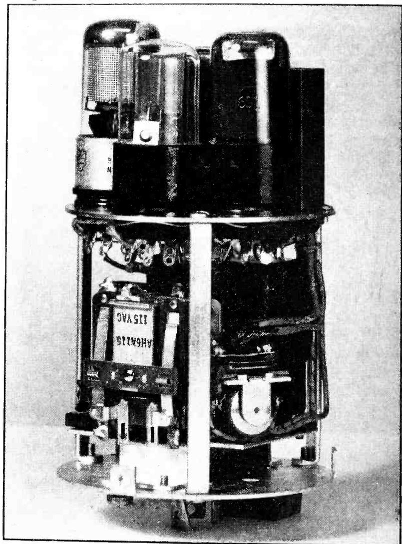
Interior of the switch, showing phototube and amplifier tubes on the top deck, component parts below, and connection socket at the bottom
