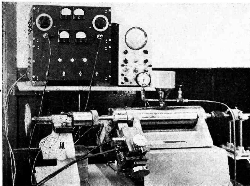
FIG. 3—Complete spindle-testing apparatus. The capacitive probes are at right angles to each other and equally distant from the precision-turned shaft extension. Amplifier and cathode-ray oscilloscope are on the shelf above
