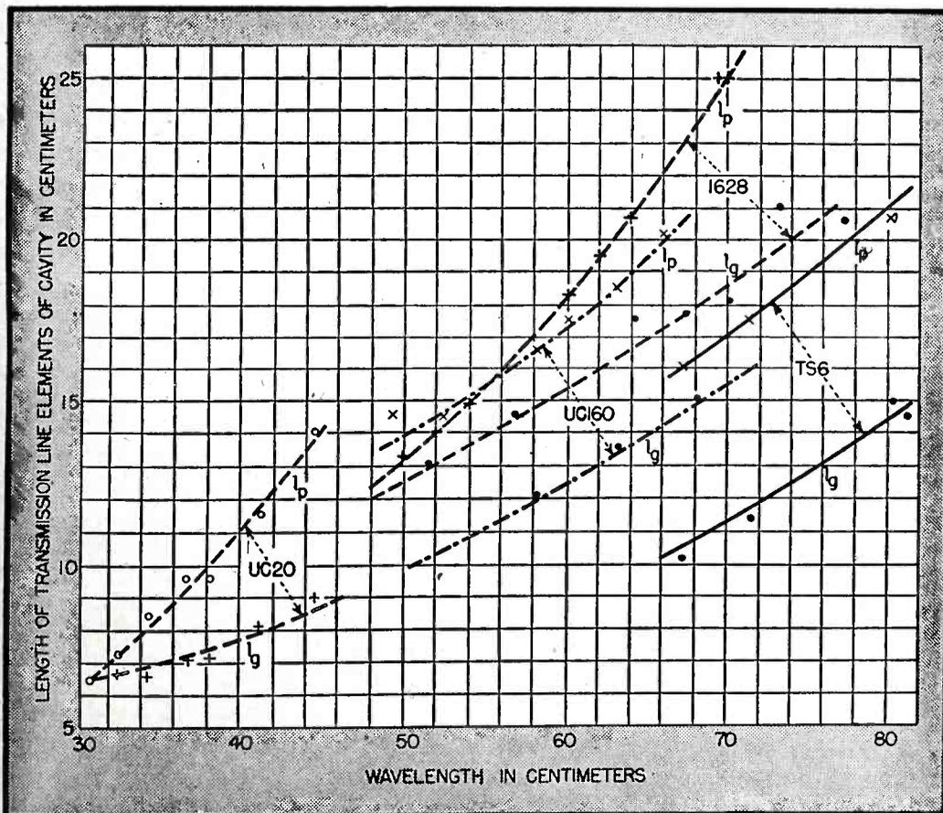
FIG. 4—Grid and plate line lengths as functions of wavelengths for the composite tank of an oscillator were plotted from data taken on about twenty different oscillators, some of which are illustrated in this article
