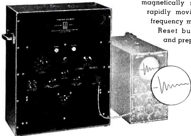
Brush Transient Recorder with Oscilloscope Showing Typical Transient
