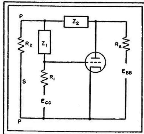
Fig. 1—In this resonant circuit, the reactances shown as blocks are both either inductors or capacitors
