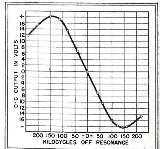
Fig. 2—Discriminator response of a production receiver
