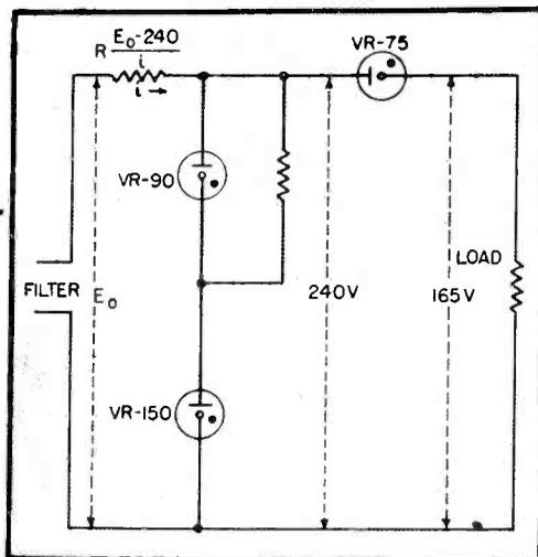
FIG. 1—Simple circuit for providing 165 volts of regulated output
