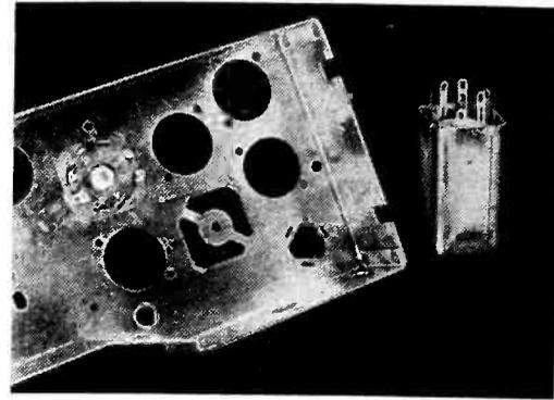
Fig. 6—Portion of chassis showing bridged cutout and a mounted i-f transformer
