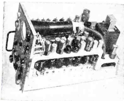
tem signals over land or sea. The equipment is particularly suitable for aircraft installation, weighing a little less than 36 pounds.
