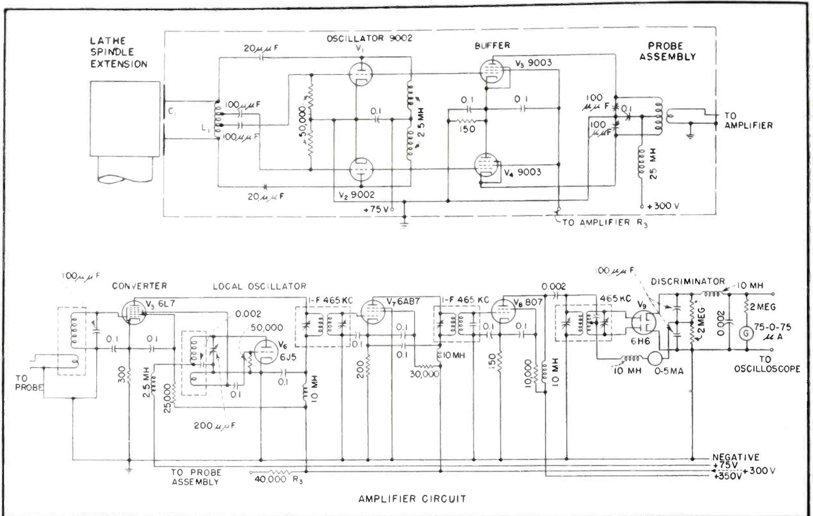
FIG. 5—Complete circuit diagram of one probe assembly and amplifier channel. Two complete channels are used in spindle testing
