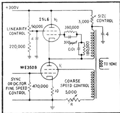
FIG. 1—Circuit of saw-tooth current oscillator used to feed horizontal deflection yoke
