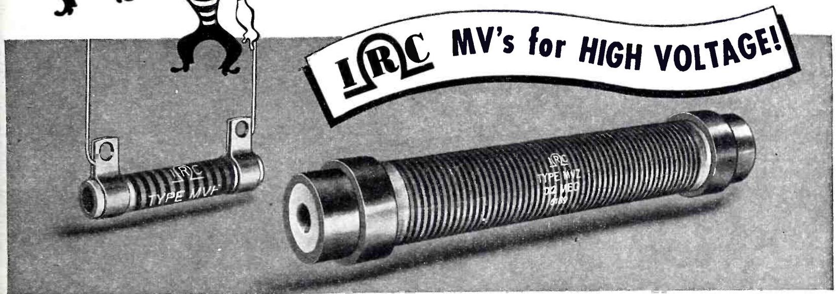
In high voltage applications where requirements are for high resistance and power, IRC MV High Voltage Metallized Resistors are designed and constructed to do the job. They are manufactured with the famous metallized coating applied spirally on ceramic forms. This provides a conducting path of extensive effective length. Turns are
