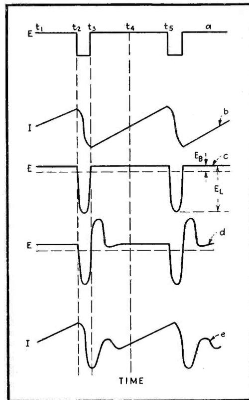
FIG. 3—Current and voltage variations in the circuit of Fig. 2 when the switch is operated
