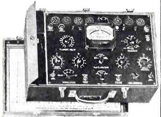
MODEL 798—JUST OUT—MUTUAL CONDUCTANCE TUBE CHECKER & SET ANALYZER. Tube Checker Ranges 0-3000, 6000, 12,000 microhmhos and Good-Bad Scale. Analyzer Ranges 0-15, 150, 750 Volts A.C. & D.C. 7.5 & 150 M.A. D.C., 100,000 & 1,000,000 ohms \$182.64
