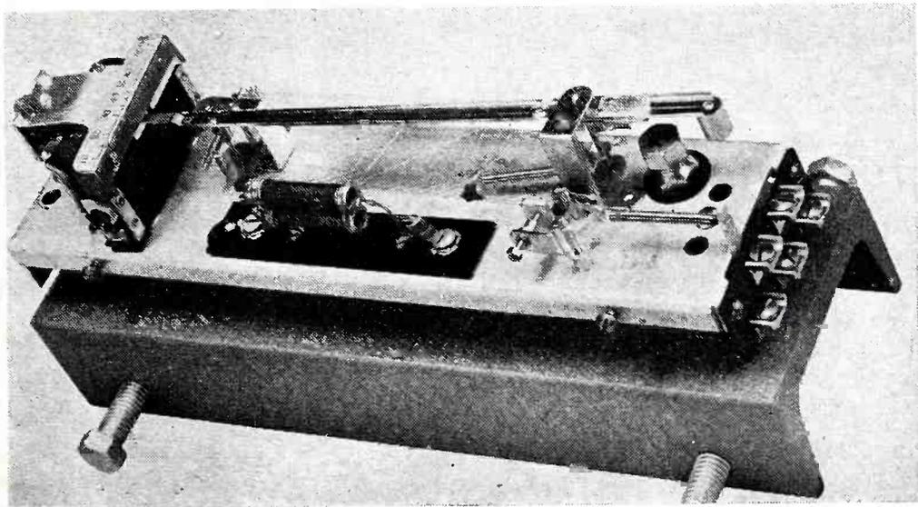
Remote measuring station, showing the two ceramic resistors and the freely moving humidity element. The scale at the left is attached to the clamp that lowers at the moment of measurement
