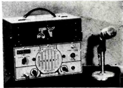
with a 5-inch permanent magnet speaker, a desk stand microphone, and is priced at \$595, less tax. The unit operates from 115-volt alternating current.
