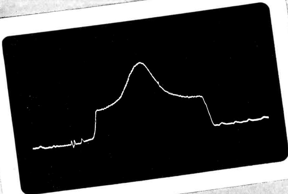
● Brush Transient Recorder caught this photoflash bulb exposure in recent tests on camera shutter synchronization. A transient of 40 milliseconds duration—automatically recorded and reproduced for study! This wave trace indicates peak light intensity at exactly the right moment—an excellent start toward a perfect picture! Such transient phenomena recording by the Brush Transient Recorder—bares production defects never before so easily measured.
