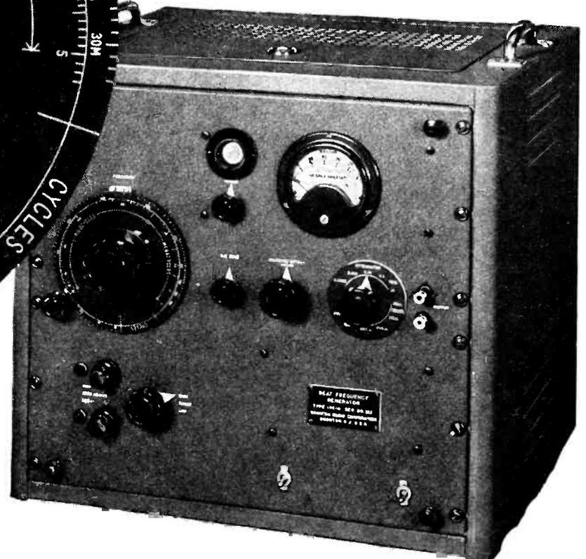
One of the most valuable instruments in the laboratory is a generator of signal voltage. Boonton Radio Engineers in designing the Type 140-A Beat Frequency Generator have provided an instrument of wide frequency coverage, capable of supplying accurate output voltages ranging from several microvolts to 30 volts and having a variety of output impedances from 20 ohms to 1000 ohms.
