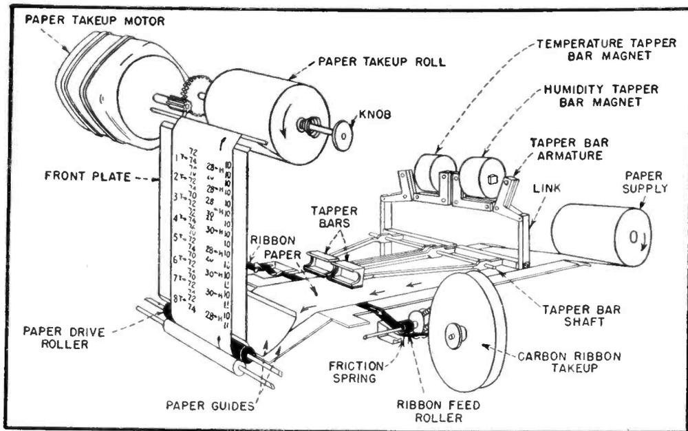
FIG. 2—Sketch of the printing mechanism in the electronic recorder, showing how the paper is fed between the printing wheels and the tapper bars
