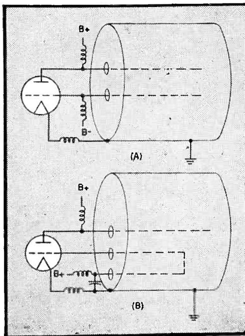
FIG. 3—(A) The circuit of Fig. 2B does not oscillate in the desired mode unless the line is inserted in a cavity. (B) A modification is to loop one of the lines in the cavity back on itself, bringing its end out of the cavity for connection to the d-c feed line
