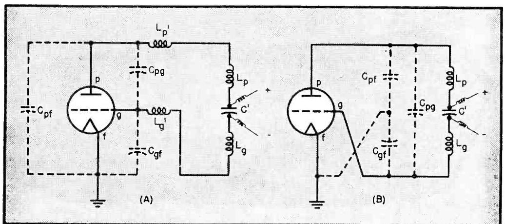
FIG. 1—The combination of interelectrode capacitances and tube lead inductances, plus—if necessary—externally added inductance, gives a high-frequency oscillator (A) which is basically a Colpitts circuit (B)
