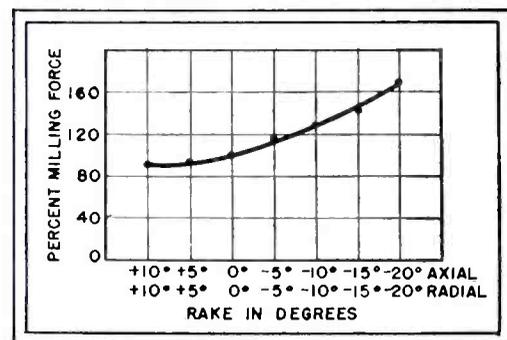
Fig. 3—Effect of rake on milling forces is plotted from many oscillograms
