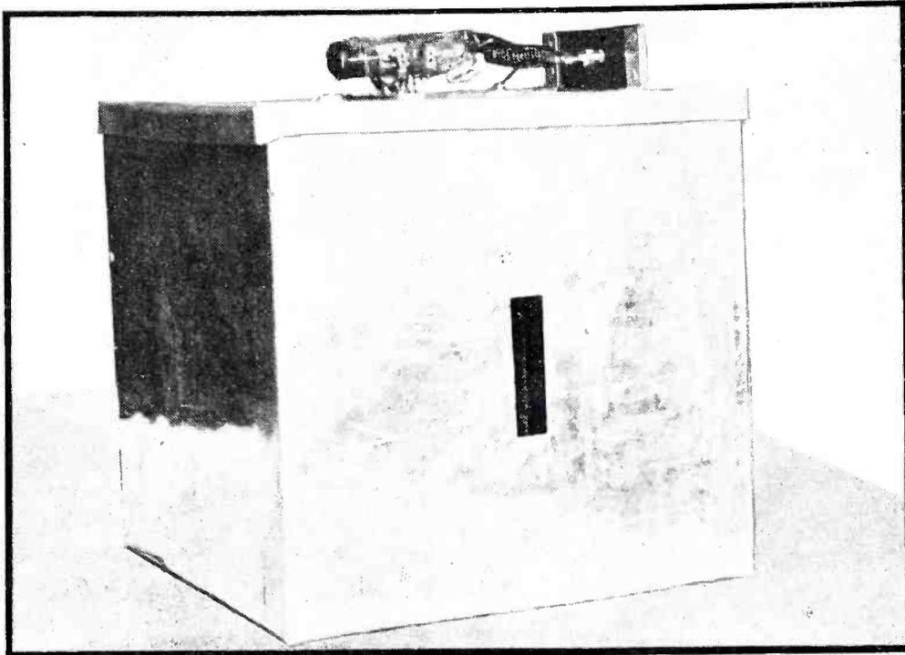
Any cavity shape can be used for the composite tank circuit. Energy can readily be withdrawn from the cavity through a suitably placed slit
