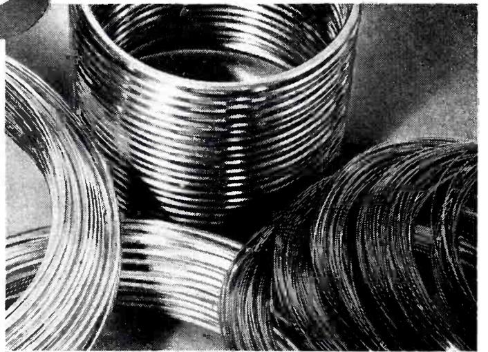
**ODD SHAPES** of wires with suitably spaced projection points are manufactured for contacts of longer lengths than generally used in welding applications.
