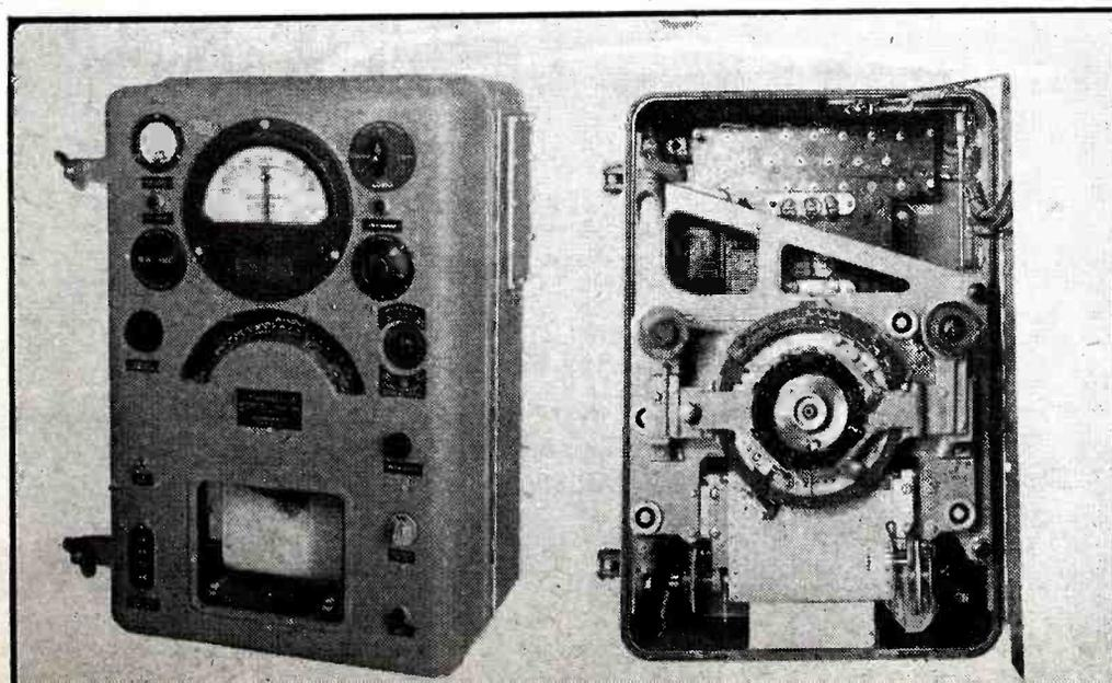
Recorder unit of Submarine Signal Co. model 788A precision depth sounder. The stylus-supporting wheel is on the shaft of an a-c motor that rotates continuously at a speed proportional to the velocity of sound in the water being explored, and current pulses burn marks in the chart as the stylus sweeps over it once in each revolution
