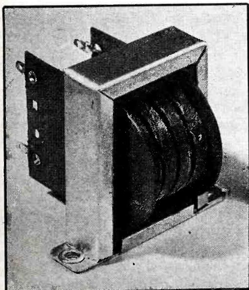
The assembled oscillator transformer has four pie windings. Construction details are given under Specifications
