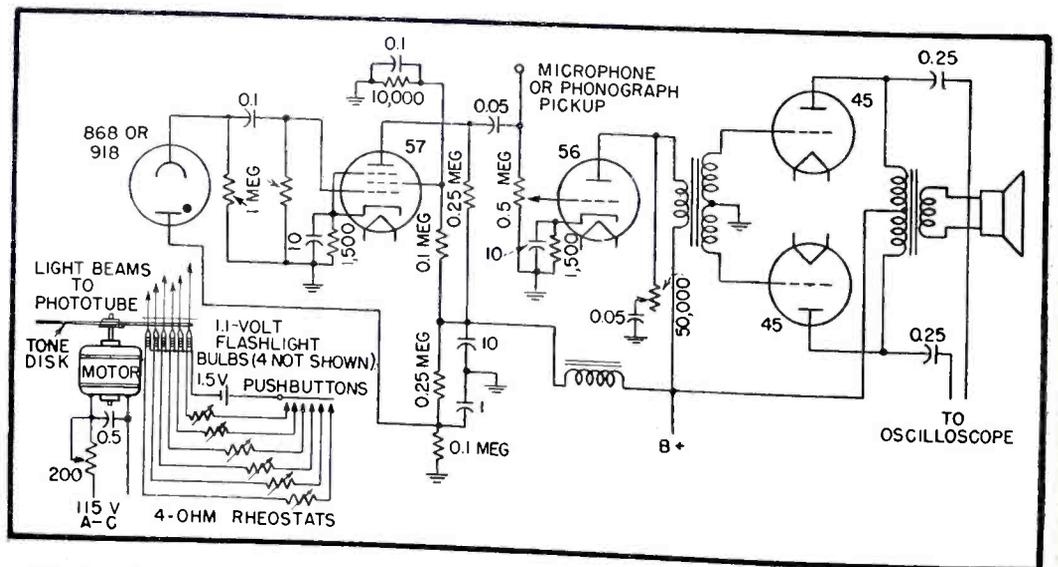
FIG. 2—Circuit diagram of photoelectric tone generator. A conventional power pack using a type 80 tube as full-wave rectifier with speaker-field choke and two 8- $\mu$ f, 450-volt electrolytics is adequate. A separate filament winding serves the output stage, with a 750-ohm resistor in the center-tap lead for bias
