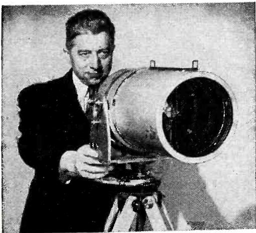
Thermistor bolometer developed for armed forces by Bell Telephone Laboratories can detect heat of person's body one-quarter mile away, locate chimneys of factories and stacks of ships at night, and increase the precision of temperature measurements in industry
