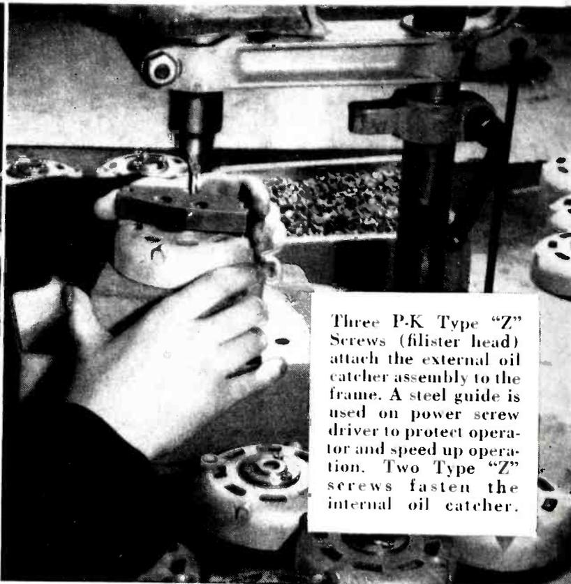
Three P-K Type "Z" Screws (filister head) attach the external oil catcher assembly to the frame. A steel guide is used on power screw driver to protect operator and speed up operation. Two Type "Z" screws fasten the internal oil catcher.
