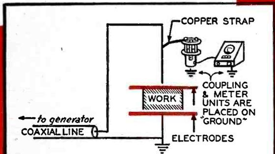
Quickly and directly measures r-f voltage between applicator electrodes. Enables you to vary load voltage during heat cycle in accordance with any pattern you select, or regulate the voltage on one load after another to assure uniform results.
