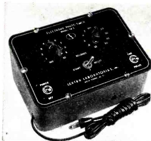
to 60 seconds are available at an accuracy of 10 percent. The unit weighs 3 pounds and measures 5½ x 8 x 3¼ inches. It operates on a-c or d-c.
