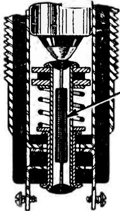
BUILT-IN RESISTOR HOUSED IN SPRING CONTACT EYELET
