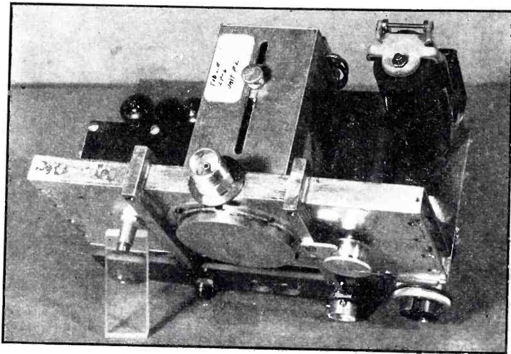
Transceiver chassis with cover removed. Fitting for coaxial line going to antenna can be seen at top center of rectangular cavity inside which is mounted the GL-446 lighthouse tube serving as r-f oscillator
