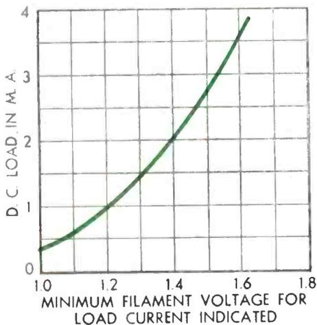
Note: Curves indicate that in a television receiver rectifier circuit supplying 250 microamperes D. C. load current, the filament voltage may fluctuate from 1.0 to 1.65 volts.
