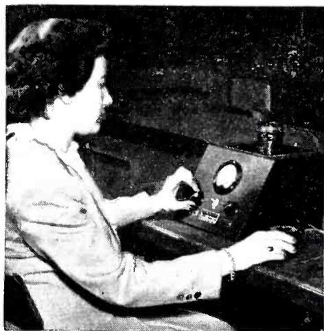
ence of short-circuited turns. The high-voltage unit indicates the induced volts per turn and faulty coils that break down under test. Additional details are given in bulletin GEA 4539.
