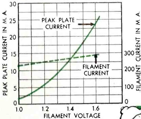
This new CHATHAM high vacuum rectifier is designed to withstand severe operating conditions and give long trouble-free service. Because of the rugged filament construction, repeated overloads do not seriously impair tube life. The 50,000 volt peak inverse voltage rating enables the tube to deliver approximately 25,000 volts D. C. output in a single tube circuit and approximately 50,000 volts D. C. output in a voltage doubling circuit.
