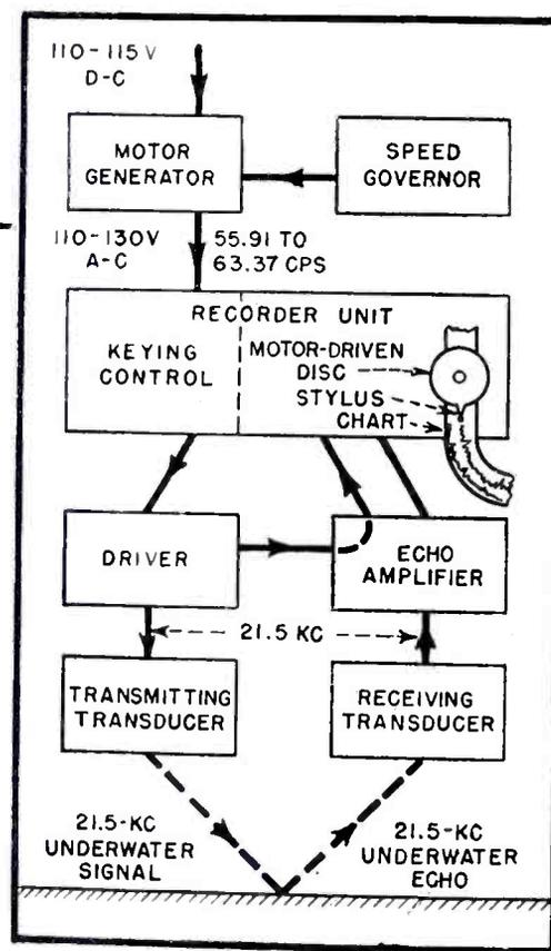
FIG. 1—Block diagram of precision depth recorder employing echo-ranging principle
