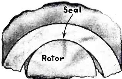
Oil Seal is provided by precise machining to 1/10,000 inch. Oil film prevents rotor from touching the stator, avoiding wear.
