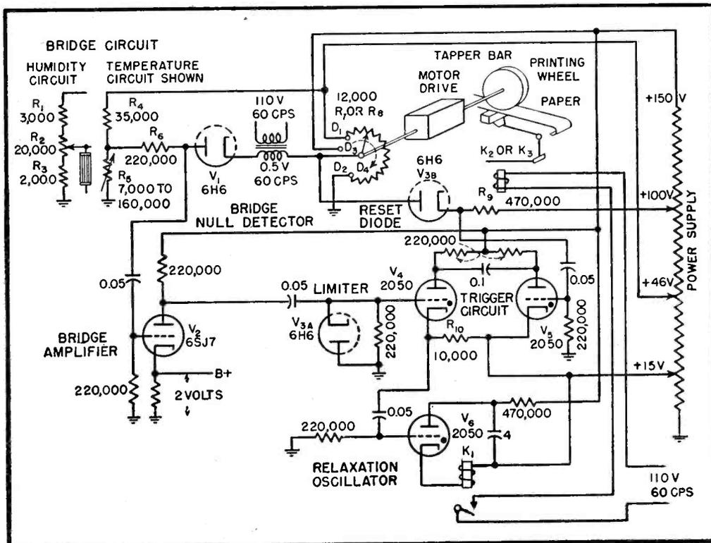
FIG. 1—Simplified wiring diagram of the recorder, showing the interconnection of the remote temperature and humidity station elements
