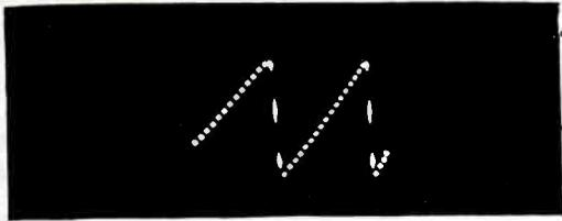
FIG. 7—Saw-tooth current through the deflection yoke
