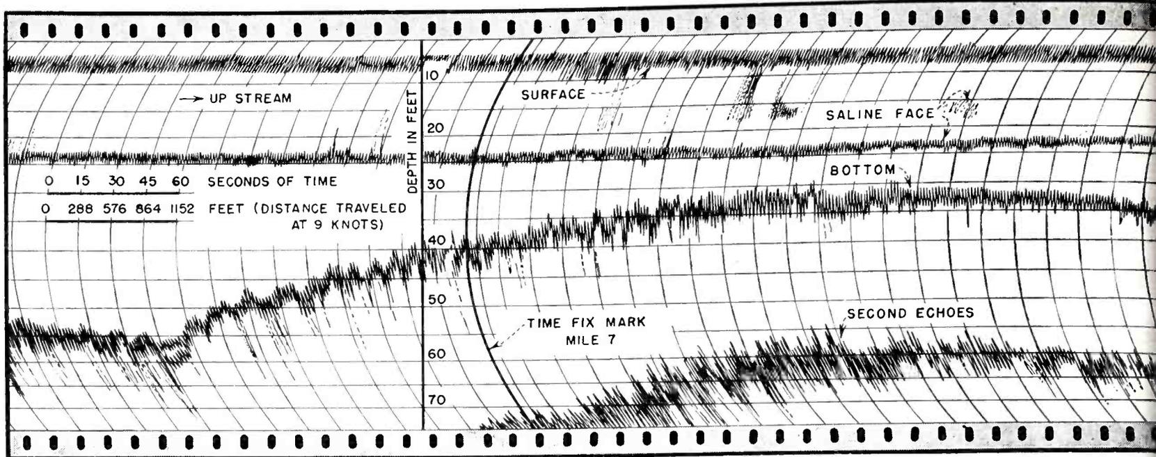
Profile of river bottom along 1.75-mile stretch of Southwest Pass, near mouth of Mississippi River, as made with precision shallow-water depth recorder. In addition to bottom depth, an experienced operator can accurately interpret such additional information as
