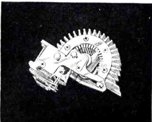
making a maximum of 8 or 4 contacts, respectively. Operated from a telephone-type dial pulser the maximum operating speed is 30 steps a second, or double that speed with self-cycling operation.
