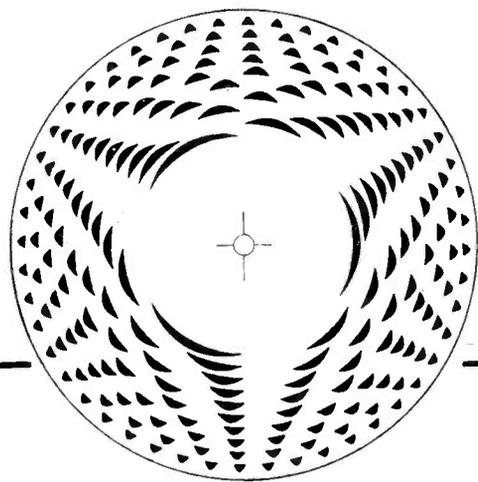
FIG. 1—Reproduction of tone wheel providing a fundamental and 2nd, 3rd, 4th, 5th, 6th, 8th, 10th, 12th and 16th harmonics. Only half of each sine-wave cycle is required because the reflected half of the pattern closely resembles the other half
