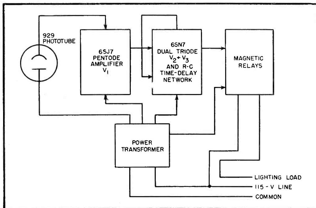
FIG. 1—Block diagram of the photoelectric street lighting control
