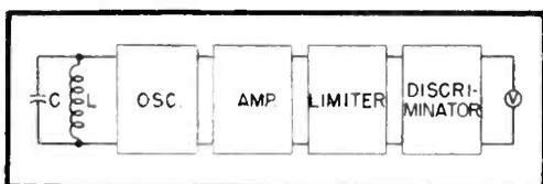
FIG. 1—Functional block diagram of the capacitive micrometer. The probe is represented by the capacitor at the left
