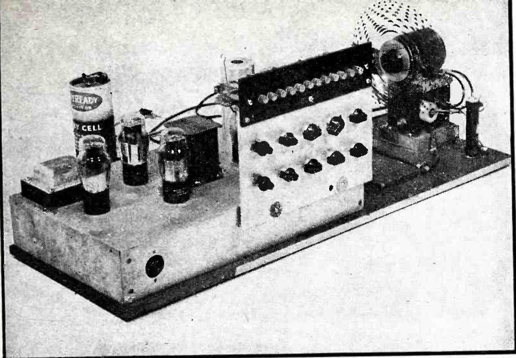
Front view showing tone generator out of its cabinet. Pushbuttons turn individual lamps on and off, while rheostats below permit changing brilliancy of any lamp to vary the amplitude of the corresponding harmonic
