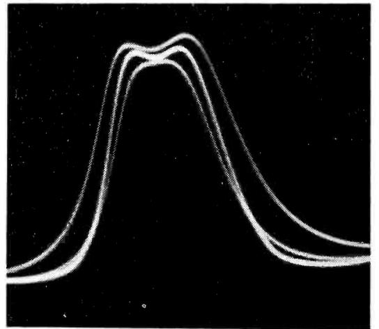
The production coil is adjusted so that its curve falls within the limit traces that have been previously standardized
