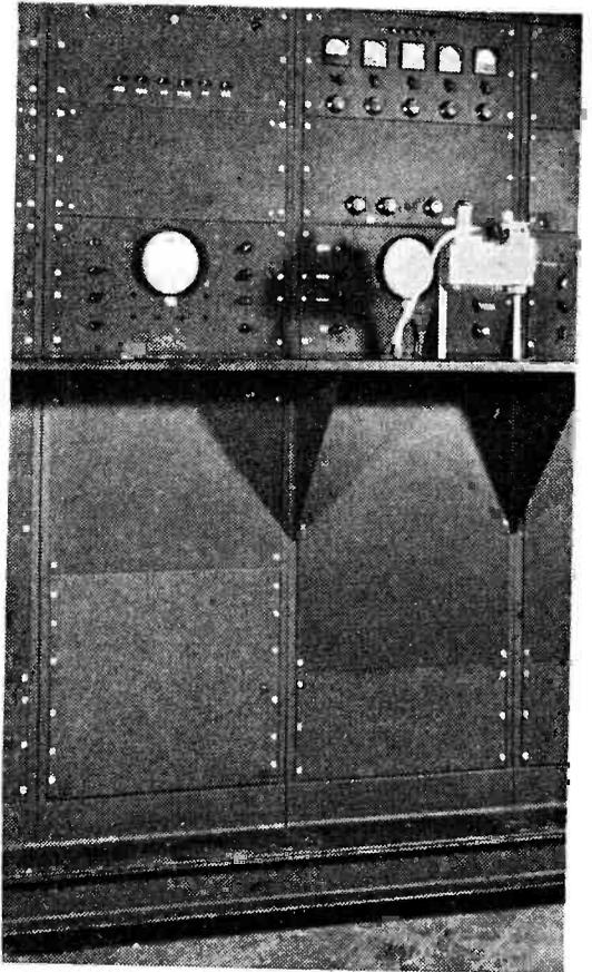
Fig. 1—Two sections of the five-channel oscillograph used to record forces in milling cutter
