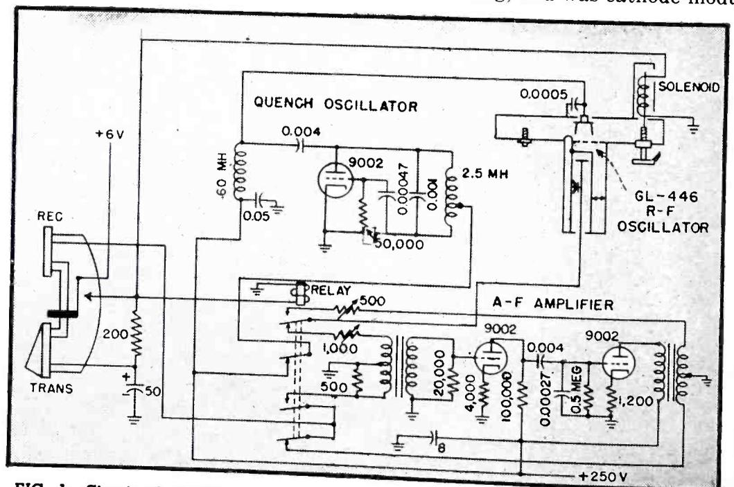
FIG. 1—Circuit of 2,700-mc portable transceiver, with relay and handset switch in receiving position. Lighthouse tube is mounted in cavity, and coaxial line going to dipole antenna is coupled into cavity at right angles to plane of diagram
