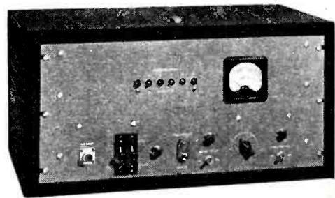
has an input sensitivity of 0.25 volt and a resolving time of better than 5 microseconds. It is little affected by changes in line voltage. Input line voltage can vary between 95 and 130 volts.
