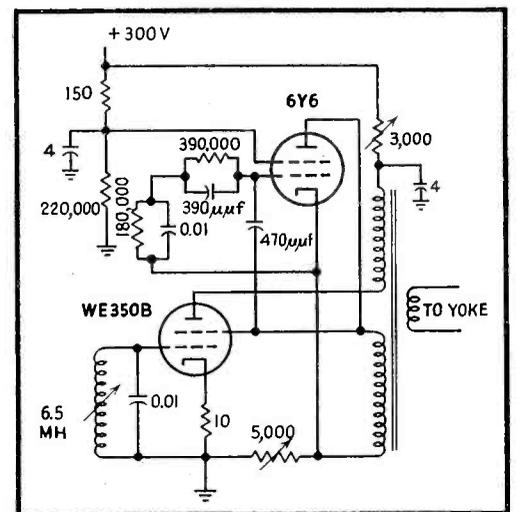
FIG. 11—To stabilize the saw-tooth oscillator, a resonant circuit is introduced into the grid circuit
