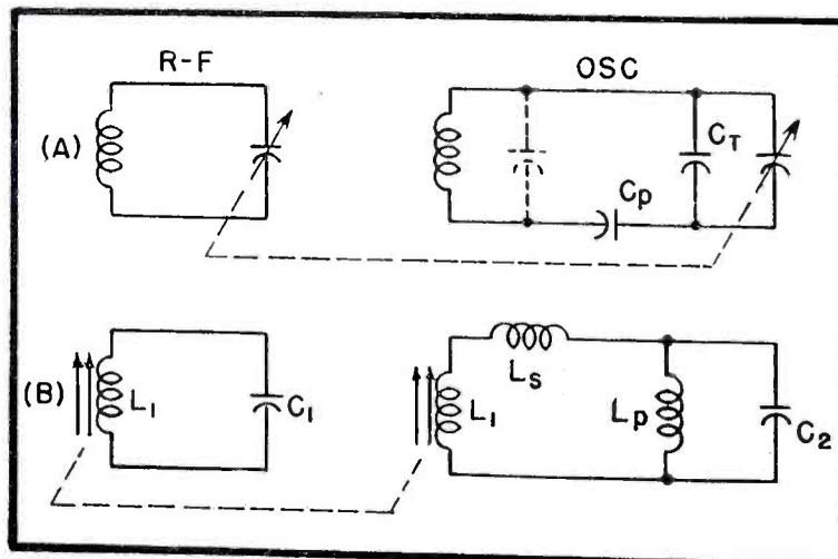
FIG. 1—Conventional variable-capacitance tuned r-f and local oscillator circuits (A) and equivalent permeability tuned circuits (B) as used in a superheterodyne receiver
