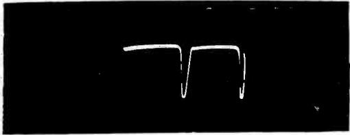
FIG. 9—Voltage across grid winding of transformer
