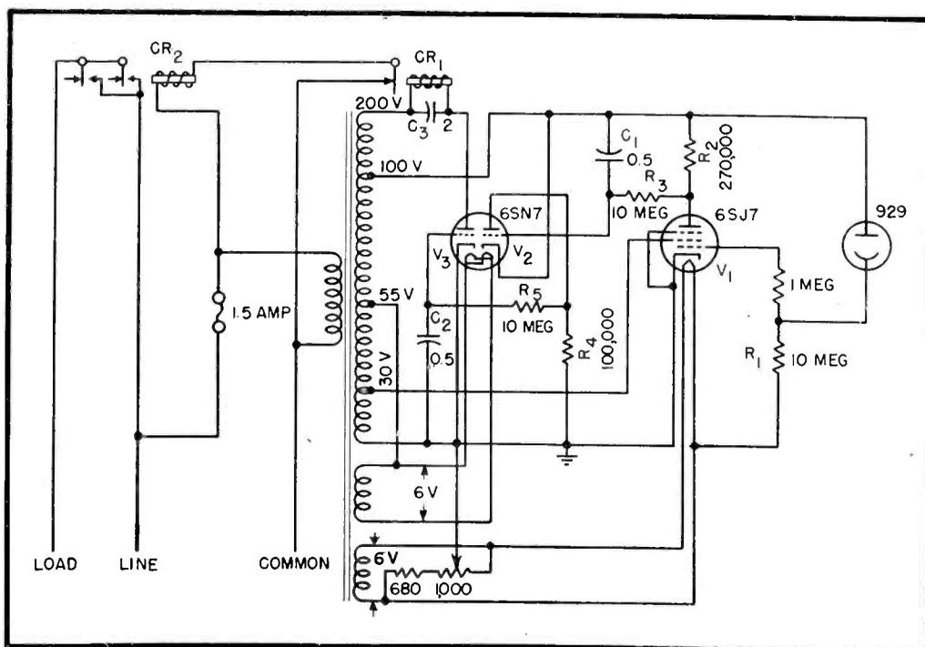
FIG. 2—Circuit diagram of the photoelectric street lighting control
