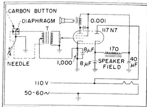
One-tube amplifier and rectifier circuit used in testing the carbon pickup. A double-button unit could be connected as shown by the dashed line
