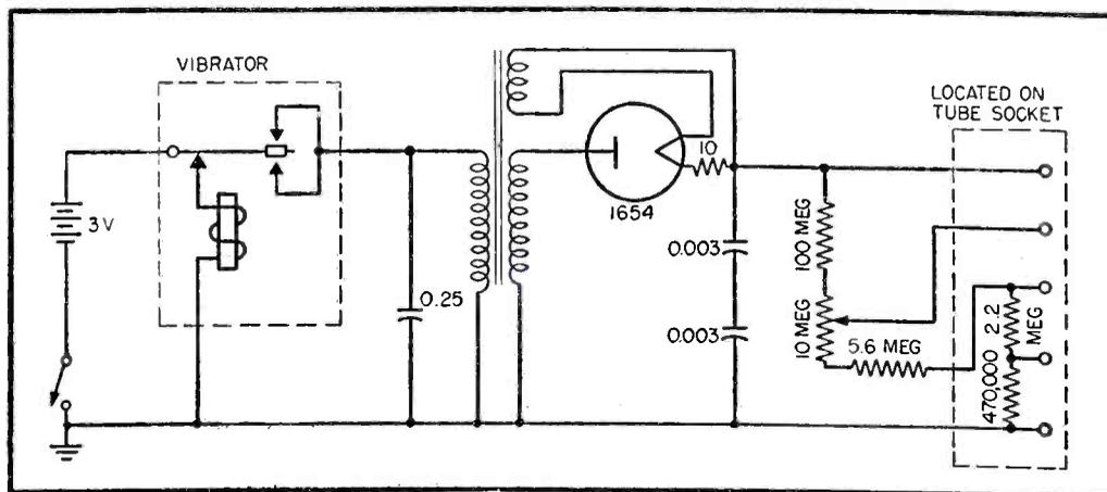
FIG. 4—Circuit of 5,000-volt pocket-size power supply
