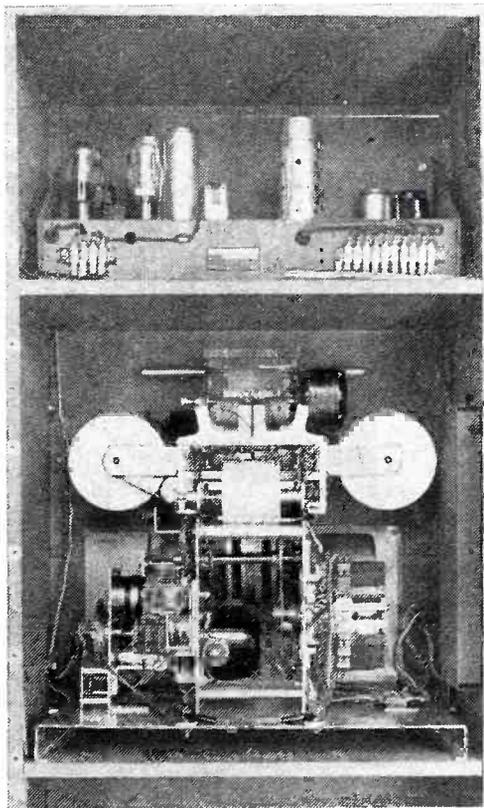
Rear of the central station. Below the electronic equipment chassis is the electromechanical printer and averaging device. The sequence switch is shown at the right. Power supply below is omitted
