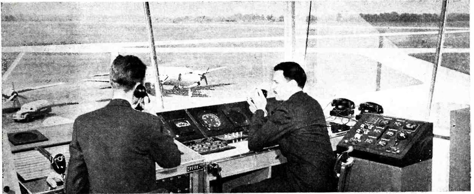
Airport control tower at Indianapolis, used by CAA in testing electronic aids to aviation. Control panel at right monitors performance of instrument landing system, and cabinet just barely visible at left houses radar scopes
