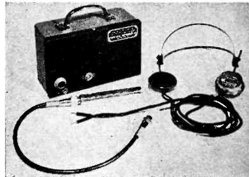
headphones. An internal oscillator converts 135 volts from the B battery to a counter operating potential of over 1,000 volts. The unit measures  $7 \times 5 \times 3$  and weighs  $4\frac{3}{4}$  pounds without batteries. It costs \$150 complete, f.o.b. Arlington.
