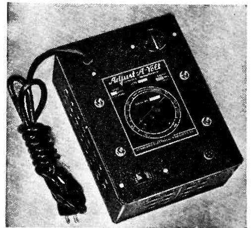
70 and 140 volt output. It is not an autotransformer and so serves to isolate primary and secondary circuits. There are four models available with maximum rating at 1,000 volt-amperes.
