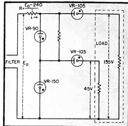
FIG. 2—Two widely different output voltages are provided by this arrangement
