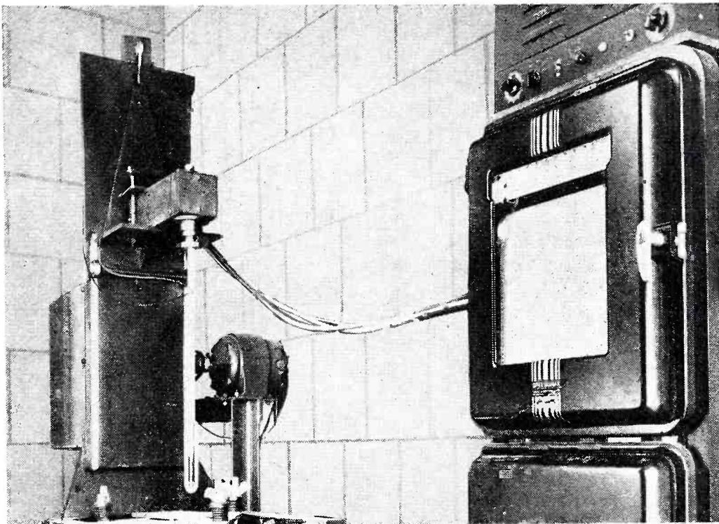
FIG. 7—High-speed dilatometer (left) and recorder
