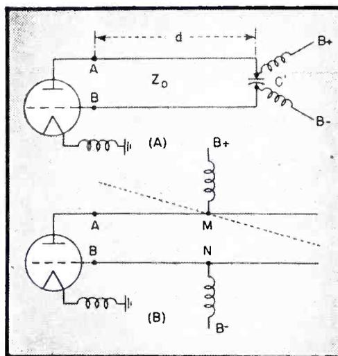
FIG. 2—(A) Transmission line version of the circuit at Fig. 1A. (B) Extension of line beyond feed points gives longer physical tank without increasing the wavelength
