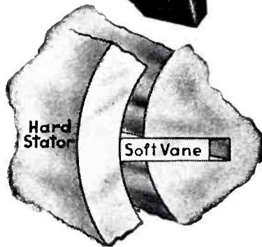
Internal Vane is softer than the stator. Wears indefinitely and improves with use.
