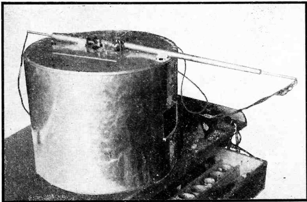
Quarter-wave stubs can be used in place of inductances to prevent reaction on the tank from the feed lines
