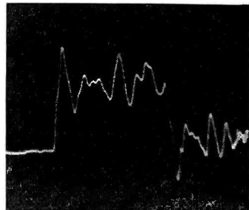
Fig. 2—Oscillograph indicates magnitude and frequency of forces in cutter as tool passes through the work
