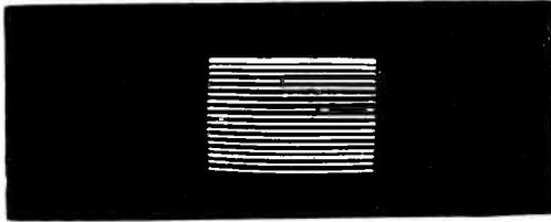
FIG. 8—Linearity of the horizontal deflection
