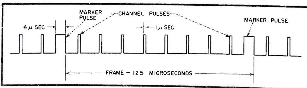
FIG. 4—Pulse multiplex signal that modulates microwave transmitter
