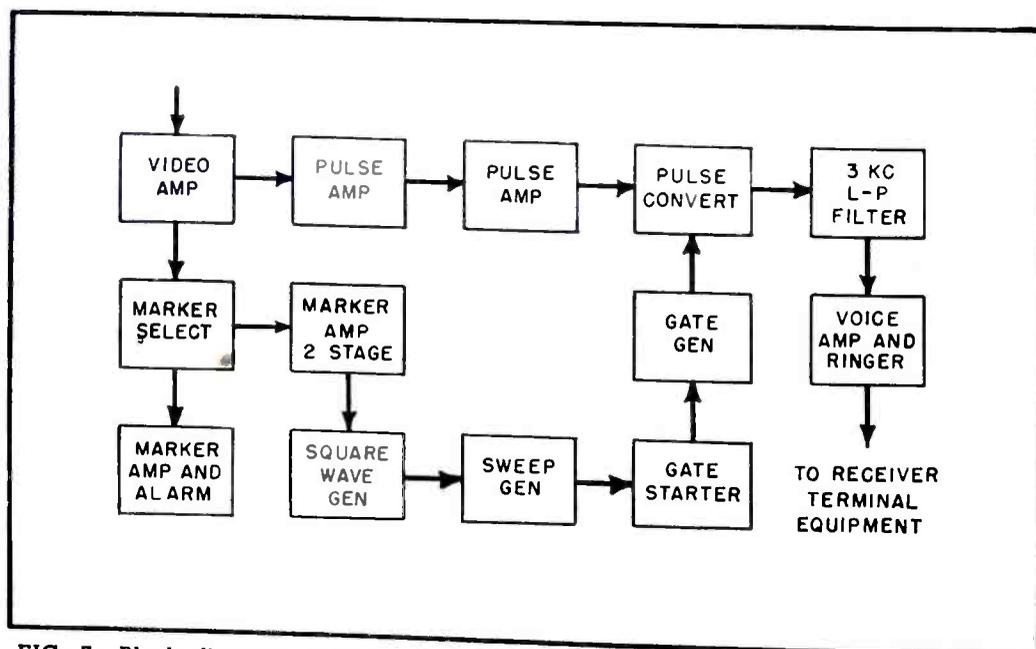
FIG. 7—Block diagram indicates sequence in which one channel of the modulated pulses is converted to voice signal in reception
