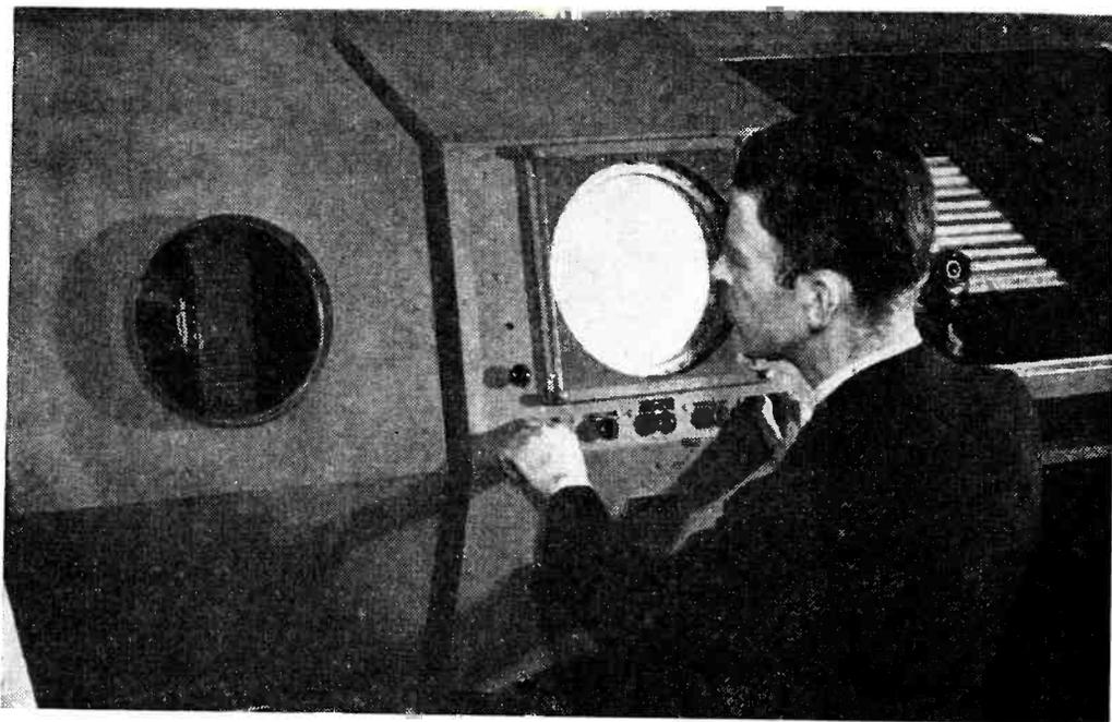
These two radar scopes give the air traffic controller a picture of all planes in the air within a radius of 30 miles from the control tower. Scope at left indicates altitudes of planes in thousands of feet, while that at right gives ppi presentation for azimuth
