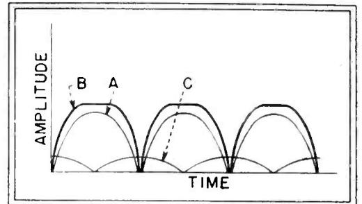
Fig. 2—Comparison of the wave shapes produced by conventional and wave-form controlled rectifiers shows closer approach to d-c in the output of the latter
