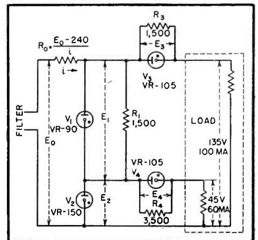
FIG. 3—For high-current requirements, resistors are shunted across the voltage-regulator tubes in series with the loads
