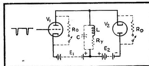
FIG. 4—Elements of basic damping circuit that acts like the switch of Fig. 2
