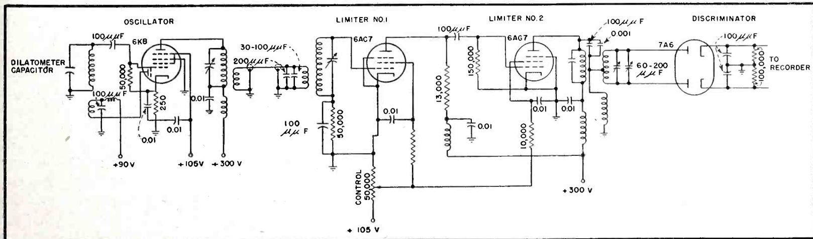
FIG. 8—Single-channel dilatometer circuit diagram. The recorder input and switching details are omitted
