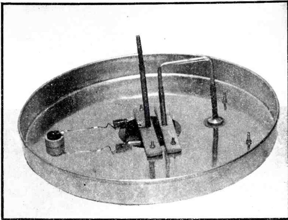
Internal disposition of lines indicates that they act as a resonant electric and magnetic exciter for the cavity
