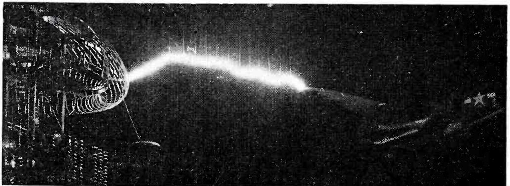
Artificial lightning leaps from electrostatic generator to Ventura twin-engine bomber suspended from roof of special laboratory at Wold-Chamberlain Airport, Minneapolis during research on causes and cures for precipitation static
