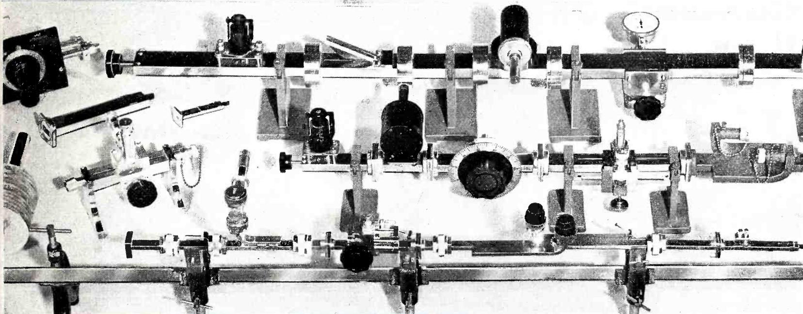
The complete line of De Mornay • Budd standard test equipment covers the frequency range from 4,000 mcs. to 27,000 mcs. It provides all R. F. waveguide units necessary for delicate, precision test work requiring extremely high accuracy in attenuation measurements, impedance measurements, impedance matching, calibration of directional couplers, VSWR frequency measurements, etc.
