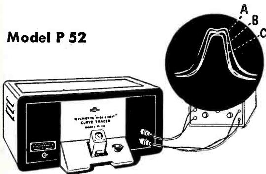
For rapid alignment of I.F. coils of frequencies from 85 kc to 11 mc. Operator adjusts test trace (B) to fall between traces of limit coils (A and C), set up to production specifications. Defective coils immediately detected. All error is eliminated as circuit changes or line voltage
