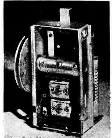
plished by moving the carriage along a rack by means of brass ribbons terminated on a brass cylinder of about  $\frac{3}{8}$ -inch diameter as illustrated. The movement is positive and claimed to be noiseless.
