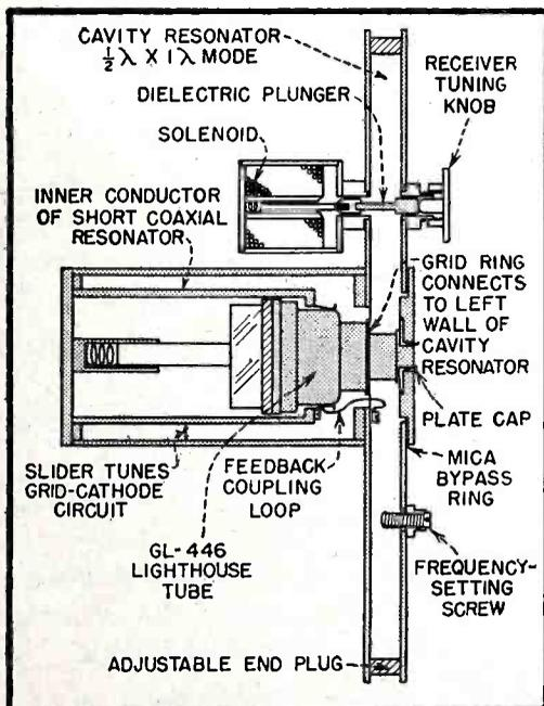
FIG. 2—Details of cavity resonator oscillator, showing frequency-compensating mechanism used to make sending and receiving frequencies the same
