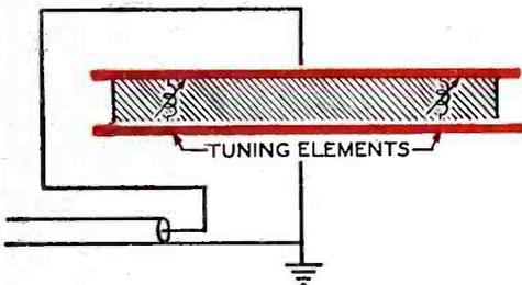
Makes it easy to measure voltage variations ("standing waves") on long electrodes. Auxiliary compensating inductances or "tuning stubs" to distribute the power evenly can be quickly and accurately adjusted.
