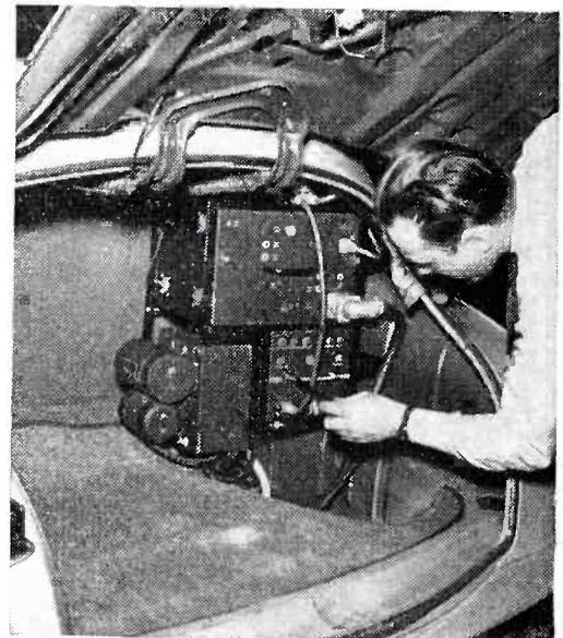
In the baggage trunk of the cab are mounted the 40-watt f-m transmitter at top, receiver at lower right, and dynamotor at lower left
