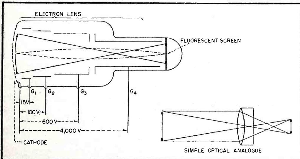
FIG. 2—Arrangement of the electrodes in the image tube, and the potentials required
