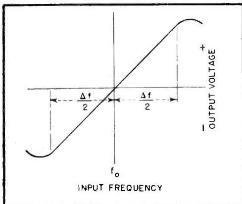
FIG. 2—The discriminator circuit characteristic shows the change in output voltage caused by change of input frequency
