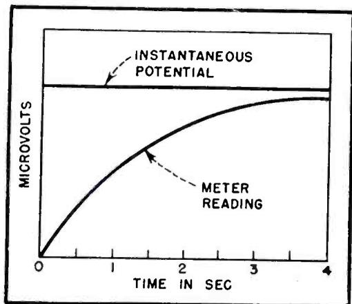
FIG. 1—Manner in which reading of microvoltmeter builds up from zero to approach instantaneous triboelectric voltage value
