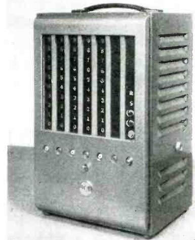
Neon-lit figures on the panel of the time interval counter can show velocities and accelerations for intervals up to one second in steps of one millionth of a second
