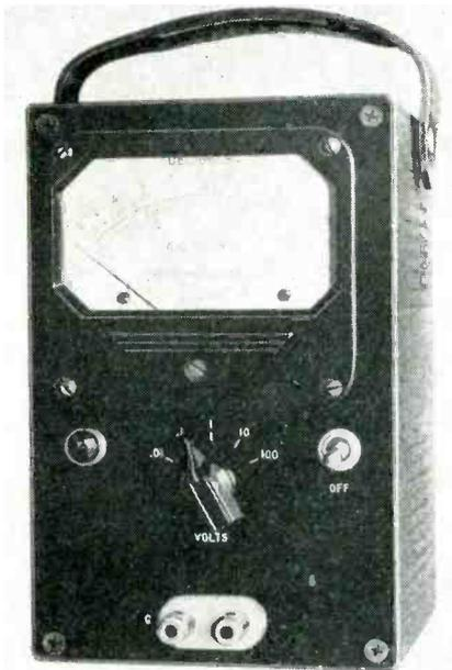
No. 1040 vacuum-tube voltmeter has a range from 0.001 to 100 volts with an accuracy of 2 percent for sinusoidal voltages. Frequency range is 10 to 200,000 cycles with 0.1 db variation. The power supply is contained in the metal cabinet.
