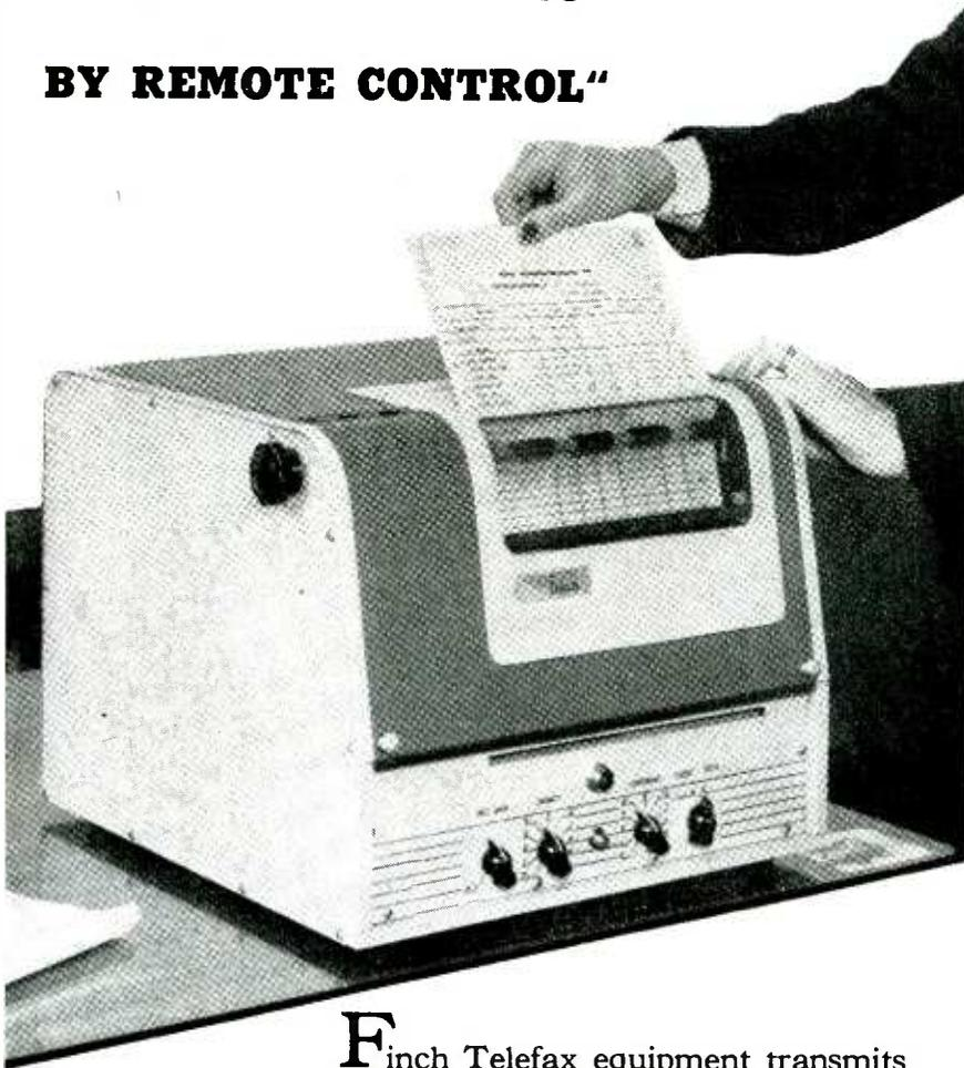
**F**inch Telefax equipment transmits and records—by radio or telephone—exact facsimiles of written or printed messages, as well as drawings, photographs, signatures, typewriting, etc. Finch Telefax is really "printing by remote control." It is the fastest known and most accurate system of communication.
