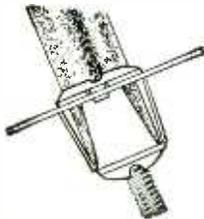
3. Snap the assembly into chassis, shield can or terminal board. Provides absolute security and rapid assembly.
