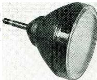
includes anode voltage of 8,000 to 10,000 volts; grid no. 2, 250 volts; grid no. 1, minus 45 volts; and focusing coil current between 88 and 116 milliamperes.
