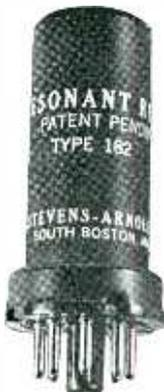
reed mechanism adjusted to respond to a narrow band of frequencies. The units are totally enclosed and based with octal-tube type connections. The ON time of the contacts is 5 percent for all frequencies from 153 to 442 cps. An auxiliary relay or vacuum tube is used to control large currents that can not be handled by the vibrating contacts. The standard coil has an impedance of 500 ohms. Further details are given in Catalog 116.
