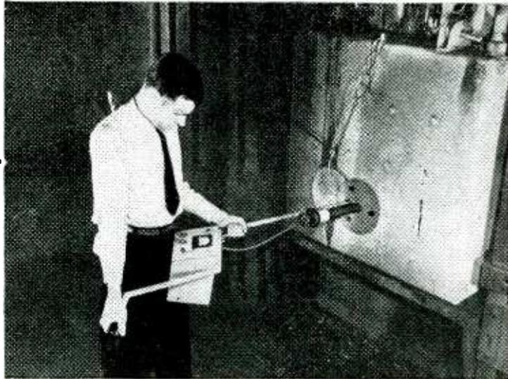
Flame radiation measuring instrument in use. This same furnace is shown in natural color on cover of this issue
