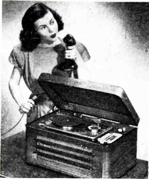
corder that uses a large drum driven by the turntable as a takeup reel. Recordings are stored on a 3½ inch spool of stainless steel wire capable of holding an hour's program. Selling price of the combination is \$169.50.
