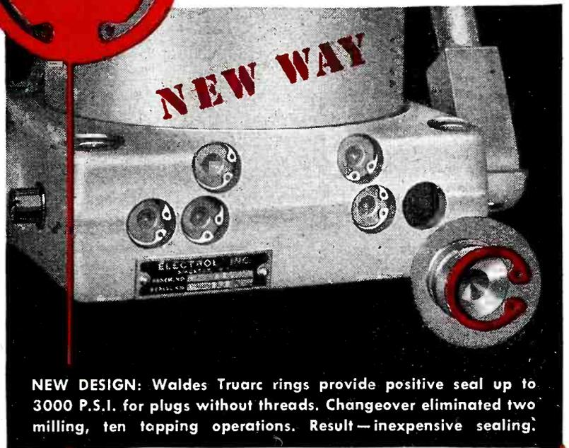
**NEW DESIGN:** Waldes Truarc rings provide positive seal up to 3000 P.S.I. for plugs without threads. Changeover eliminated two milling, ten tapping operations. Result—inexpensive sealing.
