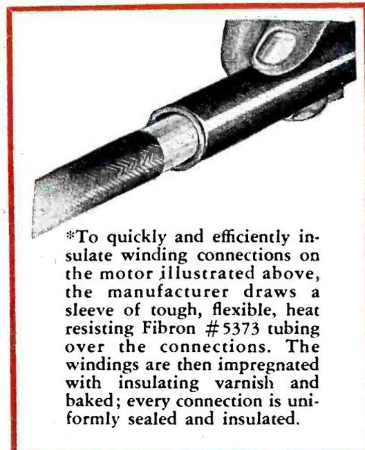
\*To quickly and efficiently insulate winding connections on the motor illustrated above, the manufacturer draws a sleeve of tough, flexible, heat resisting Fibron #5373 tubing over the connections. The windings are then impregnated with insulating varnish and baked; every connection is uniformly sealed and insulated.
