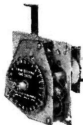
nance-free service. The Type TSC-9 switch may be connected to allow intermittent use of the radio until the time paid for has been exhausted. As many as 6 coins, providing a maximum of 12 hours use, may be deposited at one time. A continuous coin counter registers deposits up to \$25.
