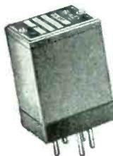
Constant temperature oven and crystal assembly in compact case. Heater current 1 ampere at 6.3 volts. Stabilizes crystal temperature at 70° C for close tolerance requirements in VHF services.
