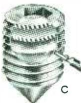
(C) Knurling of this "Unbrako" Socket Set Screw swages the threads and makes it a most excellent Self-Locker—for use where the points such as: flat, dog, cone and oval do not lend themselves to knurling. Sizes from #4 to 1-1/2" in diam.
