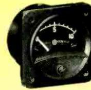
**SMALL PANEL . . .** These general-purpose panel instruments are particularly suitable for use in radio and communications equipment where accuracy and quality are required and space is at a premium. D-c, r-f, and a-f instruments operate on the permanent-magnet, moving-coil principle; alternating-current (a-c) instruments, on the moving-iron principle. 1 1/2 in. and 2 1/2 in. instruments find wide usage where minimum frontal dimensions and depth behind the panel are essential requirements.
