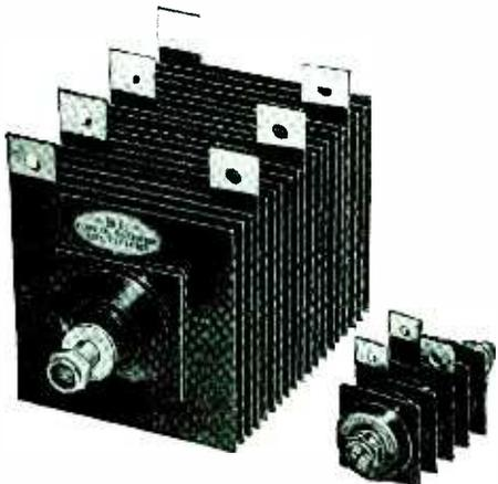
(Large Stack) Copper Sulphide. Three phase bridge, fan cooled. Output rating 100 amperes, 7 $\frac{1}{2}$  volts DC. Size over all 8" x 4 $\frac{1}{4}$ " x 3 $\frac{1}{2}$ ".
