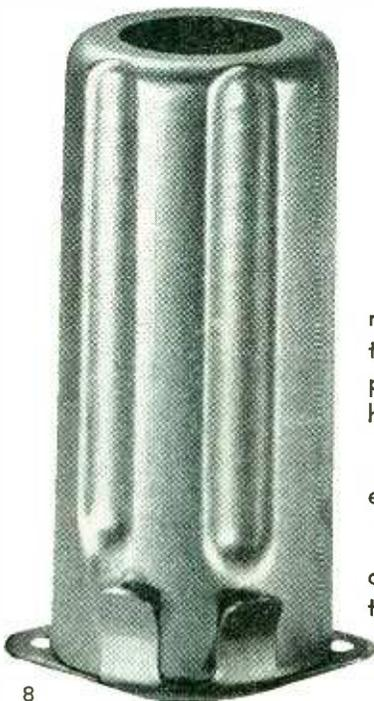
The shield is sized so that three of the flutes make a slide fit with the tube, supporting it throughout its length. A hardened and tempered spring steel clip locates the shield and holds the tube firmly in place.
