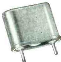
Midget holder with aluminum plated crystal mounted between spring contacts on wire supports. Hermetically sealed metal case protects assembly. Recommended for use only with low power oscillator tubes and circuits where space is at a premium.
