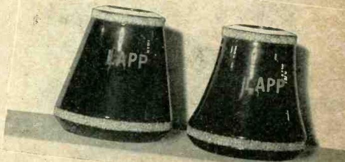
*All Lapp footing and guy insulators incorporate the Lapp patented curved-side compression cone (right). With the same dimension and same wall thickness, the curved-side cone has double the strength of the straight-side cone (left).*
