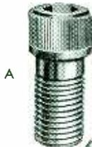
(A) The "Unbrako" Socket Head Cap Screw is a time-saver because the knurled head provides a slip- and fumble-proof grip—though the fingers and head be ever so oily—therefore, it can be screwed-in faster and farther before it becomes necessary to use a wrench. Sizes from #4 to 1-1/2" in diameter.
