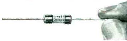
Because of their compactness, resistance to shock and vibration, and elimination of heater supplies, Sylvania Crystal Diodes have found widespread use in many types of circuits.
