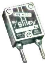
Gasket sealed holder with pressure airgap crystal assembly. Ideal for multichannel applications. Accommodates quartz plate up to .7" x .9" for adequate activity in medium power circuits. Used widely in marine radio-telephone equipment.
