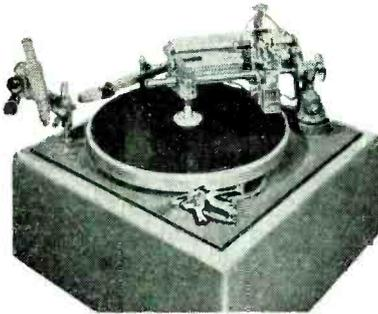
**8N Recorder (16")** is well known to broadcast and recording engineers. It is a rim driven unit employing a heavy cast iron turntable and an overhead mechanism of unusually solid construction which is driven from the center of the turntable. Change of feed pitch and direction is accomplished by changing feed screws.
