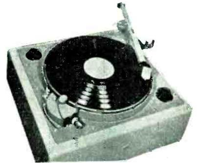
**62A Transcription Turntable** has been widely used by broadcast stations and recording studios during the past five years. It is rim driven through a machined rubber tire at the outer diameter of the turntable, providing a very simple and quiet drive.
