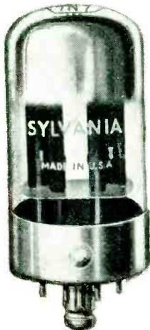
In Sylvania Lock-In receiving tubes, the contact pins are sealed into the glass bottom, thus eliminating the need for soldered connections. No top cap connections are used — a feature which contributes to compactness. Many Lock-In types are especially suitable for UHF applications, because of their low lead inductances, low interelectrode capacitances and low dielectric losses.
