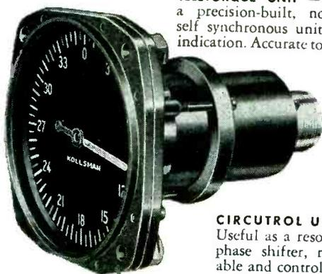
**CIRCUTROL UNIT:** Useful as a resolver, phase shifter, rotatable and control transformer or phase indicator.
