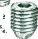
(B) The knurled cup point of this "Unbrako" Socket Set Screw makes it a Self-Locker—the point digs-in and stays dug—regardless of the most chattering vibration. Yet, it can be backed-out with a wrench and used over and over again. Sizes from #4 to 1-1/2" in diameter.
