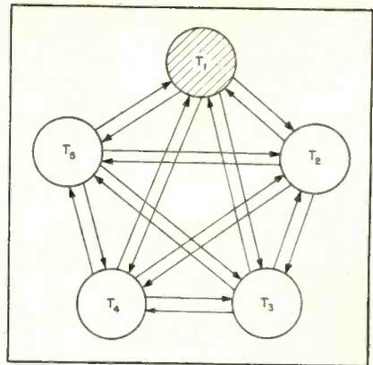
FIG. 1—Basic counter circuit consists of interconnected tubes; the number of tubes is determined by the desired scale base, the circuit here being for a base of five
