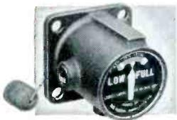
Two G-E sintered ALNICO permanent magnets, separated by an aluminum diaphragm, function as a leakproof magnetic coupling in this gage to accurately indicate the level of the insulating liquid in transformers. The rise or fall of the float actuates the dial pointer by means of the coupling.
