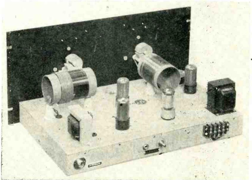
Each transmitter chassis contains r-f and a-f stages
