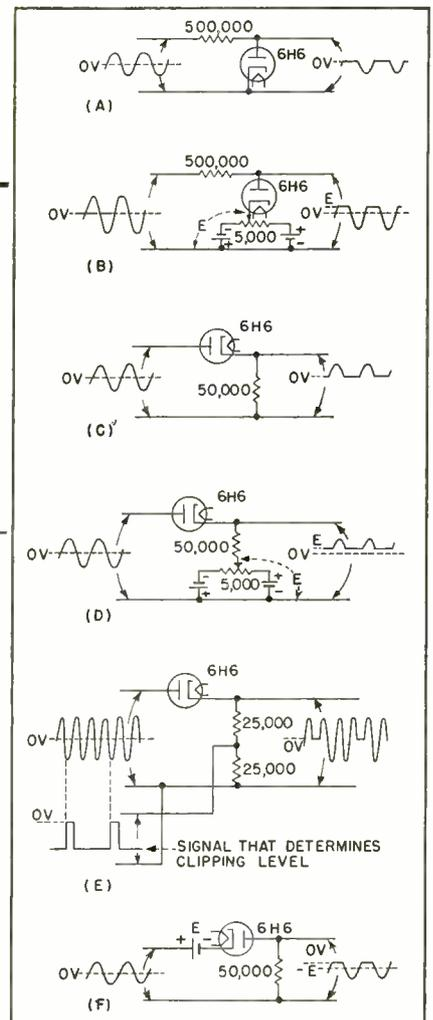
FIG. 1—Basic series and shunt diode clipping circuits
