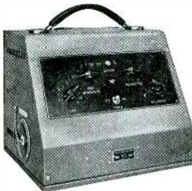
An Electronic Replacement For Sensitive Galvanometer Systems
