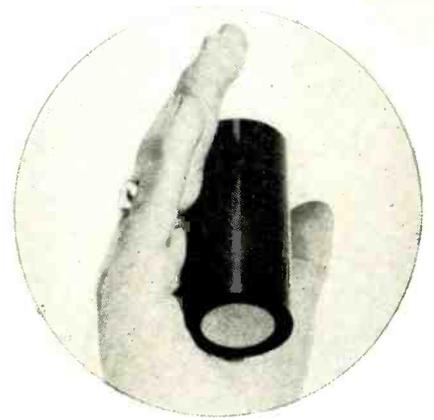
Bakelite-encased rock sample into which the tracer is injected for x-raying. Developed by Gulf Research Laboratories, the x-ray technique shows the behaviour of the entire stratum from which the sample was taken
