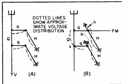
FIG. 5—Fundamental circuit of triplexer (A) showing use of two frequency-selective tuned elements, and method of adding stub elements (B) for coupling an f-m transmitter. Circuit lines represent inner conductors of coaxial lines, and ground symbol indicates shorting plug in line
