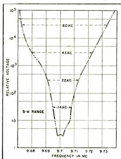
FIG. 5—Selectivity curves for the two a-m bands
