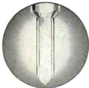
The jewelled point, with 87° included angle, correct radius and fine polish, cuts a silent shiny groove for many hours. When dulled or chipped, these points may be resharpened several times. Each resharpened Audiopoint is disc-tested to insure perfect performance. For this service return points through your dealer.
