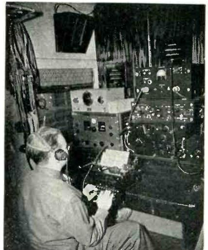
Familiar equipment appears in the receiving room of the communications center that travels with President Truman and his party on the rails. Installed in a former Pullman car, the transmitters and receivers are powered by two diesel 25-kw generators
