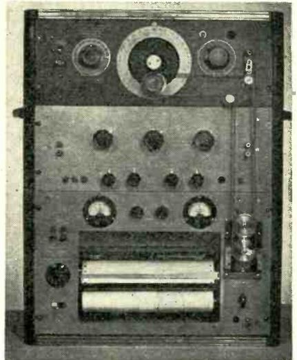
now possible with the Impedance Vectorgraph used in conjunction with a twin recorder and beat-frequency oscillator. Resistance and reactance can be separately and simultaneously recorded from 1 to 4,000 ohms in 6 ranges, with a separate expansion of either scale. Polarity of reactance is indicated. The instrument will find use in measurements of transducers, filters, and transmission lines.
