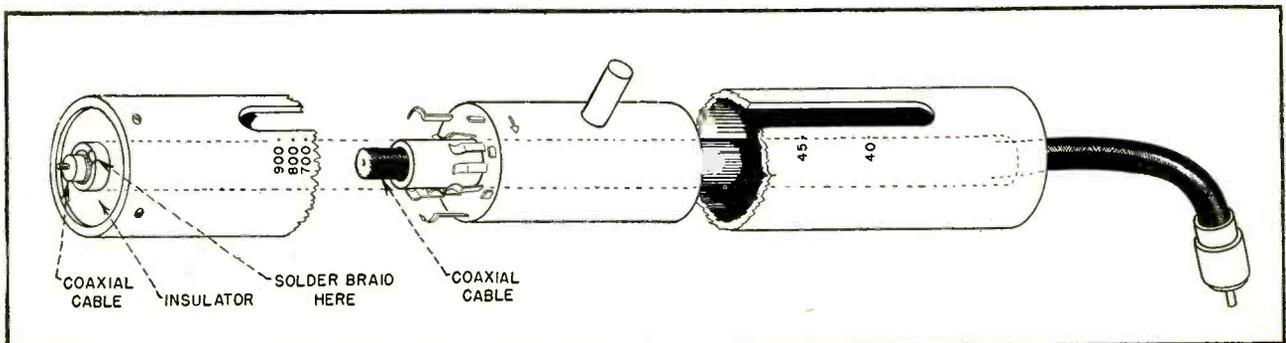
FIG. 4—Variable reactance shown in diagrams is constructed from coaxial cable over which brass tubing is fitted
