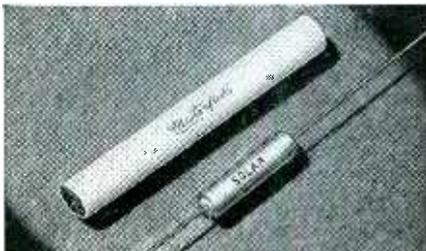
Housed in hermetically-sealed 1/4" diameter metal tubes, Solar Type QA capacitors are of ultra-compact multi-paper and foil construction. They are useful in a wide variety of applications from hearing aids to firing devices. Capacitances up to .01 mf at voltage ratings up to 600 wvdc are standard.
