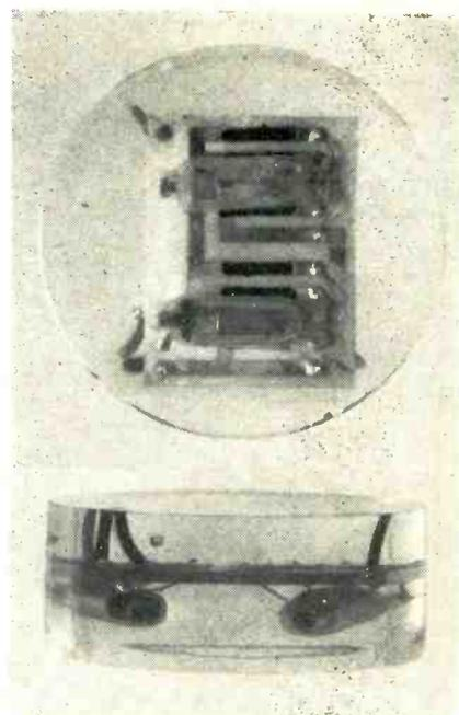
Circuits can be suspended within the casting resin by first allowing a portion of the resin to gel, after which it will support the circuit. The mold (glass or metal) is then completely filled. Printed and subminiature circuits intended for industrial or portable use can be protected from damage by potting
