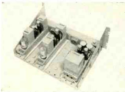
plug-in construction allows equipment to be quickly removed and an identical component plugged into its place. Another feature of this broadcast equipment is that only the two equipment types and the two tube types are necessary between microphone and transmitter input.
