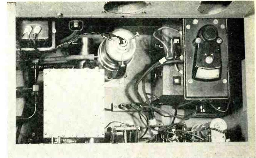
Inside the penetrometer. The smoke cell is center rear, battery box under the galvanometer. The sealed amplifier box appears left front, with a window for viewing desiccant material on top
