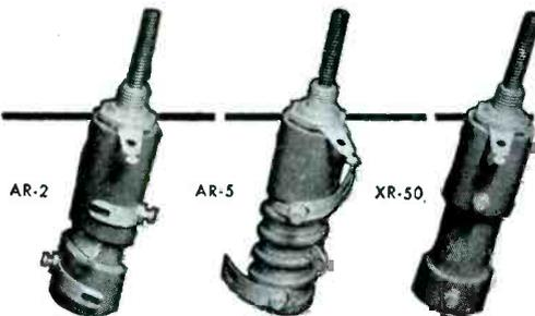
The AR-2 and AR-5 coils are high Q permeability tuned RF coils. The AR-2 coil tunes from 75 mc to 220 mc and the AR-5 coil tunes from 37 mc to 110 mc with suitable capacitors.
