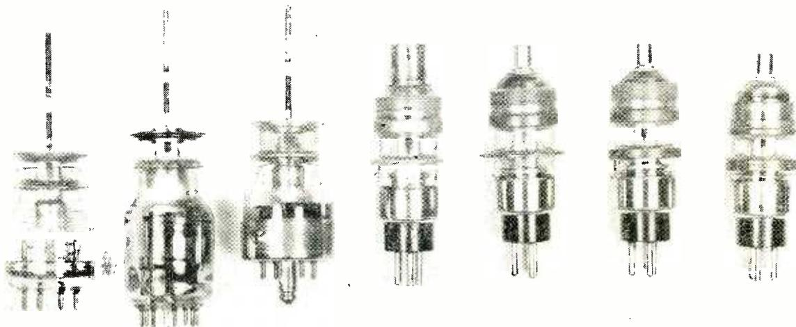
FIG. 1—Development of wide range, external cavity klystrons
