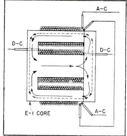
FIG. 1—Arrangement of windings on the core of the reactor. The solid arrows indicate d-c flux lines, dashed arrows the a-c flux lines
