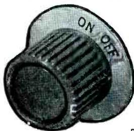
The HRS Knobs are a new series of plastic knobs with a 1 1/8" diameter chrome-plated skirt. They all fit 1/4" diameter shafts. Three types are available in Black or Gray.
