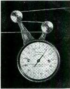
PRODUCE faster, at lower cost. Stops errors and spoilage due to faulty tension of fine wires in coil winding. One tension always works best. The tensometer helps you to determine what this is.
