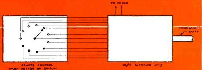
**Automatic Tuning.** The Collins Type 496E Autotune is an automatic repositioning mechanism designed specifically for tuning quality-built home radio receivers and for control of industrial equipment. Its guaranteed accuracy is one part in 36,000. Age, use, wear, and normal changes in operating conditions do not affect its precision or reliability.
