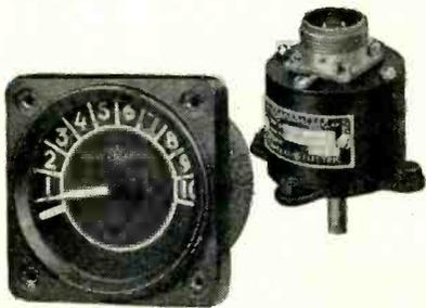
A single d-c selsyn indicating system consumes about 2 watts at either 12 or 24 volts. Any reasonable lead length may be used. Two indicating instruments can be operated from the same transmitter. Bulletin GET-1304 is a comprehensive application manual you'll find extremely helpful. Check it on the coupon.
