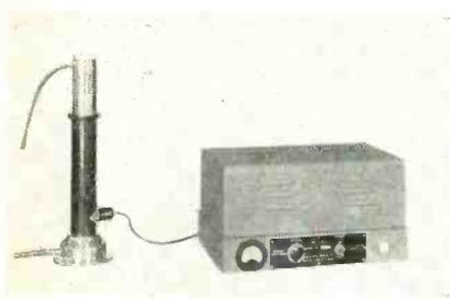
mixtures. The equipment consists of three parts—an electronic driver, a hollow vibrator column, and a cup assembly. Operation is simple and full power is obtained within a minute of connecting to the line. An illustrated bulletin is available.
