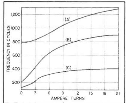
FIG. 3—Curve A applies to a silicon-steel core and a  $0.1\text{-}\mu\text{f}$  capacitor; curve B, mu-metal core and  $0.02\text{-}\mu\text{f}$  capacitor; curve C, mu-metal and  $0.1\text{-}\mu\text{f}$
