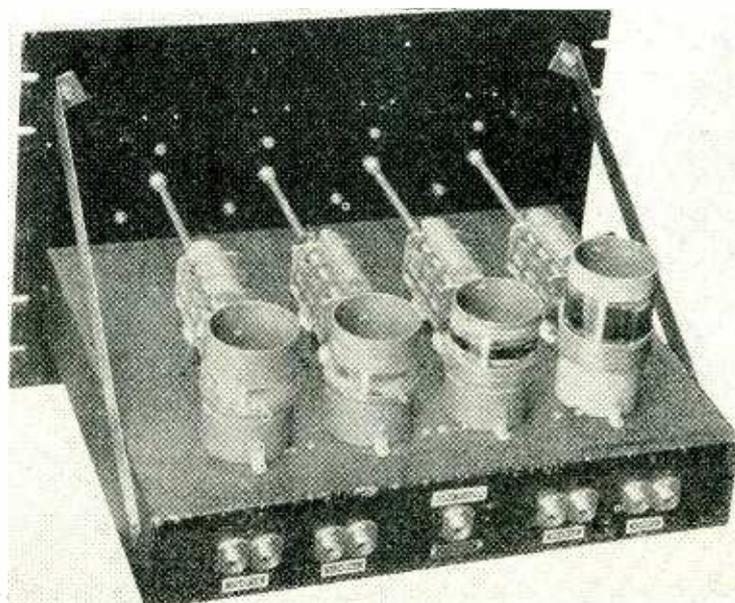
FIG. 3—Coupling unit for standard broadcast frequencies
