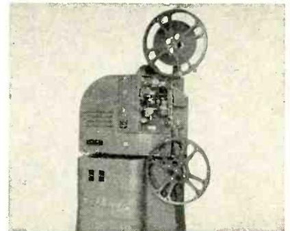
introduction of elliptical gears so that the film motion is effectively synchronized with standard television signals. Radio-frequency voltage is used on the exciter lamp filament of the sound section and a stabilizer is provided to insure sound reproduction at virtually the originally recorded pitch.
