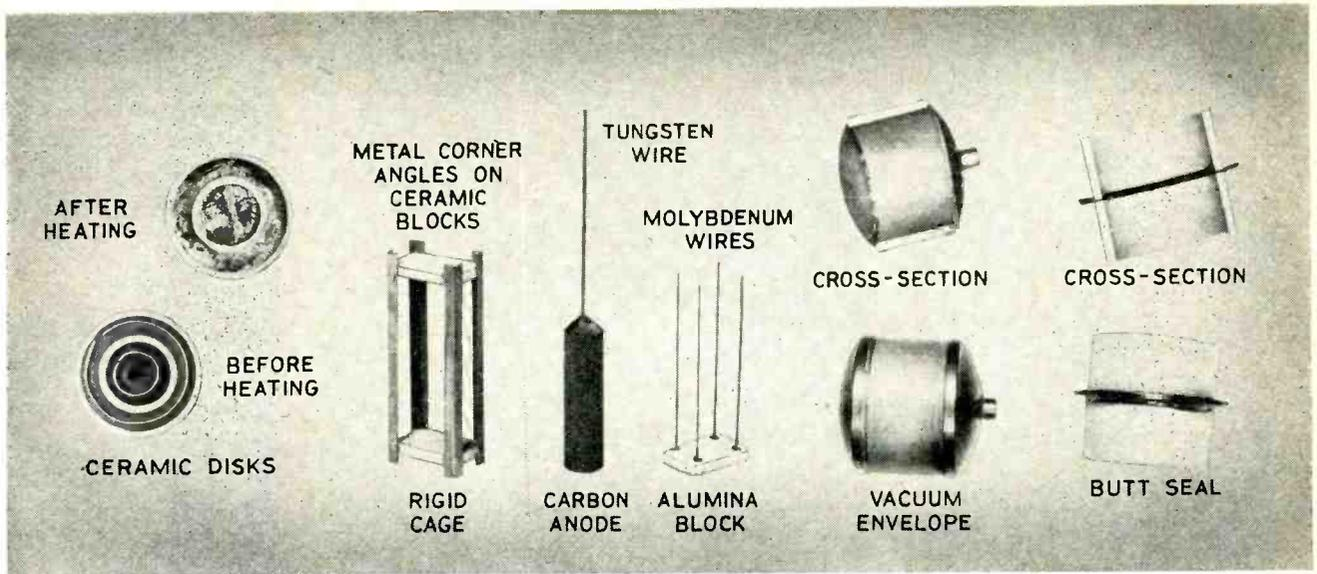
Typical examples of metal-ceramic metallizing, joining, and sealing as produced by new titanium hydride technique
