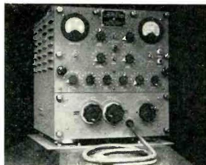
is designed to furnish an r-f signal for calibration and alignment of receivers or for general laboratory work in the range from 1,200 to 4,000 mc. Unmodulated, pulse-modulated, or frequency-modulated signals can be selected at will. The oscillator is a velocity-variation reflex type using an adjustable cavity.
