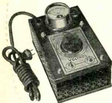
The Acme Voltrol provides a full range stepless control from 0 to 135 volts. Its regulation is accurate to within 4/10 volt adjustment. Unlike resistance regulators, the output voltage is practically independent of the load. Voltrol is the ideal testing instrument for predetermining the performance of any electrical device or product under voltage fluctuation conditions. Available in portable model (illustrated) and panel mounting types. Write for Bulletin 150.
