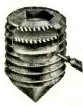
Knurling the threads of this "Unbrako" Socket Set Screw, as shown, turns it into a most excellent Self-Locker—for use where the points such as: flat, dog, cone and oval do not lend themselves to knurling.
