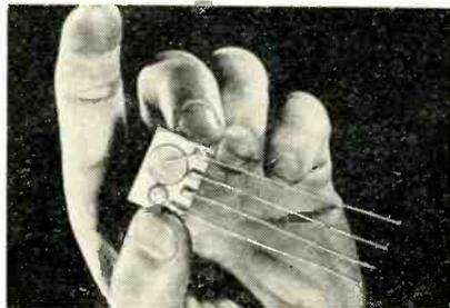
of all radio receivers now in use or production measures 1 by 3/4 by 1/2 inch. It comprises a coupling capacitor, 0.01 microfarad; plate r-f bypass, 250 micromicrofarads;
