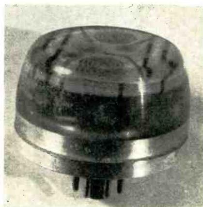
This subminiature printed plug-in multi-stage electronic industrial control unit (about 2.25 inches in diameter) is potted to provide mechanical-electrical stabilization
