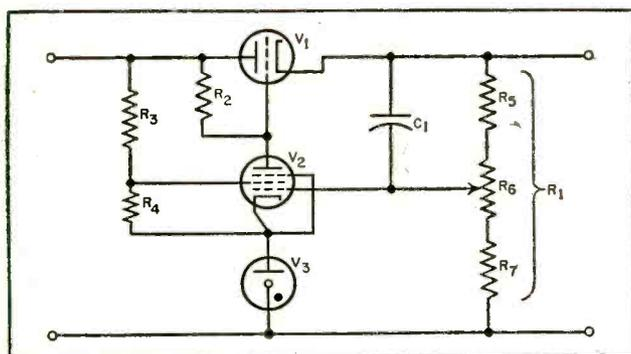
FIG. 4—Control section of a regulated supply. The text describes the values and reasons for selecting them
