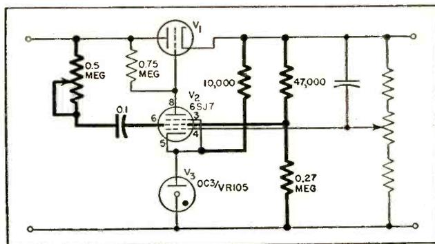
FIG. 5—Modification of the fundamental regulating circuit for extremely low ripple is shown by the heavy circuit lines
