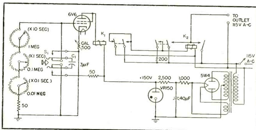
Schematic circuit diagram of the timer. The period is controlled by reduction of bias on the tube. Power is handled by the second relay  $K_2$ .
