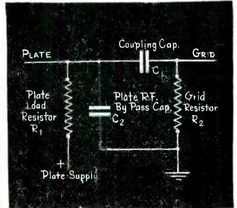
**4** First commercial application of the "printed circuit" and now available for the first time, Centralab's new *Couplate* offers a complete interstage coupling circuit which combines into one unit the plate load resistor, the grid resistor, the plate by-pass capacitor and the coupling capacitor.
