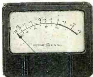
**VU METERS** are now normally stocked in the following styles: non-illuminated, no mask, "A" scale; illuminated, no mask, "A" or "B" scale. Black covers are standard; gray covers can be furnished.
