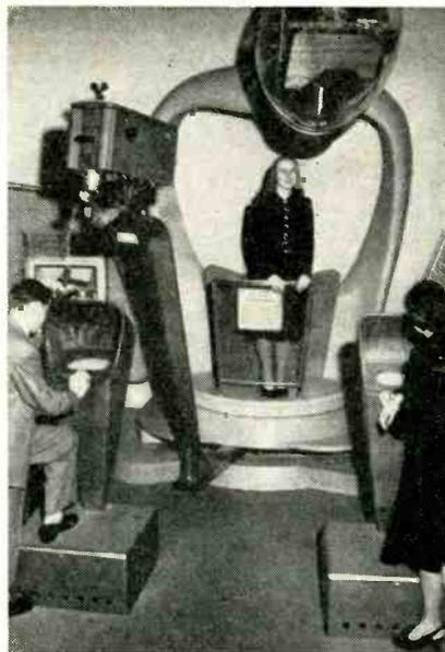
See yourself by television in this corner of the newly opened RCA Exhibition Hall in New York city. Step up on the circular platform, press a button, and the camera boom at the left will make a 120-degree traverse to show all sides of your face as you watch the screen of the television receiver in the plastic dome overhead. Friends can watch repeater screens in the foreground
