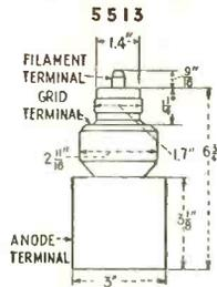
type. At  $I_b$ , 0.4 amp and  $E_c$ , 10 v,  $\mu$  is 87
