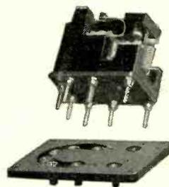
Three contact arrangements—single-pole, single-throw; double-pole, single-throw; double-pole, double-throw—provide further design flexibility. Heavy silver contacts are rated 10 amps continuous at 115/230 volts, 60 cycles, and will safely close on 45 amps and open on 20 amps maximum. Check Bulletin GEA-4668 below for further details.
