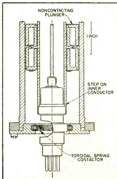
FIG. 4—Special features of cavity
