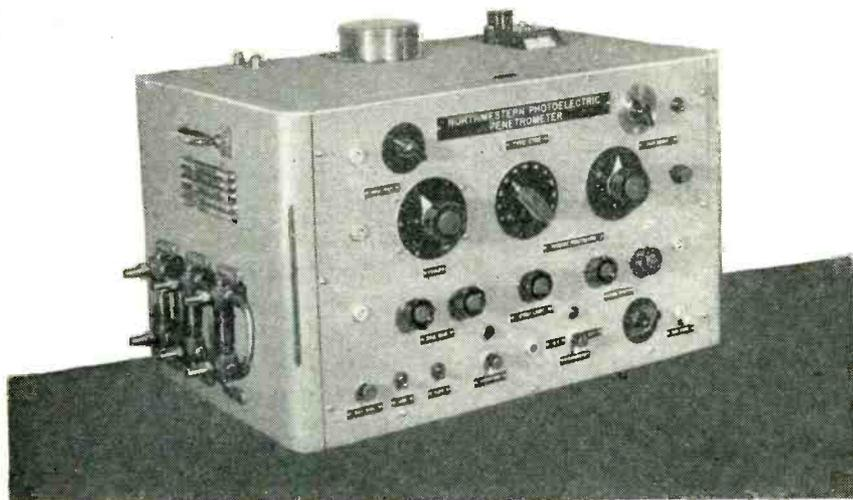
External view of the photoelectric photometer, or penetrometer. Smoke manifold is at the left
