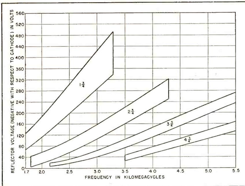
FIG. 6—Reflector mode characteristics. These characteristics are simplified to show only the tube modes omitting a multiplicity of cavity modes
