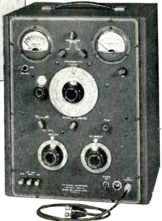
quencies ranging from 50 cycles to 15 kilocycles, any one of which may be conveniently selected by a rotary type switch for either amplitude or frequency modulation.
