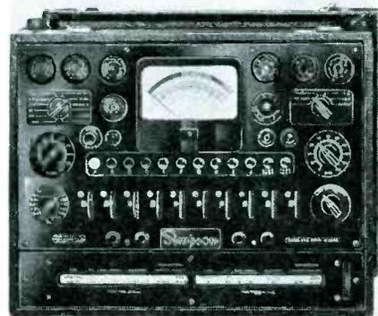
with an automatic reset mechanism that returns all switches to normal at the end of each test. Sockets for all types of tubes are provided.
