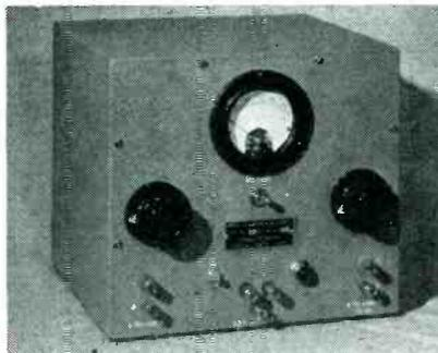
up to 300 volts at 50 milliamperes; down to minus 105 volts bias; and 6.3 volts at 2 amperes for heaters. Regulation is within 1 percent over most of the range. A voltmeter reads either positive or negative outputs.
