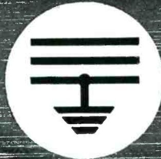
It stands for a three-wire system, with the third wire grounded. It means added personal safety and insurance against shock from "hot" circuits.
