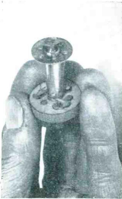
Sensing element of the leak detector, a diode of unusual design employing positive ion rather than negative electron emission and operating in air
