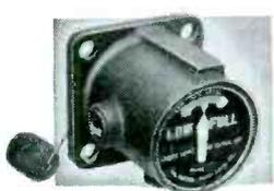
Two G-E sintered ALNICO permanent magnets, separated by an aluminum diaphragm, function as a leakproof magnetic coupling in this gage to accurately indicate the level of the insulating liquid in transformers. The rise or fall of the float actuates the dial pointer by means of the coupling.
