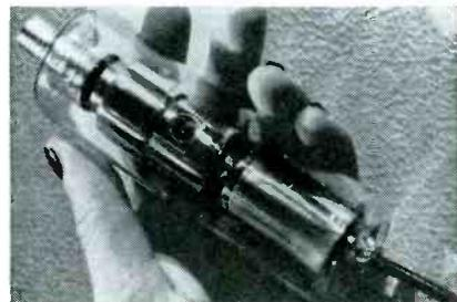
window can be used because the hooded anode reduces the electron bombardment of the envelope. Information is available on several tubes that make up this new line.
