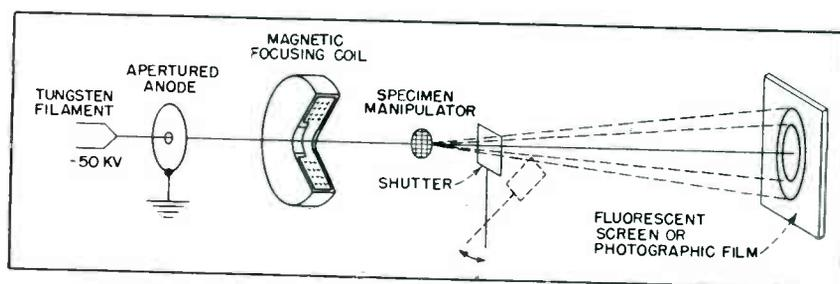
Elements of electron diffraction instrument show its operating principle
