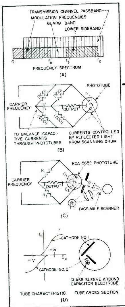
FIG. 1—Basic considerations in design of bridge modulator for facsimile
