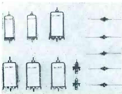
formers are stagger tuned, have a 4-mc bandwidth, with sound rejection of 150 to 1 and adjacent channel rejection of 100 to 1.
