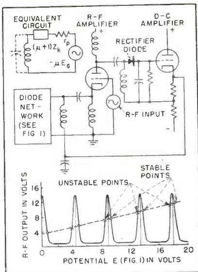
FIG. 2—Circuit stabilizes voltage
