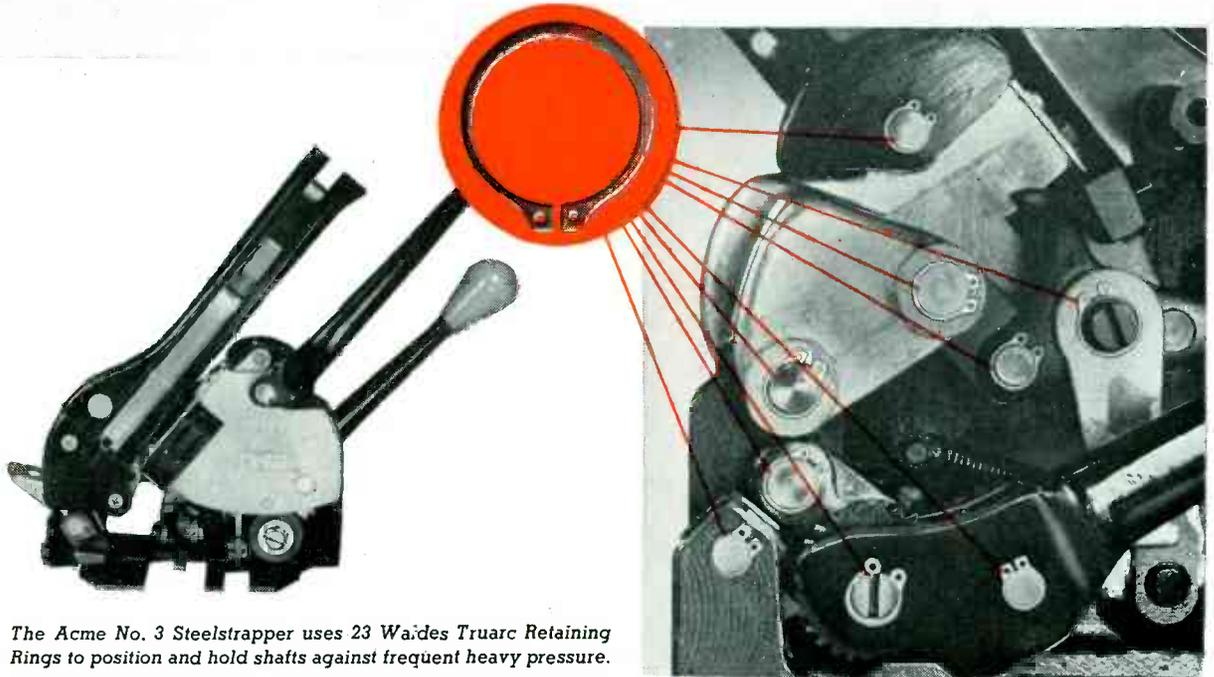
The Acme No. 3 Steelstrapper uses 23 Waldes Truarc Retaining Rings to position and hold shafts against frequent heavy pressure.
