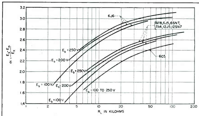
FIG. 4—Curves giving value of  $\alpha$  in terms of load resistance and plate voltage for several types of tubes
