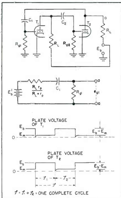
FIG. 1—Basic zero-bias free-running multivibrator, equivalent circuit, and typical time and voltage relations at the plates of the tube
