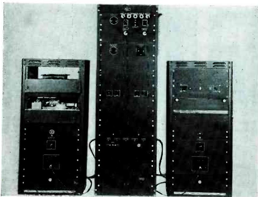
FIG. 2—Experimental sofar receiving station. Recorders and timing equipments are in smaller racks. Center cabinet contains controls, amplifiers and power
