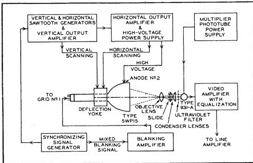
Video signal generator system for slide transparencies, using the RCA Flying Spot tube
