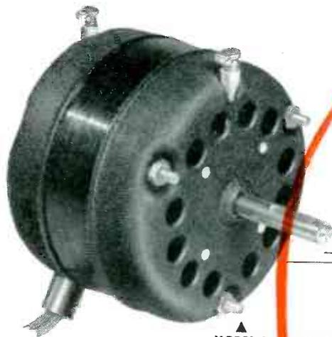
**MODEL A**—6-pole shaded pole induction motor • 60 and 50 cycles • Approx. 1000 R.P.M. full load speed • Size— $4\frac{1}{2}$ " O.D. • Length— $2\frac{3}{4}$ " to  $4\frac{3}{8}$ " depending on variable stack length • Rated at approx. 1/30th h.p. • Comes semi-open or fully enclosed with or without oilers.
