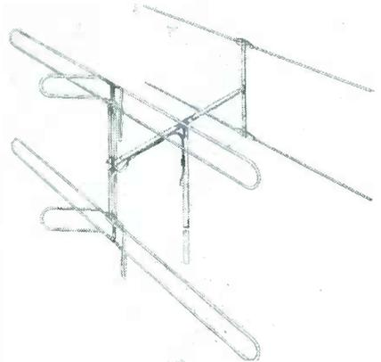
conversion kits has been assembled. In all there are 22 different types ranging from the single straight dipole to the double-stacked folded dipole with high-frequency lobes, as illustrated. The line covers the 44 to 216-mc range, channels 1 to 13 and f-m bands.
