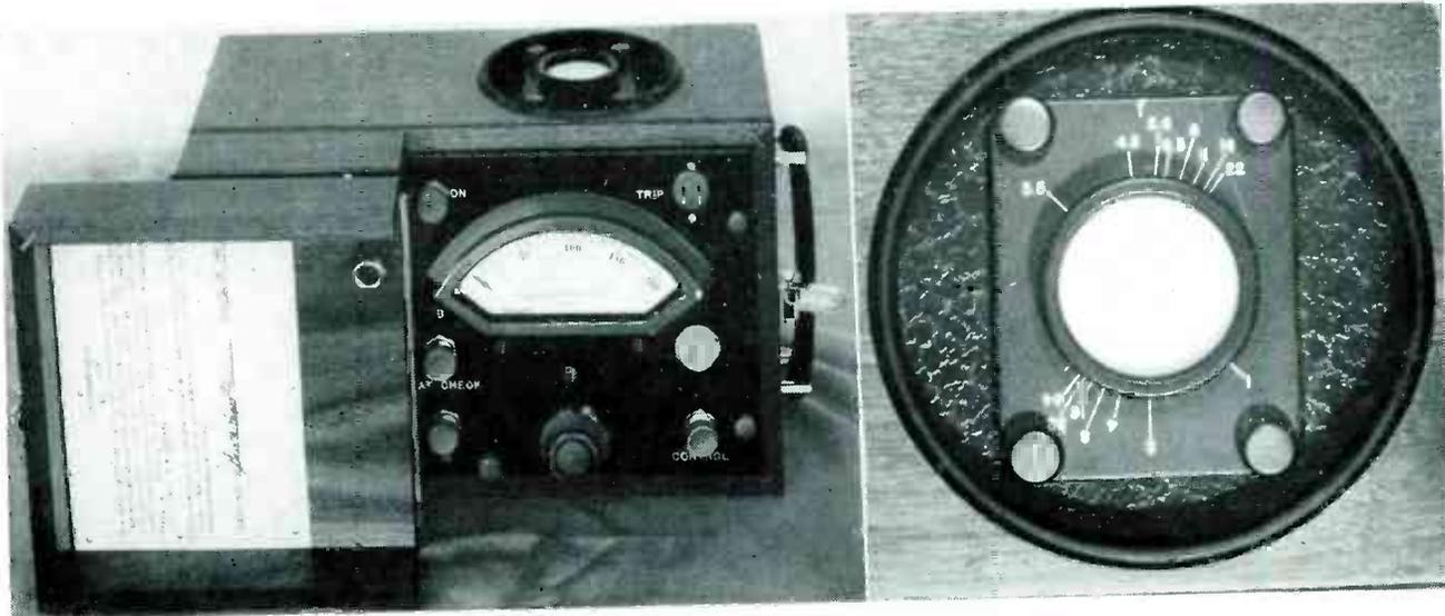
Complete battery-operated photoelectric light-integrating meter as made by General Radio Co., and closeup of phototube aperture containing Polaroid attenuator
