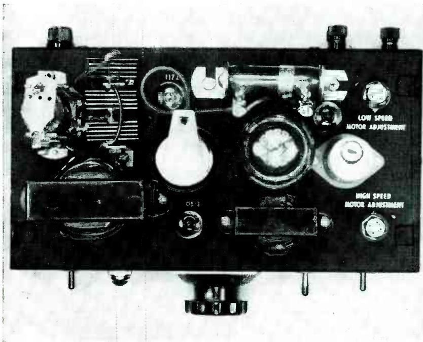
Top view of motor speed-control chassis.
