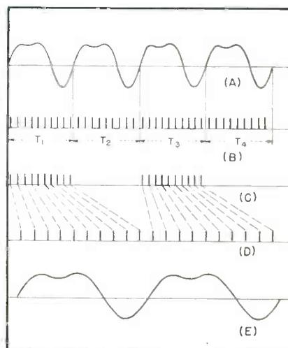
FIG. 1—Basic wave-expanding technique
