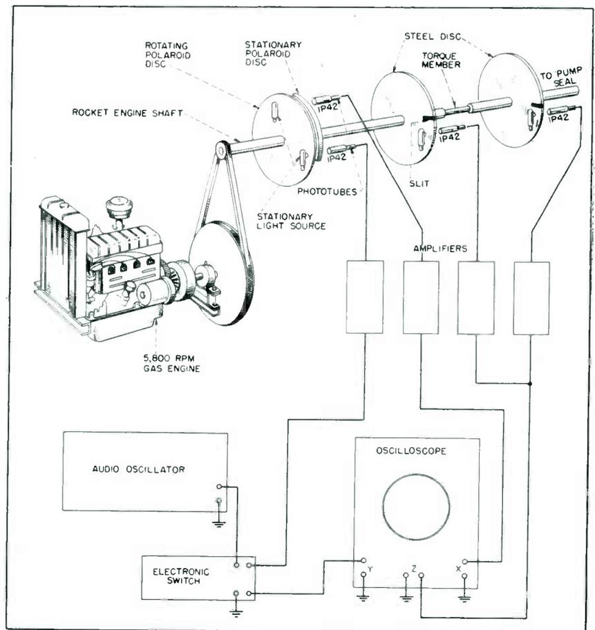
Block diagram of the rocket-engine pump-seal tester
