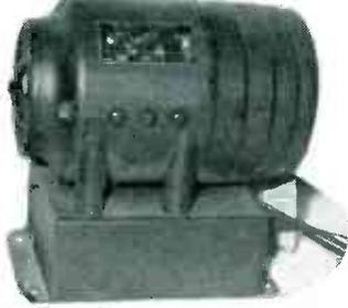
Mfd. by Kato Engineering, for marine or farm installation. Rotary type, compact and ruggedly built for continuous duty. Rubber shock mounting on filter case, with complete input and output filtering. Output-110 volts, 60 cycles AC, .225 KVA, but will operate efficiently on loads up to 300 watts. New units only.
