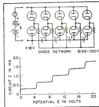
FIG. 1—Basic diode stepping circuit
