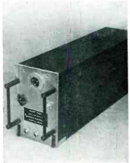
Fixed-tuned f-m broadcast receiver for bus radio service
