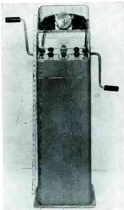
A balloon-supported antenna is used on this lifeboat equipment. When cranked it automatically sends out SOS
