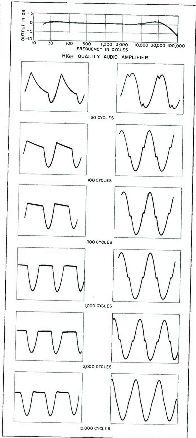
known method utilizes the circuit response to a sine wave. Nonlinear distortion is measured by noting the percentage of harmonics generated in the circuit for various frequencies and amplitudes. The effect of reactance is measured by the variation in gain as the frequency is varied.
