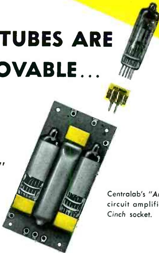
Centralab's "Ampec" printed circuit amplifier using new Cinch socket.
