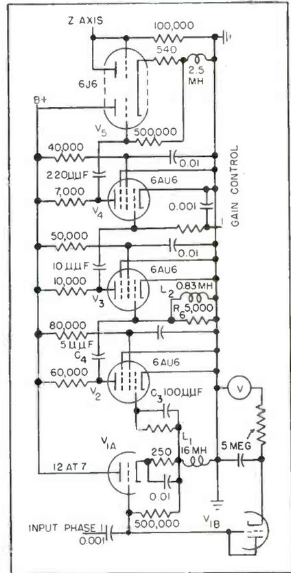
FIG. 4—Pulse generator for one phase
