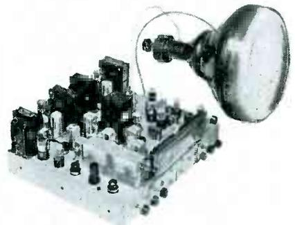
wired and tested unit, less cabinet. The receiver tunes continuously from 44 to 216 mc and a switch is provided to turn off sweep and high-voltage circuits when f-m reception alone is desired.
