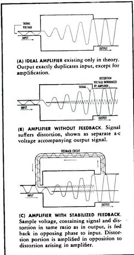
LIKE many other major advances in electronics, the development of stabilized (negative) feedback was a direct outgrowth of telephone progress. To produce telephone repeaters with the necessary gain stability and low distortion, H. S. Black, of Bell Telephone Laboratories, took a sample voltage of the amplifier output and fed it back into the amplifier in *opposing* phase. Before-and-after effects are shown in simplified form in the accompanying figures.
