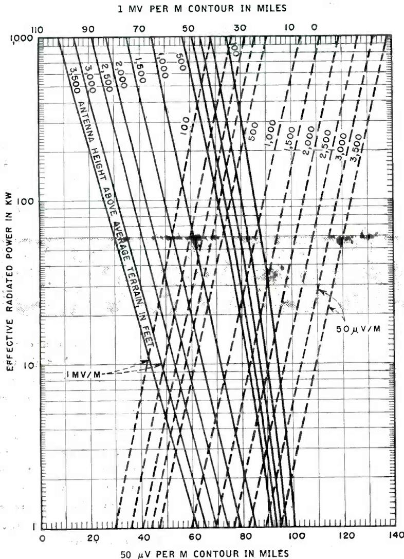
THE accompanying chart, based on FCC data, provides a quick means of determining the approximate service areas of a transmitter operating on any channel between 88 and 108 mc. Distance to the 1 mv-per-meter contour (solid lines) is shown by the upper scale and distance to the 50 microvolt-per-meter contour (dashed lines) by the lower scale, for various effective radiated powers and transmitting antenna heights. Receiving antenna height is assumed to be 30 feet above average terrain.
