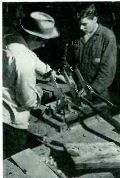
A loudspeaker mount board and several small blocks are glued simultaneously in about 30 seconds with this jig
