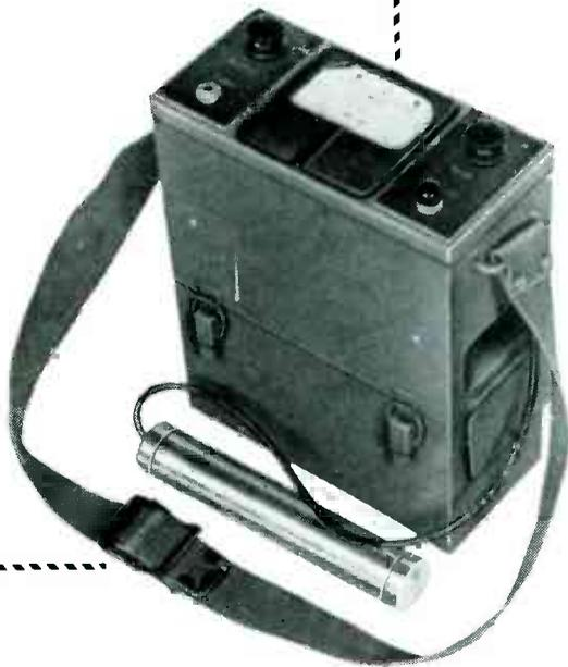
A portable battery operated instrument for the measurement of radiation intensities—incorporating precise, reliable circuits such as are usually found only in elaborate laboratory apparatus.
