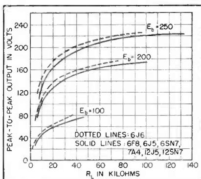
FIG. 2—Variation of output voltage with load resistance for tubes commonly used in multivibrator circuits
