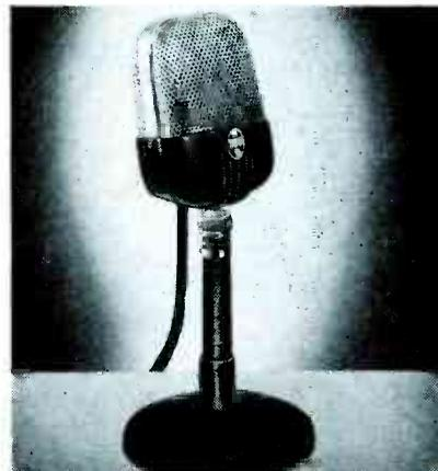
supported in an Alnico V magnet. Response is within plus or minus 5 db from 80 to 10,000 cycles. Level is 62 db below 1 volt per dyne per square centimeter at high impedance. A switch allows use into 50, 200, or 500 ohms.
