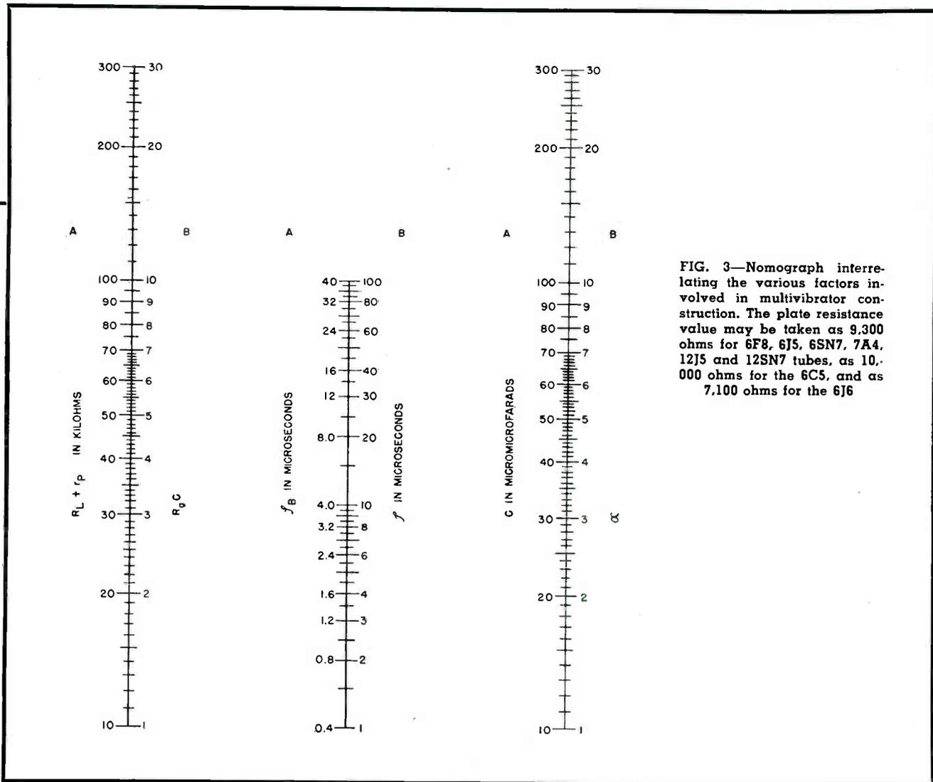
FIG. 3—Nomograph interrelating the various factors involved in multivibrator construction. The plate resistance value may be taken as 9,300 ohms for 6F8, 6J5, 6SN7, 7A4, 12J5 and 12SN7 tubes, as 10,000 ohms for the 6C5, and as 7,100 ohms for the 6J6
