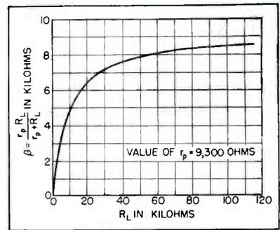
FIG. 7—Effect of load resistance
