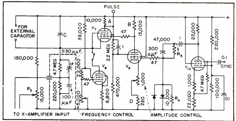
FIG. 5—Simplified schematic diagram of time base generator
