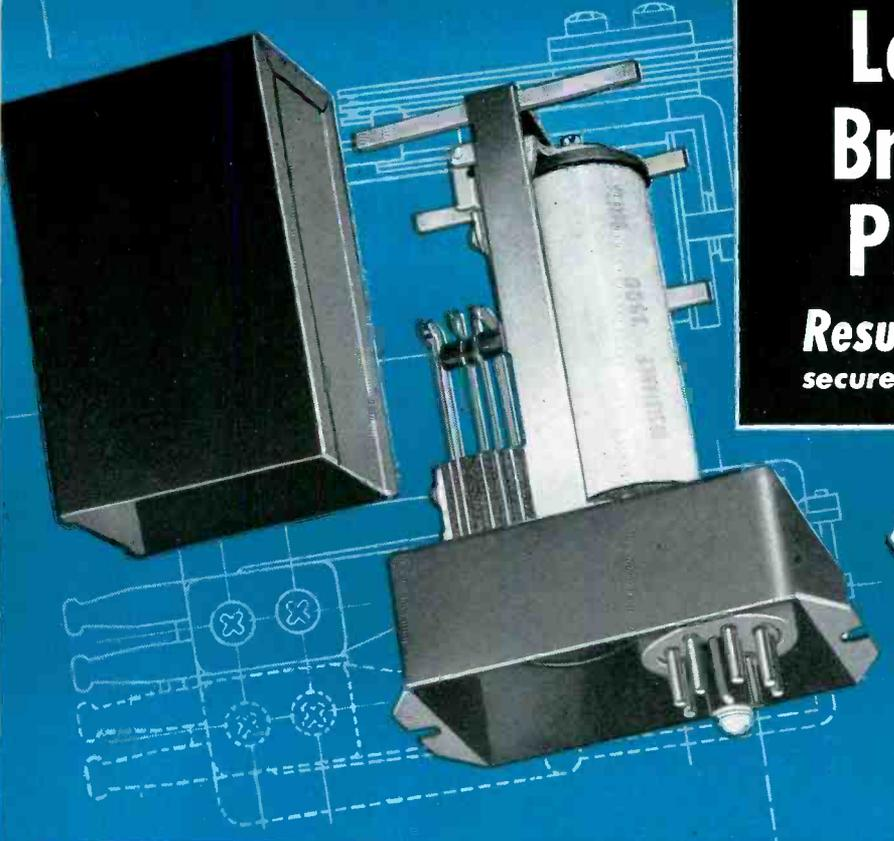
Clare Type "C" d-c Relay, dust-tight mounted on base provided with Neoprene gasket, with easily removable dust-tight steel cover, as developed for Leeds & Northrup.
