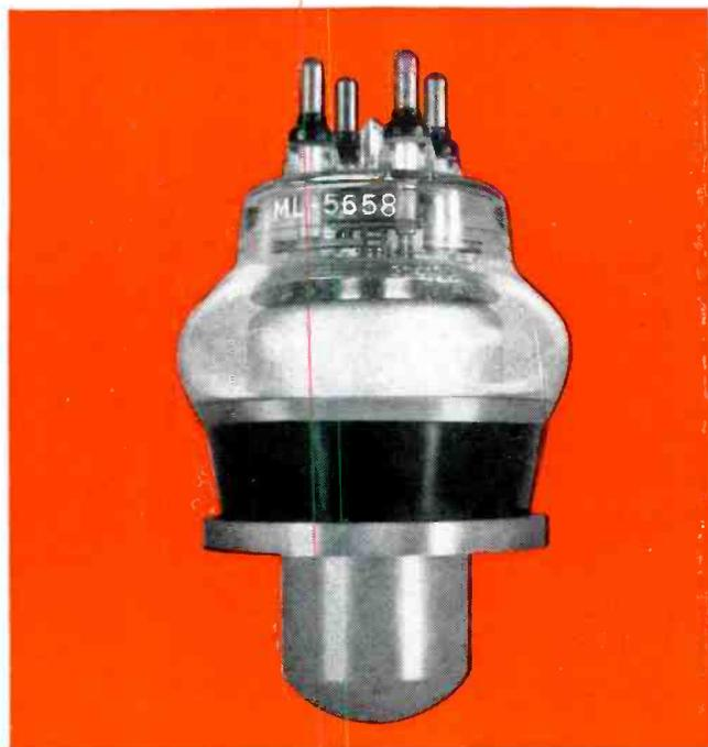
**ML-5658**, water-cooled RF oscillator, amplifier, completely interchangeable with Type 880. Max. Input, 60 kw. Max. Plate Dissipation, 20 kw. May be used at full power at frequencies as high as 20mc., and at reduced powers up to 45mc.
