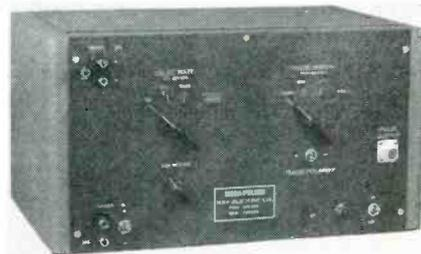
which more than covers the present video frequency range. It operates on 117 volts, 60 cycles, and has a self-contained power supply. Price is \$195.
