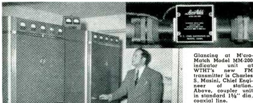
Glancing at Micro-Match Model MM-200 indicator unit at WHTT's new FM transmitter is Charles S. Masini, Chief Engineer of station. Above, coupler unit in standard 1 1/2" dia. coaxial line.
