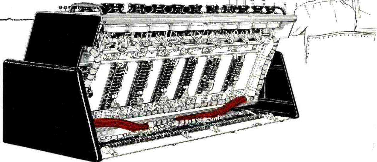
A tilting chassis is a unique feature of this broadcasting studio control made by Collins Radio Company. In rugged laboratory tests, Collins engineers found that the tilting of the chassis caused wires to be chafed. They knew the flexibility of BH Extra Flexible Fiberglas Sleevings from other applications . . . decided to try it in this console.
