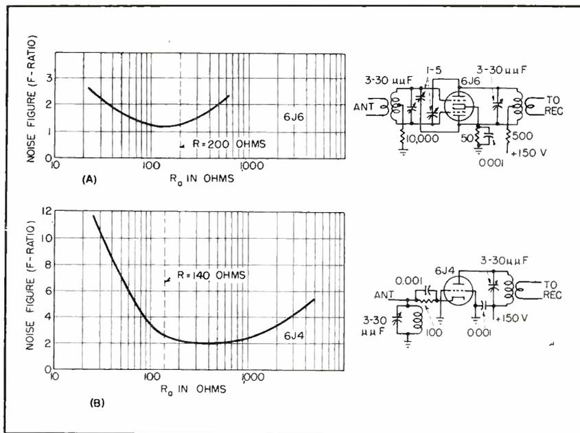
FIG. 4—Preamplifier circuits and measurements
