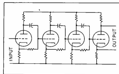
FIG. 3—Three-lattice A or B phase-shift audio network
