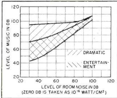
FIG. 1—Preferable dynamic range depends on the ambient noise level in the room
