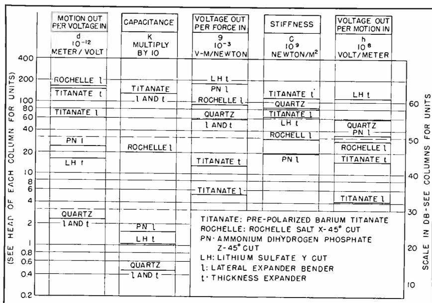
Comparison of electrical and mechanical properties of piezoelectric materials
