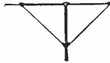
Extended V-Type Dipole Antenna for all frequencies between 44 and 216 mc. Permits proper impedance matching to 300 ohm line for TV and FM.
