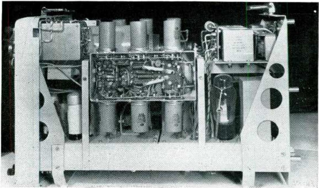
Side view of oscilloscope showing X-amplifier suspended from shock mounts. An identical 6-tube amplifier is suspended on other side of chassis
