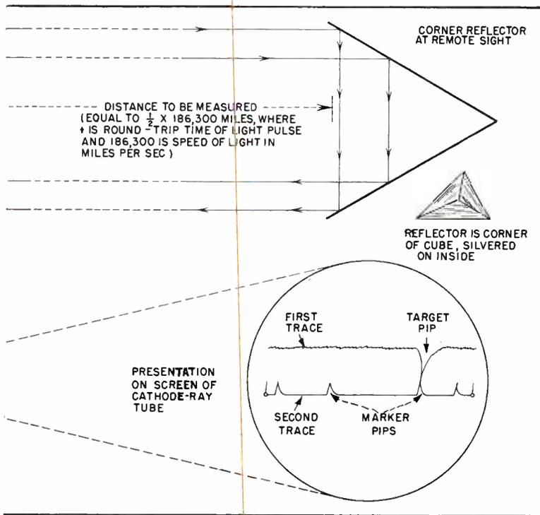
how travel time of a flash of light is used in surveying
