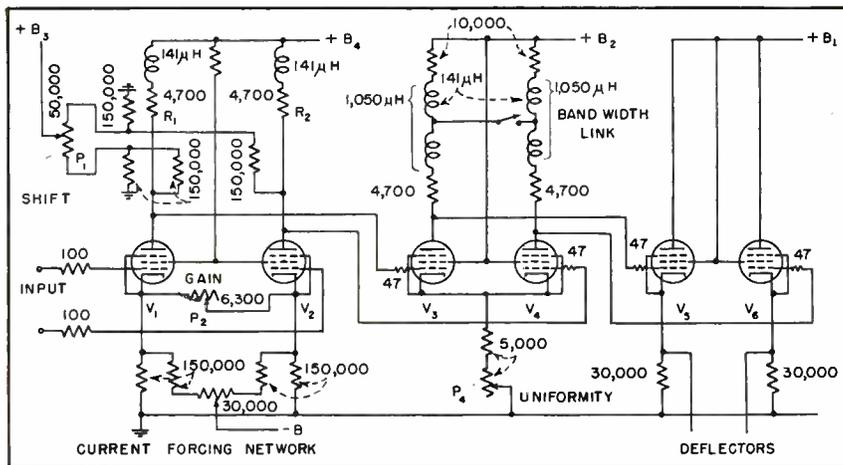
FIG. 2—Detailed circuit schematic of direct-coupled amplifier showing controls
