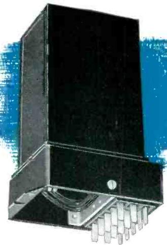
Same installation as changed for use of United Air Lines. Note installation of the 15-point plug and single flange for mounting to chassis.
