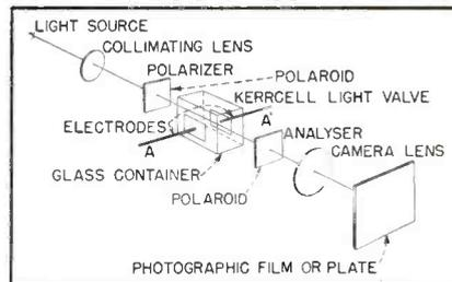
High speed Zarem shutter is Kerr cell between crossed polarizing filters
