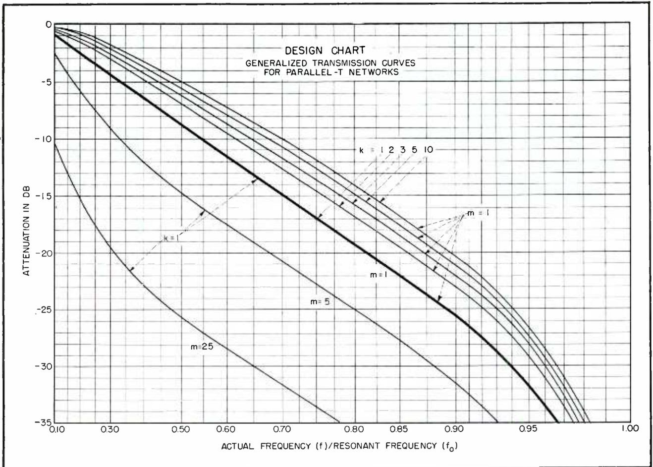
The parallel-T network loads the driving circuit at all frequencies, and at resonance presents an input impedance of  $R_1/2$  for any value of  $k$  when  $m = 1$ . Below resonance this impedance increases and above resonance it decreases. Loading the output of the network with an external load reduces the transmission on both sides of resonance, al-
