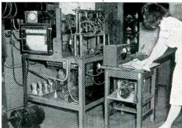
*With this unit, Mallory technicians measure contact resistance, temperature rise, and rate of wear.*
