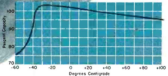
Take advantage of the small size and light weight of Pyranol® d-c capacitors for those applications in freezing temperatures and below. No need to penalize your designs with oversize capacitors resulting from the use of other dielectrics.
