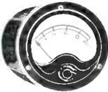
Bakelite cased meter — 27 ohms. Basic resistance may be used wherever a small 1 mil movement is needed for S-Meter in receiver or basic meter in test equipment.
