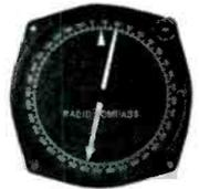
6-12 V. 60 cycles. 5 inch indicator with 0-360° dial. Heavy duty transmitter.
