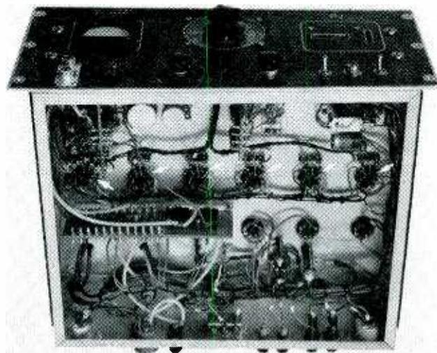
Bottom view of 64 scaler, showing simplicity of wiring. Arrows point to sockets of plug-in units
