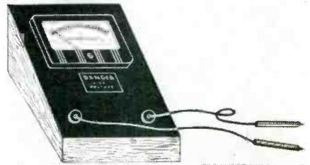
perimenters. The meter, with range from 0 to 30 kv, draws only 20 microamperes. Technical information is available.
