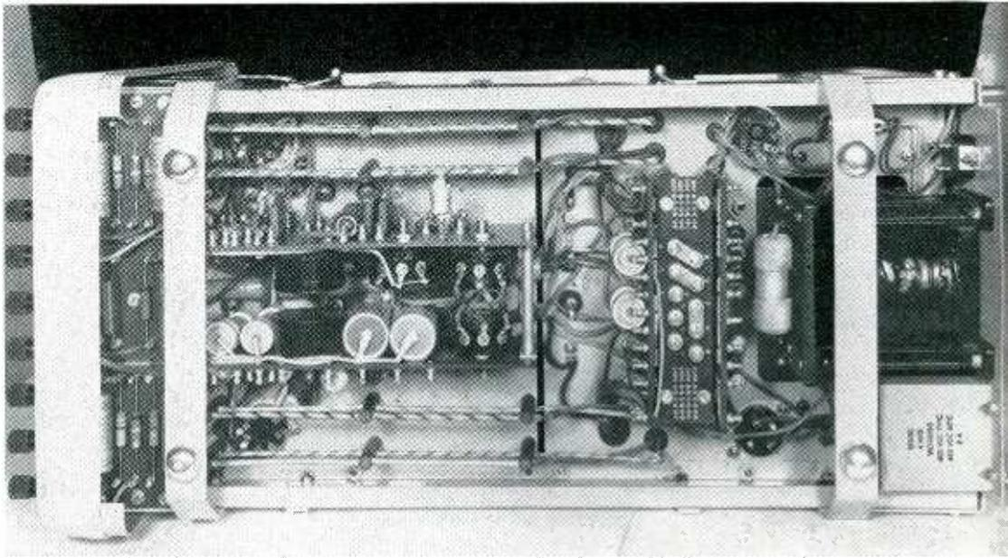
Under-chassis view of the oscilloscope showing preset amplifier controls (left of center) and spaced leads from front terminals to deflector plates
