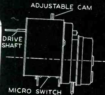
**SYNCHRONOUS TIMING MOTORS**
