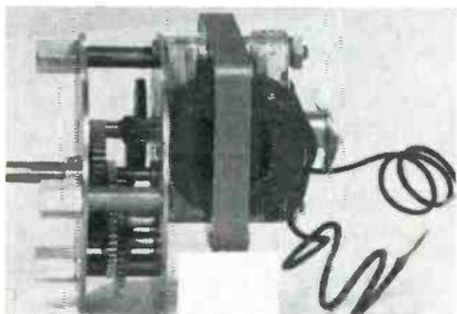
tors can be geared to produce clockwise or counterclockwise speeds from 400 to 1 rpm on the final shaft.
