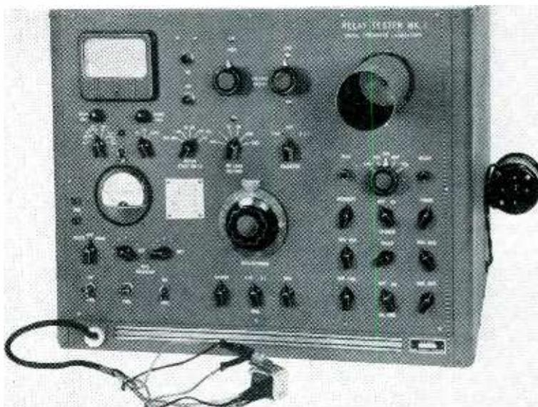
Front view of the relay tester. Color-coded leads correspond to colored schematic engraved on panel
