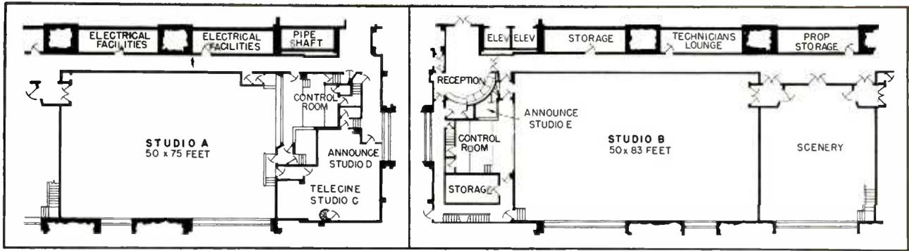
FIG. 1—Partial floor plan of Studio A, film-projection studio. FIG. 2—Simplified floor plan of Studio B, control, announce Studio E, scenery, other storage, and technician's lounge
