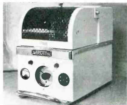
output. Heating rate can be adjusted smoothly from zero to full power by arranging the electrode, raising and lowering a knob at the top of the cabinet. Heat output and timing are indicated by dials.
