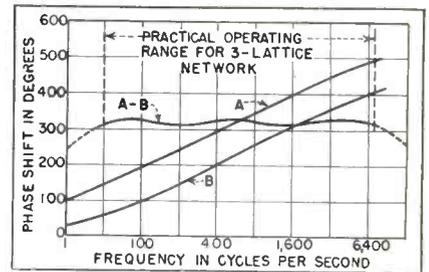
FIG. 4—Characteristics of three-lattice phase-shift network
