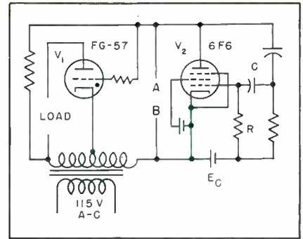
FIG. 3—Reactance-tube phase-control circuit that eliminates the transformer
