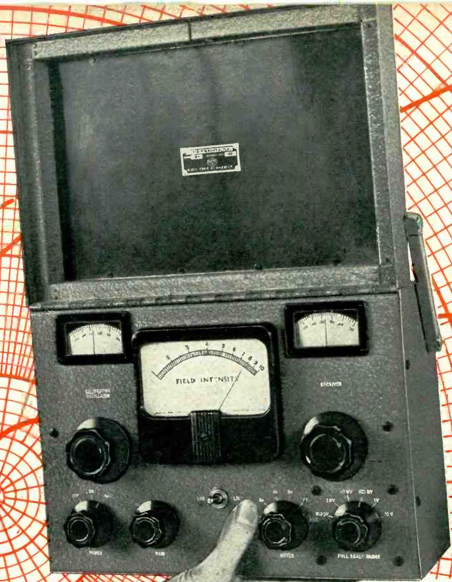
The new *Portable Field-Intensity Meter*, RCA Type WX-2—shown one-third actual size. A loop antenna is built right into the lid!
