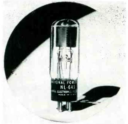
plications. Filament voltage is 2.5; filament current, 7 amp; d-c output, 2 amp; peak-current output, 10 amperes.
