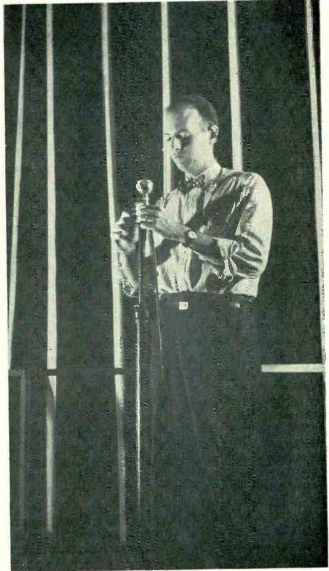
soundproof room and the measurement room, facing the microphone. A motor drive sweeps an audio signal generator gradually from 50 cycles to 20,000 cycles, while an inking pen traces on graph paper the amplified output of the microphone
