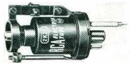
equipment are types 2K26 and 2K25. These tubes can be used both for transmission and reception, serving as local oscillator in the latter service.
