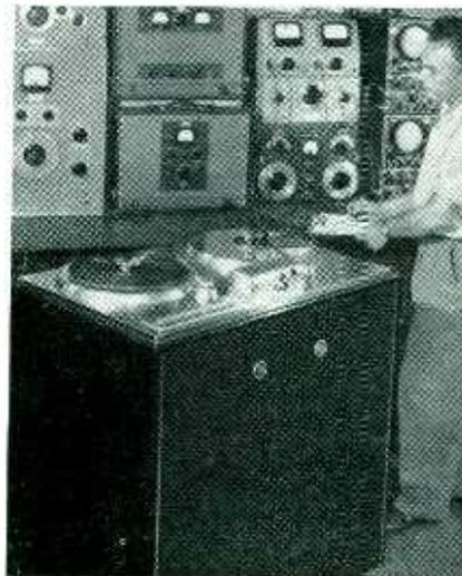
signed expressly for f-m broadcast service, the new Ampex tape recorder has a response within plus or minus 1 db between 30 and 15,000 cycles as well as other features designed for broadcast facility. Tape speed is 30 inches per second and the unit has a time capacity of 35 minutes.
