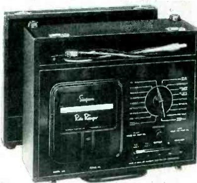
Its many applications include measurements of a-c diode balancing circuits, grid currents of oscillator tubes and power tubes, a-c diode currents and high- $\mu$  plate voltage. Direct-current sensitivity is 20,000 ohms per volt.
