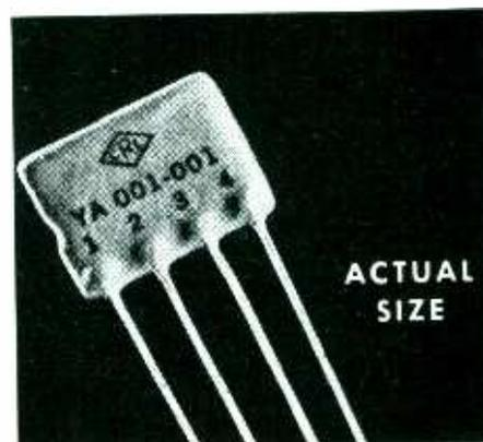
**5** CRL's *Couplate* consists of a plate lead resistor, grid resistor, plate by pass capacitor and coupling capacitor. Write for Bulletin 933.
