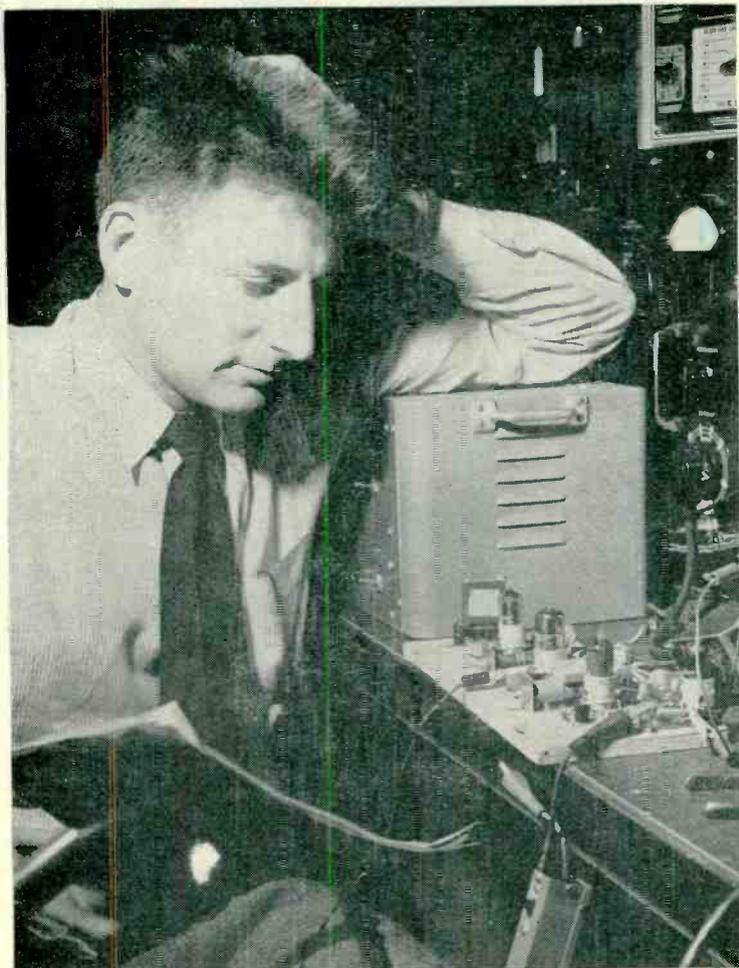
**FAMILIAR BREADBOARD**—A pause for meditation often pays during the breadboard stage of developing a new electronic product. Here is the true old fashioned breadboard, using wood screws to hold the parts on the wood base
