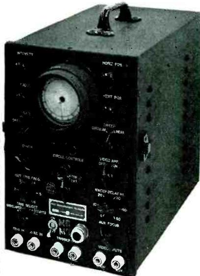
This versatile, accurate, precision built instrument is designed for precise measurement of short time intervals with circular sweep, and for test scope applications with linear sweep.
