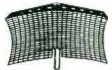
**AN MPG-1** Antenna. Rotary feed type high speed scanner antenna assembly, including horn parabolic reflector. Less internal mechanisms, 10 deg. sector scan. Approx. 12'L x 4'W x 3'H. Unused. (Gov't Cost—\$4500.00).....\$250.00
