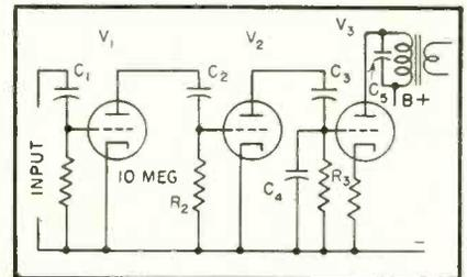
FIG. 2—Essential portions of amplitude discriminator amplifier showing cascaded discriminators and pulse reshaper
