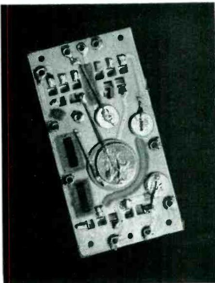
**TYPICAL "AMPEC"** — (actual size, back view) shows how you can get complete electrical circuits—tube sockets, capacitors, resistors and wiring—in one miniature Centralab amplifier unit.
