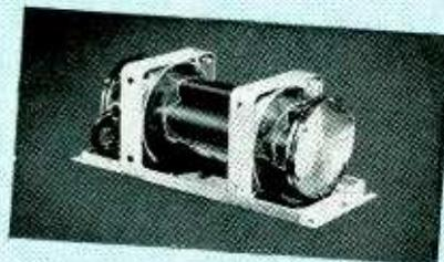
The GT crystal is mounted inside this oven in which temperature is controlled electronically with extreme accuracy. In conjunction with sponge rubber
