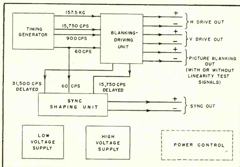
FIG. 1—Interrelation of units forming the sync generator
