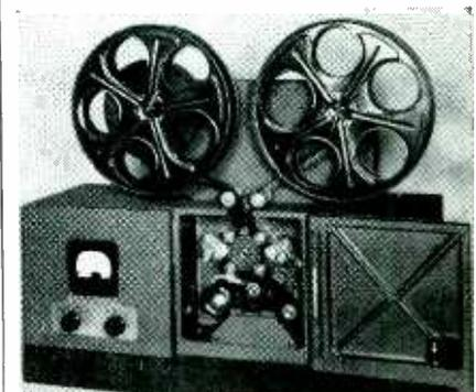
Magnetic recording makes possible this portable film sound recorder for use on location, which has reduced size and weight over comparable optical equipment. Unit at lower center houses both recording and playback heads
