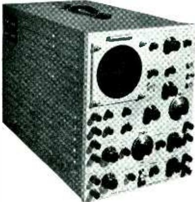
**Tektronix Type 512 Oscilloscope**
