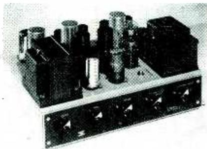
pressor reduces hum level to 86 db below maximum power output under normal operating conditions. Actual hum power level is 0.05 microwatt.
