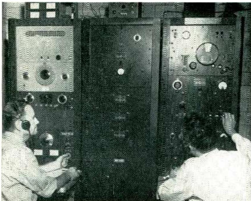
FIG. 10—Frequency-measuring equipment used in calibrating quartz-crystal blanks
