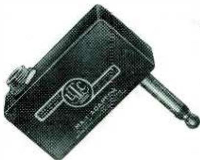
impedance microphones and pickups to high-impedance circuits. The unit matches any source from 50 to 500 ohms impedance to grid. Response is essentially flat from 50 to 10,000 cycles.
