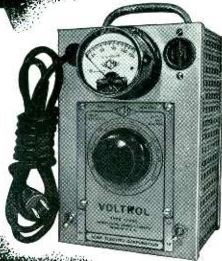
The Acme Electric Voltrol, provides a stepless range of voltage control from 0 to 135 volts. Connected to any 115 volt 60 cycle line, the secondary voltage is manually controlled, in two scale ranges with regulating dial covering complete 360° circle in each range. This permits adjustment to 4/10 volt. Regulation is unaffected by load. For detailed description of construction
