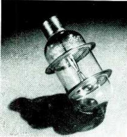
Disc seals such as in this T-R tube are possible because of the thinness and ductility of the copper
