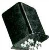
A Modulation Transformer ideally suited for use in ham and commercial speech transmitters. Will deliver 250 watts of Class B audio power from P-P 203A's, 211's, 805's, 75TL's, etc. to a Class C load with response variations not exceeding  $\pm 1$  db. over the speech range, 200-3,500 cycles. Primary impedances, 9000/6700 ohms; secondary impedances, 8000/6000/4000 ohms. A matching driver transformer is available.
