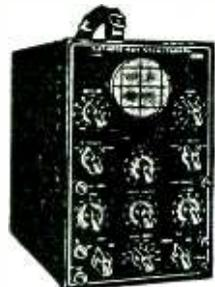
3" CRT operates at accelerating potential of 1100 V — brilliant well - defined trace, Vert amp voltage gain approx 43, horiz amp voltage gain approx 65, Freq. range vert. & hor. amp both uniform  $\pm 3$  DB from 5-100,000 CPS Input impedance 1 megohm vert., .5 megohm hor. Operates 115 V, 40-60 cycle.
