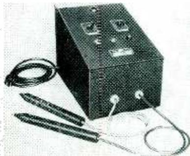
a buzzer and pilot lamp. A high reactance circuit limits output current to a low value to prevent destruction of the material under test and to lessen operator hazard.
