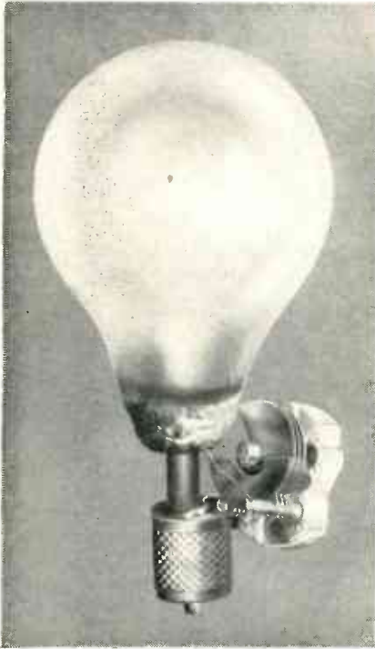
FIG. 1—Low-power dummy antenna consists of a debased 32-volt bulb and a variable capacitor
