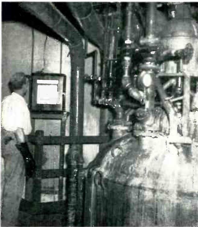
CHEMICAL INDUSTRY Temperature of synthetic resin in processing vessel at right is automatically maintained by Leeds and Northrup controller on storage tank
