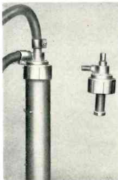
FIG. 3—Complete 5,000-watt dummy antenna is shown at left. The resistive element is at right
