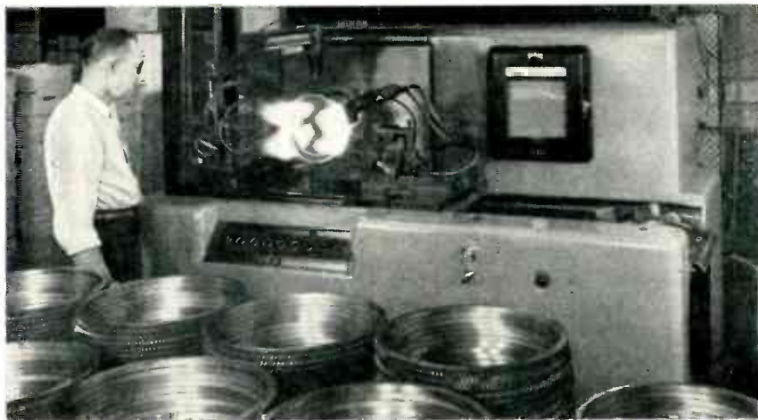
METALS INDUSTRY Newest application of electronic control in this major market for instrumentation maintains surface temperature of gears accurately to within 5 degrees F of required red-heat temperature, for selective surface hardening in Cincinnati Flamatic hardening machine. Sensitive radiation thermopile in overhead housing is focused onto work
