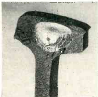
Transverse rail fracture of the type which is now prevented by early detection
