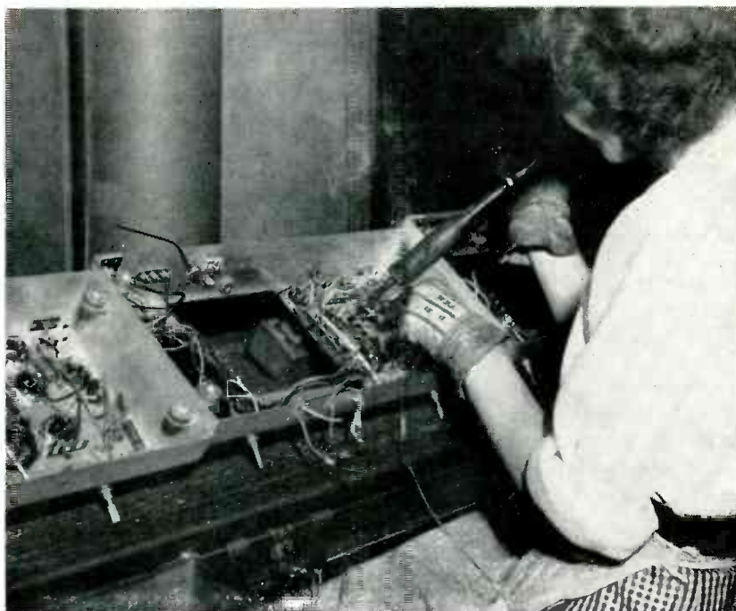
Avoiding assembly operations at soldering positions is one example of specialization that cuts costs
