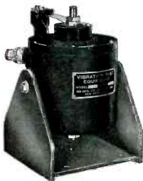
MODEL SA VIBRATION EXCITER Delivers 5 pounds force from 20 to 1,000 c.p.s., usable to 20,000 c.p.s.
