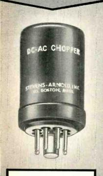
These Choppers convert low level DC into pulsating DC or AC so that 'serve-mechanism error voltages and the output of thermocouples and strain gauges, may be amplified by means of an AC rather then a DC amplifier.
