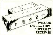
The CW-3 Superbet receiver is a 7 tube fixed-tuned aircraft frequency unit. Circuit comprises RF mixer-oscillator, IF 2nd Detector, BFO, Audio Output, BFO Limiter and 110 V Power Supply stages. Brand new with one set coils, 56-10 mcs. Less crystal. Contains 2-6K7, 6K8, 2-6C8G, 80 and 6SN7 tubes, Size: 3½" x 19" x 11½", Grey wrinkle finish. Elaborate instruction book included. Shpg. wt. 50 lbs. In original overseas crates. Brand new with 2 sets tubes, 1 set coils, and instruction book.
