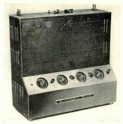
Decade direct-reading counter of four stages counting up to 10,000
