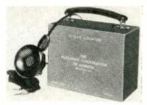
counter for prospectors. Two pounds in weight, the instrument may be clipped to the belt, allowing freedom of both hands. Clicks in an earphone and a flashing light indicate the presence of radioactive ore.
