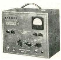
bines the functions of a scaling unit, a radiation survey meter, a countrate meter and a contamination detector. Some of its features are: continuous 24 hour per day stable operation without overheating; bi-(continued on p 200)
