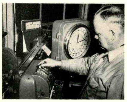
Operator sets up information to be printed, along with weight of cattle, by electronic live stock weighing instrument. Old beam-type scale may be seen in background.
