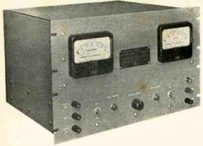
Right: MODEL PSR-102...200 to 1000 volts D.C. at 0 to 500 ma. 6.3 volts A.C. center-tapped at 10 amp; ½% or better regulation under any conditions of operation within ratings. 20 MV. or less peak-to-peak ripple voltage. Output impedance effectively zero. High voltage continuously variable from 0 to 1000 volts.
