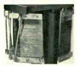
Unifitar ribbon windings on the 1,000-and 10,000-ohm decades on mica cards.
