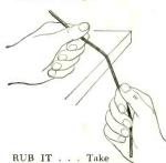
RUB IT . . . Take a length of BH "649". Hold the ends firmly. Then rub the sample up and down briskly in a sawing motion against the edge of a desk or chair. See how difficult it is to damage the coating.
