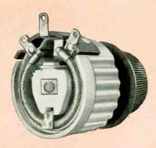
VARIABLE POWER requirements within 25 and 50 watt ratings are well handled by IRC Type PR Power Rheostats. All-metal corrugated construction gives maximum heat dissipation. PR Rheostats can be operated at full power in as little as 25% of rotation without appreciable temperature rise. Direct contact between housing and mounting panel increases ability to disperse heat. Bulletin E-2 details specifications; send for your copy.
