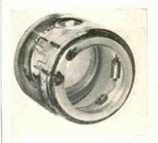
FIG. 1—British type CRI-143 infrared image converter
