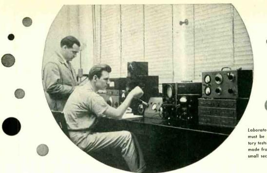
Laboratory Controlled — Every batch of CIP must be put through very extensive laboratory tests to keep quality high. Test cores are made from every batch at the lab. Above, a small section of the test equipment.
