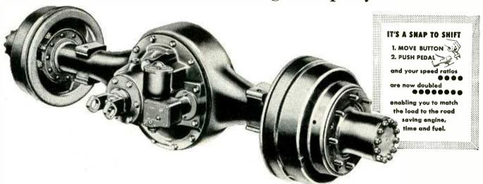
The popular Eaton 2-speed truck axle is controlled by a little button. The driver moves it and the truck's speed ratios are doubled in number. Crushing loads start with ease. Rough uphill hauls in quarries or in construction jobs are a cinch. And owners save wear, tear and money on their truck equipment!
