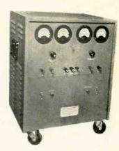
Above, right: MODEL PSR-105 ... 200 to 400 volts D.C. at 0 to 200 ma. from each of two separately controlled outputs, or 200 to 400 volts D.C. at 0 to 400 ma. 6.3 volts A.C. center-tapped at 10 amp; ½% or better regulation under any conditions of operation within ratings. 10 MV or less peak-to-peak ripple voltage. Output impedance effectively zero. Output voltages continuously variable. NET PRICE F.O.B. FACTORY......\$695.00
