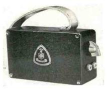
ard flashlight batteries power the unit through a vibrator power supply which furnishes the high voltage for the Geiger tube. Practically any magnetic type single or double phones having 1,000 to 24,000 ohms impedance can be used with the instrument. Further details may be found in bulletin E-5.
