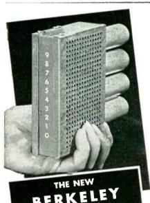
This unique packaged component is easily built into your apparatus. It has true decimal reading, and simple binary circuit with
