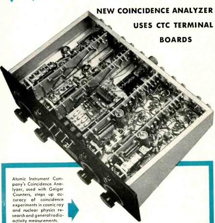
Teamwork between the engineering departments of Atomic Research Company and CTC licked a serious time problem in the manufacture of the Coincidence Analyzer. Atomic Research Company specified what they needed in terminal boards and CTC saw to it that they got what they wanted in a hurry. Five Terminal Boards made of laminated phenolic and equipped with standard CTC feedthrough and single-ended lugs comprise CTC's contribution to this excellent piece of equipment.
