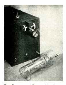
Traveling-wave oscilloscope tube, shown in foreground, is viewed through the 60-power microscope mounted on the side of the housing box for the tube
