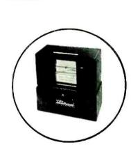
TelAutograph Corporation, New York, N. Y., designs and manufactures the TelAutograph telescriber, an instrument that transmits handwritten messages over wire to one or many remotely located receivers.
