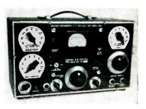
a multiplier range switch covering a total measuring range between 1 mv and 1,000 volts d-c, and a built-in 10-mv calibrator. Output varies between a few microamperes and 5 ma.
