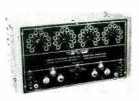
applications requiring up to 1,000 counts per second. It features the preselection of any number to be counted by setting the four decade knobs to the number desired. Automatic recycling is provided. Accuracy of the counter is unaffected by line voltage variations from 95 to 135 volts. A built-in relay provides both normally open and normally closed contacts capable of handling 5 amperes at 125 volts.
