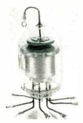
was designed especially for the aviation industry. Its maximum height, excluding leads, is 6 inches, and maximum diameter,  $2 \pm i$  inches. Filament voltage is 14 v and filament current,  $2.4 \pm 0.4$  amperes. Heating time is 180 sec and deionization time,  $200 \ \mu$  sec. Minimum ambient temperature is  $-54 \ C$  and maximum,  $+100 \ C$ .
