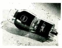
put at relatively low plate and screen voltages in applications requiring long life and reliability. The power amplifier pentode has beam characteristics and has plate dissipation of 12.5 watts with plate voltage at 200 volts. Heater voltage is 25 volts at 0.3 ampere.
