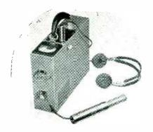
for semi-quantitative work and highly sensitive to beta and gamma-ray radiation, uses a 1B85 thyrode and two 5828 medium-mu triodes. Full scale sensitivity on three ranges is 130, 1,300 and 13,000 counts per sec. A microammeter calibrated in milliroentgens per hour, measures the average intensity of the radiation.
