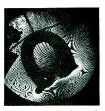
Electrons passing through magnetic field of small horseshoe magnet (about one-fourth inch wide) produced this distortion of the electron shadow of a fine wire mesh in an electron microscope
