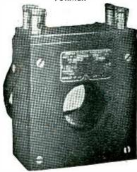
Weston Model 461 Type 4 (see .llustration). This unit can be used with any precision 5 Amperes A.C. Meter to extend the ranges of the meter to 50, 100, 200, 250, 500 or 1800 Amperes A.C. Accuracy within 3, of 17; Normal Secondary Capacity = 15 Va; Binding Posts for 10 Amperes tap; Inserted primary for 100, 200, 250, 500 and 1 1000 Amperes; Insulated for use up to 2500 volvs. List Price \$98.00. NET fob. N Y \$35.00
