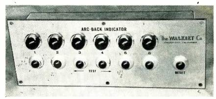
Panel lamps and test switches are on the indicating unit
