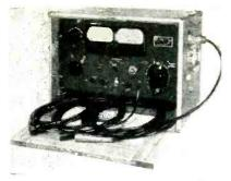
rectly on a megchmmeter scale or may be calculated in ranges from 0.3 to 20,000 megchms from the readings of a voltmeter and microammeter. The unit operates from a 115-volt, 60-cycle line and consumes a maximum of 65 watts.
