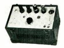
equally suitable for portable applications. A flat response from 40 to 40,000 cps, a dynamic range in excess of 60 db, and a calibrated gain control in 5-db steps from 0 to 50 db, give a calibrated amplification into a low output impedance.
