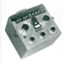
decade steps. The unit can measure resistance from 1 milliohm to 1 megohm; capacitance, from 1  $\mu\mu$ f to 100  $\mu$ f; and inductance, from 1  $\mu$ henry to 100 henrys.
