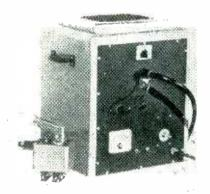
Completely cured permanent bonds are produced within a few seconds. The hand gun can be fitted with electrodes for veneering, banding, mitered corners of all angles and penetration, making it adaptable to a wide variety of jobs.
