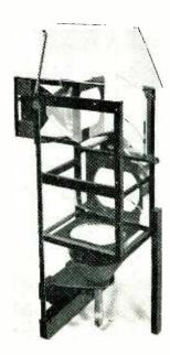
Arrangement of three 10-inch picture tubes with dichroic mirrors to produce direct-view image in RCA system. Mirrors reflect light of one primary color, pass other two
