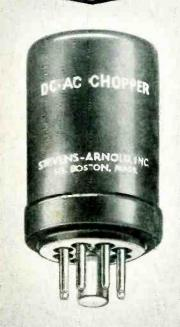
These Choppers convert low level DC into pulsating DC or AC so that servo-mechanism error voltages and the output of thermocouples and strain gauges, may be amplified by means of an AC rather than a DC amplifier.
