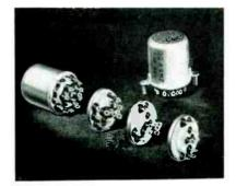
metal containers 14 in. in diameter,  $1\frac{1}{2}$  in. long and weighing only 3 ounces. Palladium contacts are nominally rated at 28 v d-c noninductive on permanent installations. For guided missile applications the contact rating may be increased to 12 amperes noninductive if the required number of relay operations does not exceed 50 to 100. Time of operation is less than 0.005 sec.
