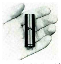
screw located outside the sealed space. This screw permits the timing to be changed over a 5 to 1 range. The miniature size,  $\frac{3}{4}$  in. in diameter and  $2\frac{3}{5}$  in. seated height, fits a 7-pin miniature tube socket. Contacts are single pole, rated at 6 amperes. Relays are available for any energizing voltage up to 125 and operate interchangeably on a-c and d-c.
