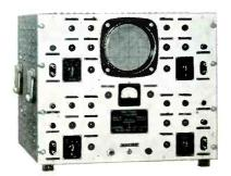
H-43 Four-channel oscilloscope for strip film recording.
