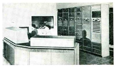
Entire populace can be warned from central control station which can broadcast both alert signals and verbal instructions during and after an attack
