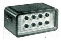
contained 24-volt a-c supply and switch for remote relay control of main amplifying equipment. Output, measured at 100, 400 and 5,000 cps is 300 mw, 2 percent at 600 ohms. Frequency response is  $\pm 1$ db, 40 to 20,000 cps.
