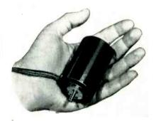
polyphase induction motor. Typical ratings for continuous duty are 1/100 h-p at 7,000 rpm on 400-cycle current or 1/300 h-p at 3,000 rpm on 60-cycle current. The type is especially suited to needs calling for high speeds and plenty of power.
