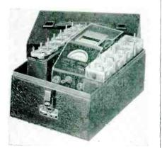
quency range to cover the entire spectrum from 200 kc to 300 mc. Included with the meter is also a remote probe for coupling into extremely small and normally inaccessible places.
