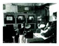
at Lime Grove studio, Control room Shepherd's Bush. Screen at bottom right shows picture being transmitted from Lime Grove. Upper screen shows cricket score being transmitted from Alexandra Palace
