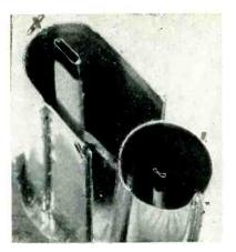
Demounted internal structure of plasmatron. Auxiliary cathode is inside cylinder, and oval-shaped main cathode is inside U-shaped anode. Electrode sizes are not critical, and tube works just as well in miniature sizes as in proportions for handling amperes of plate current. Available main cathode emis-
