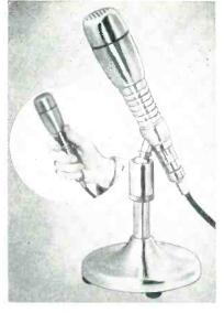
or boom use, it is quickly detachable for hand use. It is omnidirectional and available in 15,200 ohm or high impedance. Sensitivity is 56 db below 1 volt per dyne per sq cm.
