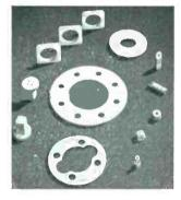
Teflon's loss factor is less than 0.0005; its dielectric constant only 2.0—at all frequencies measured to date. Teflon is serviceable throughout the entire temperature range of —110° F. to 575° F. with negligible change in critical electrical characteristics. Teflon is tough, somewhat resilient, weather-proof, has zero water absorption and is absolutely non-corroding.
