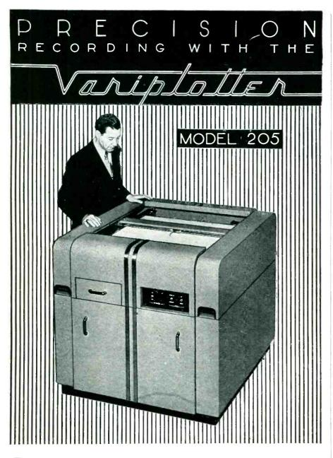
The Model 205 Variplotter, highlighting accuracy, speed, and versatility, brings to industry and laboratory a new tool with a wide field of application. This instrument will present on a 30-inch square plotting surface a precise graphic representation of one variable as a function of another variable, requiring only that the variables be expressed by d-c voltages.
