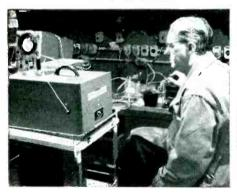
**CAPACITOR PEAK VOLTAGE** in a jetengine-ignition system is measured by a General Electric electrostatic voltmeter. It can measure peak voltages of critical ignition circuits without disturbing the ignition system itself.
