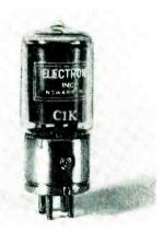
peak anode current, 8 amperes; maximum peak inverse voltage, 1,250 v; maximum peak forward voltage, 1,000 v. Grid shielding results in a grid-anode capacitance of only 1  $\mu\mu f$  with a grid-cathode capacitance of 10  $\mu\mu f$ . Critical grid current is less than 5  $\mu a$ .
