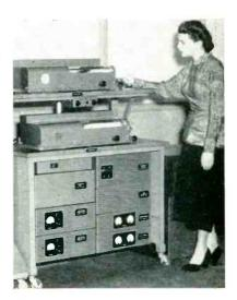
FIG. 1-Transmitting cylinders of the new facsimile system. Lower cylinder is loaded and copy is being transmitted while operator prepares upper cylinder for automatic take-over
