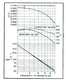
FIG. 7-Curves showing the extent of correction required for transformers with moderate distributed capacitance in the primary
