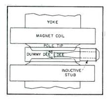
FIG. 1—Side view of the dee and cavity of the cyclotron
