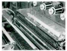
**MAXIMUM COIL DENSITY** An entirely new type of delivery shelf is used to insure coils of extreme accuracy and high density. It imparts a uniform backward pull to the paper as it is fed into the coil.
