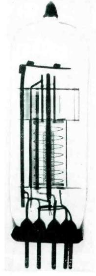
X-ray photograph of ECL 80. The screen grid, which does not reach right to the top, has been distorted in manufacture
