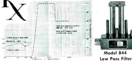
• Suppression of low-order harmonics in transmitters operating below 400 mc is the prime function of Model 844 Low Pass Filter. 40 db or more attenuation of 2nd to 5th harmonics of transmitters operating between 225-400 mc is afforded. Insertion loss and VSWR are very low thruout the pass band. Teflon insulation and rugged construction thruout assures reliability.
