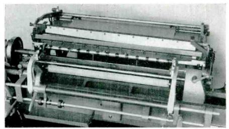
**EASY MANUAL OPERATIONS** Photo shows coil arbor in position for quick transfer. Wire turn counter can be reset quickly. No cam transfers are required when changing wire layer length, wire spools are easily changed.
