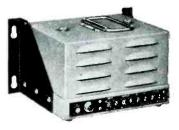
Model 1411 INDUCTRONIC D-C AMPLI-FIER—stable amplifier provides high degree of resolution even at fractional loads. Reaches steady full scale deflection in fraction of a second. Interchangeable plug-in range standards for either microamperes or millivolts.
