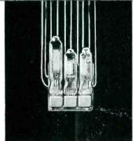
New Model 3 Ampec - a sub miniature 3 stage speech am-plifier ... dimensions: 1-1/32" x 15/16" x 11/32". Check coupon for Technical Bulletin 42-130.
