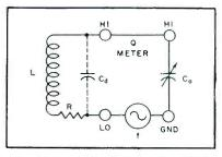
FIG. 9-Basic Q-meter circuit with the primary inductance of a transformer and its distributed capacitance connected to inductor terminals. Secondary not shown
