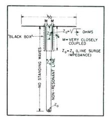
transformation—the  $\lambda/4$  section becoming a matching transformer  $(Z = \sqrt{Z_1 Z_2})$  and realizing Z in the equation by summation since the impedance rises and falls in opposite directions in the two stubs.
