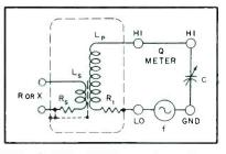
FIG. 8—Basic Q-meter circuit with a transformer connected to the inductor terminals. Electrostatic shield and dotted connections optional
