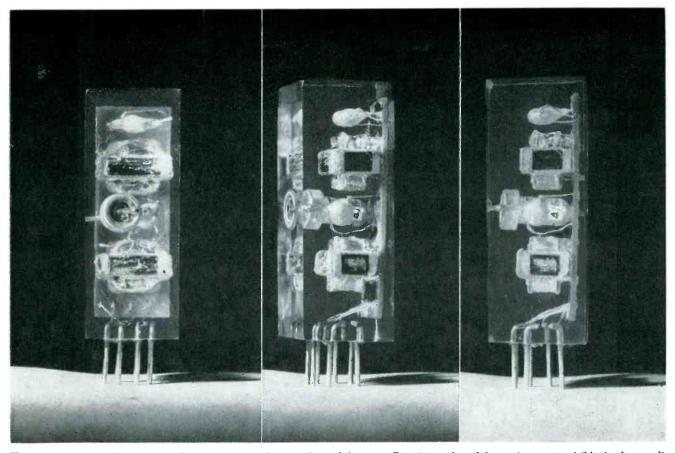
Three views of the transistor amplifier shown in photograph on left page. Experimental model transistors are visible in the amplifier as white plastic-covered beads. Transformers and other components are also visible. Unit will operate continuously for months with one penlight cell as sole power source
