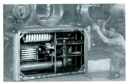
Oscillator dolly with attached dee partially removed. Type 9C21 oscillator tube at right, grid leak, metering circuits and ceramic water coil at left
