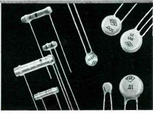
Ceramic Disc Hi-Kap Capacitors have very high capacity in extremely small size. Bulletin No. 42-4R. TC Tubulars (Temperature Compensating) — TCZ units show no capacity change over wide range of temperature; TCN's vary capacitance according to temperature. Bulletin No. 42-18. BC (Bypass Coupling) Tubulars . . . well suited to general circuit use. Bulletin No. 42-3.
