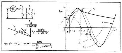
FIG. 5-Simplified video detector with diode resistance
