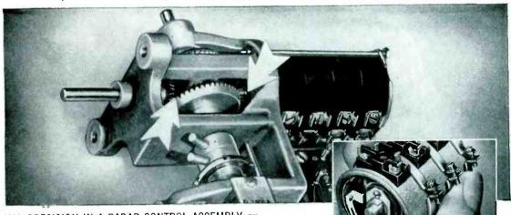
CRUCIAL PRECISION IN A RADAR CONTROL ASSEMBLY The gears on this radar control assembly were precision cut to eliminate backlash and binding, but the care that went into their manufacture could have been completely nullified if the potentiometer coupled to them was not mechanically precise. In this case, overall accuracy is assured by using a Fairchild precision unit.
