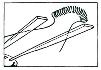
**IMPROVED JOINT.** To prevent dial lamps from being "noisy", General Electric developed a better joint—one with tungsten filament legs pressed firmly into the softer metal of the lead-in wire. It's another reason why G-E dial lamps insure customer satisfaction!
