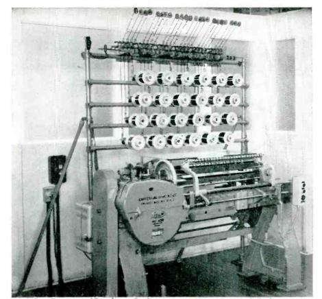
25 INSERTS A MINUTE Single or laminated insulating sheets, either paper or aretate, are fed into the Leesona No. 107 Coil Winder at rates as high as 25 per minute. Thus, on a coil containing 100 wire turns per layer, the machine can be run at speeds as high as 2500 rpm.
