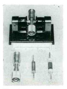
FIG. 1—The magnetic attenuator, a new, inexpensive type of microwave attenuator that requires no movable components, mechanical controls, or slotted sections in the waveguide or coaxial transmission line
