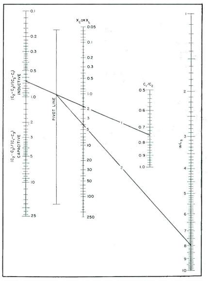
FIG. 4—Nomograph for reactance X in Eq. 17 and 18. If  $C_1$  equals 150  $\mu\mu f$ ,  $C_2$  equals 200  $\mu\mu f$ ,  $C_3$  equals 180  $\mu\mu f$  and  $\omega L$ , equals 8 ohms, then  $X_L$  equals 4 ohms
