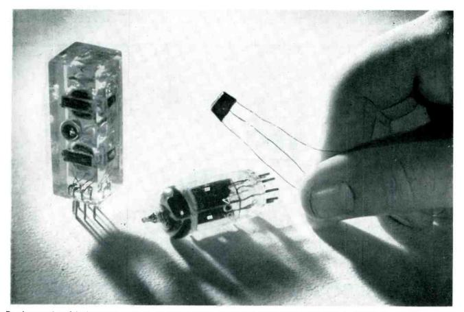
Developmental model of junction transistor illustrated (black object with three leads being held) as compared to a 6C4 miniature triode and an experimental model of a two-stage transistor amplifier imbedded in clear plastic. The amplifier has a power gain of 90 db in the audio range
