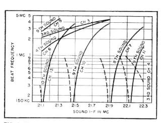
FIG. 8—Beat frequency versus sound i.f. Dotted lines in this and Fig. 9 and 10 indicate harmonic below video carrier
