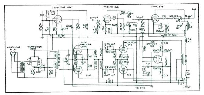
FIG. 2-Transmitter circuit is straightforward with exception of high audio frequency pre-emphasis and delayed agc circuit
