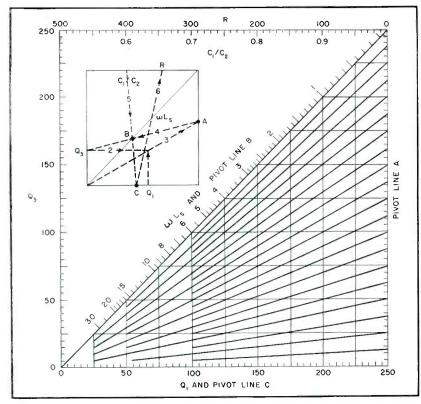
FIG. 3—Nomograph for resistance R in Eq. 10. If  $Q_1$  equals 200  $Q_3$  equals 100,  $C_1/C_2$  equals 0.75 and  $\omega L$ , equals 40 ohms, then R equals 2,000
