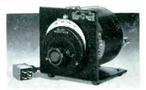
This unit os-Type 1208-A V-H-F Oscillator cillator is similar to the Type 1209-A in construction and operation. The tuning circuit employs a sliding contact which makes possible a wider frequency range of 65 to 500 Mc. The frequency calibration is accurate to  $\pm 2\%$ . Into 50 ohms the output power is 100 mw at any frequency and 500 mw in the center of the range.
