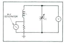
FIG. 1—Basic circuit of Q-meter method for measuring inductance
