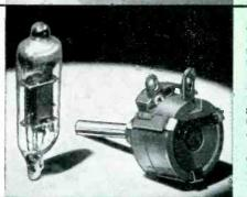
This precision potentiometer has a tapered winding held to plus/ minus 11/2% linearity as measured at 10 test points. Mechanical tolerances held to plus/minus 0.00025". Unit operates dependably over extreme ranges of temperature, humidity, altitude or barometric pressure, and severe vibration. Obviously built to a quality standard rather than to a price.
