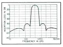
FIG. 4—Frequency response of bandpass filter
