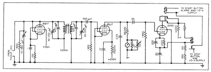
FIG. 6-Receiver section for one model RCA metal detector
