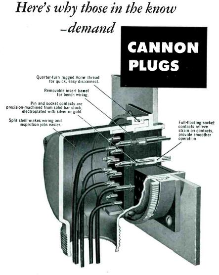
Recognition of Cannon's 36 years of sound engineering and fine, uncompromising construction has built the demand for Cannon Plugs. Here we take an inside look at the lightweight Type "K" 90° connector, forerunner of the Army-Navy Series. More features of the "K" were incorporated into the "AN" design than any other connector.
