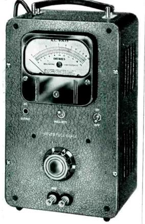
• Available precision shunt resistors permit the measurement of AC currents from 1 ampere down to one-tenth of a microampere.
