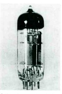
Combined pentode and triode for tv reception, tube type ECL 80, is shown in x-ray silhouette in the accompanying photograph
