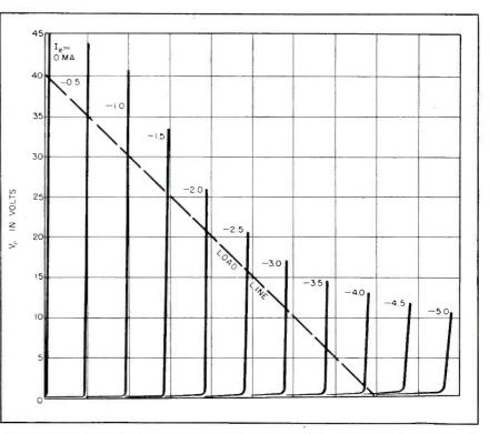
FIG. 2-Static collector voltage and current characteristics of the junction transistor. Note general similarity to the plate family of a beam tetrode
