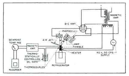
FIG. 1-Photoelectrically controlled dew-point hygrometer
