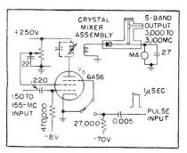
FIG. 3—Pulse-modulated r-f doubler and output stage
