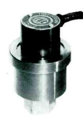
The Consolidated 9-102 Torsiograph accurately measures frequency and amplitude over a vibration range of 10 to 1000 cyclesper-second.
