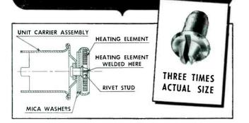
Small enough to put under your fingernail, this rivet is made by Progressive for The Cuno Engineering Corporation. Used in an automotive cigarette lighter, it serves as a post to which the center of the heating coil is spot welded and as a rivet for fastening the burner cup to the lighter shell.
