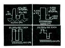
Examples of trains of pulses produced by stimulator, as recorded with dualbeam oscillograph to get timing wave with the relatively wider pulses and intervals. The diodes permit a more rapid recovery of the grid voltage after the pulse. Switching in the extra capacitor in the phantastron circuit permits extending its pulse duration to  $100,000 \ \mu sec$ .
