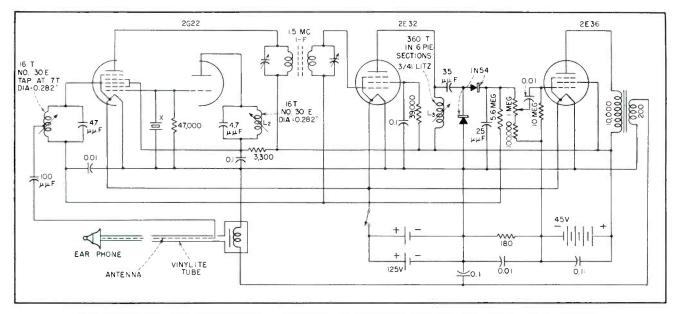
FIG. 1-Receiver uses crystal control to give single control (audio gain) operation with complete reliability
