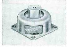
These new Barrymounts provide the aircraft and electronic engineer with a vibration isolator designed to meet the unusual temperature and environmental conditions encountered in high-altitude, high-speed flight. Employing no organic materials, these mountings are not subject to temperature influences that may affect the performance of other mountings.
