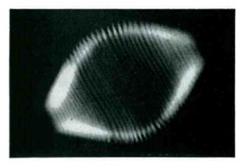
**OLD FILAMENT.** High notes often cause the filaments and lead-in wires of radio dial lamps to vibrate. In old-style lamps, they vibrate to frequencies different from those of the noise. This produces a whipping action (above) which eventually tears the filament apart.
