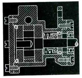
NEW WAY Just 2 Truarc Rings, set into accurately predetermined grooves, bring new simplicity of design... speedy assembly. No skilled-tabor required! No maintenancet Rings lock parts accurately for life of unit.
