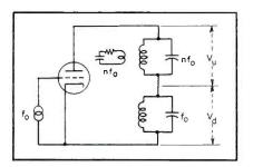
FIG. 7—Plate-line resonances owing to harmonic components
