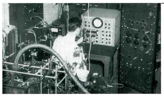
Research laboratory at New York University, showing dual-pulse electronic stimulator in rack at right. Constant-temperature salt bath containing muscle being stimulated is barely showing at lower left. Rack back of it contains various amplifiers and oscillators used with dual-beam oscillograph in center for recording mechanical and electrical responses of the muscle
