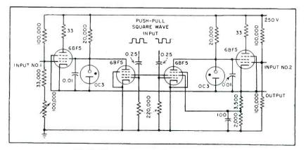
FIG. 1-Electronic switch for video frequencies
