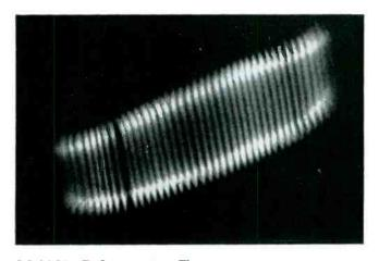
**NEW FILAMENT.** By redesigning the filament supports of G-E radio dial lamps, General Electric engineers matched the frequencies and greatly reduced the effects of vibration (above). As a result, G-E radio dial lamps give longer, more dependable service.
