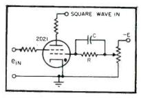
FIG. 2—Thyratron circuit with R-C compensation network
