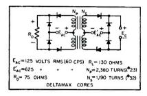
FIG. 1—Circuit diagram of parallel-connected magnetic amplifier
