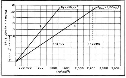
FIG. 3—Determination of  $L_0$  and effective  $C_D$  is possible from curve A. Desired capacitance change is obtained by using curve B in addition
