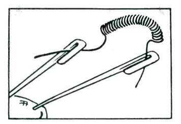
**OLD-TYPE JOINT.** Some types of dial lamps actually cause "static". Old-type clamp joints in the bulb (above) often permit changes in resistance or tiny arcs that cause the lamp to radiate bothersome interference.
