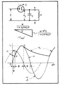
FIG. 4—Simplified video detector neglecting diode resistance
