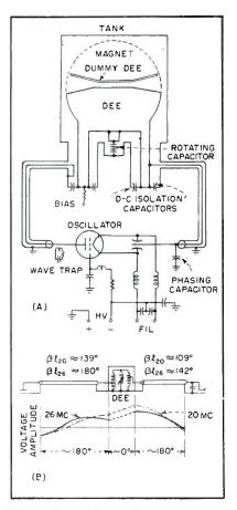
FIG. 6—Schematic circuit of the oscillator (A) showing connection to the dee, and qualitative phase and amplitude behavior of the circuit (B)
