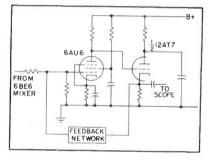
FIG. 8-Selective amplifier circuit
