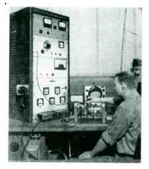
Receiver test setup
