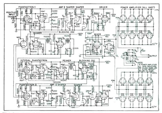
FIG. 3—Circuit of pulse generator and synchronizer. Power amplifier requires 117-volt d-c power line, and all other stages operate from a common 300-volt regulated power supply
