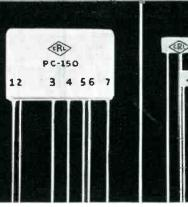
50% less soldered connections with Centralab's Audet . . . furnishes all values of all components generally found in the output stage of AC-DC radio receivers. Technical Bulletin 42-129.
