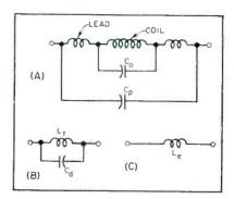
FIG. 2—Simplifying equivalents used in calculation of distributed capacitance
