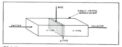
FIG. 1—Diagram of the junction transistor. A thin section of p-type germanium is formed as part of a single crystal, in intimate contact with two larger blocks of n-type material
