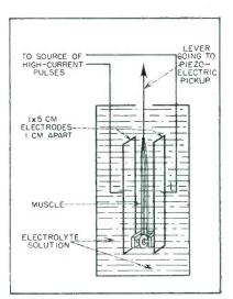
FIG. 1—Method of electrically stimulating a muscle with so-called massive electrodes connected to output of highcurrent electronic pulse generator. Muscle is clamped at its lower end, and upper end is connected through a lever to a piezoelectric pickup. Muscle (of frog) can live for many hours in the salt solution serving here as electrolyte
