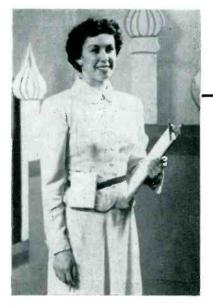
Superheterodyne receivers may be carried in pocket or worn around waist on a belt. Sound is piped from electromechanical transducer in set to ear by thin vinylite tube which also contains antenna
