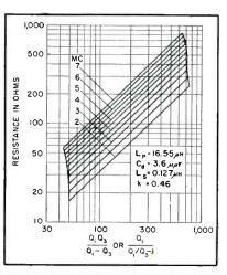
FIG. 5-Sample chart used to determine resistance of individual transformers
