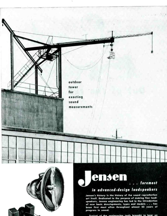
Typical of the engineering tools brought to bear on loudspeaker research, is Jensen's outdoor tower . . . high in the air, away from reflecting surfaces . . . used for precise measurements of acoustic performance,
