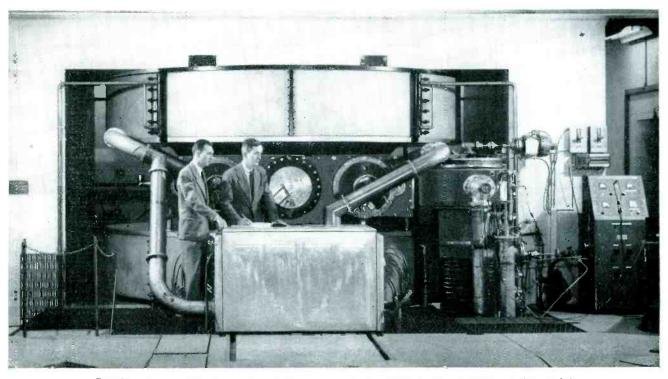
Complete r-f setup with dee in place between magnet poles. Cathode line at right and plate at left
