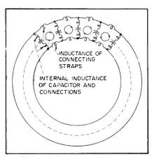
FIG. 8-Capacitor ring resonances
