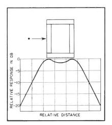
FIG. 3—Relative-amplitude response of quadrant coil system
