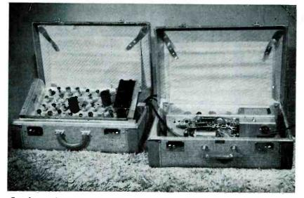
Complete rack-panel equipment in carrying case (left) with associated regulated power supply operating from 117-v outlet (at right)
