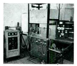
Trolley exhaust for sealing-off standard diodes.
