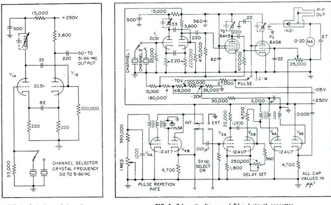
FIG. 1-Cathode-coupled oscillator
