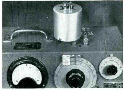
Two to seven-megacycle transformer plugged into the Q-meter inductor terminals
