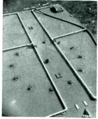
On the reinforced roof of the transmitter coach, a choice of mounts is provided for proper parasitic whips for the f-m audio transmitting system of Signal Corps mobile television caravan
