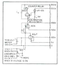
FIG. 2—Spark outage integrator instrument for recording outage time resulting from sparks in d-c high voltage sytems
