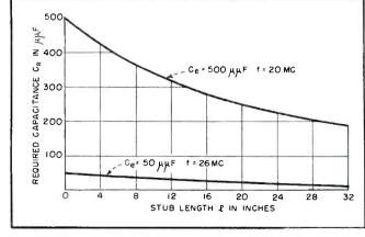
FIG. 4—Stub length versus required terminal capacitance for a representative cyclotron oscillator
