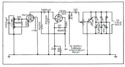
FIG. 7-Oscillator section of the RCA detector
