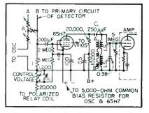
FIG. 5—Automatic drift compensation circuit
