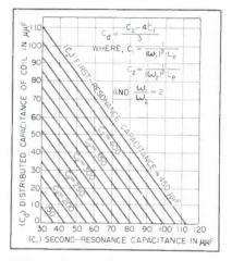
FIG. 3-Distributed capacitance curves
