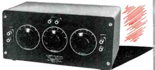
This equipment is particularly applicable to extremely accurate measurements from D.C. to 200 kc. and can be used up to the lower radio frequencies. The Decade type switches make the box convenient to use. In addition, there are switch stops which prevent return from full to zero attenuation when making adjustments. A total of 110 Db. is available in 1.0 Db. steps, or 111 Db. is available in 0.1 Db. steps. Both of these types may be obtained in either a balanced H or an unbalanced T network.
