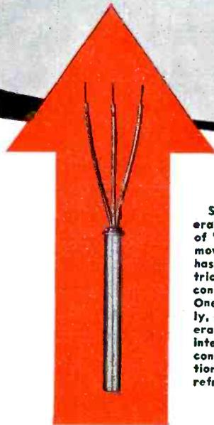
Servel's latest model refrigerator retains all the features of "silent" operation, using no moving parts; but the gas flame has been replaced by an electric heating unit of Nichrome containing two resistance wires. One of these operates constantly, and maintains normal refrigeration; the other operates intermittently, by thermostatic control, and supplies the additional heat required when extra refrigeration is necessary.
