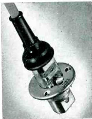
The Cannon UA Series consists of 2 plug types and 5 receptacles, all having 3 gold-plated contacts for 15 amp service. Socket contacts are full-floating. The "G" contact engages first, breaks last for "no noise" grounding or shielding purposes.
