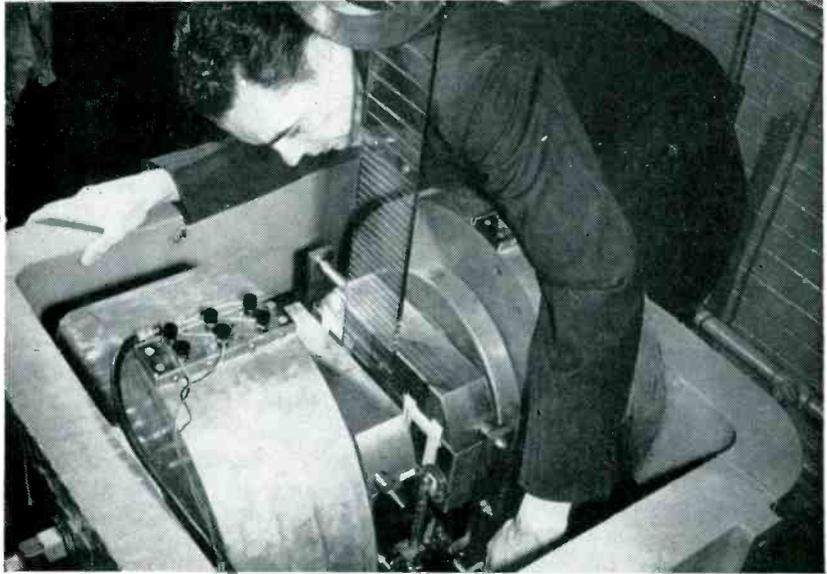
The nuclear resonance probe being used to measure the field distribution of a magnet. The probe, at lower center, is mounted on a crossfeed for accurate positioning in the magnet gap
