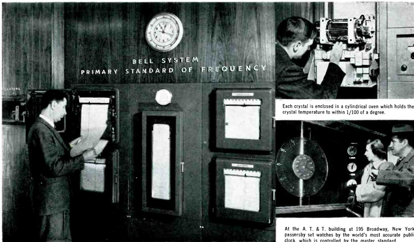
Each crystal is enclosed in a cylindrical oven which holds the crystal temperature to within 1/100 of a degree.
