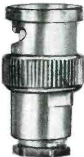
The BNC Connectors shown are small, lightweight Connectors designed for use with small cables such as RG-58/u, RG-59/u and RG-71/u. Widely used for video and aircraft test equipment, they are recommended for frequencies as high as 3000 M.C., where impedance matching is important. The BNC series is used successfully in the region of microwave frequencies.
