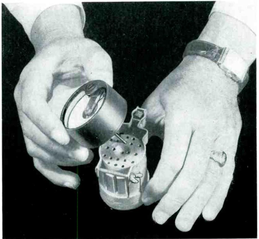
FIG. 2—Plug and flux meter setup used to make field measurements on ion traps and centering units
