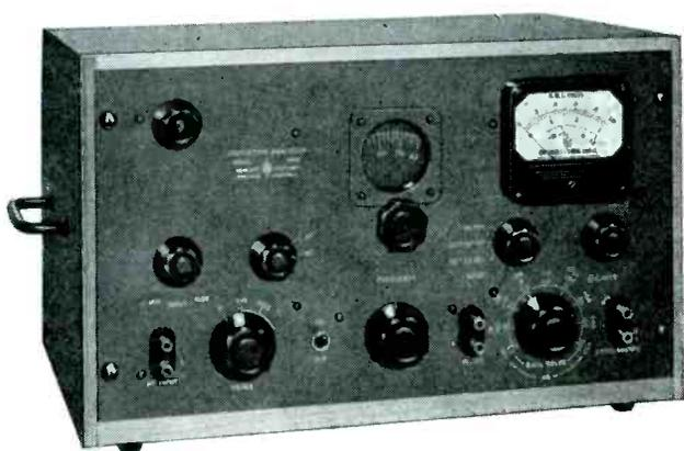
**-hp- 330B DISTORTION ANALYZER** (left) is an unusually versatile instrument offering fast, accurate measurement of distortion values as low as 0.1% at any frequency between 20 cps and 20 kc. The equipment also quickly determines voltage level and power output, measures amplifier gain and response, measures audio noise and hum (direct readings), determines unknown audio frequencies and serves as a high-gain, wide-band, stabilized amplifier.
