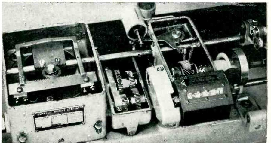
**READILY-ADJUSTABLE TRAVERSE MECHANISM** permits winding any length of coil from 1/16 in. to 2 13/16 in. without changing cams. A single setting applies to all the winding heads.
