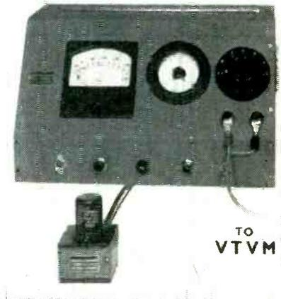
Test setup used at The Liquidmeter Corp. for high-speed checking of all electrical characteristics of a bridge transformer that is plugged into box in foreground
