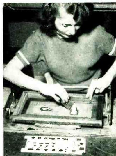
Forcing ink through stencil onto flat chassis like that in foreground; wood lever arrangement lifts screen straight up when job is done, to prevent smearing of letters
