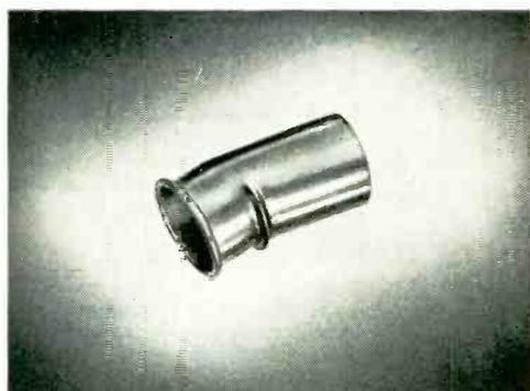
**The Finished Part.** Final stage in the fabrication of the part, shown above at three stages of production, is a bend nicely controlled for both precise angle and freedom from other, unwanted distortion.
