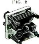
9-62 mmfd per section, 6-34 mmfd sections in series. Double ceramic end plates and bearings. 1/4" diam. shaft, 5/16" long. .065 Plate spacing end plates 1-3/8" square.
