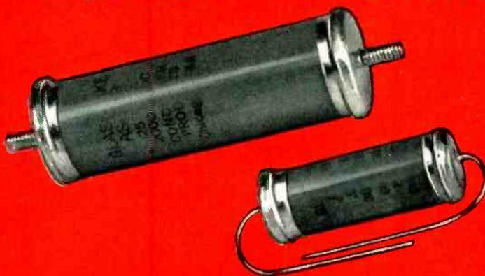
Glassmike capacitors are wound with the plastic film which accentuates the electrical characteristics you require, and results in capacitor design of minimum size. The metal ferrules, soldered to silver bands at each end of the hermetically-sealed glass tubes, eliminate mounting problems.
