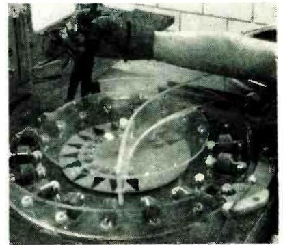
Removing shorted capacitor with fuse tongs. Transparent Lucite fences and circular cover minimize chances of shock while permitting quick removal of shorted units. Neon lamp lights to indicate which unit is shorted
