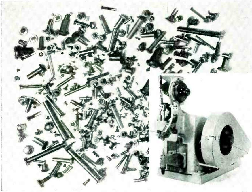
Tubular and bifurcated rivets from 1/16" to 2 1/4" long are assembled by special automatic machines
