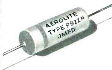
Series P92ZN Aerolene-impregnated metallized-paper capacitors are modified plastic-tubular duranite-end-sealed units in paper cases. Operating temperatures of  $-30^{\circ}\text{C}$ . to  $+100^{\circ}\text{C}$ . 200, 400 and 600 V. D. C. 0.01 to 2.0 mfd.
