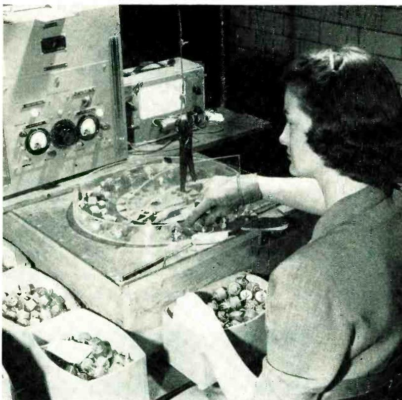
Setup for production testing of high-voltage ceramic capacitors. Turntable is driven by standard rotary actuator. Spring-loaded cam in foreground insures precise positioning over contacts underneath after each movement of table
