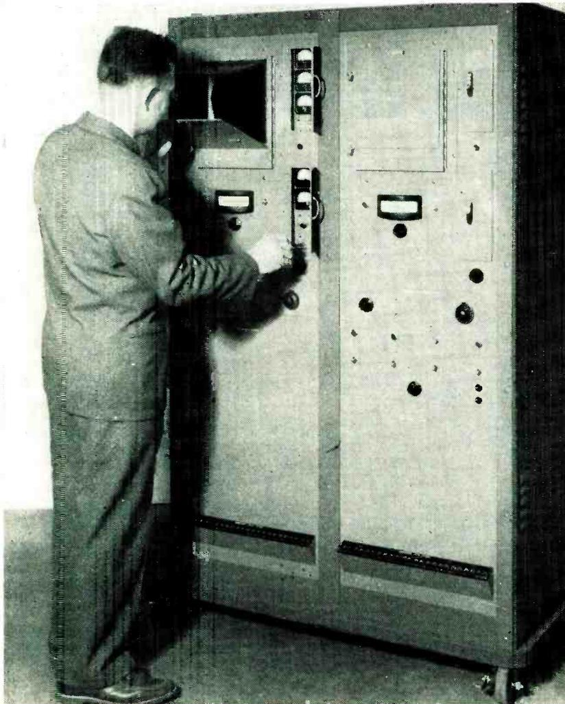
Complete instrument contains two function generators. Specimen sheet is placed behind hinged door and crt spot focused by viewing on ground glass in folding hood
