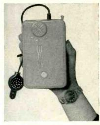
On the market in West Germany is this 13/8 by 43/8 by 6 11/16-inch unit selling for 680 deutschmarks (\$162). It runs on four internal dry batteries (two in parallel power a 9-volt motor) and holds enough 0.05-millimeter wire to operate continuously for 150 minutes at 30 centimeters per second
