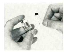
NEW JUNCTION TRANSISTORS, still experimental, also use germanium but have no point contacts. Current is amplified as it flows through germanium "sandwich"—an electron-poor layer of the metal between two electron-rich ends. This new transistor runs on as little as one-millionth of the power of small vacuum tubes.
