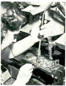
FAST SOLDERING for production-line work is possible with this iron. Calrod\* heater gives plenty of heat to ensure uniformly-strong soldered joints.
