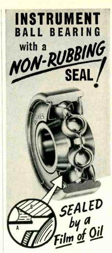
In the new RMB FILMOSEAL bearing, a capillary film of oil forms between cylindrical washer (A) and the tapered O.D. of inner race (B). This strong film of oil seals the bearing — keeps the lubricant in, keeps dirt out — yet there is no rubbing contact between the sealing elements.
