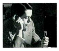
MOIST PAPER AND COIN generate enough current to drive audio oscillator using junction transistors. Half as big as a penny matchbox, an experimental two-stage transistor amplifier does the work of miniature-tube amplifiers ten times larger.
