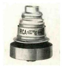
filtering for tv receivers. Style 412 is rated at 20 kv and style 414 at 10 kv. The case insulation is of low-loss, molded thermosetting plastic. Ring convolutions are molded into the surface of the 20-kv capacitor to prevent surface leakages that are caused by ordinary handling and a consequent deposit of conductive materials. The convoluted design increases the effective surface creepage path by more than 14 percent.
