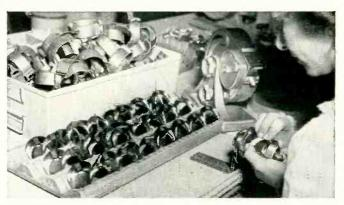
**3 TAPE HOLDS** coils together during assembly on simulated television tube neck.
