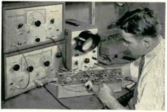
FACTORY TEST ALIGNMENT. Only 2 cables are connected to receiver during alignment. When receiver oscillators are lined up with the G-E crystal-controlled marker generator, the local station signal will fall where it belongs. The General Electric variable permeability sweep provides long-term extremely stable operation.
