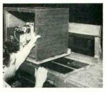
Small section of bench is pivoted and cut out in cabinet tip-up arrangement used by Emerson
