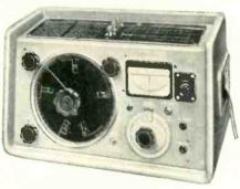
RESISTANCE, CAPACI-TANCE, INDUCTANCE and power factor are measured quickly and accurately on this Marconi engineered instrument.
