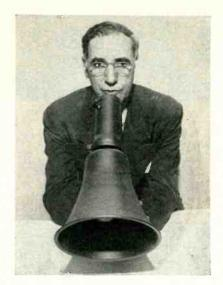
Experimental megaphone developed by General Electric is completely selfcontained, with transistors and small batteries located in unit near mouthpiece
