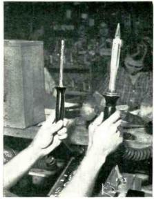
**THIN SHANK**  $(\frac{5}{16}$ -inch diameter) gives ready access to close-quarter joints. Lighter weight  $(3\frac{1}{2})$  ounces) causes less operator fatigue than with regular irons.
