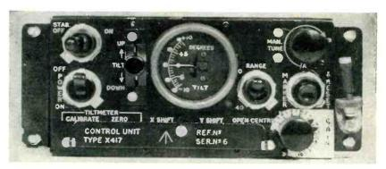
FIG. 2—Control unit of the lightweight airborne radar used in tests. The tilt of the antenna is shown by the small meter at the center
