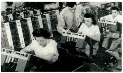
Method of using chassis cradles in aisles between benches for assembly of scalers and counting rate meters
