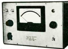
Far more versatile than conventional types, the C.G.S. peak pulse voltmeter reads rapidly and accurately on pulse widths of .25 microseconds and at repetition rates of 10 pps. The instrument reads on either positive or negative pulses. Controls include an on-off, range selector and input polarity switch; zero set control. A switch which throws a D.C. restorer into the circuit provides accurate peak to peak measurements of sine and square waves.
