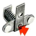
REPLACING A RIVET . . . Rollpin serves as guide shaft for spring-loaded electrical interlock contacts. The Square D Company reports that rivet failure previously occurred at the clinched end under normal operating impact and vibration.
