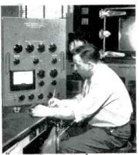
Q meter measurements on low frequency coils
