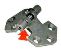
REPLACING A HEADED PIN . . . In this hinge pin application, Rollpin is simply and inexpensively driven in place, greatly reducing assembly costs. Constant spring tension holds Rollpin firmly in place . . . eliminates loosening of hinge due to wear.
