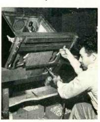
Installing chassis mounting bolts through cutouts in pallet on Emerson production line
