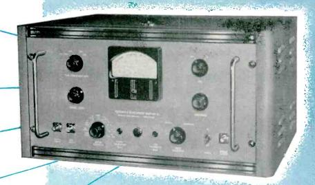
Type 275 Amplifier is a high gain linear audio amplifier designed to accurately indicate voltage standing wave ratios. The application of expansion circuit techniques provides a full scale deflection of 1:1.3. This means greater accuracy for low VSWR measurements.
