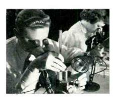
ASSEMBLY PROBLEMS, such as fixing hairthin wires to barely visible germanium wafers, have been solved through new tools and mechanized techniques. Finished transistors withstand great vibration and shock. Engineers see many opportunities for these rugged devices in national defense.
