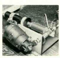
Soldering housing to base. Solder is fed automatically to joint through copper tubing that serves as guide. Entire operation takes only about 5 seconds
