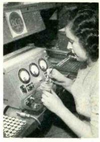
Bending grid support with tweezers to equalize interelectrode capacitances of 6J6 triode sections as measured by dual capacitance bridge. Before each test, tube structure is held in pipe at left and lint or dirt is blown out by air blast from copper tubing, controlled by footoperated valve
