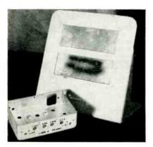
Two brass stencils and holding fixture for applying lettering to front and rear of a small r-f oscillator chassis. Guides behind fixture serve to position and hold units at a time for spraying, doubling speed of operation
