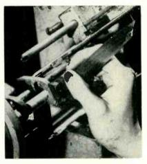
Applying blue-dyed paste with ordinary sponge-tipped envelope sealer to anchor end of metallized paper and at same time identify outer-foil end of roll
