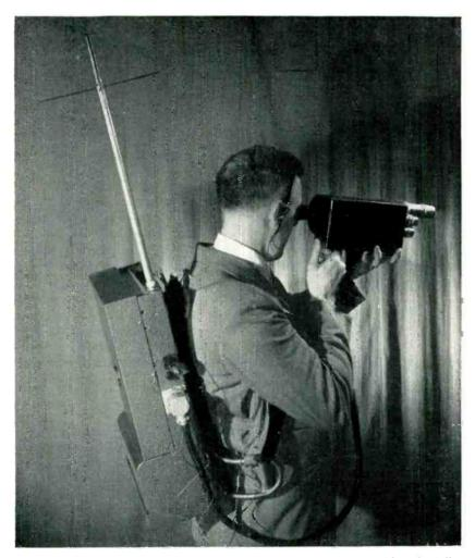
Pack set weighs 45 lb with batteries and dynamotor, and camera adds only 8 lb more. Headphones are used to receive radioed instructions from control station.
