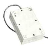
Accelerometer (half size)
