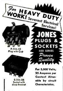
Socket contacts phosphor bronze, knife-switch type, cadmium plated. Plug contacts hard brass, cadmium plated. 2, 4, 6, 8, 10, and 12 contacts. Plugs and sockets polarized. Long leakage path from terminal, and terminal to ground. Caps and brackets, steel parkerized (rust-proofed). Plug and socket blacks interchangeable in caps and brackets. Terminal connections most accessible. Cap insulated with canvas bakelite.
