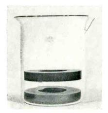
Two magnets of Ferroxdure as used in loudspeaker circuits magnetized in the direction of the axis
