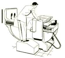
Keleket "C" Supertilt Table in vertical position. MICRO unit shown is one of eight which perform key functions in table operation.
