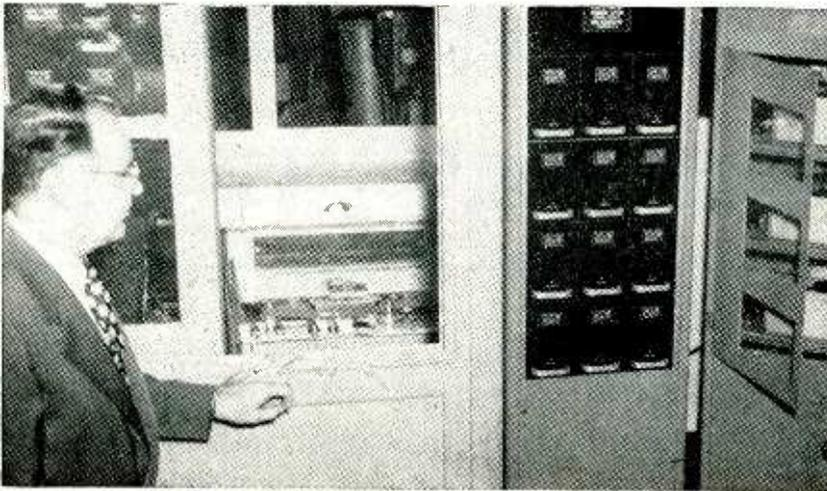
Vibration recorder shelter. From left to right, major components are: record modulator-amplifier; magnetic-tape recorder; playback demodulator-amplifier; and strip-chart recorder
