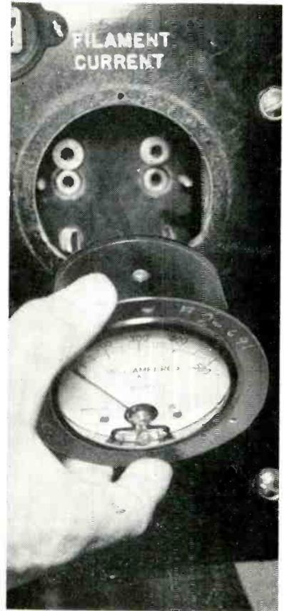
Plugging meter into test set
