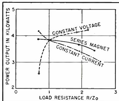
FIG. 7—Effect on output power of varying pure resistance loads
