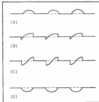
FIG. 1—Curves show output of gated amplifier for sine wave input at various phase angles
