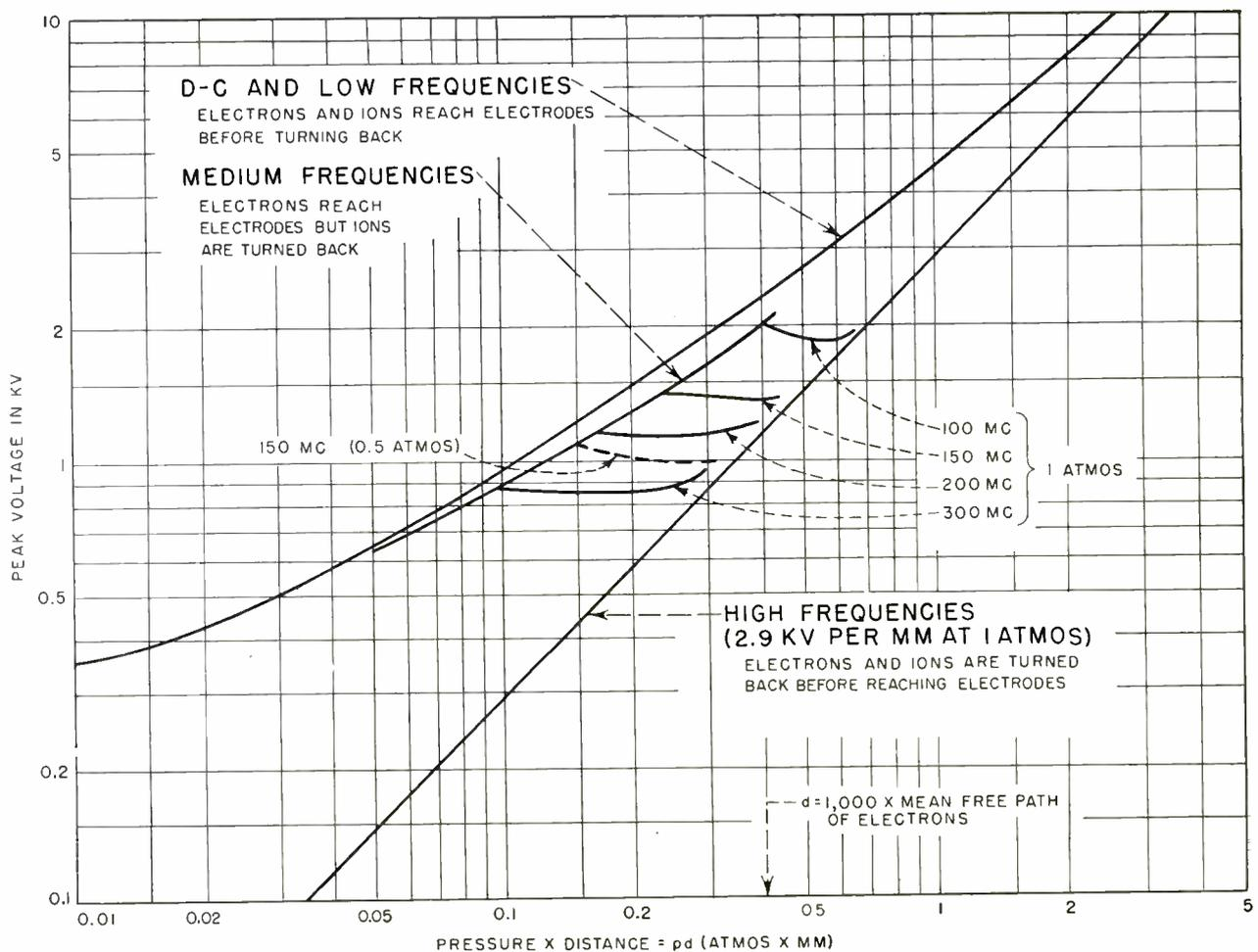
Chart giving breakdown voltage in air between parallel planes. For atmospheric pressure, horizontal scale represents distance in millimeters between the plane electrodes
