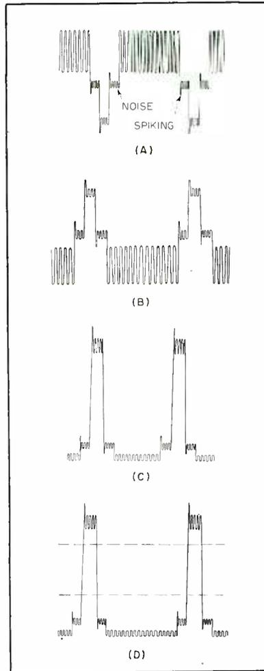
FIG. 4—Operation of sync-channel cleanup of spiking
