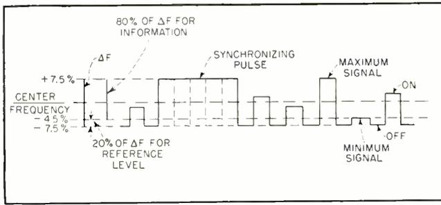
FIG. 1—Research and Development Board standard wave-forms for pulse-amplitude modulation of an f-m subcarrier. Maximum signal represents 7.5-percent deviation from subcarrier center frequency
