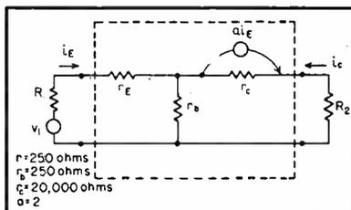
FIG. 6—Equivalent T circuit and type-A average element values
