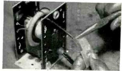
Squeezing heat-softened plastic to form seal
