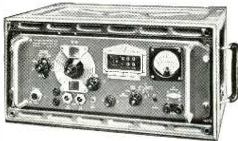
For carriers in the range 2.5 to 200 megacycles, this ruggedized deviation meter is ideal. With crystal-standardized deviation ranges of 5, 25 and 75 kilocycles, alternative high- and low-level buffered inlets, visual checking for optimum tuning and level, together with a separately buffered audio outlet, FM Deviation Meter TF 934 incorporates every desirable refinement. There are no critical tuned circuits to drift and the overall demodulation distortion is less than 0.1 per cent.
