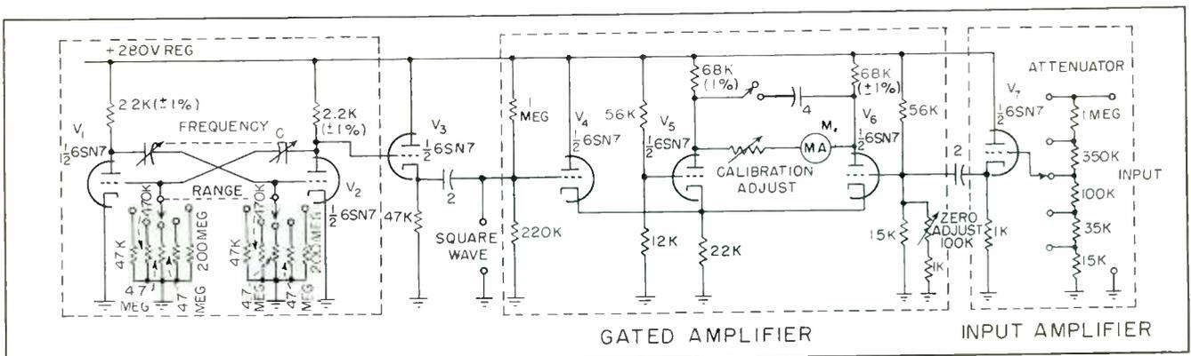
FIG. 3—Complete circuit, less power supply. The multivibrator range switch provides frequency-multiplying factors of 2, 10, 100, 1,000 and 10,000. Auxiliary terminals are provided for using the square wave output of the multivibrator separately
