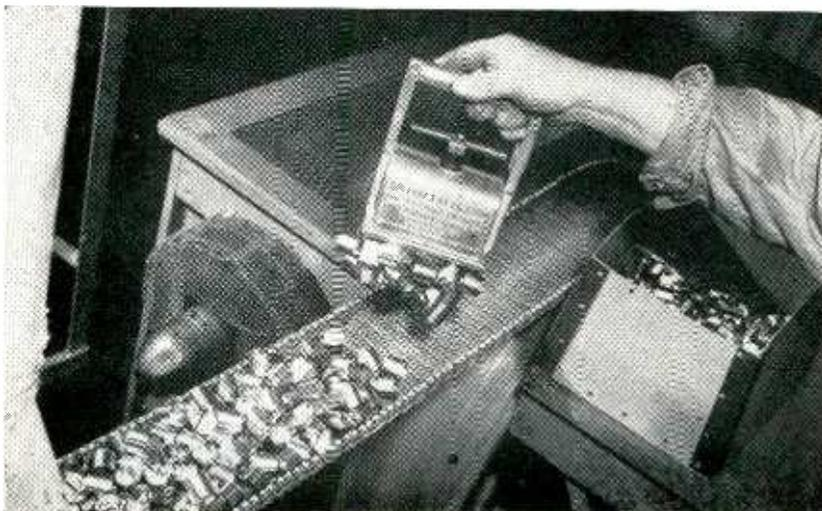
Lifting hot anodes from moving woven-wire conveyor which runs through baking oven
