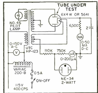
FIG. 3—Simple test circuit for checking 6X4W ruggedized and 5641 Arinc rectifier tubes
