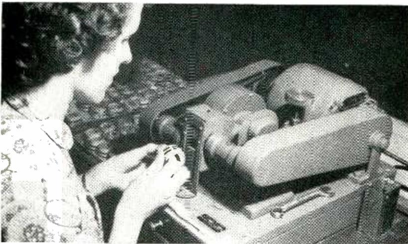
All leads of this magnetic amplifier coil are cleanly stripped of enamel when inserted in the opening. Wire brushes pull the enamel away from the operator; this direction of rotation also serves to pull in flexible fine-wire leads so they get stripped for the desired length
