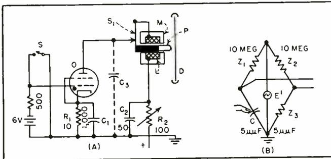
FIG. 1—Simple circuit diagram for thyatron-controlled electromagnetic system (A) and grid control via hand-capacitance bridge (B)
