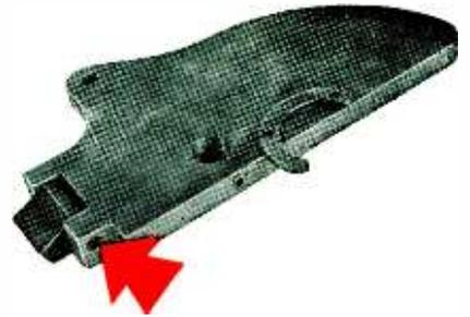
**AS A CLEVIS PIN . . .** here Rollpin holds firmly in clevis, permits free action of moving member. Rollpin application above is with the plate of a home workshop tool.
