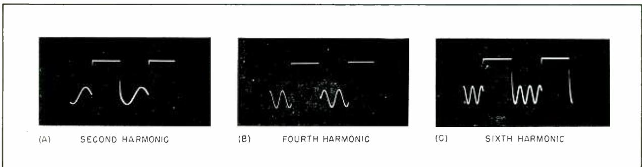
FIG. 6—Oscillograms of meter tube plate waveforms for even harmonics
