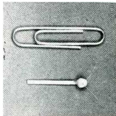
The M1689 bead-type point-contact transistor, progress in miniaturization
