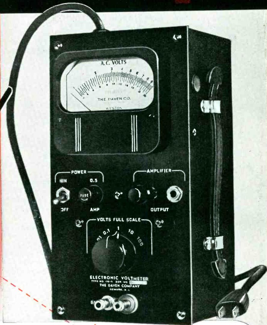
**1.** Input stages of the amplifier are shock mounted to reduce microphonics.
