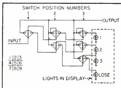
FIG. 2—Details of one of the eight sections of the defensive circuit
