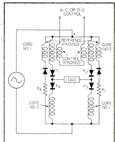
FIG. 1—Basic circuit shows use of bridge configuration to eliminate need for center tap transformer
