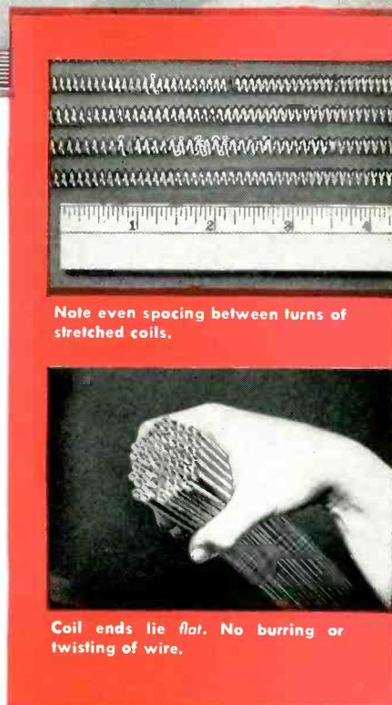
Note even spacing between turns of stretched coils.
