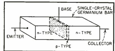
FIG. 3—Components of the n-p-n Junction transistor
