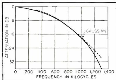
FIG. 7—Attenuation characteristics of pulse shaper
