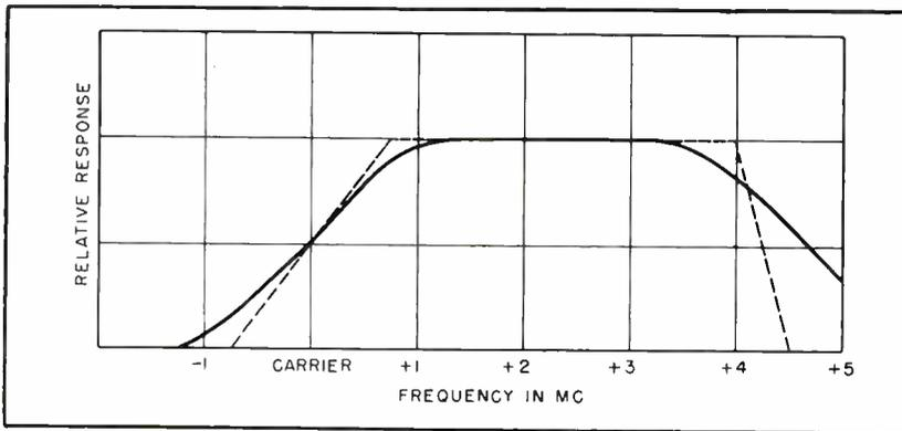
FIG. 4—Average system amplitude characteristics showing relative frequencies in megacycles
