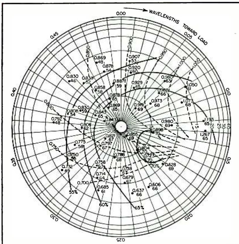
FIG. 5—Rieke diagram for a plate current of 1.0 amp and magnetic field of 1.200 gauss. Radial coordinate is the voltage reflection coefficient (scale marked in db) and azimuthal coordinate is phase angle of reflection coefficient (scale marked in wavelengths displacement of standing wave minimum). Upper numbers are wavelength (add 29,000 cm), dotted lines are constant-wavelength contours, lower numbers are percent efficiency and solid lines are constant-efficiency contours
