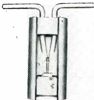
FIG. 1—Type-A cartridge structure used in earliest transistors
