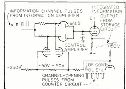
FIG. 4—Information gate is opened by sequencing pulse. Storage circuit holds information during off time
