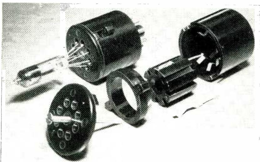
Component parts of locking adapter. In background is an assembled adapter with subminiature tube locked in position
