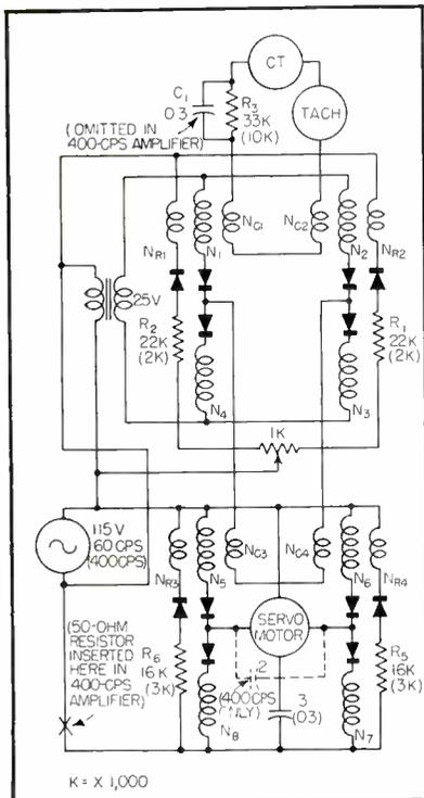
FIG. 2—Complete circuit showing parts values for 60-cps and 400-cps (in parentheses) two-stage magnetic servo amplifiers
