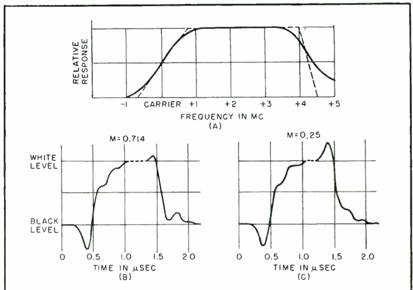
FIG. 3—Standard system amplitude characteristics (A) and output envelope waveforms for varying degrees of modulation (B) and (C)
