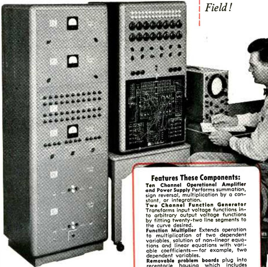
Typical Low Priced BECKMAN EASE COMPUTER Installation showing 20-channel operational amplifier and power supply, 2-channel function generator, 3-channel function multiplier, typical variable component and over-voltage panel, 30-channel problem board.
