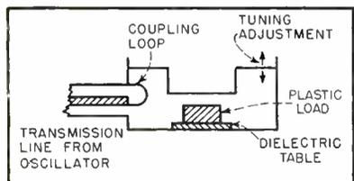
FIG. 11—Resonant cavity for heating plastic preforms
