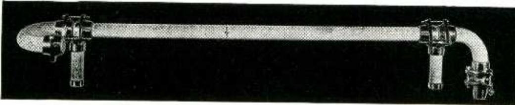
**LAPP PORCELAIN PIPE** Inside pipe diameters of  $\frac{3}{4}$ , 1,  $1\frac{1}{4}$ ,  $1\frac{1}{2}$ , 2 and 3". Available in straight pipe up to 60" lengths, 90° and 180° elbows, and fittings. All connections are swivel-type. Stand off insulators attach directly to bolts which hold pipe sections together. Metal fittings are bronze, polished heavy chrome plated.
