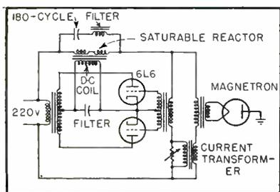
FIG. 10—Constant-temperature filament regulator circuit
