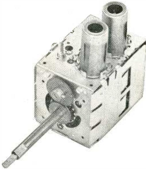
The Model TT-7 features 12 VHF channels plus 1 or 2 UHF inputs with appropriate UHF power switching built in. Available for 41 mc. IF systems. (Can be supplied for 21 mc. IF systems.)
