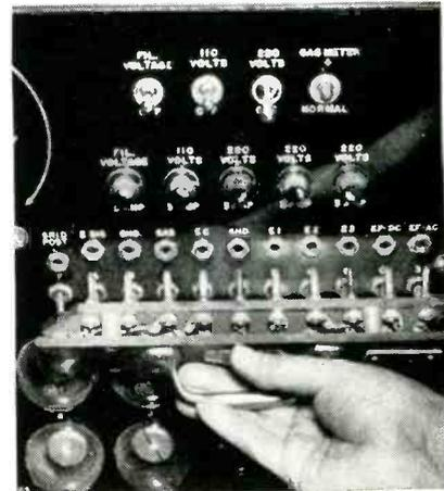
Changing voltage patch panel in test set. Switches and controls provide additional circuit changes that make test set as nearly universal as possible
