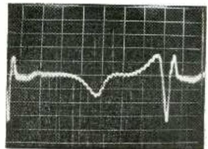
Example of heart-potential pattern obtained with equipment connected as radioelectrocardiograph (RECG), with center electrode at sterno-xiphoid junction on chest and other electrodes two inches to right and left. This location gives minimum interference from signals generated by working muscles. Timing voltage and plastic grid overlay are superimposed on pattern
