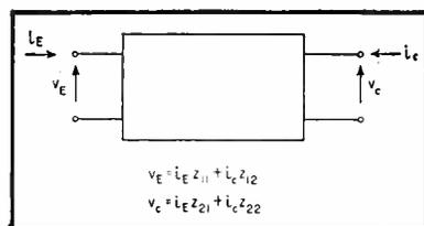
FIG. 5—General linear transistor
