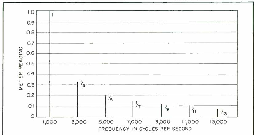
FIG. 7—Chart shows analyzer readings for 1,000-cps square-wave input
