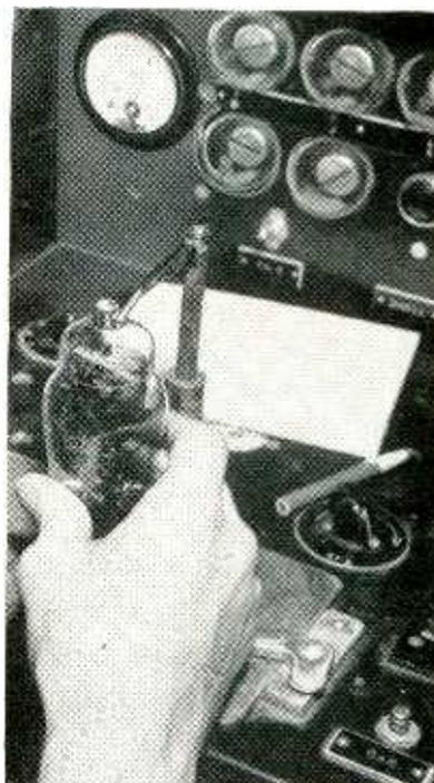
Testing 6CD6G in universal shorts and gas test set. Tube socket panel is held down by locking latch at right, needed for larger tubes. Coil spring makes top cap connection
