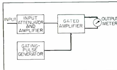
FIG. 2—Block diagram of stages in the wave analyzer
