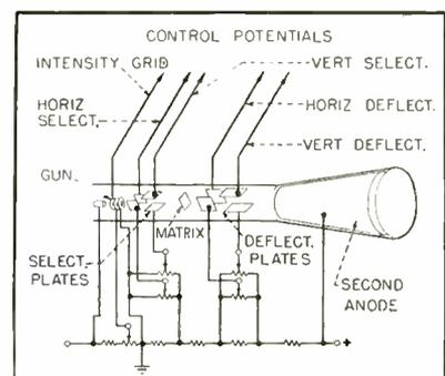
FIG. 1—Schematic-mechanical drawing of the special cathode ray tube
