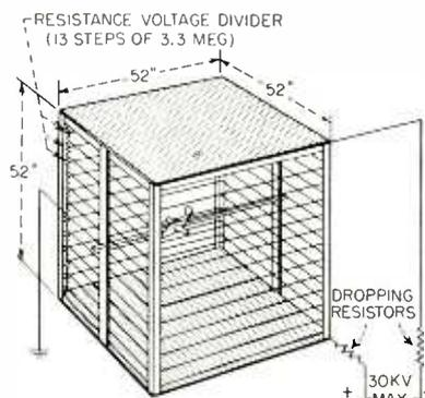
**A** UNIFORM electrostatic field is produced between the plates of a large parallel-plate capacitor made in the form of a cube shown in the cover photograph and the accompanying drawing. Fringing field effects are prevented in this Stanford Research Institute system by means of the wires shown. Each wire is made
