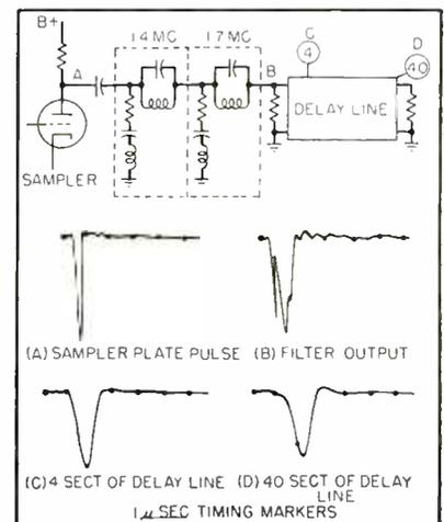
FIG. 6—Pulse shaper smooths pulses to forestall pulse interference
