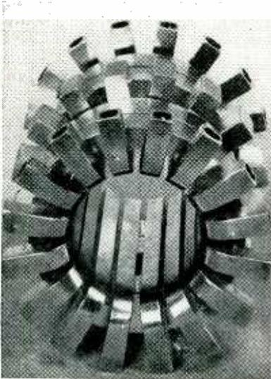
Water-cooled magnetron anode rated at 80 kw
