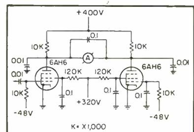
FIG. 2—Test circuit for obtaining the square-law characteristic
