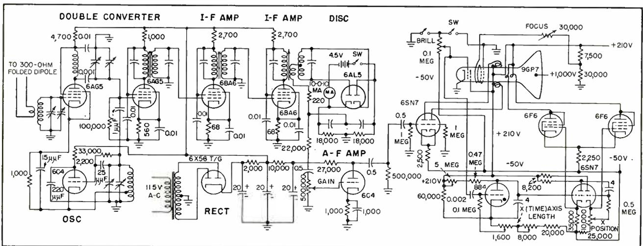
FIG. 3—Receiving and observing system of the REEG. The a-f amplifier delivers a signal output of several volts to the viewing section at the right, using a special long-persistence cathode-ray oscilloscope with a plate camera
