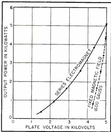
FIG. 6—Effect of plate voltage on output power
