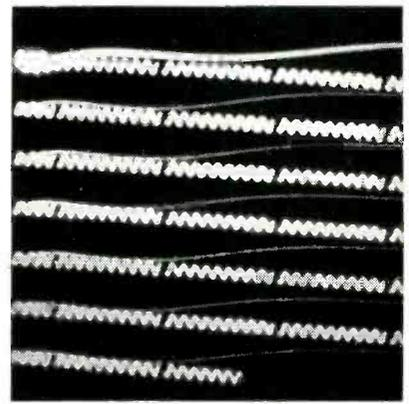
FIG. 3—Raster of Fig. 1 with ten-mc modulation applied
