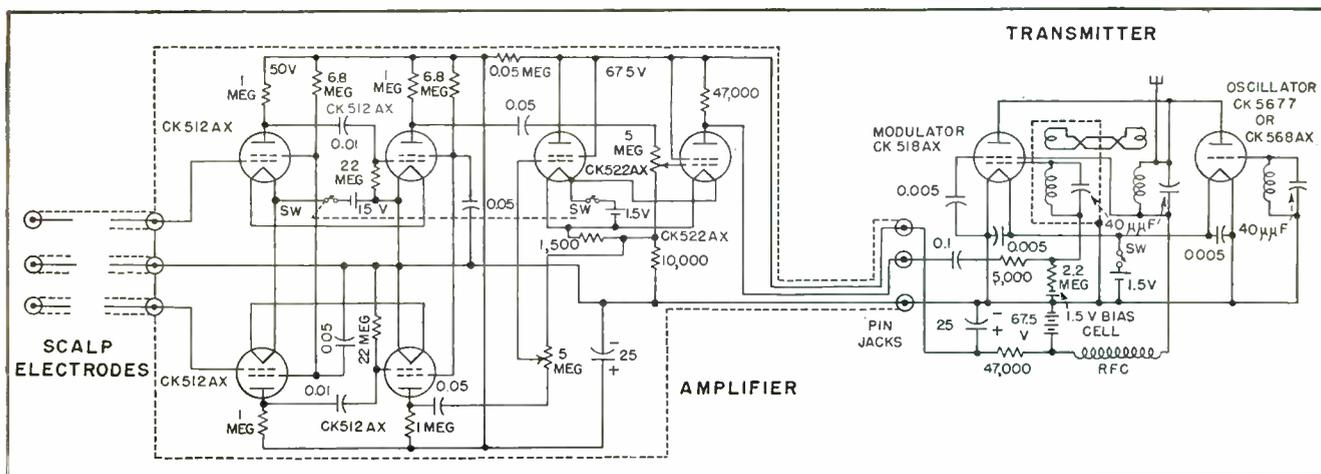
FIG. 1—Portable voltage amplifier and transmitter of radioelectroencephalograph, in two housings having total weight of only 2.6 lb
