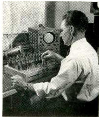
Tube under test with electronic circuits designed for use in a high-speed printer
