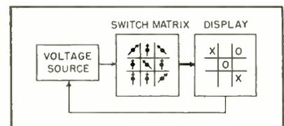
FIG. 1—Basic block diagram of the tick-tack-toe machine
