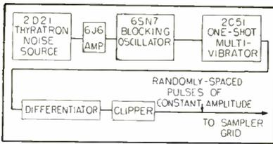
FIG. 3—Random pulser uses 2D21 thyratron as noise source for generating irregularly-spaced keying pulses
