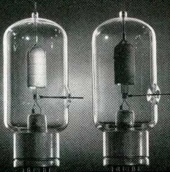
Los Gatos Type 254 Triode with tantalum anode. Plate dissipation is 75 watts.
