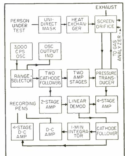
FIG. 1—Block diagram of the polyneumograph
