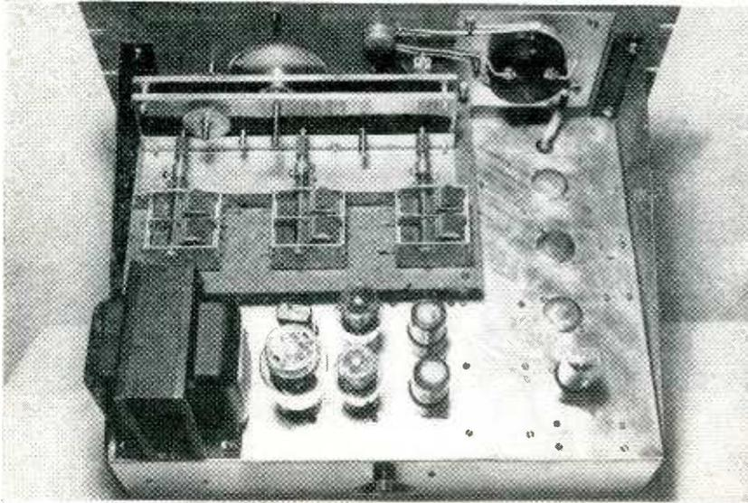
Rear view shows use of broadcast-type variable capacitors for setting frequency
