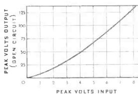
Fig. 1: Linearity of -hp- 460B Fast-Pulse Amplifier
