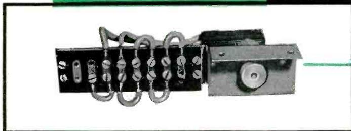
Close-up of safety screw and safety switch assembly which actuates MICRO precision switch when screw is removed from safety door of Trion "Standard Package" Electric Air Filter. Small photo shows location of MICRO panel mounting switch located at rear of terminal board assembly.
