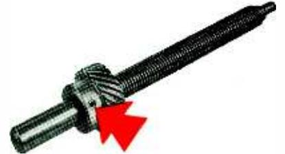
**AS A SIMPLE FASTENER . . .** Rollpin replaces a set screw in pinning a gear to a shaft. Assembly time is shorter, service life longer. Vibration-proof flush fit. Easily removable.
