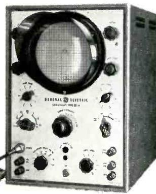
**Type ST-2A**—For general purpose use in laboratories. Excellent wide frequency response for TV receiver circuit work and industrial testing. Special features include a DC vertical amplifier to adapt the equipment to a wide range of applications. Deflection pattern can be expanded to several times the diameter of 5-inch tube.
