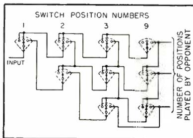
FIG. 3—Switching arrangements for the counter circuit
