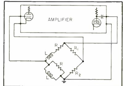
FIG. 1—Basic schematic of oscillator
