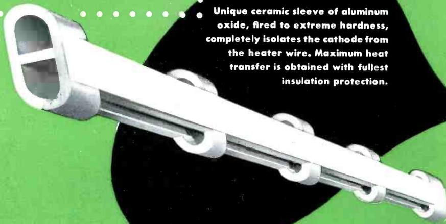
Unique ceramic sleeve of aluminum oxide, fired to extreme hardness, completely isolates the cathode from the heater wire. Maximum heat transfer is obtained with fullest insulation protection.
