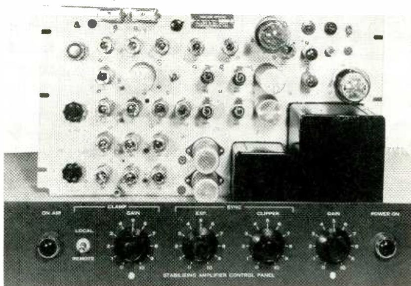
The stabilizing amplifier is rack mounted with a remote control panel for quick adjustment by operator
