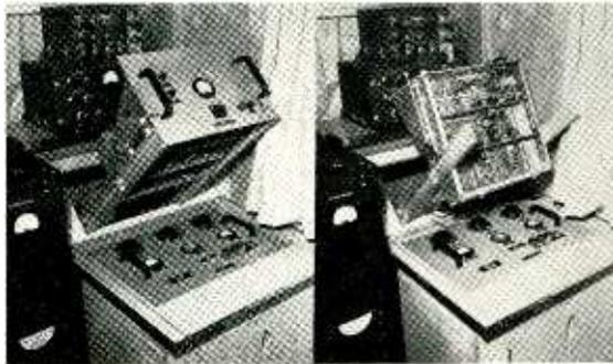
Photo shows Raydist navigation, tracking and surveying system master station where components are installed in vertical position, using Grant Slides at top and bottom of rack. Developed by Hastings Instrument Co., Inc., Hampton, Va.
