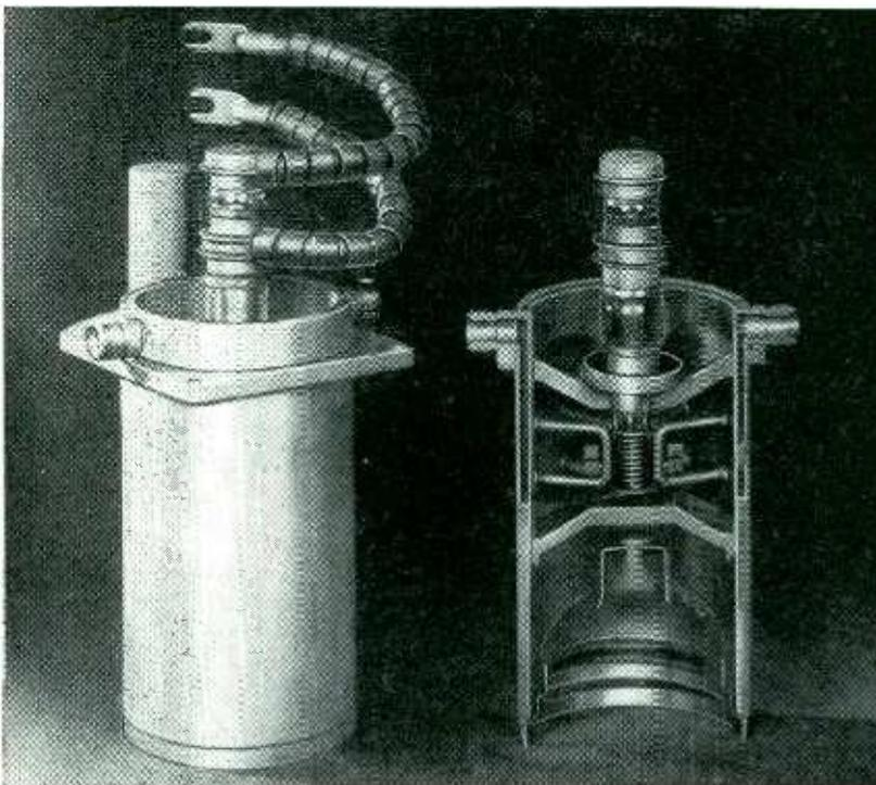
Complete and cut-away views of a water-cooled 915-mc magnetron with plate dissipation rating of 3,000 watts
