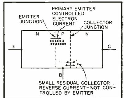
FIG. 4—Schematic diagram of a junction transistor
