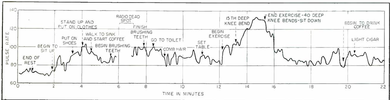
Pulse rate changes during normal human activity, as calculated and plotted from curves obtained with RECG equipment. Subject shows good recovery time back to his normal from the 130 rate arising from exercise
