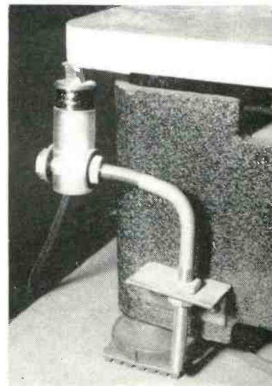
Corner of paper-jogger table, showing how amplitude-measuring coil is mounted
