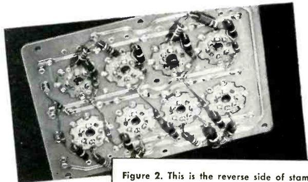
Figure 2. This is the reverse side of stamped circuit shown in figure 1. Both sides of the circuit were stamped in one operation.
