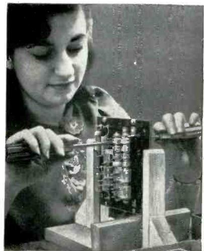
Simple wood fixture holds panel upright for maximum convenience in mounting parts on both sides
