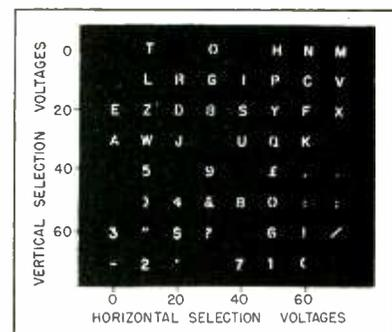
FIG. 3—Matrix layout for use in a message receiver
