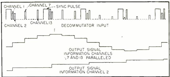
FIG. 2—Typical decommutator waveforms illustrate action of storage circuit. Output signal from information channel 2 shows original intelligence-carrying waveform reconstructed from sample pulses
