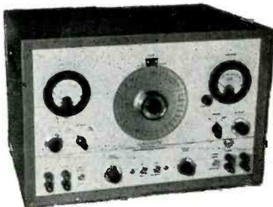
Test analyzer for use in development and PRODUCTION of SERVOMECHANISMS and PROCESS CONTROLS. Measures FREQUENCY RESPONSE, PHASE SHIFT 0.1 to 20 CYCLES SINE WAVE, SQUARE WAVE, MODULATED CARRIER, 50 to 800 CYCLES.
