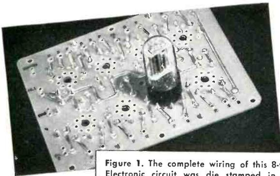
Figure 1. The complete wiring of this 8-tube Electronic circuit was die stamped in one operation. Its 90 connections soldered in another.
