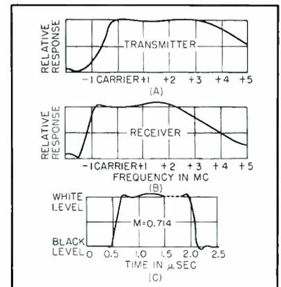
FIG. 8—Transmitter (A), receiver (B) and square-wave (C) characteristics of proposed system standards
