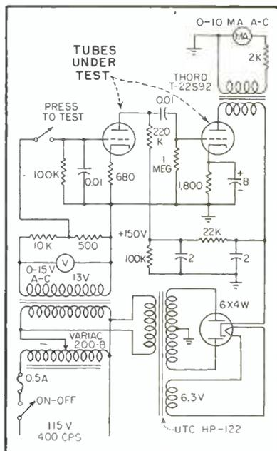
FIG. 1—Circuit arrangement for incoming-inspection test of voltage amplifier tubes for airborne electronic equipment
