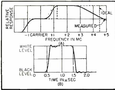
FIG. 6—Proposed step-type characteristic and resultant square-wave envelope obtained
