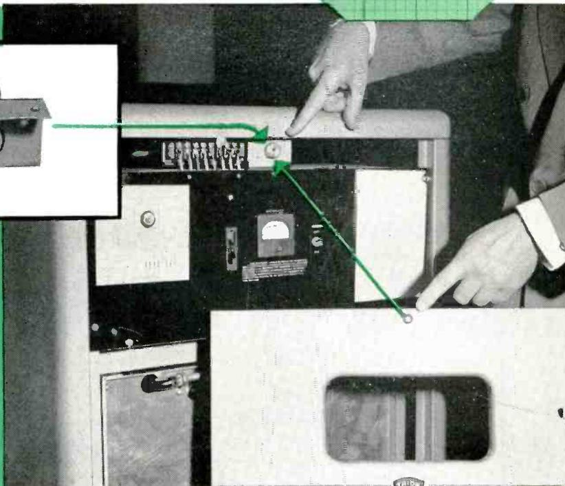
● Every Trion Electric Air Filter made by Trion, Inc. uses a MICRO precision switch to break primary circuits before access to high voltage areas is possible. Thus the complete safety of maintenance, operation and other personnel is assured.
