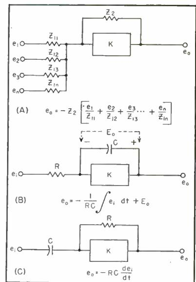
FIG. 2—Fundamental processes in analog computing are (A) summation, (B) integration and (C) differentiation
