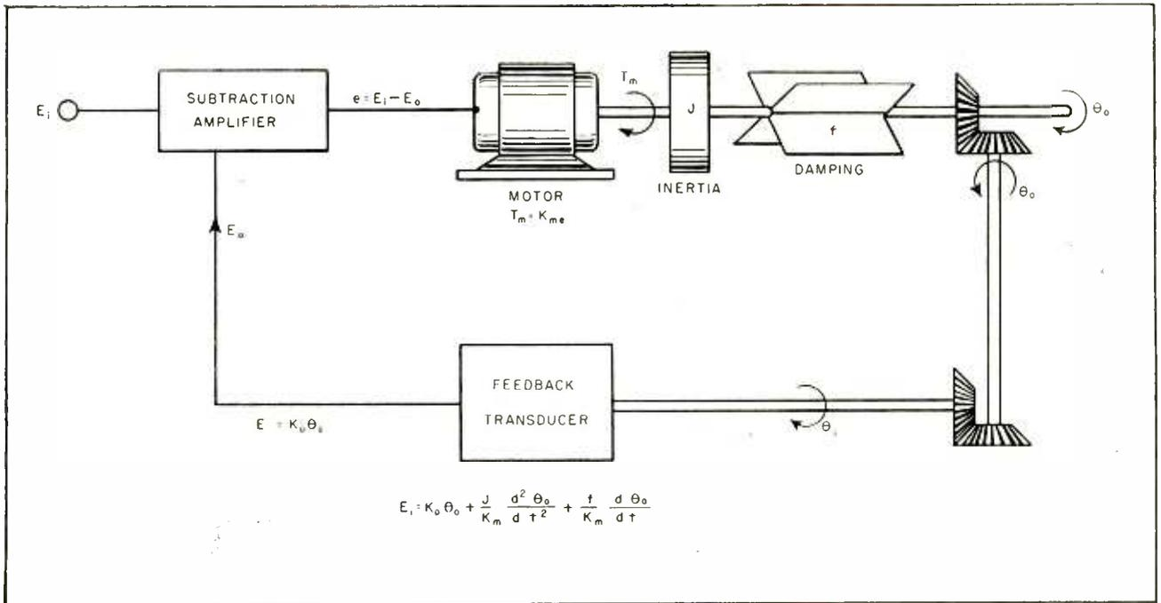
FIG. 3—Closed-loop servo system and its differential equation
