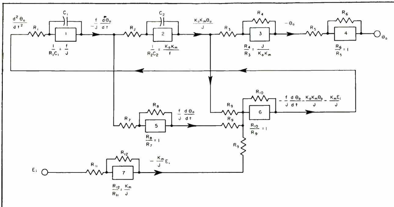
FIG. 4—Electronic analog solution of closed-loop system shown in Fig. 3
