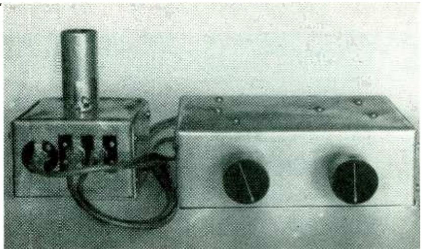
Typical oscillator construction. Tuning unit and amplifier have separate chassis
