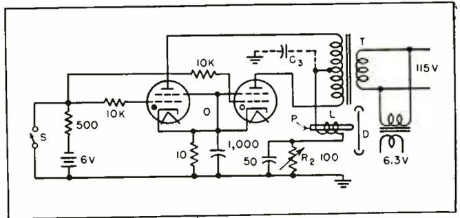
FIG. 2—Practical direct a-c type thyatron circuit free from mechanical contacts. Thyratrons are connected in push-pull arrangement
