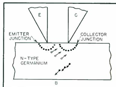
FIG. 2—Schematic diagram of a point-contact transistor
