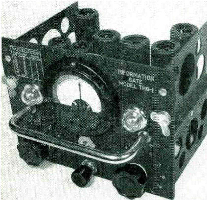
Information gate is basic building block of electronic decommutator
