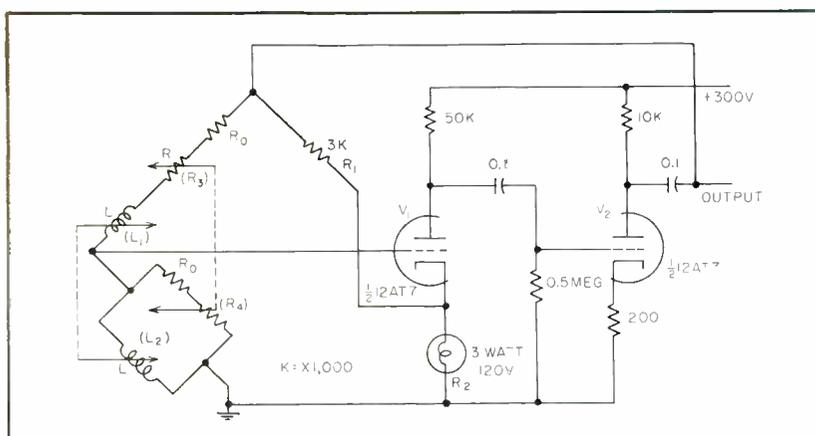
FIG. 4—Schematic diagram of R-L oscillator. For linear case  $R_3=R_4=R$  and  $L_1=L_2=L$
