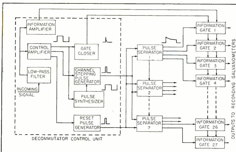
FIG. 3—Block diagram of electronic decommutator for 27 channels. Counter circuits supply sequencing trigger pulses to information gates
