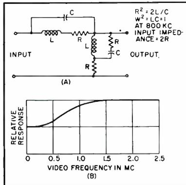
FIG. 7—Amplitude-correcting network for use at video-frequency level
