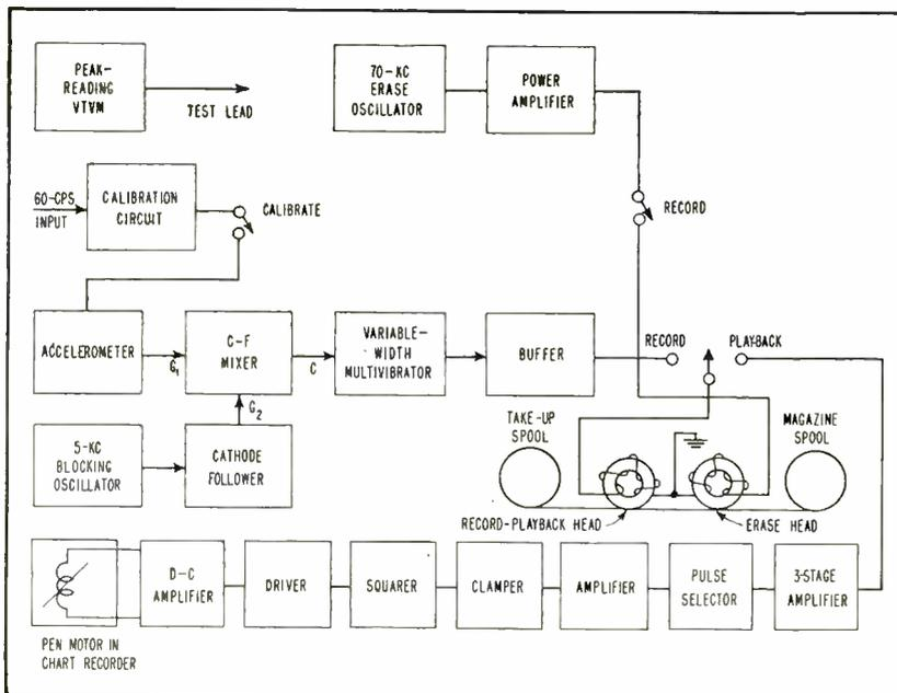
FIG. 1—Block diagram shows how system frequency response is extended using tape recorder to play back data at reduced speed
