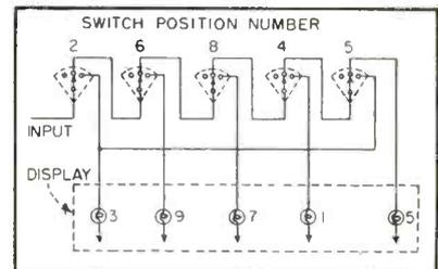
FIG. 5—Portion of special instruction section of switch matrix
