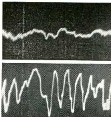
Examples of brain-wave patterns obtained from REEG system, for walking subject with eyes open (low-amplitude pattern) and with eyes closed (high-amplitude pattern)
