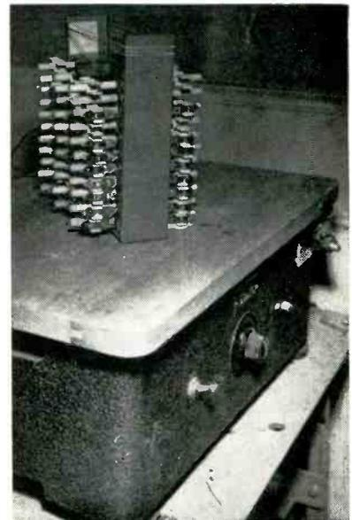
Vibration-testing type 5900 premium subminiature tubes a hundred at a time in fixture resting on table of paper jogger. Amplitude-measuring coil is at right rear corner of table
