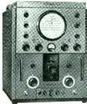
**Model SA20S** — Frequency range, with S-band head — 2400 to 3650 mc.
