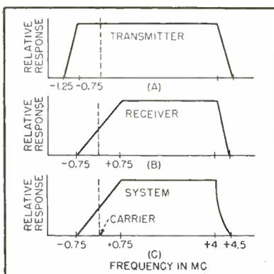
FIG. 2—Standard tv broadcast system transmission-amplitude characteristics
