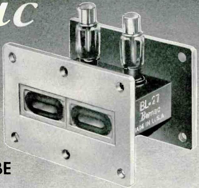
Each section of the BL27 is electrically similar to Type 1B63A. The two sections have a common wave guide wall and a common gas fill. Used with short-slot hybrids,\* the BL27 provides a highly compact duplexer of utmost simplicity, with excellent performance over the band of 8500-9600 mc. with respect to both transmission and reception characteristics.
