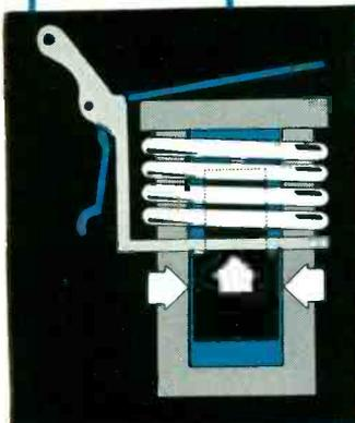
TIME DELAY is provided by a hermetically sealed, hydraulic-magnetic element. On small overloads the delay is provided while the movable core is drawn toward the pole piece, increasing magnetic flux to trip the circuit breaker. On short circuits, the core is not a factor and tripping is instantaneous. Between these extremes the delay is proportioned to the overload in accordance with the time delay curve selected.
