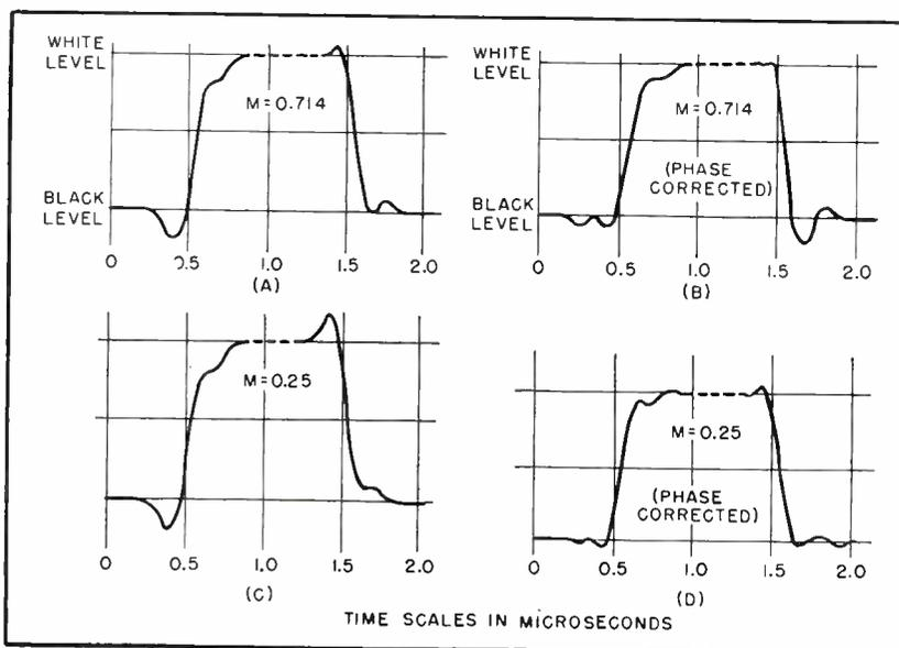
FIG. 5—Envelopes of resultant square waves for varying degrees of modulation (A) and (C) phase corrected (B) and (D)
