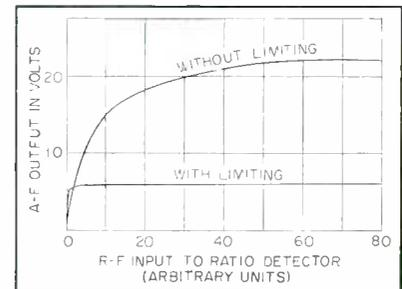
FIG. 4—Action of dry-battery limiter stage of receiver
