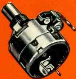
TYPE GC-45, 15/16" diameter variable composition resistor. Wattage rating: 1/2 watt for resistances through 10,000 ohms, 1/3 watt for resistances over 10,000 ohms through 100,000 ohms, 1/4 watt with 500 volts maximum across end terminals for resistances over 100,000 ohms. Available with or without illustrated attached switch and in concentric shaft tandem construction C2-45 as shown above.
