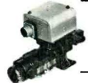
**ROTARY OIL COOLER FLAP ACTUATOR** — Lear Model 156-W24 volts d-c @ 9.0 amp. Motor speed 10,000 rpm. Intermittent duty. Potentiometer follow-up and adjustable limit switches. 7½" x 3½" x 5½". Wt. 4 lb. #SA-343 ..... \$19.50
