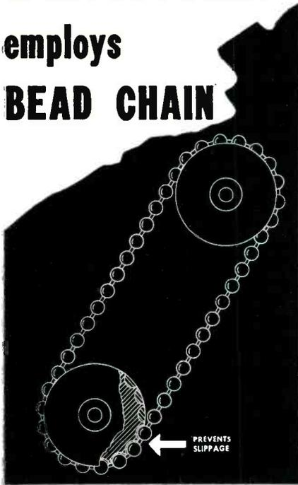
Because of its unique characteristics, Bead Chain is frequently employed by alert designers to make a simple, low-cost and highly efficient sprocket drive. Ideal for many products, it has been proved on business machines, television tuners, venetian blinds, etc. Slippage is absolutely prevented as each bead fits into an individual pocket.
