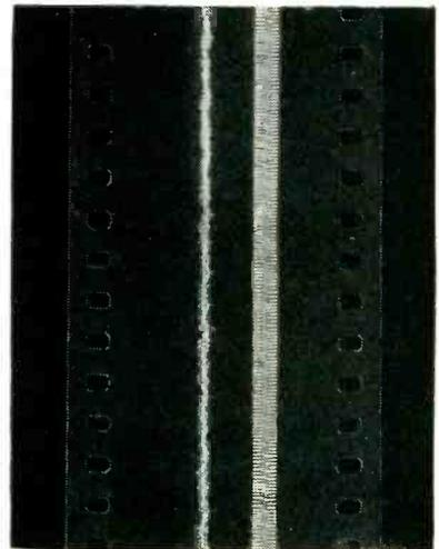
FIG. 1—Continuous moving film recording of output of recorded c-w signal shows flutter, but over 9,000 feet of film is required for 15 minutes of tape.
