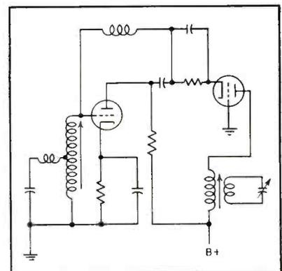
FIG. 10—Cascode i-f amplifier is most suitable for single-ended converters
