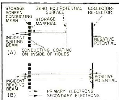
FIG. 3—Electron beam action during writing (A) and reading
