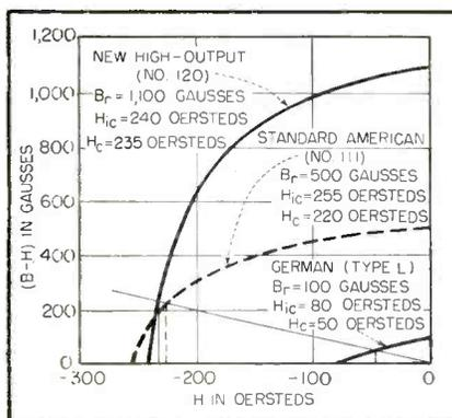
FIG. 1—Hysteresis curves showing differences in magnetic properties
