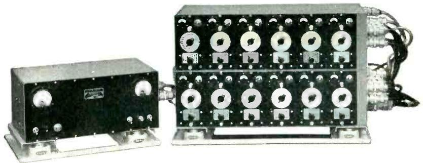
The Century Vibration and Stress Analysis System provides all of the necessary equipment to amplify and record vibration and stress-strain phenomena over a frequency range from 0 to 2000 cps.
