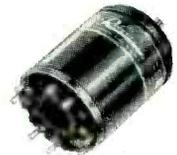
A new miniature resolver in a Navord size 15 case featuring very high input impedance (17,500 ohms when tuned at 400 cps) and a large dynamic range of operation. The unit can withstand better than 50G shock or vibration and operates perfectly above altitudes of 50,000 feet. Type R-151 is winding compensated.
