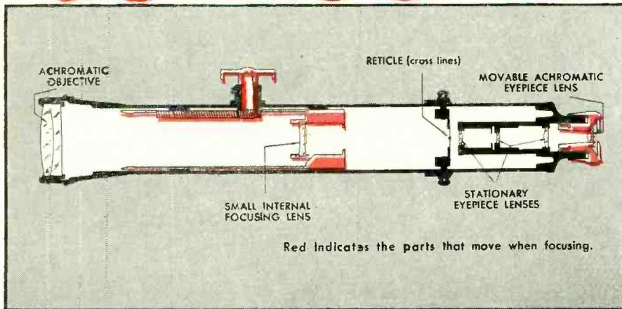
Cross lines so fine as to be almost invisible can be placed inside the instrument at exactly the place where the miniature picture is formed. Then the eyepiece will greatly magnify not only the picture but the cross lines as well so that both are seen together. Basically, that is the principle of the tele-
