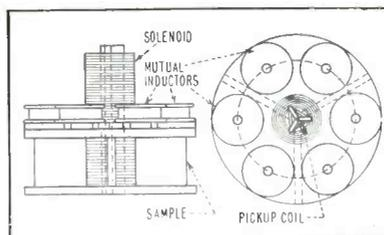
FIG. 5—Pickup device used with a magnetic tape sample when testing performance characteristics
