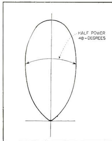
FIG. 2—Circular polarization of transmission as measured in a helix-to-helix overall system
