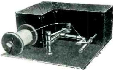
A completely self-contained, self-powered unit for winding pi or universal coils of variable width, to a diameter of 4 inches.
