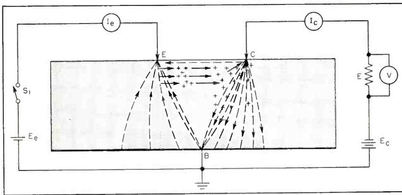
FIG. 4—Drawing shows simplified essentials of transistor action (when  $S_1$  is closed) for point contact transistor. Plus signs indicate positively-charged holes that migrate from emitter toward collector
