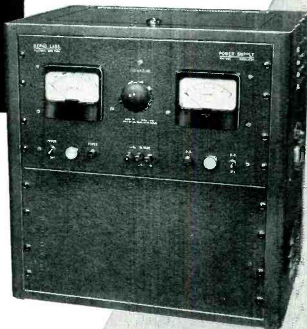
**OUTPUT TERMINATIONS:** DC terminals are clearly marked on the front panel. Either positive or negative terminal of the supply may be grounded. DC terminals are isolated from the chassis. A binding post mounted on the front panel is available for connecting to the chassis. All terminals are also brought out at the back of the chassis.
