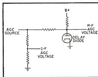
FIG. 6—Cross-over network for reducing agc bias on i-f amplifier
