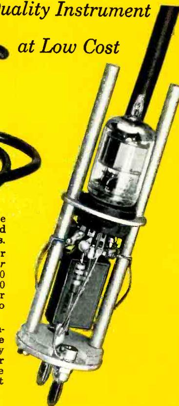
The input voltage is rectified by one section of the twin diode and the d-c passed on to the grid of a triode in one arm of a balanced amplifier circuit. The other, "inactive", diode balances the effects of contact potential of the input diode. The balanced amplifier circuit insures minimum shift in calibration with line voltage changes.
