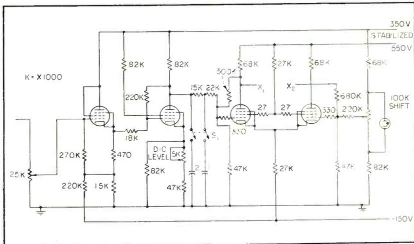
FIG. 7—Horizontal deflection amplifier responds only to low-frequency  $f_2$ , is direct-coupled. Miniature pentodes are used (Brimar 8D3 or 6AK5)
