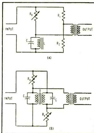
FIG. 2—Two alternate audio filters using a parallel-resonant circuit (A) and a tuned transformer (B) to attenuate a single frequency
