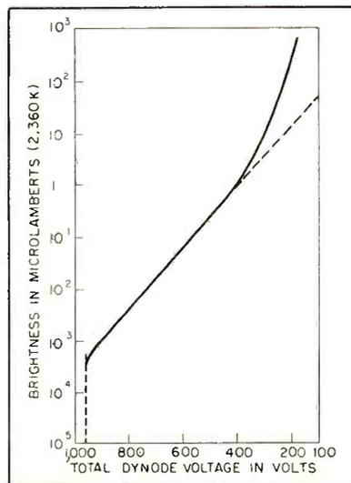
FIG. 4—Dynode voltage-light intensity characteristic for phototube
