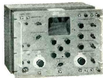
4. New Input impedance without probe—1 Megohm. With Probe—10 Megohms.
