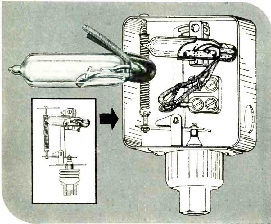
THESE illustrations show how a HONEYWELL Mercury Switch was used to provide direct control and high capacity for substantial electrical loads from a light energy pressure system without the use of intermediate relays.
