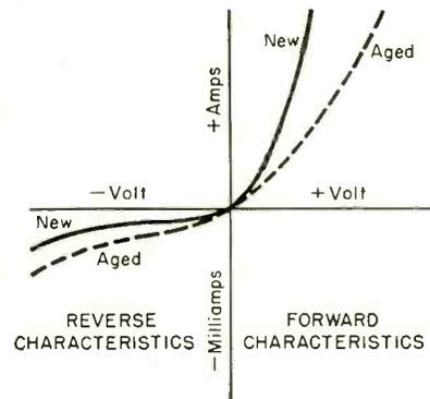
Therefore, if you wish to determine the quality of a rectifier cell, it is necessary to consider the forward and reverse characteristics and the effect that aging has on both characteristics.
