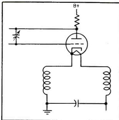
FIG. 5—Transmission line-tuned oscillator covers full uhf band
