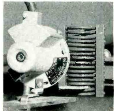
Closeup view of detector and work coil of induction heating unit
