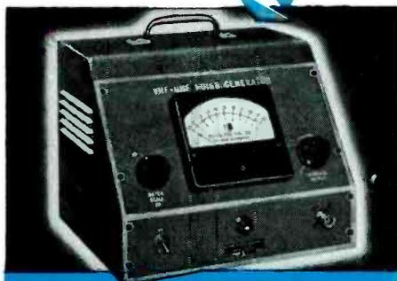
**TYPE 904 NOISE GENERATOR** — a direct reading noise source permits measurements of noise factors up to 20 db for r-f amplifiers and receivers operating in the range from 10 to 1000 mc/s. A TT-1 coaxial diode with a nominal input impedance of 50 ohms is used. VSWR is approximately 1.25, housed in handsome steel cabinet.
