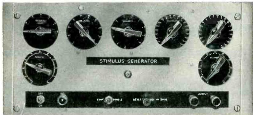
Front panel of the instrument showing the various controls for repetition rate, pulse width and amplitude
