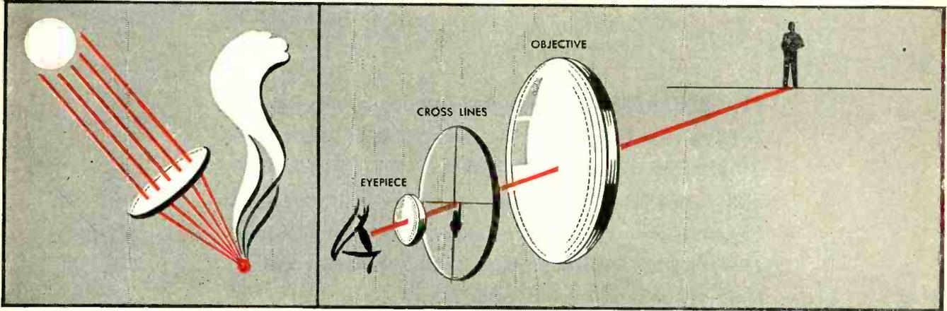
Even an ordinary reading glass can produce an image of sorts. That happens when the sun's rays are focused on a piece of paper as shown. All the rays passing through the lens concentrate at approximately one point where they form a small inverted picture or image of the sun.
