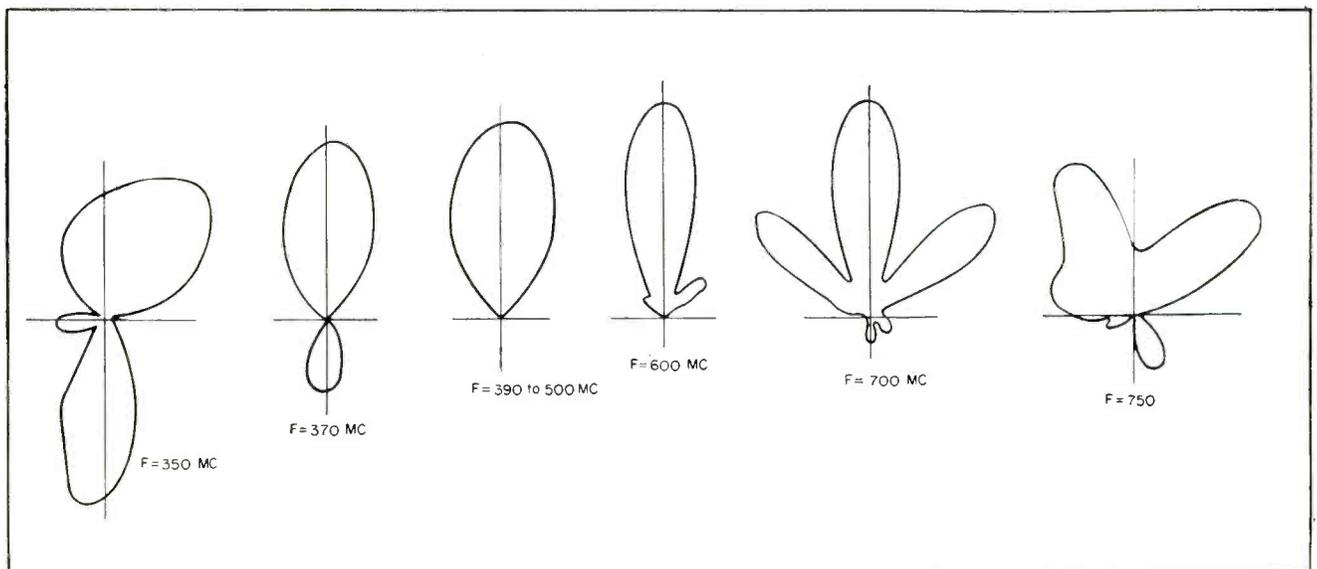
FIG. 3—Pattern for helix designed at 450 mc stays unidirectional from 390 to 600 mc. Half power beam width at 390 mc is 53 degrees, at 600 mc is 38 degrees, representing a very high-gain mode of operation
