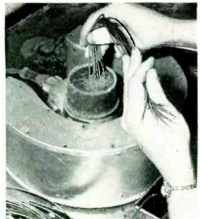
Aluminum guard prevents solder pot from being knocked over and at same time serves as convenient hand rest for controlling immersion of wires in solder
