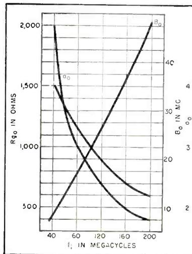
FIG. 9—Turns ratio, bandwidth and optimum  $R_{go}$  versus i-f frequency
