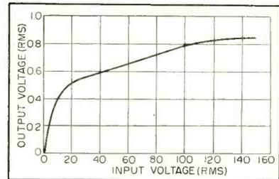
FIG. 7—Mechanical filter overload characteristic at 455 kc
