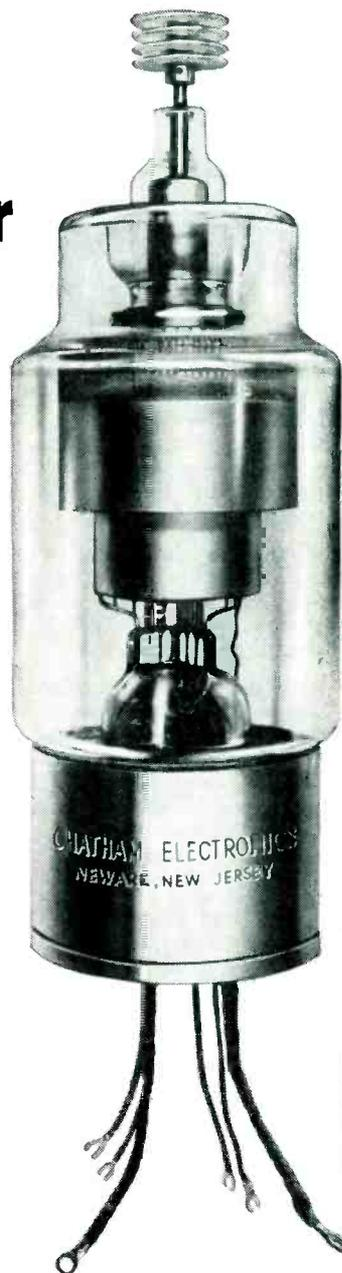
Low carbon Nickel was the choice for the spun anode sleeve and other critical parts in this 40 million watt power tube produced by the Chatham Electronics Corp., Newark 2, N. J.
