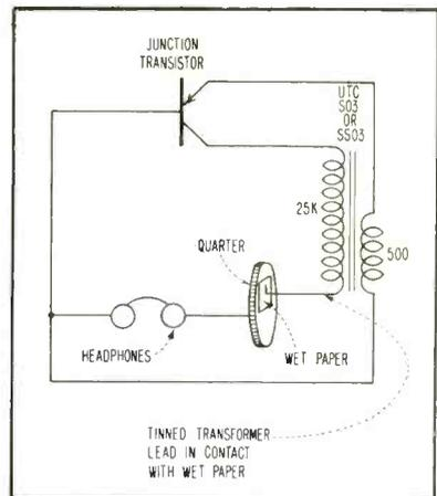
Simple oscillator uses commercially available parts. Tone is heard in headphones from transistor oscillator powered by power source made from a quarter, a tinned transformer lead, and a piece of saliva-soaked paper
