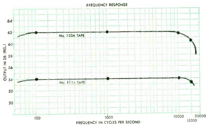
The frequency response characteristics of both No. 120A and No. 111A tapes are virtually identical at 15 ips tape speed. These curves were made with each tape set at optimum bias and an input level 15 db below 1% 3rd harmonic distortion.
