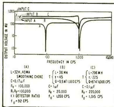
FIG. 3—Attenuation curves obtained with filters using various values of circuit components
