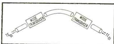
FIG. 4—Representation of the kinds of elements that are necessary in a normal-mode bend
