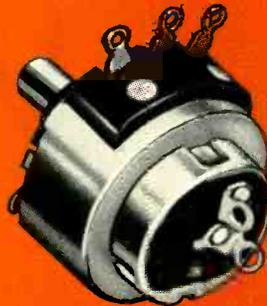
TYPE GC-252, 2 watt, 1 17/64" diameter variable wirewound resistor. Available with or without illustrated attached switch and in concentric shaft tandem construction C2-252 as shown above.
