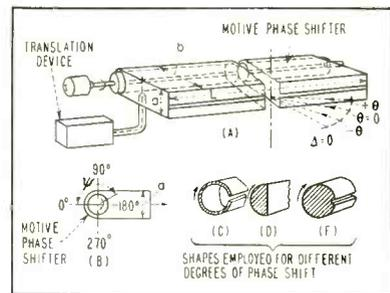
FIG. 7—Nonmechanical antenna director uses motor-driven phase shifter within a fixed antenna structure
