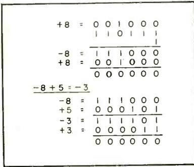
FIG. 8—Examples of binary arithmetic with negative numbers
