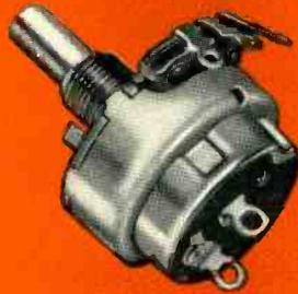
TYPE GC-35, 1 1/8" diameter variable composition resistor. Wattage ratings: 3/4 watt for resistances through 10,000 ohms, 2/3 watt for resistances over 10,000 ohms through 25,000 ohms, 1/2 watt with 500 volts maximum across end terminals for resistances over 25,000 ohms. Available with or without illustrated attached switch and in concentric shaft tandem construction C2-35 as shown above.
