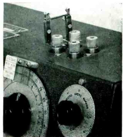
Calibrating bar in place on Q meter
