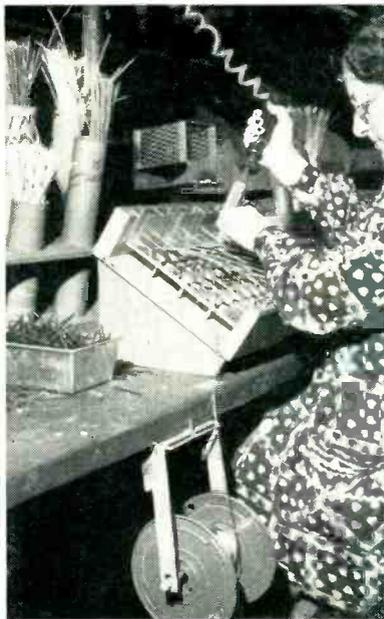
Fixture for holding three-potentiometer strips. Soldering iron is plugged into overhead outlet, and rests in horizontal holder at back of bench when not in use. Solder reel holder is screwed to bottom of bench
