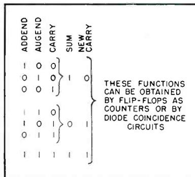
FIG. 6—Three-terminal binary adder
