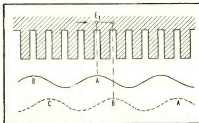
FIG. 2—Electron group  $E_1$  interacts with successive peaks of electromagnetic wave in phase
