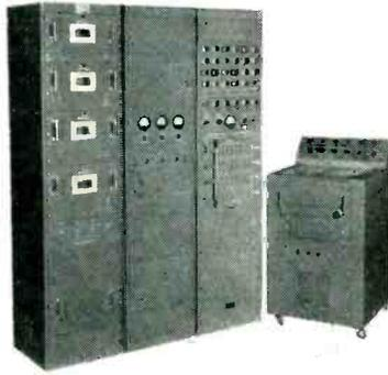
**THE REAC FAMILY** of electronic and electro-mechanical units continues to grow in number and capability. The Electronic Function Generator and the Electronic Multiplier were recently introduced for real time applications requiring high speed response, where mechanical methods with their inherent frequency limitations were unsatisfactory.
