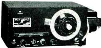
The Type 105-B Micrometer Frequency Meter measures center frequency deviation on any number of transmitters, AM or FM, from 0.1 MC. to 175 MC. The accuracy, determined by over 500 field tests, is conservatively guaranteed better than 0.0025%, surpassing FCC requirements. Readily checked against WWV. \$22.00
