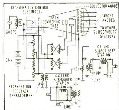
FIG. 8—Cathode-ray beam-switching tube is used as an inertialess switch-board for telephone subscribers
