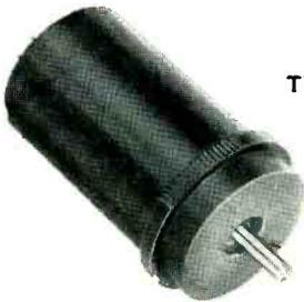
For 60, 400 or 1000 cycle operation; network or winding compensated for high precision trigonometric applications and winding compensated for additional sweep circuit usage. The winding compensated resolvers type R-602 are capable of operation within a frequency range of 10 to 40,000 cps.
