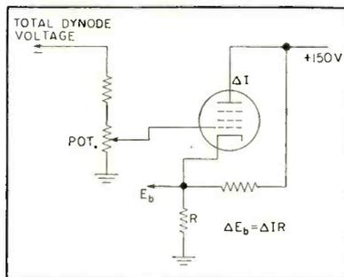
FIG. 5—Basic correcting circuit for high-intensity response
