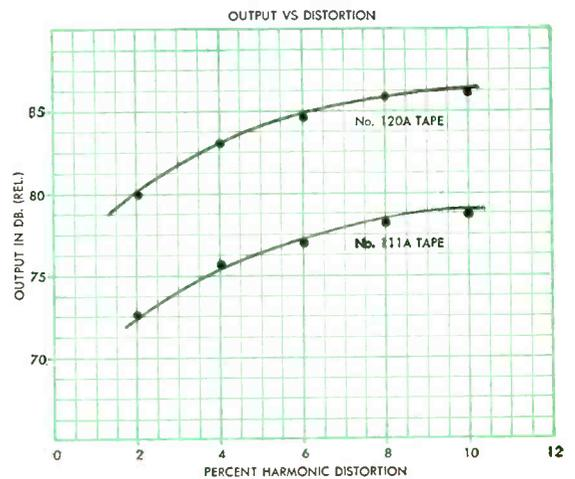
This graph shows the 8 db increase in output of High-Output Magnetic Tape No. 120A over No. 111A at any given distortion level. When compared with other brands of magnetic tape, the difference in output is as much as 12 db!
