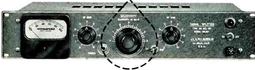
The McLAUGHLIN type MCL-50 SIGNAL-SPLITTER is the first and only selectivity converter deliberately designed to provide exact jam-free-bandwidths for every CW/SPEECH receiving conditions. It is compact, requiring only 3½ inches of rack-panel space . . . Simple connection to I-F in receiver . . . Has self-contained power supply and audio amplifier . . . Output is 18 dbm/600 ohms. Price \$1200
