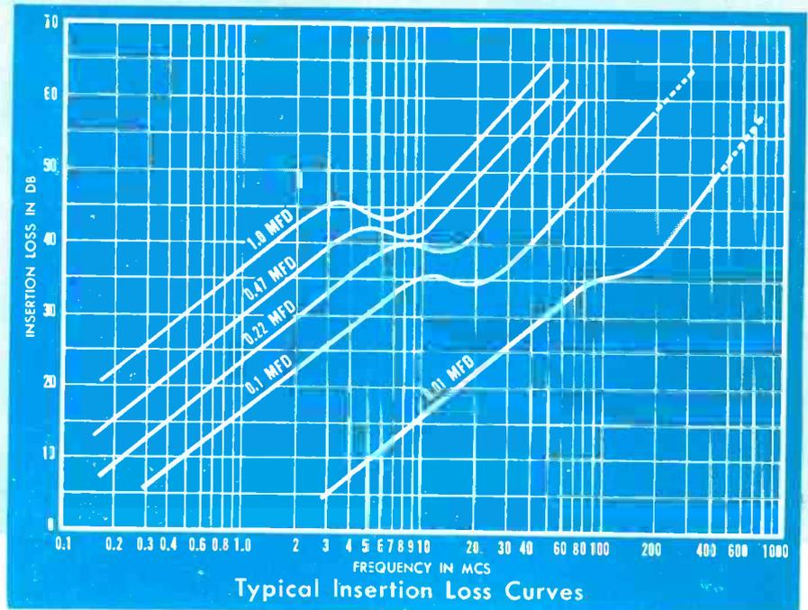
**T**HRU-PASS CAPACITORS are a new Sprague development for use in radio interference reduction in communication and radar equipment.
