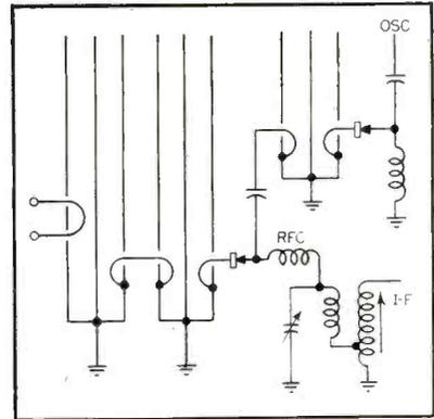
FIG. 3—Single-channel converter designed for minimum noise figure
