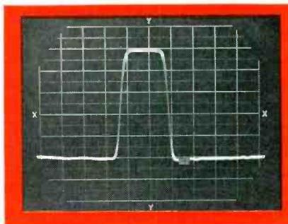
**SWEEP DELAY** The accurately calibrated delay of the 401 provides means for measuring pulse widths, time intervals between pulses, accurately calibrating sweeps and other useful applications wherein accurate time measurements are required.
