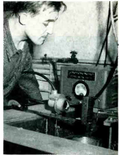
Experimental setup of optical thermometer, here aimed between turns of work coil to measure heat of test sample inside
