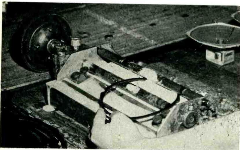
Wringer-type cement applicator driven by friction from assembly-line belt, designed by Crosley for applying cement to speaker gaskets
