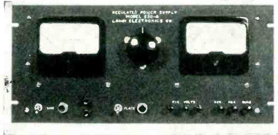
This unit is designed for general laboratory use where good regulation, low ripple, and low output impedance along with wide voltage range and heavy load current are required. It incorporates a bias and filament supply so that this single source may supply all the power required for most design or test set ups.
