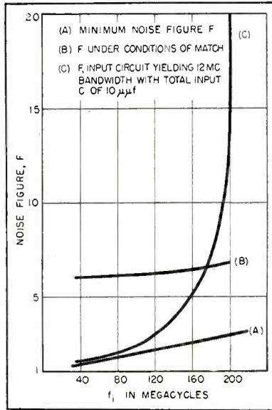
FIG. 8—Noise figure  $F$  versus frequency
