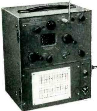
**Direct Reading VHF Frequency Meter Model FM-3**
