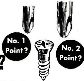
The Phillips screw and the two XCELITE Phillips points are shown actual size. You can use the #1 point—but it will fit somewhat loosely, and damage results to both screw and point. The #2 point does fit snugly, even though it appears too large. So, to make your points last longer, always try a size larger screwdriver than you think would fit.
