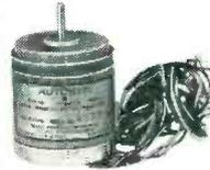
**HIGH PRECISION AUTOSYN** — Pioneer Type AY-201-3-B transmitter or control transformer for controlled servo circuits. Same as AY-200-3 and AY-202-3 except for shaft detail. 26 volts 400 cycle single phase. Max. error 15 min. Eclipse-Pioneer specification sheet available on request. Wt. 5 oz. max. #SA-365 ..... \$27.50
