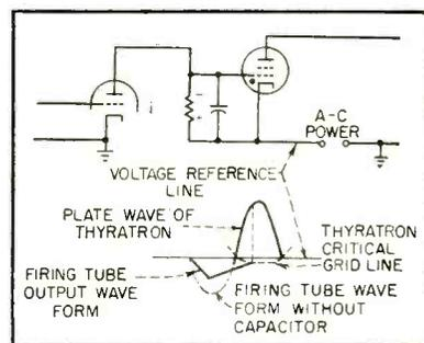
FIG. 3—RC network in grid circuit generates saw-tooth wave whose amplitude can be varied to control firing time of thyatron
