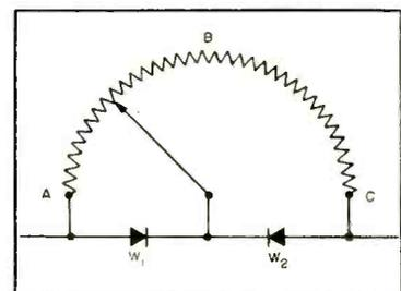
FIG. 6—Back-to-back rectifiers and motor-driven arm vary voltage at low frequency from plus to minus
