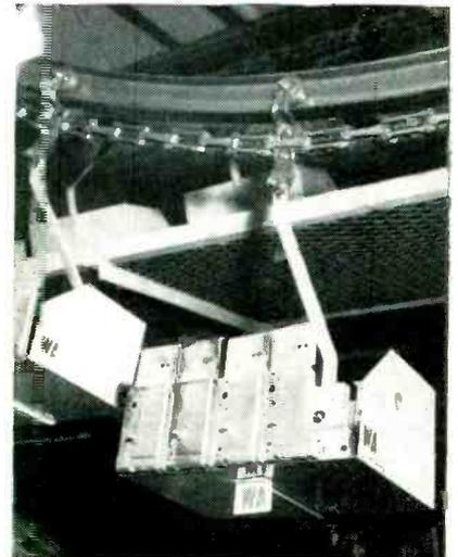
Use of conveyor pan for wrap-around auto radio housings
