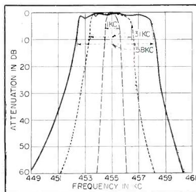
FIG. 1—Frequency response of three different mechanical filter designs described in text
