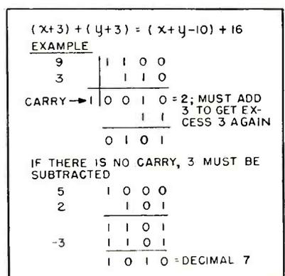
FIG. 16—Excess-three arithmetic
