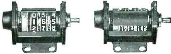
Companion shutter counters used as dual direction indicators. One counter add, while the other subtracts. Shutter blanks out counter which is on negative side of 000.
