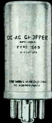
These Choppers convert low level DC into pulsating DC or AC so that servo-mechanism error voltages and the output of thermocouples and strain gauges, may be amplified by means of an AC rather than a DC amplifier.
