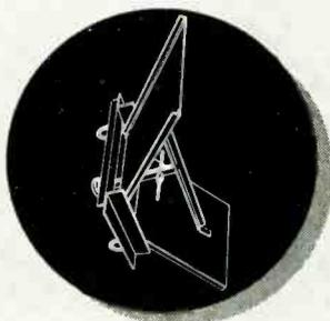
**The Corner Reflector antenna**, 8db forward gain, broadband, horizontal or vertical polarization.
