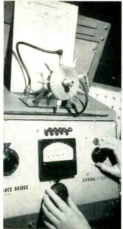
Tube is plugged into holes in center of adapter on top of bridge, and metal shield is pushed over tube as shown, for sampling inspection check of inter-electrode capacitance. Chart behind adapter gives approximate values and bridge connections
