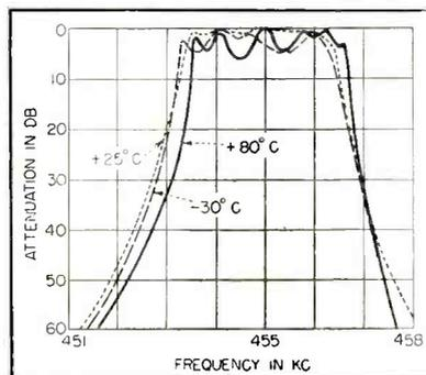
FIG. 10—Curves show temperature dependence of mechanical filters
