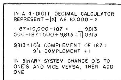
FIG. 7—Negative numbers in a digital computer
