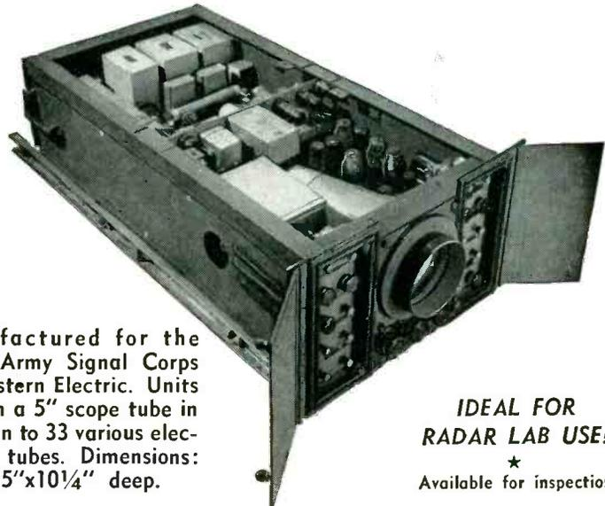
Manufactured for the U. S. Army Signal Corps by Western Electric. Units contain a 5" scope tube in addition to 33 various electronics tubes. Dimensions: 17 1/4 x 35 1/2 x 10 1/4" deep.
