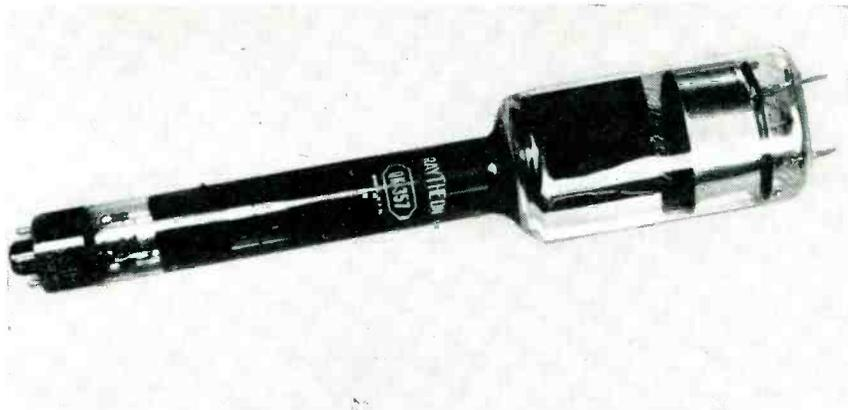
Improved-design recording tube gives long storage time despite repeated playbacks. Electron lens between anode and first screen avoids performance limitations of earlier-model tube
