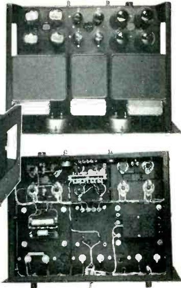
Design features of the new Eastgap Model Two Regulated Power Supply assure reliability. Ripple including noise and jitter less than 1/3 millivolt. Impedance — 1/20 ohm or less throughout load range. 15 microfarad oil condenser directly across output for impulse stability. Stabilized high-performance balanced-input amplifier. All transformers and inductors are hermetic and have grain oriented cores. Operates from 50-60 cycle, 115 volt line. Suitable either on bench or rack.
