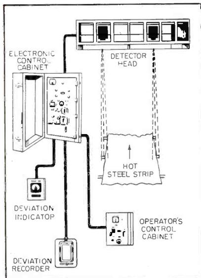
FIG. 1—Arrangement of main units of width gage
