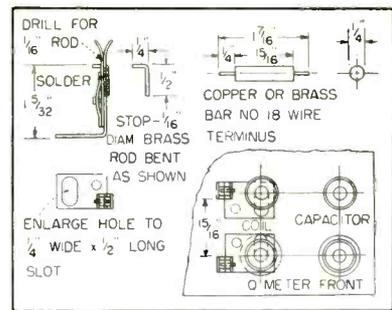
FIG. 2—Construction of special terminal clips and brass calibrating bar
