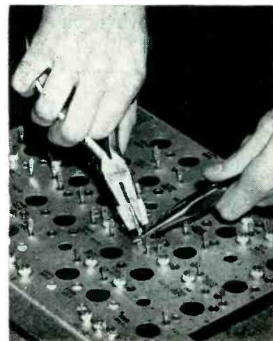
Method of holding tools for stripping insulation close to chassis
