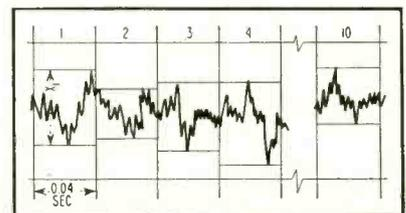
FIG. 2—Short samples provide sufficient accuracy in making flutter measurements on instrumentation tape recorders
