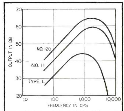
FIG. 3—Frequency response curves, recorded at constant current
