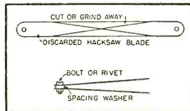
Method of making homemade tweezers for speeding electrical maintenance work. The points can be filed and bent to suit the needs of any job
