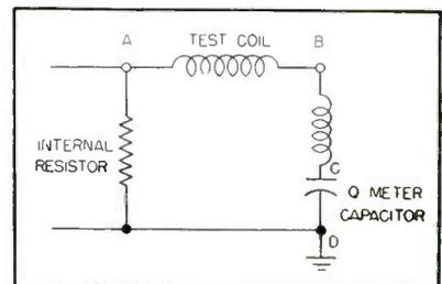
FIG. 1—Output circuit of Q meter
