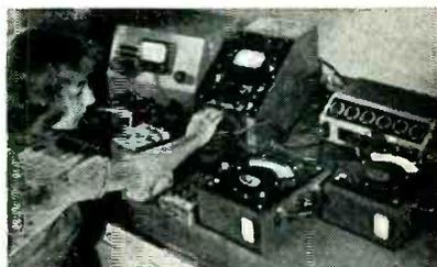
**POWER LOSS MEASUREMENT**—Losses as low as 15 micro watts in the range of 20 c to 200 MC can be measured and analyzed and possible improvements effected.
