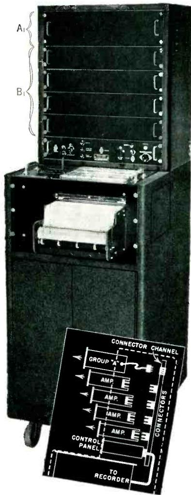
As shown in the diagram, removing or interchanging any of the amplifiers or other instruments is simply a matter of sliding the unit in or out of the mounting rack where contact is made automatically by plug-in connectors. Screws at the four corners of the panel hold the instrument in place.
