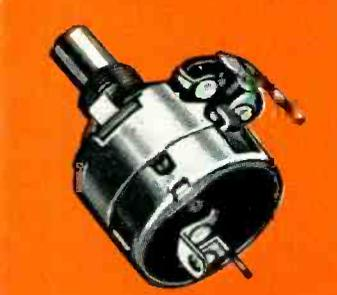
TYPE GC-45, 15/16" diameter variable composition resistor. Wattage rating: 1/2 watt for resistances through 10,000 ohms, 1/3 watt for resistances over 10,000 ohms through 100,000 ohms, 1/4 watt with 500 volts maximum across end terminals for resistances over 100,000 ohms. Available with or without illustrated attached switch and in concentric shaft tandem construction C2-45 as shown above.
