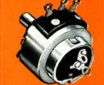
TYPE GC-252, 2 watt, 1 17/64" diameter variable wirewound resistor. Available with or without illustrated attached switch and in concentric shaft tandem construction C2-252 as shown above.
