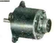
● REMOTE POSITION TRANSMITTER — GE 8TJ9. 360 degrees (Continuously rotatable) potentiometer Taps @ 120 deg. Two contacts 180 deg. apart. 24 volts d-c. Weighs 4 oz. SA-1A3 .. \$3.75
