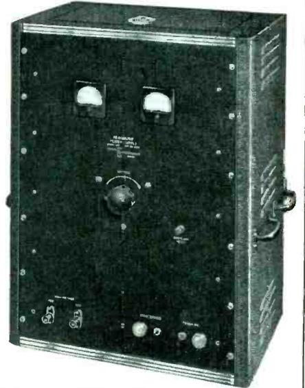
For evaluating the dynamic characteristics of rate gyros and angular accelerometers
