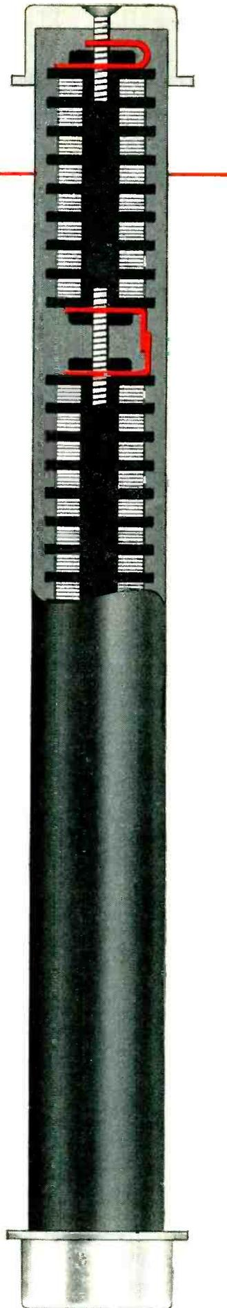
"Meter multiplier" —  $9\frac{25}{32}$ " long, ferrule type—houses four I-T-E precision resistors wound on bobbins of the same material as the encapsulation. This assures uniform low coefficient of expansion throughout the resistor resulting in a true hermetic seal.
