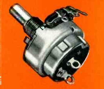
TYPE GC-35, 1 1/8" diameter variable composition resistor. Wattage rating: 3/4 watt for resistances through 10,000 ohms, 2/3 watt for resistances over 10,000 ohms through 25,000 ohms, 1/2 watt with 500 volts maximum across end terminals for resistances over 25,000 ohms. Available with or without illustrated attached switch and in concentric shaft tandem construction C2-35 as shown above.
