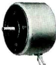
Type F4H92H-1CC **400 CYCLE—RING MOUNTED** Propeller Fan. 115 volt, 400 cycle, 130 C.F.M. at .5" S.P., single phase.
