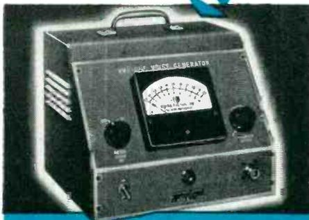
**TYPE 904 NOISE GENERATOR** — a direct reading noise source permits measurements of noise factors up to 20 db for r-f amplifiers and receivers operating in the range from 10 to 1000 mc/s. A T1-1 coaxial diode with a nominal input impedance of 50 ohms is used. VSWR is approximately 1.25, housed in hard-steel cabinet.
