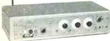
Dual use: high gain condenser-coupled amplifier, voltage gain of 10,000; or low gain direct-coupled amplifier, voltage gain of 250 by a flick of the switch. Records voltage, current characteristics; venous, arterial manometer pressure, vibration studies, electrocardiograms, etc.
