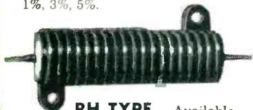
**RH TYPE** — Available in 25, 50 and 250 watt sizes. Silicone sealed in die-cast, black anodized radiator finned housing for maximum heat dissipation.
