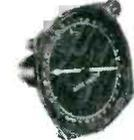
Fairchild Instrument. 5 inch 0 to 360 degree dial. 26 volts-400 cycles single phase. May be operated on 10 to 15 volts 60 cycles. Kollsman design. SA-284 ..... \$6.50 ea.
