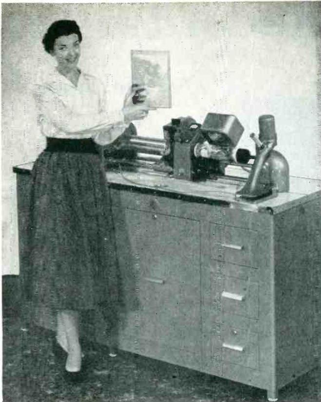
Console model of engraver, with operator holding finished plate. Flashing-lamp microscope is provided for examining dot-burning operation while machine is in operation. All amplifiers are underneath, along with a fireproof compartment for plates
