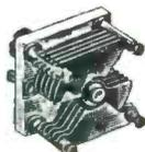
9-62 mmfd per section. 6-34 mmfd sections in series. Double ceramic end plates and bearings. 1/4" diam. shaft. 5/16" long. .065 Plate spacing end plates 1-3/8" square.
