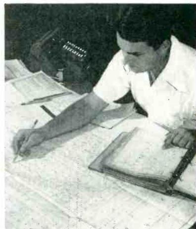
Checking availability of stock dies for tube socket holes in large rectifier chassis, at Brooklyn, N. Y. plant of Kay Metal Products Co. Prints of all available dies are filed in looseleaf notebooks like that in use here, for quick reference
