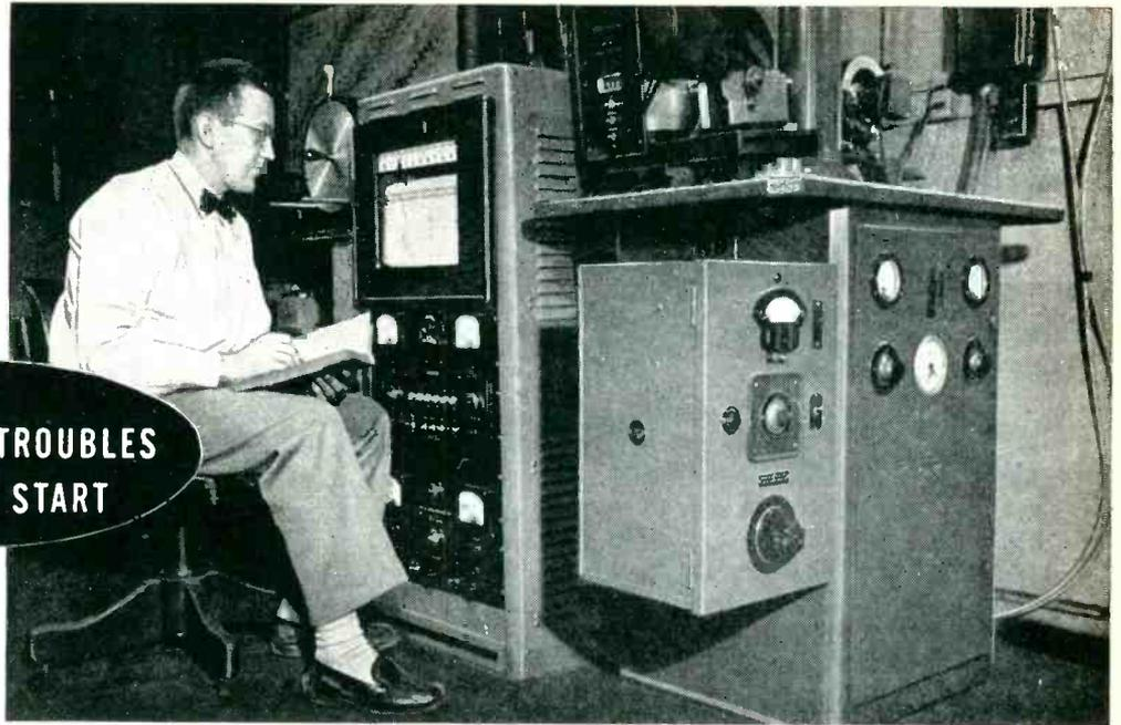
*X-ray diffraction equipment in the Mallory Contact Engineering Laboratory. It is so sensitive it will identify contaminating films of less than a hundredth of a micron.*
