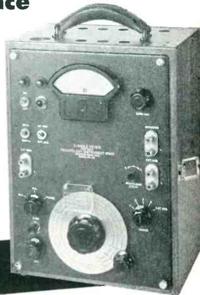
The type 310A Z-Angle Meter measures impedance directly in polar coordinates as an impedance magnitude in ohms and phase angle in degrees:  $Z/\theta$ . Impedance Range: .5 to 100,000 ohms, covered by a single dial and a four position range switch.
