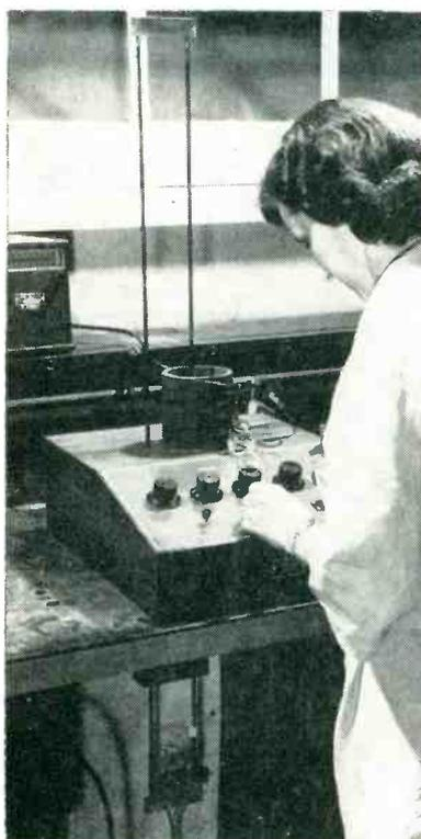
Checking large air-core coil with turns counter. Standard coil used for comparison is mounted within the control panel, where it is protected from damage
