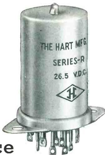
Rating for rating, "Diamond H" Series R hermetically sealed, miniature aircraft type 4PDT relays are smallest (1.6 cubic inches), lightest (3.76 ounces), have widest temperature range ( $-65^{\circ}$  to  $+200^{\circ}$ C.), greatest operating shock resistance (to 50 "G" and higher) and excel all others in their field in ability to break high currents and high voltages.
