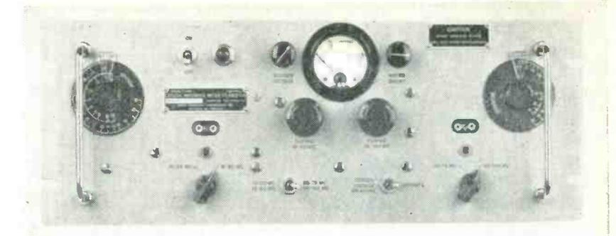
Front panel of newest addition to crystal-testing series, the TS-683/TSM. This is intended for the range of 10 mc to 75 mc, but has actually been calibrated up to 140 mc
