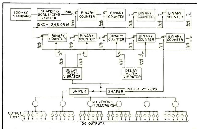
FIG. 3—Master timing system used to insure that time of each flash will be determinable to within 1 microsecond
