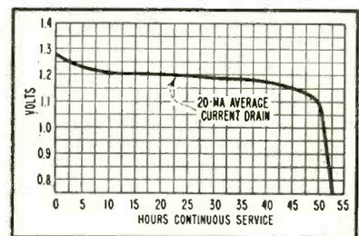
FIG. 2—Variation of potential with 20-ma drain of RM-1 cell
