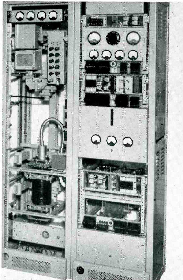
Part of repeater bay with traveling-wave tube mounted in its circuit
