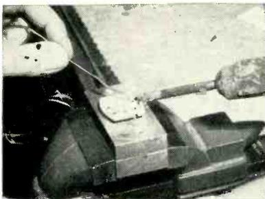
Soldering leads to end plate
