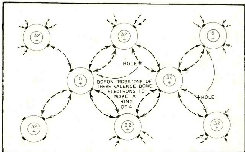
FIG. 6—Germanium crystal structure showing an atom of boron replacing one of germanium, adding an electron to its valence ring of 3 and forming covalent bonds with nearest neighbors. A hole is created in the valence bond where the "robbed" electron had been
