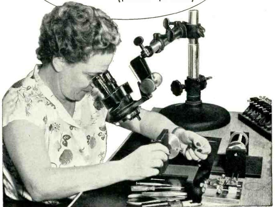
At the Hathaway Instrument Company, tiny galvanometer coils are wound with wire so fine that it is almost invisible to the unaided eye. Ingenious tooling and use of an AO Stereoscopic Microscope assure fast, precise workmanship.
