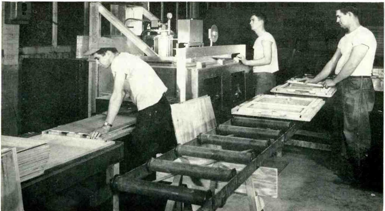
**CABINET WALL GLUING**—Glue used to join mounting blocks and other wood members to panels of television cabinet subassemblies are cured in about 15 seconds in this Westinghouse 10-kw installation. Man at right places blocks and strips in pallet-type positioning jig; outer panel is set over this after glue is applied
