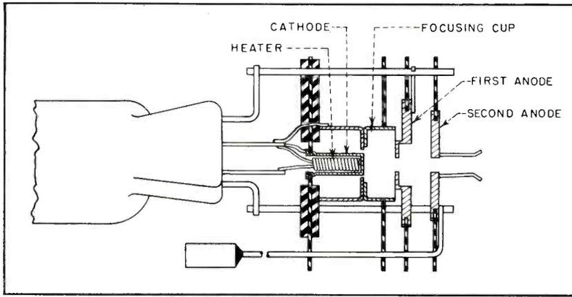
FIG. 4—Details of electron gun used in the traveling-wave tube
