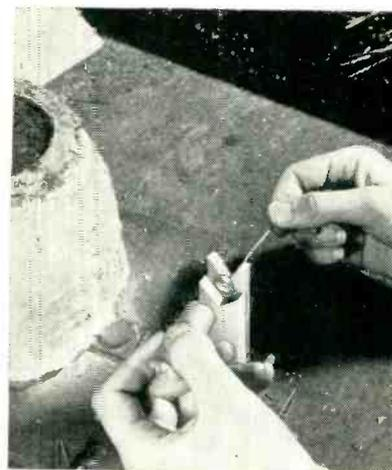
Method of pressing capacitor against pigtail held in jig
