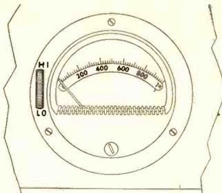
The Marion Multi-Dialer Model MD-1 shown here (ruggedized movement) is available with five self-contained ranges in volts, milliamperes, microamperes and amperes. It is also available custom-engineered to your end-product so that it may be installed on your panel and when appropriate scale is selected it will automatically insert the instrument with appropriate accessories into five separate measuring circuits and/or ranges in your equipment.
