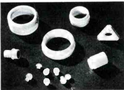
The precision insulating parts required for this electronic instrument are produced by the Tri Point Manufacturing Company of Brooklyn, N.Y. Tri Point uses rod and tubing extruded from Kel-F polymer and then machines the necessary parts on standard automatic screw machines. The ready machinability of Kel-F permits this company to maintain tolerances within .001" on all parts supplied to the Aviation Engineering Corporation of Woodside, N.Y., manufacturers of this aircraft instrument.
