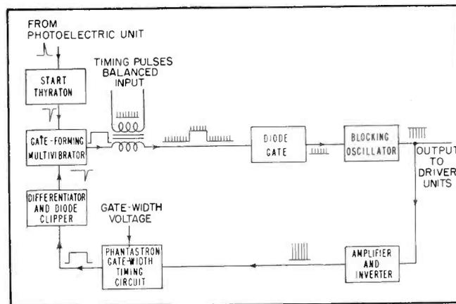
FIG. 6—Gating unit, showing timing signals on square-waves
