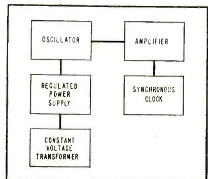
FIG. 2—Arrangement for calibrating oscillator
