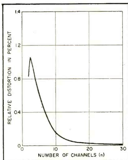
FIG. 5—Relative distortion versus number of channels for fourth-order terms
