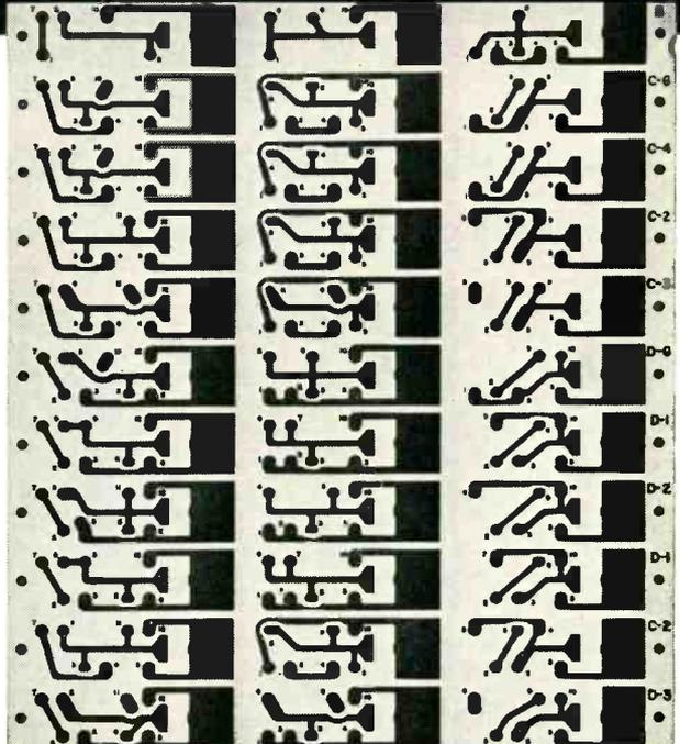
G-E Print-Wire circuit designed for radio turret tuning.
