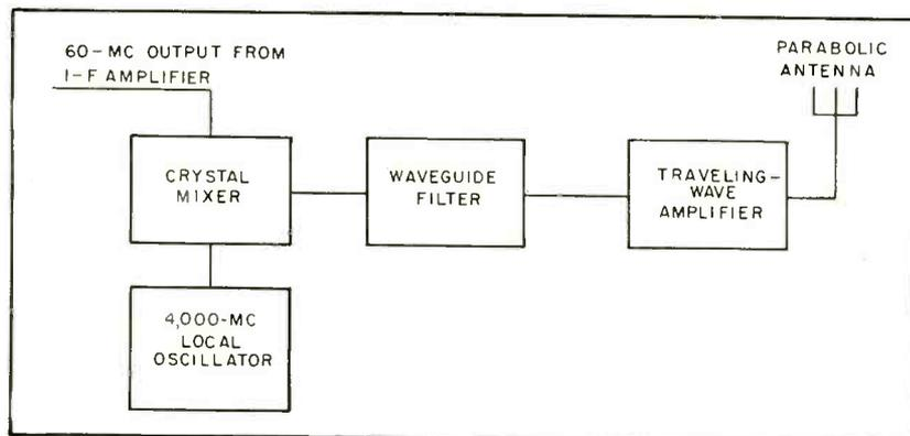
FIG. 1—Output stages of microwave repeater showing function of twt amplifier
