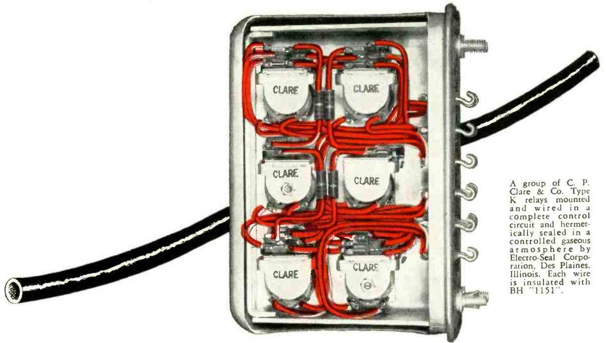
A group of C. P. Clare & Co. Type K relays mounted and wired in a complete control circuit and hermetically sealed in a controlled gaseous atmosphere by Electro-Seal Corporation, Des Plaines, Illinois. Each wire is insulated with BH "1151".
