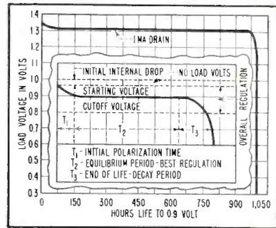
FIG. 1—RM cell load voltage vs time at constant load at 70 F. Inset, typical voltage regulation
