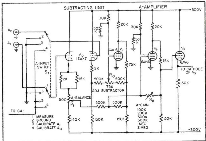
FIG. 2—Circuit determines voltage drop across probes on surface of semiconductor and provides amplified version for oscilloscope presentation
