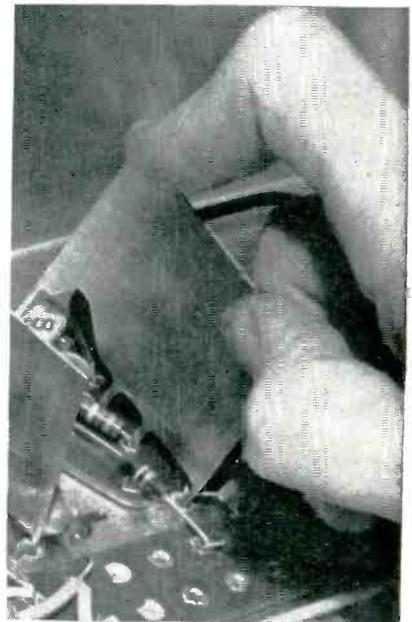
Tube socket shields have comb-like teeth that fit into ground pin holes for anchoring simultaneously with leads
