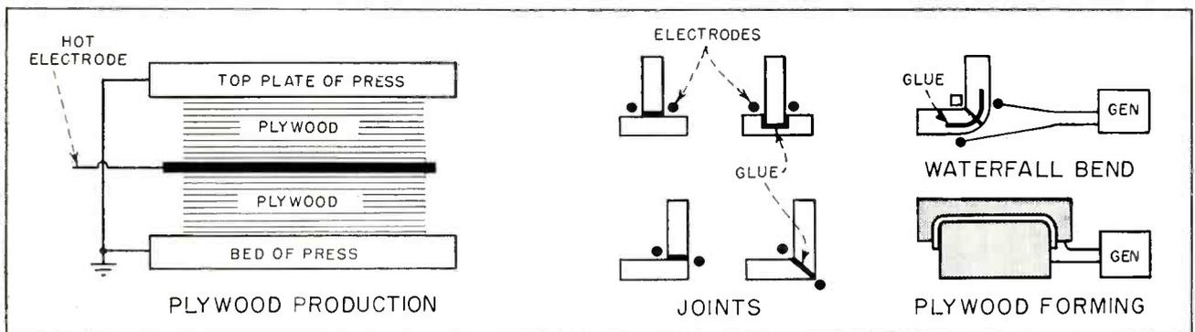
**FIG. 2**—Examples of electrode shapes and locations used for some of the commonest types of joints in wood materials
