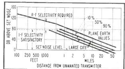
FIG. 1—Estimated intensity of unwanted signals at 150 mc for 100 watts radiated power
