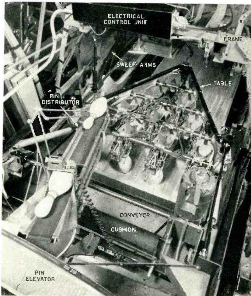
Major components of the automatic pinspotter. Electrical control unit determines proper operating cycles for sweep and table
