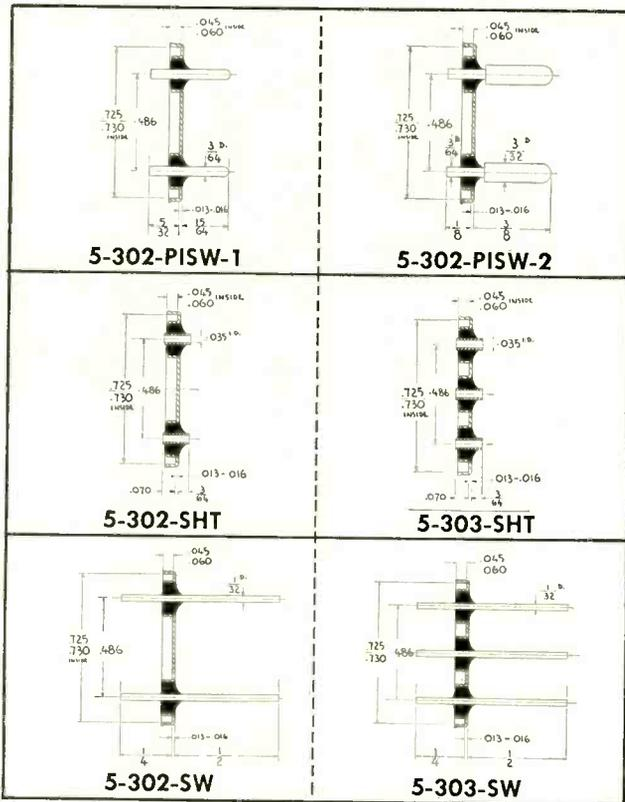
Fusite's design of Crystal Can Headers combines the ruggedness of a metal base with large size glass areas surrounding the electrodes, assuring a safe rating of 1500 V(RMS). Several of the terminals shown are available with attached crystal springs to your specification. They fit standard crystal cans. As an optional feature these terminals can be furnished with adjusting hole for thermostat applications.
