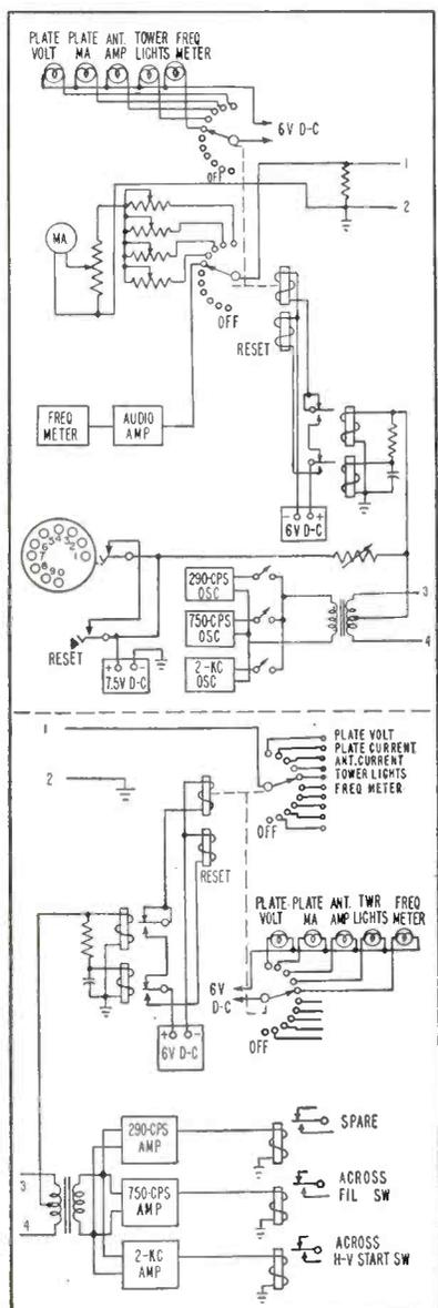
FIG. 2—Step control uses tones with stepping switch for monitoring
