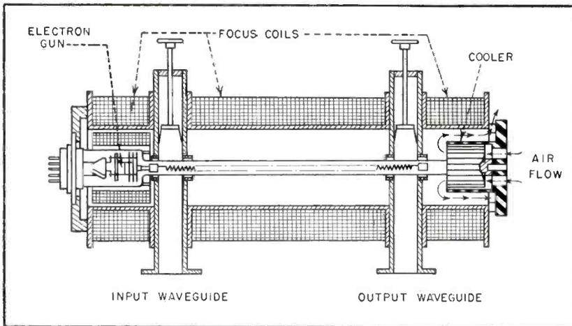
FIG. 2—Cutaway sketch showing traveling-wave tube connected in its circuit
