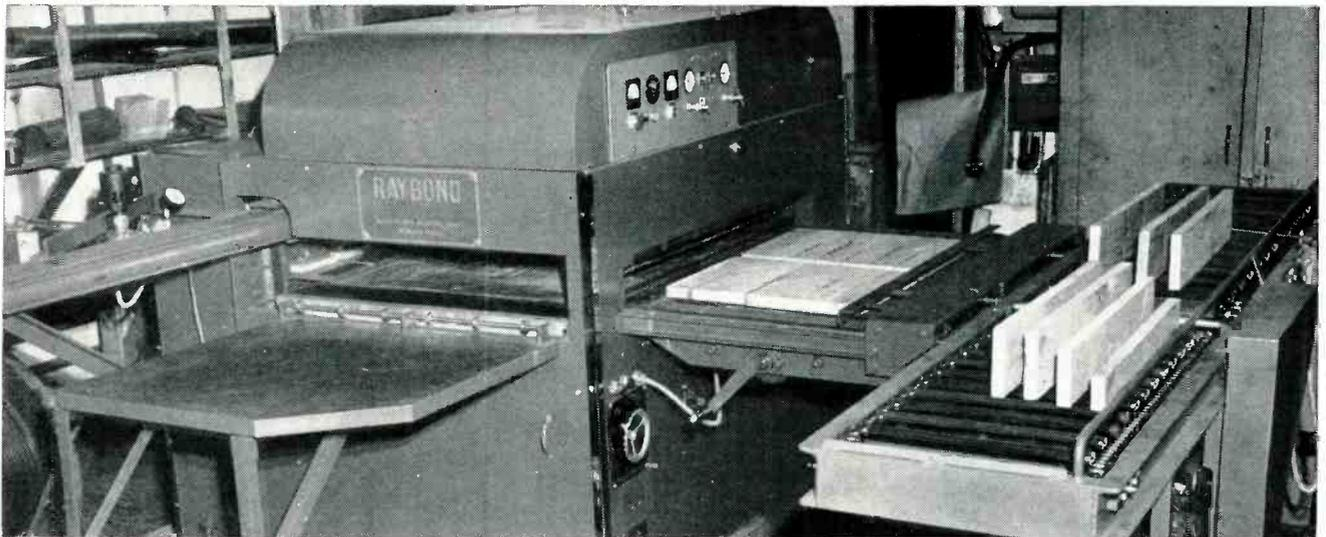
**PANEL EDGE GLUING**—One-man edge-gluing machine setup developed by Electronic Heating Corp. for producing large panels and core stock used in furniture. Glue is applied to edges of pieces by conveyor-type applicator at right, after which operator places them on bed of machine to start sequence of moving into press, applying pressure, heating for about 40 seconds, opening press and ejecting
