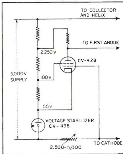
FIG. 5—Circuit used to stabilize twt cathode current
