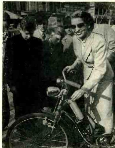
Germany gets set to tap the European bicycle market with this \$11.40 bike radio. Loudspeaker is built into the lamp housing. Two dry cells fit under the saddle
