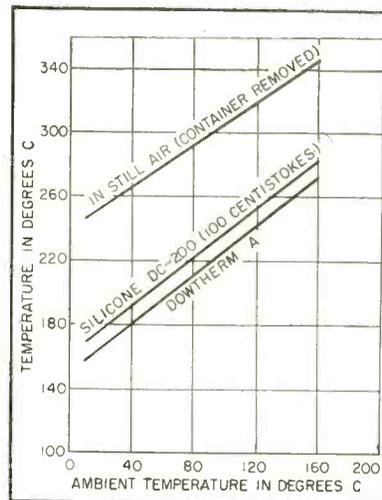
FIG. 4—Comparison of potting in two different fluids and in still air
