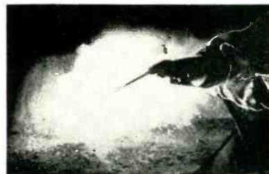
Burning through refractory material with new electric arc torch operating from standard welding generator
