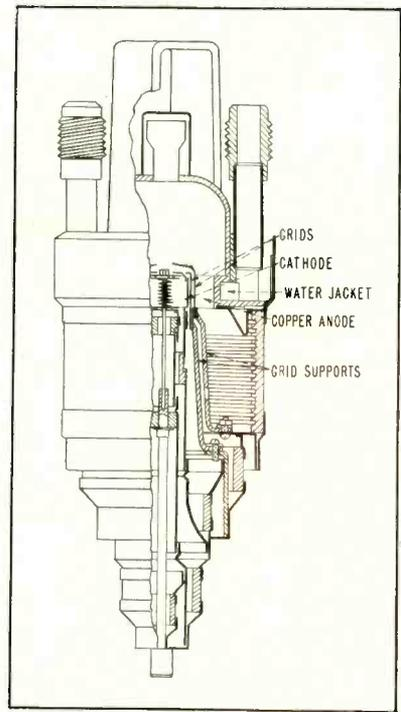
FIG. 2—Five-kw power output tetrode GL-6182
