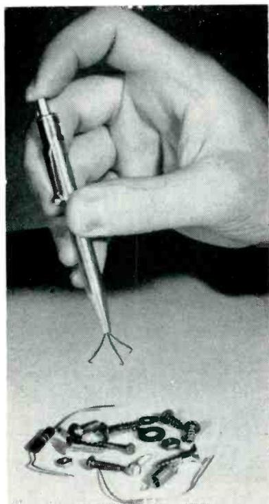
Depressing top plunger spreads pick-up fingers of stainless steel tool
