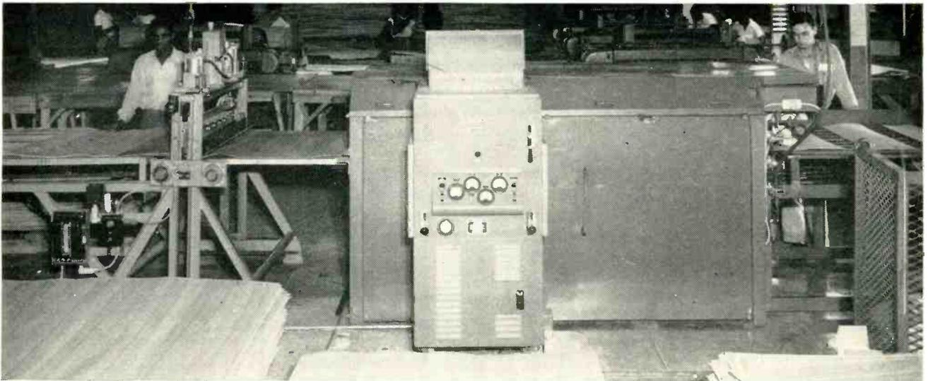
**VENEER EDGE GLUER**—Conveyor brings small sheets of veneer stock into machine at right, where rollers apply glue to edges and hold edges together during passage between electrodes of electronic generator. Continuous glued sheet emerging at 45 feet per minute is cut automatically into large sheets by air-operated clipper at left in this Northwest Syndicate, Inc. installation
