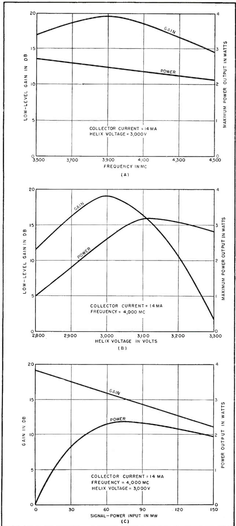
FIG. 3—Electrical characteristics of traveling-wave tube showing variation in gain
