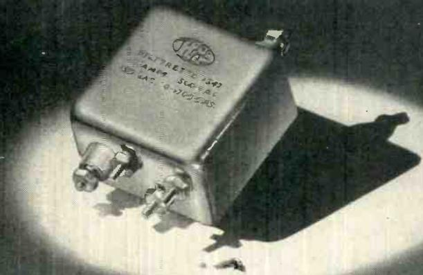
In a space only 2" x 2" x 1-3/16", you can get better than 86 db attenuation throughout most of the useful range up to 1000 megacycles by using any one of the #1547 series of Tobe interference filters. With their extremely low series resistance, these effective filters have negligible voltage drop and only slight temperature rise. Hermetically sealed, Series 1547 filters meet military specifications for use from 55C to +105C.
