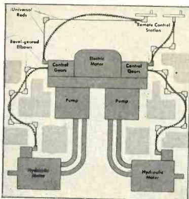
In fact, only 4 standard S.S. White flexible shafts were needed to replace the 35 parts that were formerly used. The flexible shaft system **cost 90% less, reduced assembly time and labor, eliminated alignment problems and provided 100% improved performance.** It's savings like
