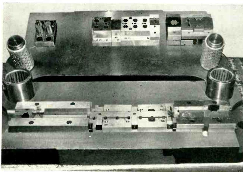
Top and bottom dies for producing integral-eyelet saddles for tube sockets. Aligning pins on upper die, surrounded by ball bearings, slide up and down in mating cylinders of lower die. Blank strip stock enters at right, and finished saddles are ejected at left, as indicated by strip shown below
