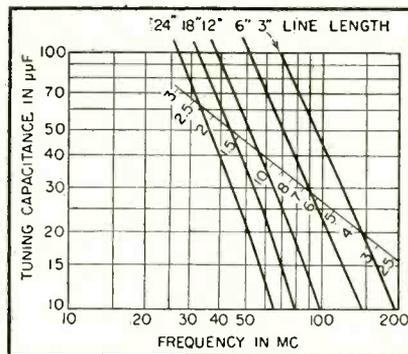
FIG. 3—Chart for shorted quarter-wave tuned parallel line having a characteristic impedance of 157 ohms. Diagonal overlay scale shows logarithmic spacing of curves
