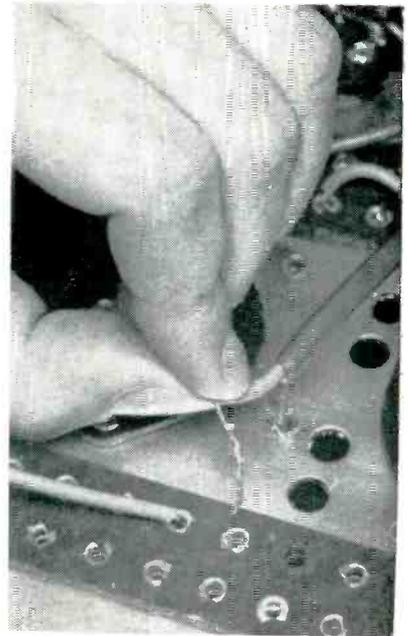
Method of inserting shielded wiring in pin strip. Braided shield has already been pushed into a ground pin
