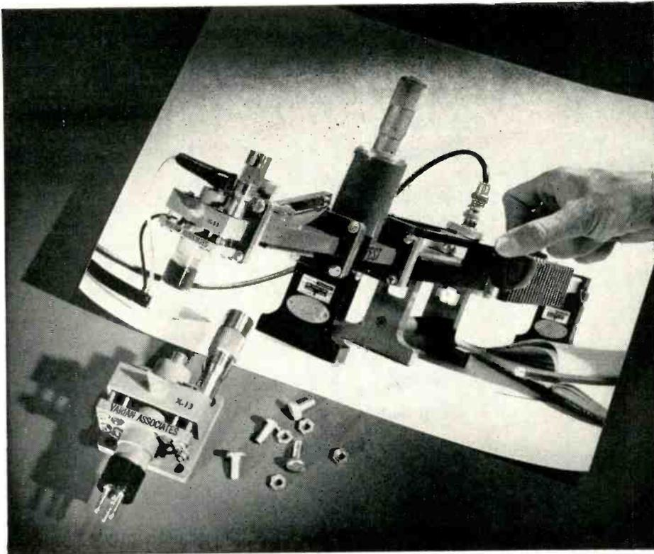
**IN LABORATORIES** throughout the electronic field, the Varian X-13 Klystron is widely used as a general-purpose x-band signal source. In the typical setup above (checking load reflection), note the compactness, the convenience of connection, and the way the tube bolts directly to the waveguide.
