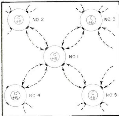
FIG. 3—Covalent bond structure in a tetraivalent atom lattice. Such valence bonds may involve atoms of carbon (diamond), germanium and silicon, among others. Note how each electron is bound by valence bond and not free to take part in conduction process
