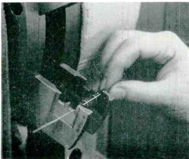
Loading molded paper capacitor on one of the eight pairs of die blocks of the ferris-wheel lead former and cutter
