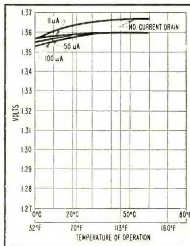
FIG. 5—EMF vs temperature at light loads
