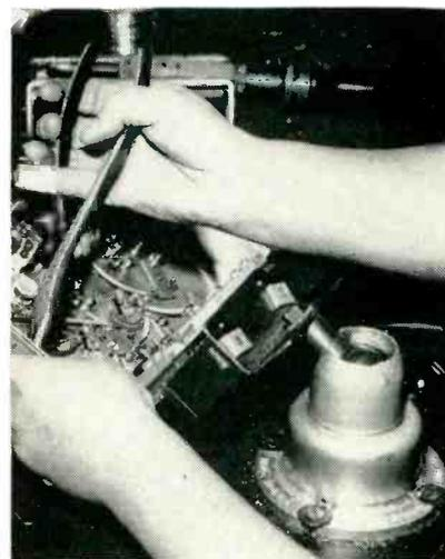
Type of holder used for gripping side of chassis. A screwdriver is required for inserting and removing a chassis. This setup is sufficiently rigid for heavy soldering and assembly work
