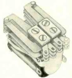
Newly developed MJ miniature telephone type relay features longer and more flexible contact arms which result in a lower spring load rate. This structure permits wider contact gap, more overtravel, improvement in sensitivity, faster action and longer life. MJ supplied open or hermetically sealed, with maximum of 12 contact springs, for either DC or 60 cycle AC operation.
