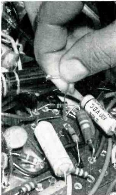
Inserting lead of molded paper capacitor in pin that already has three leads. Four leads are limit for easy insertion
