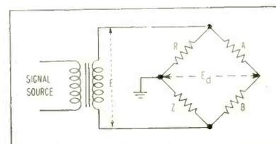
FIG. 2—Simple bridge circuit shows derivation of voltage  $E_d$
