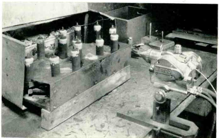
Setup for spraying molten copper on ends of rotating resistors. Gear drives for the resistors are under the metal housing
