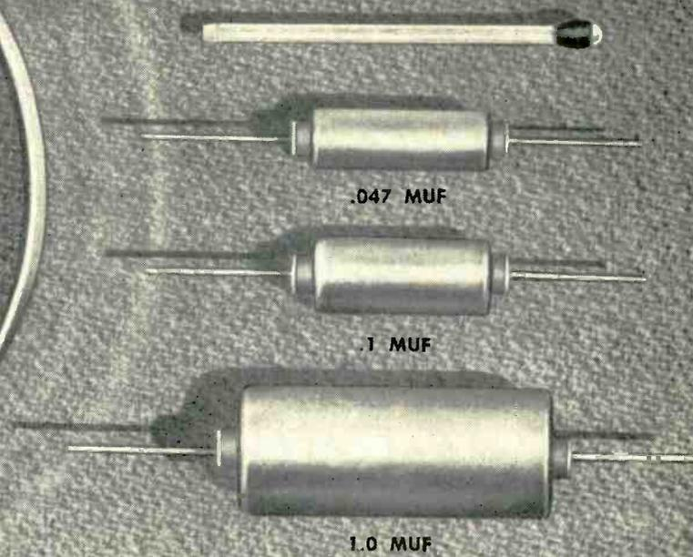
**SMALL SIZE** graphically shown by these actual G-E subminiature capacitors compared with a common match. Cut-away view, about 1½ times actual size, shows features.
