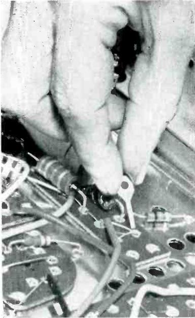
Inserting punched copper strip in pin to which a lead of an above-chassis component must be soldered later
