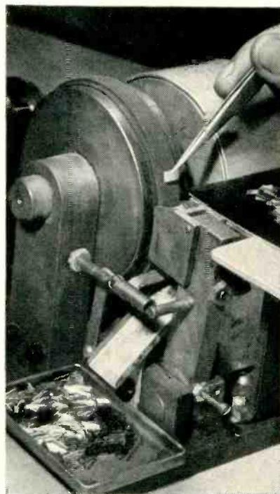
Dropping flat piece into sleeve-rolling machine. Finished sleeves drop into tray at lower left
