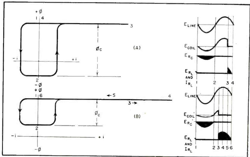
FIG. 3—Voltage waveforms and flux-current curves show effect of variation in control resistance on output
