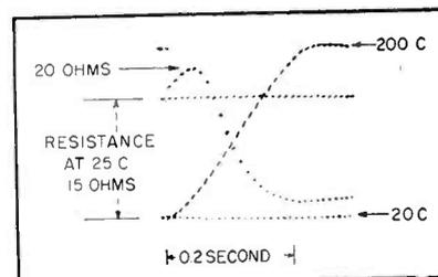
FIG. 9—Tracing of typical oscillogram of resistance-temperature characteristic for germanium sample
