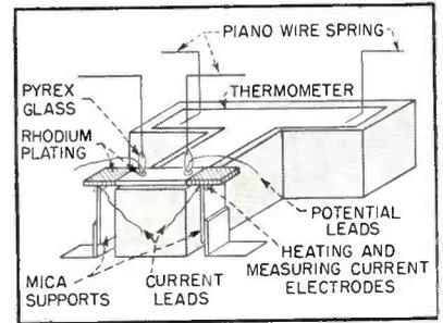
FIG. 6—Specimen holder design is largely responsible for versatility of bulk semiconductor resistance-temperature characteristic equipment
