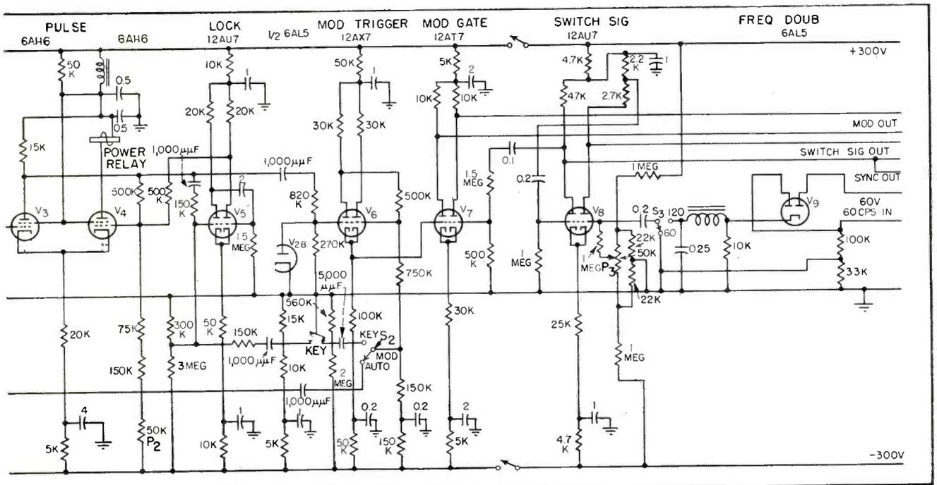
determines length of current pulse that is passed through semiconductor specimen to heat it to the desired temperature
