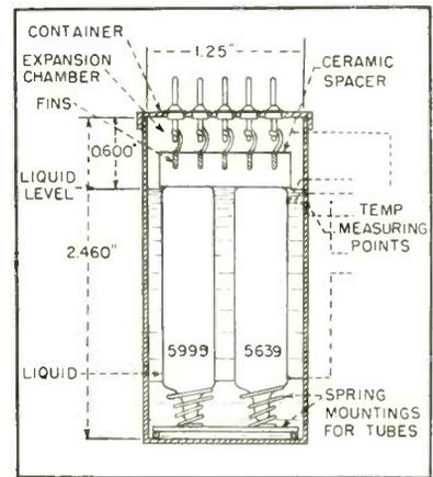
FIG. 2—Cross-section of potted unit with tubes in place
