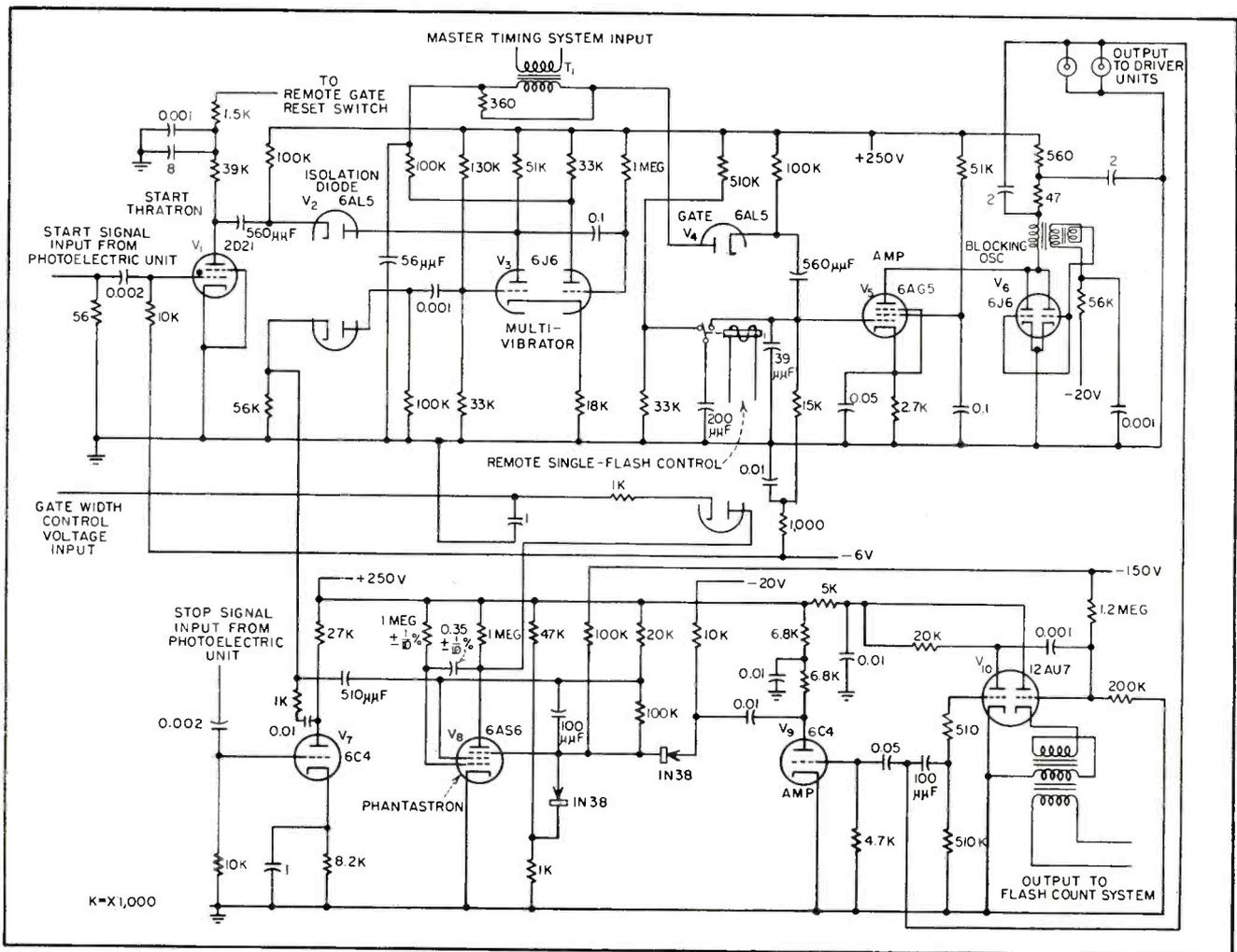
FIG. 7—Circuit of gating unit used to pass timing signals only when rocket is in camera range
