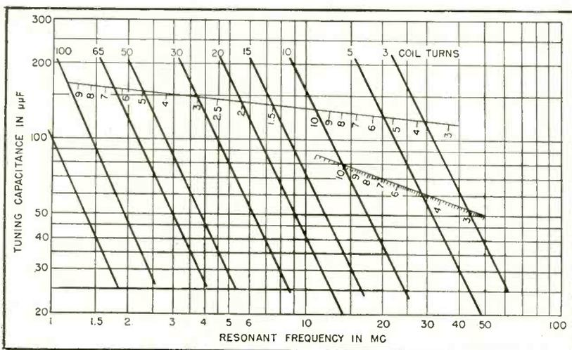
FIG. 1—Example of graphical design procedure for a coil 1 inch in diameter and 1½ inches long, with various numbers of turns spaced to fill entire length. Accuracy is excellent up to approximately 200 mc as method takes into account distributed capacitance and other sources of error usually neglected because of calculation difficulty. Charts for other coils can be prepared after a few simple measurements
