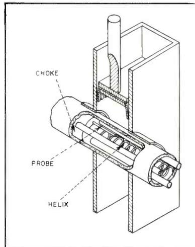
FIG. 6—Method for coupling waveguide to twt helix
