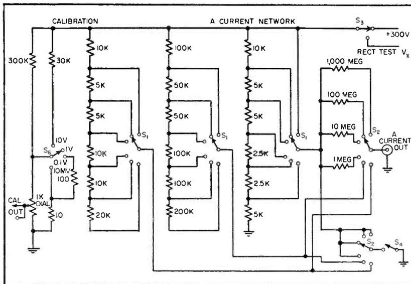
FIG. 7—Calibrator circuit. Precision resistors are selected by  $S_1$ .
