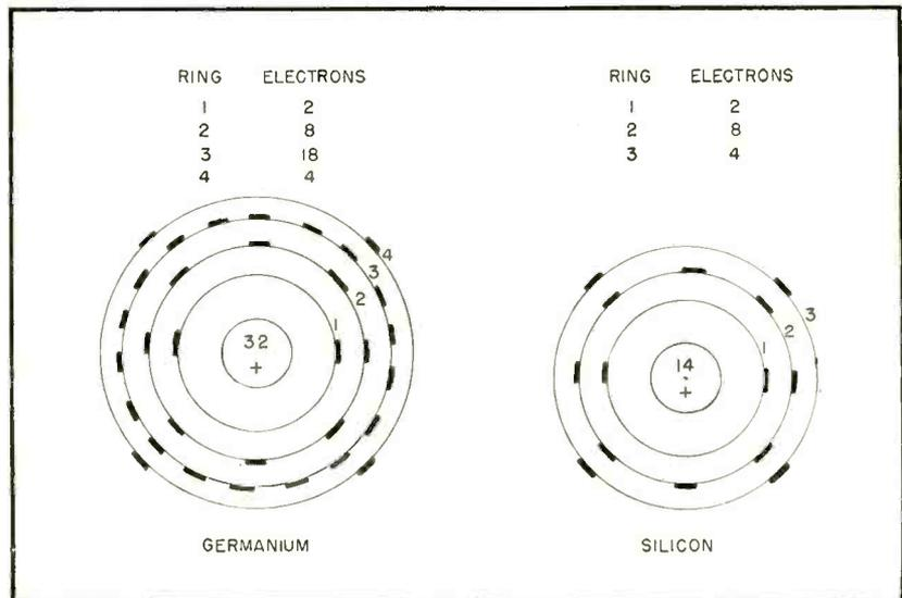
FIG. 1—Schematic representation of germanium and silicon atoms shows electron rings surrounding nucleus. Note the 2-8-18-4 arrangement for Ge and 2-8-4 arrangement for Si. First three rings for Ge and first two for Si are complete rings.
