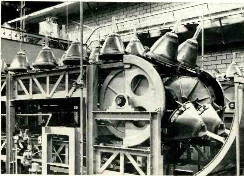
Screen-settling machine begins to roll as . . .
