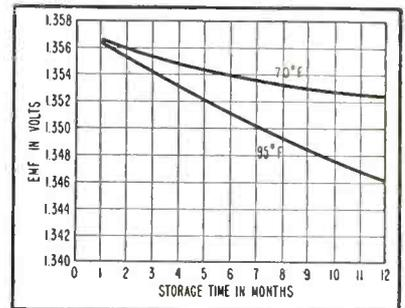
FIG. 3—EMF vs storage time at two temperatures
