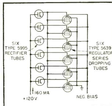
**FIG. 1—Schematic diagram of subassembly used in potting tests**
