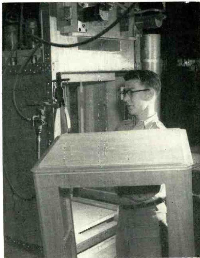
**JOINTS**—Air-operated press and Westinghouse high-frequency generator equipment for setting glue in joints of entire television receiver console cabinet in one two-minute operation
