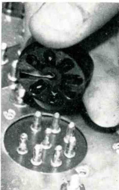
One of the molded adapters developed for use with special dip-soldered tube sockets. Projecting leads are sheared off before adapter is pushed on
