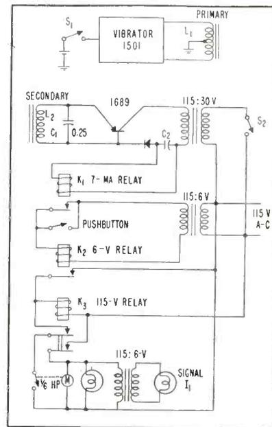
FIG. 2—Transistor-controlled automatic garage door mechanism
