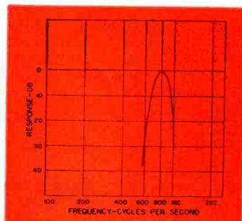
This 600 ohm miniaturized 1 KC band pass filter is housed in a case only 1" x 1 3/4" x 2 1/2".
