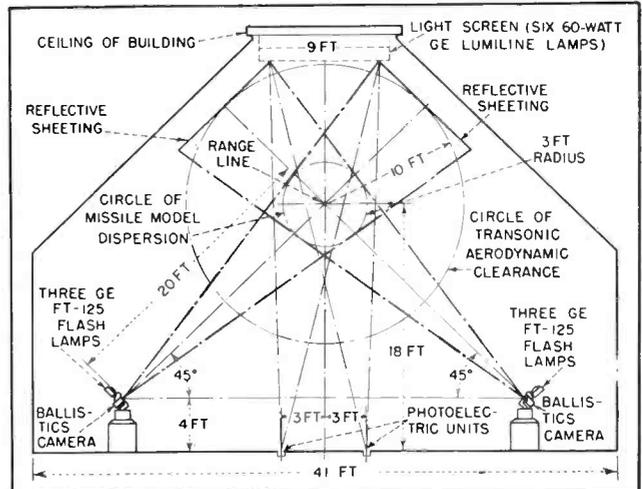
FIG. 2—Cross-section of range, showing one pair of cameras with lamp banks
