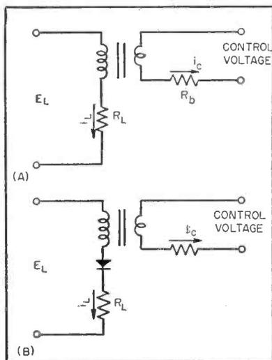
FIG. 1—Simple saturable reactor and self-saturating magnetic amplifier circuits
