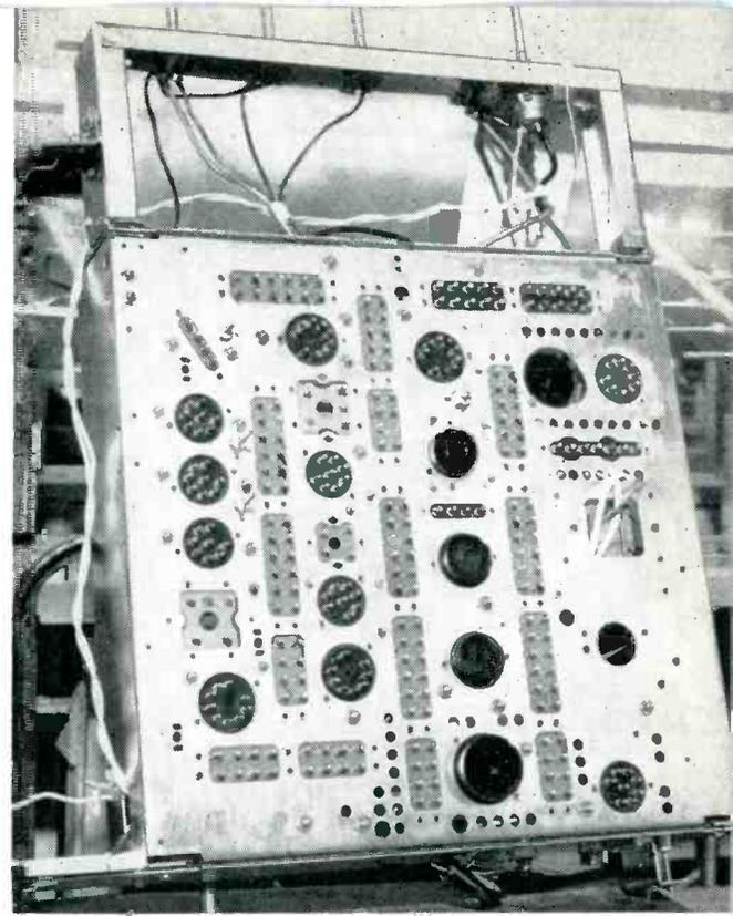
Appearance of top of television receiver chassis after dip-soldering of the 424 pin-type terminals having over 1,000 individual leads. Socket adapters are added after soldering
