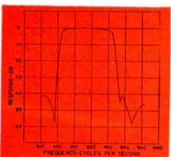
This band pass filter is designed for sharp cut-off at both ends of the range ... 10,000 ohms ... case dimensions 1 3/8" x 2 1/2" x 3 1/4".
