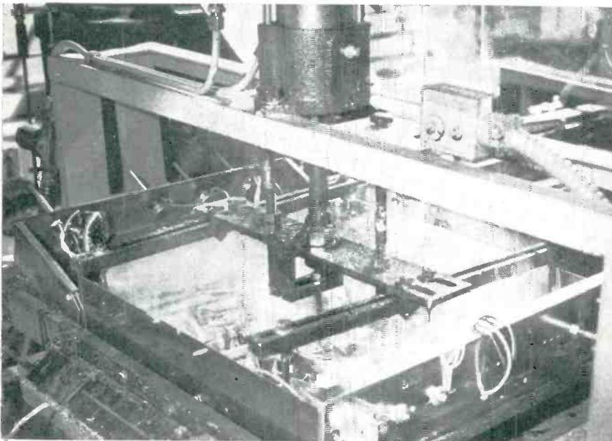
Television chassis in solder pool of machine, with rosin fumes rising in clouds. Air cylinder at top counteracts bellying of chassis with heat by lowering rods that hold chassis firmly down on bars projecting slightly above surface of solder pool
