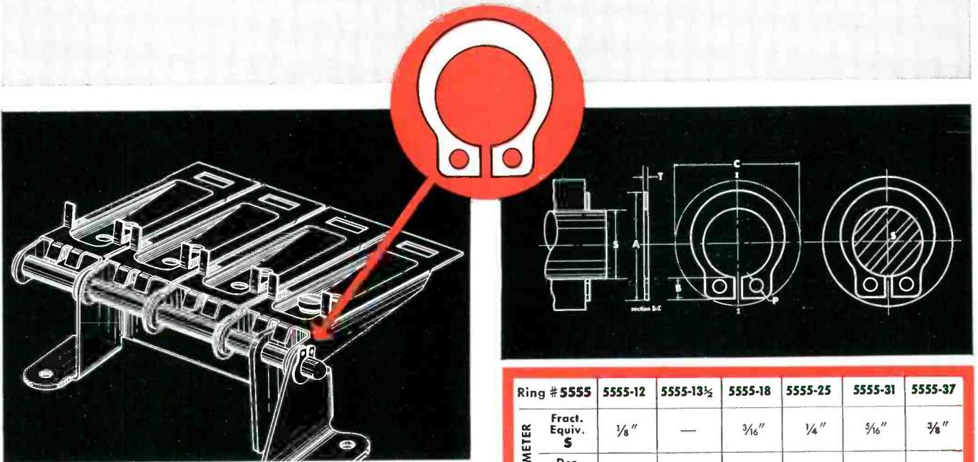
The Waldes Truarc Grip Ring is a new, low cost fastener that provides a positioning shoulder secure against moderate thrusts or vibration. Installed on a straight ungrooved shaft, the Truarc Grip Ring can be assembled and disassembled in either direction with Truarc pliers.
