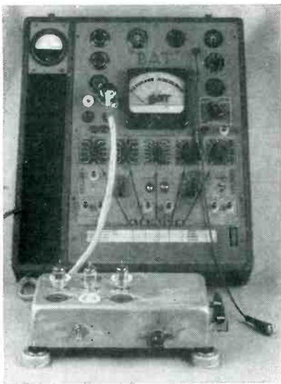
Method of connecting adapter to standard tube tester with cable and plug. This unit has three each of three different types of sockets (4-pin, octal and 7-pin miniature), to permit warming up two tubes while one is being tested
