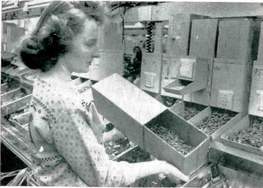
Parts boxes like these are placed under lead-forming machines for loading, and fit directly into metal dispensing bins on main assembly line. Elimination of handling operations insures that leads will be correctly bent for dropping into chassis pin holes
