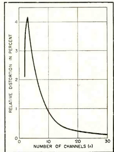
**FIG. 4—Relative distortion versus number of channels for third-order terms**
