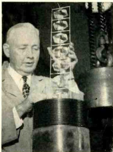
Batch of 11 perfect 160-gram quartz crystals being unloaded by A. C. Walker after growing 48 days in 4-foot autoclave at Bell Telephone Labs in Murray Hill, N. J. Threaded cap is removed with huge wrench and chain hoist, after which welded-steel inner liner is sawed open. Project is sponsored by Signal Corps Engineering Labs of Fort Monmouth
