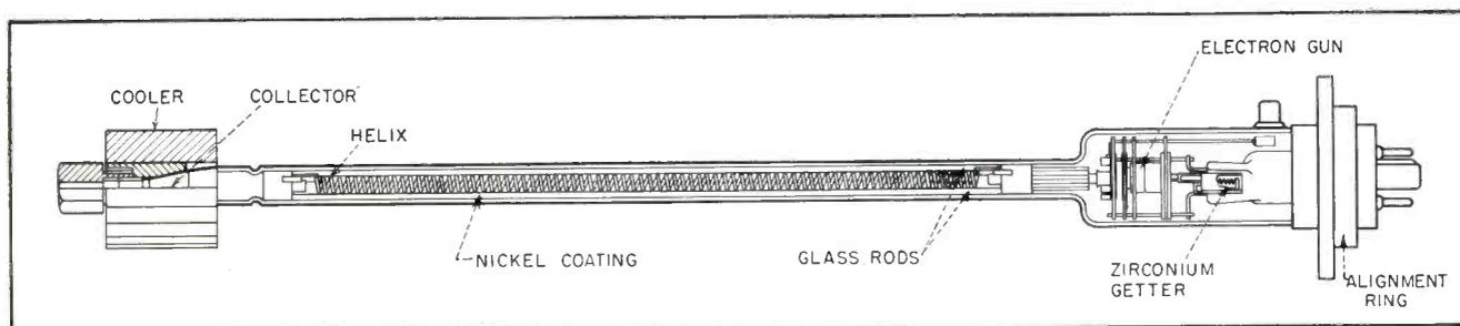
Principal features of traveling-wave tube, type CV-2188
