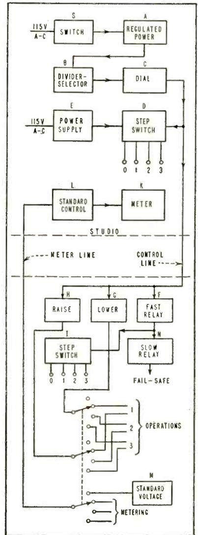
FIG. 1—Remote control provides for raising and lowering functions, as in tuning final stage
