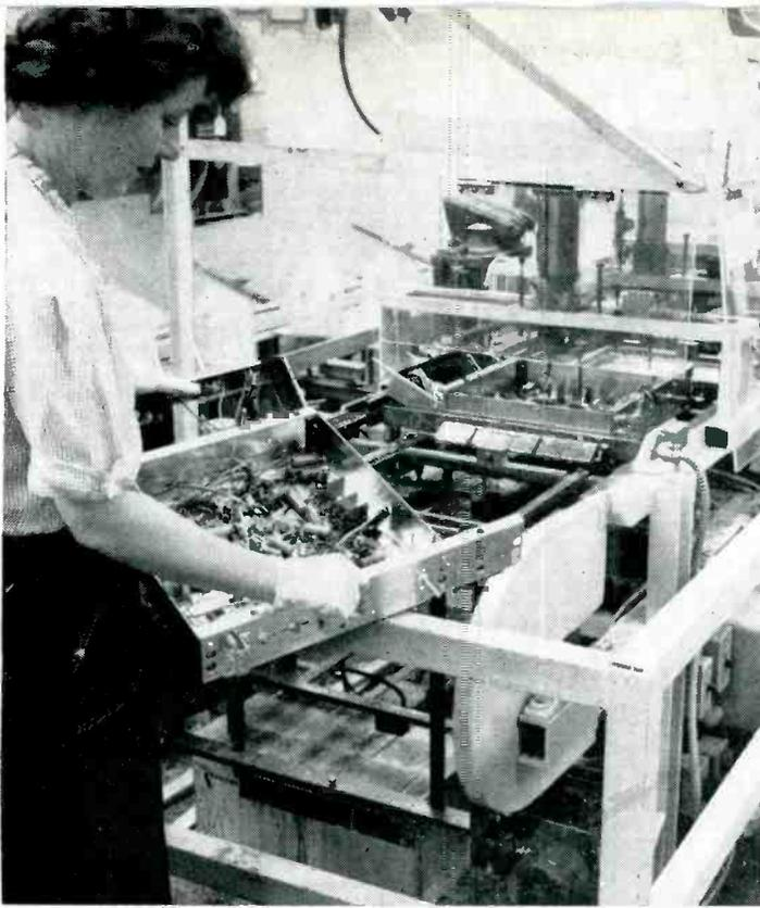
Loading chassis onto conveyor of dip-soldering machine for television assembly line. Hood with Lucite draws off rosin fumes, keeping them entirely away from workers
