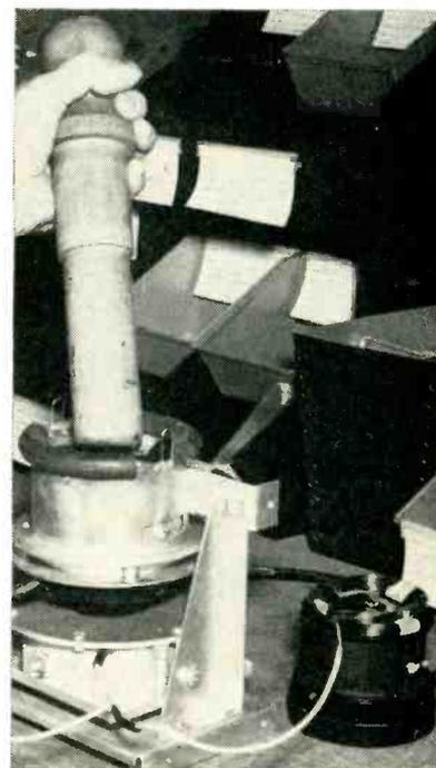
Wood rod used to keep dirt out of completed yoke assembly during testing of individual coils
