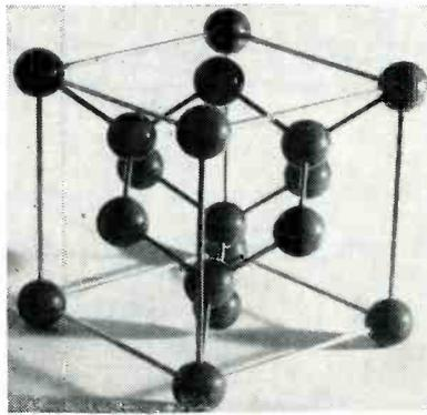
FIG. 7—A three-dimensional representation of the crystal lattice of germanium. Note the hexagonal arrangement of the atoms. Corner atoms are considered as shared by eight similar cubical crystals with a common vertex, and the total contribution of all the corner atoms to a unit crystal is one atom. Crystal refers to the entire cubical structure; lattice refers to the arrangement of atoms within the crystal volume
