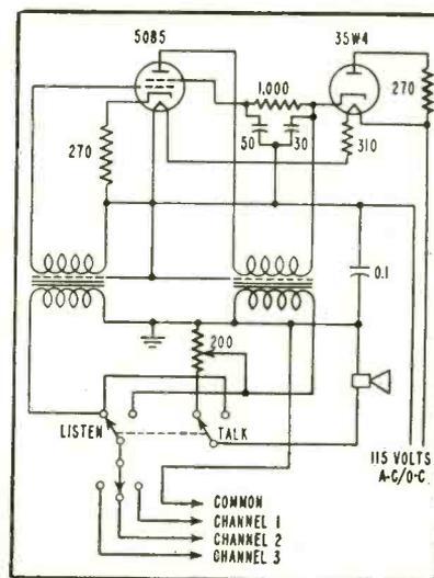
FIG. 1—Circuit of split-amplifier unit of a low-noise intercommunication system
