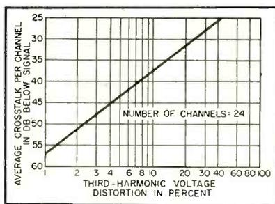
FIG. 8—Average crosstalk per channel versus third-harmonic voltage distortion
