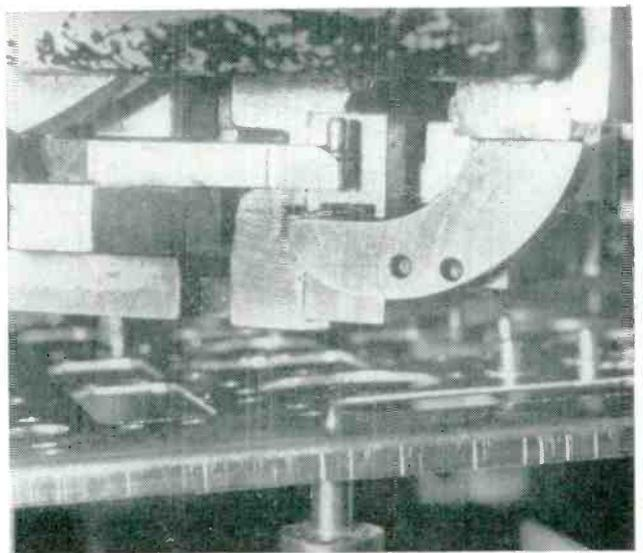
After ground riveter pushes tubular pin through cupped washer, upper anvil retracts and pin is pushed through chassis onto pointed anvil
