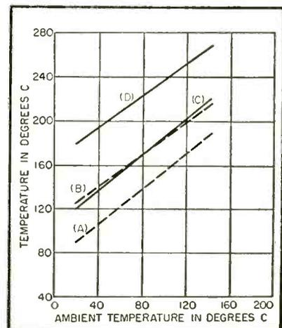
FIG. 3—Temperature chart for type 5639 tube in potted unit. Liquid temperature with heaters on (A), liquid temperature with heaters and plate power on (B), temperatures of tube base with heater on (C) and with heater and plate on (D)
