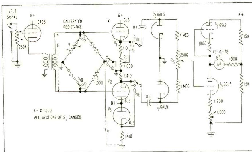
FIG. 1—Circuit of the bridge, balanced rectifier and indicator. To save space in actual equipment, phase and calibrated resistance are mounted coaxially
