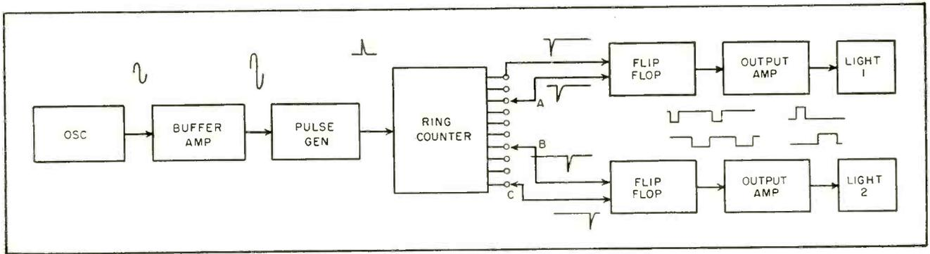
FIG. 1—Block diagram of binocular stimulator showing pulse lengths and phase relationships of signals in two separate output channels. Ring counter gives single negative pulses on successive output taps
