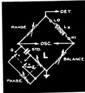
RESISTANCE, CAPACITANCE, INDUCTANCE and power factor are measured quickly and accurately on this Marconi engineered instrument.
