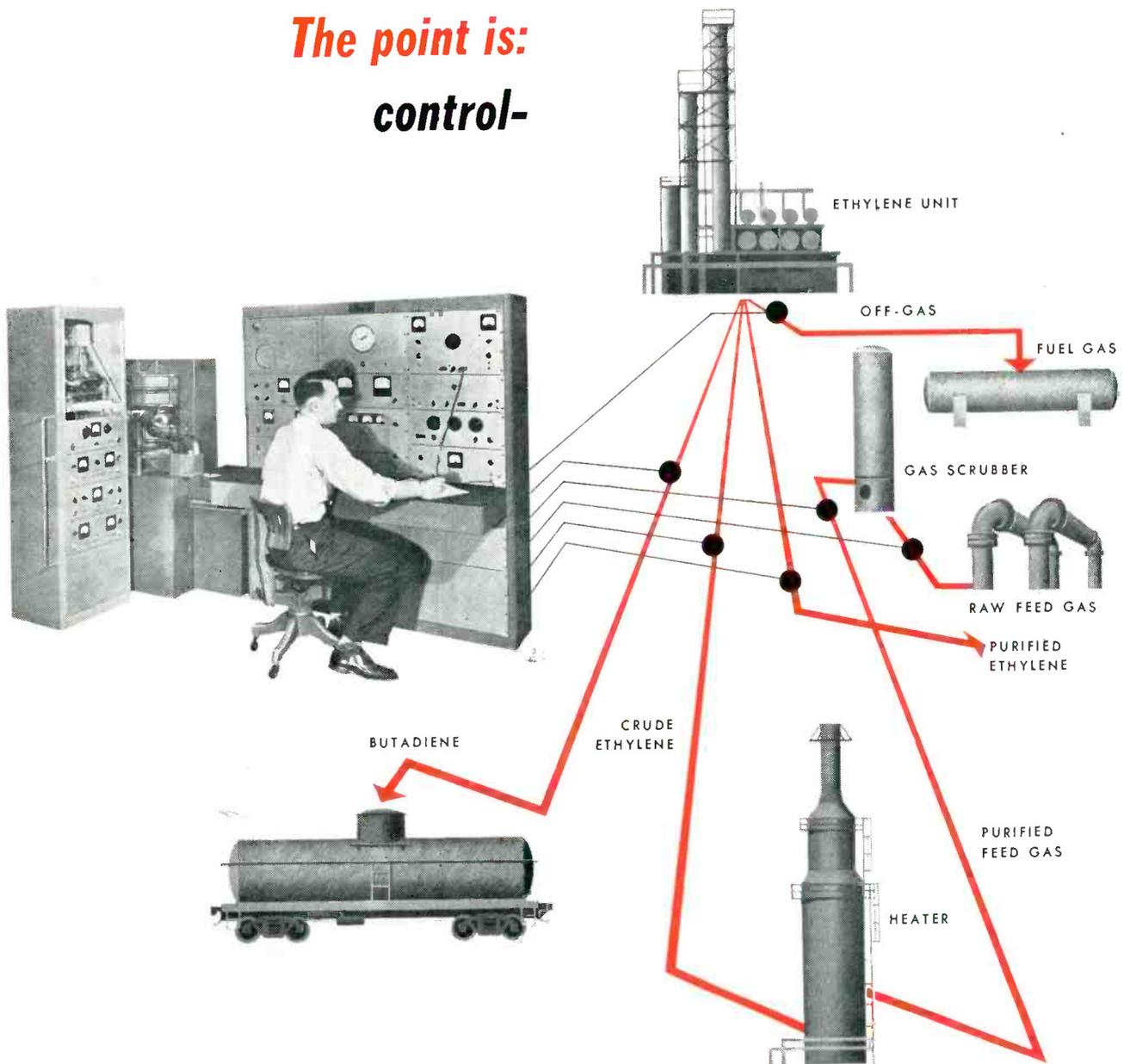
IN THE huge Texas plant of Jefferson Chemical Company, Inc., at Port Neches, Texas, approximately 50,000 complex control analyses of hydrocarbon mixtures have been made on a single Consolidated Analytical Mass Spectrometer since 1947. These figures indicate the speed, accuracy, and trouble-free service that can be built into a sensitive analytical instrument. For year-in, year-
