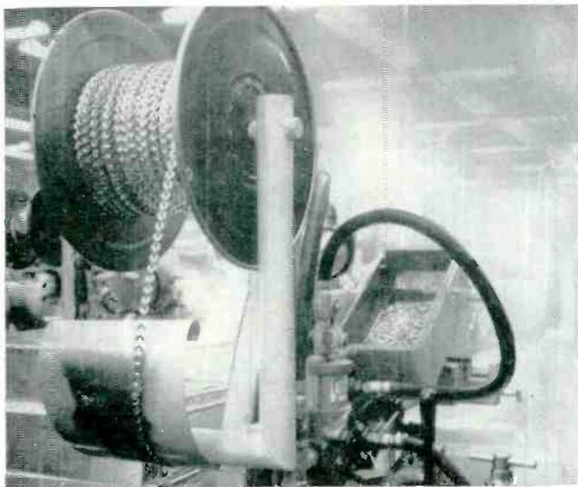
Rear of ground riveter, showing spring-steel washers in strip form and oscillating hopper for aligning terminal pins and feeding them down slide to chassis hole
