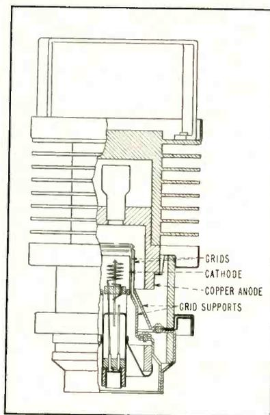
FIG. 1—Cut-away view of GL-6283, 250-watt uhf driver
