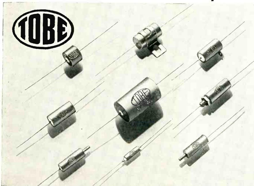
**For miniaturized apparatus** and where the self-healing characteristic is desirable, specify Tobe metallized-paper glass-terminal tubulars. Capacitance ratings from 0.01 to 10 mfd. Voltage ratings from 150 to 600 volts d-c. Mineral-wax or mineral-oil impregnation for temperatures  $-55$  to  $+85^{\circ}\text{C}$ ; silicone-fluid impregnation for  $-55$  to  $+105^{\circ}\text{C}$  range.
