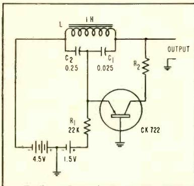
FIG. 1—Transistor oscillator suitable for fixed-frequency audio source, using two-terminal inductance
