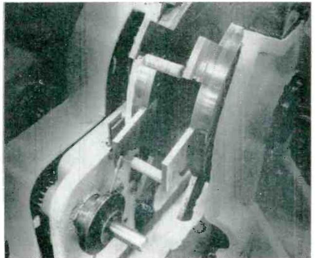
Rotating arm at rear, geared to main drive of ferris wheel, pushes processed components out of die blocks to chute below
