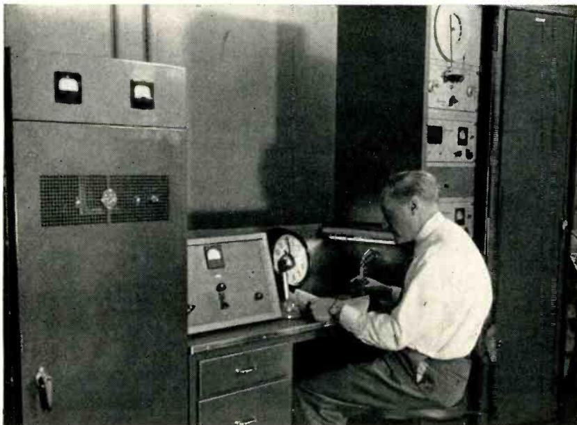
Forecaster at La Guardia Field reads latest information onto magnetic tape (right) which repeats five-sector forecasts endlessly via relay transmitter (left) until next hourly forecast is recorded. Main transmitter in Manhattan broadcasts data on 162.55 mc from 6 am to 6 pm, KW035
