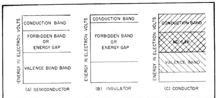
FIG. 4—Energy level diagrams show differentiation of semiconductors, insulators and conductors by presence and width of various bands
