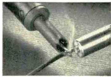
Solder right up to the bushing with G-E Silicone end seal—no danger of cracking glass.
