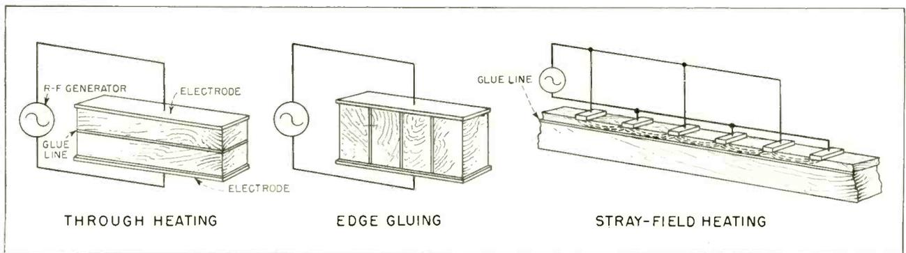
**FIG. 1**—Three basic production techniques employed by woodworking industry for electronic curing of glue lines
