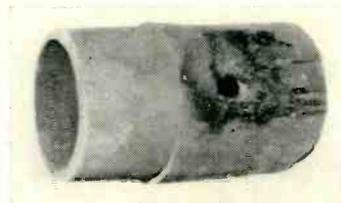
Example of hole made in ceramic bushing with arc torch
