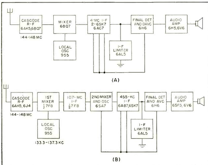
FIG. 2—Limiting circuit has been successfully used in civil defense receivers using both single and double conversion arrangements
