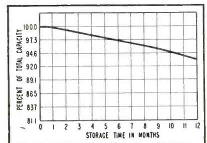
FIG. 4—Percent total capacity vs storage time at 70 F
