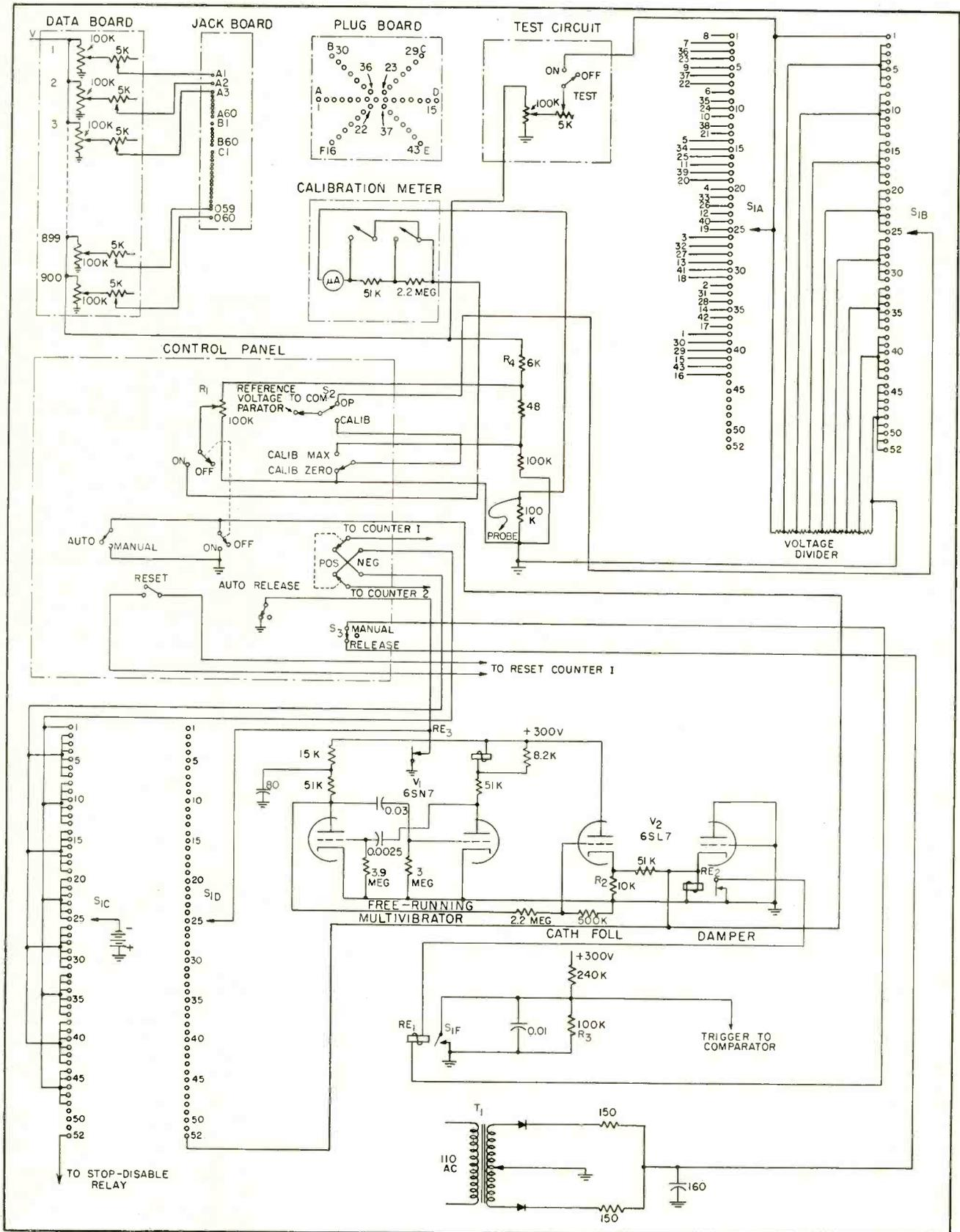
FIG. 1—Stepping switch in control unit governs analog multiplication of initial data values by proper coefficients. Free-running multi-vibrator is basic timing unit
