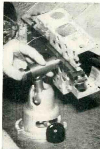
Indexing-type chassis-holding fixture. By pushing end of shaft against spring action as shown, operator can rotate entire chassis to desired new position. Crossbar in shaft drops into slots in outer sleeve of fixture to give rigid locking when thumb is released
