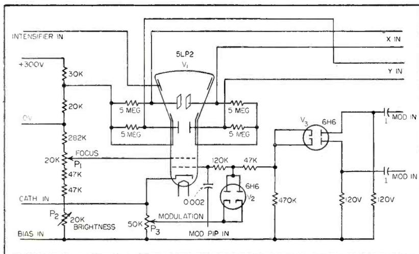
FIG. 8—Schematic diagram of display unit
