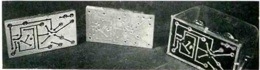
Examples of the three major steps in producing circuit wiring by metallizing. Left—adhesive mask applied to dielectric panel after insertion of eyelets. Center—appearance of masked panel after metallizing. Right—completed amplifier unit after stripping of mask, assembly of components and mounting
