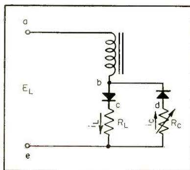
FIG. 2—Magnetic amplifier with reset control. The core is reset by current flowing through  $R_c$  during each half cycle when load current is blocked by rectifier in series with load
