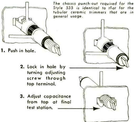
The chassis punch-out required for the Style 535 is identical to that for the tubular ceramic trimmers that are in general usage.
