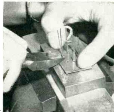
Use of spacer sheet as guide for cutting leads at other end of group to final length. Heat-absorbing brass block is divided into two parts so it can be removed after soldering is completed. Finished end plate rests in hole in wood jig clamped in vise
