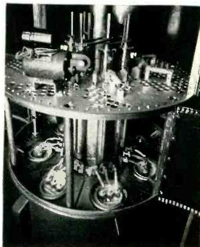
Power output of any current 5-kw vhf transmitter can be stepped up to either 25 or 20 kw, depending on the channel, with this RCA vhf conversion amplifier. The equipment consists of aural and visual power amplifier and blower units, aural and visual power supply and filter units, aural and visual control units, vestigial side-band filter and other accessories
