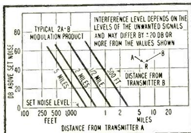
FIG. 2—Estimated intermodulation interference generated in mobile receiver at 150 mc for 100 watts radiated power
