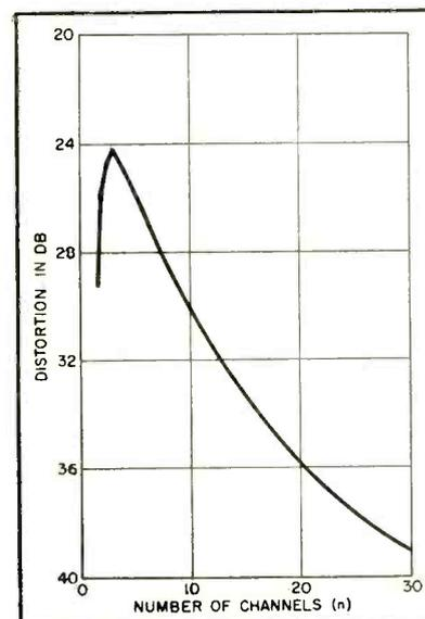
FIG. 7—Distortion falling within an octave and due to third-order terms
