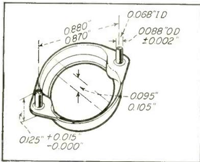
Dimensions of finished saddle having integral eyelets
