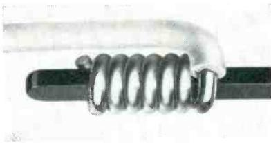
Example of finished solderless wrapped connection on rectangular terminal
