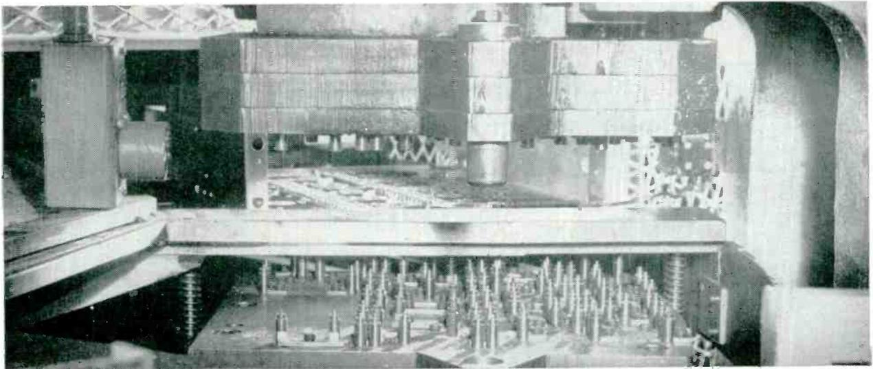
Riveter dies do work of 93 individual riveting machines in one stroke. Phototube at left stops press if chassis is missing
