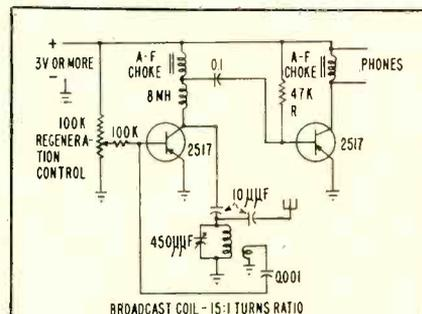
THE CIRCUIT of the receiver shown above is self-explanatory. It should be noted, however, that not all of the available type 2N517 transistors will oscillate up to the top of the broadcast band.
