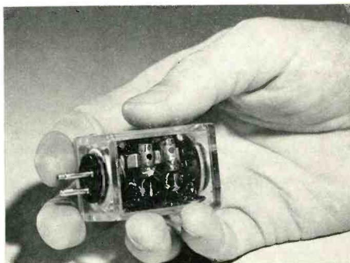
The tiny amplifier shown has the distinction of being among the first transistorized devices to be produced in quantity. Designed and manufactured by Sapan Engineering Co. for Bell Laboratories, the amplifier uses two point-contact transistors and provides 30 to 40 db gain when inserted in a high-impedance line such as a microphone cable. Several hundred of these units will be manufactured for demonstration purposes
