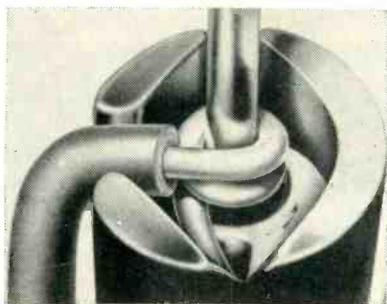
Muzzle of wiring tool, showing appearance of connection at the instant when two turns have been wrapped around terminal by rotation of the inner spindle in the direction shown by the curved arrow
