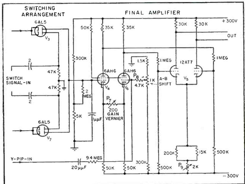
FIG. 3—Switching circuit alternately samples specimen resistance signal produced by circuit of Fig. 2 and signal from gold film resistance thermometer circuit (Fig. 5)
