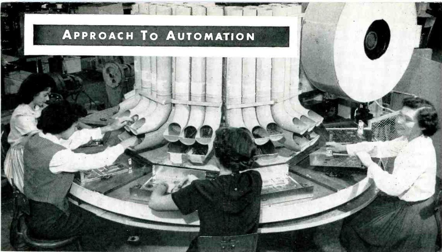
Rotary riveter, nicknamed the pipe organ, uses 40-ton press to fasten 93 rivets in one operation after workers drop into each chassis the special sockets and pin plates needed for dip soldering. Rotary table indexes to next operator every 12 seconds, making capacity of machine 300 completed units per hour. Captive rivets are already on each piece loaded in
