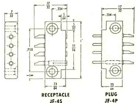
**MONOBLOC\* CONSTRUCTION** eliminates unnecessary creepage paths and reduces the number of moisture and dust pockets.
