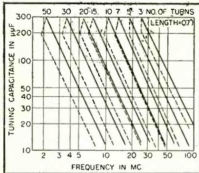
FIG. 2—Chart for National XR-50 coil form. Dotted lines indicate change obtained when using XR-50 iron slug. Copper slug gives shift in opposite direction from the solid lines
