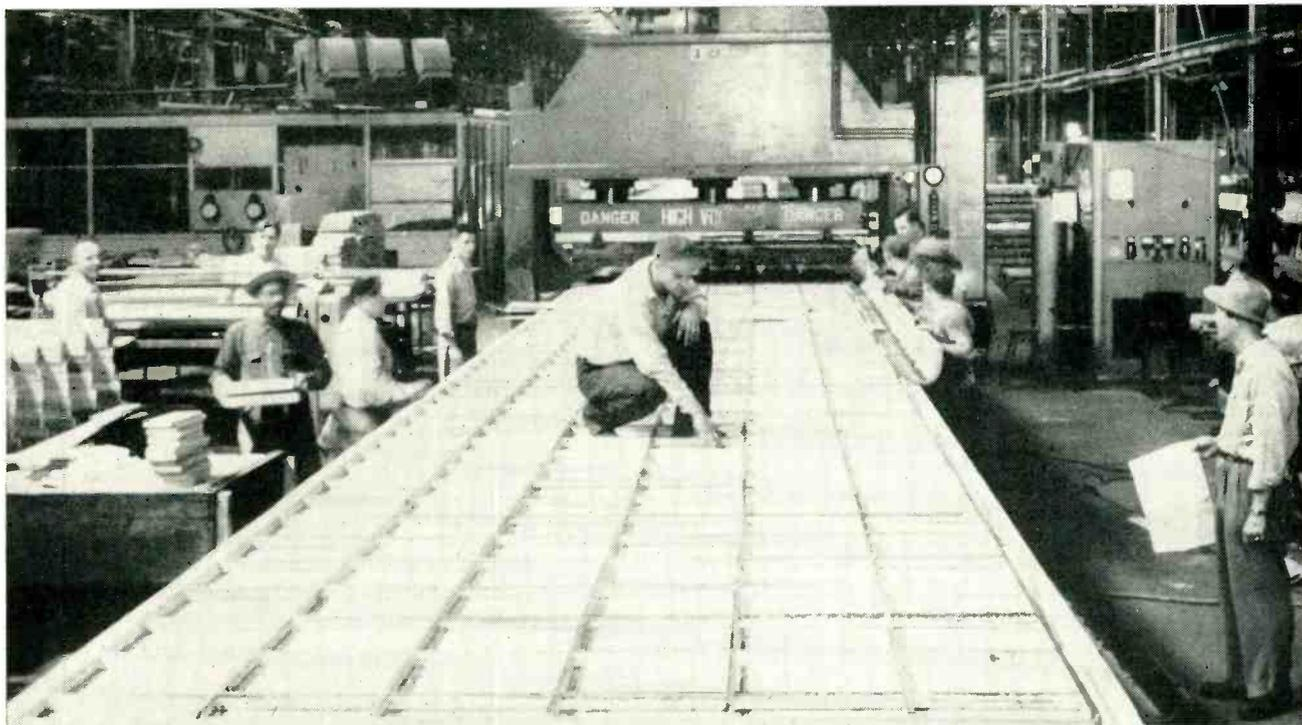
**BOXCAR WALL GLUING**—Entire wall subassembly for plywood freightcar is here being prepared for moving into electronically heated press to cure glue joints between reinforcing strips and plywood faces. Equipment was developed by Thermex Division of The Girdler Corp. Resulting cars are stronger than conventional steel cars
