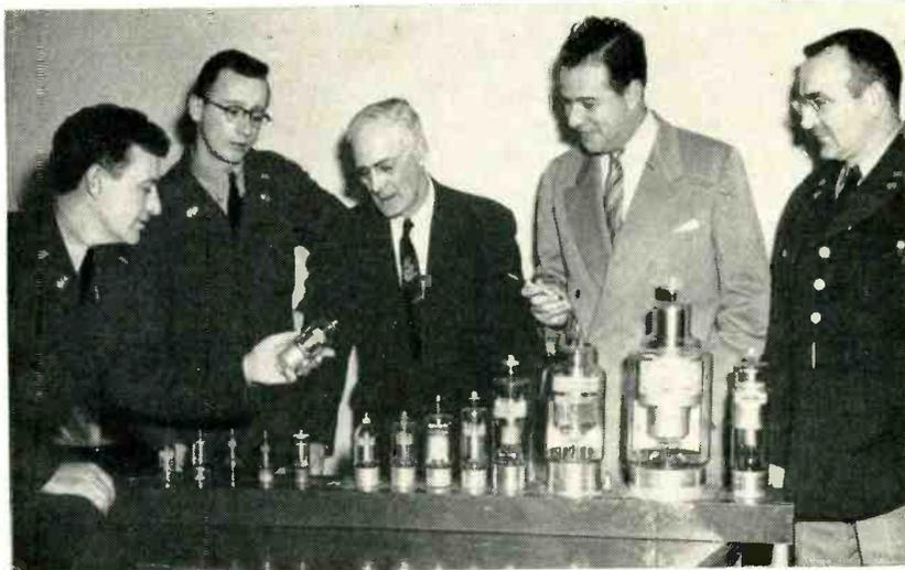
**HYDROGEN THYRATRONS** ranging from a few kilowatts to 40 megawatts produced from emergency development program led by Signal Corps engineers. Rapid expansion on M-Day is possible because . . .
