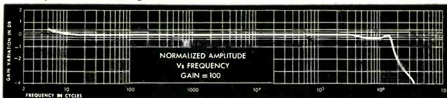
**Amplification Accuracy:**  $\pm 2\%$  of nominal — dependent on precision resistors only; Unaffected by normal tube characteristics or line variations.
