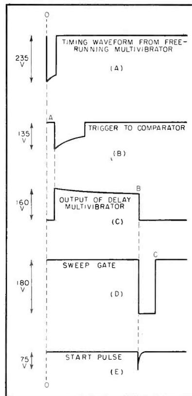
FIG. 3—Waveforms from voltage comparator
