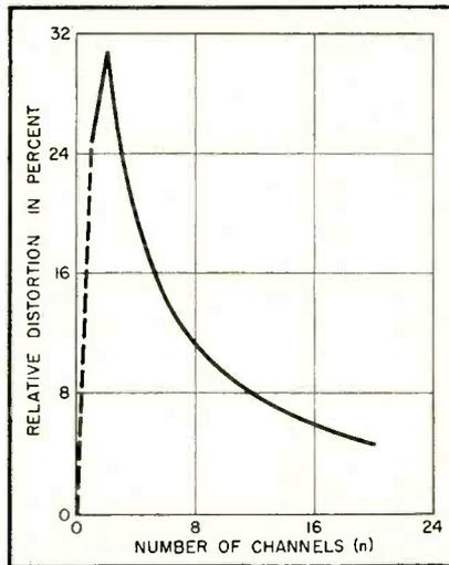
**FIG. 3—Relative distortion versus number of channels for second-order terms**
