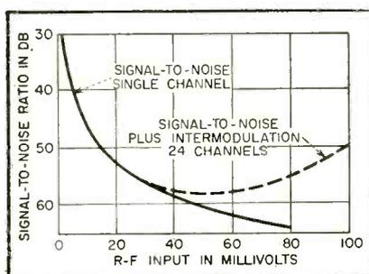
FIG. 1—Signal-to-noise ratio vs r-f voltage input. Dashed line shows noise increase with all channels operating
