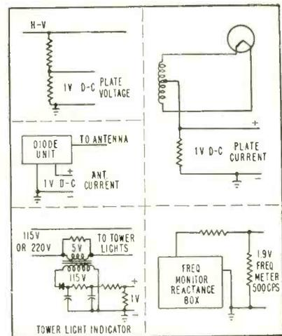
FIG. 3—Monitoring voltages are obtained in several ways
