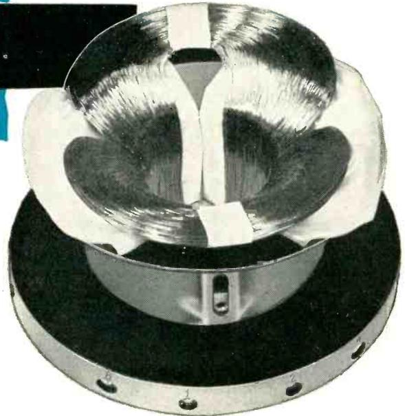
Mounted I-T-E 90° deflection yoke. New flare design lets yoke ride well up on kinescope neck—allows  $\frac{1}{8}$ " pullback for fine adjustment without causing neck shadow.
