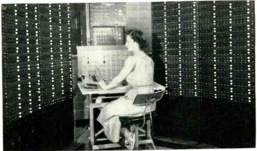
Computer operator reads answers on counter-chronograph (center), initial values are set up on data boards, left and right
