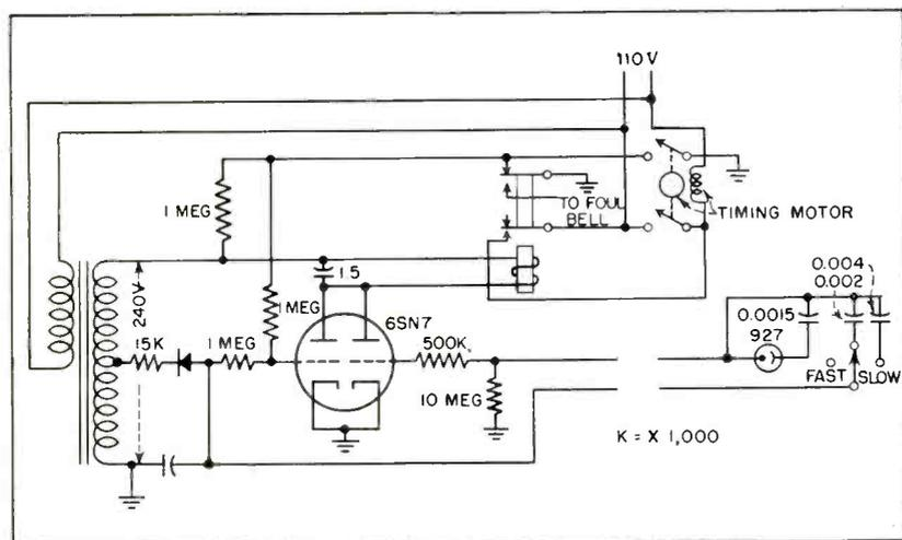
Circuit of the foul-detecting unit. Cam-operated switches control foul bell and light
