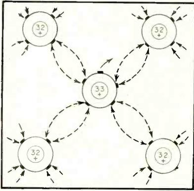
FIG. 5—Germanium crystal structure, showing an atom of arsenic replacing one of germanium to form its own valence bonds with adjacent atoms and leaving one electron to add to the possible current carriers. The fifth valence electron of the arsenic does not enter into a valence bond. A small amount of energy will bring it up to the conduction band of energy levels where it can act as a carrier of current
