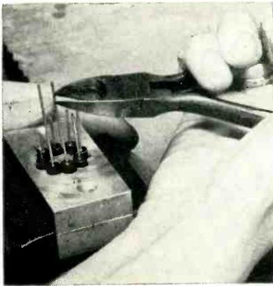
Cutting resistor leads to different temporary lengths to facilitate insertion of leads in holes of end plate
