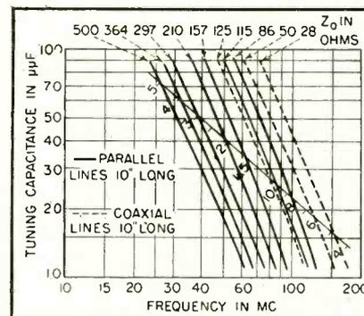
FIG. 4—Chart for 10-inch length of transmission line used as tuning element. Solid curves are for parallel lines; dotted curves are for coaxial lines of same length
