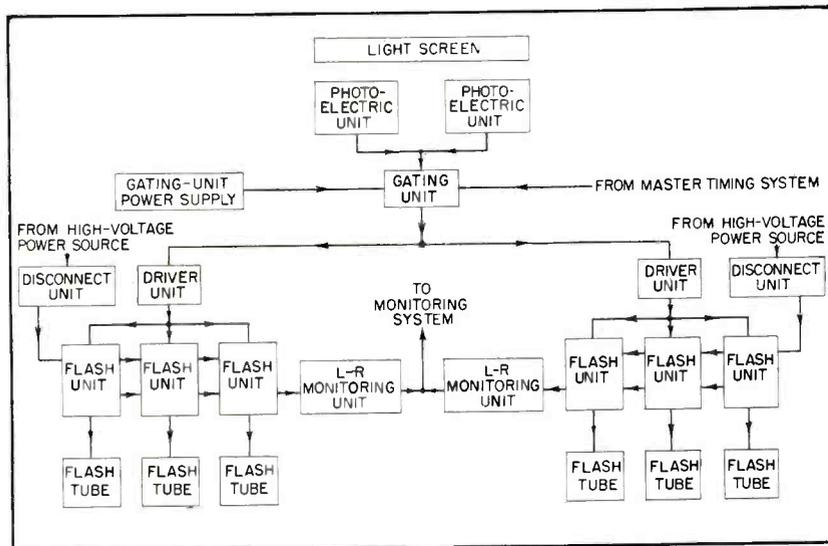
FIG. 4—Photoelectric system used for un gating precision timing signals at each station in sequence as rocket flies down the range
