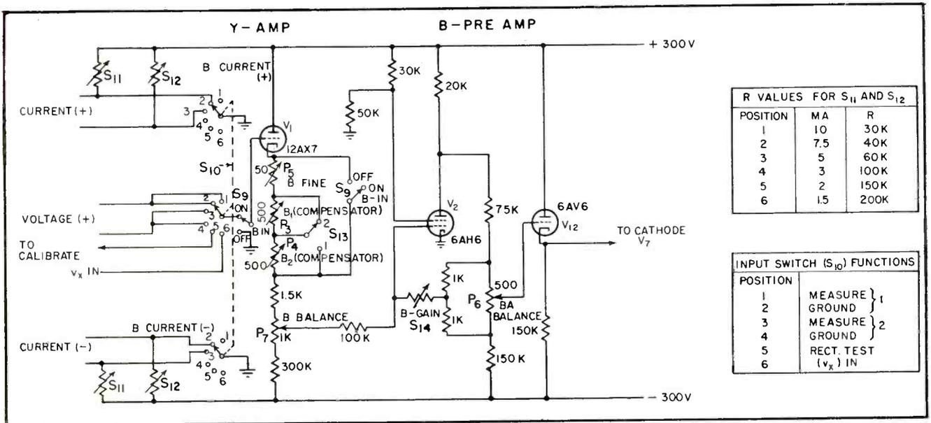
FIG. 5—Circuit permits scope presentation of specimen temperature by producing signal proportional to resistance of gold film thermometer
