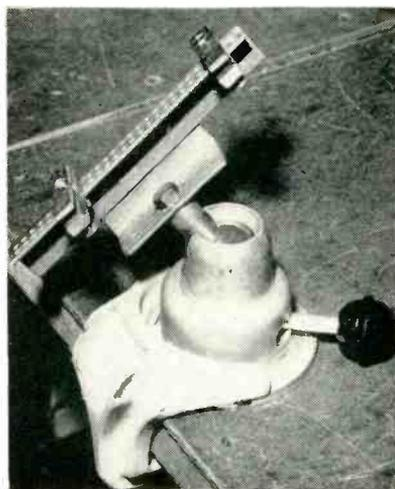
Closeup of chassis-holding fixture, showing also how C-clamp is used to fasten holding tool to bench
