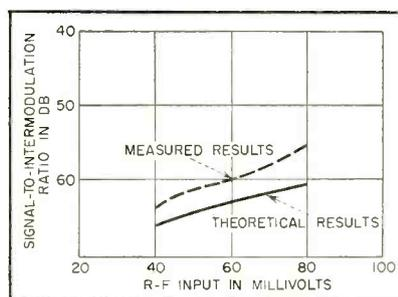
FIG. 2—Signal-to-intermodulation ratio versus r-f voltage input illustrates agreement of calculated and measured results
