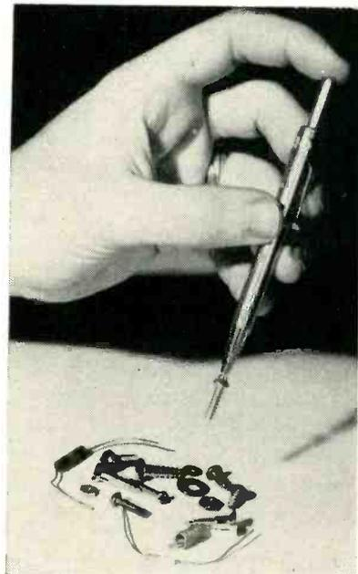
Releasing plunger of tool retracts fingers for gripping screw or other small object
