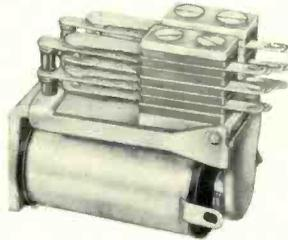
Smallest and most versatile of the telephone type relays, MH Series offers maximum coil power, a wide selection of contact combinations and high contact capacity. Available open or hermetically sealed with maximum of 12 contact springs for either DC or 60 cycle AC operation.
