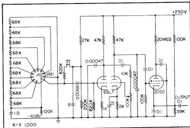
FIG. 5—Multiplier phototube and amplifier circuit arrangement
