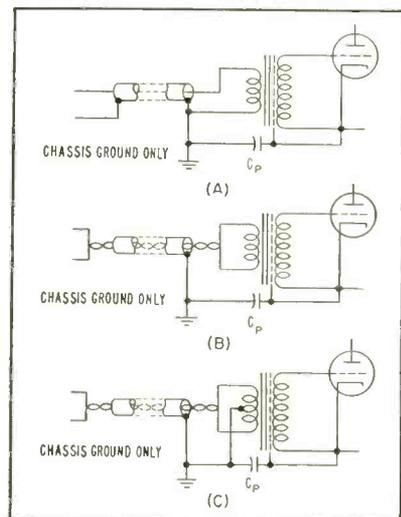
FIG. 2—Three input circuits for intercom systems
