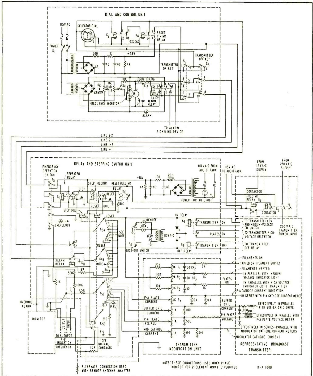
FIG. 1—Schematic diagram of Canadian GE remote-control equipment employing two telephone pairs and stepping switch for operating and monitoring 1-kw  $\alpha$ -m broadcast transmitter
