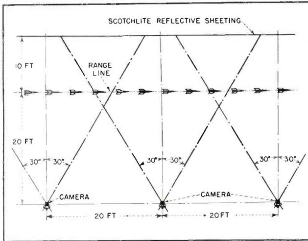
FIG. 1—Orientation used for cameras so each obtains six images of rocket
