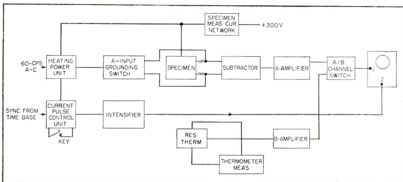
FIG. 1—Block diagram of equipment used in determining resistance-temperature characteristics of bulk semiconductors
