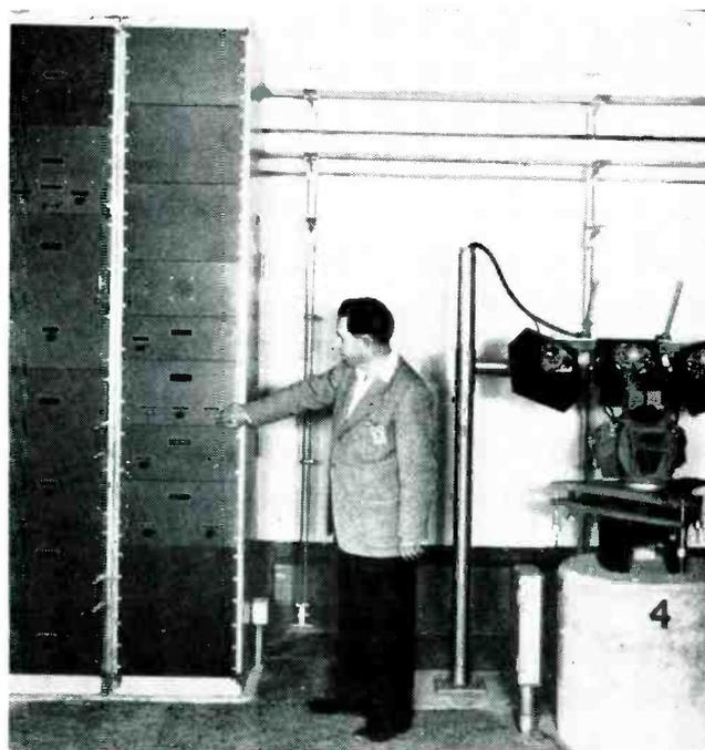
Instrumentation, lamp setup and ballistic camera at one station. Opposite position for station has only one vertical rack as photoelectric ungating equipment serves for both sets of flash lamps. Tubes to detect missile are set into floor of building
