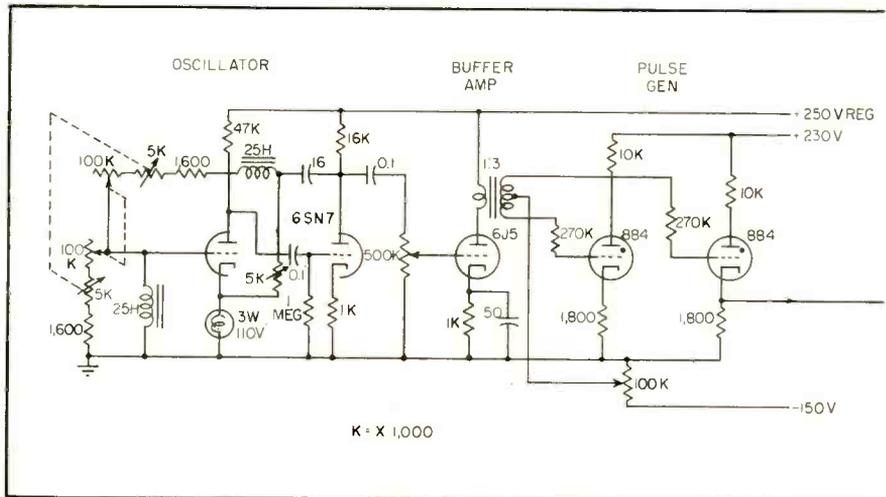
FIG. 2—Circuit diagram of visual testing apparatus. Only one output channel is shown
