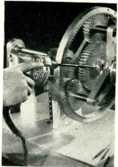
Using drill extension rod with ordinary electric drill. Individual chucks are available for each drill size, as at lower right
