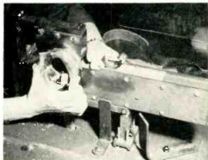
Rotating yoke by hand to wrap insulation around it under pressure. Tape sticks to Saran and pulls the cambric around as the yoke is turned
