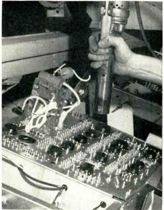
Method of using motor-driven wobble gun to push tube socket adapters onto socket pin plates
