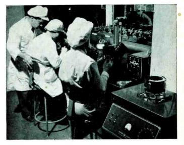
Hidden to the naked eye is the probable life of a precision bearing. This life depends on measurements by microscopic instruments and on microscopic cleanliness.
