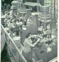
Production operations — including mixing, molding, drilling, tapping and stamping are mechanized. This assures uniform quality, fast operation, low costs.
