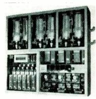
Locomotive ignitron cubicle houses six tubes and associated apparatus
