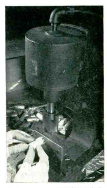
Holding leads of electrolytic unit in position for shearing ends to correct length. Foot-operated valve actuates diaphragm that drives shearing blade downward
