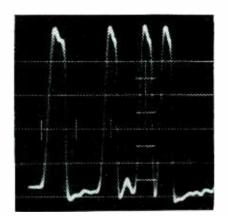
FIG. 3-Same situation as Fig. 2 but with synchroscope gain boosted 30 db so that the second of the 6.67-mc pulses shows more clearly; spurious responses of delay line are here 45 db down
