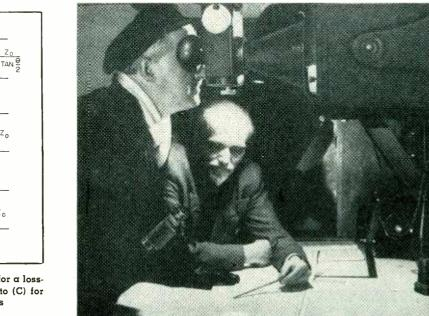
Identification of light blobs on a radar screen, indicating objects surrounding a ship, is often difficult for a navigator. A British invention makes it possible to superimpose the radar display upon a standard chart of the area. The chart comparison unit, which is attached to the radar indicator, also projects an arrow upon the chart below to show the navigator his position and heading
