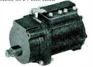
**Electrical Rating:** Rated for operation on 240 volt A.C., two phase, 400 cps. It may also be operated on 208 volt A.C., single phase, 400 cps using a .08 uf capacitor in series with one of the windings.
