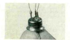
Conduction-cooled 20-watt transistor
