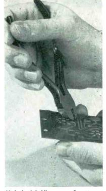
Method of holding new pliers to get optimum visibility while cutting and crimping leads. Replaceable temperedsteel springs keep pliers open, ready for immediate use
