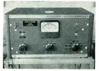
Front control panel of harmonic analyzer has adjustment for input amplitude, meter-range selector and harmonic selector
