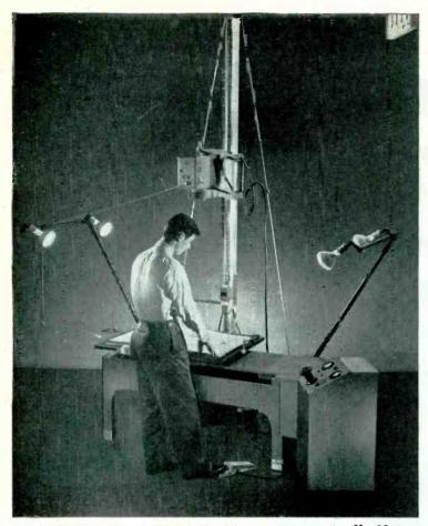
**EASTMAN KODAK'S RECORDAK MICRO-FILE MACHINE** can microfilm 32 acres of valuable records for storage in only 12 cubic feet of filing space. Accurate performance of Ward Leonard Vitrohm rheostat (in circle) helps to assure clear, sharp, reproduction on microfilm.
