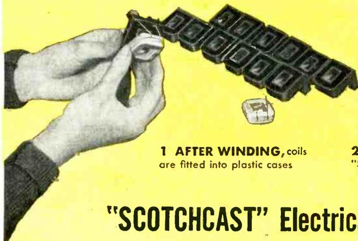
**1 AFTER WINDING**, coils are fitted into plastic cases
