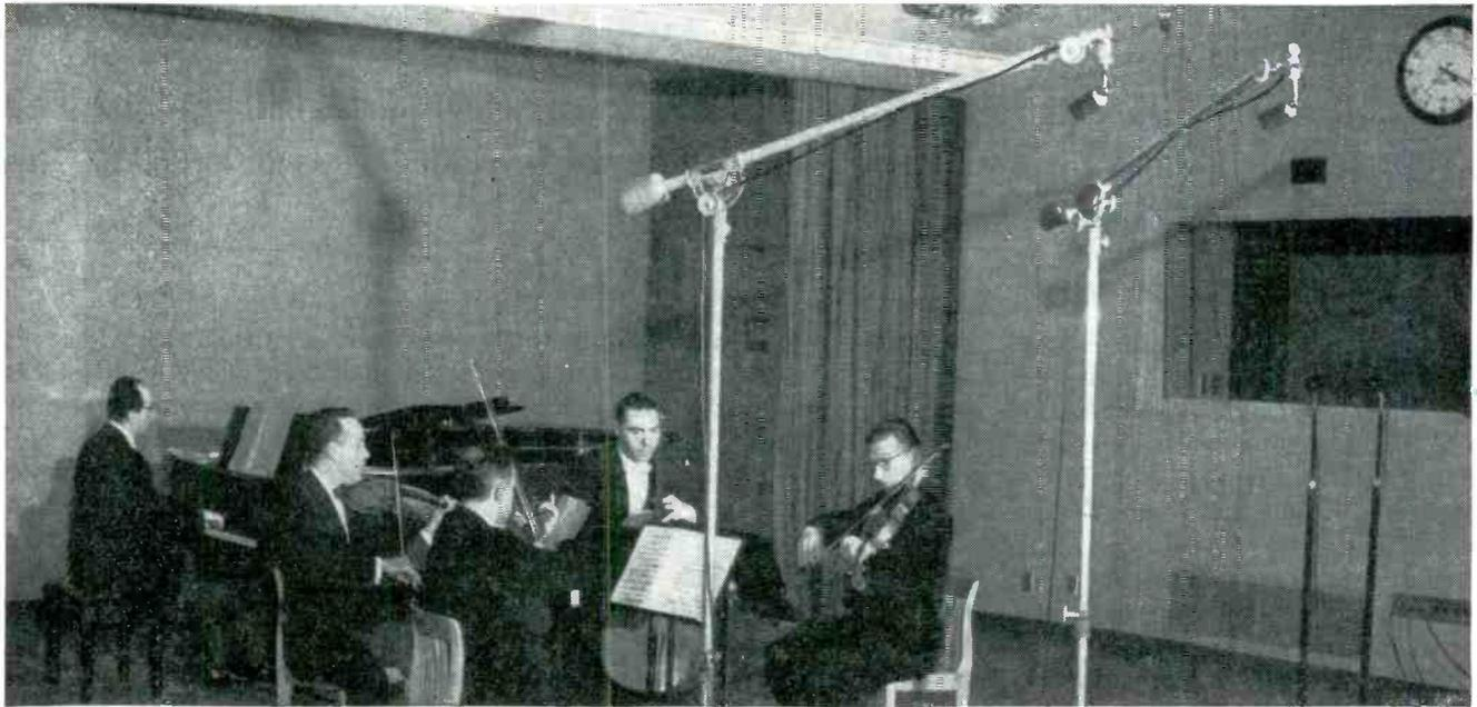
Microphone arrangement for a binaural broadcast. Announcer's microphones are at right near control-room window
