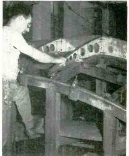
Setup for bending tubing to precise shape by hand without using mandrels inside tubing and without distorting the tubing cross-section. Three men are used for the shaping operation. Small lever-action clamps hold the tubing against the curved template. The operator is here positioning the structural back frame of the screen for subsequent welding to the tubing
