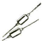
Also perfectly suited to transistor applications, these tiny, Mallory-developed Silverlytic Capacitors have been expressly designed for the requirements of low voltage circuits and miniaturization.
