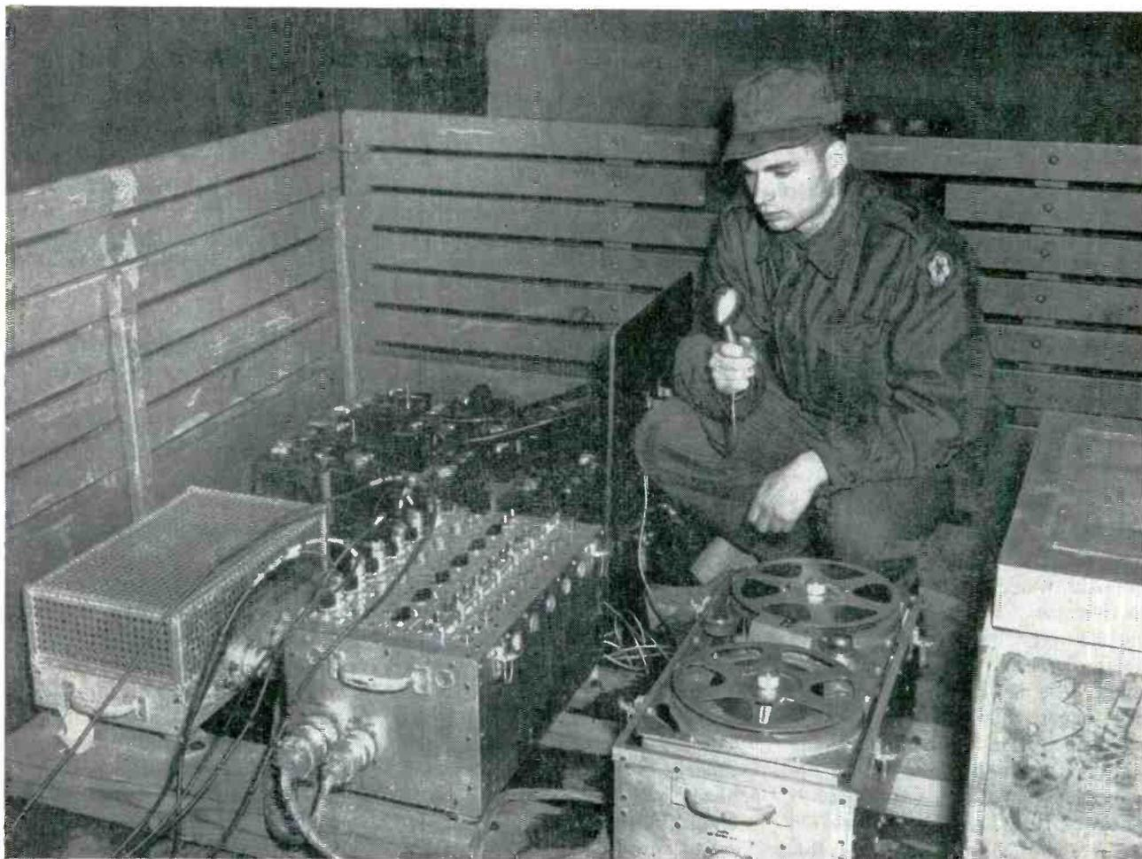
Tape transport mechanism and associated units mounted in truck. Voice channel is provided for commentary on changing road and test conditions, so that any section of resulting tape recording can be readily identified
