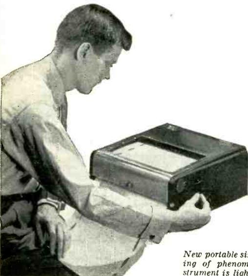
*New portable six-channel oscillograph simplifies recording of phenomena in the shop or in the field. Instrument is lightweight, self-contained, and easy to use.*
