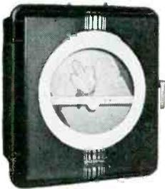
If you are measuring . . . or contemplate measuring . . . a signal or quantity as a function of angular displacement, it will pay you to investigate this new Speedomax Polar Recorder. Tedious point-by-point plotting is completely eliminated with the use of this instru-
