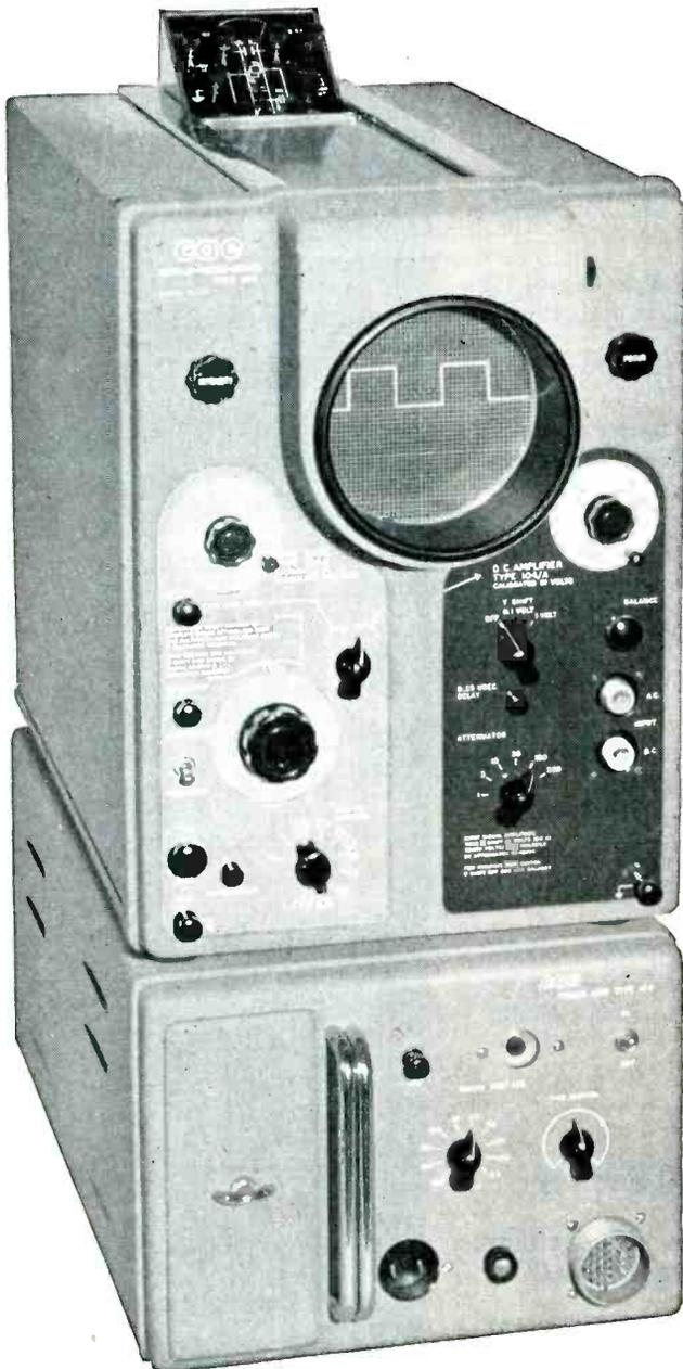
By using interchangeable D.C. Amplifier and Time Base Units, one CAE Oscilloscope performs the operations of several different types of oscilloscopes resulting in a considerable *saving in capital expenditure.*
