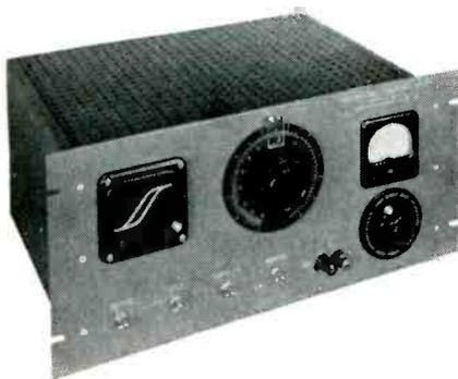
Inductance range is from one to 200 henries. Direct current through the reactor under test is accurately controllable from one to 500 milliamperes, limited only by the resistance of the coil windings. The effect of a change of dc on the inductance value is immediately measurable, by simple rebalancing. The inductance is measured at a constant frequency of 120 cps.
