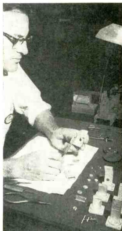
Applying No. 718 flat brazing wire to joint area during assembly of flange to a waveguide prior to dip brazing
