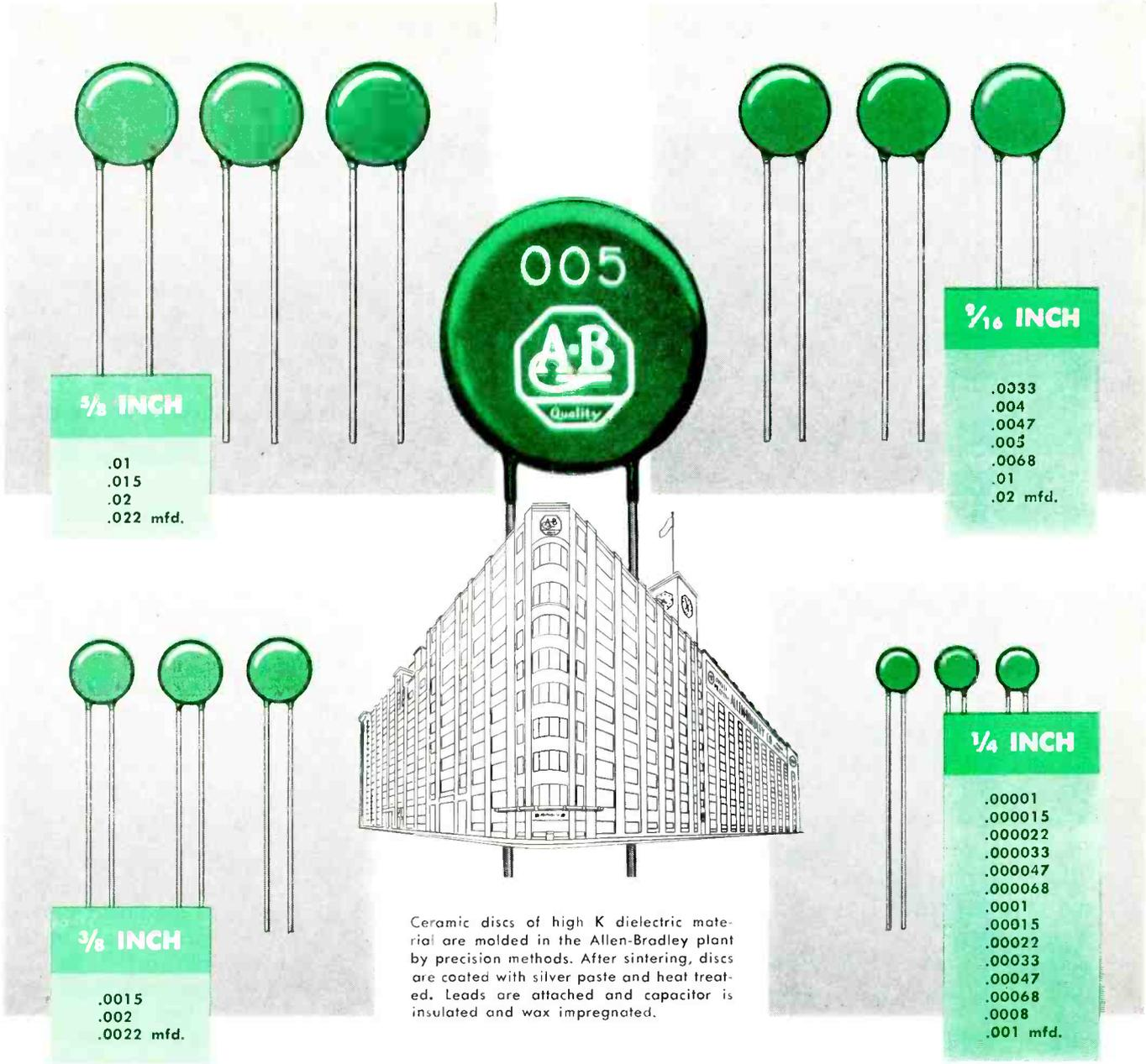
Ceramic discs of high K dielectric material are molded in the Allen-Bradley plant by precision methods. After sintering, discs are coated with silver paste and heat treated. Leads are attached and capacitor is insulated and wax impregnated.
