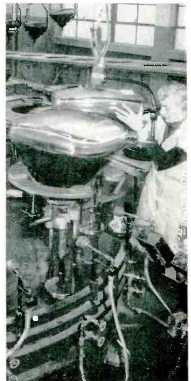
Method of using vacuum lifting aid for loading 27-inch picture tubes into 8-tube automatic sealing machine
