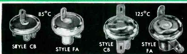
Values from 15 mmf to 8100 mmf are available in tolerances as close as  $\pm 2\%$ . Rated at 500 VDCW. "Q" value exceeds 1000 for values above 100 mmf. Available for maximum operating temperatures of 85°C. and 125°C. Extremely low inductance makes these very compact capacitors ideal for VHF and UHF applications.
