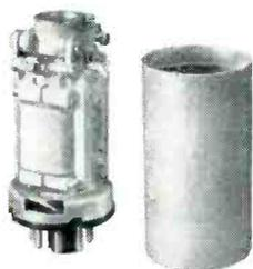
This is a picture of the Sigma Series 72 polar telegraph relay to which the Sgt. referred. Neither major carrier of telegraph traffic regularly use it. They should not however be criticized for this. Each makes, or is responsible for someone else making, one of their own design, and although there is nothing "modern" about either, each has the virtue of thirty or so years of service proof. Like the DC3 Airplane, against which let nothing be said!
