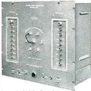
Model 100: Single Pulse Generator, Model 200: Double Pulse Generator, Model 300: Three or more pulse outputs. Rise time .001 usec. Pulse width .001 usec. to several usec. Pulse amplitude from 0.006 volts to 100 volts into low impedance cables (50 ohms or more).
