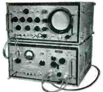
FXR ANTENNA PATTERN ANALYZERS are general purpose test equipments designed for measuring the radiation patterns of rotating antenna systems. The analyzer, a receiver and indicator unit, has the following characteristics:
