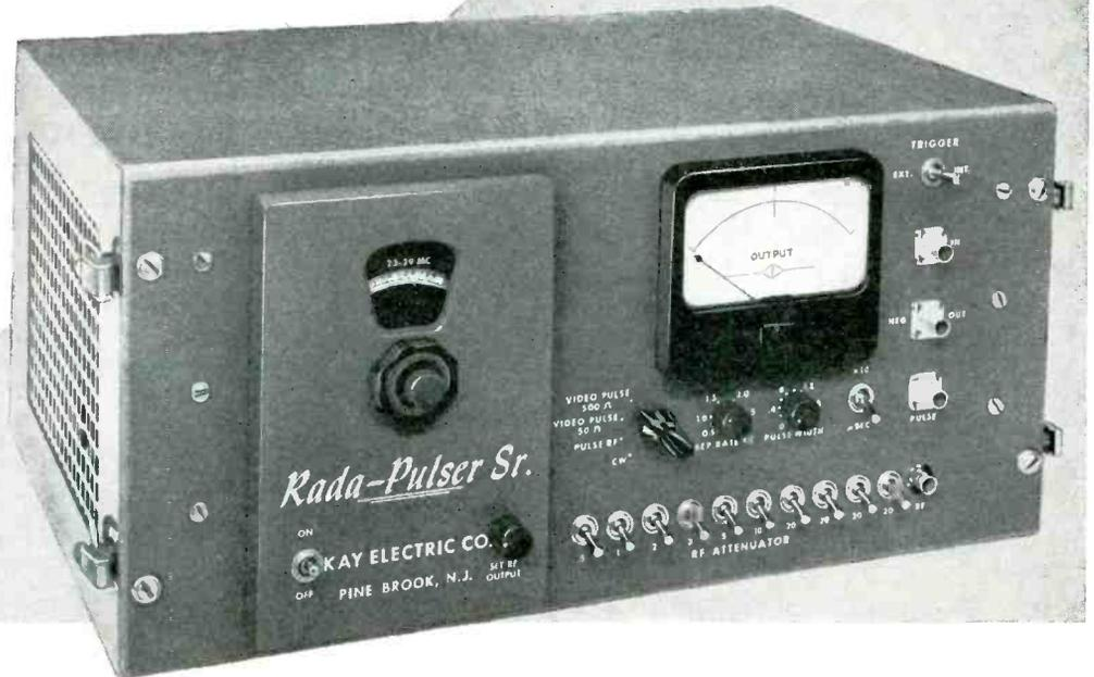
The RADA-PULSER SR., is a CW, pulsed-carrier and video pulse generator, covering the 12 to 80 mc range in five overlapping bands, with a wide choice of pulse widths and repetition rates. In conjunction with an oscilloscope, or a synchroscope, it may be used to obtain a graphic display of the steady state and transient response of r-f and i-f amplifiers.
