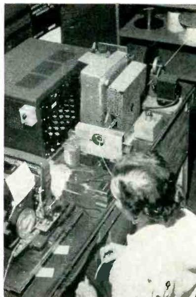
Setup for measuring, cutting and printing wires for electronic aircraft cables
