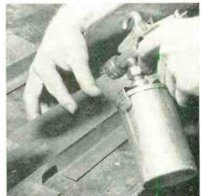
Method of pressing stencil down against chassis with fingers in vicinity of window being sprayed
