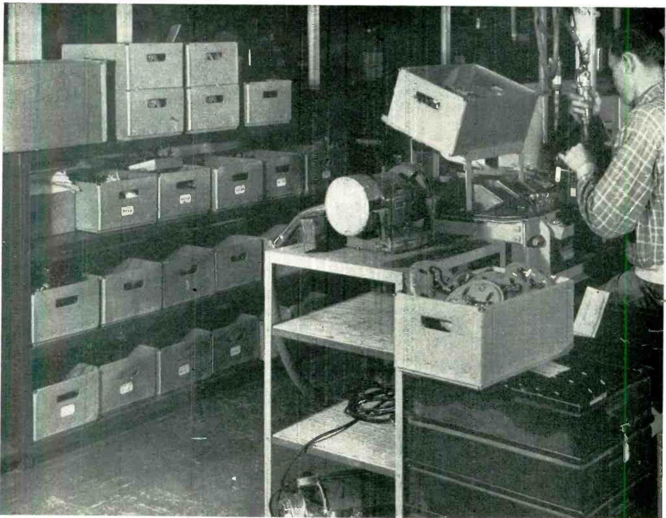
Fibreboard tote boxes in use on precision instrument assembly line, along with conventional metal boxes. Note use of Electrolux vacuum cleaner under grinder, with hose going to sheet-metal enclosure around buffing wheel, to keep down dust during operations
