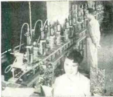
DESIGNED and built by Admiral Corporation engineers, this 30-foot long battery of machines automatically assembles approximately half of the company's vertical chassis for 21-inch television receivers. Blank printed circuit boards start down the one at the far end.
