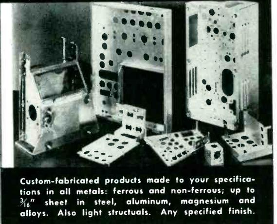
Custom-fabricated products made to your specifications in all metals: ferrous and non-ferrous; up to 3/16" sheet in steel, aluminum, magnesium and alloys. Also light structurals. Any specified finish.
