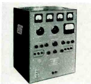
THE W. L. MAXSON CORP., 460 W. 34th St., New York 1, N. Y. An electronic instrument for precise measurement of phase difference between two sinusoidal voltages, model P-1060 precision phase meter provides absolute accuracy of 0.1 deg with incremental accuracy of 0.01 deg operating throughout the frequency range from 30 to 20,000 cps. Any phase angle from 0 to 360 deg may be measured without am-
