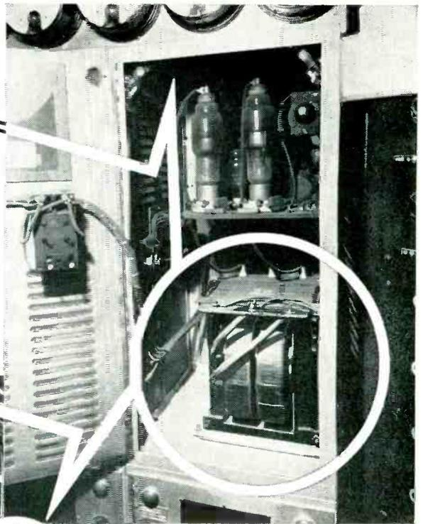
Above photo, with cabinet safety door open, shows NWL Transformer in place. Photo at left shows tube-sealex machine. Cabinet containing transformer is shown within circle.
