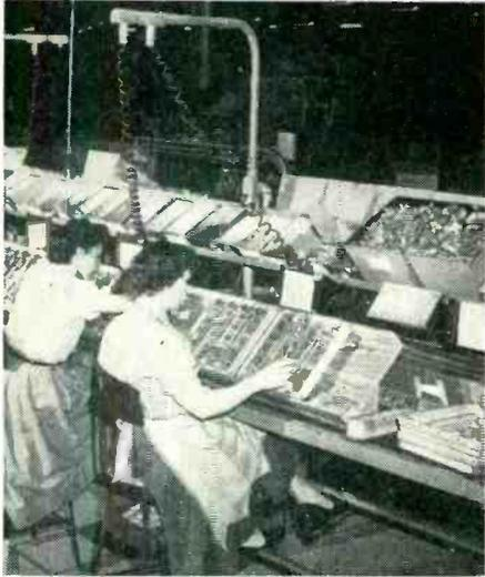
Start of assembly line for i-f strips, showing operator loading strips into four-strip rack
