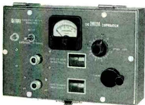
A self-contained instrument with two coaxial resonators tuned by a single control, type N input connectors, crystal detectors, and crystal current meter for resonance indication. Features 0.2% accuracy, high loaded Q, frequency reading from a universal calibration chart in the removable cover (not illustrated). No correction charts are required. The entire frequency range is free from spurious responses or other ambiguities.
