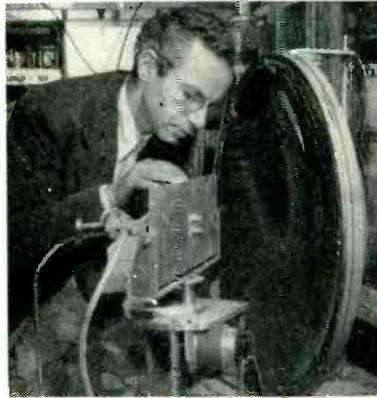
Millimeter wave generator produces frequencies between those of radio and infrared. New waves might be used for short-distance communications
