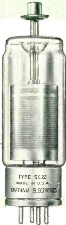
A three electrode zero bias thyatron with peak power handling capacity to 2.6 megawatts
