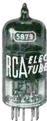
**RCA-5879**—is a sharp-cutoff pentode of the 9-pin miniature type intended for use as an audio amplifier in applications requiring reduced microphonics, leakage, noise, and hum. It is especially well-suited for input stages of medium-gain public address systems, home sound recorders, and general-purpose audio systems.
