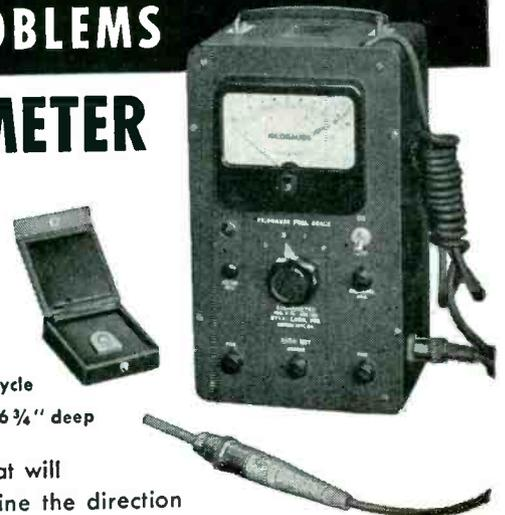
A complete precision built unit that will measure flux density and determine the direction of "flow". It will locate and measure "stray fields", plot variations in strength and offers a fine use for checking production lots against a standard. It is simple to operate—no ballistic readings... no jerking or pulling. Comes in protective carrying case.
