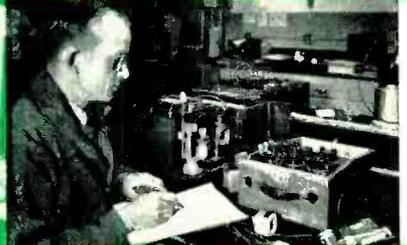
Other quality control tests are made as fabrication progresses. Corrosion resistance of insulating materials is checked as coil assemblies are tested.
