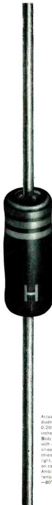
Actual size, diode glass body: 0.265 by 0.103 inches, maximum. Body is coated with opaque silicone enamel to shield crystal from light. Color-coded on cathode end. Ambient operating temperature range: -80° to +200° C.
