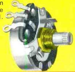
Concentric shaft tandem control with conventional bushing mounting. Designed for front panel dual knob applications, such as contrast and volume. Available in various combinations of composition or wirewound front and rear sections with or without on-off switch attached to rear section. CTS type GC-C252-45 with wirewound front section, composition rear section and on-off switch illustrated.
