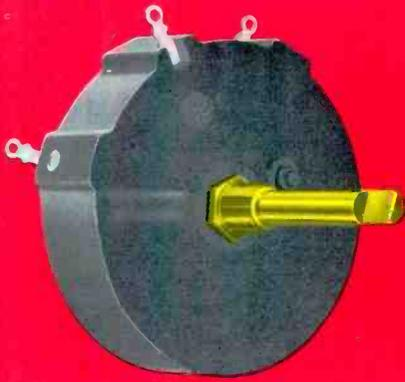
High voltage control for focus applications. Rated up to 5,000 volts DC across end terminals and 2 1/2 watts depending on total resistance. Will operate up to 15,000 volts DC above ground when mounted on insulated panel. CTS type 85.
