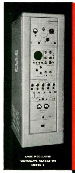
Four Interchangeable Microwave Oscillator Units - each with single control direct reading dial...cover the range 1000 to 10,750 mcs...constructed with precision power monito circuit to maintain 1 mw power output reference level...keying circuit assures rapid rise time of medulated RF output...employs noncontacting chokes...built-in RF detecto:...can be modulated externally.
