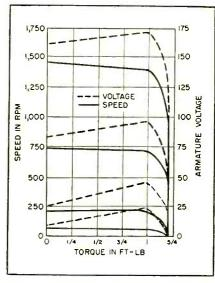
FIG. 8—Regulation curves for shunt-motor controlled by circuit of Fig. 7
