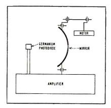
FIG. 8-Combining lens with mirror
