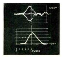
FIG. 5-Digit-plane output (upper), and pulse fed into gate tube after amplification and rectification (lower)
