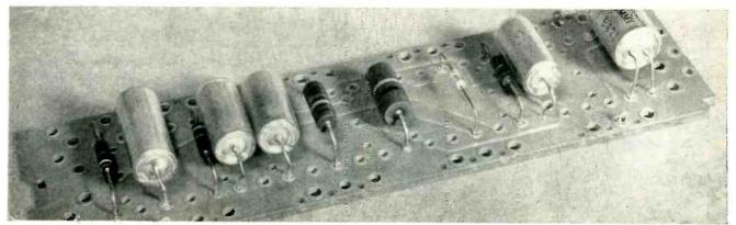
Example of 11-component panel assembled by machine, with four-lead pulse transformer at right. Extra punched holes permit use of same panel with different printed wiring for other circuits of computer, cutting panel-punching costs
