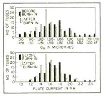
Effect of burn-in on range of mutual conductance and plate current for batch of 6BF7 tubes
