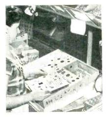
Placing subassembly chassis plate in position on main color receiver chassis resting in special wood pallet
