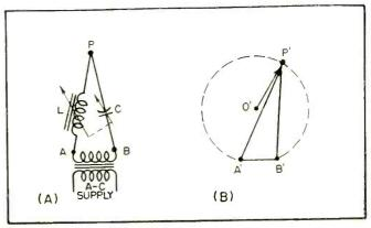
FIG. 2—Basic new phase-shifting circuit uses variable capacitive reactance and variable inductive reactance
