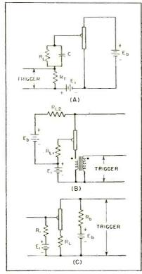
FIG. 8—Variations of double-base diode switching circuits showing junction-triggered type (A) base-one triggered (B) and base-two triggered (C)
