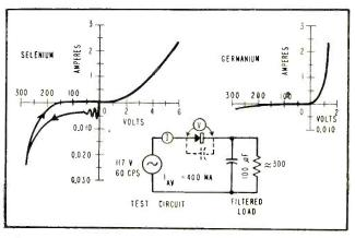
FIG. 11—Volt-ampere characteristics of selenium rectifier and equivalent germanium rectifier (Transistor Products, Inc.)
