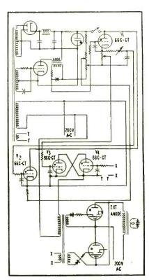
FIG. 4—Spot welder control circult using two vibrating-ignitor tubes. Circuits of exciting anodes are not shown
