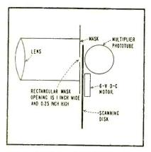
FIG. 1—Simplest optical arrangement of scanner-type dimmer
