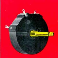
High voltage control for focus applications. Rated up to 5,000 volts DC across end terminals and 2 1/2 wafts depending on total resistance. Will operate up to 15,000 volts DC above ground when mounted on insulated panel. CTS type 85.
