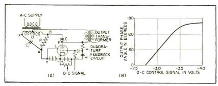
FIG. 9—Variable inductive reactance is replaced by reactance tube (A) to achieve desired phase-shift control voltage characteristic (B)
