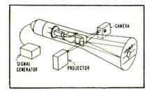
Optical images can be projected through the neck of a crt and reflected onto the inner surface of the tube face. One mirror can be used in photographing the resultant display
