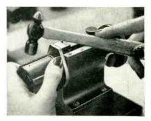
Tapping first drive pin into housing to anchor far end of coil
