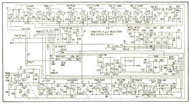
FIG. 2—Complete circuit, with plug-in connectors omitted for simplicity. Dashed lines connect all units mechanically ganged to crystal selector switch (lower left) for automatic tuning
