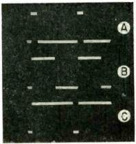
FIG. 8—Differential gain with 10-percent duty cycle (A) 50 percent (B) and 90 percent (C)
