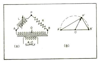
FIG. 1—Classical phase-shifter used to control ignition angle of control rectifiers. Maximum theoretical phase shift is 180 deg
