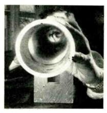
Section of copper waveguide through which a Bell Labs engineer is peering will simultaneously carry tens of thousands of conversations and hundred of tv programs. For technical details, see p 212
