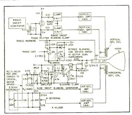
FIG. 11—B scan and retrace blanking circuit, with B-ppi transfer switch shown in B position
