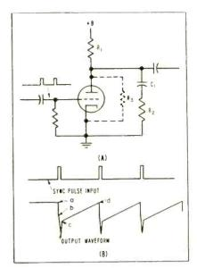
FIG. 1—Sawtooth generator (A) and output waveform produced (B)
