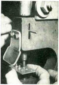
Operating the manual riveter. Protruding rod moves upper die down against light spring action. Operator inserts terminal in board, brings board into upper jaw as shown, then pulls down jaw with left hand to insure that terminal seats perfectly. Pressing foot pedal then pulls down cable attached to actuating air value of riveter.
