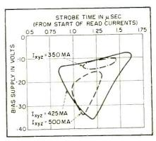
FIG. 7—Failure bias bounds in sense gates as a function of the sample or strobe time
