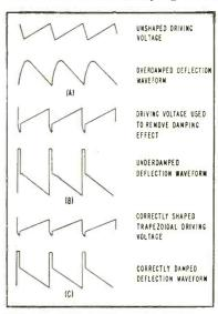
FIG. 2—Driving-voltage waveforms and deflection-voltage waveforms showing effects of overdamping (A), underdamping (B) and correct damping (C)
