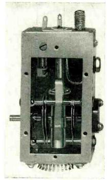
Transmitter tuning cavity, with pulley shaft projecting at left
