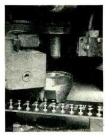
Riveting head in position. Terminal was previously dropped into conical lower member where it is held by spring in upright position until die descends
