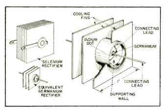
FIG. 10—Construction of germanium power rectifier (Transistor Products, Inc.) and comparison with equivalent selenium unit
