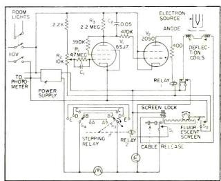
FIG. 1—Circuit diagram of exposure timer. The charge on  $C_1$  controls the tube operation
