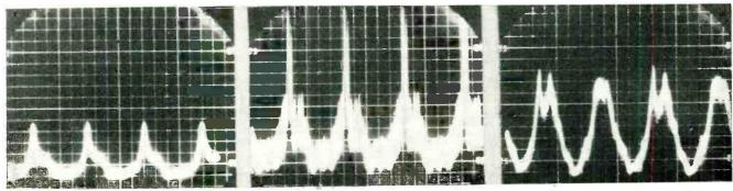
FIG. 6—Relay-contact resistance variations in 130-db sound field. Excitation frequencies are, left to right: 950, 1,000 and 1,400 cps
