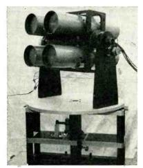
Multiple photoelectric photometer used to measure and record night airglow. Colored filters in each telescope allow various light frequencies to be observed
