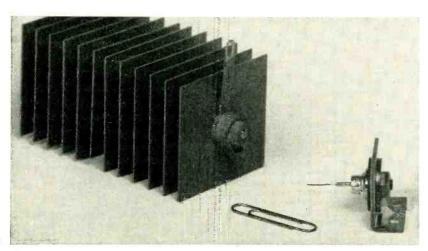
FIG. 13—Relative sizes of silicon junction rectifier (right) and conventional selenium rectifier having the same power-handling capacity
