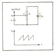
FIG. 4—Saw-tooth waveform produced by double-base diode oscillator circuit
