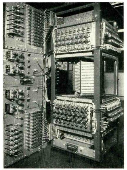
Campleted stack is shown installed in the stall. Rack at left of stall contains the cathode followers. The two wide panels in the center contain the read and write gate generators
