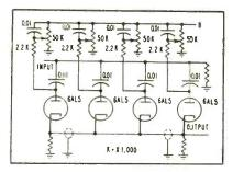
FIG. 1-Pulse multiplier produces four output pulses for single input pulse
