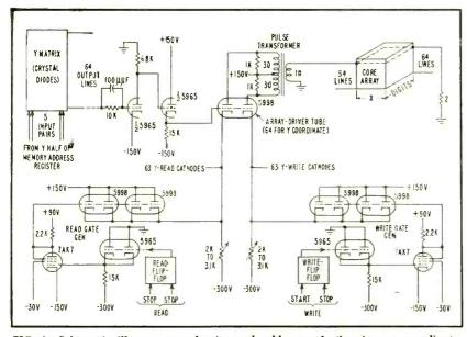
FIG. 3—Schematic illustrates read-write and address selection in one coordinate. Components such as parasitic-suppression resistors and power-supply decoupling filters are omitted to simplify diagram
