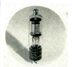
filament voltage, 2.5 v; filament current, 9 amperes; peak inverse voltage, 1,250.
