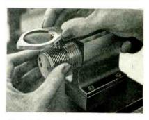
As first step, coil is threaded onto drum while gate is held out of way
