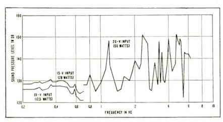
FIG. 3—Sound pressure levels in test chamber at different frequencies for constant voltage inputs. Reference level of 0-db is taken at 2 imes 10<sup>-4</sup> dynes per sq cm
