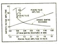
FIG, 4—Peaking-pulse amplitude and dynamic damping resistance plotted against sawtooth driving voltage
