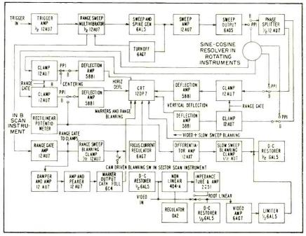
FIG. 9—Functional block diagram of the indicator. An unregulated oscillator supply provides 6 kv for the crt
