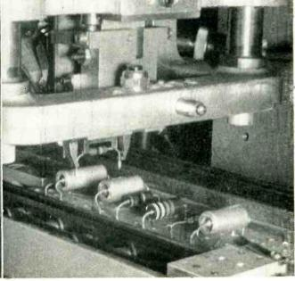
Resistor-inserting position, showing how conical sleeves on leads are pushed into panel holes (Continued on page 10)
