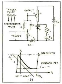
FIG. 5—Regenerative-pulse amplifier circuit (A) and input characteristic of amplifier (B)
