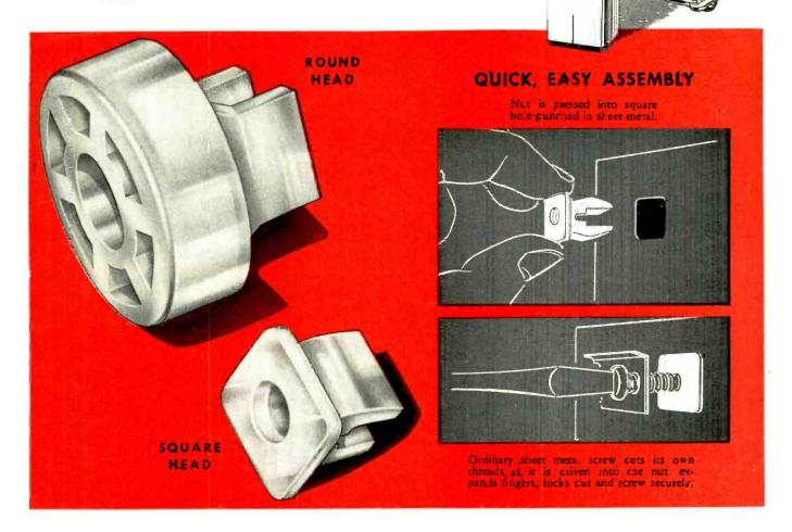
United-Carr's new self-locking, plastic nut is designed for blind application and can be used with all types of metal finishes without scratching or chipping the surface. Its plastic fingers provide rigid anchorage yet will not mar paint, polished metals or even porcelain.
