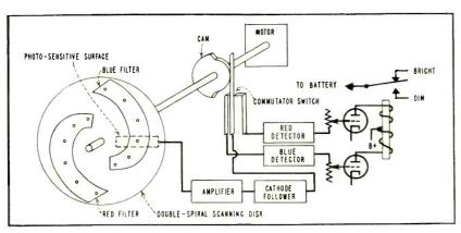
FIG. 5—Dual-channel circuit gives high sensitivity for taillights
