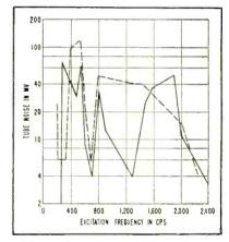
FIG. 5—Microphonics spectra for two tubes in 120-db sound field
