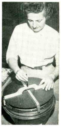
Marking center of picture tube by rotating crayen in centering fixture
