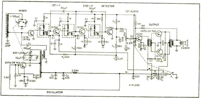
FIG. 1—Superheterodyne receiver uses eight pnp transistors. Note that collectors are negative with respect to grounded emitters
