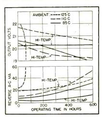
FIG. 5-Comparison of conventional selenium rectifier (unlabeled curves) and high-temperature selenium rectifier in single-phase bridge circuit with 26 v rms input and I ampere d-c output (Radio Receptor Co.)
