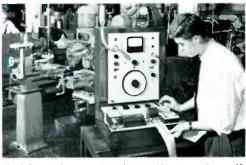
Third-Octave Spectrum Recorder provides a complete, self-Initia-Octave Spectrum Recorder provides a complete, sericontained system for noise analysis and recording — no extras to buy. Precision microphone and microphone calibration apparatus available. System automatically scans and plots sounds from 35 cycles to 18,000 cycles per second in  $\frac{1}{3}$  octave steps.
