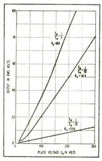
FIG. 3-Oscillator output versus plate voltage for several conditions
