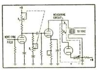
FIG 3—Circuit for automatic damping of vertical-deflection waveform. Diode circuit has been added for the purpose of making dynamic measurements
