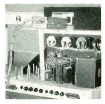
Rear of tester, showing plug and cable at upper left for making connections automatically to amplifier under test
