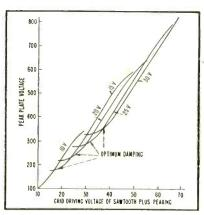
FIG. 5—Sawtooth-plus-peaking values for various levels of sawtooth input
