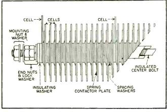
FIG. 3—Life test data on three developmental selenium rectifiers FIG. 4—Typical selenium rectifier assembly (Fansteel Metallurgical Corp.)
