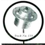
Type CK5 Low Inertia Servo Motor: 2 phase; 26 volts, 400 cycle; stalled torque .5" oz; speed 3460 rpm; reversing time 0.4 seconds; weight 6 oz - length 13/4"; Pianeer Instrument. \$22.50 each
