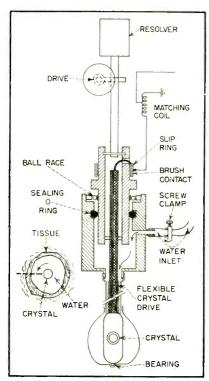
FIG. 8—Composite view of rotary scanning ppi crystal applicator, with mechanical details shown in section
