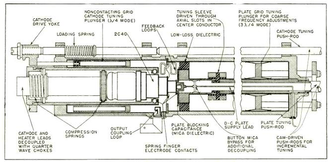
FIG. 1—End-to-end form of grid-separation circuit using a 2C40 oscillator operating in the 1,000 to 1,500-mc region
