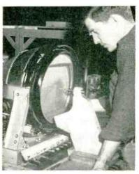
Centering picture tube on chassis by lining up crayon mark with centering plunger
