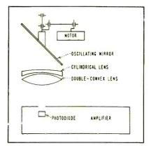
FIG. 6-Oscillating mirror scanner
