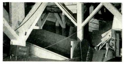
In the Weyerhauser Timber Co. sawmill at Longview, Wash., mill ends and edgings are recovered for production of pulp. The salvage is conveyed to chipper machines that cut the scrap into small pieces before being sent on to a chemical digester.
