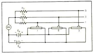
FIG 10—Three-bit binary decoding network. Switching units are turned on by positive pulses at the input
