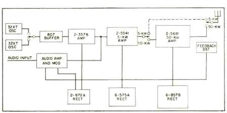
FIG. 2—Complete 50-kw transmitter, showing power switchover provisions for daytime and nighttime operation
