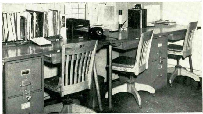
Inexpensive engineering-department desks made from doors, dowel rods and filing cabinets have added advantage of keeping confidential material within reach while meeting security requirements. Note use of simple metal plate and hasp for locking two-drawer files
