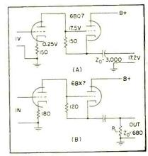
FIG. 3—Double-triode circuit uses cathode-follower principle (A) that evolves into current amplifier type (B)
