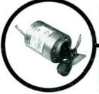
No. 168A Propeller Fan Blower: 115 volts; 320/1000 cycle; single phose; Motor OD' 1.45; Length 1.937"; weight 7 oz; CFM 33 over; speed 11,000: 2½,is\* blode; American Electronic Mfg. Inc. \$15.00 each
