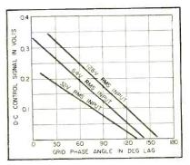
FIG. 6—Control characteristics of saturable reactor circuit of Fig. 5
