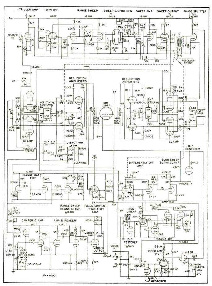
FIG. 10—Schematic diagram of the scanning indicator. One power supply provides 330 volts at 200 ma for the deflection amplifiers and focus coil. A regulated supply furnishes 275 volts at 250 ma for all other tubes
