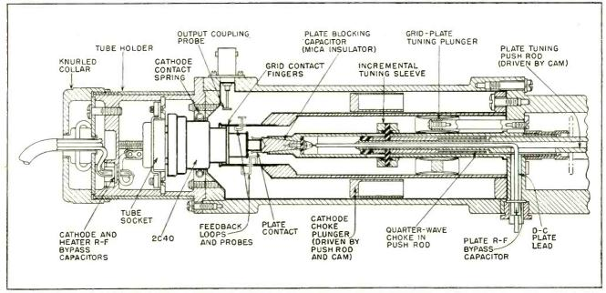
FIG. 2—Folded-back construction, using a 2C40 tube, designed to operate in the 3,000-mc region
