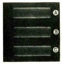
FIG. 10—Differential gain test signal through amplifier and high-pass filter at amplitude of 1.5 volt. peak-to-peak. Duty cycles of 10 (Å) 50 (B) and 90 percent (C)
