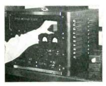
Method of plugging amplifier into panel for test
