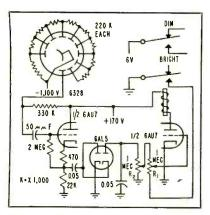
FIG. 2—Circuit uses special automotive type multiplier phototube
