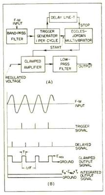
FIG. 3—Final form of f-m discriminator (A) using band-pass filter and trigger generator to start multivibrator. Pertinent waveforms at (B)
