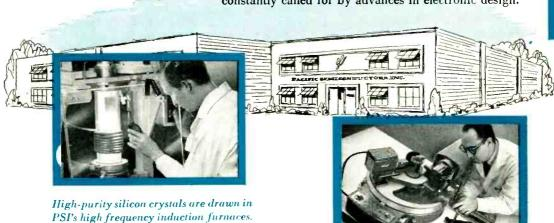
slicing wafer for silicon junction diodes.
