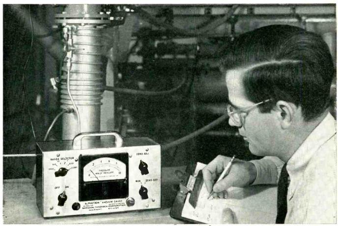
The AC-operated Model 517, newest of the Alphatron® Vacuum Gauges, with 6 ronges covering pressures from 1000 to .0001 mm. Hg. Price: \$425.
