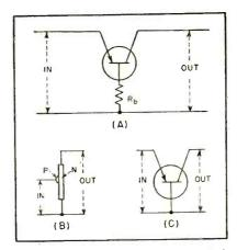
FIG. 7—Point-contact transistor switch
