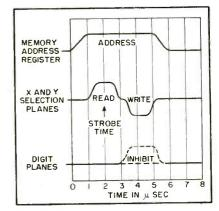
FIG. 2—Timing diagram of the currents in the core-memory array lines
