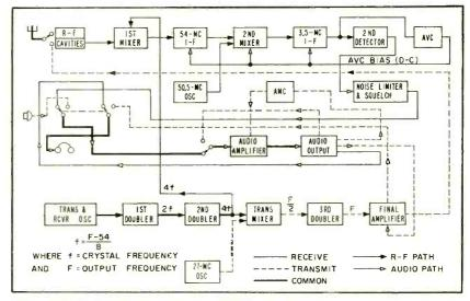
FIG. 1—Block diagram of Radio Set AN/PRC-14, designed for optimum operation with minimum number of stages and minimum space and weight
