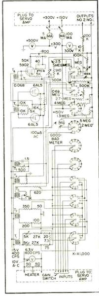
FIG. 2—When amplifier under test is plugged in, its terminals automatically make contact with plug terminals at top and bottom of circuit. Ten-deck, eleven-position selector switch is then swung through its positions while watching good-bad scale of microammeter
