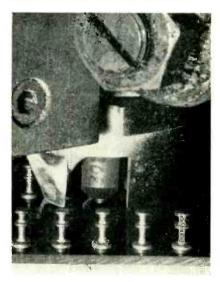
Die in lowest position, for holding down lug while it is being swaged underneath
