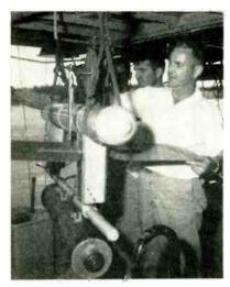
Camera buoy monitored fish and net in action
