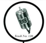
Type R200-1-A Synchro Control Transformer: rotor 1 phase; 26 volt; stator 3 phase; 11.8 volts; 400 cycle; 0D 1.0.62; motor tength 14%4; weight, 3.5 oz.; Kearfott Co., \$15.00
