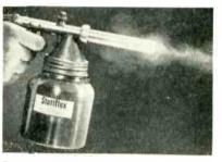
Positively charged powder being blown from special gun
