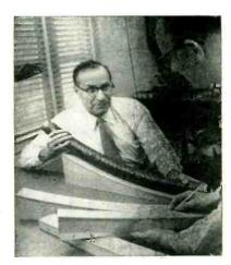
New waveguide for 50-kmc signals can be bent to around corners. Wood forms having various radii of curvature are used in propagation tests
