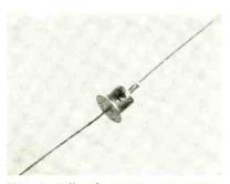
FIG. 6—Diffused-junction germanium rectifier has axial pigtail leads
