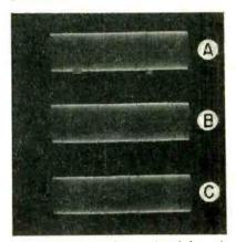
FIG. 9—Differential gain signal through high-pass filter for 10, 50 and 90-percent duty cycle, viewed from top to bottom
