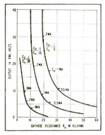
FIG. 2—Oscillator output versus cathode resistance. Plate current is given on curves at points of interest
