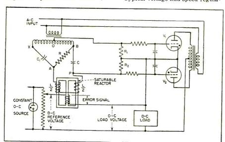
FIG. 7—Negative-feedback circuit delivers constant voltage to d-c load from full-wave thyratron rectifier
