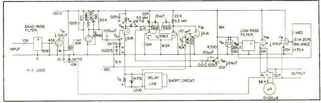
FIG. 1—Complete circuit of the new discriminator. Band-pass filter, delay line and low-pass filters selected for frequency
