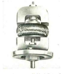
range for any individual Rotoroid is from 50 to 150 percent of the nominal value. Inductance variation in the Rotoroid is obtained by the rotation of one of a pair of permanent magnets placed on apposite sides of the winding. As a result, no external d-c power is required for biasing, the inductance variation with rotation of the control knob is nearly linear, and high Q and low harmonic distortion are preserved even with extreme variation of inductance.
