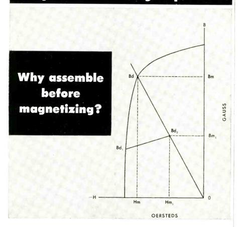
A closed circuit magnet exists when the magnet is magnetized in its assembly of soft iron or other magnetic materials and is not removed later. Normally, there is a specified air gap. The chart illustrates the demagnetization curve for Alnico permanent magnet material.
