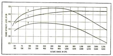
FIG. 1—Typical sound spectra of aircraft jet engine at full thrust measured 10 feet from tailpipe (A), sound level at inboard equipment bay of aircraft (B) and average sound pressure level obtainable in test chamber (C). The 0-db reference level for airborne sound intensity is  $10^{-10}$  watt per sq cm
