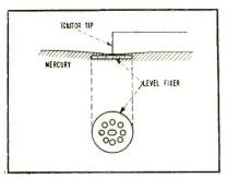
FIG. 2-Level fixing unit in mercury pool eliminates timing changes resulting from variation in mercury level
