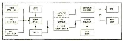
FIG. 2—High-intensity-sound test chamber and associated driving, sensing and monitoring equipment used for testing components
