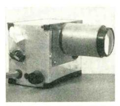
Experimental model of oscillating-mirror headlight dimmer that increases selectivity
