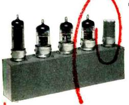
400-CPS AIRPAX CHOPPER PLUGS INTO 7-PIN MINIATURE SOCKET IN THIS COMPACT D-C AMPLIFIER
