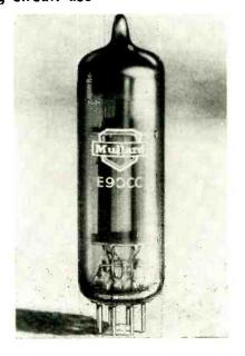
than 10 v. The E90CC is on a miniature all-glass base. It has a heater rating of 6.3 v, 0.4 ampere and an anode dissipation of 2 w per anode.
