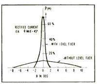
FIG. 3-Range of ignition phasing with and without level fixer
