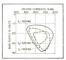
FIG. 6-Failure bias bounds in sense gates plotted as a function of the driving currents
