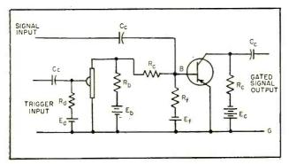
FIG. 9—Gating circuit employs double-base diode to gate transistors
