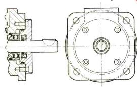
Experimental Way: One cast retainer plate plus four socket head cap screws hold unit together. Assembly requires skilled labor, machinery, time-consuming careful adjustment.
