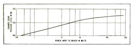
FIG. 4—Sound pressure level in test chamber at test chamber resonance of 2,300 cps. Reference level is same as that in Fig. 3
