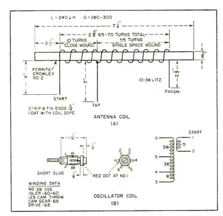
FIG. 2—Winding data for antenna (A) and oscillator (B) coils. Other components are available commercially
