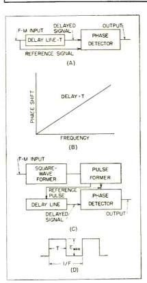
FIG. 2—Basic delay-line discriminator (A), characteristics (B), pulse formation to represent phase angle (C) and multivibrator output waveform (D)
