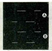
FIG. 6—Square wave of 15-kc frequency shows no impairment through amplifier
