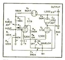
FIG. 3—Noise limiter and squelch circuits of receiver
