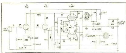
FIG. 2—Operting version of video distribution amplifier includes special bootstrap output stage further explained in Fig. 3
