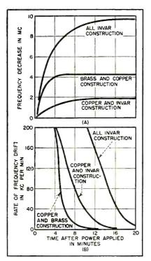
FIG. 3—Poor thermal conductivity of Invar, in one oscillator design, overshadows its dimensional stability
