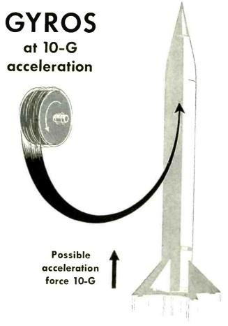
The gyroscope in a missile guidance system must be able to withstand acceleration forces up to 10 G's in any direction. This gyroscope, designed and developed by the Guided Missile Development Division of the U. S. Army and the Ford Instrument Company, will function under this acceleration. Tests have shown these gyros to be accurate to 1/50° per hour drift, or better.
