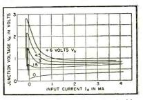
FIG. 2—Input characteristic of a double-base diode
