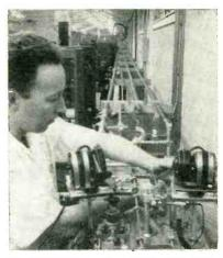
Flexible hollow tubes of two-inch diameter under test at Holmdel, N. J. permit transmission of 50-kmc waves with less loss than conventional waveguides
