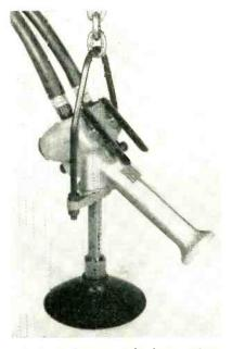
Left lever lowers, right lever raises, and center button on handle breaks vacuum of vacuum lifting tool
