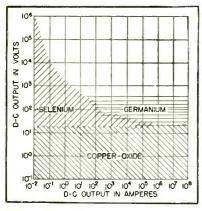
FIG. 1—Economical operating ranges of principal types of metallic rectifiers (General Electric Co.)
