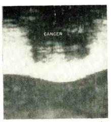
FIG. 6—The normal nipple of a patient is shown at left; the opposite nipple showed a bright area of stronger echoes right. These are the first recognizable records of cancer in living tissue. Basic echo-ranging equipment transmits a 1- $\mu$ sec pulse of ultrasound at a carrier frequency of 15 mc
