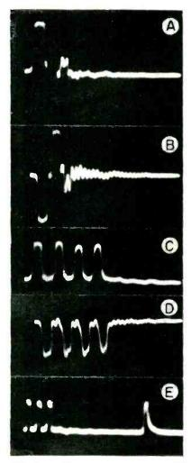
FIG. 2—Positive (A) and negative (B) 20-usec input pulses to multiplier. Four output pulses (C) and (D) are separated by equivalent of 10 meters of RG-59/U cable. Final pulse of (E) is separated from group by equivalent of 100 meters of cable
