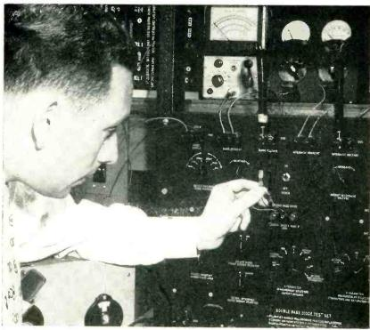
Laboratory test in progress checks characteristics of a double-base diode
