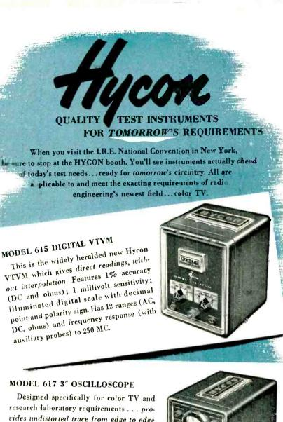
Designed specifically for color TV and research laboratory requirements . . . provides undistorted trace from edge to edge on a special flat 3" CRT. Features high deflection sensitivity (.01 v/in. rms); 4.5 MC vertical bandpass, flat within ± 1 db; internal 5% calibrating voltage. Small, lightweight...but accurate enough for the most exacting work.
