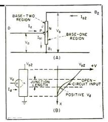
FIG. 1—Double-base diode construction (A) and potential through bar (B)
