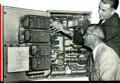
Mr. Dornhoefer (upper right) inspects current production of magnetic amplifier regulator with Mr. J. F. Hysler. Rating of the motor generator set it regulates: Output: 5KVA, 120 V, 3 phase, 400 cycles. Input: 175 to 345 V, DC. Regulation accuracy: ±0.5% on both voltage and frequency.
