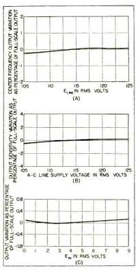
Performance characteristics, showing effects of line-voltage fluctuation on center frequency (A), output sensitivity (B) and input level on output sensitivity (C)
