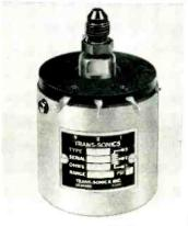
The Trans-Sonics® Baroresistor is a rugged pressure actuated potentiometer designed and field tested for use in operational aircraft. This pressure transmitter provides a simple and reliable means of varying fire control equipment and autopilot performance as a function of pressure (altitude).
