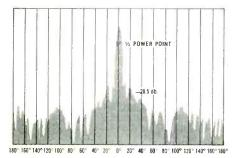
Model 2K6CF Beam Pattern, E. Plane, at 1920 MC
