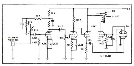
FIG. 7—Method of providing required amplification for photodiode
