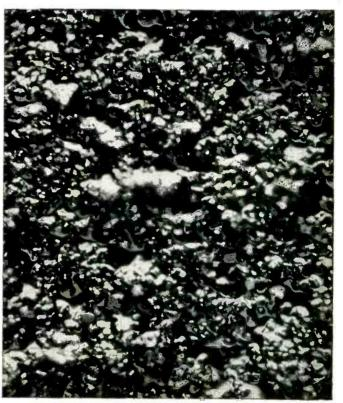
WESTINGHOUSE TUBE — Here's a photomicragraph of the Westinghouse aluminized tube manufactured with the exclusive Westinghouse "Flow-Filming" process, taken under the same conditions. Nate the smoother, more even aluminum coating. It means you get maximum reflection, sharper, more detailed images.
