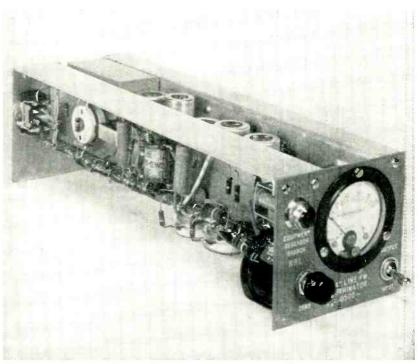
Prototype model of the f-m discriminator shows its small size and single control
