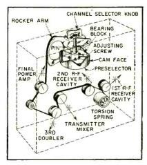
FIG. 4—Method of linking all tunable controls with the four-position channel selector knob for automatic tuning
