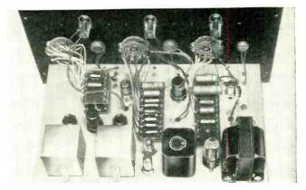
Front and rear views of sonar target simulator. Tip-jack test points above outlets on front panel permit oscilloscope monitoring
