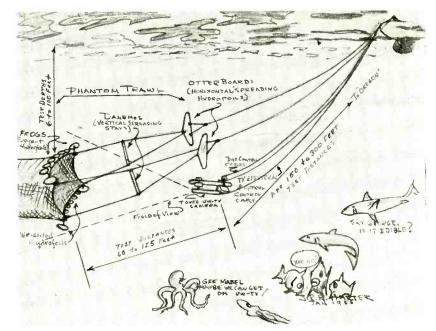
Electronics and Experimental Diving Groups at BuShips used tv and fishing equipment shown above for rating nets (see p 26). We have added "frogs", "danemos" and "otter boards" to our lexicon
