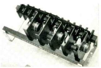
FIG. 8—Stacked germanium rectifiers, under development, provide 5 amp d-c output per cell
