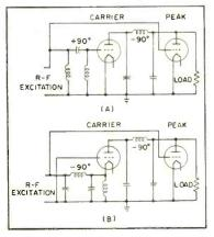
FIG. 1—Conventional Doherty amplifier (A) and grounded-grid version (B)
