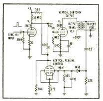
FIG. 7—Automatic damping circuit for vertical output system
