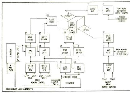
FIG. 1—Magnetic-core memory gives arbitrary or random access to any one of its registers every  $\bf 6$  microseconds
