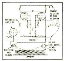
FIG. 5-Photoelectric modification of the circuit of Fig. 4 employs light source
