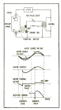
FIG. 1—Vibrating-ignitor ignitron with operating circuit. Waveforms are at various points in circuit during operating cycle
