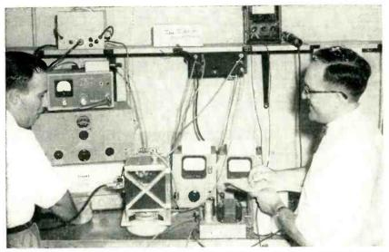
Typical operating setup of test chamber. Tube under test is visible through plastic window in high-intensity noise chamber
