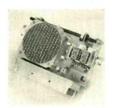
Front of set. Transistors are mounted on chassis between loudspeaker and tuning capacitor
