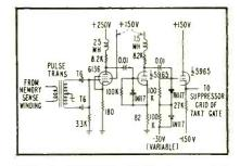
FIG. 4—Simplified schematic of sense amplifier. Cathode degeneration is used to help stabilize gain
