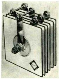
FIG. 2—Three-phase full-wave bridge rectifier rated for maximum a-c input of 40 v rms and d-c output of 32 amperes has selenium cells 6 inches square (Bogue Electric Mfg. Co.)
