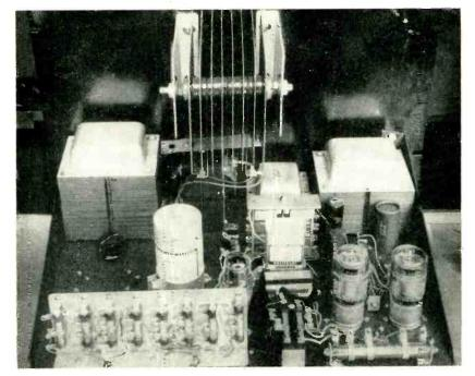
Prototype chassis for automatic program control of mass production machines. No error amplifier tubes are used because of the sensitivity of the phase-shifting circuit
