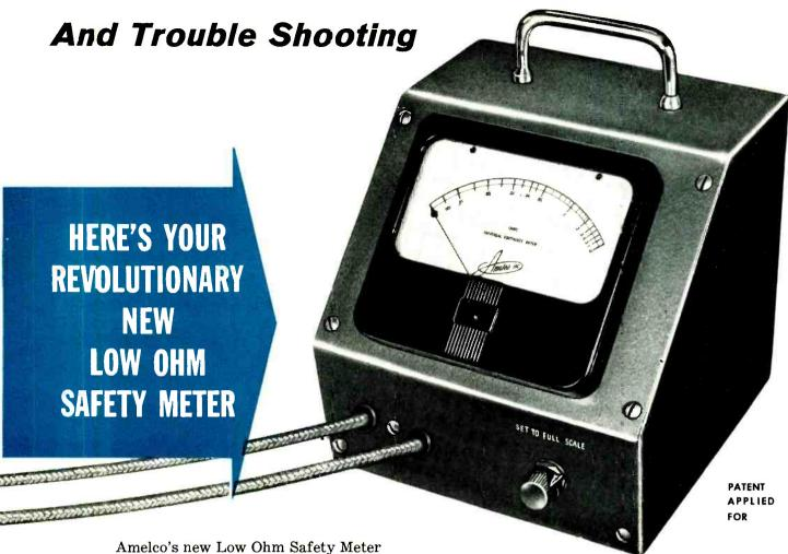
Amelco's new Low Ohm Safety Meter checks the original wiring, including high current filament circuits, etc., which cannot be reliably checked with any other production instrument. More important the Low Ohm Safety Meter saves hours and hours of trouble shooting.
