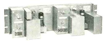
**A** send and a receive panel require 51/4 " of mounting space on a standard 19" rock
