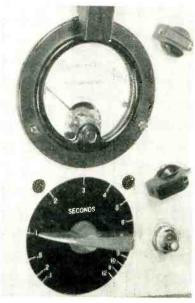
Time control and pilot lights are mounted below the photometer
