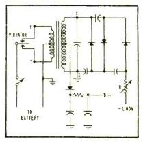
FIG. 3—Selenium-rectifier voltage tripler for phototube dynodes
