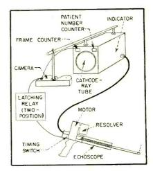
FIG. 12-Equipment for three-dimensional mass rectal scanning. Crystal follows a helical path with alternate revolutions photographed
