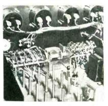
Gear drive system for eleven-position test selector switch
