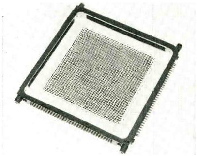
Completed core-memory digit plane with the 4,096 cores spaced on 0.1-inch centers. Overall dimensions of the plane are about  $10 \times 10 \times 34$  inches. Memory employs simultaneous excitation of x and y coordinates, a 2-beat cycle and the principle of sampling of the output signal
