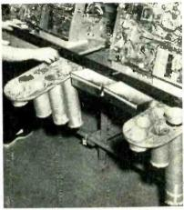
Deep-well wire holders and cake pans support parts on moving-conveyor line
