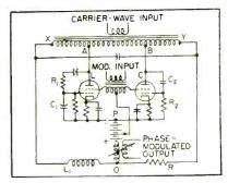
FIG. 10—Reactance-tube wide-angle phase modulator has low distortion
