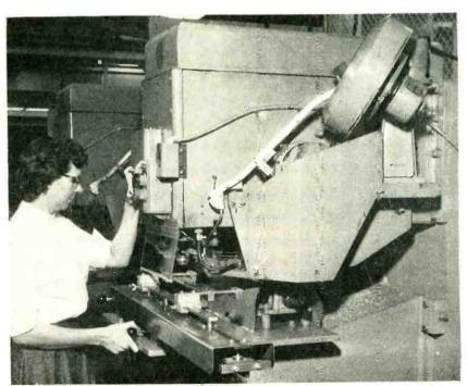
When the start button is pressed, this machine automatically produces terminal boards from phenolic blanks. The operator can tend three or more machines simultaneously since her work merely involves removing finished boards and reloading
