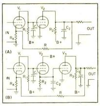
FIG. 1—Development of negative feedback amplifier with two low-pass sections (A) and three-section circuit (B)
