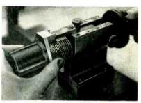
Holding housing against gate while turning crank to thread coil and drum into housing
