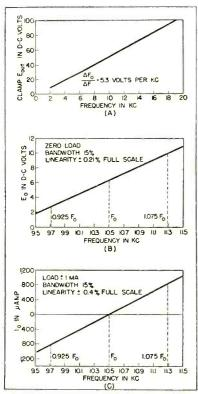
FIG. 4—Linearity characteristics for wide-band operation (A), telemetering band voltage output (B) and current output (C)
