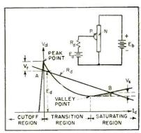
FIG. 3—Three regions are obtained from experimental input chaarcteristic
