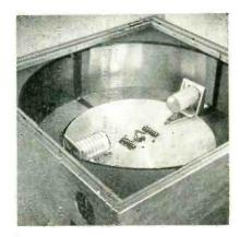
Method of mounting two eight-potentiometer units on turntable
