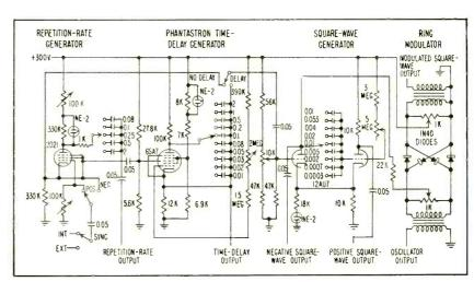
Target simulator combines repetition-rate, time-delay and square-wave generators in one unit. Neon lamps show if circuits are operating
