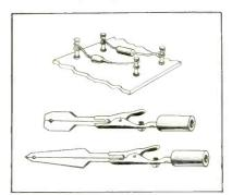
GERMANIUM and silicon crystal diodes often require special care in assembly to prevent damage to sensitive elements. When soldering is required, allow extra lead length for strain relief, and use heat-dissipating clamps on leads to prevent
