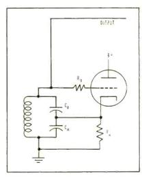
FIG. 1-Modified Harris oscillator circuit requires no chokes or inductor taps
