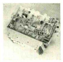
Rear of chassis showing interconnecting wiring. Flashlight batteries are mounted below case
