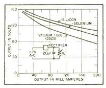
FIG. 12—Regulation curves of three rectifiers (Transitron Electronic Corp.)
