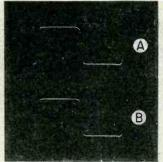
FIG. 5—Square wave (1 mc) displayed directly (A) and via amplifier (B)
