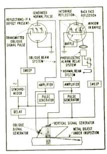
FIG. 2—Oblique and vertical signals insure that false indications do not result when using ultrasonic inspection techniques
