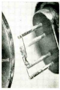
Automatic electrode-attaching machine under the watchful eye of R. P. Riesz of Bell Labs displays colored lights and meter readings that monitor progress of junction. Gold wires attached between junction and output terminals (right) shown magnified many times and compared with edge of a coin (Continued on page 14)
