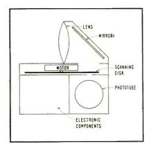
FIG. 4-Method of using mirror
