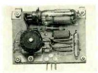
Plug-in panels produced by dip-soldering for squelch circuit (left) and a-f amplifier
