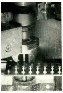
Drilling head in position
