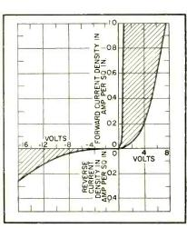
FIG. 14—Effect of temperature on titanium-dioxide cells. Shading shows range.
