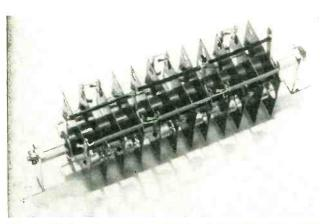
FIG. 7—Stacked germanium rectifiers on radiating fins, rated 70 v rms input per cell and 0.5 amp d-c output to resistive load
