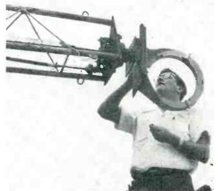
FIG. 2—Panning head and driver shafts. Ring mounted on plate holds transmitter and dish antenna
