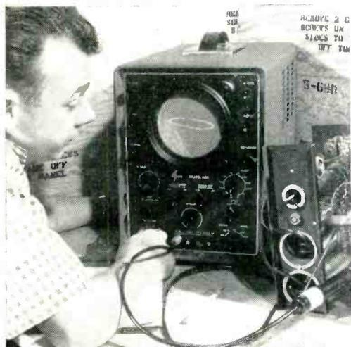
Oscilloscope incorporating triggered sweep
