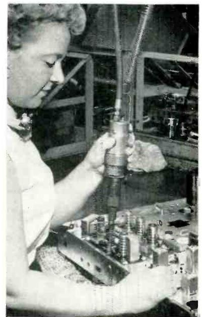
Driving mounting screw into sound circuit board of color-tv set. The board already installed directly behind serves as the picture i-f section
