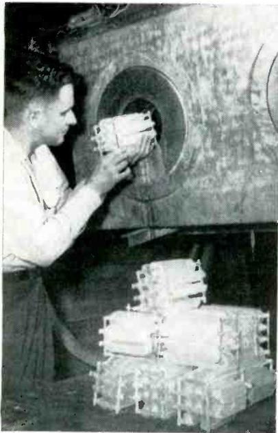
Removing batch of half-pound grown quartz crystals from Clevite autoclave. All crystals are essentially identical in shape, weight and orientation
