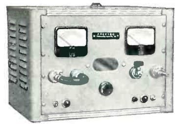
bench cabinet with all controls and gages conveniently located on the front panel. The portable, versatile instrument is suited for altitude test chambers, evacuation of tubes, and leak detection of mechanical and electrical components.
