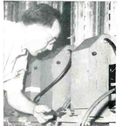
Method of repositioning insertion head laterally, after first loosening bolts of locking clamp just below transverse screw
