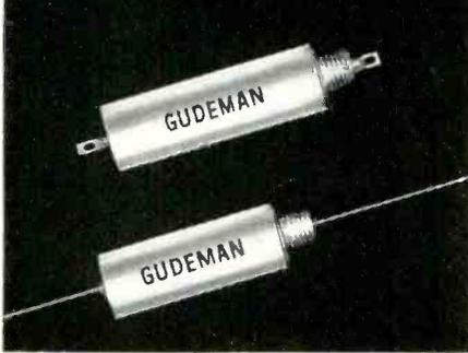
The Gudeman Feed-Thru Capacitor, Types 271 and 272, is a three-terminal component designed to be used for R.F. Interference suppression in a manner similar to a low pass filter. The typical insertion loss characteristics for these Feed-Thru Capacitors when measured in a 50 ohm line are in accordance with MIL-Standard 220.
