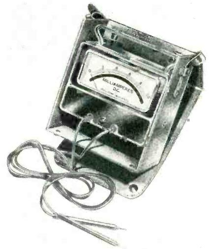
vide up to 6 ranges with a multiplier switch. This switch also protects the meter movement when set in transit position by damping the meter movement and thereby giving additional protection during storage and transit.
