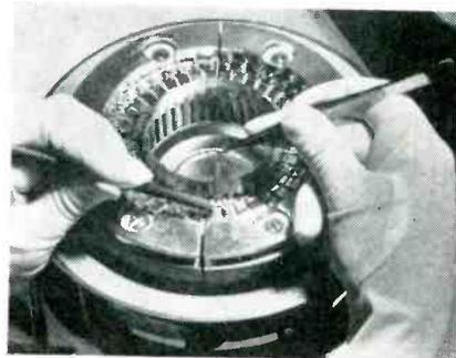
Typical of the step-by-step sequence of operations in assembling a beam-power, water-cooled RCA tetrode for use in uhf television is that of placing cathodes in position with tweezers. As shown in the photograph, the tool in the left hand is used to depress the pantograph cathode spring to which the cathode is clipped
