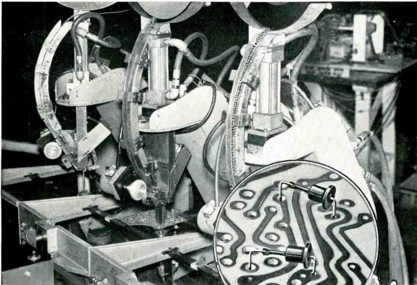
**AUTOMATIC ASSEMBLY**, using the new G-E Silicon Rectifiers, is made possible by the Axial Lead design. There is no heat sink required, no troublesome screw terminals. Leads slip easily into the board, and dip-soldering quickly completes the assembly.
