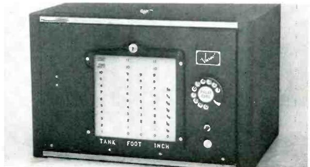
Receiving station for liquid level pulse code telemetering system
