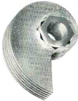
Spacing the parallelism of a special tuning condenser for electronic test equipment had to be held to very close tolerances. "Use of the Kodak Contour Projector," the company reports, "permits economical measurements of parallelism to an accuracy impossible to obtain by other methods."
