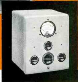
New Model 193A Ionization Gauge and Model 192A Ionization Gauge Amplifier provide a convenient, accurate and dependable method of monitoring pressures from  $10^{-4}$  to  $10^{-7}$  mm Hg. The ion gauge can operate for months without attention; the cost and inconvenience of burned out gauges, poisoned cathodes, grid heating, etc., is eliminated.
