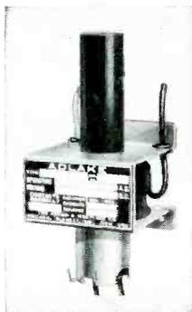
Adlake relays require no maintenance whatever...are quiet and chatterless...free from explosion hazard. Dust, dirt, moisture and temperature changes can't affect their operation. Mercury-to-mercury contact gives ideal snap action, with no burning, pitting or sticking. Time delay characteristics are fixed and non-adjustable.
