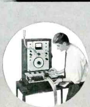
**SPECTRUM RECORDER** is integrated system for noise and vibration recording in one-third octave steps.
