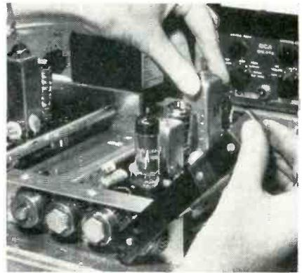
Moving lever to rotate gear train that brings spring clips into position to push wiring board down over contacts
