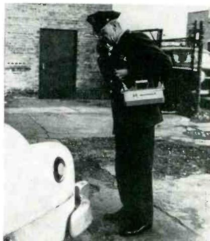
Among the growing list of transistorized firsts is the Motorola two-way portable communications set that employs transistors in i-f amplifiers and audio stages of the receiver. Battery drain is thereby reduced more than 70 percent
