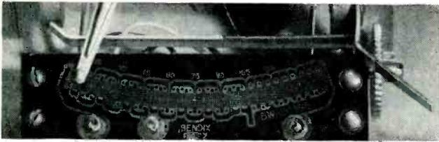
Baroswitch operated by the variation of atmospheric pressure in weather sounding radio telemeter switches the signal elements
