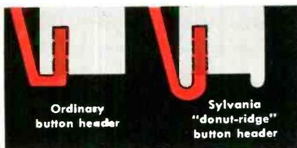
Here's a simple reliability test you can make yourself to demonstrate important advantages of Sylvania's "donut-ridge" button header. When you bend the tube leads as shown, ordinary headers will flake, chip, or crack: but leads bend cleanly around the "donut-ridge" header in Sylvania "Gold-Brand" subminiatures.
