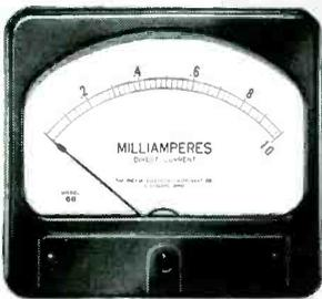
Molded-phenolic sealed cases for semi-flush or surface mounting. Has new miniature-type movement and extra long scale. DC scale length 3 3/4". AC scale length 3 3/8". Permits choice of two mounting stud locations for maximum versatility. Illumination technique permits easy bulb change from front panel. Also available without illumination feature.
