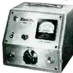
The WAVELINE Model 2200 microwave noise source—gas noise tube in combination with its Waveguide mount and power unit—provides a random noise source of known output level in the frequency range from 2,600 to 26,000 MCS. Throughout this range it also functions as an untuned termination.
