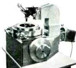
This famous microscope designed for the Univ. of Calif. and Naval Research Lab.—the same precision instrument which confirmed the discovery of the anti-proton—is now available to other colleges and research centers. Stage noise of less than 0.1 micron guaranteed in X, Y and Z traverses. Hydraulically controlled Z traverse. Binocular head and basic optics included. Automatic programmer optional. Price \$5,500.
