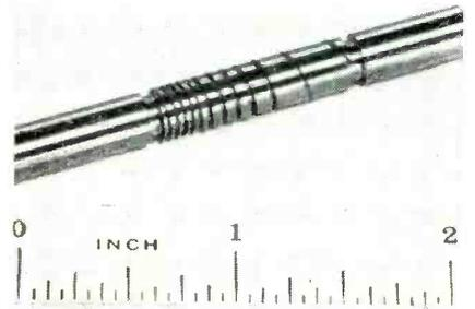
Sample screw cut with lathe attachment. Screw pitch is determined by cam
