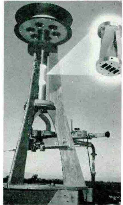
Four-waveguide twisted section, shown in inset at upper right, is mounted within tube supporting antenna of instantaneous direction finder that receives radar signals from all directions simultaneously over wide frequency range to determine direction of enemy pulsed radar
