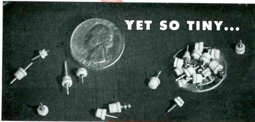
Unbelievably so. A dozen of these subminiature stand-offs and feed-thrus fit comfortably on a quarter. Sizes from .093" to .179" bushing dia. All due to the proper application of Teflon, the "miracle insulator", by the pioneer and specialist—SEALLECTRO!
