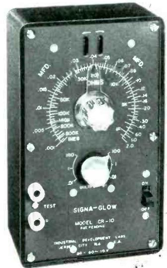
convenient scale divisions. The unit uses no batteries, is always ready for use by plugging into a 115 v 60 cycle outlet.
