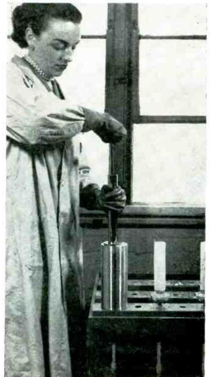
Metal can provides support for applicator while pushing down on plunger to force foam into antenna cavity. Scotch tape holds paper in position on antennas awaiting filling, to prevent surplus foam from overflowing down outside
