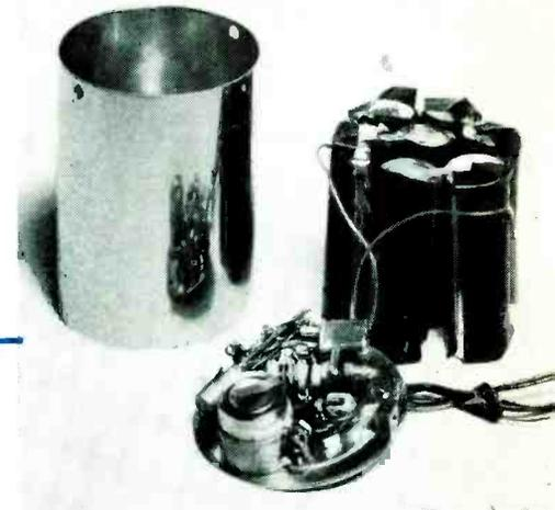
Transistor oscillator for satellite tracking is shown with silver-cell battery pack. Single high-frequency transistor is at rear center of plate
