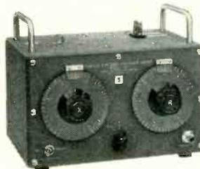
**Impedance Meter, Line Fault Analyzer**
