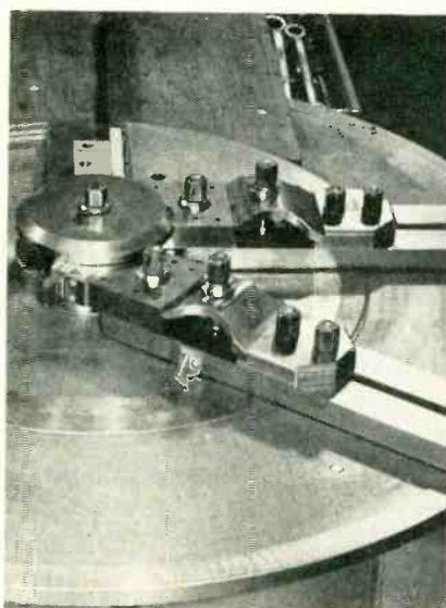
FIG. 4—At the start of bending operation, moving arm at right foreground is manually moved clockwise to bend tubing held down by circular top plate at center of table
