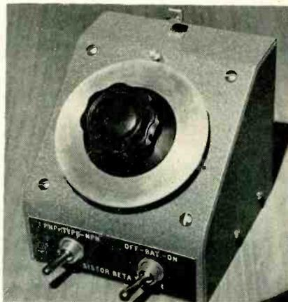
Transistor beta tester with calibrated and engraved dial
