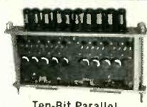
Ten-Bit Parallel Output (Serial Input) Using Magnistors
