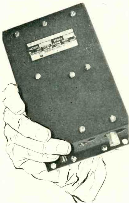
An extremely rugged unit designed for high-shock impact and extreme environmental conditions. Subminiaturized and crystal-stabilized.
