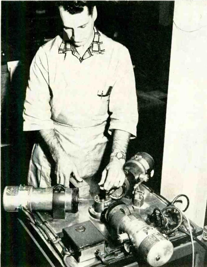
THREE No. 56 holes are simultaneously drilled 120 degrees apart in the stainless steel housing of a servo motor while the operator holds the housing in position on a centering fixture, in a drilling setup developed by the Mechatrol Div. of Servomechanisms, Inc., Westbury, N. Y. The new setup has cut drilling time to one-third and greatly reduced breakage of the small drills.
