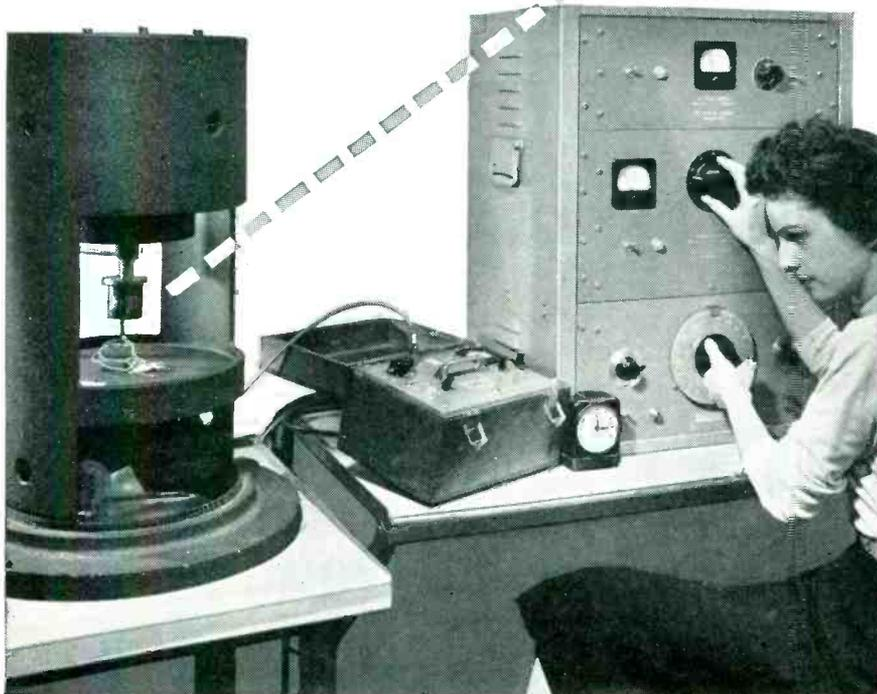
Vibration... with frequencies up to 500 cycles per second and up to 15 G's... might prove to be a shattering experience for some servo motors. But *not* for a G-M Servo!
