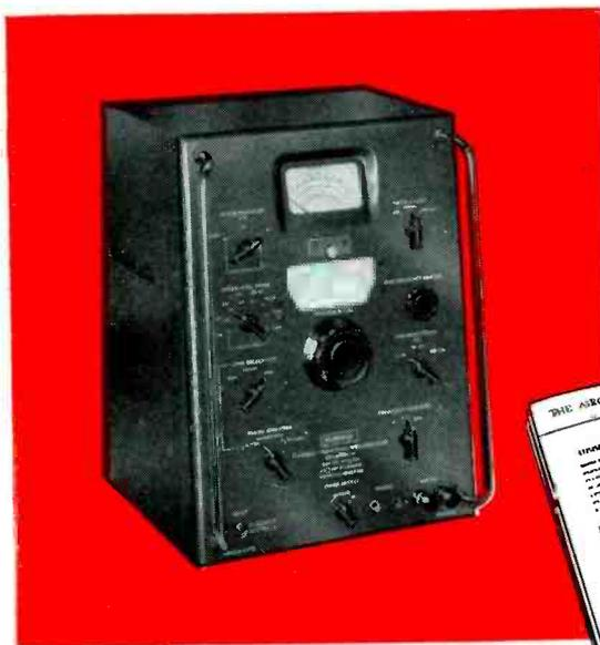
The Muirhead-Pametrada Wave Analyser covers the frequency range encountered in vibration tests of aircraft engines—whether pure jet, turbo prop or piston.
