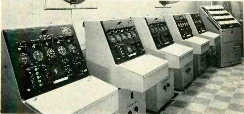
Five monitor consoles and address board (right) used for assigning identities to aircraft at Tacan data-link ground station. Each console displays complete information for a selected aircraft as well as ordered condition
