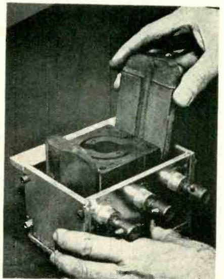
Assembling parts to be bonded in special jig. Thumbscrews on side and at far end provide all the contact pressure needed
