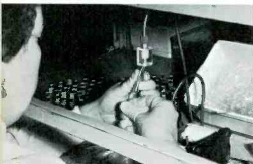
**Visual inspection**—visual inspection criteria as outlined in MIL-E-1C is applied to Guided Missile Tube production. This highly stringent and definitive spec helps to insure optimum reliability.
