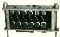
Six-Bit Digital Comparator Using Magnistors
