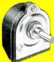
**TYPE H**—Industrial potentiometer. Rated 5 watts at 40°C. Total resistance values from 50 ohms to 2 megohms. Operating life in excess of 100,000 cycles with less than 10% resistance change. Less than 5% change after 100 hrs. at 40°C and 98% humidity. Max. voltage 750 v, d-c.
