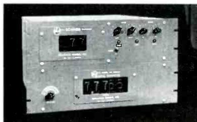
Input scanners used with NLS digital voltmeters or digital ohmmeters provide for automatic scanning of many inputs and when used with data recorders provide complete automatic systems.
