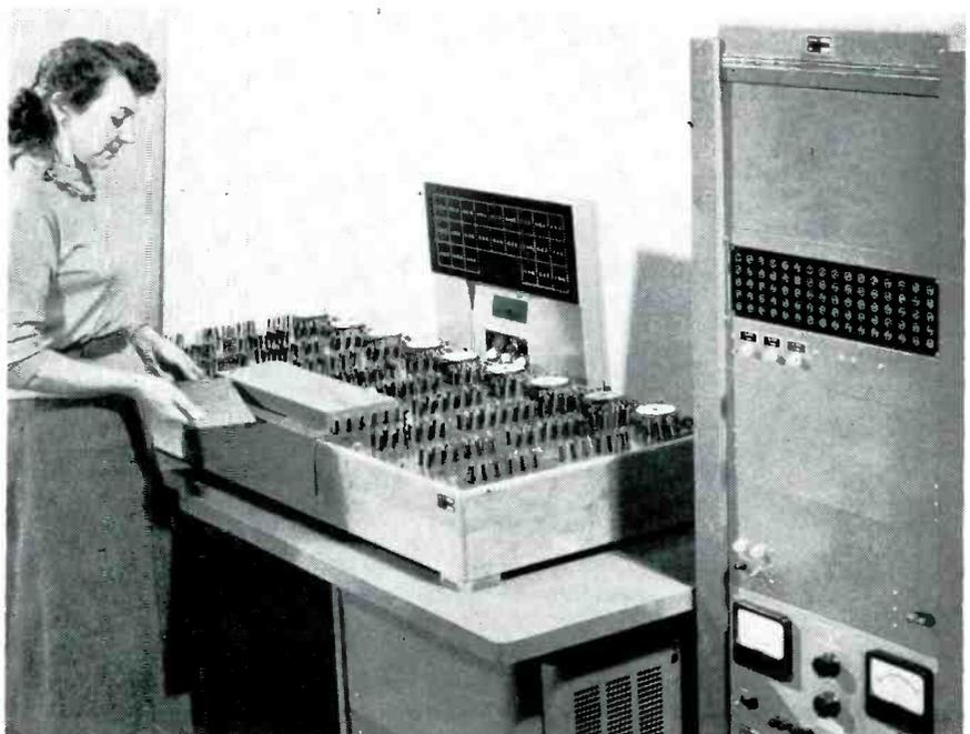
Inserting punched card which controls programming for measuring d-c resistance values of windings in up to 24 transformers. Hooks on ends of test leads speed connecting
