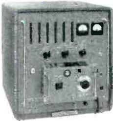
**-hp- 524B Electronic Counter.** Regarded by many engineers as the world's finest electronic counter, **-hp- 524B** with plug-in Frequency Converters measures frequency 10 cps to 220 MC; with **-hp- 540A** Transfer Oscillator measures frequency to 12 KMC; with **-hp- 526B** measures interval 1  $\mu$ sec to 100 days; with **-hp- 526C** measures period with greatly increased accuracy.
