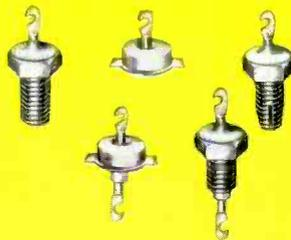
**FEED-THRU & STAND-OFF CAPACITORS**—In standard nominal values from 4.7 to 1000 mmf. No parallel resonance effects up to 1000 mcs, as normally encountered with tubular types. Rugged construction, with solder tabs or screw thread mountings.
