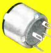
**TYPE F**—Rated 1/4 watt at 70°C. Diameter 1/2", length approx. 1/2". Total resistance values from 100 ohms to 5 megohms. Standard tapers. Made for screwdriver adjustment. Terminals and grounding lug, also used for mounting, spaced for 0.1" printed circuit layout. Non-magnetic.
