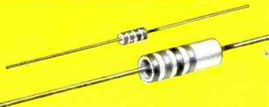
**HERMETICALLY SEALED RESISTORS**—Hot-molded composition resistors sealed in ceramic tubes for protection against humidity and moisture. Type ES rated 1 watt; Type TS rated 1/8 watt. No-load operating temperatures: ES, 165°C; TS, 110°C.
