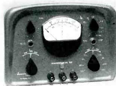
to 500. The circuit employs 1-percent calibrating and attenuating resistors and a 2-percent meter movement. The instrument features etched circuitry, interlocking selector switch wiring, and a test socket which accommodates linear or triangular pin configurations. The power supply consists of mercury cell batteries with an operational life of 1,000 hours.
