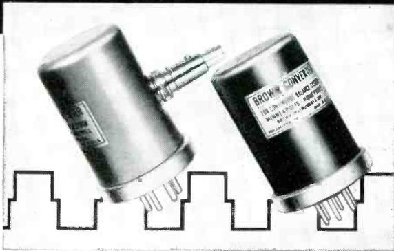
**CONVERTERS**—Handle d-c signals as small as  $10^{-8}$  volt. SPDT switching action. Sensitive, stable performance. Ideal for computers, servomechanisms, balancing circuits. Available with special features such as fungus proofing, grounded housing, mica-filled base, various contact percentages. Weight: 10 ounces. Driving coils in 60, 40 and 25 cycle converters are energized by 6.3 volt a-c. 400 cycle uses 18 volts. Other coil ratings as follows:
