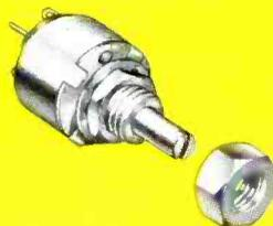
**TYPE G**—Rated 1/2 watt at 70°C. Diameter 1/2". Total resistance values from 100 ohms to 5 megohms, in standard tapers. Made with lock type or plain bushings; with plain, flatted, or slotted shafts up to 2 1/2" long. All metal parts nonmagnetic. Available with built-in line switch.
