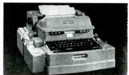
Flexowriter equipment for typewriting of data and simultaneous paper tape punching may be used with NLS digital voltmeters and ohmmeters. NLS Flexowriter converters are provided for this purpose.
