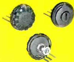
**TYPE T**—Rated 1/2 watt at 70°C. Total resistance values from 100 ohms to 5 megohms. Standard tapers. Molded plastic cover also serves as actuator. This makes unit extremely flat and compact. Screw-driver slot or knurled surface. Operating life in excess of 50,000 cycles.
