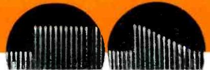
Two-percent change in 60c voltage input (left oscillogram) is corrected in 12c or 0.2 sec (right) by G-R Line-Voltage Regulator.
