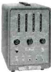
**-hp- 521A Industrial Counter.** Direct reading, 1 cps to 120 KC. Measures frequency, speed, rpm, random events, other phenomena with transducers. Time of count 0.1 or 1 second, variable display time. Sturdy, rugged, simple to use, low cost. Also **-hp- 521C**, 5 place registration, crystal controlled time base.
