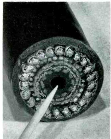
Contrahelical-wound cable having hose in center for air or hydraulic fluid used to release umbilical plug when missile is fired from launcher
