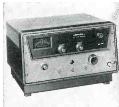
is capacitor tuned. Band switching is by single knob which simultaneously selects the proper grid coil and plate tank inductance. The output circuit is a pi-network for fixed 52-ohm output impedance. High voltage for plates and screens is obtained from two 866A rectifiers while screen voltage is regulated by two OB2 and one OA2 tubes.
