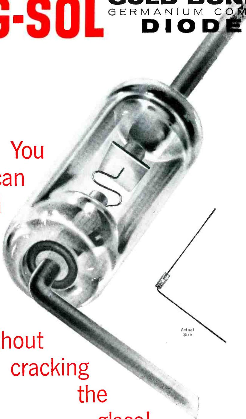
Here's the answer to the problem of how to make computer diodes so the lead wires can be sharply bent close to the glass body without cracking the end seal. It's the "ring seal" design, an exclusive Tung-Sol construction feature embodying a metal collar fused into the end-seal. The collar absorbs the strain of lead wire bends, thereby preventing damage to the diode enclosure.
