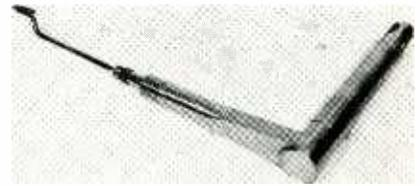
Filer fits standard flexible shaft to provide reciprocating motion of hard filing
