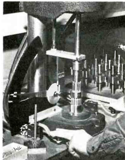
Pointer of indicator, at center line on scale, indicates that stack is at desired height. Pointer is actuated by downward projection bolted to ram of press. For safety, operator must press down two valves as shown when operating press
