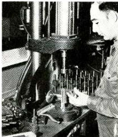
First step in assembly, after central arbor has been dropped into fixture, is positioning of heavy end spider over arbor and slot alignment pins
