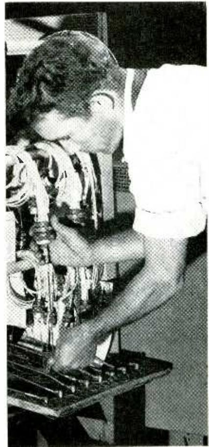
**STEP 5**—Applying rubber-band anchors to hold connectors steady for potting
