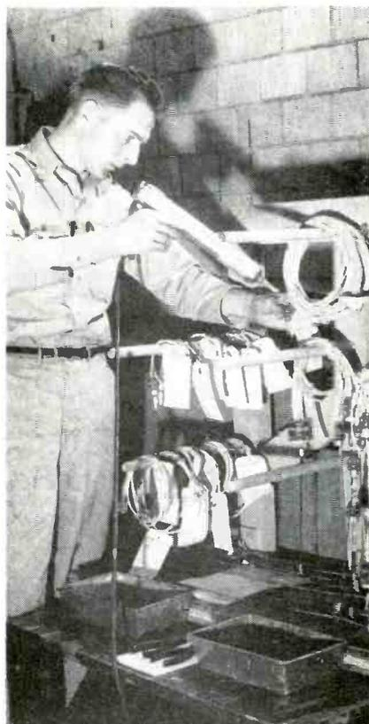
**STEP 7—Filling connector by using air-operated potting gun**
