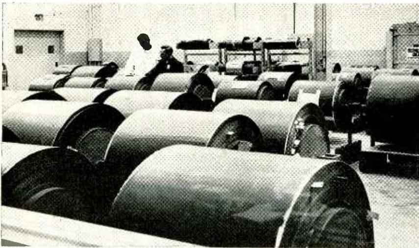
**OVERSIZE ROLLS** of magnetic tape will not be here long before slitting and packaging at 3M plant, as demand rises steadily and . . .
