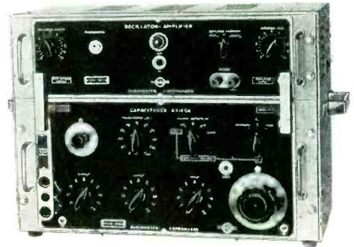
Shielded cables used without introducing errors. Measures directly single capacitances from complex capacitance networks • The type CMB1 bridge is unique for all measurements on tubes, cables, transformers, etc. Built-in 1000 cps oscillator and detector amplifier.
