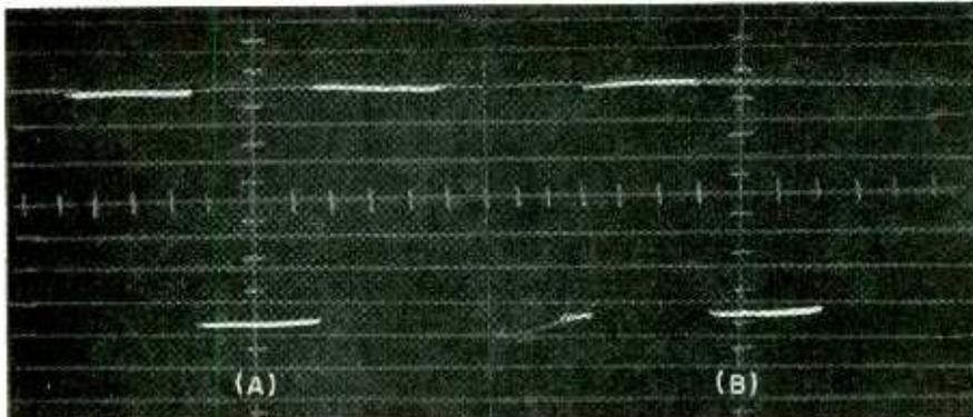
FIG. 5—Control voltages of 5.5 and 52 v applied to multivibrator of Fig. 3 produce 6.500 (A) and 600- $\mu$ sec (B) outputs respectively
