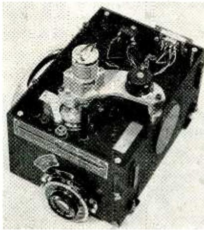
**Gearcase for the recording camera**
