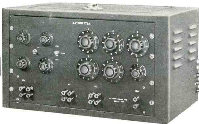
The Transformers, Inc. Ratiometer is a precision instrument to measure any voltage ratio from 0.000001 to 1.111111. Transformer ratios can be accurately measured at "no load" and under full load. Two models are available:
