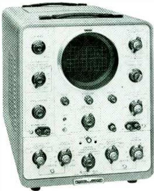
**High Frequency Cabinet Oscilloscope, Model 150A.** Covers dc to 10 MC with new reliability and convenience. Two plug-in preamplifiers for high gain or dual channel measurement (see below). 24 direct-reading sweep times; sweeps 0.02  $\mu\text{sec}/\text{cm}$  to 15 sec/cm. Universal automatic triggering; one preset condition insures optimum triggering. \$1,100.00.
