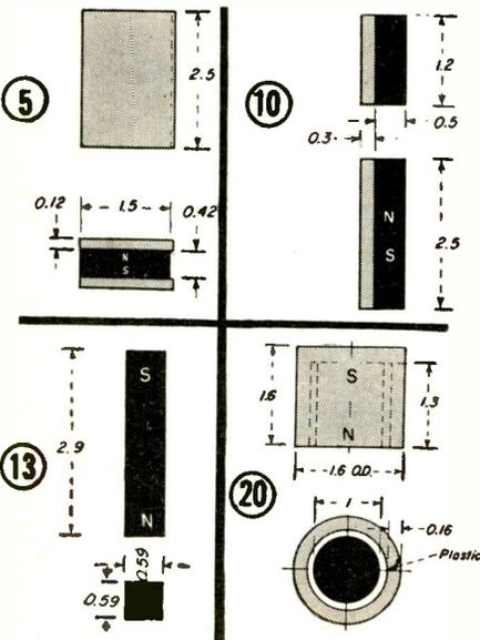
FIG. 1. Four of the basic designs for holding magnets. From these designs other holding magnets, geometrically similar but with any desired pull force, can be derived. Magnetic material is in black, steel in gray; all dimensions are in inches. Design numbers correspond to those on effectiveness curves and in Performance Table II.
