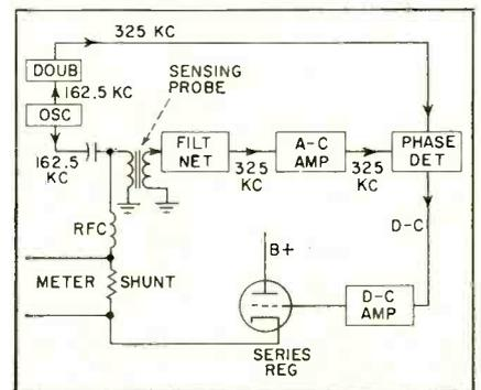
FIG. 3—Functions of magnetometer elements
