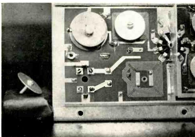
Closeup of i-f amplifier shows the aluminum vanes, mounted on steel screws, used for tuning the coils
