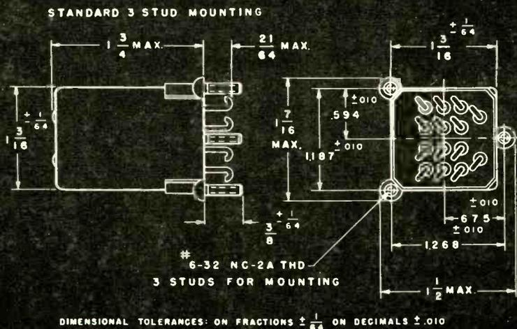
The Allied CH-12D Relay was developed to meet the more rigid requirements of vibration, shock, temperature, rupture and overload conditions of the latest MIL spec. This relay is constructed with the latest improved materials and processes available. This relay is available with other mounting arrangements, such as 4 mounting studs, 2 mounting studs or holes with Allied MHY-12D mounting dimensions. For additional information write for Bulletin CH.
