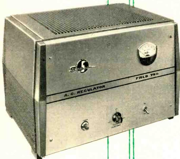
This *new* type of AC Regulator, the Sorensen FRLD 750, features the ability to reduce line distortion below 0.35%, with *exceptionally* fast response time. Transients caused by line or load changes are suppressed within less than one cycle.
