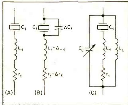
FIG. 2—Basic crystal circuit (A), lower impedance version (B) and its use with tuned circuit
