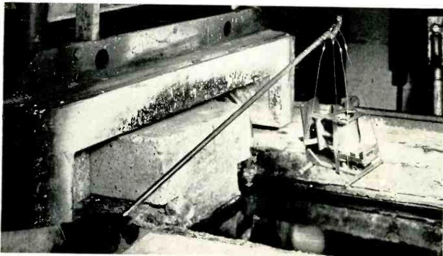
Klystron tube mount in holding fixture is lifted from molten salt bath. Operator uses "fishpole" to avoid 1,100 F heat
