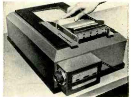
Silicon-rubber squeegee is used after solder bath to provide smooth coating on conductors
