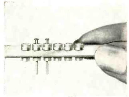
Feed-thru capacitor saves space and lowers assembly cost
