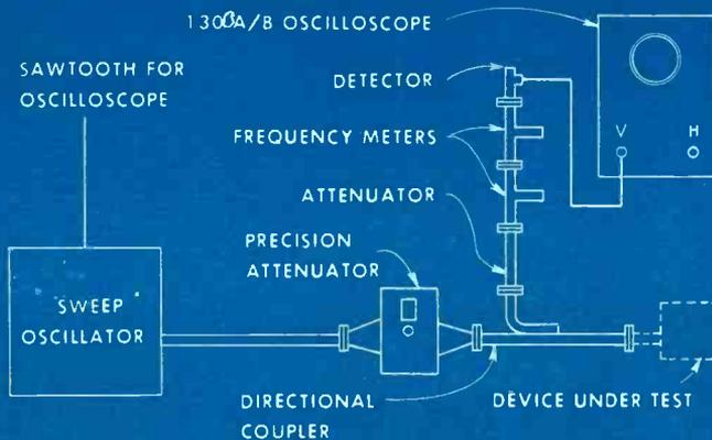
◀ Figure 1. Arrangement for high speed microwave measurement to provide rapid visual display with -hp- 130A/B oscilloscope. Can be used for G, J, X and P bands.
