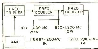
FIG. 4—Additional frequency-doubler circuit in uhf unit handles 1,700-2,400-mc band of the exciter
