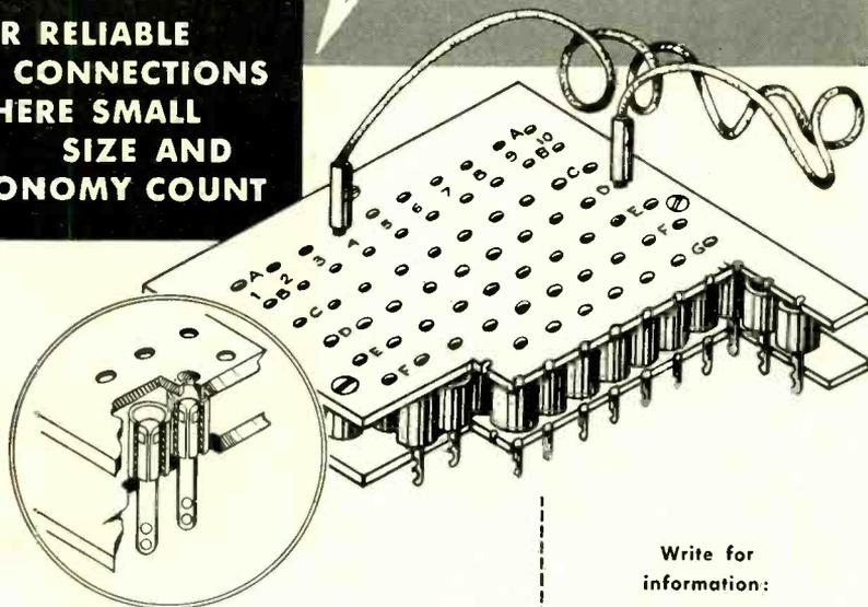
Vector Patch-Boards provide simple, economical units for multiple-connection, single conductor patching. Useful for low cost computers, test boards and a multitude of connecting applications. Receptacles are 0.265" on centers and take .087-.091 diameter plugs. Patch cords also available. Standard boards available or readily made to size required.
