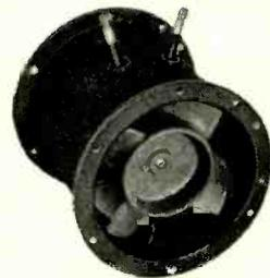
Small aluminum axial-flow fan. Capacity: 110 cfm @ 0.6" sp to 165 cfm, free delivery @ 7250 rpm. Write for Bulletin 3812.
