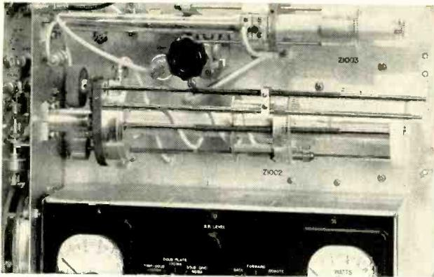
Closeup of uhf unit shows amplifier, tripler and doubler stages. Cavities are partially disassembled to show inner parts
