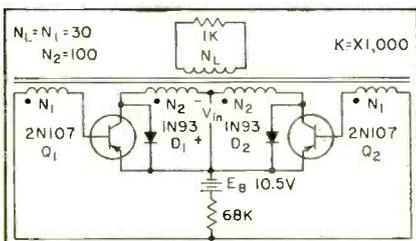
FIG. 1—Inverter is analogous to free-running cathode-coupled multivibrator
