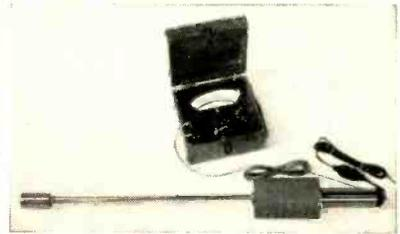
Rawson-Lush patented Rotating Coil type, now available with a wide range of coil sizes to give different sensitivities. New large coil type 726 indicates the Earth's magnetic field.
