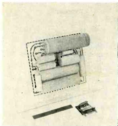
Components assembled on layout board give 3-D picture of completed unit
