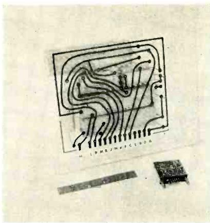
Board transparency makes taping the wiring pattern a simple procedure
