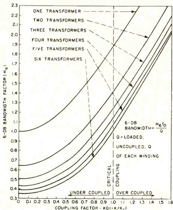
FIG. 3—Six-db bandwidth factor for transformers with two identical coupled circuits
