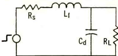
Where  $R_s$  is the internal resistance of the pulse source,  $R_L$  load resistance,  $L_l$  and  $C_d$ , leakage inductance and distributed capacitance, respectively. If the transformer is matched ( $R_s = N^2 R_L$ ), this circuit is valid for step-up and step-down transformers.
