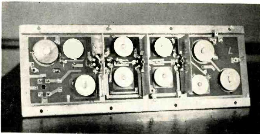
Photograph of i-f amplifier showing layout and spacing arrangement between the coils in the center of the strip. This arrangement greatly reduced d-c leakage
