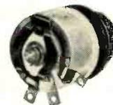
Functions smoothly under the most adverse conditions. Terminals of strong, corrosion resistant alloy, are permanently welded to winding form. Wound ring is made an integral part of the refractory base by vitreous enamel. Shafts are insulated. Three terminals permit use as potentiometer or rheostat.
