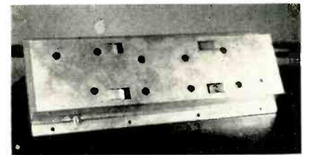
Details of shielding for i-f amplifier show punched chassis containing spring surfaces for good shielding contact
