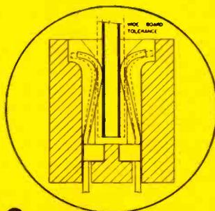
**3. WIDE BOARD TOLERANCE RANGE,** controlled and repeated insertion and retention forces are assured over card range thickness of .062 or .093 of +.010.
