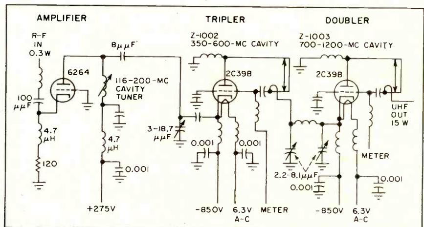
FIG. 5—Common-grid voltage tripler and voltage doubler of uhf unit are tuned with coaxial resonators. Input coil for r-f has five turns of number 20 wire with 0.25-in. diameter
