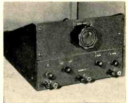
Front view of analyzer. Knob is used to control bias placed on input wave
