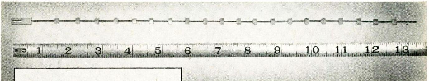
This precisely-threaded rod (used in calculating machines) is of .047" dia. stock, 120 pitch, with continuous threading along its entire 12" length. Threading accuracy and critical dimensions are measured and checked speedily and efficiently with a J&L Comparator.
