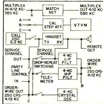
FIG. 6—Party-line feature on service channel in level panel permits voice exchange between link stations
