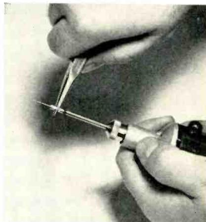
Drill extension holds drills without solder so that drills may be changed with pair of pliers
