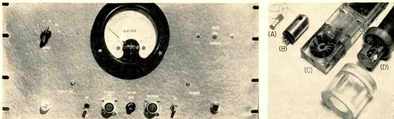
Front panel includes variable controls, meter and connections for optional devices (left) Sensing probes (right) include basic unmounted element (A), 10-gauss uncooled model (B), 100-gauss convection-cooled version (C) and 300-gauss conduction-cooled unit (D)
