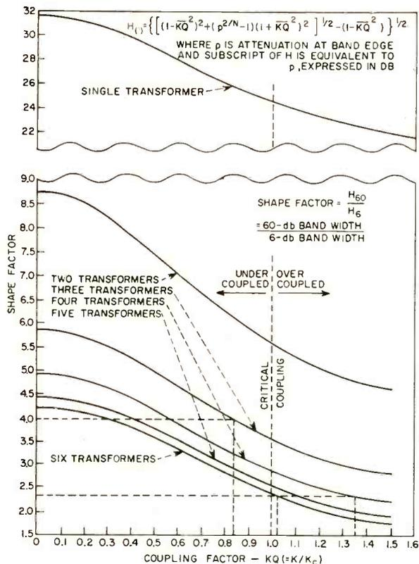
FIG. 1—Shape factors for single and cascaded double-tuned transformers vs coupling factor. Curves are solutions of the equation shown which also applies to Fig. 2 and 3
