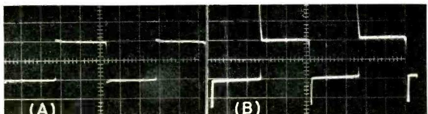
FIG. 2—Diodes of modified inverter clip spikes of output (A) while original inverter spikes appear (B). Scales are 1 v per amplitude division and 0.5 millisecc per time division
