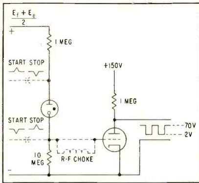
FIG. 1—Gating circuit may use 6AV6, ½12AX7 or other triode types to produce low repetition rate pulses
