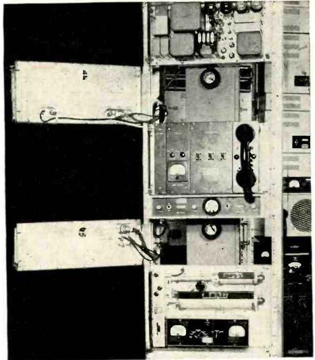
Dust covers are removed from exciter and two chassis are hinged out to show cabling and air connections
