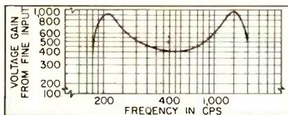
FIG. 3—Two-speed servo amplifier voltage gain-frequency characteristics.
