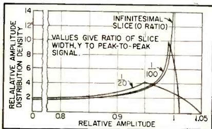
FIG. 5—Theoretical amplitude-distribution of a sine wave for different ratios of slice width to peak-to-peak sine-wave amplitude as used in technique described
