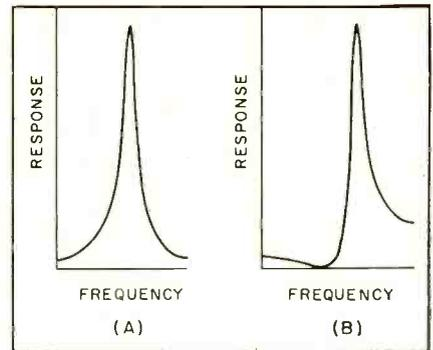
FIG. 3—Crystal circuit response when paralleled by resistor (A) and with  $L_1$  or  $C_1$  misadjusted
