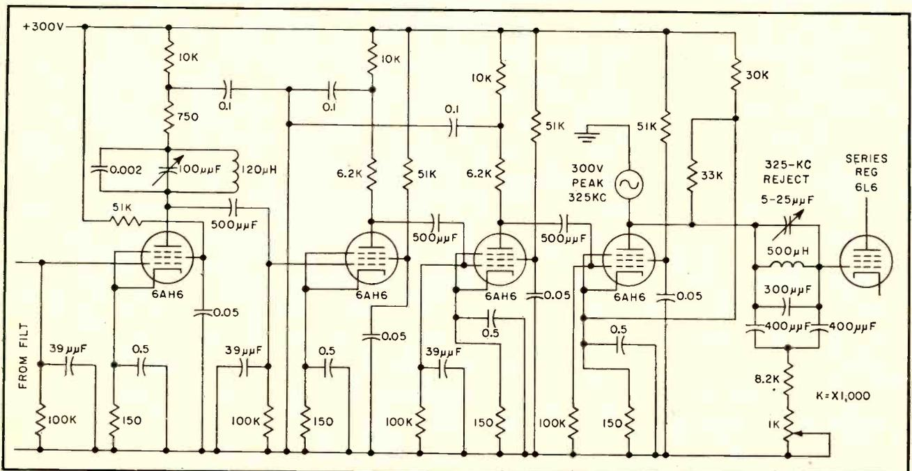
FIG. 5—Circuit details of the a-c amplifier, phase detector and d-c amplifier elements of the magnetometer system
