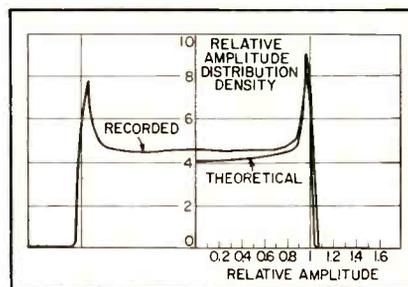
FIG. 6—Theoretical and recorded distribution density for a sine wave. Slice width  $\Delta y$  to peak-to-peak input ratio at 1/20
