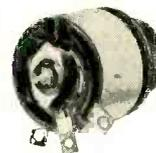
Featuring porcelain-vitreous enamel construction, Type AM rheostats are exceptionally rugged, compact and possess excellent heat dissipating characteristics. Resistive element is wound on a flat, pure mica form, placed within a refractory base and completely embedded in vitreous enamel.
