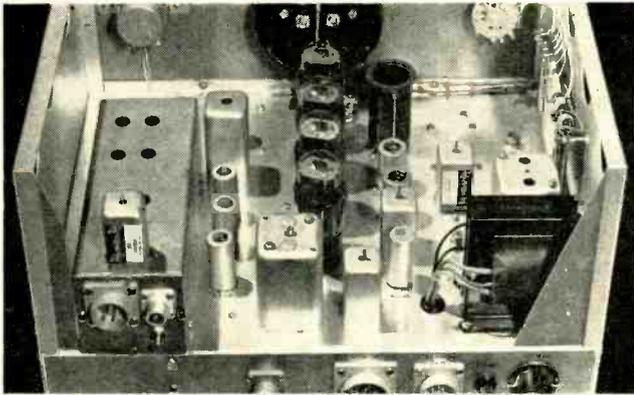
Top chassis view shows standard component used in the construction of the magnetometer
