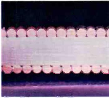
**Large, gas-tight contact areas.** Just four turns of wire produce a contact area greater than the cross-sectional area of wire. Surface adhesion at contact areas prevents damage from severe temperature changes, humidity, corrosive atmospheres and vibration.
