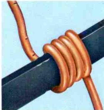
**High-pressure, metal-to-metal contact.** After wrapping, cold flow of copper causes pressure in center of contact area to drop from 100,000 psi. to about 29,000 psi. The metal then stabilizes . . . pressure remains constant. Keller "Wire-Wrap" tools produce a clean metal-to-metal contact. As connection ages, it becomes mechanically stronger due to solid state diffusion.
