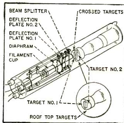
FIG. 1—X-ray tube, type 1, has crossed targets. Type 2 has a roof-top target
