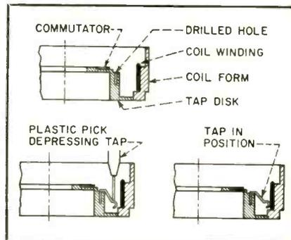
Method of springing tap into position against pot coil
