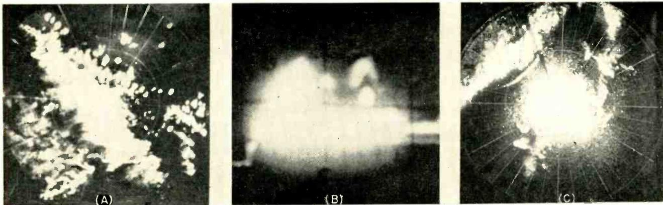
Radar displays of several angel types. Lower left section of (A) is lightning echo. Circular echo under inverted-U mantel echo of (B) was rising at 250 ft/min. Thin diagonal line in upper left region of (C) is echo from clear sky just ahead of squall line
