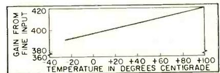
FIG. 5—Two-speed servo amplifier voltage gain-temperature characteristics. Gain at room temperature is about 400
