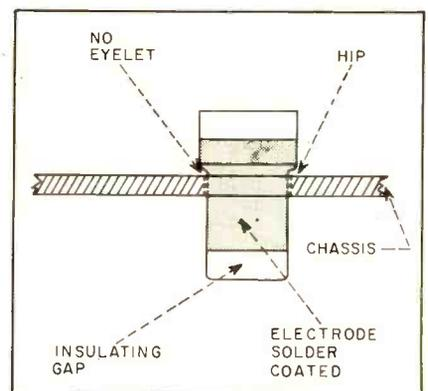
Hip keeps capacitor at uniform height and snug in hole
