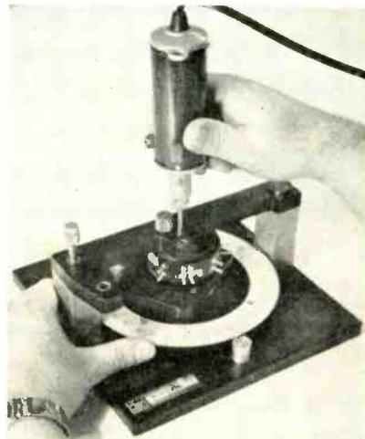
Tap hole is drilled through bushing after pot is positioned in drill jig
