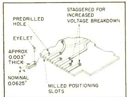
U-shaped copper contact strips anchor printed circuit conductors at mating edge of board
