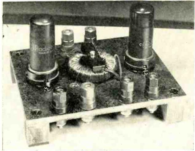
Component layout indicates physical relationship and relative size for transistorized inverter (left) and tube inverter (right)
