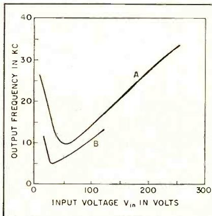
FIG. 7—Frequency characteristics for electron-tube inverter using separate half-tubes A and a single common cathode without grid resistors B
