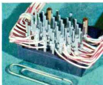
**Close terminal spacing.** Today's trend toward compact electrical assemblies naturally demands close spacing of terminals. The small diameter of the Keller "Wire-Wrap" tool tip permits close terminal spacing. In addition, a number of wires can be connected to the same terminal.
