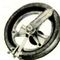
High temperature enamel affords maximum safety under overloading. H-H bus-bar construction provides ample resistance, ample safety under maximum current requirements. Constant pressure contact arm provides trouble-free operation.
