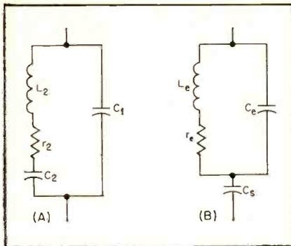
FIG. 1—Equivalent circuits for piezoelectric crystal. E-R version formulas for (A) to (B) are given in article
