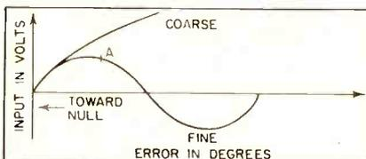
FIG. 4—Phase error voltage relationship between coarse and fine signals in the two-speed servo system. Switching between two signals should occur to the left of point A
