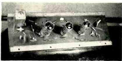
The i-f strip with the top shield removed (left). Shielding for the sound trap in the luminance detector circuit is taken care of by a small copper strip enclosing the trap on sides not adjacent to ground
