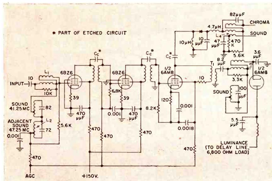
FIG. 1—Schematic diagram of the 41-mc i-f amplifier. Traps are printed on the same board with the wiring and other coils and are vane tuned
