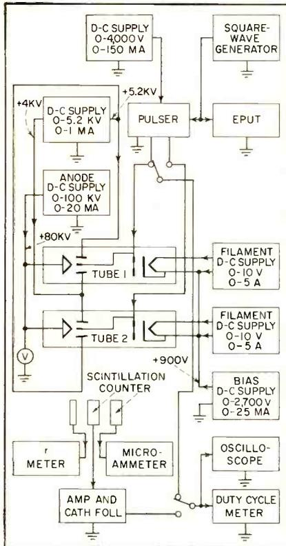
FIG. 3—Ultimate system uses two, type-2 tubes. Principal components are shown
