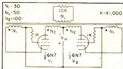
FIG. 6—Differential electron tube inverter gives best results when separate grid resistors are used
