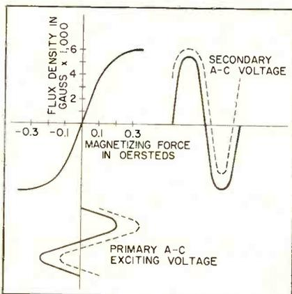
FIG. 2—Excitation level and magnetic characteristics of core cause secondary voltage to be rich in odd harmonics
