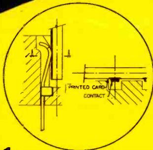
**1. NEW CONTACT DESIGN,** scientifically curved for minimum abrasion during repeated card insertion.
