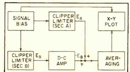
FIG. 2—Block diagram of amplitude-distribution analyzer. Analyzer effectively inspects only small amplitude interval of input wave. Input wave to be analyzed is biased and then amplitude gated by two clipper limiters, one samples positive slice and the other samples negative. Output is average voltage  $E$  of gated portion
