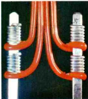
**No embrittlement or stress concentrations.** Embrittlement caused by change in metallic structure is impossible. No heat is used in making solderless wrapped connections. Elimination of stress concentration where wire joins terminal results in superior vibration life.
