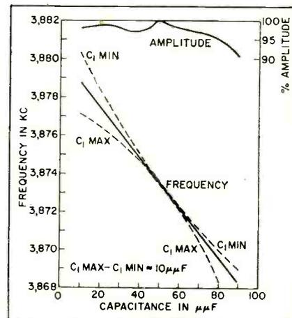
FIG. 5—Performance of variable-frequency crystal oscillator
