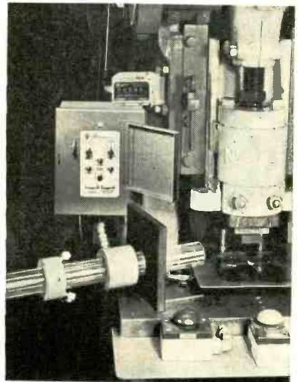
Punch press is stopped to avoid breaking die if punched piece is not ejected through r-f coil mounted on tube
