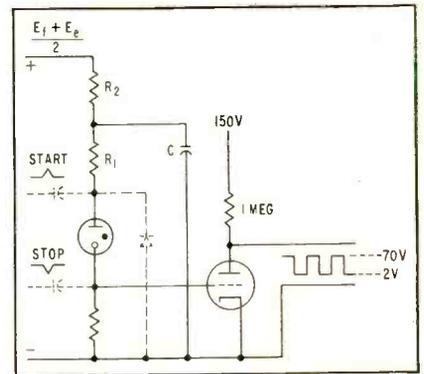
FIG. 2—If  $R_2$  is much greater than  $R_1$  and the reciprocal of time on is much less than  $\text{prf}$ , time on  $\approx 2.303 R_1 C \log_{10} (E_f + E_e) / 2E_e$ , while dead time  $= 2.303 R_2 C \log_{10} (E_f + E_e) / 2E_e$
