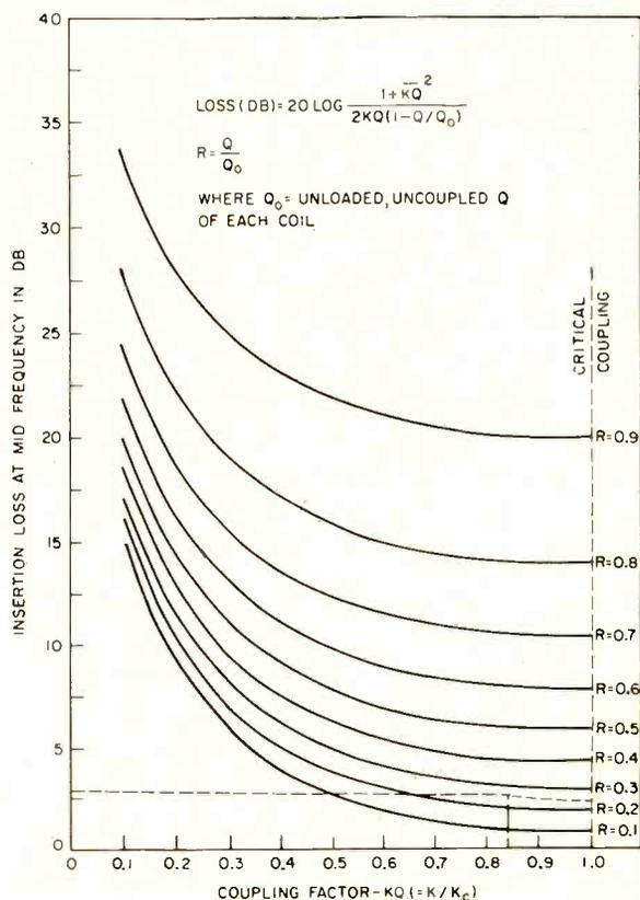
FIG. 4—Insertion loss of a single transformer at its midfrequency for varying values of the  $Q/Q_0$  ratio
