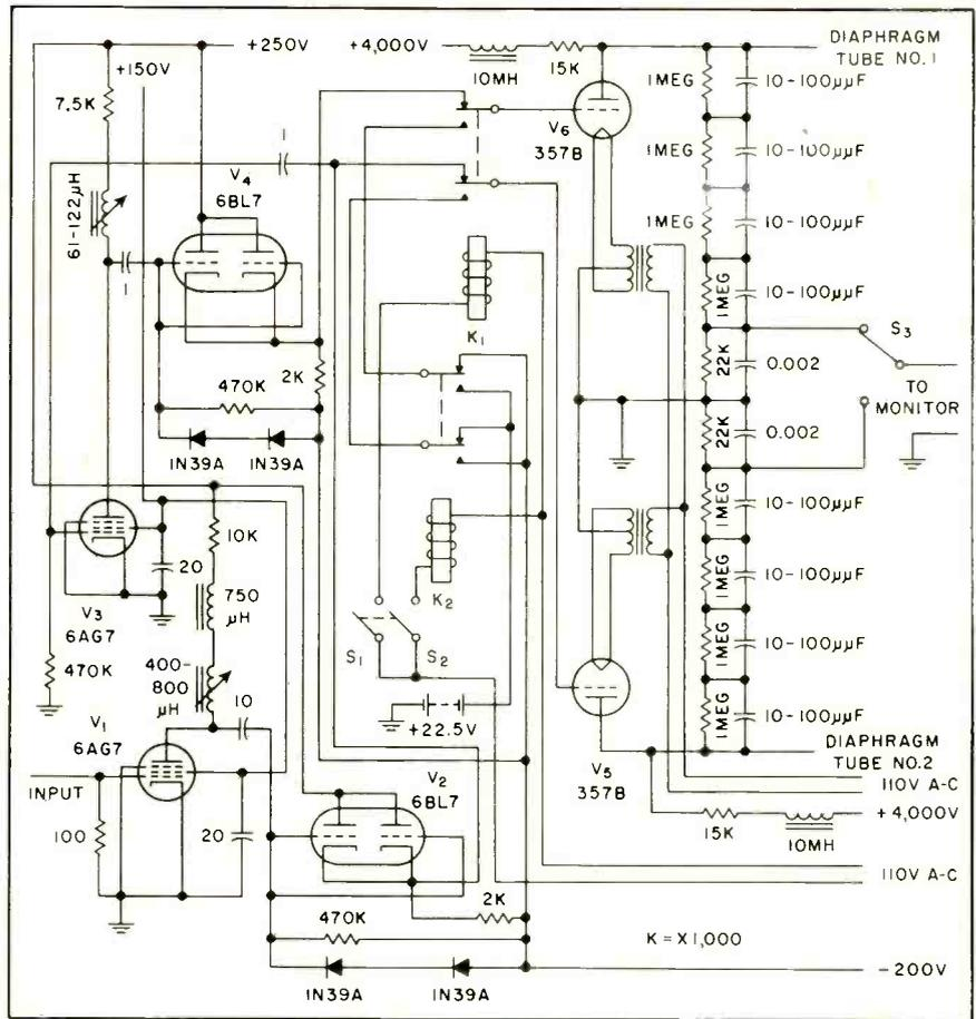
Since average anode current is a function of duty cycle, constant anode voltage is difficult to maintain with commercial X-ray high-voltage supplies. Commercially available power supplies are not capable of holding the instantaneous tube output sufficiently constant. This difficulty was overcome by installing a second X-ray tube. The diaphragms in each tube were pulsed alternately to maintain constant anode voltage and current.
