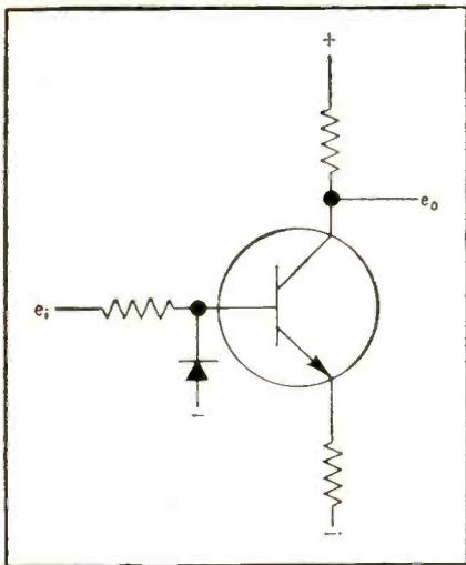
FIG. 2—If too much compensation results in this circuit, part of diode current can be bled to ground
