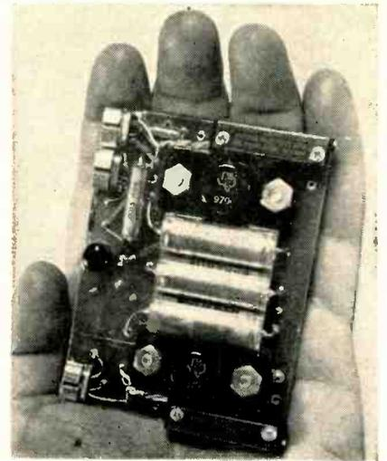
Transistorized servo amplifier can be held in palm of hand. Amplifier contains five transistors and four Zener diodes
