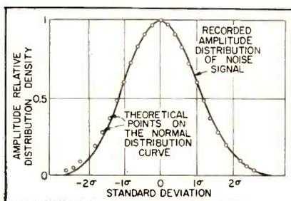
FIG. 7—Recorded amplitude distribution of the output of a random noise generator
