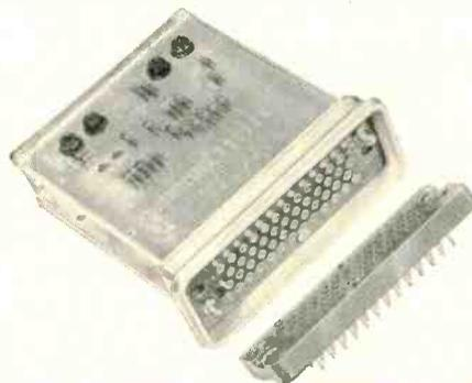
Continental Connector and New Closed Entry Contacts Used with Printed Circuit Application for Classified Intercontinental Ballistic Missile.
