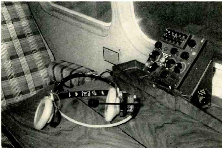
Radio monitoring facilities are provided for two passengers in a Dove airplane equipped to demonstrate electronic instruments. The equipment, made by Smiths Aircraft Instruments, Ltd., England, includes automatic radio beacon coupling and automatic approach on the instrument landing system. Portions of the autopilot are also installed in the cabin
