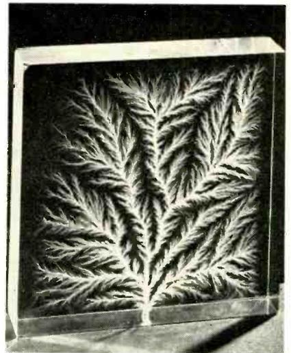
Mullard in England made this tree-like pattern with one of their linear accelerators. Electronics from the accelerator penetrated the polished surface of the plastic block causing a charge to accumulate inside the block. The charge was released by inserting a sharp pin in the bottom, resulting in the tree effect which shows the discharge path
