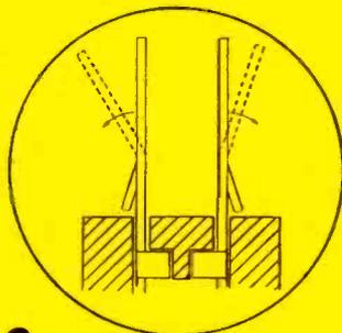
**2. CONTROLLED TERMINAL HARDNESS,** heat-treated beryllium copper permits flexibility in crucial areas maintaining maximum strength and no-creep.
