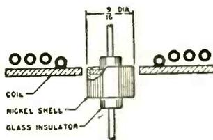
Concentrator-type coil creates high intensity, restricted heating at joint of nickel shell and tinned glass, thus causing solder to flow for permanent seal.
