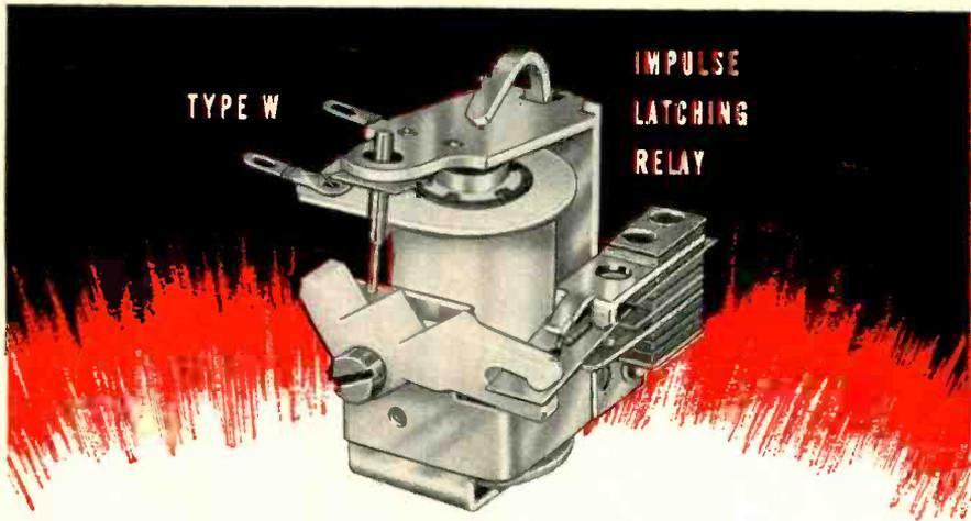
Features an insulated rocker arm activated by a single coil, instead of the usual two. Ideal for machine controls, appliances, positioning devices, remote TV controls and other applications where opposite switching is desired each time circuit is pulsed. Contact combinations up to 4 "C"; rated  $7\frac{1}{2}$  amperes @ 115 V. AC resistive.
