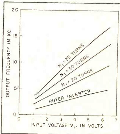
FIG. 4—Frequency characteristics of modified circuit (lowest curve) has components of Fig. 3. Remaining curves for differential inverter with  $N_1$  as parameter
