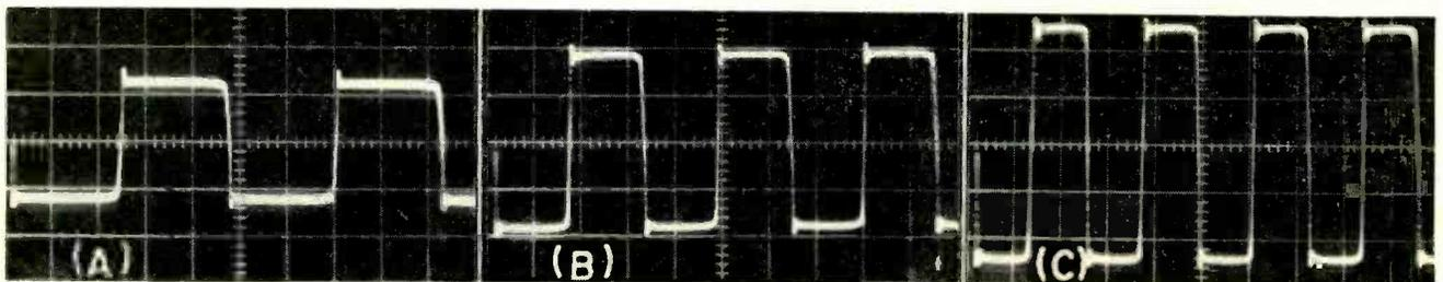
FIG. 5—Output waveform of differential inverter of Fig. 3 with  $0.01 \mu\text{f}$  capacitor connected between collector and emitter of each transistor to clip pip. Input voltage  $V_{in} = 3 \text{ v}$  (A),  $4.5 \text{ v}$  (B) and  $6 \text{ v}$  (C). Each waveform amplitude is  $2 \text{ v}$  per large division and time scale is  $50 \text{ sec}$  per large division
