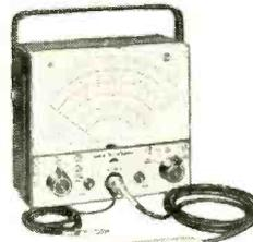
**Senior VoltOhmyst® WV-98A**—ideal for TV, radar and other types of pulse work. Provides accuracy of  $\pm 3\%$  on both ac and dc measurements. Measures directly peak-to-peak values of complex wave forms and rms values of sine waves. Features  $\pm 1\%$  multiplier and shunt resistors, a 2% meter movement,  $\pm 3\%$  on AC and DC voltages. Less than  $\pm 1\%$  tracking error. Large (6½" w.) full-vision meter provides easy readings. \$79.50\*
