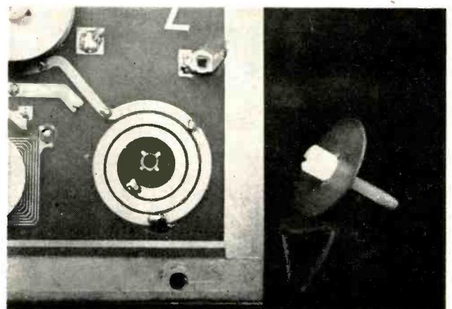
View of the bifilar trap with vane removed shows nylon-screw mounting hole. Screw and vane are at right
