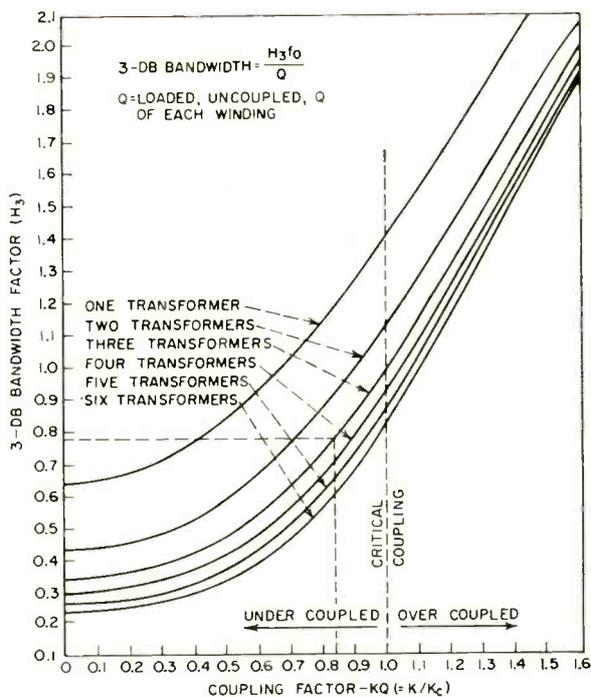
FIG. 2—Three-dB bandwidth factor for transformers with two identical coupled circuits
