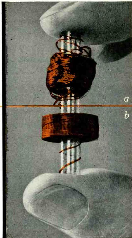
**THE PROBLEM:** To develop a solderable film-coated wire without fabric for winding universal lattice-wound coils without adhesive application.
