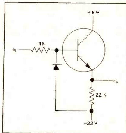
FIG. 1—Germanium diode with 4,000-ohm input resistor compensates drift in silicon transistor amplifier
