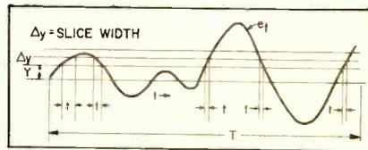
FIG. 1—System is based on the principle that the amplitude distribution density plot is the ratio of  $\Sigma t$  to  $T$
