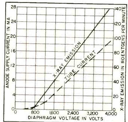
FIG. 2—Cutoff characteristics of the second X-ray tube described in this article
