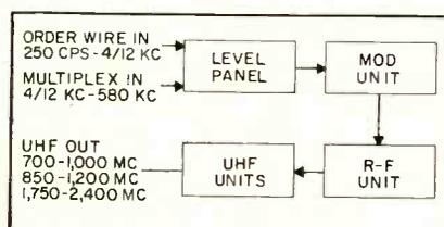
FIG. 1—Exciter consists of four blocks plus power supplies, switching panels and accessories
