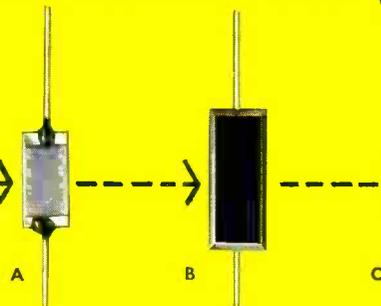
The construction of the  $\frac{1}{4}$ ,  $\frac{1}{2}$ , and 1-watt resistors is identical. At left is an enlarged view of the metal alloy grid, mounted on glass, that forms the resistance element. (A) Actual size of 1-watt element, (B) encapsulating epoxy resin body, (C) finished unit hermetically sealed in ceramic tube.
