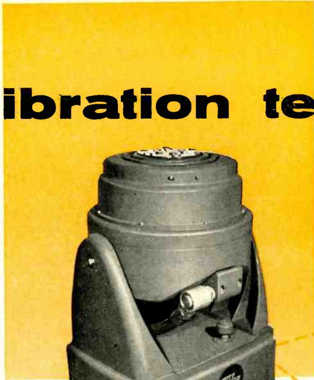
**MB MODEL C10VB EXCITER** rated for frequencies up to 6000 cps. Works in environmental test chambers, combining vibration with altitude and temperature testing.
