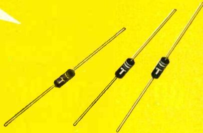
High ratings of 600 volts and 400 ma (150 ma at 150°C) are now yours in a tiny glass envelope only .1 inch by .3 inch in size. This versatile package is ideal for printed circuits, subminiature power supplies, D.C. blocking, high voltage series strings, and other applications where space is at a premium.
