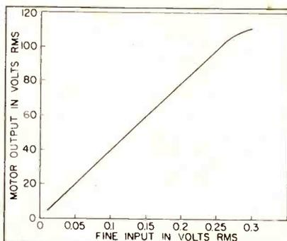
FIG. 2—Two-speed servo amplifier voltage gain characteristics
