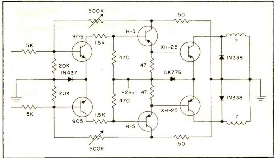
FIG. 2—Push-pull relay capable of handling 10 amperes has high-speed response
