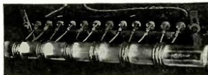
Induction heating apparatus used in zone refining. The six coils shown provide simultaneous molten zones in the ingot as it passes through the tube containing the protective atmosphere.
