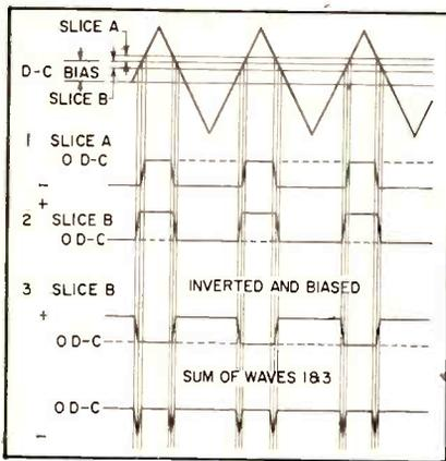
FIG. 4—Circuit waveforms of the analyzer for an input triangular wave
