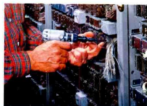
Switchboard panels of telephone dialing system are interconnected with electrical "Wire-Wrap" tool. In manufacture of panel subassemblies, connection of wires to relay terminals is made with air-powered tools.
