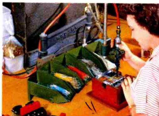
Relay panels on oil burner stack controls are wired with vertically mounted Keller "Wire-Wrap" air tools faster and at less cost than with soldering methods. Maintenance cost of tools like this is less than that for soldering operations.
