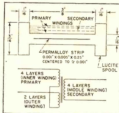
FIG. 1—Mechanical and electrical details of sensing probe construction. The primary acts as a magnetic quadrupole when current flows in opposite directions
