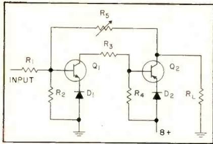
FIG. 1—Basic transistor relay circuit is controlled by Zener diode  $D_1$ .
