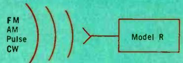
A multi-purpose broadband microwave receiver is indispensable for quantitative analysis of microwave signals and monitoring of all types of radio and radar communications. With a test antenna connected to the r-f input, power and frequency comparisons of virtually any type of signal encountered in microwave work (AM, FM, cw and pulse) may be read directly on the front panel meter. Trigger output reproduces pulse width and repetition rate, at the same time eliminating noise that may be present.
