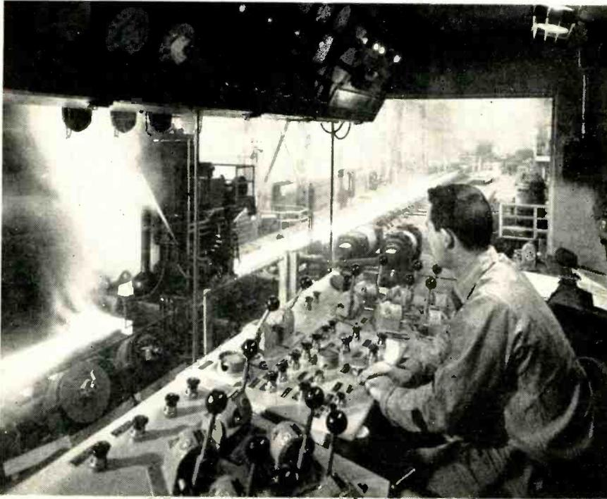
Digital and analog techniques are combined to control the operation of reverse roughing mill in new steel plant
