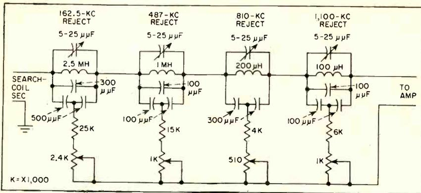
FIG. 4—Multisection bridged-T filter is used to reduce sensing probe output to second harmonic alone without encountering excessive phase shift
