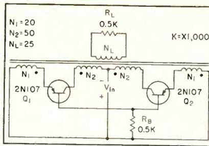
FIG. 3—Magnetic inverter with differentially connected windings oscillates without current bias
