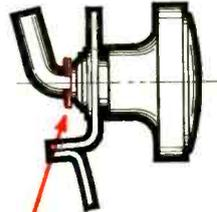
B & J Tool uses series 5555 grip ring to secure parts of damper control made for Vulcan Radiator. Shaft formerly was machined down to provide coil spring shoulder, often broke during bending operation. (Rejects ran as high as 80%!) New design eliminated rejects and field failures, cut production costs 33%.
