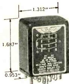
9220... *Balanced Armature* relay. Rectangular configuration... with a variety of mountings and terminals available. Hermetic sealing is 100% tested by mass spectrometer.
