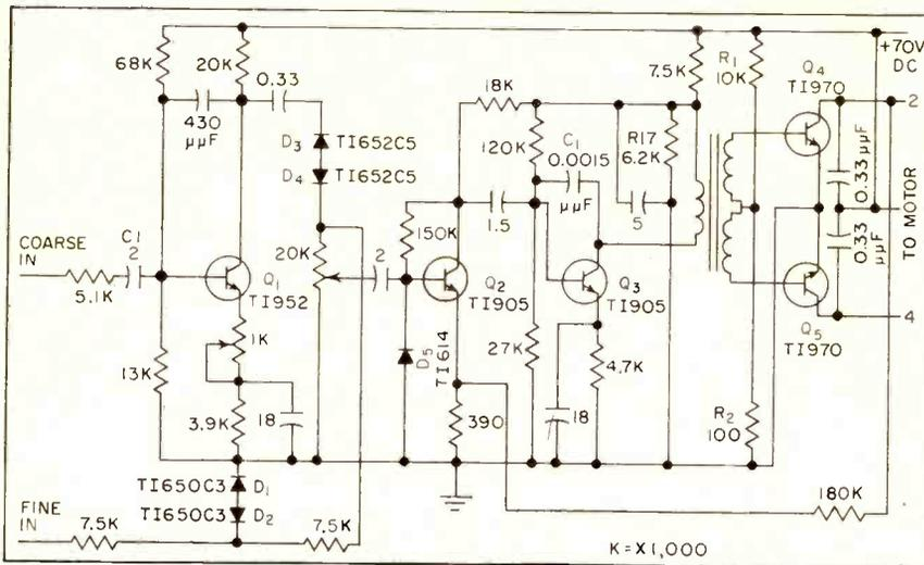
FIG. 1—Silicon transistors and diodes ensure reliable operation in extreme temperatures. Maximum coarse and fine signal input is 26 volts rms at 400 cps. Voltage gain of coarse amplifier  $Q_1$  is about 25 and that of feedback amplifier  $Q_2$ ,  $Q_3$ ,  $Q_4$  and  $Q_5$  is 460
