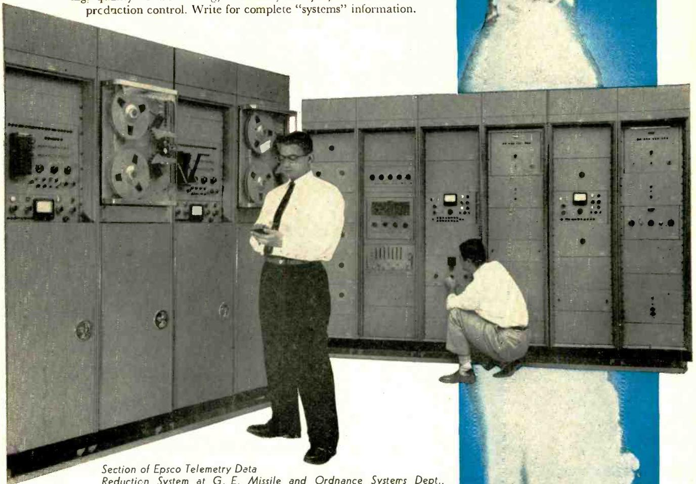
Section of Epsco Telemetry Data Reduction System at G. E. Missile and Ordnance Systems Dept., Philadelphia. System pre-edits and prepares raw data for digital computer analysis . . . at peak rates of more than 15,000 numerical words per second . . . with better than 0.1% data resolution.
