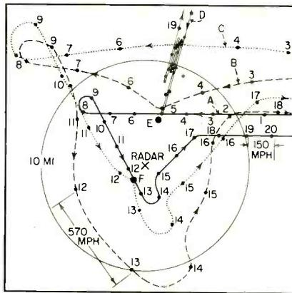
Echo from secondary scattering. Line A is aircraft path, line B is echo from aircraft to point E to aircraft to receiver. Line C shows similar scattering involving point F. Line D shows scattering from E to aircraft to E to receiver
