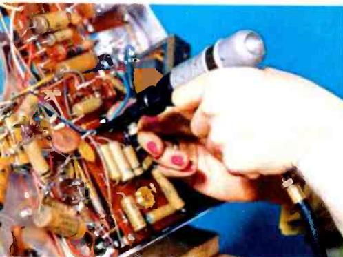
Television chassis wiring with Keller "Wire-Wrap" tools helps cut production costs and simplifies quality control processes. Only a periodic check of the connection produced is required to insure consistent quality.
