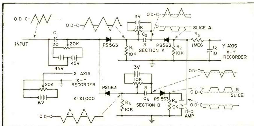
FIG. 3—Schematic of amplitude-distribution analyzer. Clipper limiter A samples d-c biased input signal between zero and positive half of slice width. Clipper limiter B samples d-c biased input signal between zero and negative half of slice width. Output of B is inverted and biased to produce positive square wave by a d-c amplifier. Recorder plots average wave  $E$  of combined A and B output
