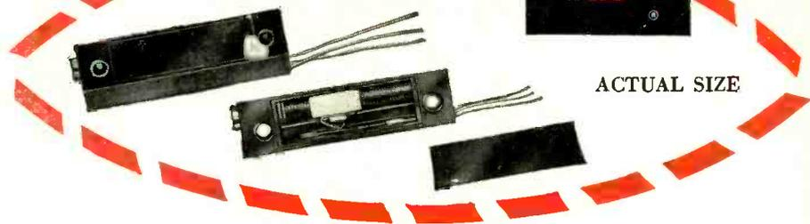
Now available as a wirewound or film type trimmer that is moisture proof, subminiature in size and withstands a temperature of 225°C., in a higher resistance range.
