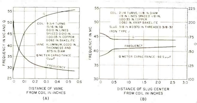
Fig. 2—Frequency and Q plotted against distance from the coil using aluminum vanes on steel screw (A) and powdered iron slug tuning (B)
