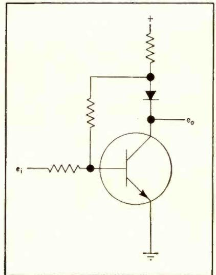
FIG. 3—Silicon diode with transistor junction form adder circuit to offset temperature drift
