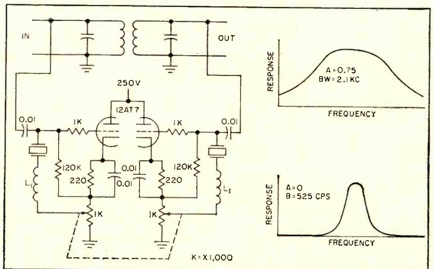
FIG. 4—Variable bandwidth circuit and responses at 848.54-kc center frequency
