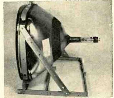
Triangular structure assembled with tube straps in place
