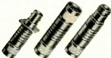
You can specify these small "in-the-line" pads in any conceivable combination of male and female Type C and Type N connectors. Single pads with female connectors can be provided with flange for panel mounting. Convenient to use... pads have maximum length of only 3" for any attenuation value. Electrically, pads are the same as those in turret model above.
