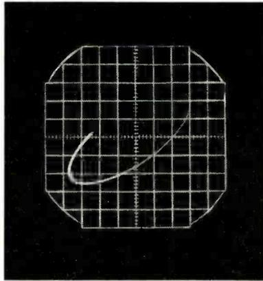
Lissajou display of 70-kc signal shows vertical voltage leading horizontal by an angle of 38 degrees
