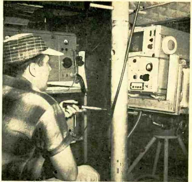
Television camera is positioned in open door of helicopter (left). Quarter-wave stub transmitting antenna extends below body when airborne. Internal view of helicopter (right) shows arrangement of camera chain and adjunct equipment
