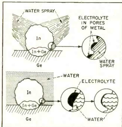
Jet spray (top) leaves electrolyte in pores for later removal by soaking (bottom)
