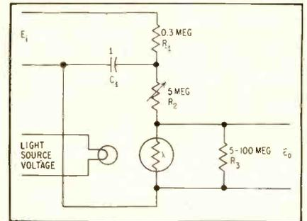
FIG. 1—Photoconductive chopper offers low noise level and resistance to vibration
