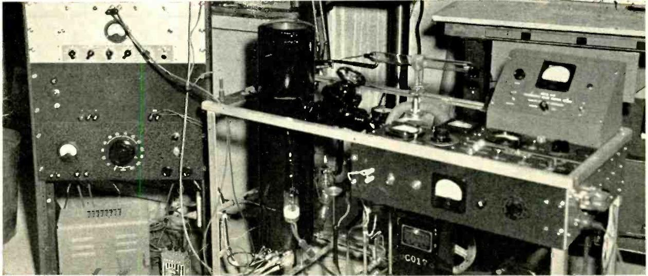
First experimental model of the Peritron. Vacuum tank is a 6-in. diam 30-in. long, seamless brass tube mounted in an angle iron table. Screen is viewed through a convex Pyrex window sealed to a shoulder turned in the upper end of the tank. Relay rack contains control circuits
