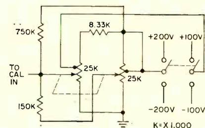
FIG. 4—Precision potentiometer circuit provides various input voltages into photoformer for calibration purposes
