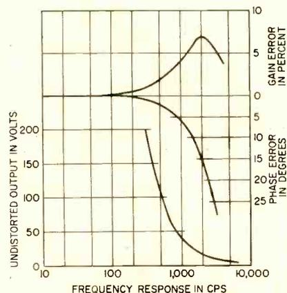
FIG. 2—Frequency response, phase error and gain error curves of photoformer. Response is flat to about 300 cps
