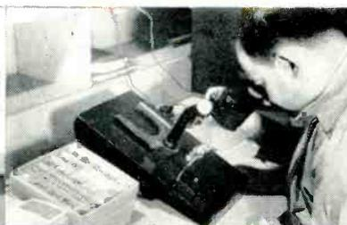
Hermetic terminals on microscope check.
