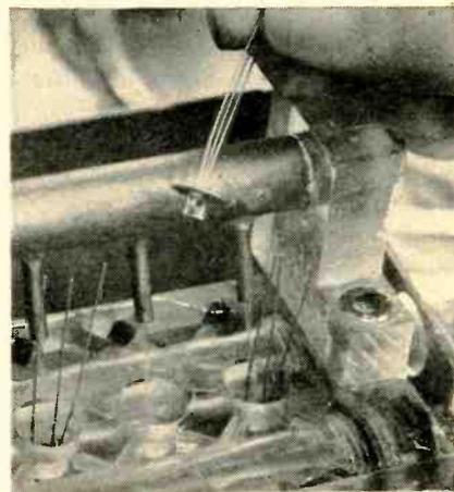
Transistor is removed from electrolyte and quickly placed in jet spray. Dried electrolyte is hard to remove
