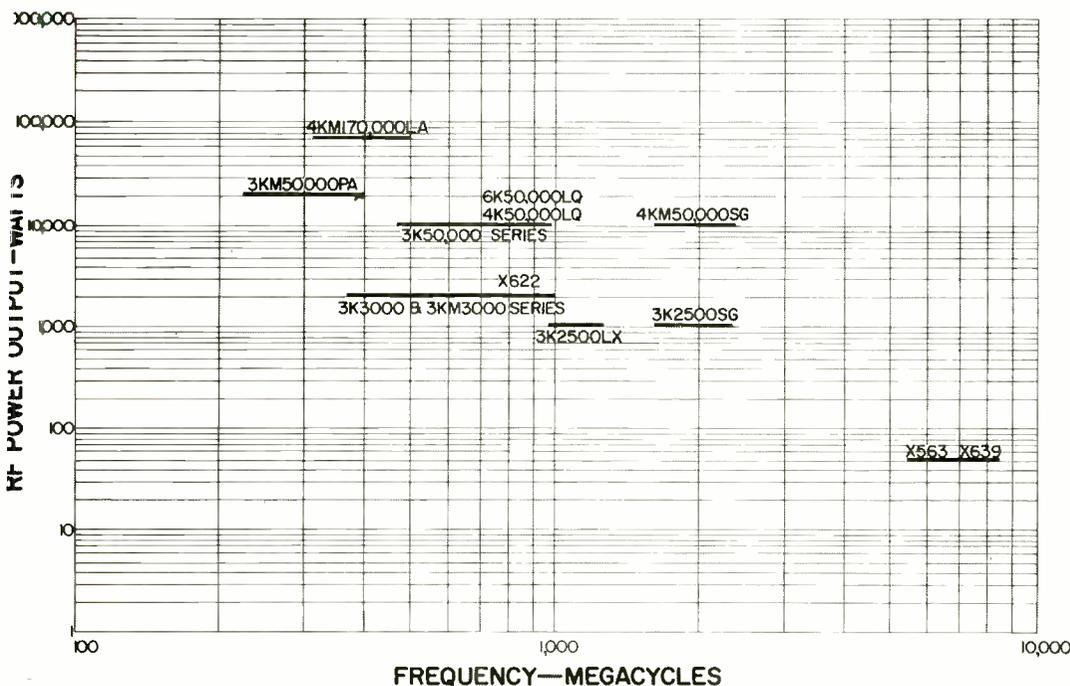
The broad frequency coverage and wide range of power levels now offered by Eimac amplifier klystrons is shown in the accompanying charts. Frequency coverage extends into the SHF range and multi-megawatt pulse output powers are available.
