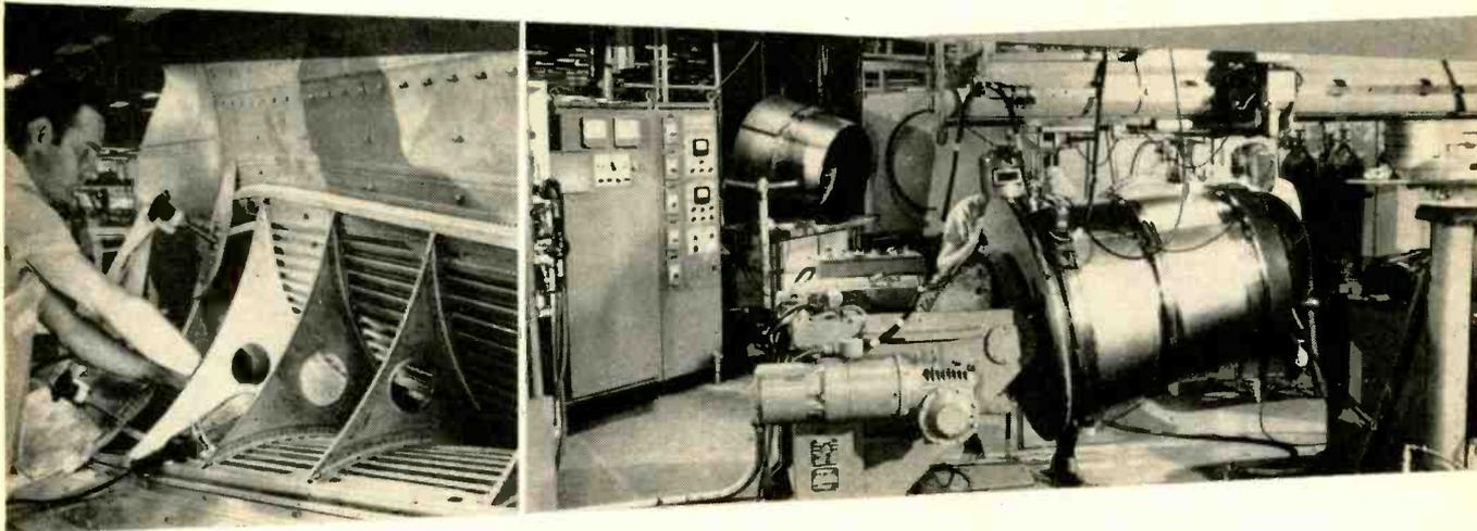
At Temco titanium is keeping its promises to the aircraft industry. No longer the intransigent metal, titanium in precision assemblies has become routine here. Through the development of Temco's Ti-Brite process, the tough titanium scale which once limited the material's usefulness is electrolytically removed without etching or disturbing the most precise dimensions.
