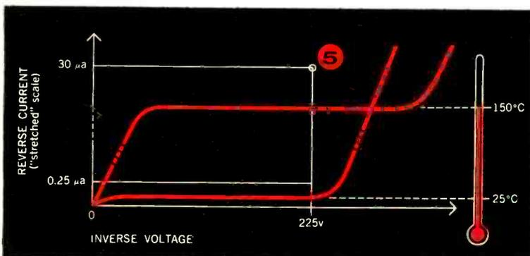
**NEW FROM SPERRY** is this high-temperature S-130 series silicon diode which gives you greater current-handling capability than germanium diodes — *with no sacrifice in recovery time!*
