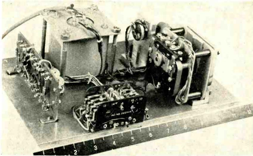
Transistorized relay servo has transistor amplifier (left), step-function potentiometer (right rear), reversible motor (right) and differential relay (front)
