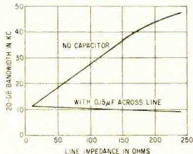
FIG. 3—Receiver selectivity as a function of line impedance
