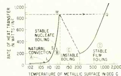
FIG. 1—Boiling heat-transfer curve for small metallic surface in still water. Zones A, B, C and D correspond to different physical phenomena as indicated. Region beyond Q is where melting point of copper is exceeded
