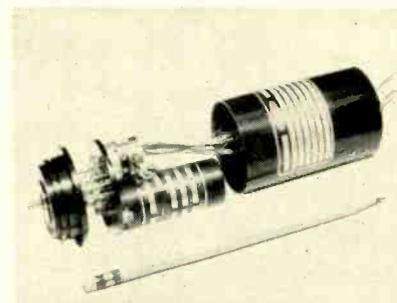
Servo component turret package contains a size 11 motor-tachometer, gear-head and potentiometer
