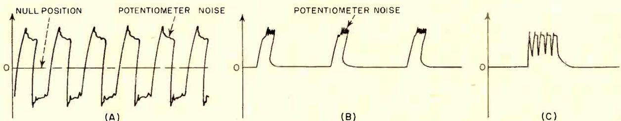
FIG. 4—Slider voltage of step-function potentiometer has undamped oscillations (A) and response to three step displacements of output shaft (B). Damping voltage (C) applied to base of o.f. transistor has exponential character
