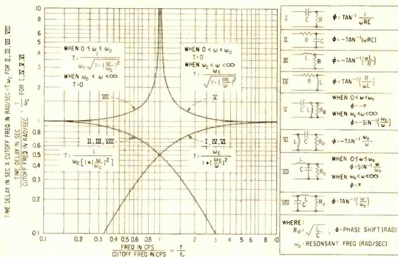
FIG. 1—Time delay curves for networks. Time delay characteristics produced in ordinary R-L-C networks are important design factors. Many applications use linear delay dispersion plotted above
