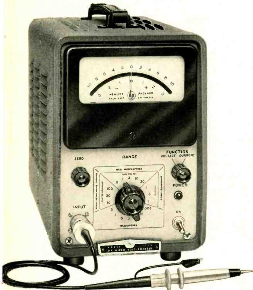
The all-new *-hp-* 425A Microvolt-Ammeter will provide engineers, physicists, chemists and physiological scientists with one compact, direct-reading instrument measuring minute voltages and currents with speed, simplicity and 10 times the sensitivity of the complex equipment arrays previously required.
