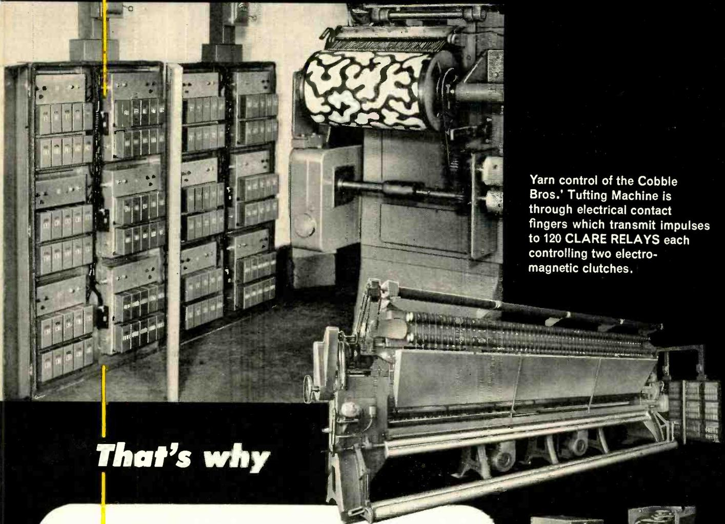
Yarn control of the Cobble Bros.' Tufting Machine is through electrical contact fingers which transmit impulses to 120 CLARE RELAYS each controlling two electro-magnetic clutches.
