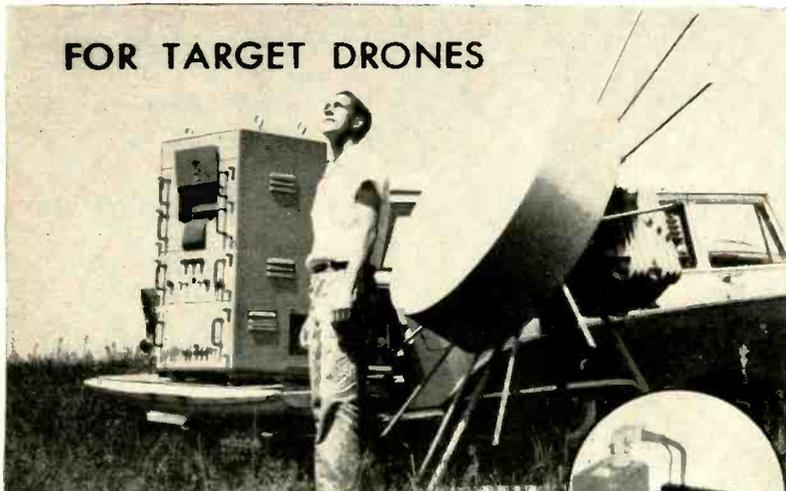
**OUTSTANDING FEATURES:** Meets MIL-E-5272A 5400B, 16400 -- provides data in 2 min. -- requires transponder in drone only -- measures salvo firings -- determines miss on multiple targets. Target equipment (less power supply) under 2 lbs. Accuracy confirmed by field tests.
