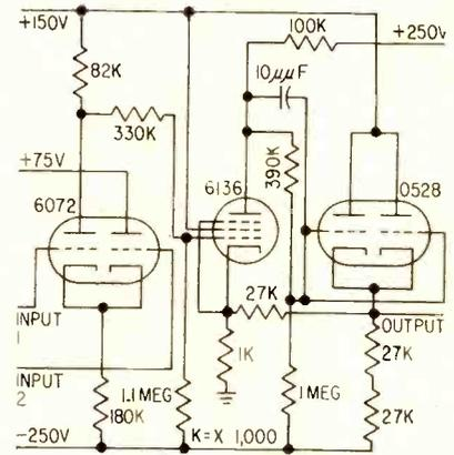
FIG. 12—Schematic diagram of an operational amplifier
