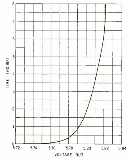
FIG. 4—Drift rate was 5 mv/hr after one hour
