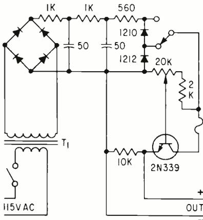
FIG. 1—Silicon transistor in precision voltage source isolates control potentiometer from output current
