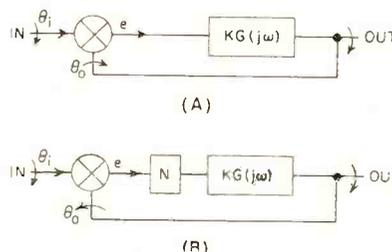
FIG. 1—Linear (A) and relay (B) servo systems can both be used as positional units in antenna systems and the like
