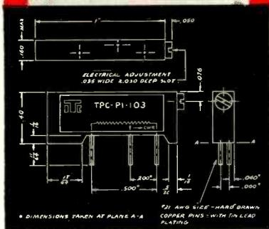
Constructed of high-temperature-resistant plastic, with a 37 turn lead-screw adjustment for fine trimming, the TPC trimmer is a masterpiece of miniaturization. Virtually hermetic sealed, this newest addition to the TIC line is moisture proof. Power rating is 1 watt at 70°C. derated to 0 at 225°C. Pretinned leads accommodate hot-tin dipping techniques. Lead separations are in multiples of 0.1" in accordance with standard printed circuit separations.
