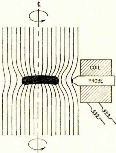
FIG. 1—Diagram clarifies principle involved in the detection of small variations in the flux pattern caused by spinning ferromagnetic object (black) in a magnetic field. The amount of eccentricity is exaggerated to emphasize the variation in flux lines
