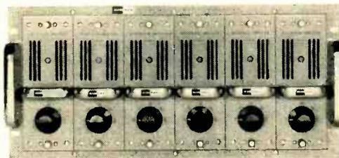
KIN TEL 114A differential DC amplifiers . . . convenient, interchangeable plug-in mounting in either 6-amplifier 19" rack mount modules or single-amplifier cabinets.
