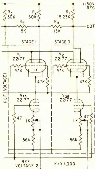
FIG. 10—Circuitry for two of the 11 decoders used
