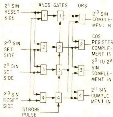
FIG. 4—Logical design of register complementer
