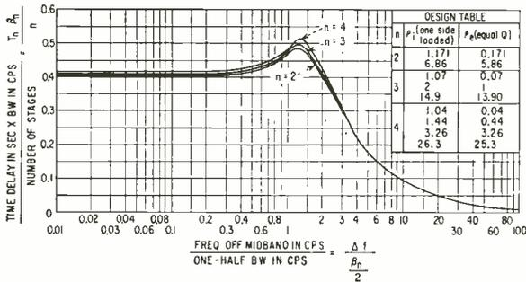
**FIG. 6**—Time delay curves for stagger damping. A plan for broadening the bandwidth of a number of cascaded double-tuned circuits is called stagger damping. It consists of cascaded undercoupled and overcoupled circuits. A properly designed, flat, stagger-damped n-uple has a product of overall bandwidth and mean stage gain equal to that of a one-side, loaded double-tuned circuit. Curves were based on data shown in design table
