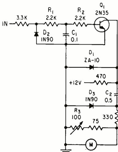
FIG. 1—Simple tachometer circuit uses zener diode to compensate variations in vehicle 12-volt system
