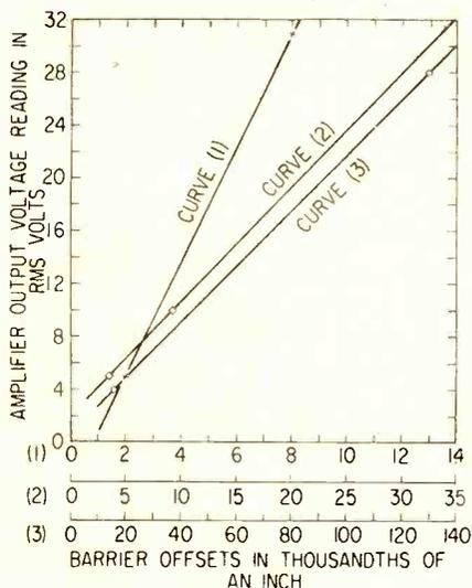
FIG. 3—Offset of encapsulated metal barrier is plotted against amplifier output. Offset readings, plotted on three lines, enhance instrument accuracy
