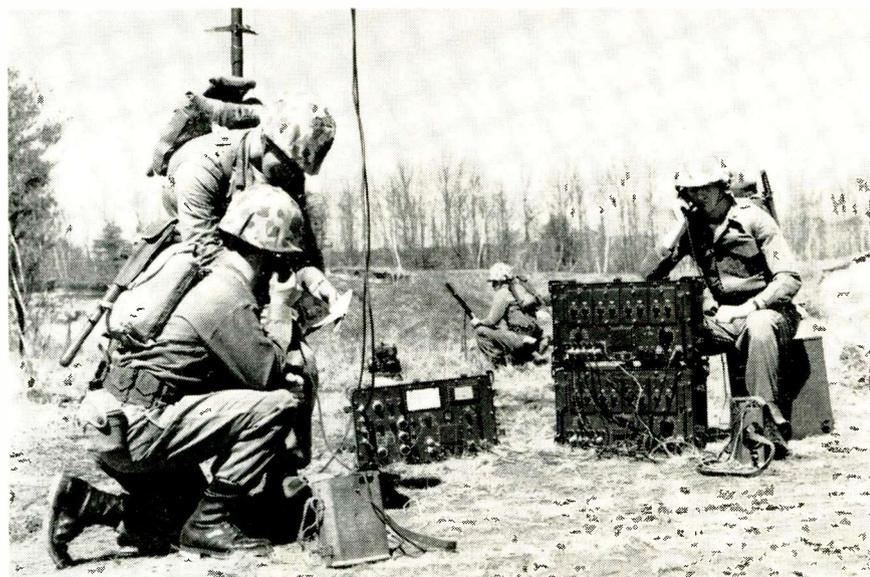
Extremely narrow sky path minimizes possibility of interception of new communications gear. Raytheon produced system being operated by Marine Corps unit has 40-mile effective range
