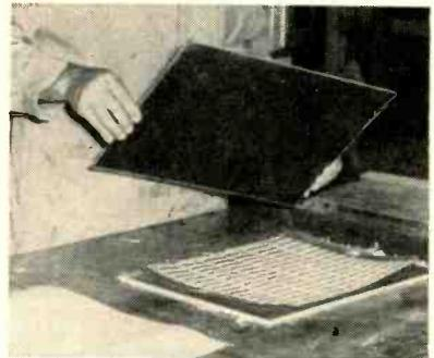
Sandwiches of 90 commutators each are prepared for insertion in hydraulic press
