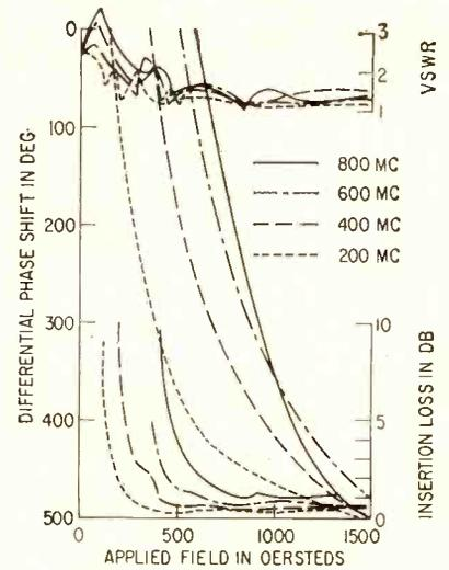
FIG. 2—Phase-shifter characteristics at 200, 400, 600 and 800 mc
