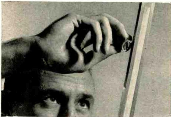
**Electromagnetic positioning** of cutting edges is directed by this etched metal bar, a significant innovation which aided in the Hughes Products development of the first all-electronically controlled machine tool line.
