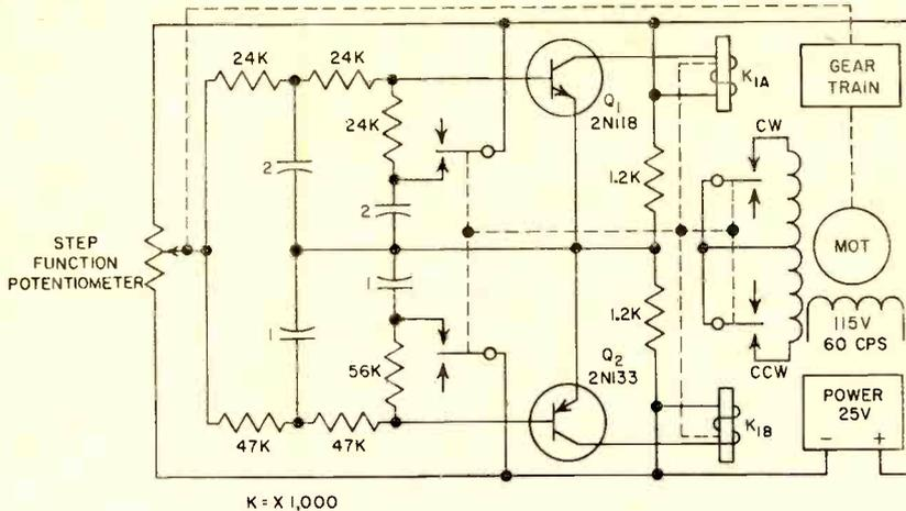
FIG. 2—Tapping positive voltage off step-function potentiometer causes current flow in  $Q_1$  transistor, operation of relay  $K_{1A}$  and upward movement of arms. Negative voltage moves arms downward reversing direction of motor travel
