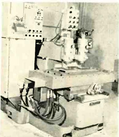
Positioning table is set up under twin drilling heads. More than 2 heads may be used
