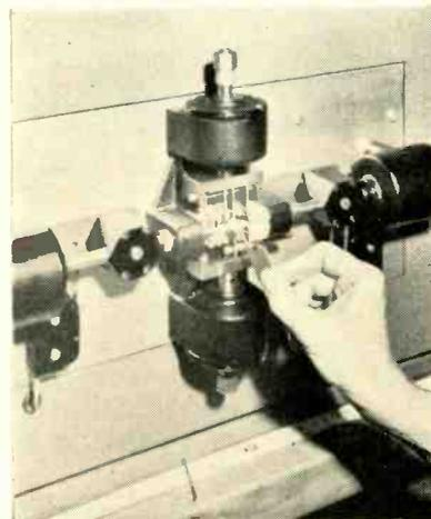
Blade position determines strip lengths and micrometers adjust cutting depth
