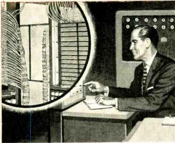
**ELECTRONIC BUSINESS MACHINES**—Non-flammability, safe emergency overloading, and solder resistance are three important reasons why TFE resins are used in machines such as this data-processing equipment. Servicing of wiring panels can be done quickly, with a minimum of downtime, because TFE resins are unaffected by soldering temperatures.
