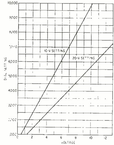
FIG. 3—Plot shows output voltages for potentiometer settings on both voltage ranges
