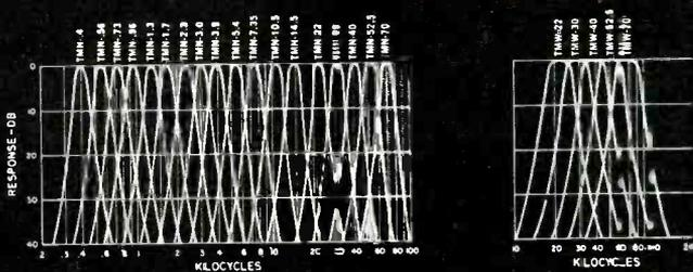
UTC standard telemetering filters provide extreme miniaturization with maximum stability, a complete set of 18 filters taking 19 cubic inches. They are 100K in and out and have an insertion loss of less than 6 db, 4 pin header for small Winchester socket.
