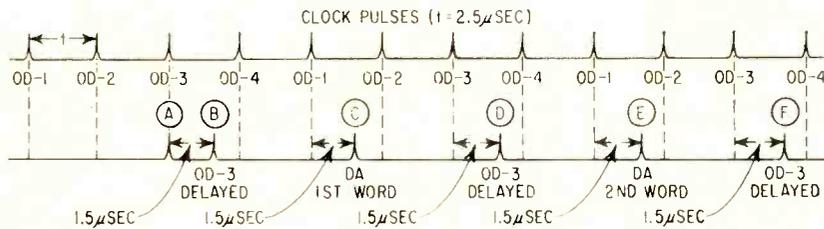
FIG. 3—Timing chart for monitor. Clock pulses are spaced 2.5  $\mu$ sec apart and cycle is repeated every 10  $\mu$ sec. Data available (DA) pulse arrives with both first and second words
