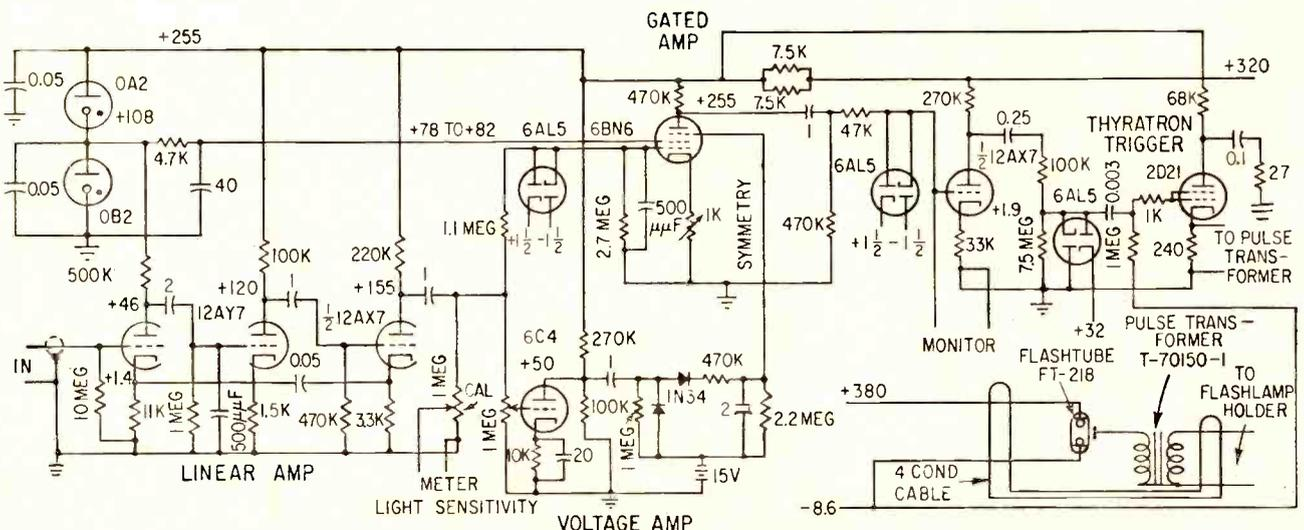
FIG. 2—Flashtube trigger circuit uses a thyatron switch to discharge a capacitor across high-voltage pulse transformer primary
