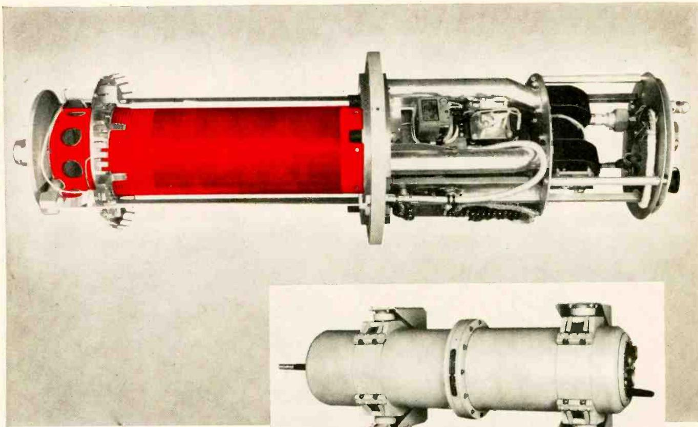
ITT Laboratories use a silicone-glass laminate as the main coil form in their AN/SRT-14, 15, 16 radio transmitting set. Laminate is tubular, 5.62" dia., wound with .064" silver wire. Primary reason for specifying silicone-glass: low loss factor at high frequencies.
