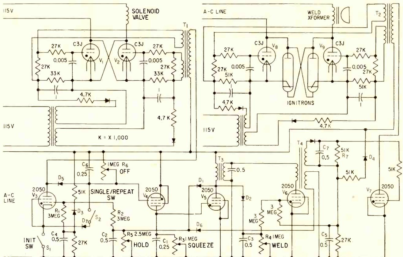
FIG. 1—Schematic of a typical control for a high-speed resistance welding gun. Fuses and overload protection circuits are not shown. This circuit affords either single-shot operation or continuous recycling of the timing functions
