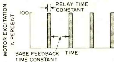
FIG. 6—Graph shows motor excitation time as function of relay time constant, and braking time as a function of feedback time constant
