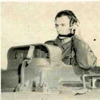
Electronic earphone contains miniature microphone which generates noise signals opposite in phase to loud unwanted noises. When two sound waves meet in earcup, most of total noise energy is dissipated. Developed by U. S. Army Signal Research and Development Lab, Ft. Monmouth together with RCA, the earphone works with a special electronic inverter and amplifier unit
