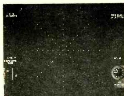
FIG. 1—Display of selected long-range-radar inputs to SAGE computer. Display is presented on a 16-in. crt mounted in console. Dots simulate targets in display used to check monitor operation. Test display differs from tactical display in that all noise and other spurious returns are filtered out. As in a ppi display, north is up, east to the right, etc. Data panels show equipment name, time of day, exposure time of photograph, radar site and type of message
