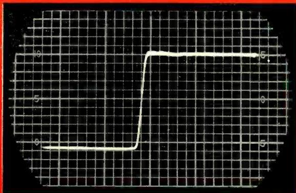
Leading edge of a typical pulse connected directly to the deflection plates of a cathode-ray tube. Sweep rate is 0.01 usec./scale division.
