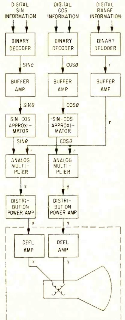
FIG. 9—Block diagram of analog portion of the monitor showing various operational stages
