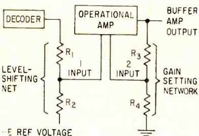
FIG. 11—Simplified circuitry for a buffer unit
