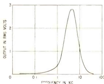
FIG. 2—Tuned amplifier response showing bandwidth and gain
