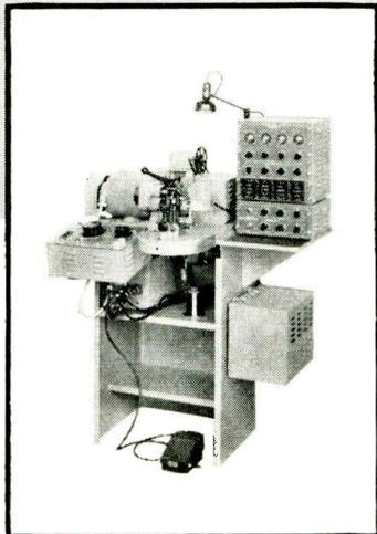
The TW 300, designed for easy servicing and maintenance, cuts production time and operator fatigue to the bone. Flexibility in production of new coil types with superior electrical characteristics is unlimited because of the new control system with automatic winding features. This machine is a significant advance toward complete automation of toroidal winding.
