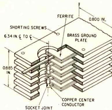
FIG. 1—Cross-section of folded uhf phase shifter
