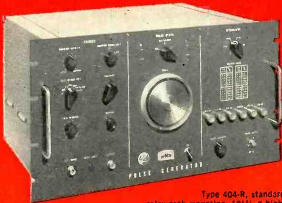
Type 404-R, standard relay rack mounting, 10 $\frac{1}{16}$ " high, 16 $\frac{5}{16}$ " cabinet width, 17 $\frac{1}{2}$ " deep.
