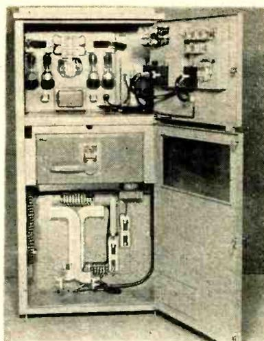
Interior view of resistance welding control unit. The relays at top are safety cutout devices; all other functions are electronically controlled
