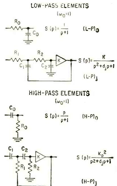
FIG. 2—Elemental frequency-determining circuits with feedback
