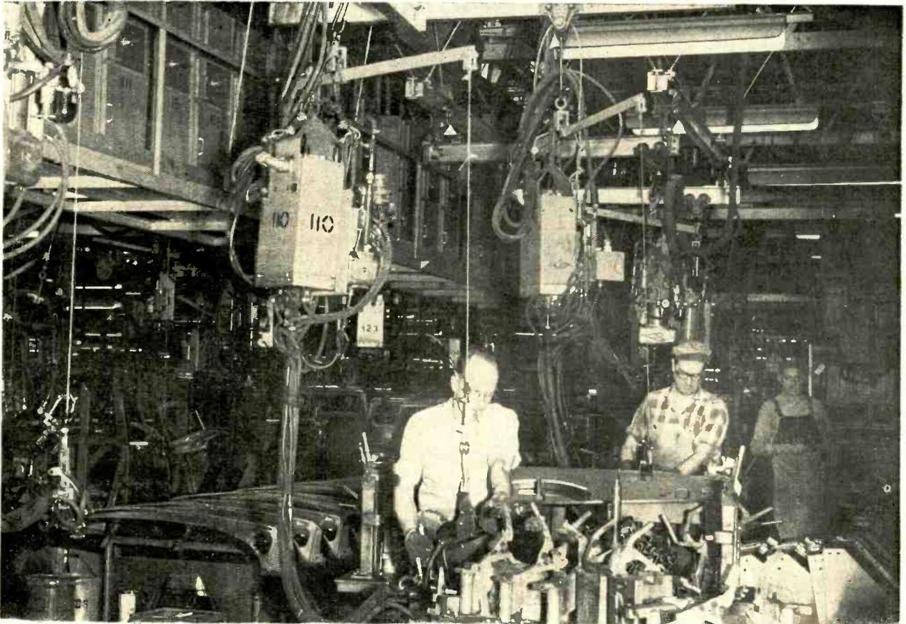
Protracted delays caused by maintenance problems in any of the high-speed resistance welding stations in a production line, such as in this automotive plant, can be costly. All-electronic controls have reduced down time by as much as 90 percent because of their innate reliability. In this installation, all the control units are mounted on a catwalk overhead for ease of maintenance
