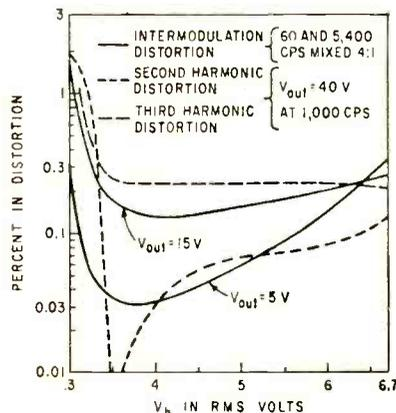
FIG. 6—Intermodulation and harmonic distortion versus heater voltage
