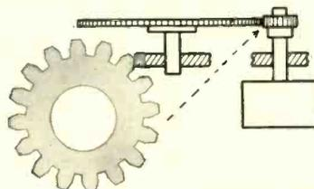
**HIGH-VOLTAGE (1800v.) RF ISOLATION** is achieved by miniature C-D-F Dilecto gears in an aircraft receiver-transmitter switch. They also had to exhibit dimensional stability through a wide temperature range, resistance to fungus growth and thermal shock.
