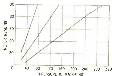
FIG. 3—Calibration curves for different operating ranges
