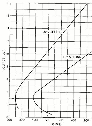
FIG. 2—Output impedance as a function of output voltage is shown for 10 and 20-volt settings
