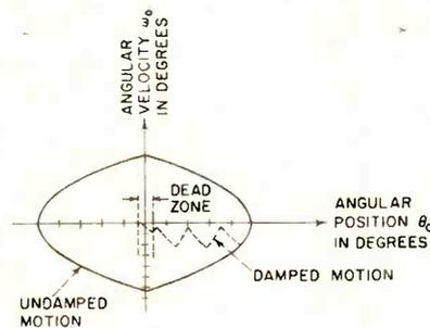
FIG. 5—Position and velocity of output shaft is superimposed on phase-plane sketch for damped and undamped cases
