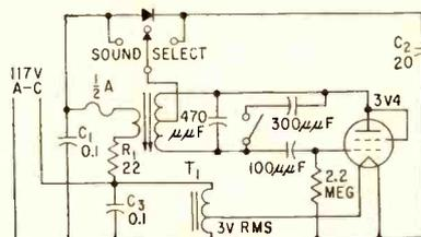
FIG. 1—Complete remote-control carrier-current transmitter
