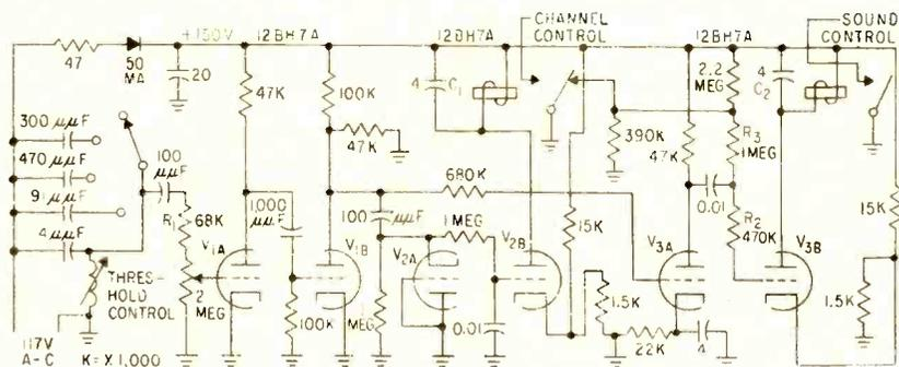
FIG. 2—One part of receiver detects only unmodulated carrier while other part detects both modulated and unmodulated signals
