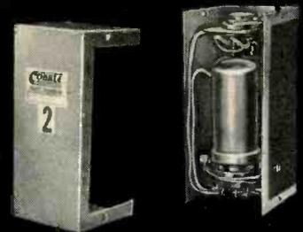
Each relay is housed with a transistor in this modular type unit. The module is then plugged into the control system.
