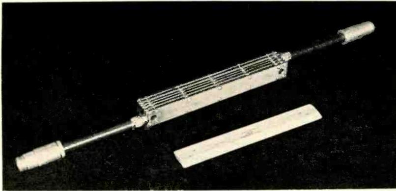
Small physical size of phase shifter is evident here
