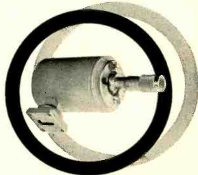
Each instrument covers a wide segment of the total range. Only 11 sizes serve from 2.6 KMC to 90 KMC. Accuracy is so high they may be used as secondary standards. Nitrogen filled and sealed for long life and high Q. Bi-metallic structure provides high degree of thermal compensation. Write for literature.
