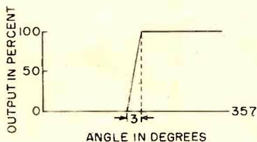
FIG. 3—Characteristic of step-function potentiometer has 3-deg segment during which there is linear variation from zero to full output current
