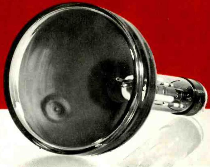
New five-inch experimental evaporated phosphor CRT
