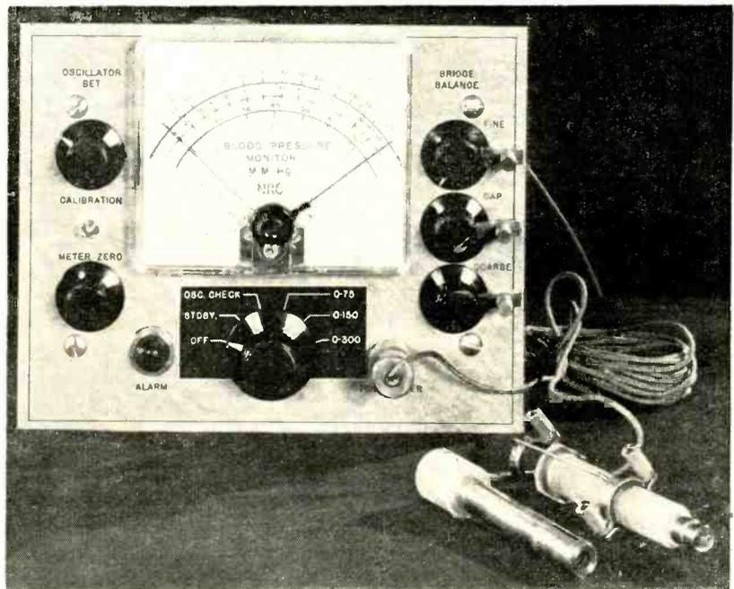
Compactness, accuracy and dependability of unit make it ideal for operating-room service. Complete instrument measures only 8 by 10 by 10 in.
