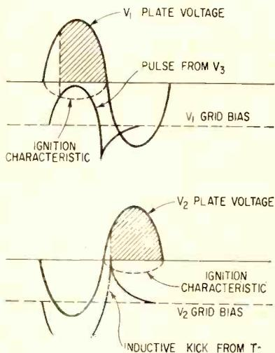
FIG. 2—Waveforms depict how full-wave control of solenoid valve is maintained by single positive pulse from  $V_3$ . Shaded area indicates ignition period
