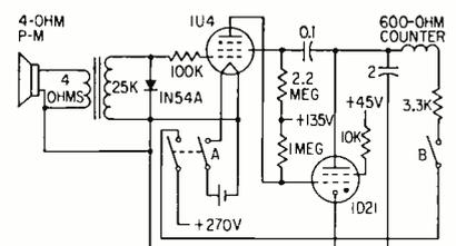
FIG. 1—P-m speaker functions as sensor in self-contained shot and blast counter
