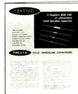
STA Type Solid Tantalum Capacitor, voltage ranges up to 60 Volts (wvdc). Bulletin 6.112
