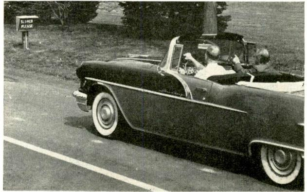
Illuminated sign actuated by RCA's roadside signaling system advises driver his car is exceeding speed limit
