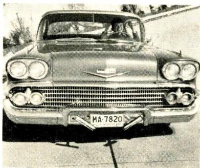
FIG. 3—GM Research's Autoguide system takes over steering function from driver. In demonstration auto above, driver retains control of brake and accelerator
