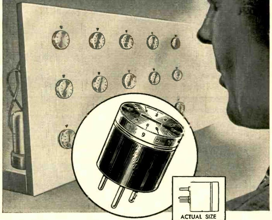
**Plugged into printed circuits or mounted on control panels**, this new ½" pot speeds adjustments by letting you see what you've set. Its dual-calibrated dial tells at a glance slider location, shaft angle and voltage percentage. The 300° winding angle is equally graduated from 0 to 10. Zero on the dial lines up with a scribe line on the side of the pot at 0° rotation. Terminals are located on a standard 0.1" grid, as used in printed circuits.
