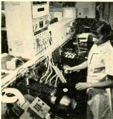
Racks of diodes are tested in oil baths
