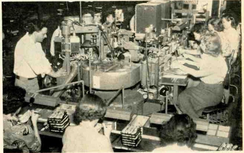
At top speed, this tube cage assembly machine represents a production rate of more than 100 assemblies an hour for each operator required
