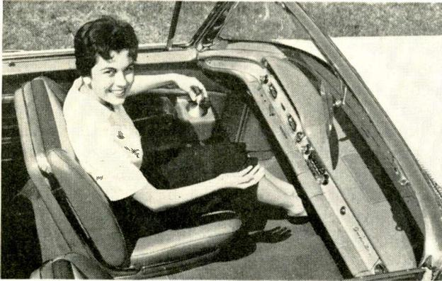
Steering, accelerating and braking operations are all done by moving single stick in GM's Unicontrol system
