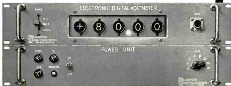
Both the 7000 and 8000 Series develop voltage state BCD outputs for data recorder entry. Standard code is 2, 4, 2, 1; other codes available on special order.
