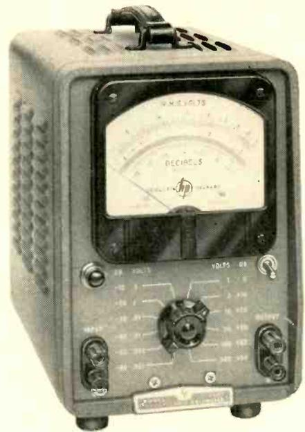
New, convenient *-hp-* 400L is a unique instrument combining a specially designed logarithmic meter movement with the many desirable features of *-hp-* 400D and 400H voltmeters.
