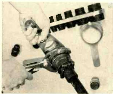
SPECIALIZED WRENCHES for assembling or disassembling Cannon, Bendix Scintilla or Amphenol AN connectors have been developed by Spec Tool Co., in cooperation with Cannon Electric Co. Each of the combination type male or female wrenches will grip 12 sizes of connectors. Photo shows how the male wrench is used with a pair of pliers. In the background are a female wrench and a single-size wrench.
