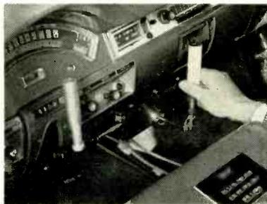
FIG. 1—Ford's control system uses two tiller sticks. Right is for steering, left controls automatic transmission
