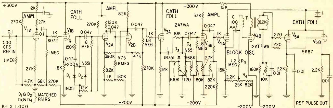
FIG. 7—Reference-pulse generator supplies a 500-cps reference pulse to the analog and digital phase meters
