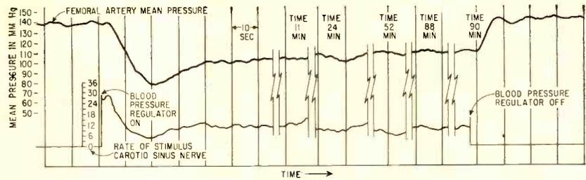
FIG. 7—Tracing of record showing regulation of pressure by stimulation of carotid sinus nerve with blood pressure regulator unit
