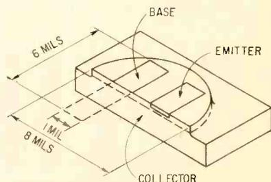
FIG. 3—Closeup of diffused-base germanium wafer
