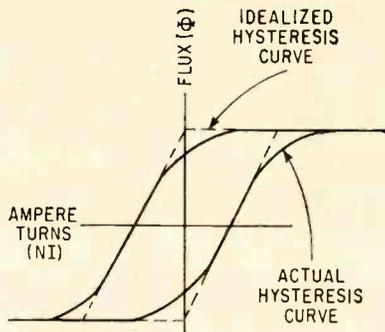
FIG. 2—Curves show actual and idealized hysteresis curves for magnetic material used in demodulator
