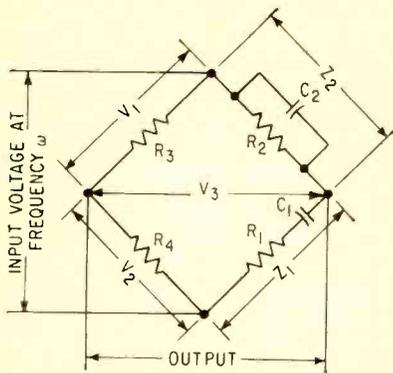
FIG. 1—Basic Wien bridge is balanced when  $V_3 = 0$
