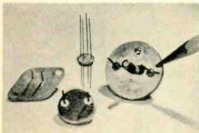
Power transistor bases show how leads are sealed directly to copper base without need for metal eyelets
