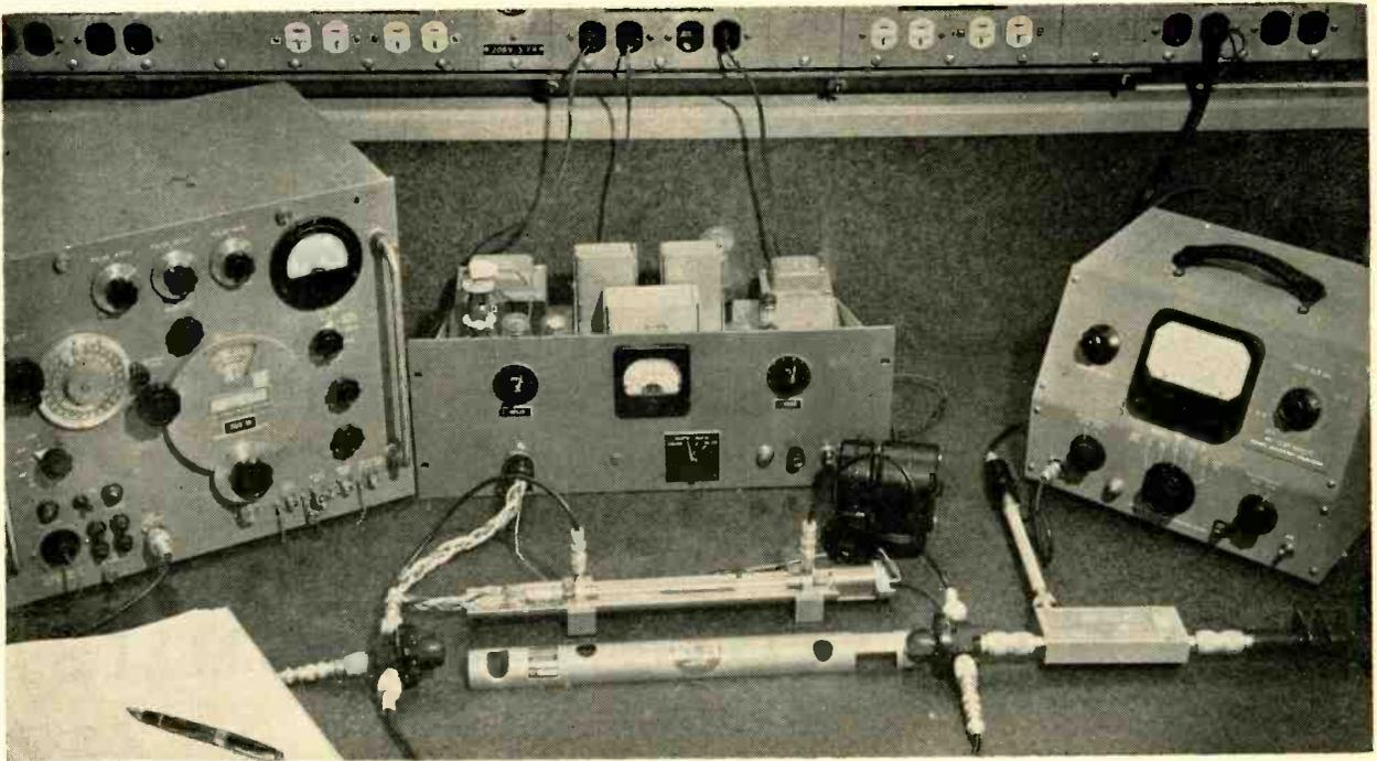
Estiatron encased in a thin shell is shown in typical bench setup prior to checking characteristics
