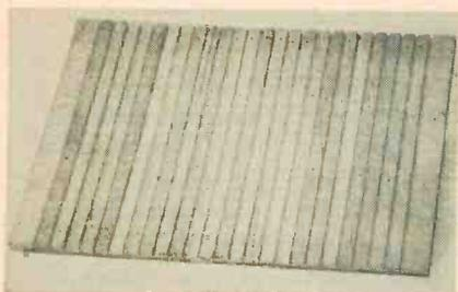
Board holder is pine strips nailed on plywood
