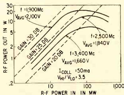
FIG. 6—R-f power output as a function of r-f power input
