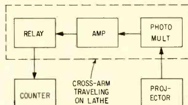
FIG. 1—Block diagram of electronic micrometer for printed circuit checking
