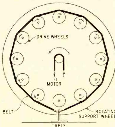
FIG. 2—Rear view of rotating support wheel
