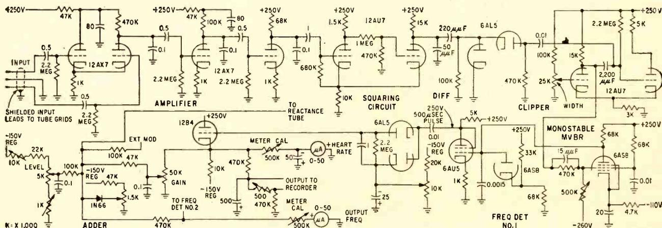
FIG. 6—Sections of heart rate regulator which use different circuits. Separate power supply is conventional
