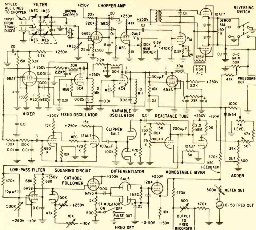
FIG. 5—Complete circuit diagram of blood pressure regulator. Power supplies are conventional, hence not shown
