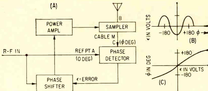
FIG. 1—Block diagram (A) of basic phase-control system. Input-output characteristics of phase detector (B) and phase shifter (C) determine system response
