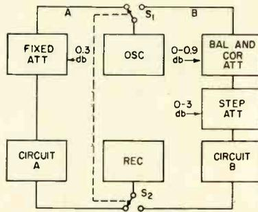
FIG. 1—Signal output of paths A and B must be equalized within 0.1 db in measuring technique described in text
