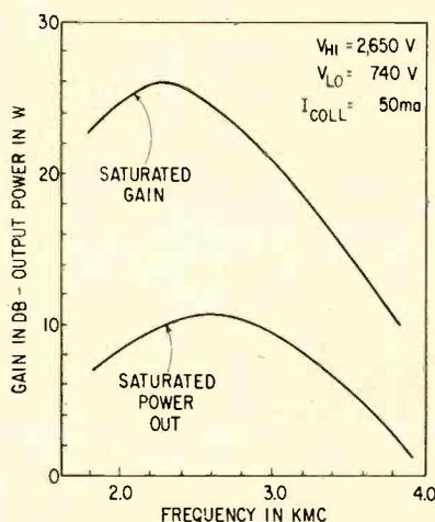
FIG. 5—Saturated gain and power output as a function of frequency. Voltages held fixed at optimum values for 3 kmc
