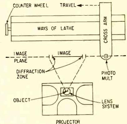
FIG. 2—Mechanical arrangement of the precision measuring machine. Image of object to be measured is scanned by phototube as arm travels down lathe
