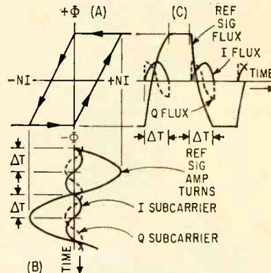
FIG. 3—Graphical analysis shows that only *I* component can be produced because reference signal saturates core except during time  $\Delta T$
