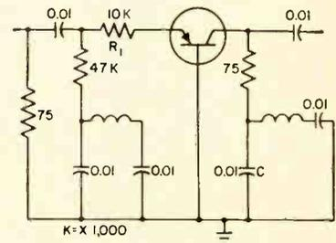
FIG. 2—Capacitor C of transistor circuit to be measured must be increased in value for frequencies below 1 mc
