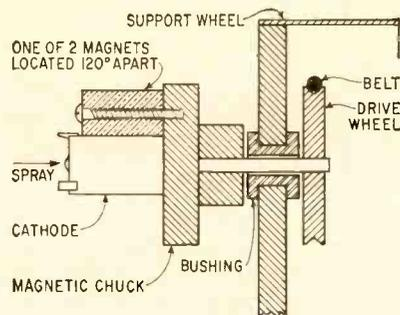
FIG. 1—Cutaway view of chuck and drive wheel assembly
