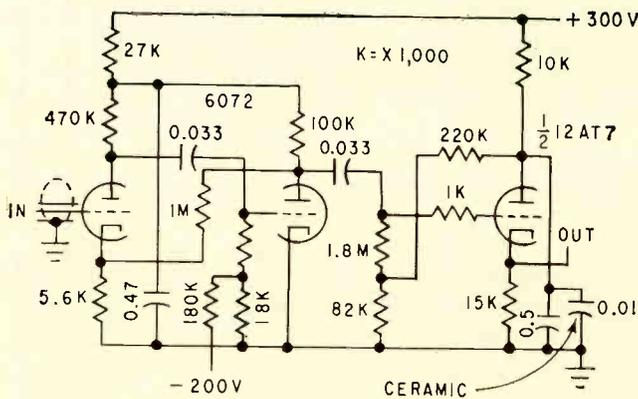
FIG. 6—Buffer circuit of the tracking system
