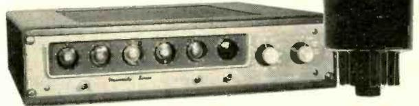
Baird-Atomic uses DEKATRON glow transfer tubes in all instruments where counting and read-out are required. A typical application is the Atomic Instrument Line's Model 134 Scaler for ultra-high speed counting of beta and gamma radioactivity . . . up to 1,000,000 counts/minute! The input circuit incorporates a fast, constant-sensitivity Schmitt discriminator driving a beam switching decade with glow tube read-out . . . 6 DEKATRONS.
