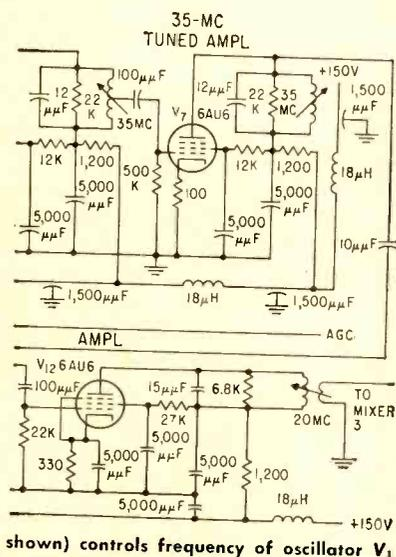
shown) controls frequency of oscillator V<sub>1</sub>
