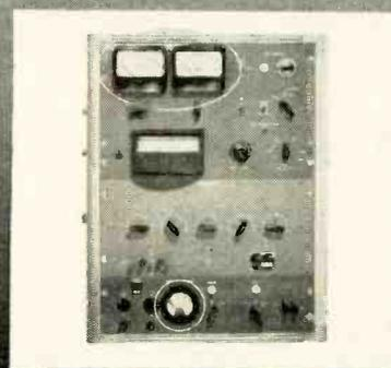
**AFTER . . .** 3 trio VTVMs integrally built-in now are always on hand to measure just the parameters you designate.
