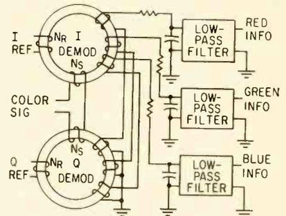
FIG. 4—Complete system shows core outputs integrated and filtered to produce red, green and blue information
