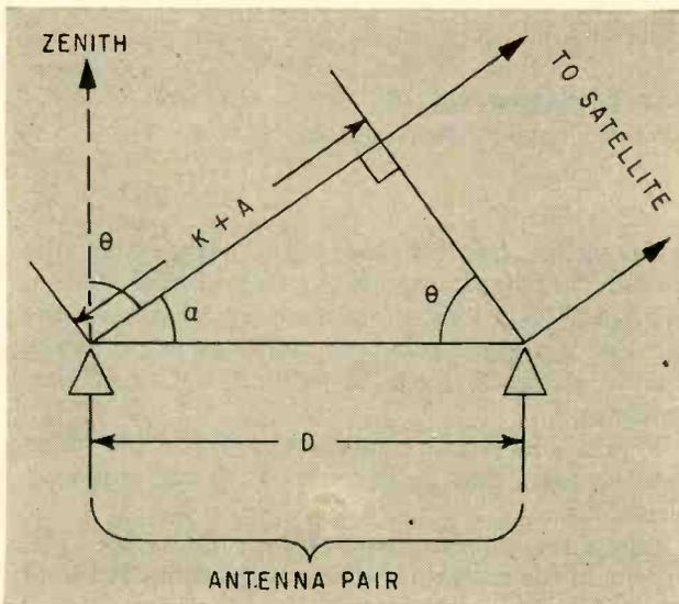
FIG. 2—Minitrack system angular relationship of antenna pairs with respect to satellite position
