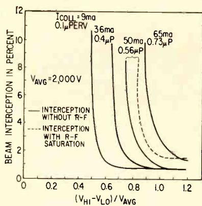
FIG. 4—Beam interception as a function of the ratio of voltage difference to average voltage
