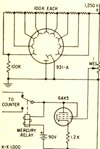
FIG. 3—Multiplier-phototube control circuit. The mercury relay controls the electronic counter
