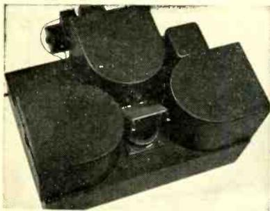
The object to be measured is placed beneath lens of opaque projector, and casts image in plane parallel to lathe
