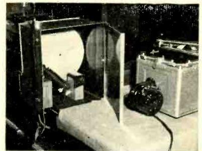
Counter wheel is directly geared to the main screw of the lathe. Light beam, through holes, indicates lathe travel
