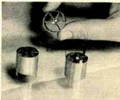
Type of cathode sprayed on inside surfaces
