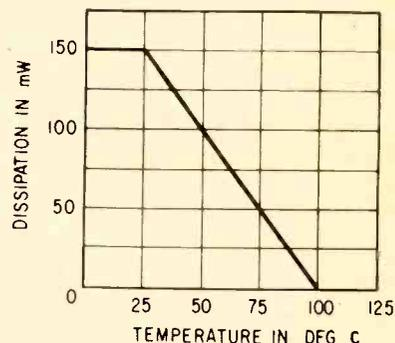
FIG. 1—Typical derating curve for TI 2N559 transistor
