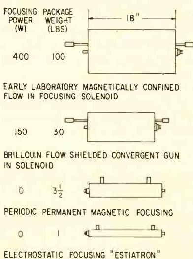
FIG. 1—Size and weight comparison for 10-w 5-band traveling-wave amplifiers
