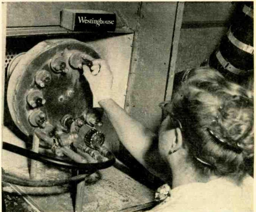
Magnetic chucks speed loading of nickel cathodes on rotating fixture
