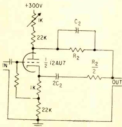
FIG. 2—Wien bridge filter does not have high Q but provides good rejection
