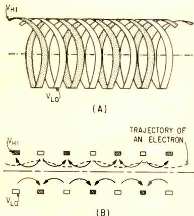
FIG. 3—Bifilar helices for electrostatic focusing. Bifilar helix structure (A) and forces exerted on an electron by the periodic electrostatic field and the trajectory of an electron (B)
