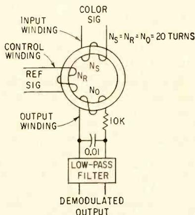
FIG. 1—Basic magnetic demodulator has input winding with color information, reference winding and output winding that supplies demodulated *I* or *Q* information
