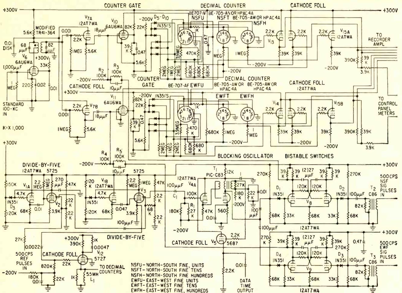
FIG. 8—Digital phase meter measures the phase angle between the signal and the reference pulse
