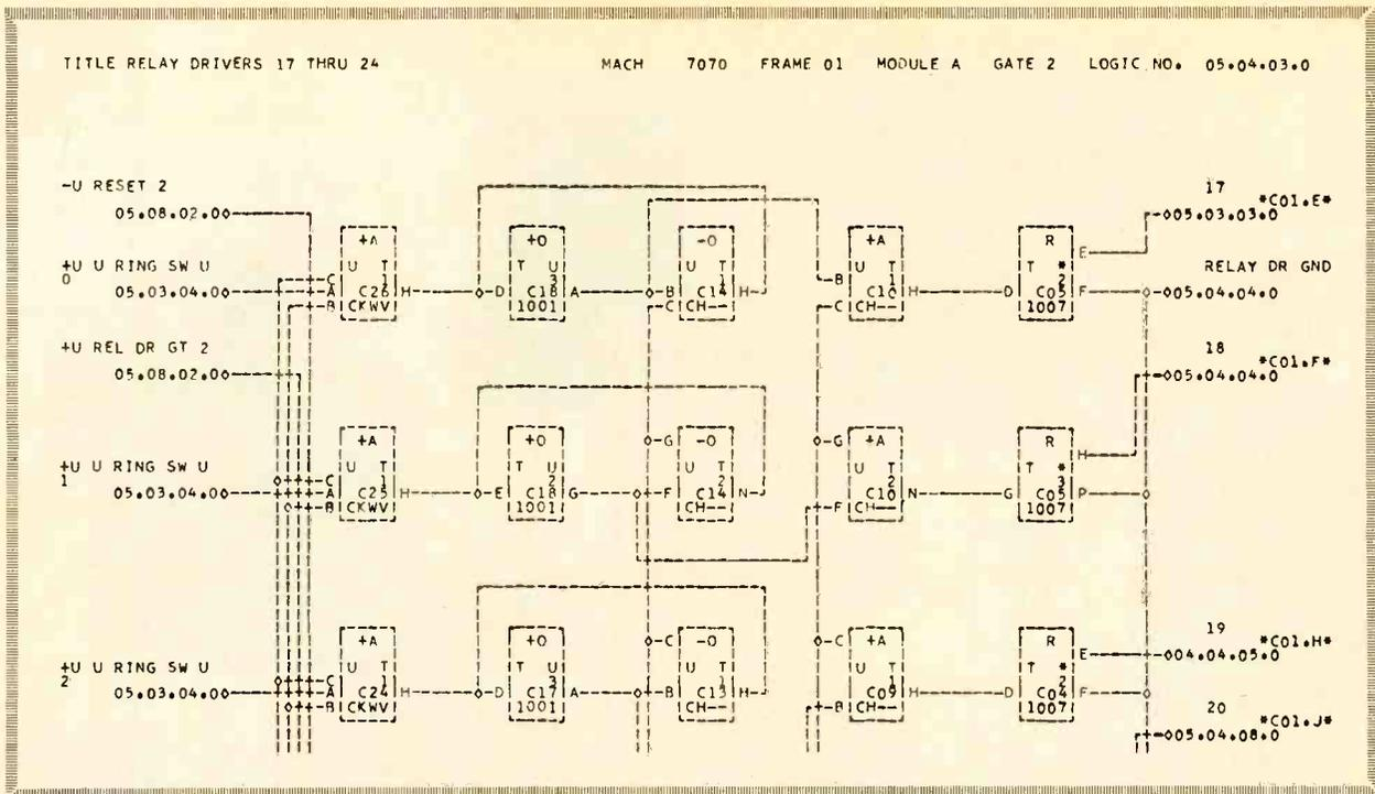
From an engineer's rough logic sketch, IBM computer produces a finished drawing. Diamonds are connection points
