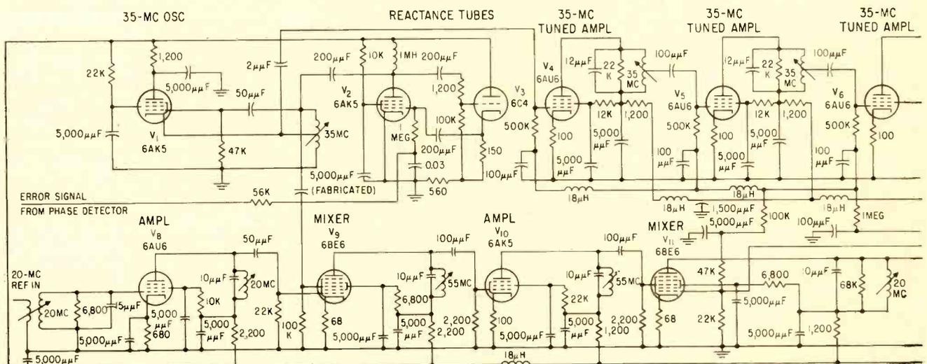
FIG. 3—Schematic diagram of the phase-shifting circuit used in the phase-stabilized system. Error signal from the phase detector (not through reactance tubes  $V_2$  and  $V_3$ ). Output of fixed-tuned stages  $V_4$  through  $V_7$  is shifted as a function of the d-c error signal
