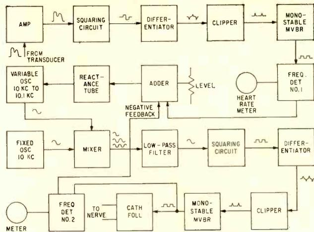
FIG. 4—Heart rate regulator similarly senses arterial pressure, but delivers pulses to vagus nerve that controls muscles of heart
