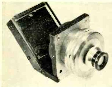
Lens and front-surface mirror. Image from front-surface mirror is reflected on to plane scanned by phototube
