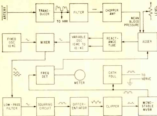
FIG. 3—Electronic blood pressure regulator senses arterial pressure and delivers controlling pulses to carotid sinus nerve
