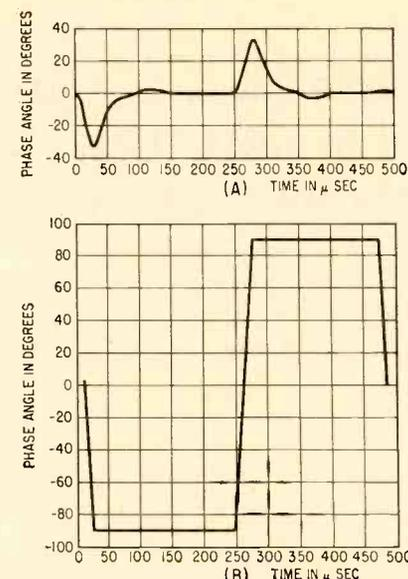
FIG. 4—System response to a step-function change in phase angle; (A) is closed-loop, (B) open-loop response
