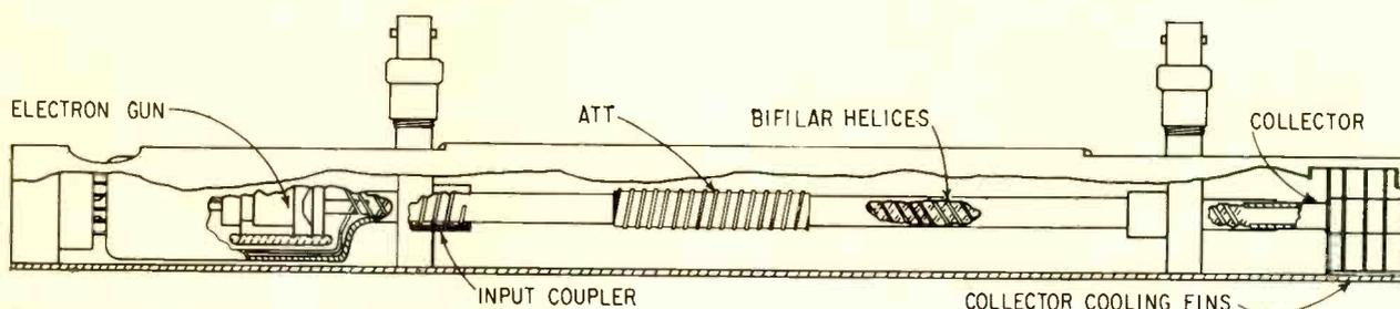
FIG. 2—Cutaway sketch of a packaged Estiatron
