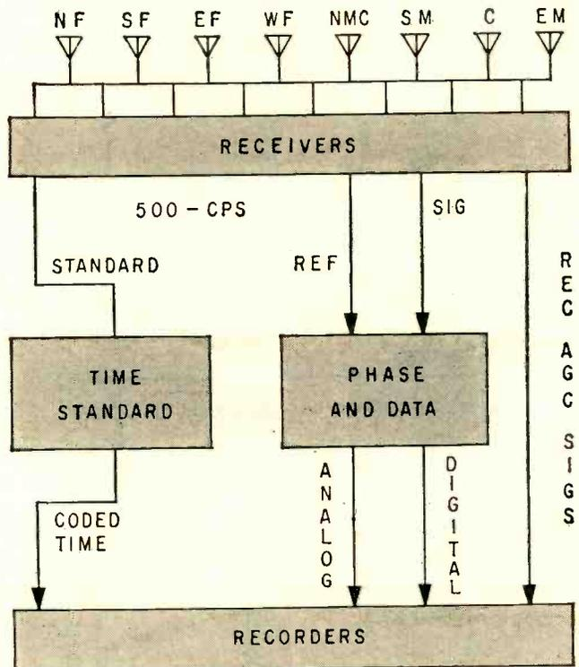
FIG. 3—Simplified block diagram of data and time system at each ground station
