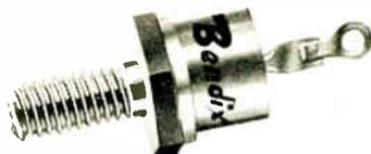
have piv ratings ranging from 50 to 600 v and can deliver 5 amperes of rectified current. Operating temperature extends from -65 C to +175 C. The rectifier package is in conformance with the latest JETEC proposed standards. Units are
