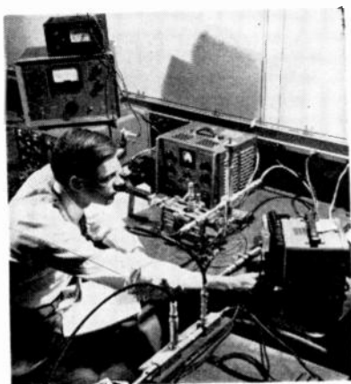
Low-noise parametric amplifier developed at GE received Pioneer IV's signals beyond 400,000 miles
