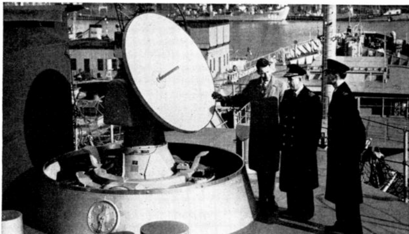
First photo of Collins AN/SRN-4 radio sextant installed aboard USS Compass Island, Navy's experimental navigation ship. Gear automatically tracks thermal radiation from both sun and moon. (See ELECTRONICS, p 24, June 10, 1957)
