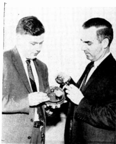
Heart of communications system in Vanguard "Cloud Cover Satellite" now orbiting is basic tape recorder (left). Unit is 5\frac{1}{2} -in. wide, weighs 1 lb, 5 oz, and records weather on global scale. Right: 75-ft tape is checked by engineer from Army Signal Lab, which developed recorder, and official of Minnesota Mining & Mfg., developer of the special instrumentation tape
