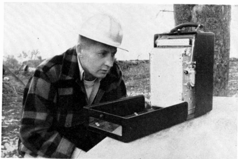
Twenty-pen recorder by Esterline-Angus monitors weather variables in burn area of forest in state of Washington. Replacing large numbers of instruments previously required, recorder supplies wind-current data need in study of forest-fire control
