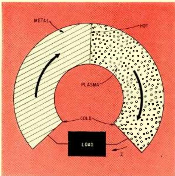
FIG. 16—Basic plasma-metallic thermocouple
