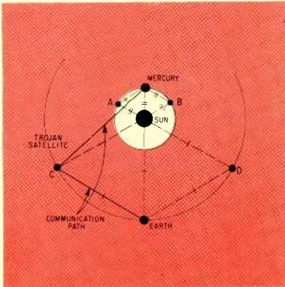
FIG. 9—Relay satellite placed at a Trojan point of two bodies in space will remain stabilized in that position
