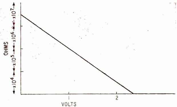
FIG. 5—A linear voltage increase across a 1N472 diode causes a logarithmic decrease of diode resistance
