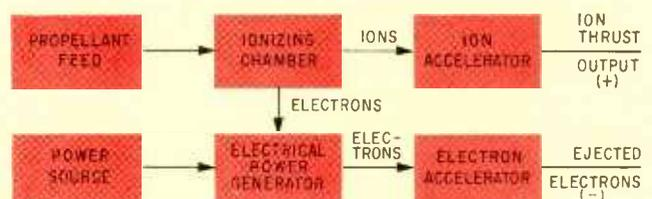
FIG. 3—Basic components of ion-drive propulsion system
