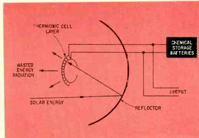
FIG. 14—Basic arrangement for thermionic-converter system
