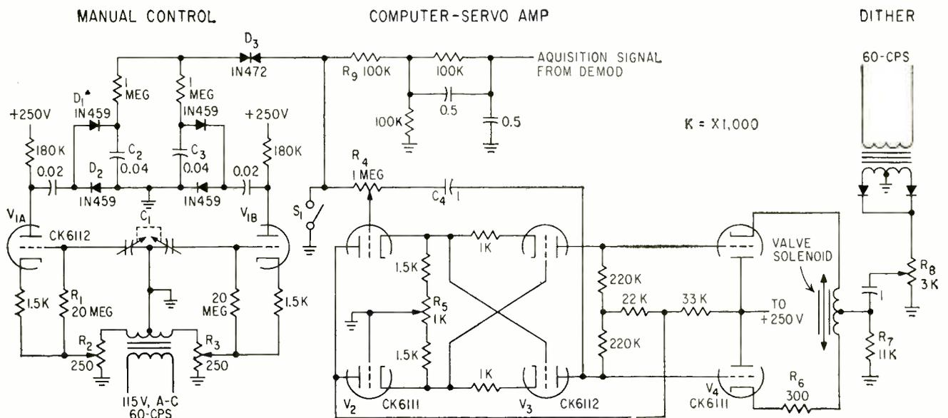
FIG. 2—Section of capacitor  $C_1$  controls the current through the solenoid. After passing through the lead network and  $R_1$ , the radar acquisition signal is applied to a grid of  $V_2$
