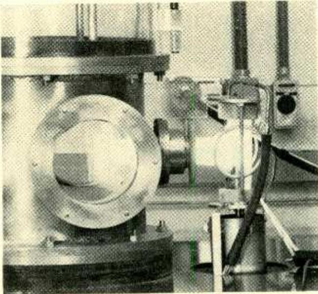
Exhaust plasma from experimental General Electric T-tube accelerator deflects scale vane, visible in porthole at left, to give approximate indication of thrust produced
