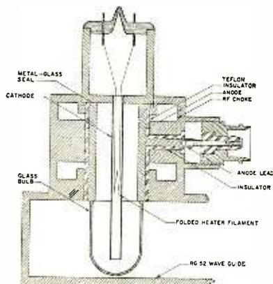
FIG 1—Probe-type cylindrical diode mount assembly
