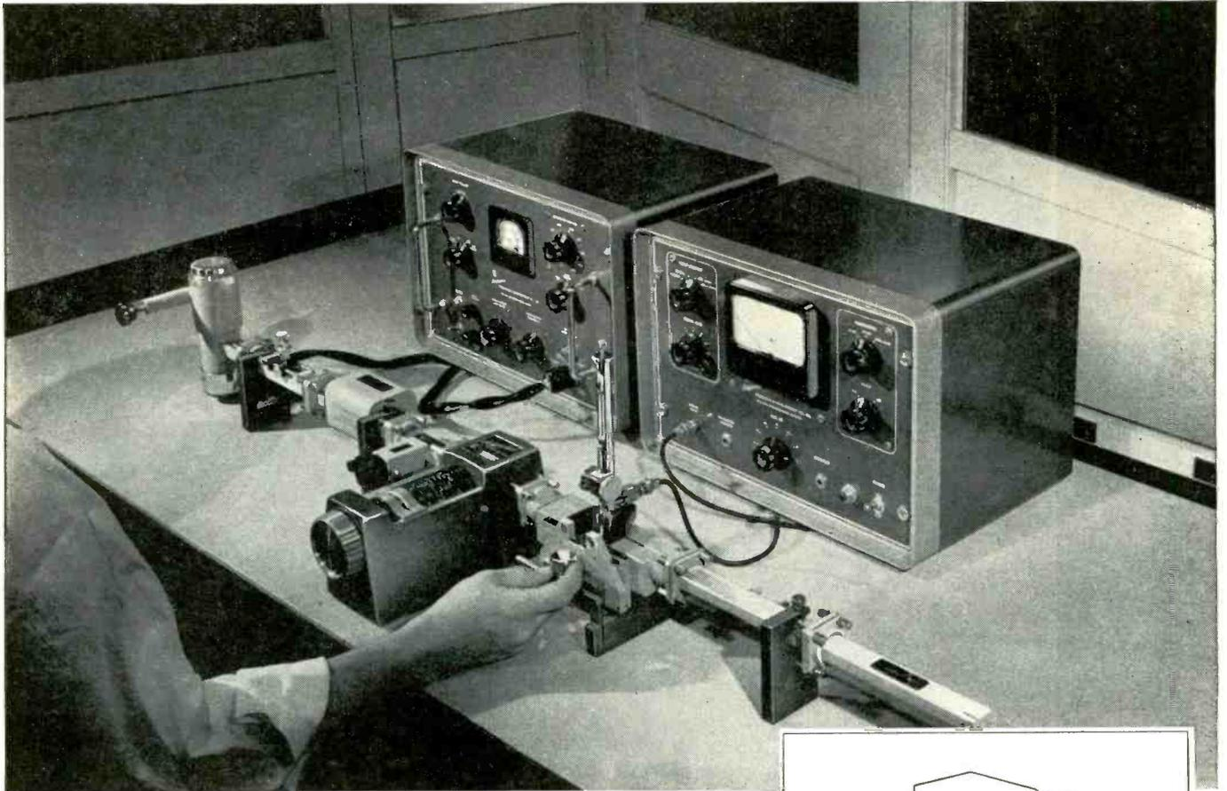
This microwave measurement bench is for the determination of Voltage Standing Wave Ratio using the slotted-line technique. Other systems utilizing directional couplers or magic tees for measurement of VSWR are known, but the use of the Slotted Section assures maximum accuracy.
