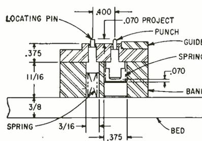
FIG. 2—Lower mechanism in loading position
