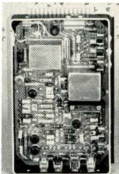
Layout of operational amplifier avoids closing of feedback loops through stray capacitances
