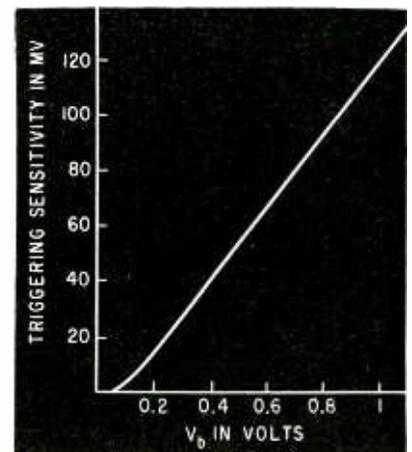
FIG. 5—Threshold sensitivity characteristics of Fig. 4A
