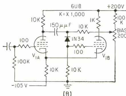
FIG. 4—Examples of sensitive multivibrator design: (A) satisfies stability criterion; (B) is a cathode-coupled version of circuit
