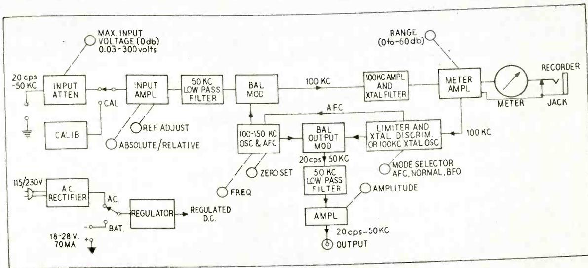
Figure 1. Block diagram, Model 302A Harmonic Wave Analyzer
