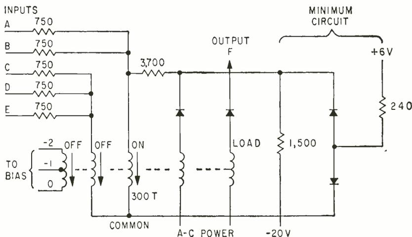
FIG. 1—Multipurpose circuit; the control-winding arrows denote the direction of current flow that produces an ON or OFF effect on the output
