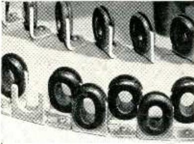
Grommet arrangement. Grommet has been removed from form at left
