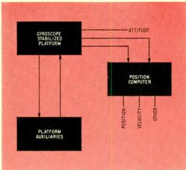
FIG. 12—Basic inertial guidance system necessary to obtain proper velocity vector during initial flight phase
