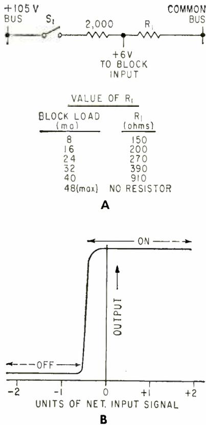
FIG. 2—Input bus circuit to logic circuits (A), saturation curve of magnetic amplifier (B), time-delay circuit (C) and OR block (D)
