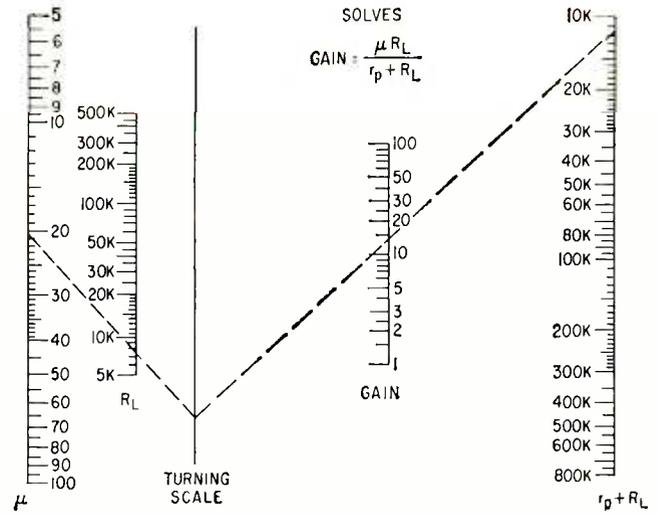
FIG. 4—Triode stage gain nomogram used when amplification factor, load resistor and plate resistance of stage are known
