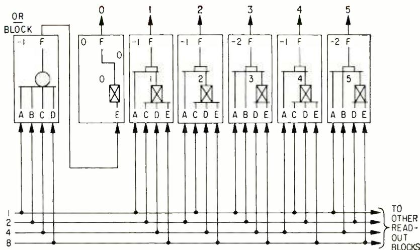
FIG. 6—Outputs of blocks go to indicators such as lights or a printer
