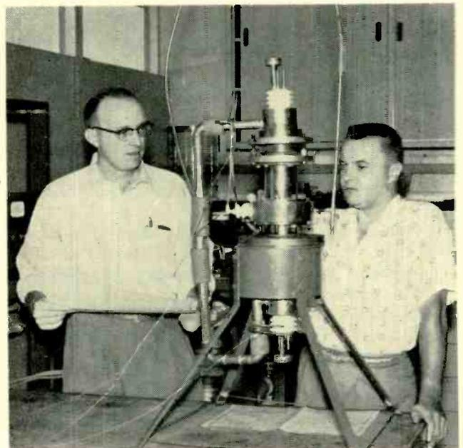
Test chamber for plasma thermocouple is inspected by two of scientists that developed new power generator at University of California's Los Alamos Scientific Laboratory
