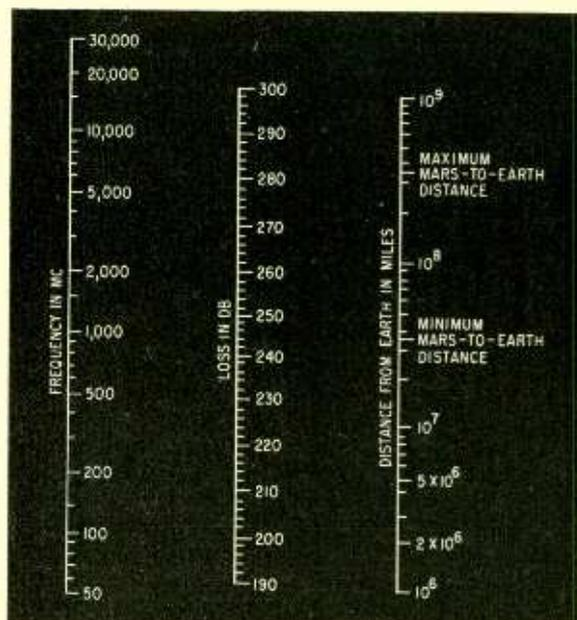
FIG. 5—Nomogram for determination of free-space transmission loss at various distances from Earth
