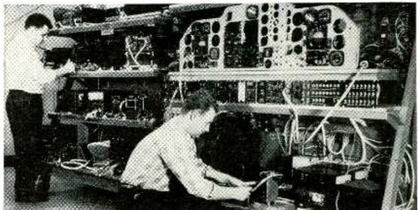
Helicopter's electronic system being "debugged" in mockup before installation in six Sikorsky S-58's soon to be delivered to Coast Guard. Gear includes instruments for all-weather flying, communications and automatic stabilization
