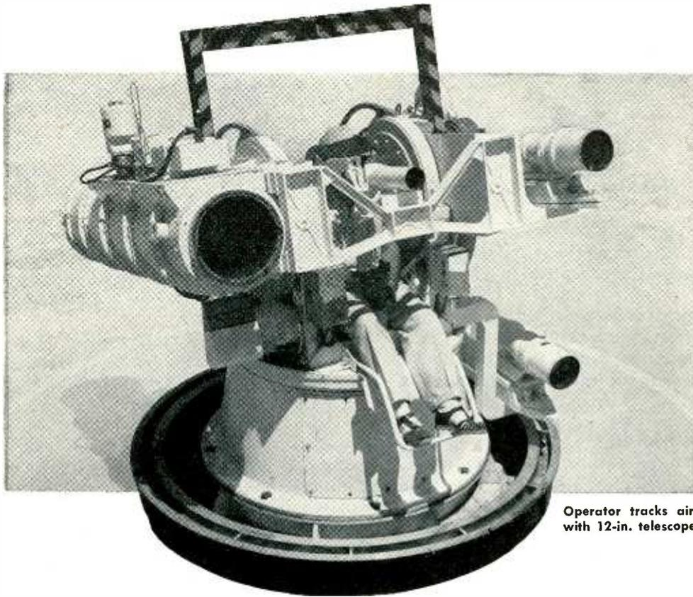
Operator tracks airborne object with 12-in. telescope
