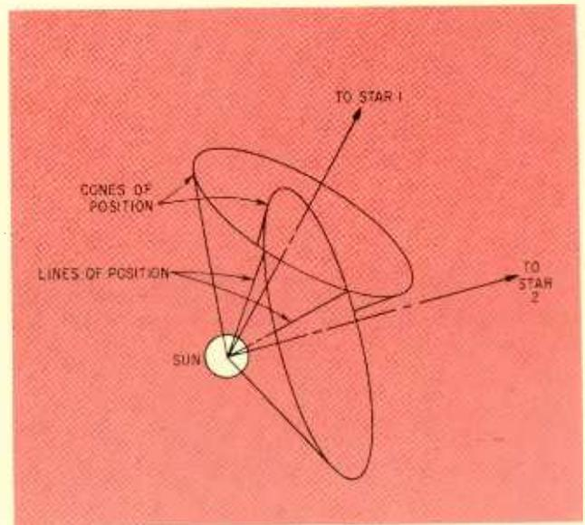
FIG. 13—Position in space along radial component can be fixed from two stars and Sun
