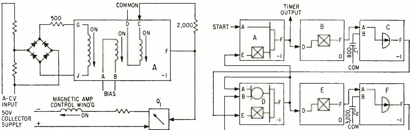
FIG. 5—High-voltage multipurpose block with isolated control winding (left); adjustable timer (right)
