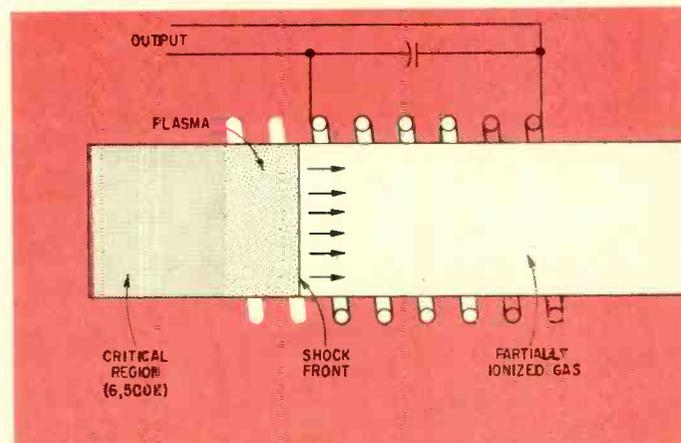
FIG. 15—Plasma-fission reactor would produce electricity directly
