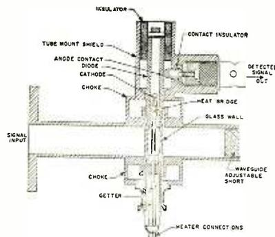
FIG 2—Crossguide diode and mount assembly
