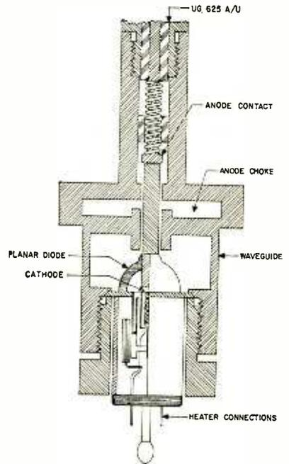
FIG 3—Planar diode and mount assembly
