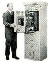
EASY ACCESS—ENTIRE TRANSPORT ASSEMBLY SWINGS OPEN ON STURDY HINGES FOR FULL ACCESS TO ALL COMPONENTS. SPECIALLY DESIGNED REEL MOTORS WITHSTAND INTERNAL TEMPERATURES TO 250°C.
