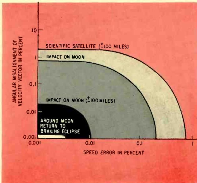
FIG. 10—Maximum permissible errors for angular alignment and magnitude of space vehicle velocity vector at power cutoff
