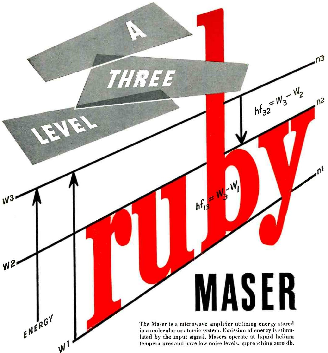
The Maser is a microwave amplifier utilizing energy stored in a molecular or atomic system. Emission of energy is stimulated by the input signal. Masers operate at liquid helium temperatures and have low noise levels, approaching zero db.
