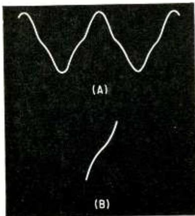
**FIG. 5—Uncompensated amplifier output (A) and transfer characteristic (B)**
