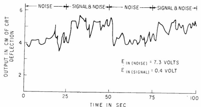
FIG. 4—Experimental waveforms showing actual improvement in signal detectability obtained with crosscorrelator
