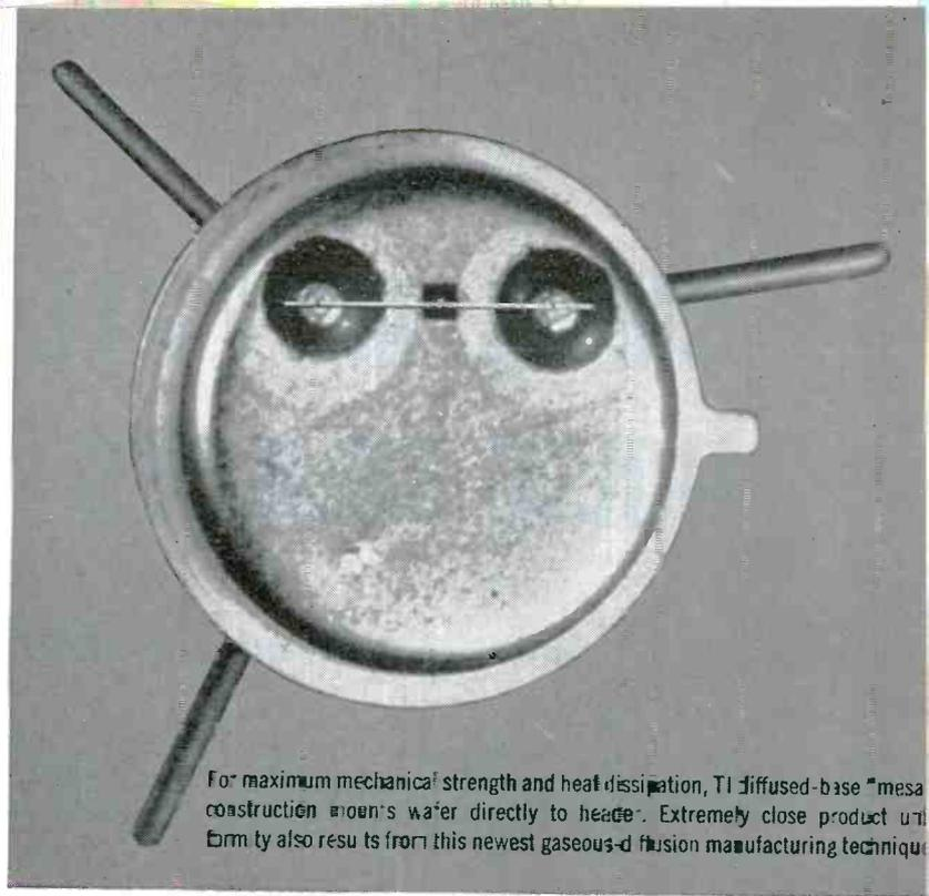
For maximum mechanical strength and heat dissipation, TI diffused-base "mesa" construction mounts wires directly to header. Extremely close product uniformity also results from this newest gaseous-diffusion manufacturing technique.
