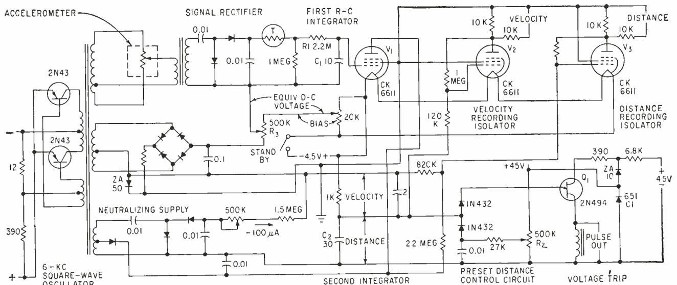
FIG. 2—Unijunction transistor is triggered when accumulated charge on  $C_2$  reaches level analogous to preset distance
