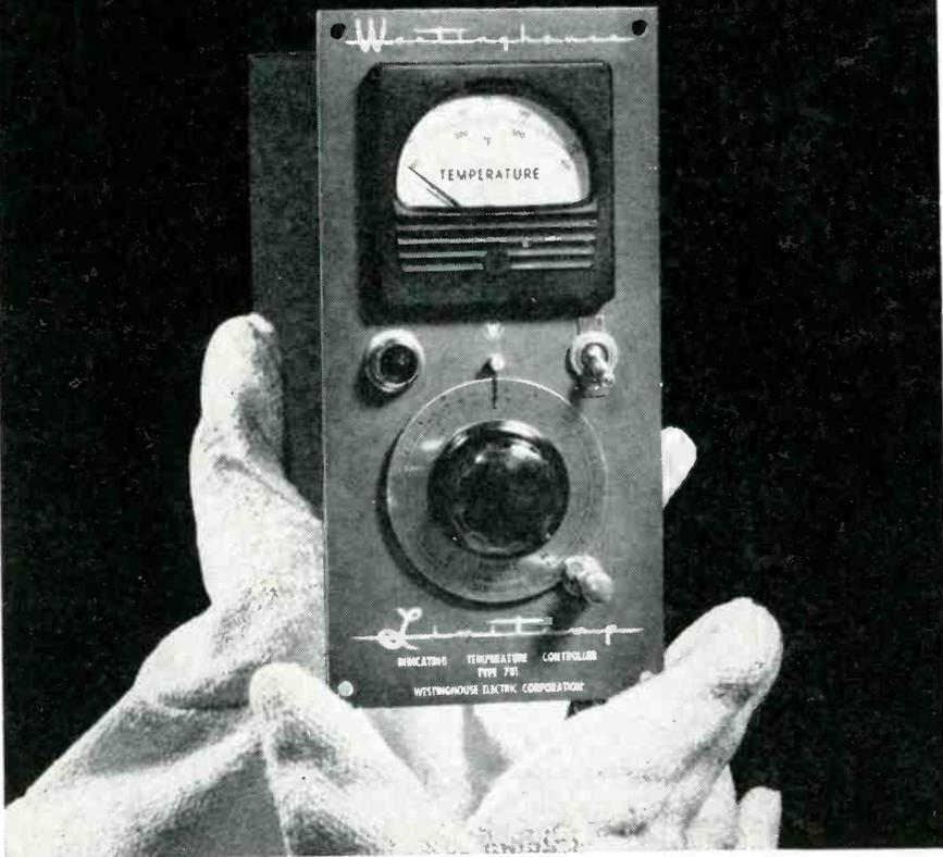
Limitemp\* is a new, medium-priced control device that is ideal for monitoring or controlling temperatures between 100° F and 400° F. Controller may be used to indicate temperature and sound an alarm if temperature exceeds the preset point. A few applications include windings of large rotating machines, bearings, process temperatures and controlling temperatures in critical areas such as nuclear controls.
