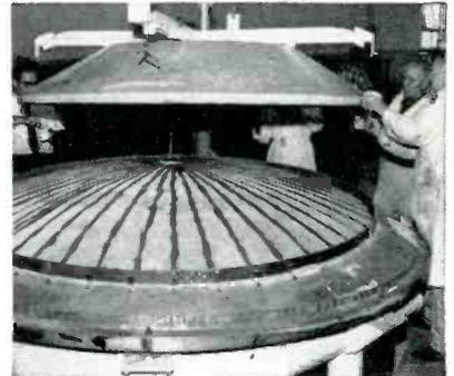
Adhesive on ribs and perimeter readies unit for final assembly
