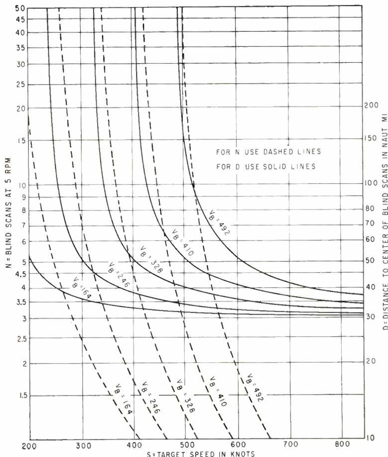
FIG. 1—Chart determines blind speeds and scans within range of expected traffic
