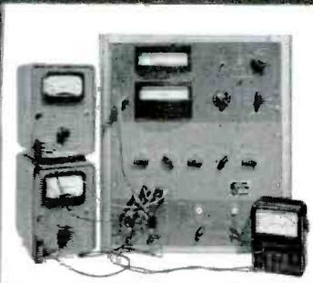
**BEFORE** . . . 3 external instruments were used to measure AC and DC voltage. . . cluttered, tedious, wasteful, subject to error.
