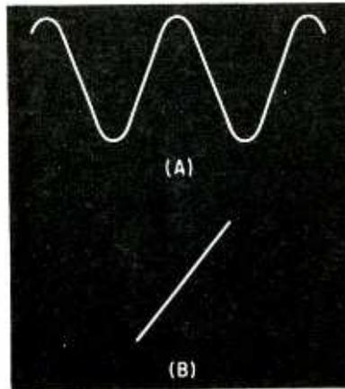
**FIG. 6—Compensated amplifier output (A) and transfer characteristic (B)**
