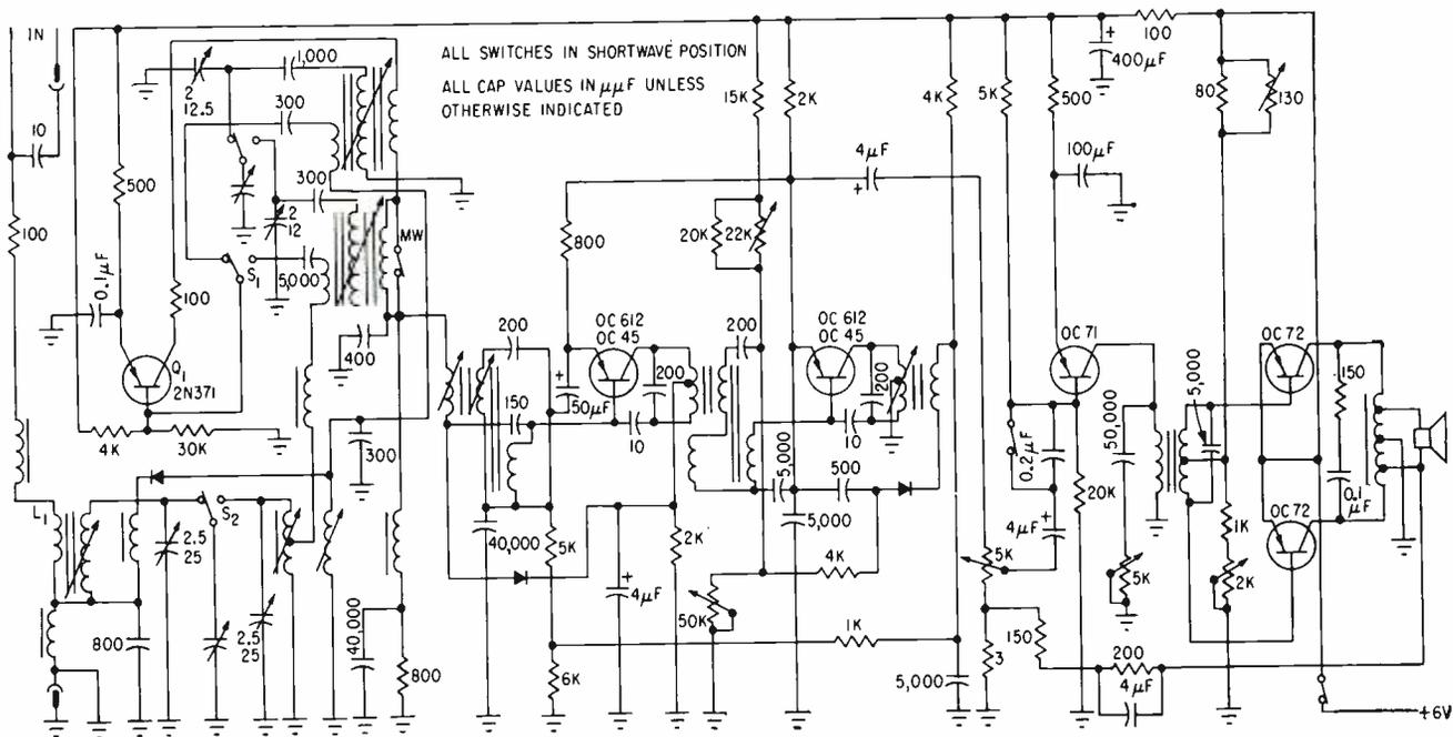
FIG. 2—Short-wave and broadcast-band receiver circuit developed by Loewe, Opta, GmbH uses RCA drift transistors
