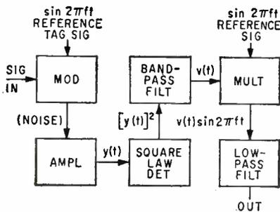
FIG. 2—Dicke radiometer combines received signal with reference signal, then uses duplicate of reference signal to produce large output at filter
