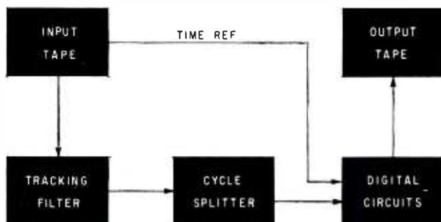
FIG. 2—Block diagram of automatic Doppler cycle counter
