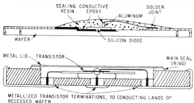
FIG. 1—Preliminary diode and transistor designs
