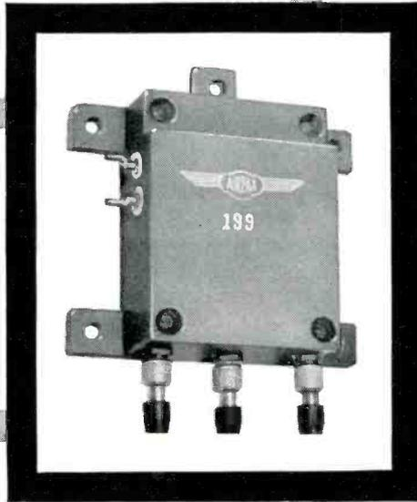
Designed for use in the 100 to 400 megacycle range, the chopper samples two incoming signal sources for a single load or distributes a low level signal to two loads in a periodic manner. Switching frequency is 100 cycles per second.
