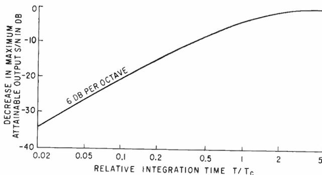
FIG. 3—Attainable signal-to-noise improvement is function of the ratio  $T/T_c$ .
