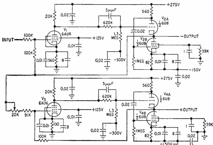
FIG. 7—Wideband driver has low output impedance with balanced output
