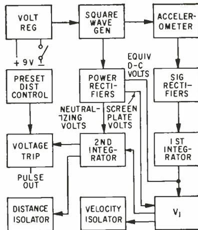
FIG. 1—Two tubes can be added to double integrator to get velocity and distance information for recording
