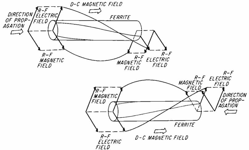
FIG. 1—Direction of rotation for an advancing portion of the wave is clockwise, viewed in the direction of the d-c field irrespective of the direction of wave propagation
