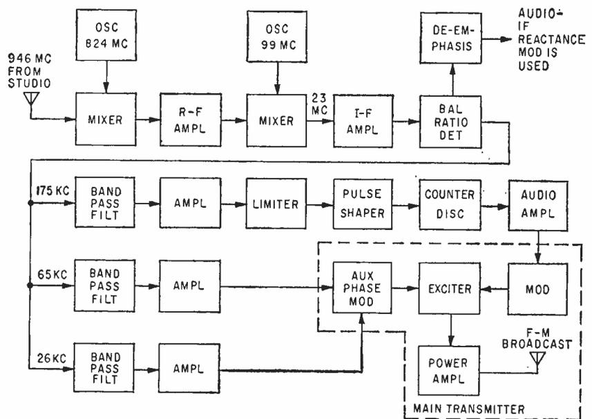
FIG. 2—Mountain-top receiver and main, or broadcast, transmitter. Receiver picks up three programs sent from studio and main transmitter broadcasts them
