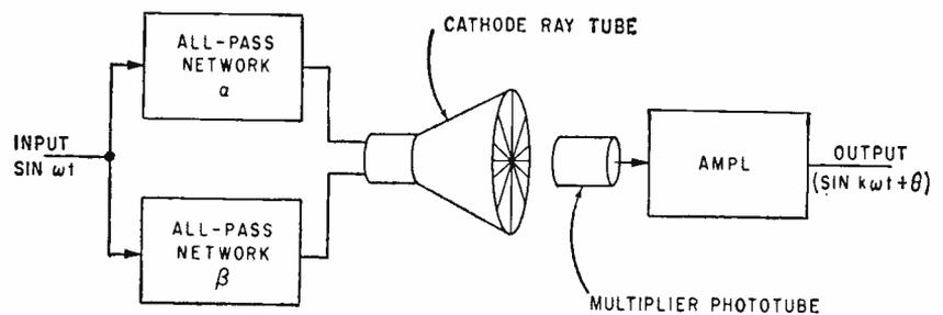
FIG. 5—Cycle-splitter arrangement provides frequency multiplication and digital conversion
