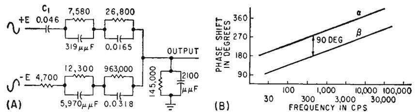
FIG. 6—Networks such as shown in (A) are designed to maintain outputs at close to 90-deg phase difference over wide frequency range. Characteristics are shown in (B)
