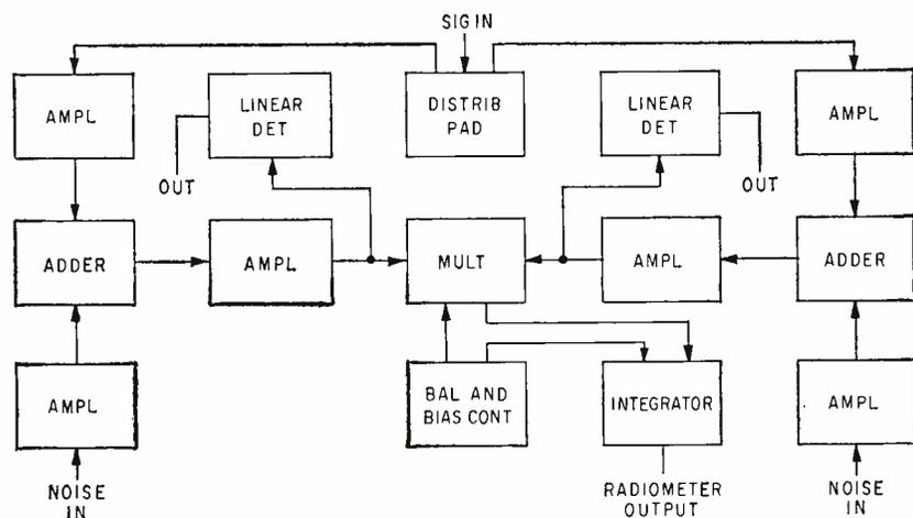
FIG. 5—Simulated two-receiver radiometer used to test agreement with theoretical predictions
