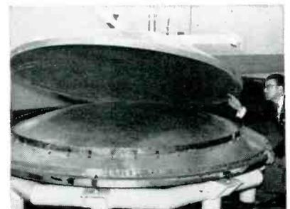
After curing, assembly is lifted off paraboloid face mold
