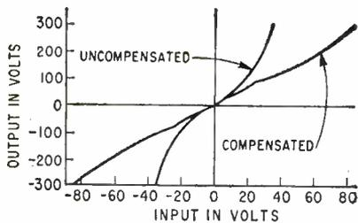
FIG. 3—Comparison of compensated and uncompensated push-pull 6L6 transfer characteristics
