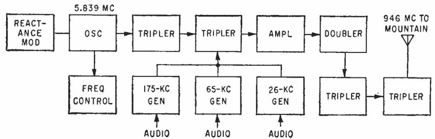
FIG. 1—Studio transmitter. Reactance-tube modulator, formerly used to modulate stl transmitter, now controls oscillator frequency
