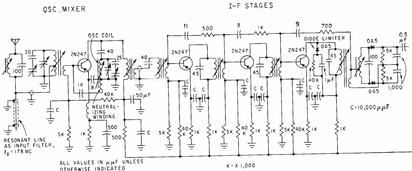
FIG. 3—Very-high-frequency receiver, developed by Graetz Kommanditgesellschaft, Altena (Westfalen). A low value i-f, 6.75 mc, provides
