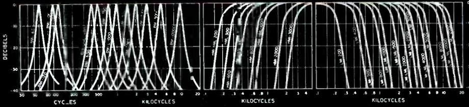
This standardized group of filters covers most popular filter applications and frequencies. Units are in compact, drawn, magnetic shielding cases... 1 1/16 x 1 1/16 base, 1 3/8 high for BMI, LMI, BML; others 2 1/2 high. There are six basic types:
