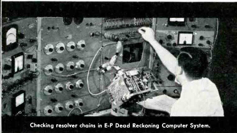
Checking resolver chains in E-P Dead Reckoning Computer System.
