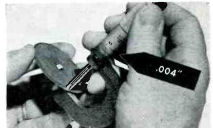
**Diamond-hard, yet paper-thin.** Miking of this Norton diamond cut-off wheel shows an extreme thinness of .004" — a typical result of Norton leadership in developing diamond wheels "tailor-made" to every application for finest results.
