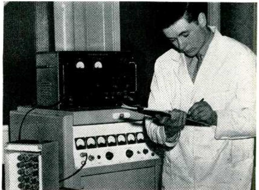
Checking a 40-kc filter bank (on bench at left) with counter accurate to 0.1 cps
