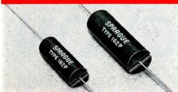
**NEW!**... DIFILM Type 162P slotted-base multi-purpose molded case capacitors for auto radios and other severe vibration applications. Slot prevents collection of moisture around leads when capacitor is end-mounted against chassis.
