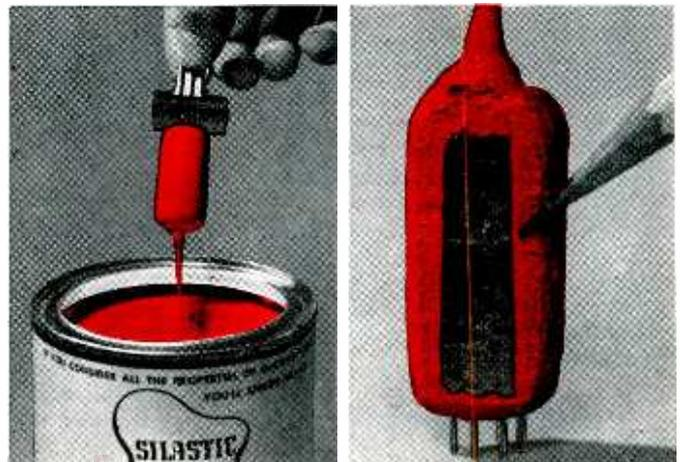
Electronic tube encapsulated with Silastic.
