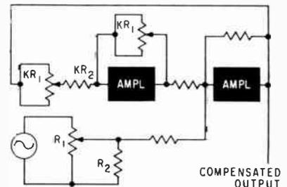
FIG. 5—The general compensation case using operational amplifiers
