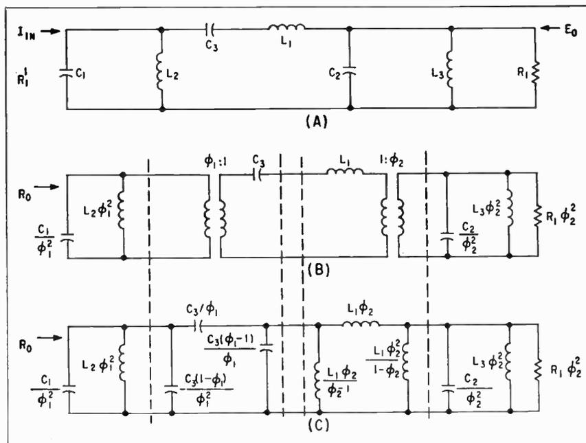
FIG. 1—Triple bandpass filter and equivalent circuits
