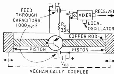
FIG. 3—Basic arrangement for power gain measurement at high frequencies
