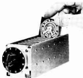
in. by 2 in., 3 in. by 3 in. and 4 in. by 4 in. with lengths to accommodate up to 36 wafers. All connections are to a single bank of receptacles and are conveniently accessible from one side of the aluminum housing. Wafers can be made to include printed circuitry and components in addition to their normal switching function.
