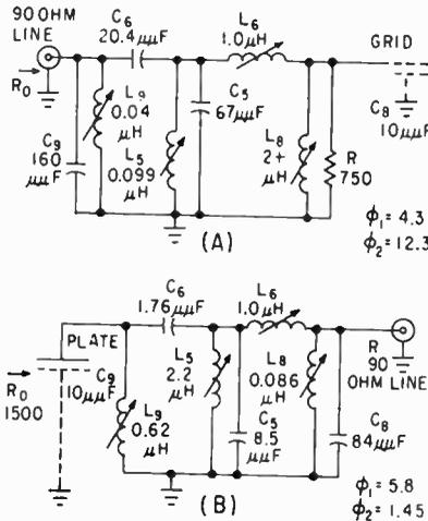
FIG. 3—Transmission from a 90-ohm line to 10- $\mu\mu\text{f}$  grid (A); from a 10- $\mu\mu\text{f}$  plate to a 90-ohm line (B)
