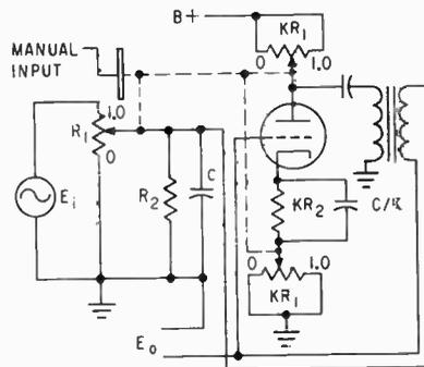
FIG. 4—Compensating for a resistance and capacitance load
