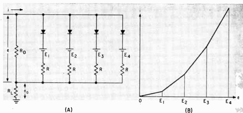
FIG. 4—Fundamental squaring circuit (A) and its operation (B) to produce  $e_{0i} = ki = k'e$
