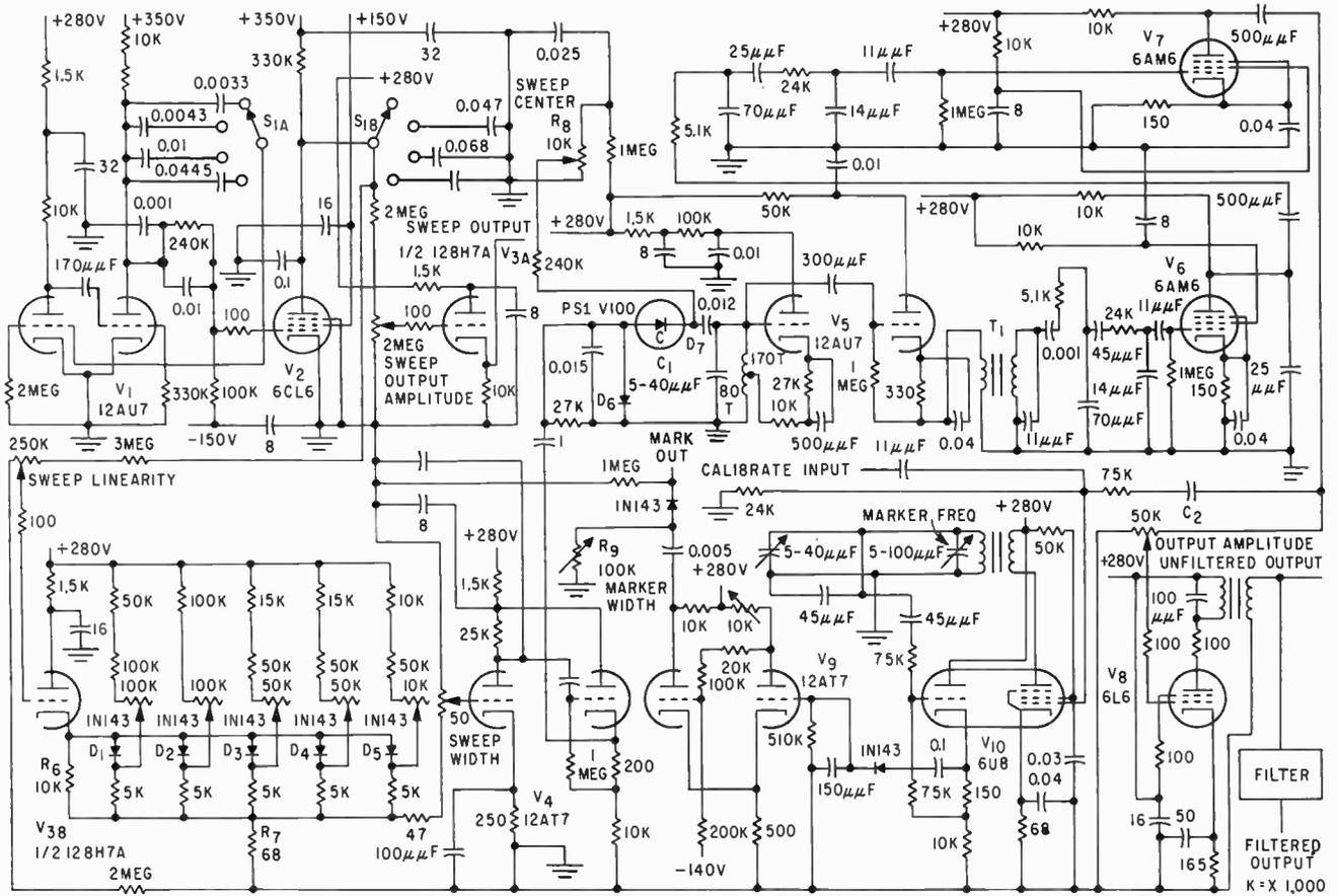
FIG. 3—Oscillator circuit ( $V_6$ ) shows how reverse-biased p-n junction voltage-variable capacitor is used to generate a variable-frequency output. Plate voltage of squarer  $V_3$  must be regulated
