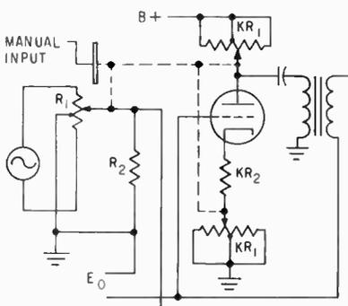
FIG. 3—Error compensation with tapped potentiometers
