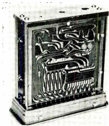
One of the most significant single component developments in building of the computer for the Titan was the use of a sealed chassis. A glass-epoxy copper-clad laminate was chosen for the circuit board material
