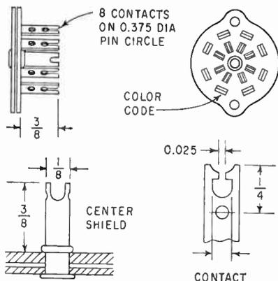
FIG. 1—Tube socket terminal design
