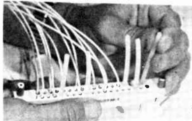
Plastic rods are inserted in plug connector (Burndy PD35M-1)
