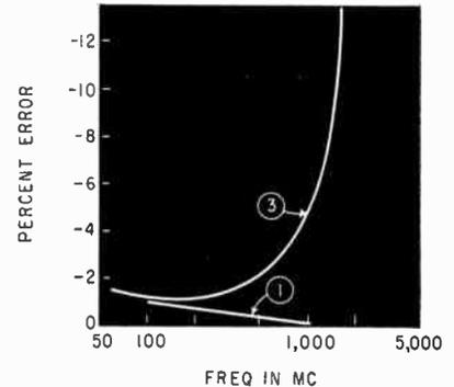
FIG. 6—Error in  $f_{max}$  measurements caused by Q factor in ideal and actual line
