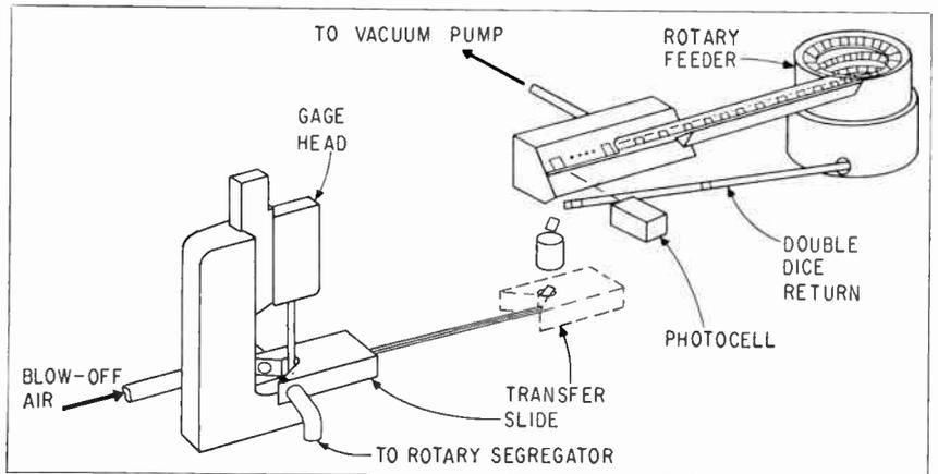
FIG. 1—Basic parts of gaging and sorting mechanism. Vibratory feeder, gravity, cam-operated slide and air blow are used to move dice
