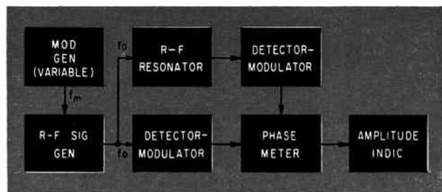
FIG. 1—Test set-up for measurement of resonator Q by observing envelope phase shift
