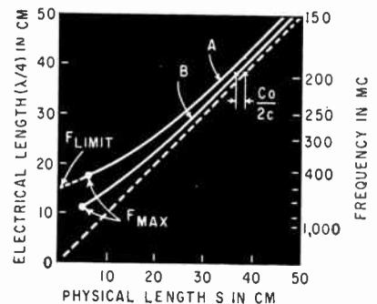
FIG. 4—Relation between electrical and physical length of transmission line. (A) is for 2N501 transistor with 4-cm leads,  $V_e = -15$  v,  $I_c = 5$  ma. Curve (B) is for 2N502 with 0.6-cm leads, same operating parameters
