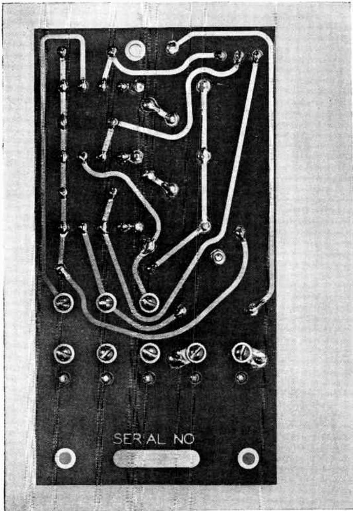
**High strength-to-weight ratio.** This printed wiring board for a phase failure relay (manufactured by Phase-Guard Co., Carnegie, Pa., and distributed by Stradley Engineering Co., Pittsburgh) was designed with CDF Di-Clad 28E (epoxy resin laminated with medium weave glass cloth) for high mechanical strength, very low moisture-absorption, and good insulation resistance. Details upon request.
