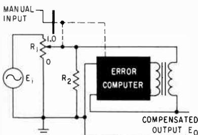
FIG. 1—Loading error is computed and used for compensation
