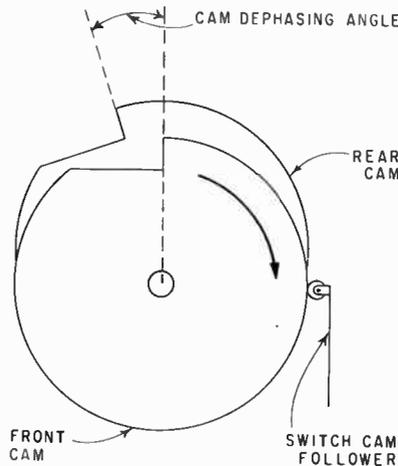
FIG. 1—Cams provide warmup time equal to dephasing angle divided by 360 multiplied by time of one shaft revolution
