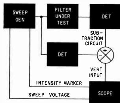
FIG. 5—When the oscilloscope sweep is calibrated in frequency, the characteristics of the filter under test may be observed
