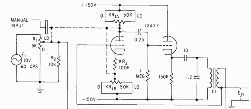
FIG. 2—Practical circuit for error computer reduces loading error 97 percent
