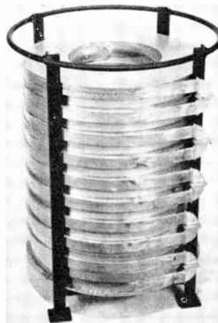
Nineteen-coil waveguide assembly
