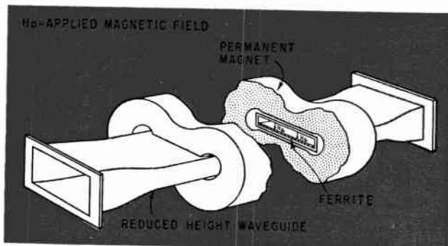
FIG. 2—Method of suppressing unwanted signals in waveguide by use of ferrite slabs magnetized to resonance
