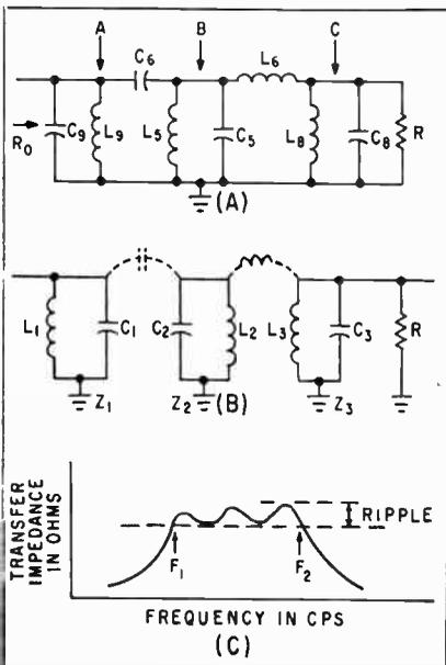
**FIG. 2—Circuit used in conjunction with design box (A), triple-tuned bandpass transformer circuit (B) and frequency response of filters (C)**
