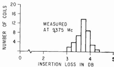
FIG. 1—Distribution of insertion loss values for 40 coiled waveguide sections
