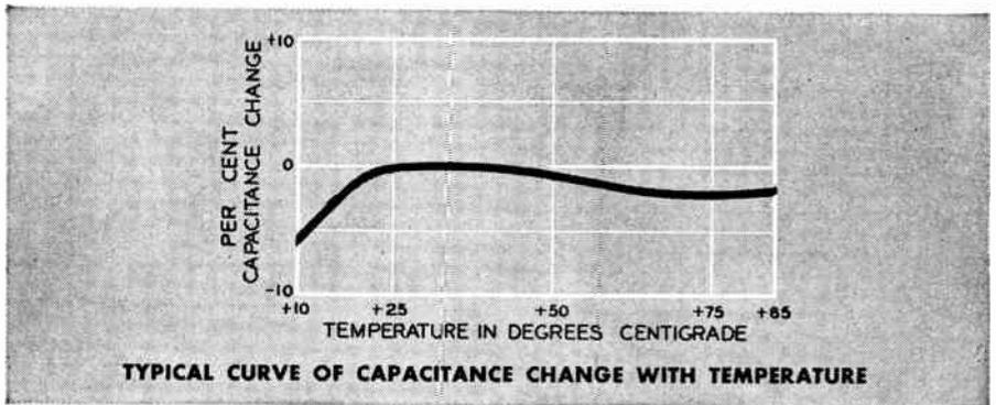
Cera-Mite Capacitors are now available in Formulation 40 from .001 to .02  $\mu$ F, 250, 500 and 1000 volts d-c. Engineering Data Sheets 6106 and 6125 list complete ratings and specifications.
