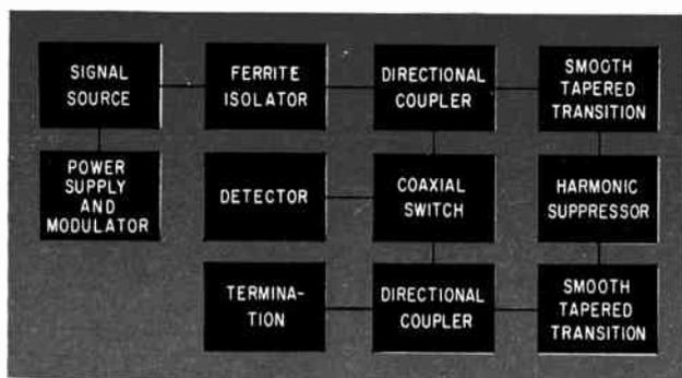
FIG. 3—Low power test setup for measuring effectiveness of spurious frequency suppression
