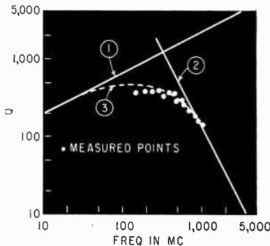
FIG. 5—Q of transmission line as a function of frequency for ideal and actual lines
