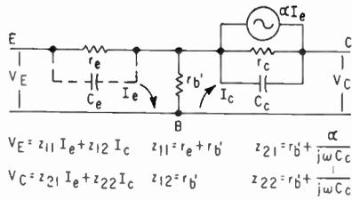
FIG. 1—High-frequency equivalent circuit for a transistor represented as a four-pole tee network
