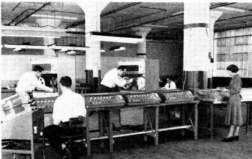
Transactor system gets final inspection at Stromberg Time Corp. factory prior to installation at U.S. Naval Gun Factory, Washington, D.C. Units in foreground gather and instantly transmit information to Compiler (two in background), where it is recorded on punched tape for use of other data-processing equipment
