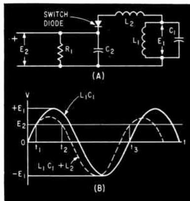
FIG. 1—Fundamental reactance-switch modulator (A) and cycle of operation (B)
