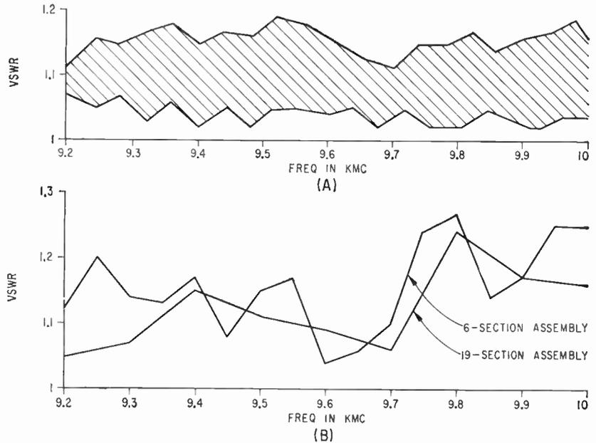
FIG. 2—Frequency in kmc plotted against vswr. Maximum and minimum deviation is given for 40 individual coiled waveguide sections, (A), and for coiled waveguide assemblies, (B)
