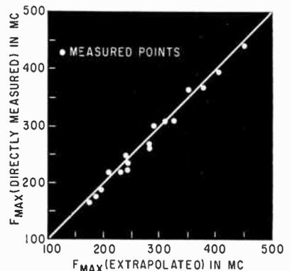
FIG. 8—Correlation of maximum frequency of oscillation values determined by extrapolation and direct measurement
