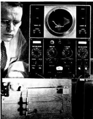
Strain in vibrating beam is plotted against time in upper waveform at same time as beam strain is plotted against acceleration of beam by DuMont dual-beam oscilloscope
